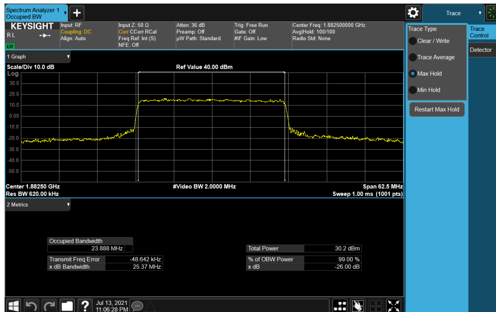
Plot 7-47. Occupied Bandwidth Plot (NR Band n25 - 25.0MHz CP-OFDM 16QAM - Full RB)
