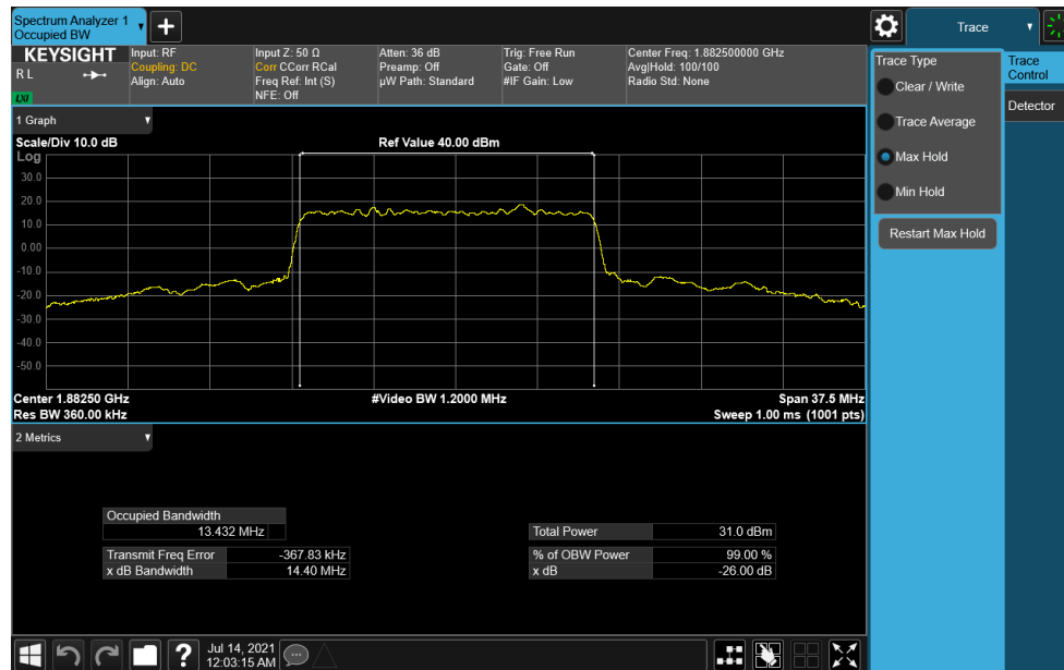
Plot 7-35. Occupied Bandwidth Plot (NR Band n25/n2 - 15.0MHz DFT-s-OFDM \pi/2 BPSK - Full RB)
