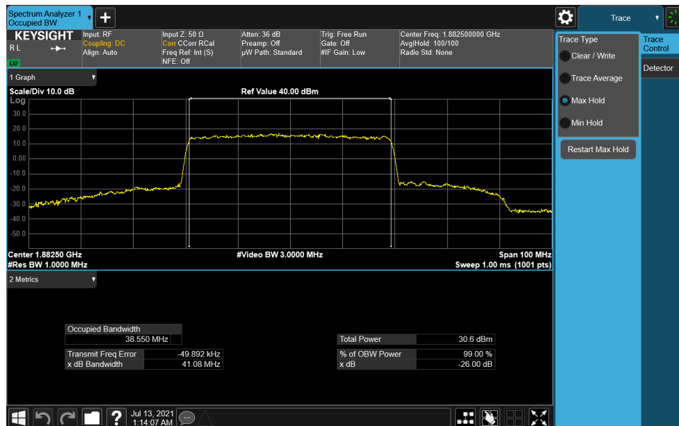
Plot 7-57. Occupied Bandwidth Plot (NR Band n25 - 40.0MHz CP-OFDM 16QAM - Full RB)
