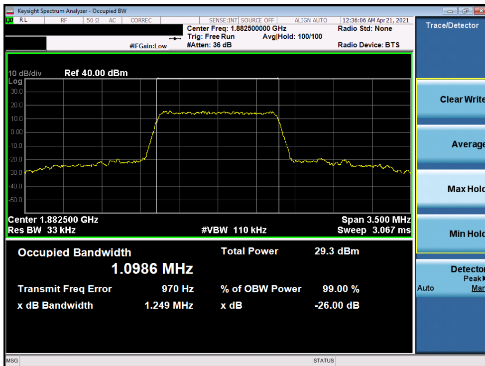
Plot 7-4. Occupied Bandwidth Plot (LTE Band 25/2 - 1.4MHz 256-QAM - Full RB Configuration)
