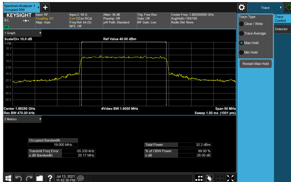
Plot 7-42. Occupied Bandwidth Plot (NR Band n25/n2 - 20.0MHz CP-OFDM 16QAM - Full RB)
