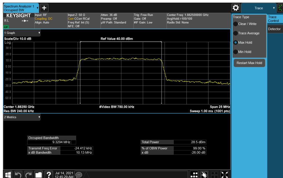
Plot 7-34. Occupied Bandwidth Plot (NR Band n25/n2 - 10.0MHz CP-OFDM 256QAM - Full RB)
