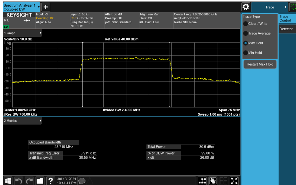
Plot 7-51. Occupied Bandwidth Plot (NR Band n25 - 30.0MHz CP-OFDM QPSK - Full RB)
