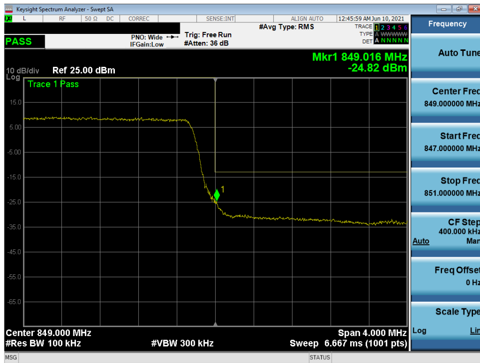
Plot 7-88. Upper BE Plot (LTE Band 5 - 5MHz QPSK – Full RB Configuration)
