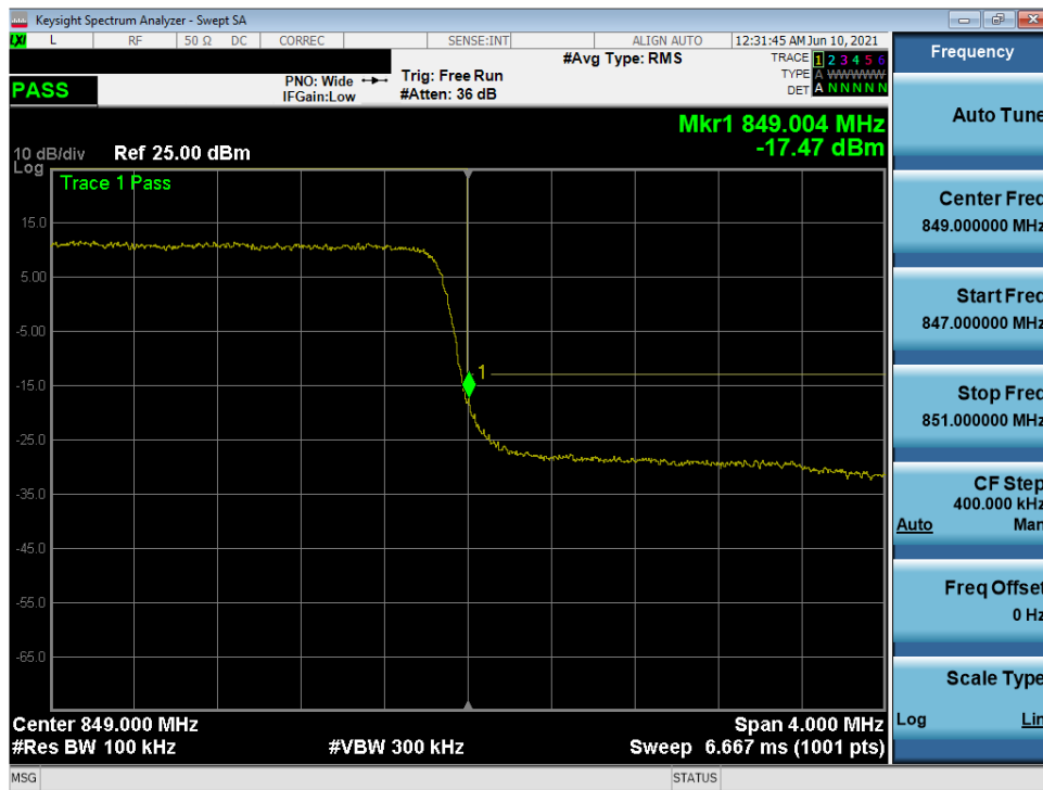
Plot 7-86. Upper BE Plot (LTE Band 5 - 3MHz QPSK – Full RB Configuration)
