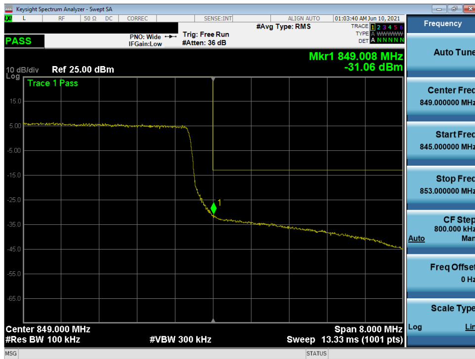
Plot 7-90. Upper BE Plot (LTE Band 5 - 10MHz QPSK – Full RB Configuration)
