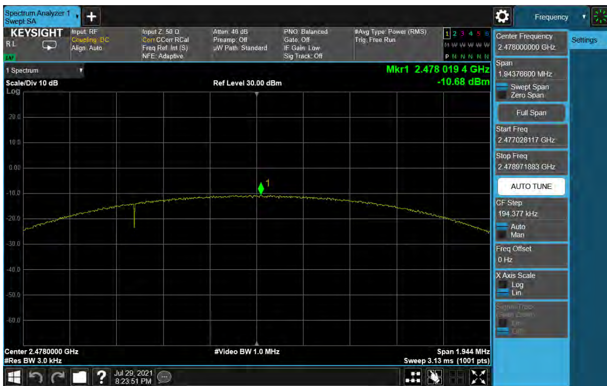
Plot 7-60. Power Spectral Density Plot Antenna WF7 (Bluetooth (LE), 2Mbps, iPA – Ch. 38)
