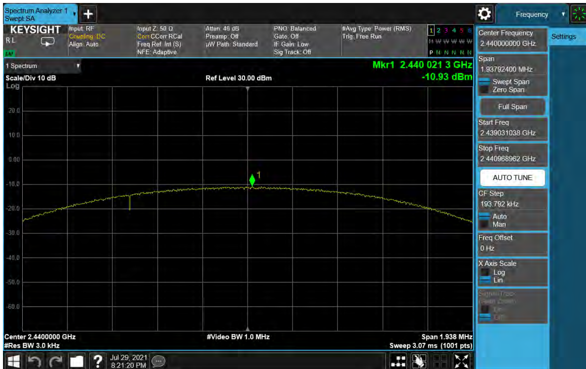
Plot 7-58. Power Spectral Density Plot Antenna WF7 (Bluetooth (LE), 2Mbps, iPA – Ch. 19)
