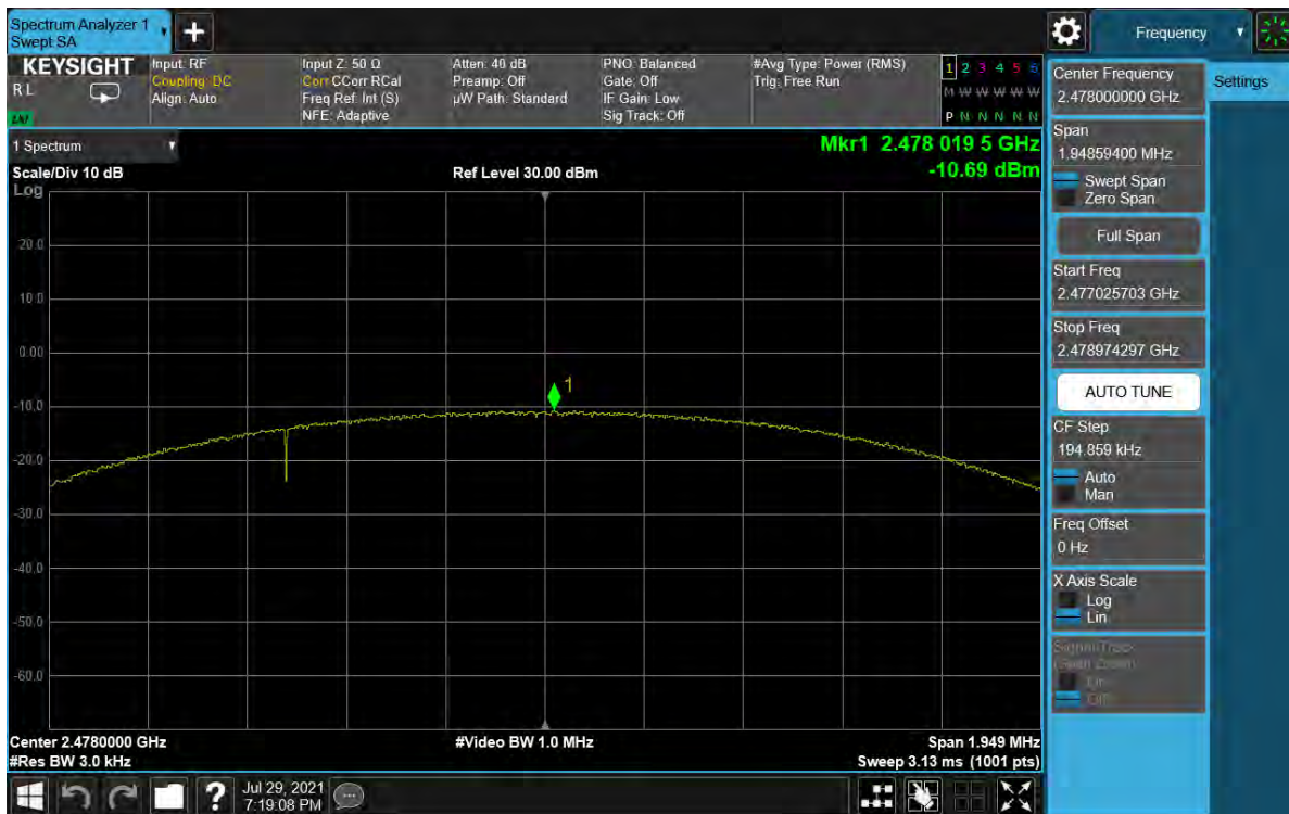
Plot 7-59. Power Spectral Density Plot Antenna WF8 (Bluetooth (LE), 2Mbps, iPA – Ch. 38)
