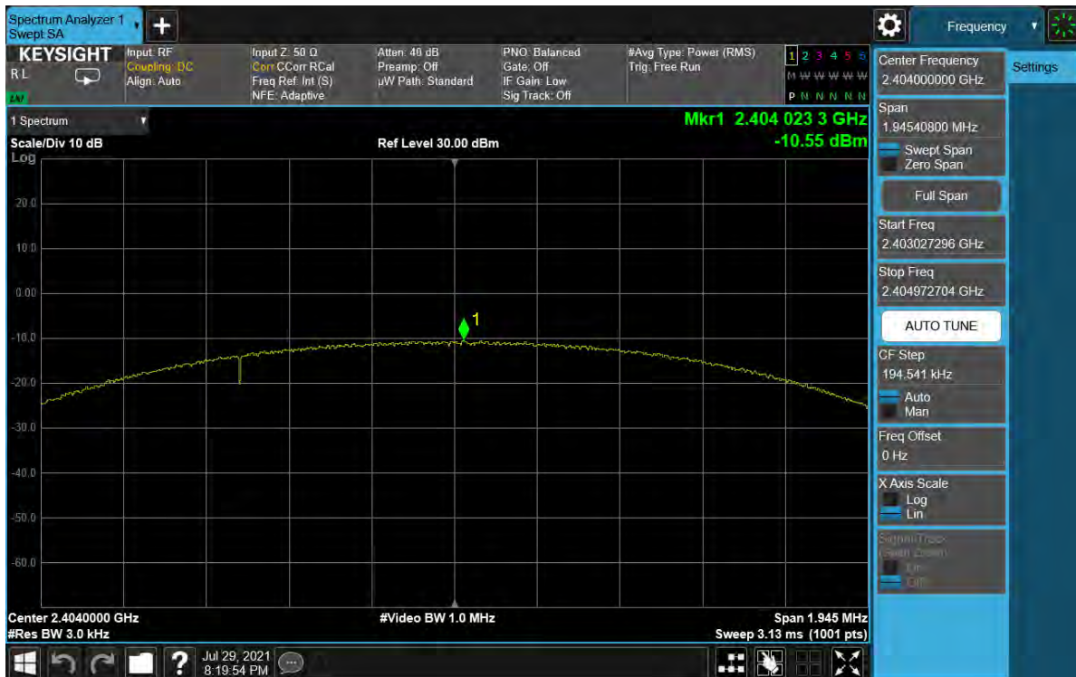
Plot 7-56. Power Spectral Density Plot Antenna WF7 (Bluetooth (LE), 2Mbps, iPA – Ch. 1)
