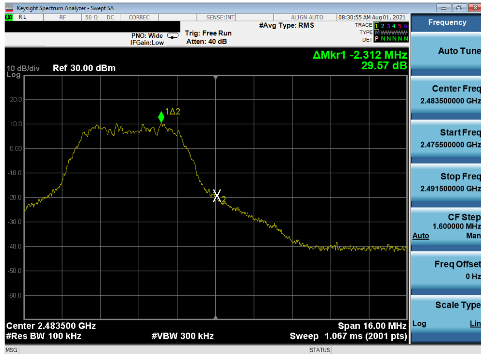
Plot 7-64. Band Edge Plot Antenna WF8 (Bluetooth (HDR8), ePA – Ch. 73)
