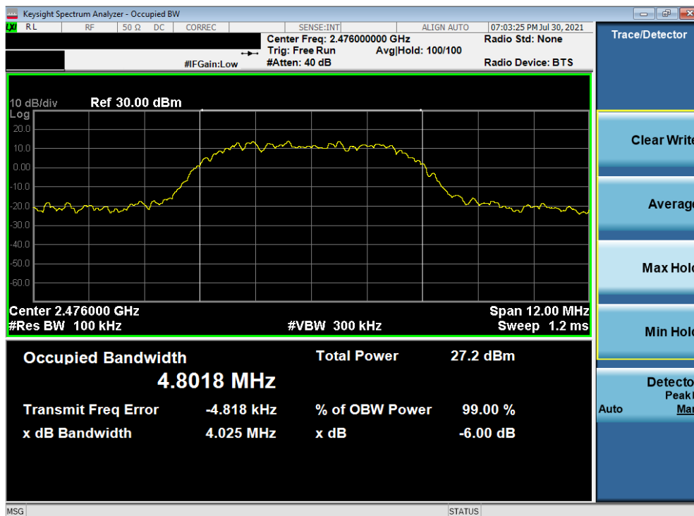
Plot 7-12. 6dB BW & 99% OBW Plot Antenna WF7 (Bluetooth (HDR8), 8Mbps, ePA – Ch. 73)
