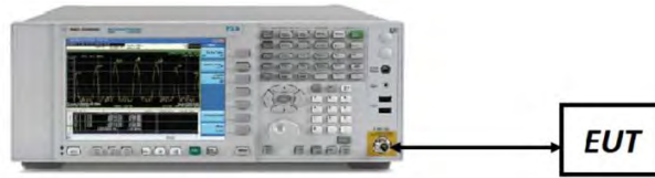
Figure 7-1. Test Instrument & Measurement Setup
