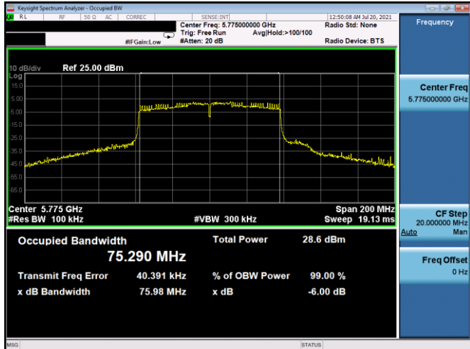
Plot 7-131. 6dB BW & 99% OBW Antenna WF2 (80MHz BW 802.11ac – Ch. 155, MCS2)
