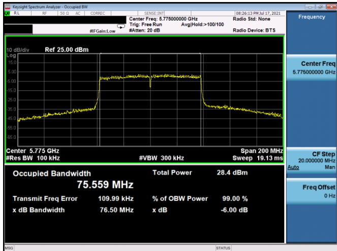
Plot 7-143. 6dB BW & 99% OBW Antenna WF2 (80MHz BW 802.11ac – Ch. 155, MCS5)
