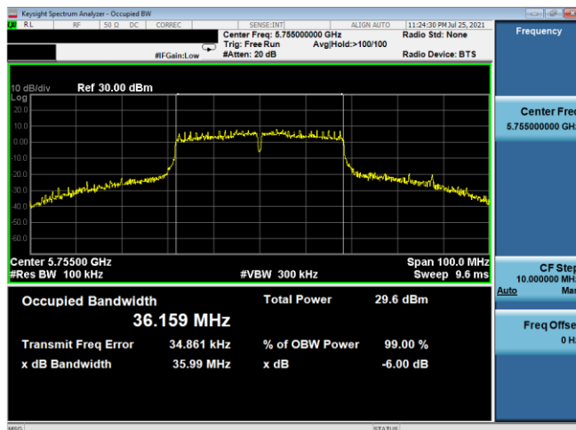
Plot 7-135. 6dB BW & 99% OBW Antenna WF2 (40MHz BW 802.11n – Ch. 151, MCS3)
