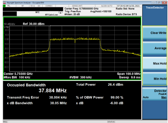
Plot 7-130. 6dB BW & 99% OBW Antenna WF5T (40MHz BW 802.11ax(SU) – Ch. 151, MCS2)
