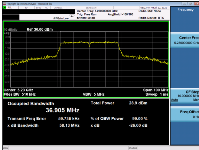
Plot 7-93. 26dB BW & 99% OBW Antenna WF2 (40MHz BW 802.11n – Ch. 46, MCS5)
