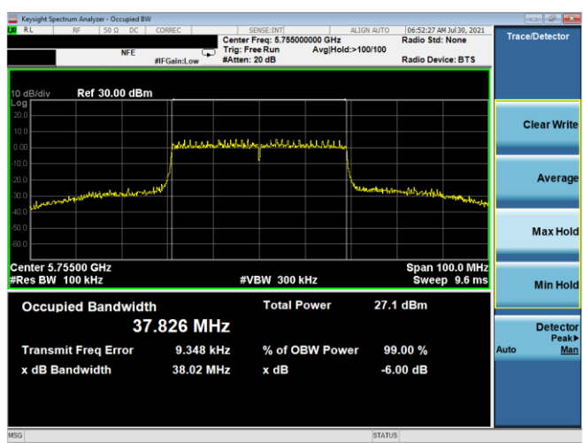
Plot 7-112. 6dB BW & 99% OBW Antenna WF5T (40MHz BW 802.11ax(SU) – Ch. 151, MCS2)
