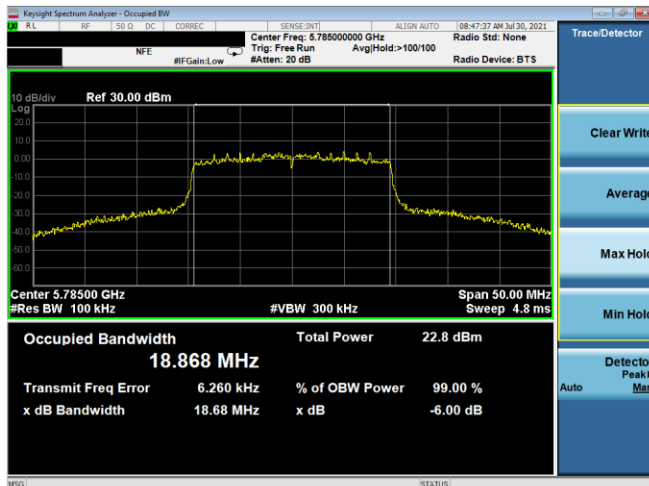
Plot 7-116. 6dB BW & 99% OBW Antenna WF5T (20MHz BW 802.11ax(SU) – Ch. 157, MCS3)
