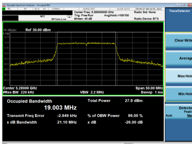
Plot 7-98. 26dB BW & 99% OBW Antenna WF2 (20MHz BW 802.11ax(SU) – Ch. 56, MCS5)
