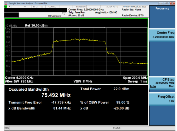
Plot 7-29. 26dB BW & 99% OBW Antenna WF5T (80MHz BW 802.11ac – Ch. 58, MCS3)
