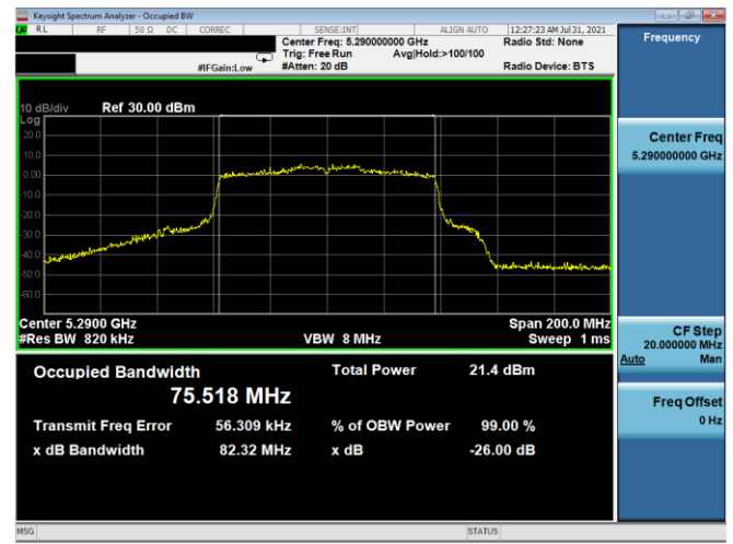
Plot 7-11. 26dB BW & 99% OBW Antenna WF5T (80MHz BW 802.11ac – Ch. 58, MCS2)
