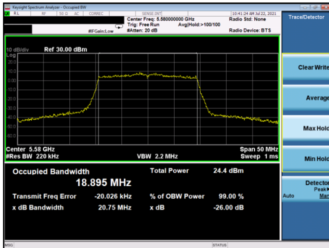
Plot 7-50. 26dB BW & 99% OBW Antenna WF5T (20MHz BW 802.11ax(SU) – Ch. 116, MCS5)
