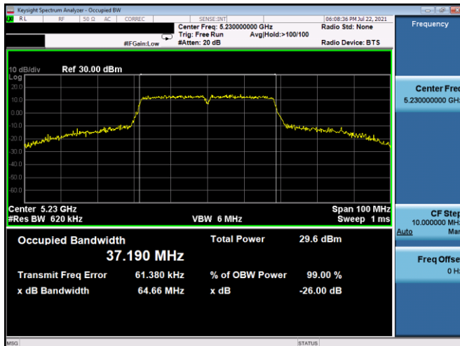
Plot 7-39. 26dB BW & 99% OBW Antenna WF5T (40MHz BW 802.11n – Ch. 46, MCS5)
