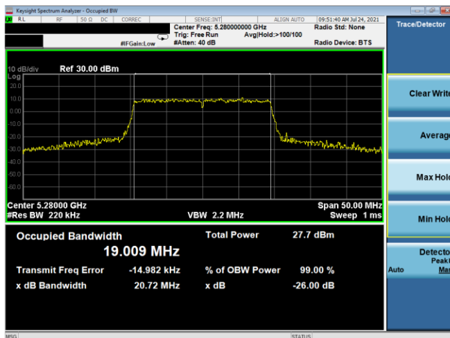
Plot 7-44. 26dB BW & 99% OBW Antenna WF5T (20MHz BW 802.11ax(SU) – Ch. 56, MCS5)
