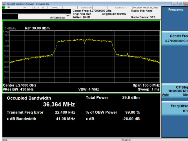
Plot 7-27. 26dB BW & 99% OBW Antenna WF5T (40MHz BW 802.11n – Ch. 54, MCS3)
