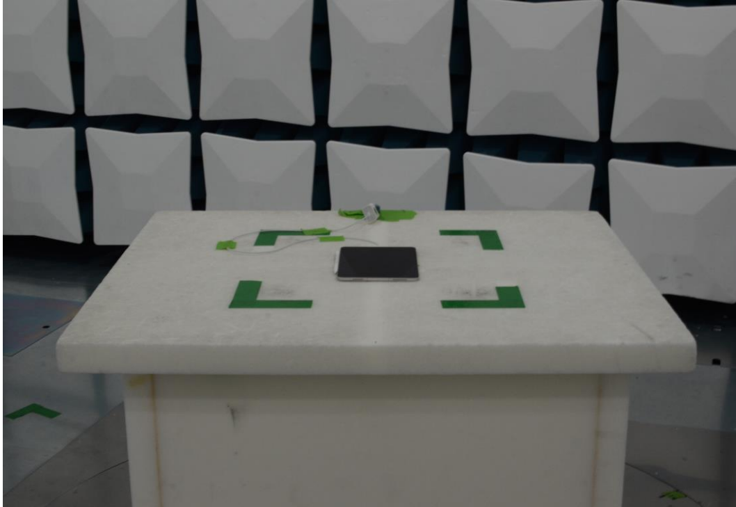
Figure 11: 30MHz-1GHz Test Setup (Front View)
