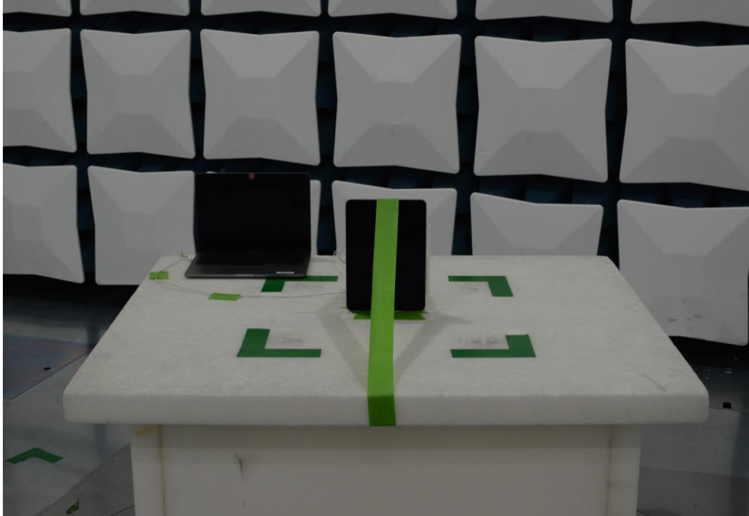
Figure 21: 30MHz-1GHz Test Setup (Front View)
