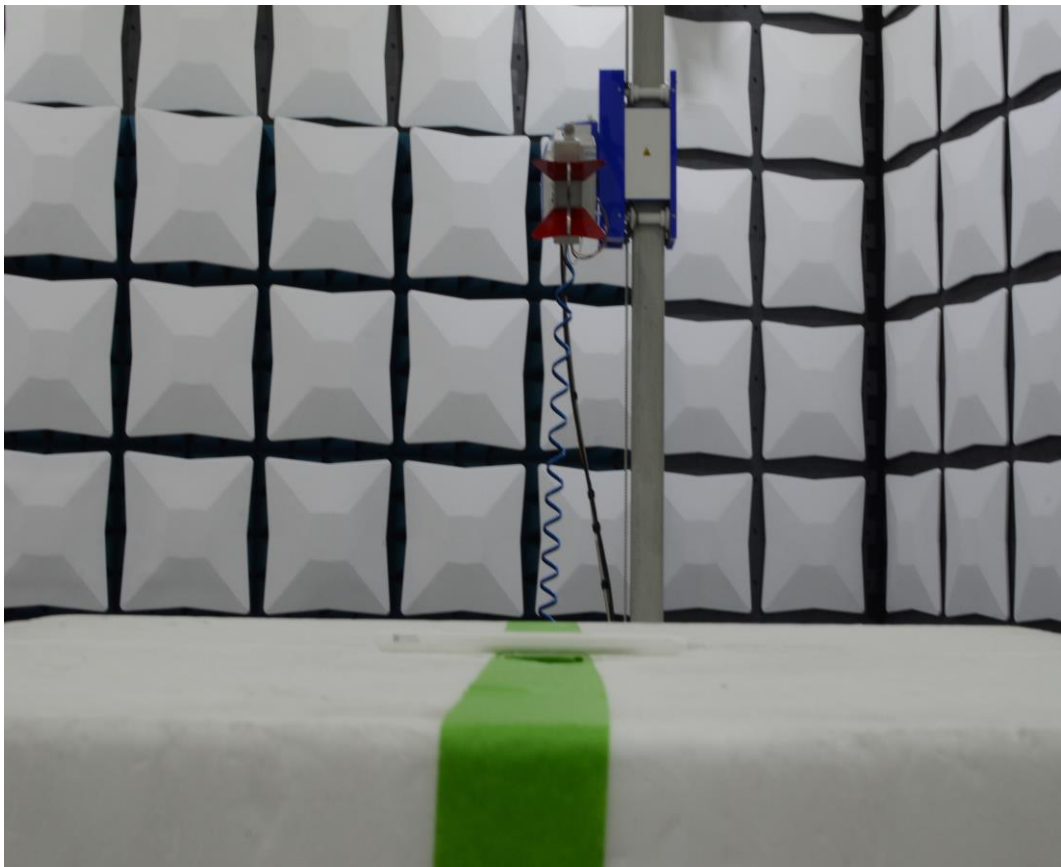
Figure 8: 1-18GHz Test Setup (Rear View)
