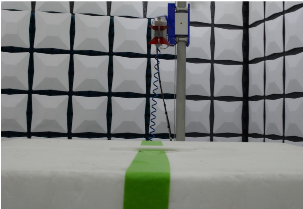
Figure 6: 1-18GHz Test Setup (Rear View)
