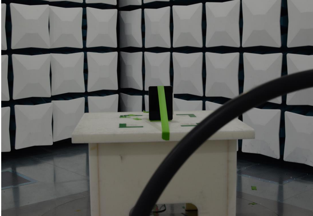
Figure 25: 9kHz-30MHz Test Setup (Front View)
