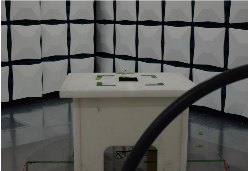
Figure 23: 9kHz-30MHz Test Setup (Front View)
