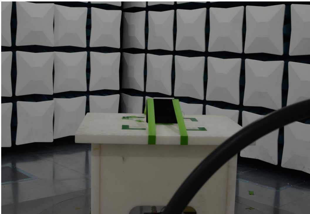
Figure 24: 9kHz-30MHz Test Setup (Front View)
