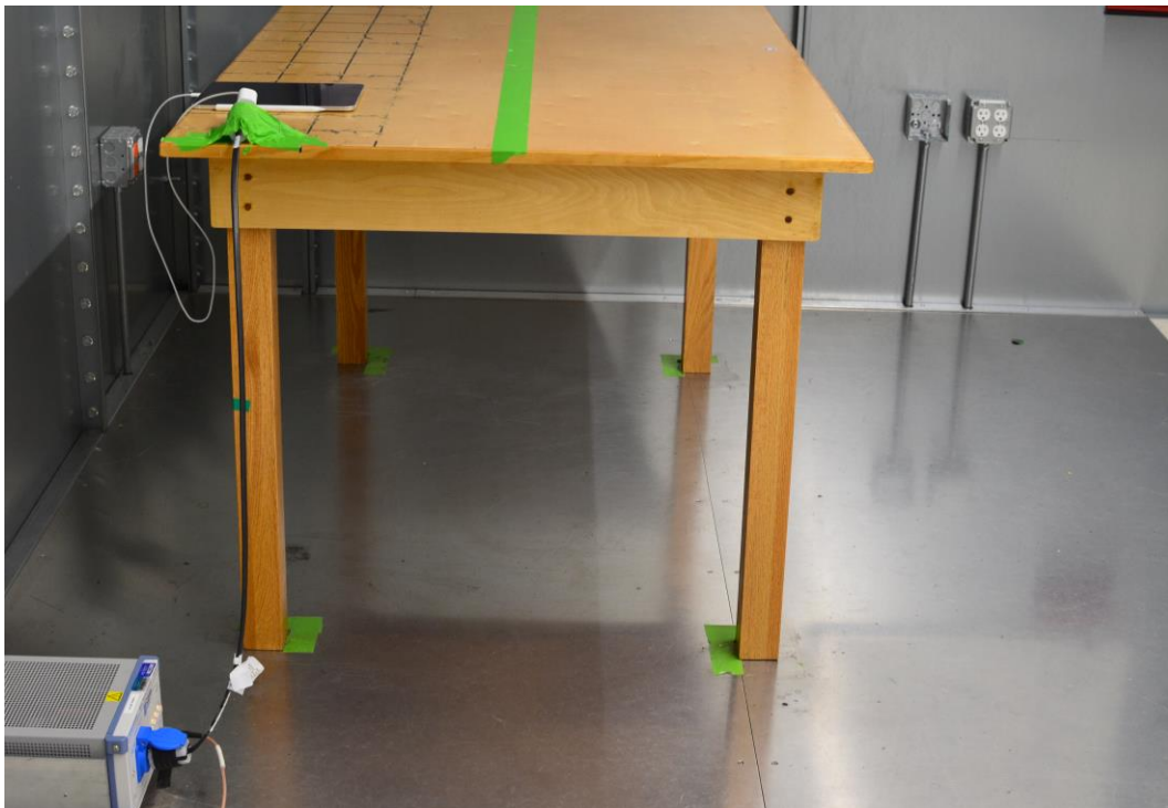
Figure 2: AC Line Conducted Emissions (Side View)
