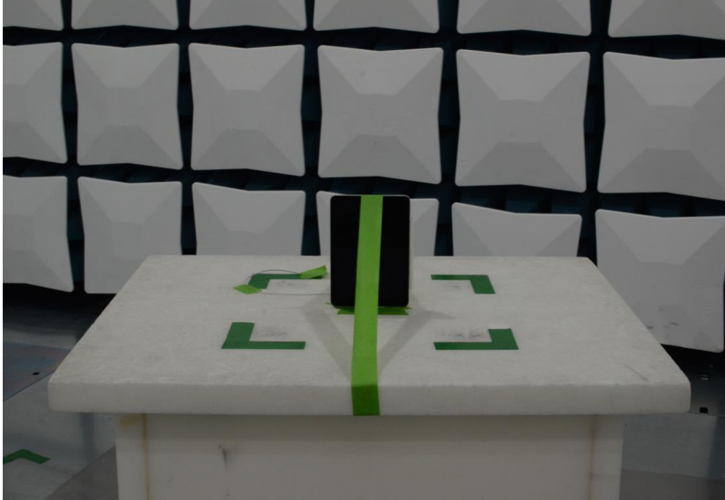
Figure 15: 30MHz-1GHz Test Setup (Front View)
