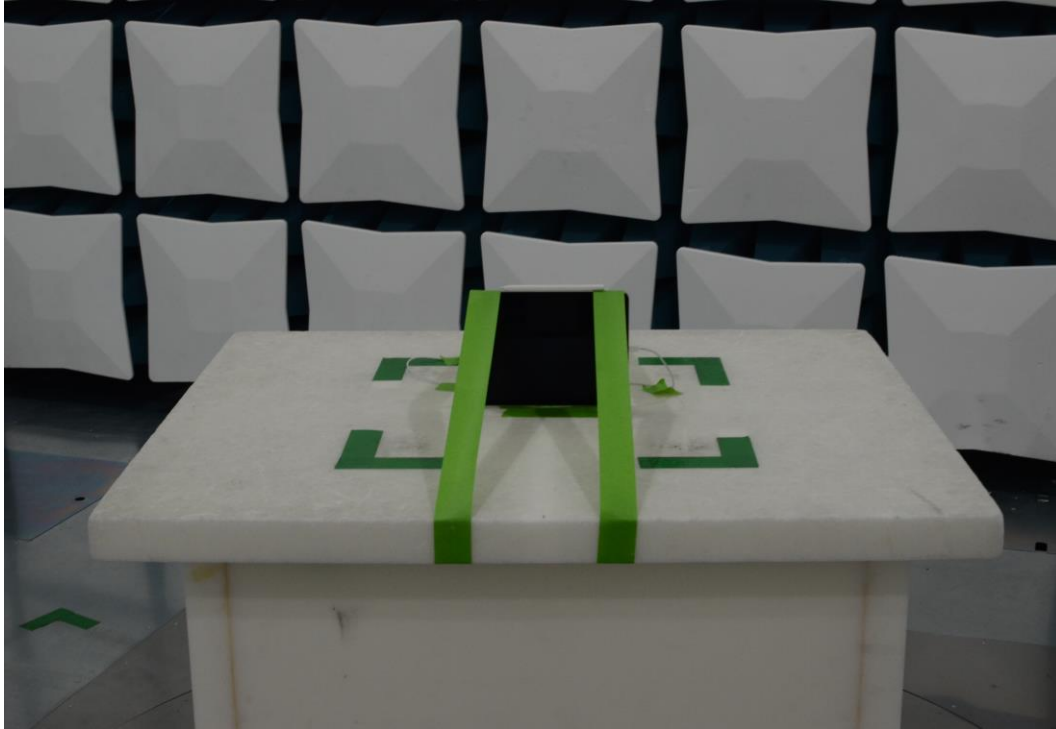
Figure 13: 30MHz-1GHz Test Setup (Front View)
