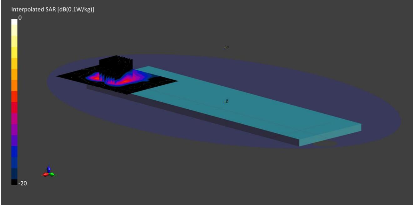
Communication System: IEEE 802.15.1 Bluetooth (GFSK, DH1) UID: 10030; Frequency: 2480.0 MHz; Duty Cycle: 0.31; Medium: HSL; Site63\_25Mar2021\_183051\_Head - 2450 5%; Medium parameters used:  $f = 2480.0$  MHz;  $\sigma = 1.77$  S/m;  $\epsilon_r = 38.9$ ;  $\rho = 1000$  kg/m<sup>3</sup>;  $\Delta\epsilon_r = -0.77$  %;  $\Delta\sigma = -3.52$  %; No correction
