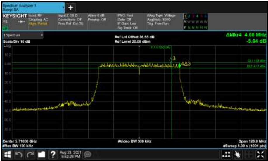
Figure 858 - Core 1 (B) 5710 MHz (CH142) 6 dB Bandwidth
