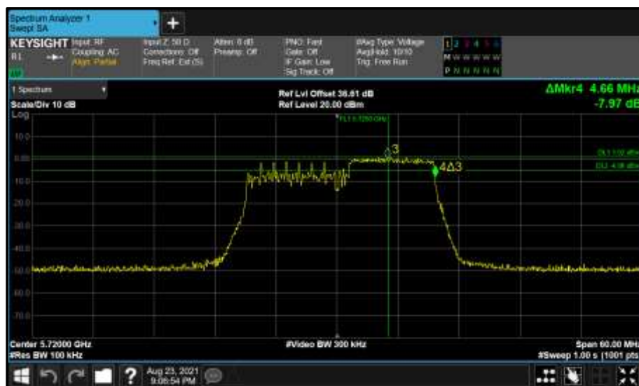
Figure 820 - Core 1 (B) 5720 MHz (CH144) 6 dB Bandwidth
