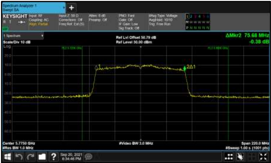
Figure 933 - Core 1 (B) 5775 MHz (CH155) 99% Bandwidth
