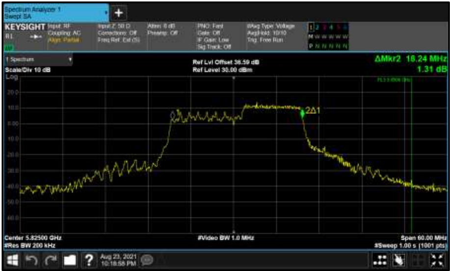
Figure 831 - Core 1 (B) 5825 MHz (CH165) 99% Bandwidth
