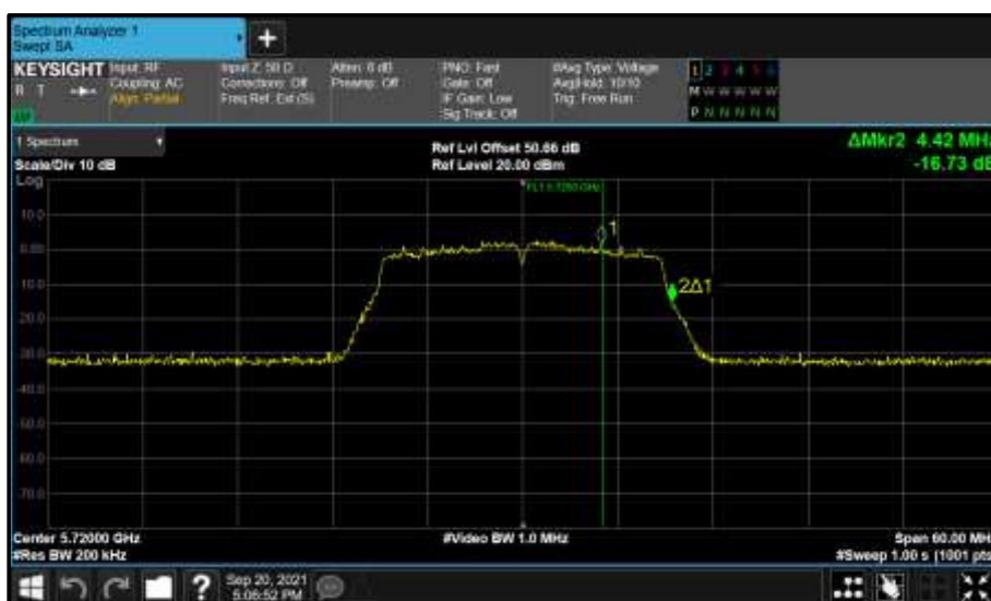
Figure 901 - Core 1 (B) 5720 MHz (CH144) 99% Bandwidth
