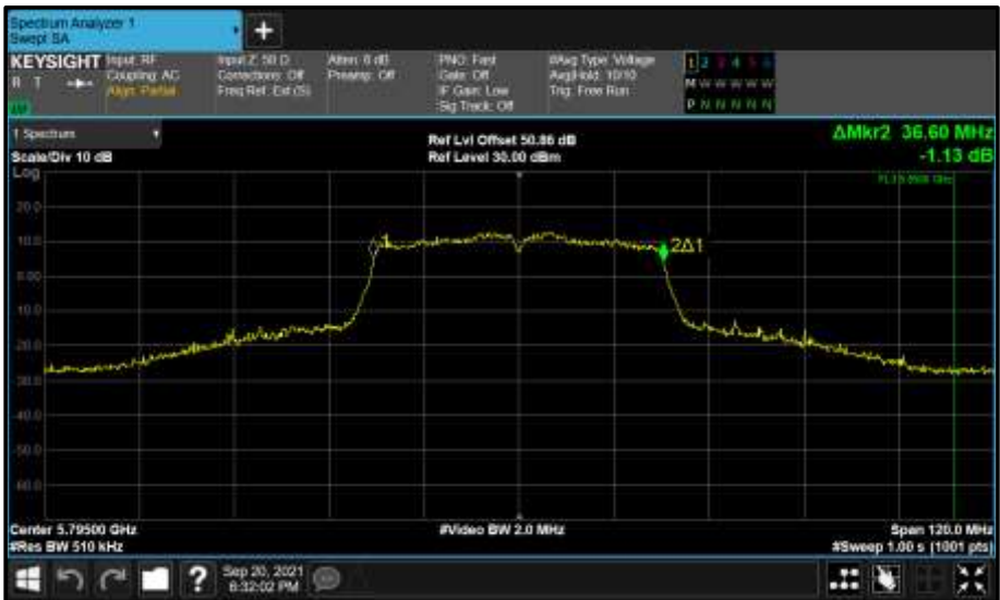
Figure 925 - Core 1 (B) 5795 MHz (CH159) 99% Bandwidth
