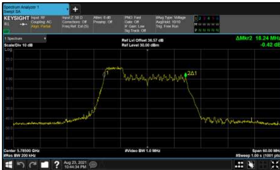
Figure 801 - Core 0 (A) 5785 MHz (CH157) 99% Bandwidth
