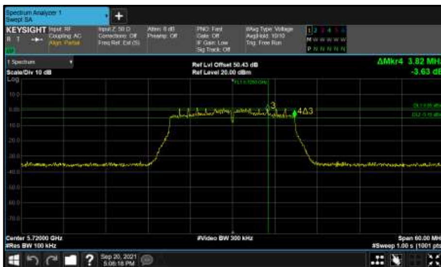
Figure 900 - Core 0 (A) 5720 MHz (CH144) 6 dB Bandwidth
