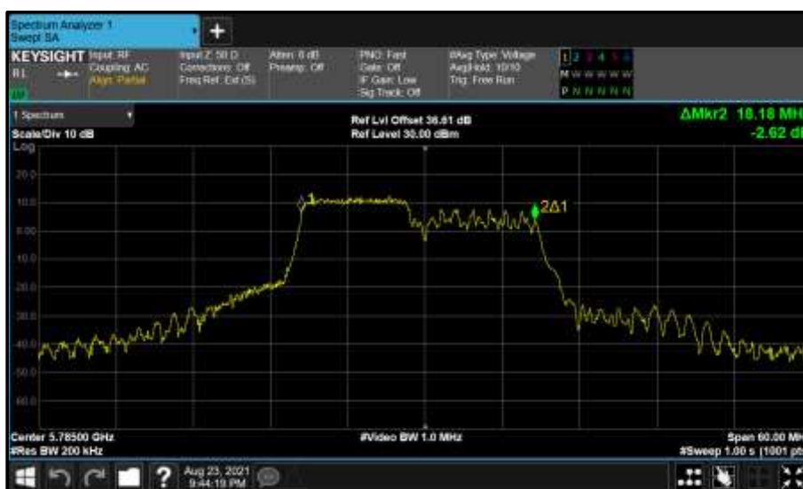
Figure 813 - Core 1 (B) 5785 MHz (CH157) 99% Bandwidth
