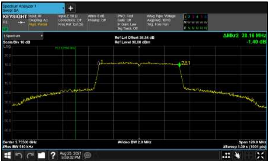
Figure 859 - Core 0 (A) 5755 MHz (CH151) 99% Bandwidth
