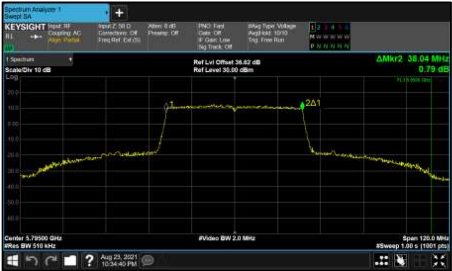
Figure 877 - Core 1 (B) 5795 MHz (CH159) 99% Bandwidth
