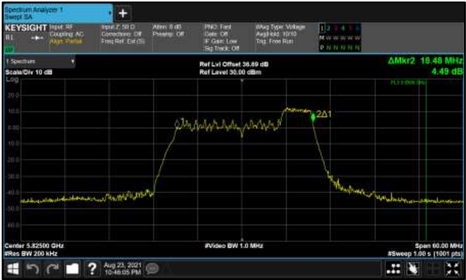
Figure 805 - Core 0 (A) 5825 MHz (CH165) 99% Bandwidth
