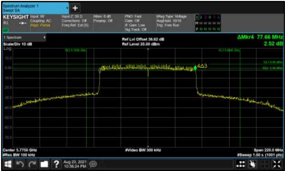
Figure 898 - Core 1 (B) 5775 MHz (CH155) 6 dB Bandwidth
