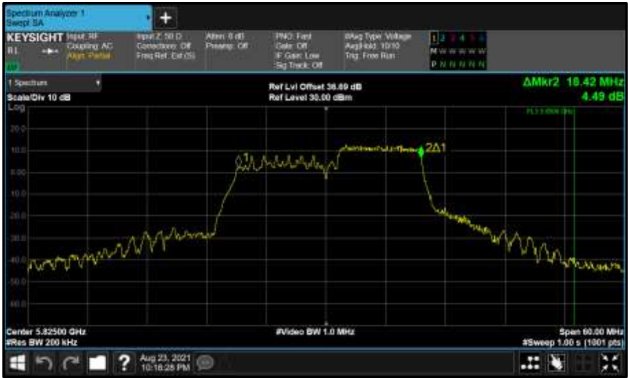
Figure 829 - Core 0 (A) 5825 MHz (CH165) 99% Bandwidth
