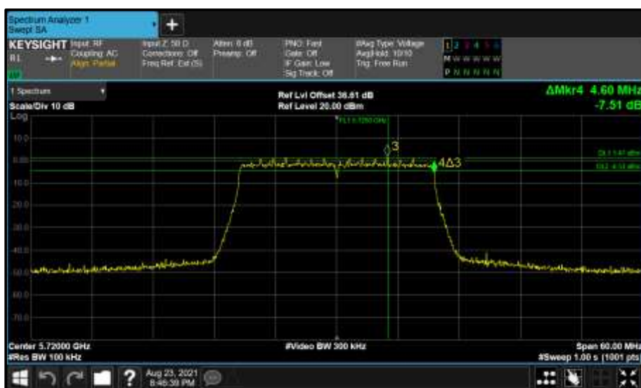
Figure 710 - Core 1 (B) 5720 MHz (CH144) 6 dB Bandwidth
