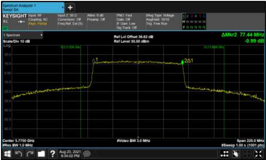
Figure 881 - Core 1 (B) 5775 MHz (CH155) 99% Bandwidth
