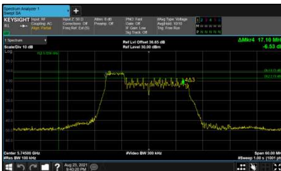
Figure 772 - Core 1 (B) 5745 MHz (CH149) 6 dB Bandwidth
