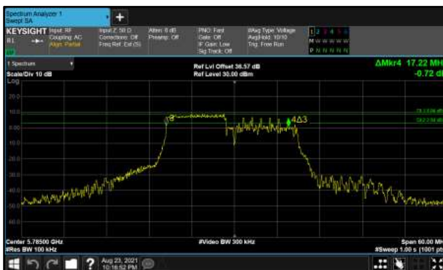
Figure 826 - Core 0 (A) 5785 MHz (CH157) 6 dB Bandwidth
