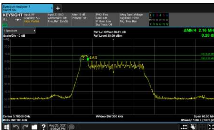
Figure 742 - Core 1 (B) 5785 MHz (CH157) 6 dB Bandwidth
