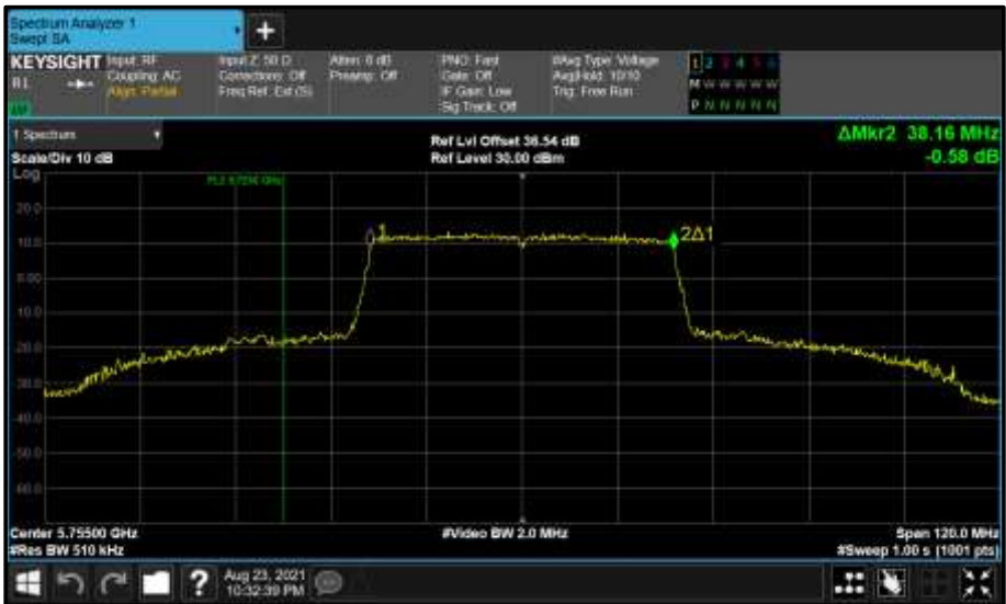
Figure 871 - Core 0 (A) 5755 MHz (CH151) 99% Bandwidth
