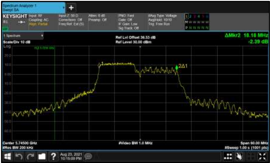
Figure 821 - Core 0 (A) 5745 MHz (CH149) 99% Bandwidth
