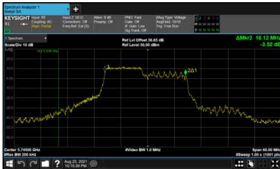
Figure 823 - Core 1 (B) 5745 MHz (CH149) 99% Bandwidth
