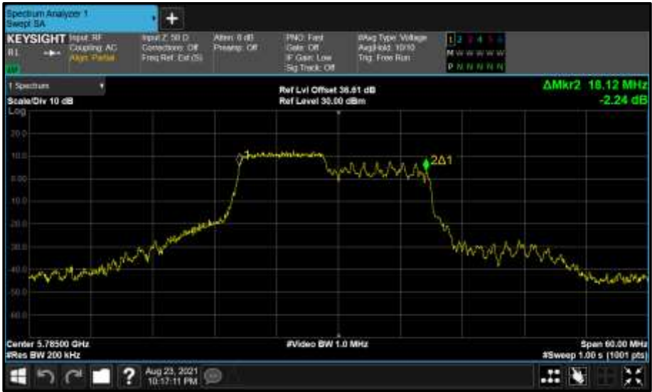
Figure 827 - Core 1 (B) 5785 MHz (CH157) 99% Bandwidth
