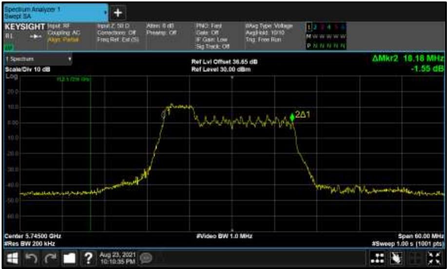
Figure 783 - Core 1 (B) 5745 MHz (CH149) 99% Bandwidth
