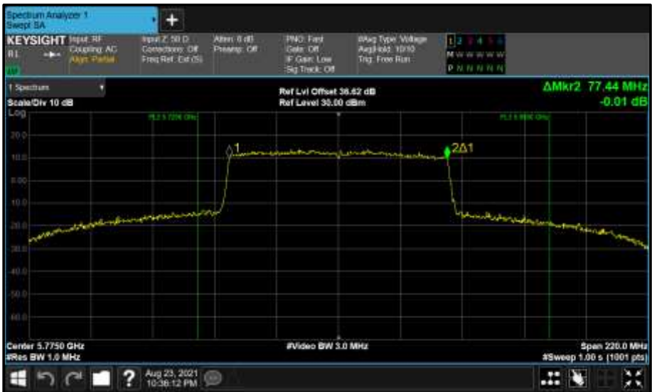
Figure 897 - Core 1 (B) 5775 MHz (CH155) 99% Bandwidth
