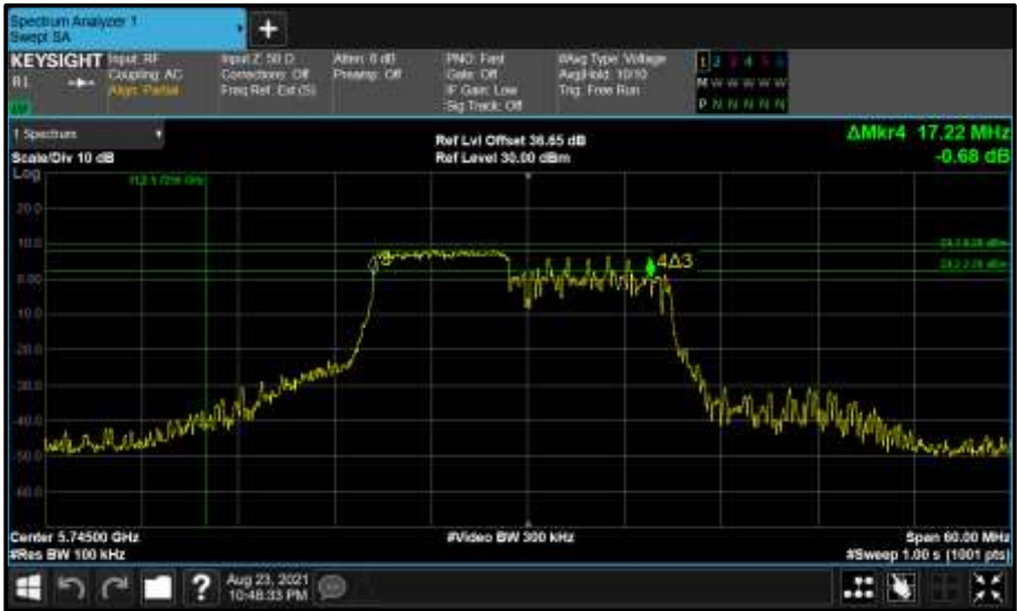
Figure 840 - Core 1 (B) 5745 MHz (CH149) 6 dB Bandwidth
