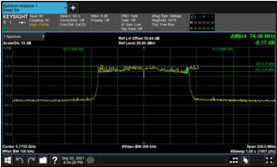
Figure 932 - Core 0 (A) 5775 MHz (CH155) 6 dB Bandwidth
