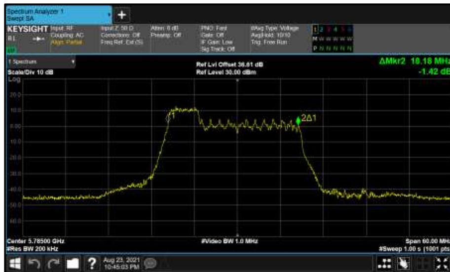
Figure 803 - Core 1 (B) 5785 MHz (CH157) 99% Bandwidth
