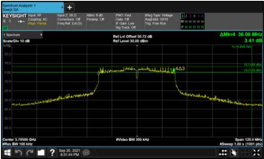
Figure 924 - Core 0 (A) 5795 MHz (CH159) 6 dB Bandwidth
