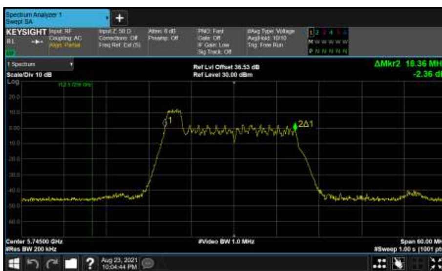
Figure 745 - Core 0 (A) 5745 MHz (CH149) 99% Bandwidth
