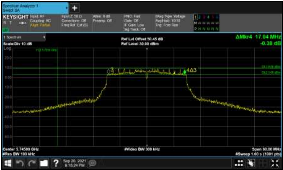
Figure 904 - Core 0 (A) 5745 MHz (CH149) 6 dB Bandwidth
