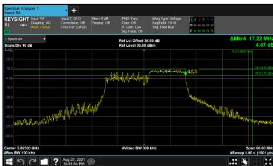
Figure 848 - Core 1 (B) 5825 MHz (CH165) 6 dB Bandwidth
