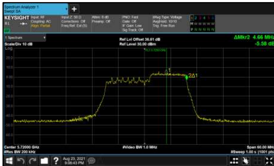
Figure 819 - Core 1 (B) 5720 MHz (CH144) 99% Bandwidth
