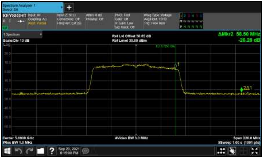
Figure 929 - Core 1 (B) 5690 MHz (CH138) 99% Bandwidth
