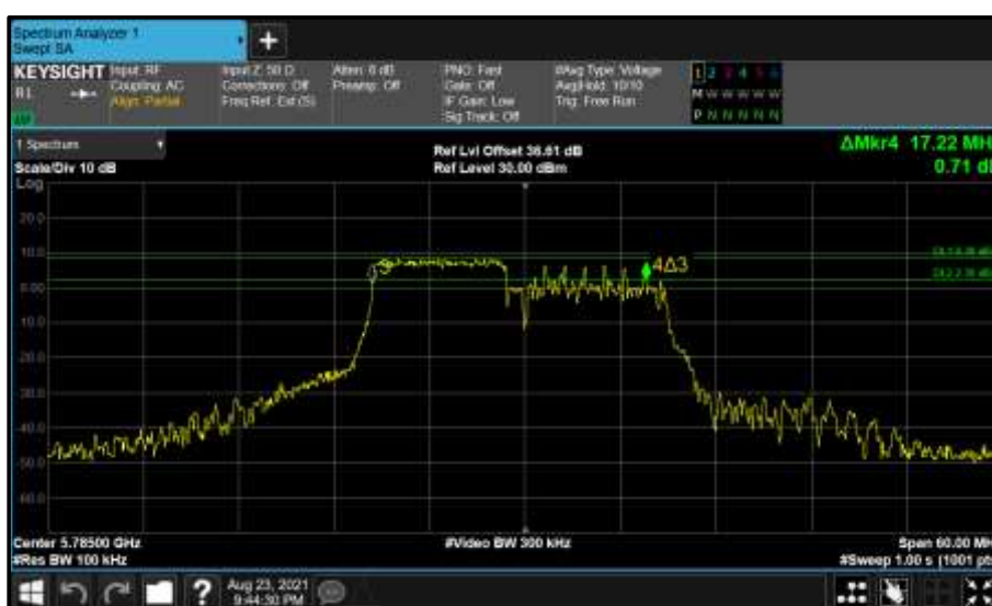
Figure 814 - Core 1 (B) 5785 MHz (CH157) 6 dB Bandwidth
