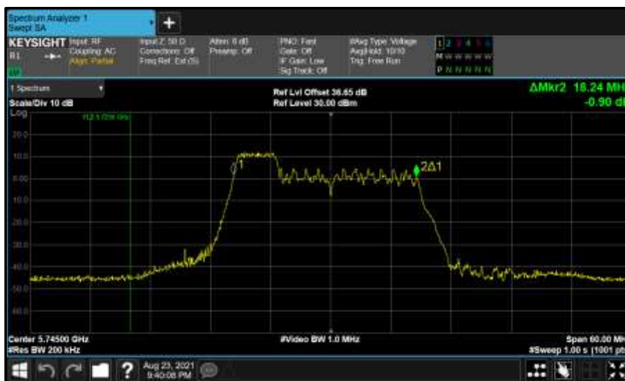
Figure 771 - Core 1 (B) 5745 MHz (CH149) 99% Bandwidth
