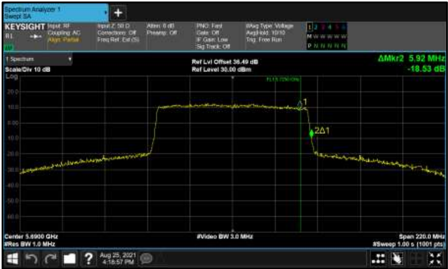
Figure 893 - Core 1 (B) 5690 MHz (CH138) 99% Bandwidth
