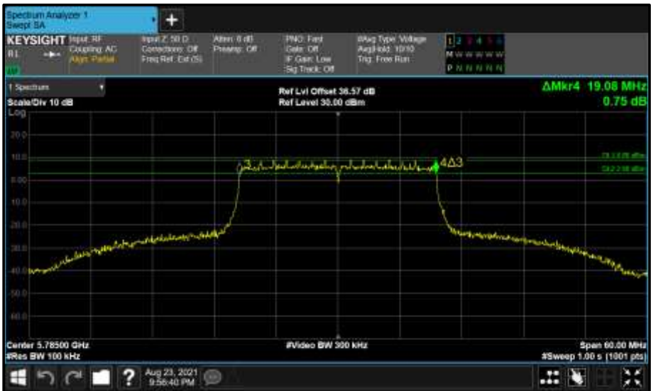
Figure 716 - Core 0 (A) 5785 MHz (CH157) 6 dB Bandwidth
