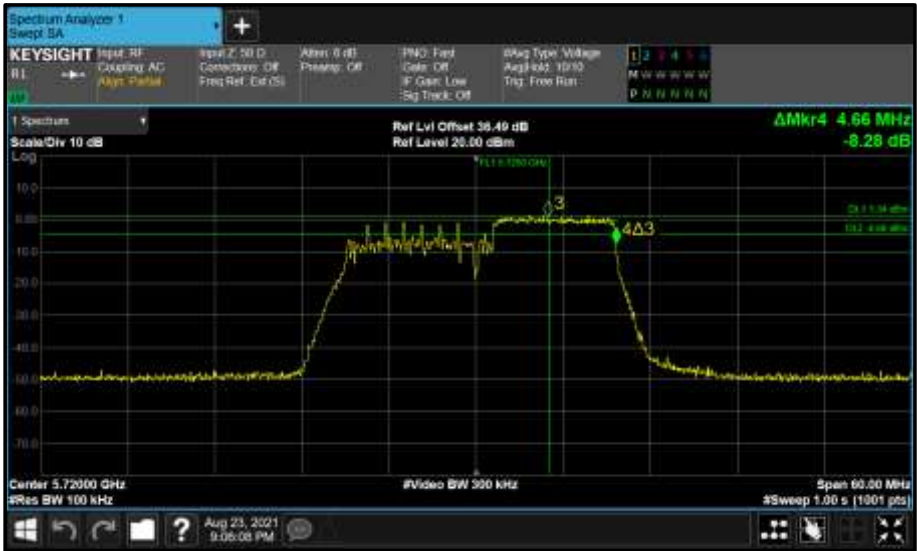
Figure 818 - Core 0 (A) 5720 MHz (CH144) 6 dB Bandwidth
