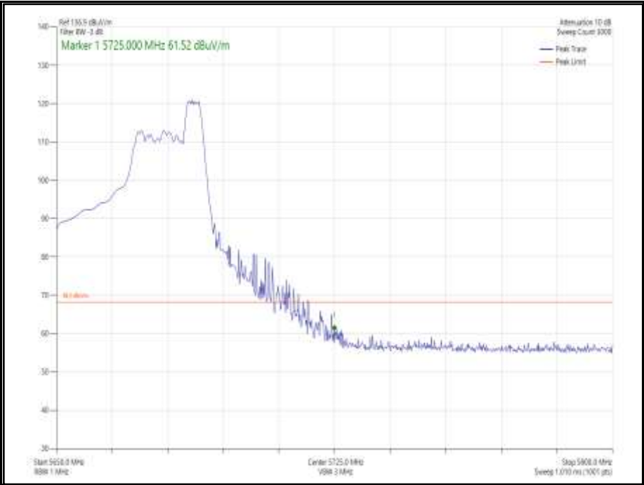
Figure 982 - 802.11ax HE40, Core 1, 26-17 - 5670 MHz Band Edge Frequency 5725 MHz
