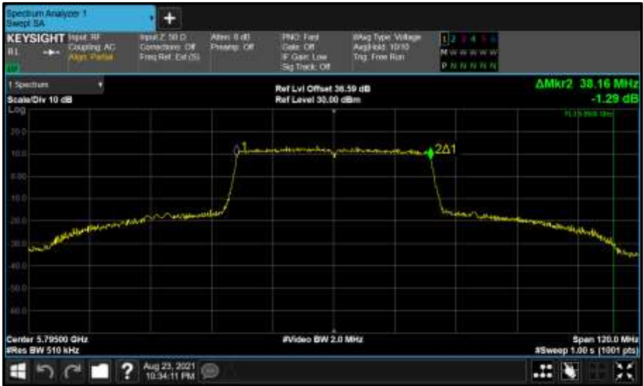
Figure 875 - Core 0 (A) 5795 MHz (CH159) 99% Bandwidth
