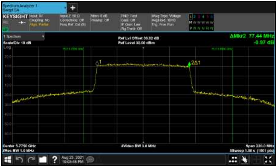
Figure 889 - Core 1 (B) 5775 MHz (CH155) 99% Bandwidth
