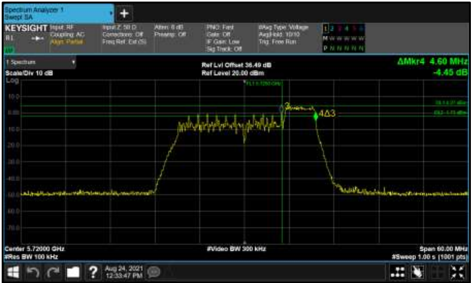
Figure 794 - Core 0 (A) 5720 MHz (CH144) 6 dB Bandwidth
