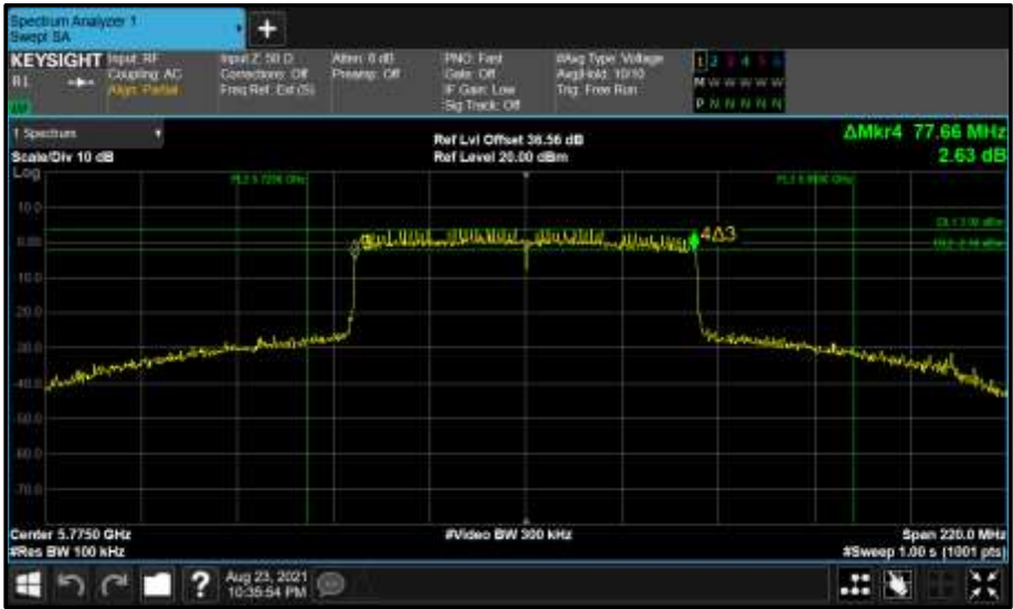
Figure 896 - Core 0 (A) 5775 MHz (CH155) 6 dB Bandwidth
