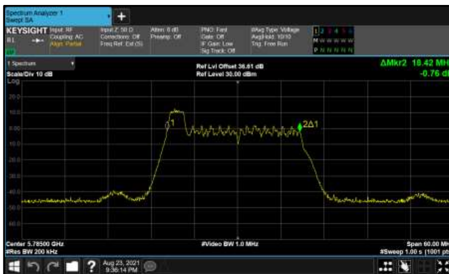
Figure 741 - Core 1 (B) 5785 MHz (CH157) 99% Bandwidth
