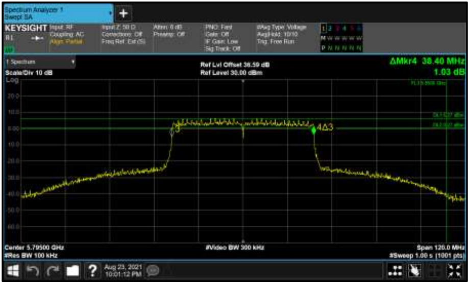
Figure 864 - Core 0 (A) 5795 MHz (CH159) 6 dB Bandwidth
