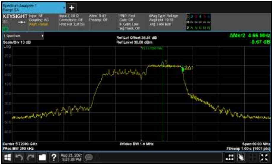
Figure 809 - Core 1 (B) 5720 MHz (CH144) 99% Bandwidth
