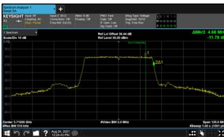
Figure 867 - Core 0 (A) 5710 MHz (CH142) 99% Bandwidth
