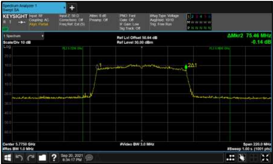
Figure 931 - Core 0 (A) 5775 MHz (CH155) 99% Bandwidth
