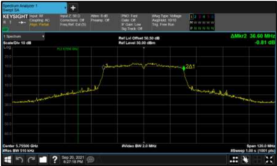
Figure 919 - Core 0 (A) 5755 MHz (CH151) 99% Bandwidth
