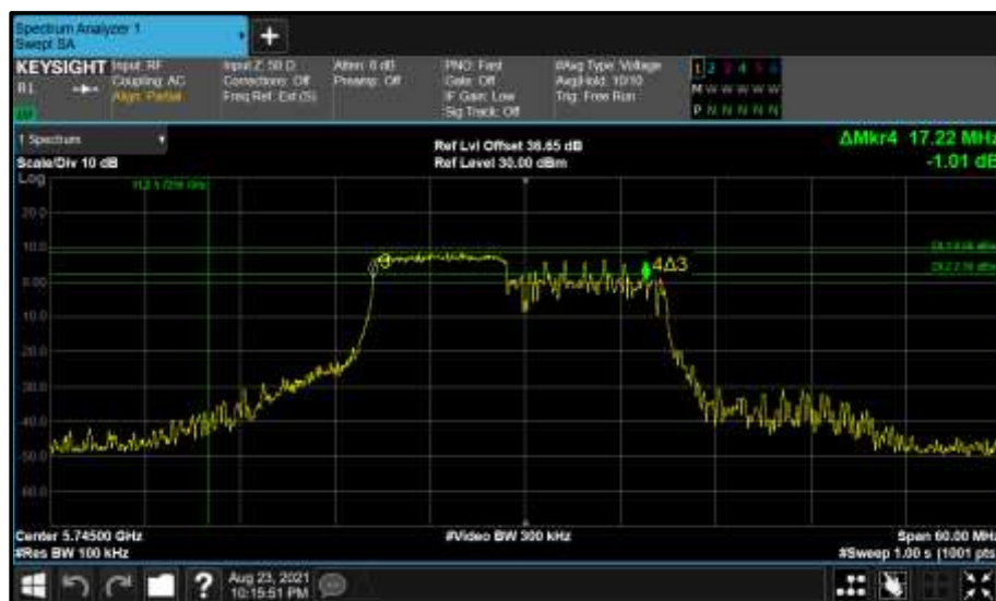
Figure 824 - Core 1 (B) 5745 MHz (CH149) 6 dB Bandwidth
