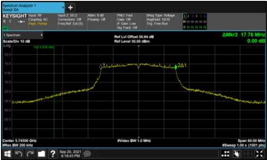
Figure 905 - Core 1 (B) 5745 MHz (CH149) 99% Bandwidth
