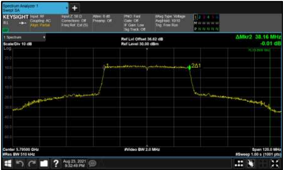
Figure 853 - Core 1 (B) 5795 MHz (CH159) 99% Bandwidth
