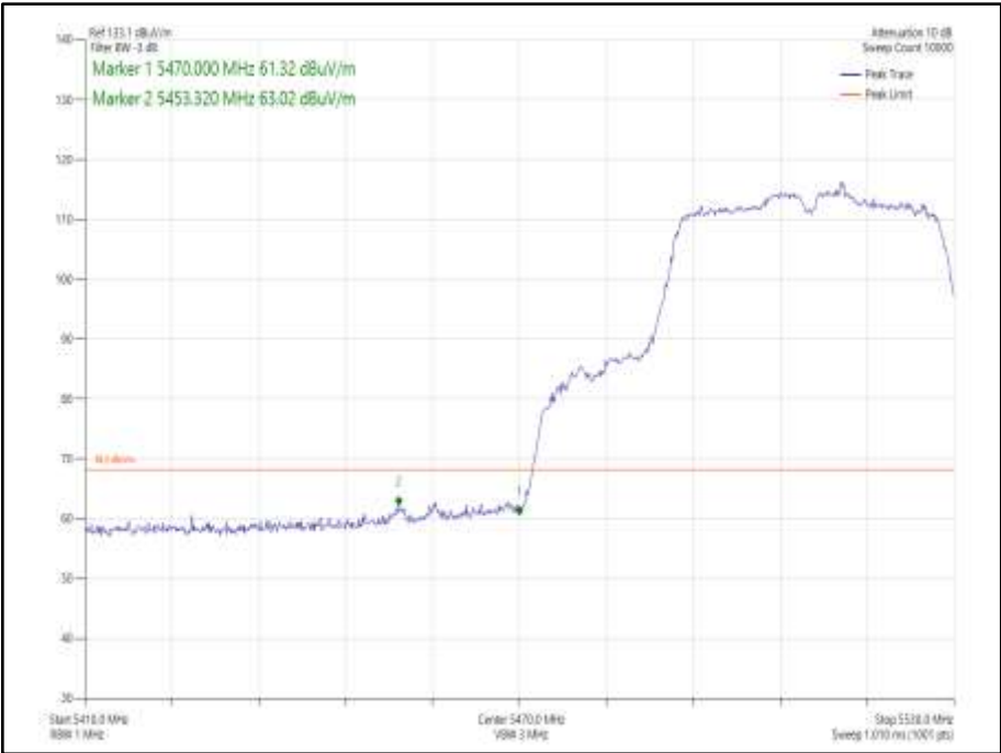
Figure 988 - 802.11n HT40 SDM, Cores 0-1 - 5510 MHz Band Edge Frequency 5470 MHz
