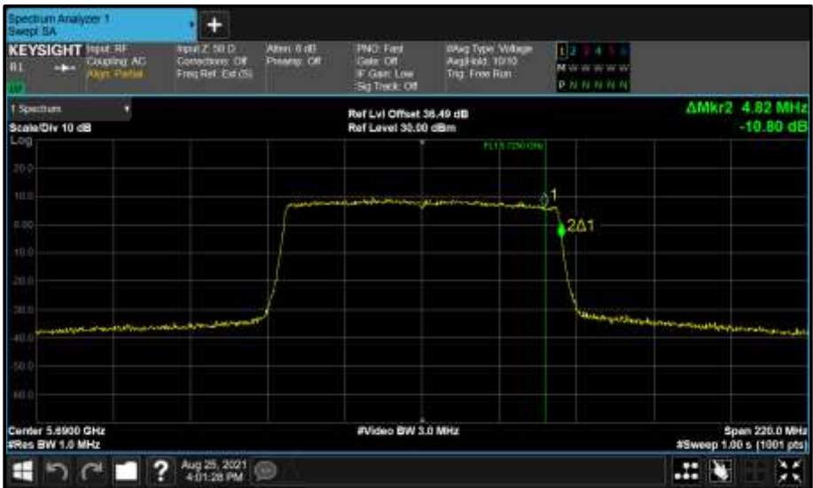
Figure 885 - Core 1 (B) 5690 MHz (CH138) 99% Bandwidth
