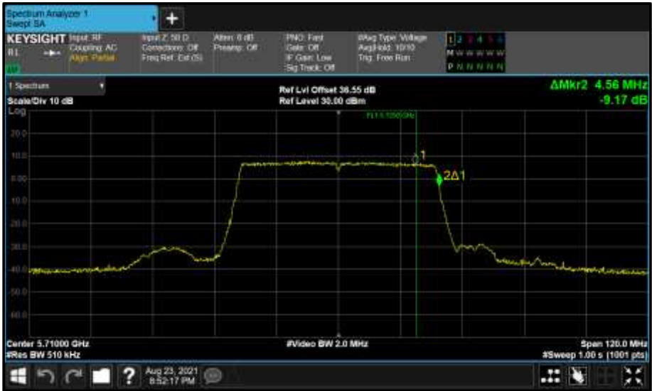
Figure 857 - Core 1 (B) 5710 MHz (CH142) 99% Bandwidth
