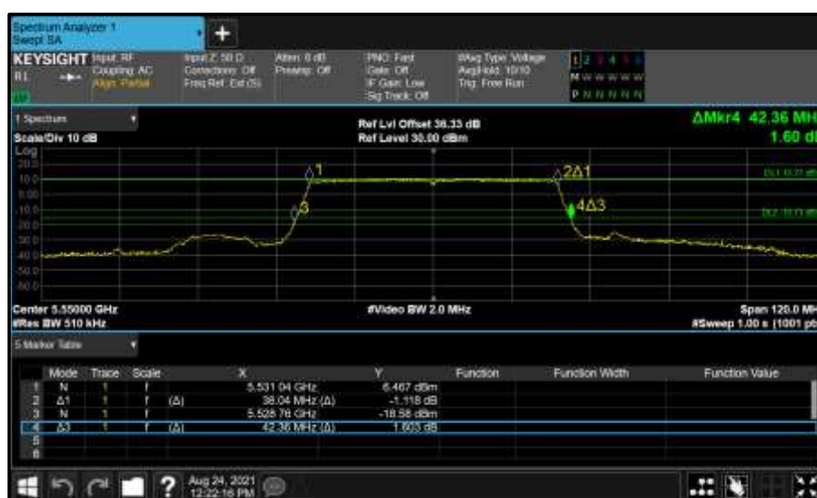
Figure 564 - Core 1 (B) 5550 MHz (CH110) 26 dB and 99% Bandwidth
