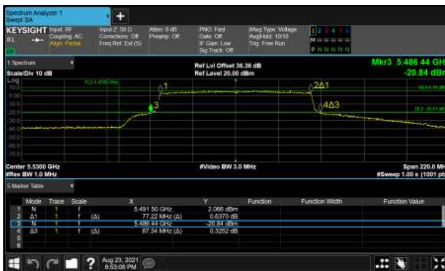
Figure 571 - Core 0 (A) 5530 MHz (CH106) 26 dB and 99% Bandwidth
