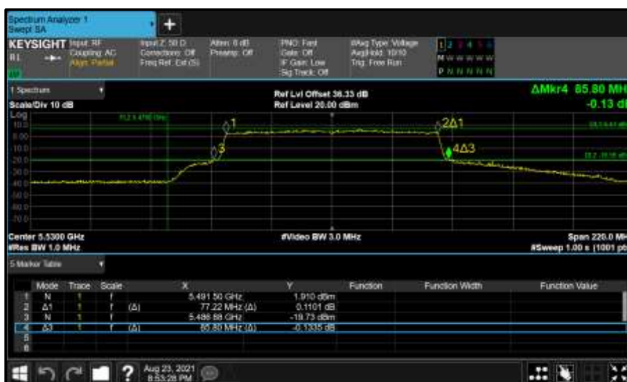
Figure 572 - Core 1 (B) 5530 MHz (CH106) 26 dB and 99% Bandwidth
