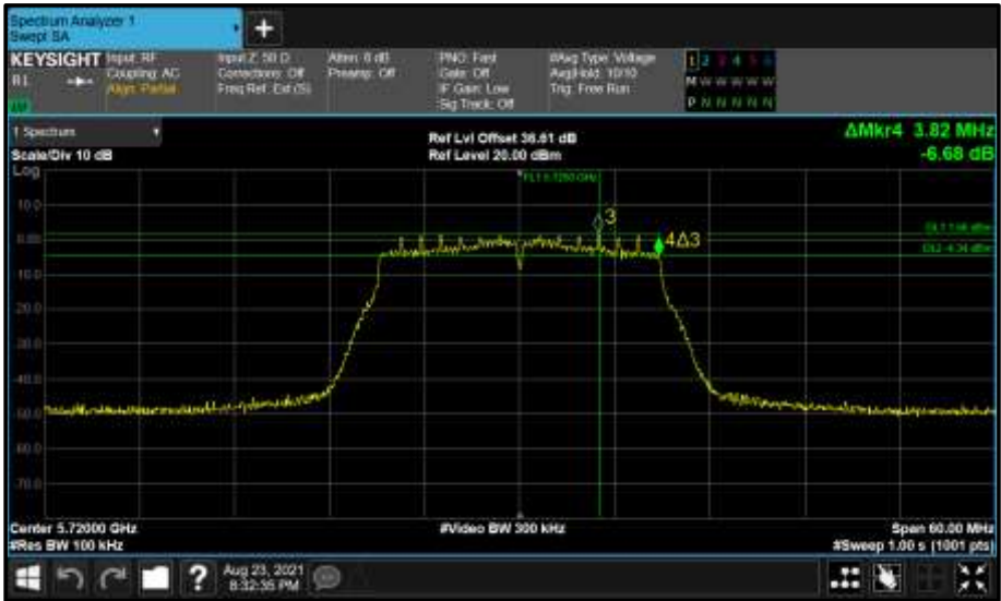
Figure 620 - Core 1 (B) 5720 MHz (CH144) 6 dB Bandwidth
