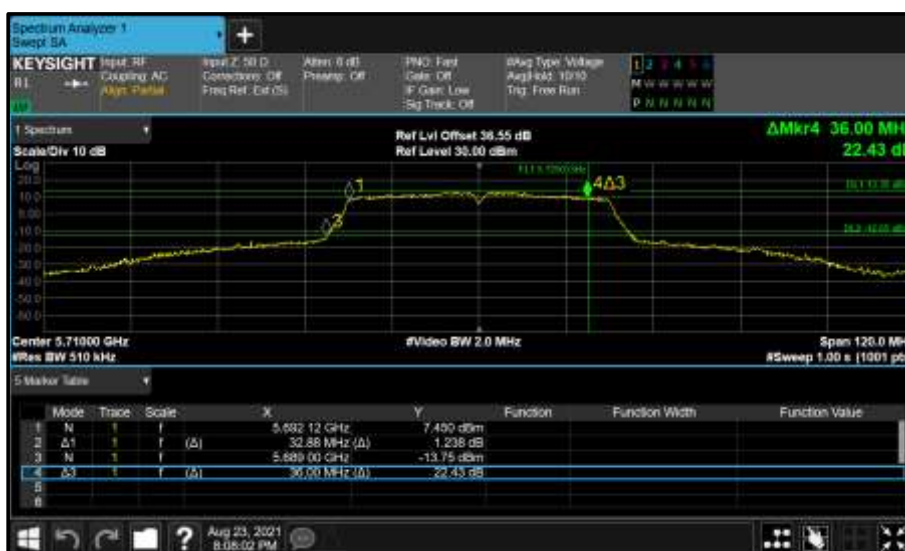
Figure 457 - Core 1 (B) 5710 MHz (CH142) 26 dB and 99% Bandwidth
