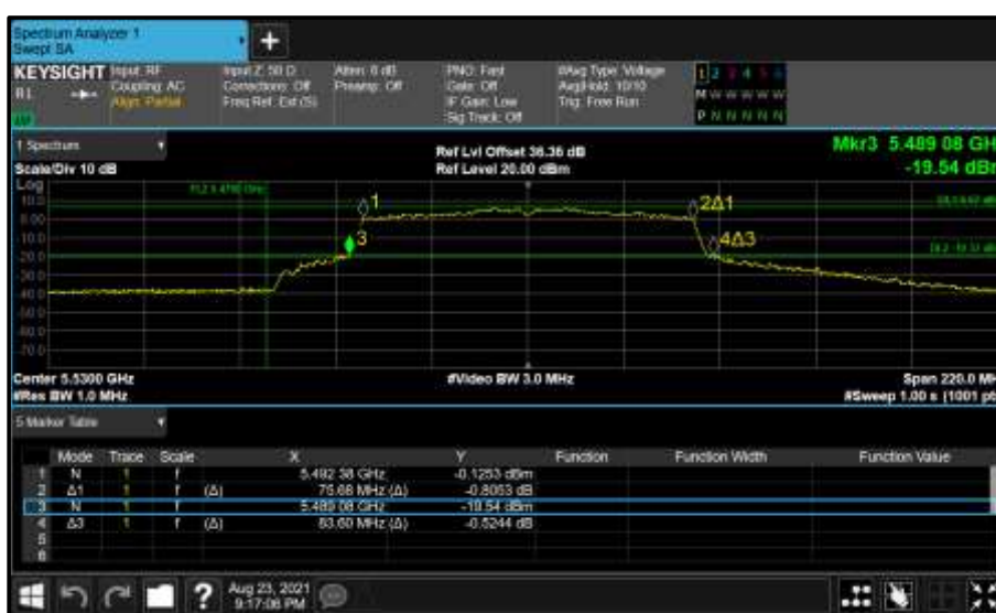
Figure 483 - Core 0 (A) 5530 MHz (CH106) 26 dB and 99% Bandwidth
