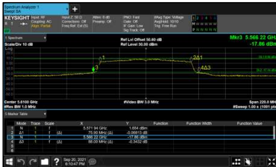
Figure 598 - Core 1 (B) 5610 MHz (CH122) 26 dB and 99% Bandwidth
