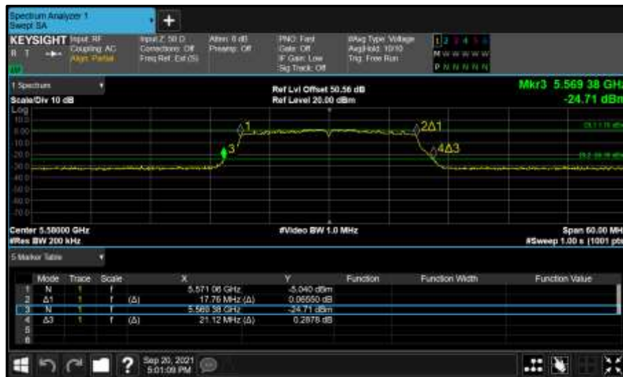
Figure 582 - Core 1 (B) 5580 MHz (CH116) 26 dB and 99% Bandwidth
