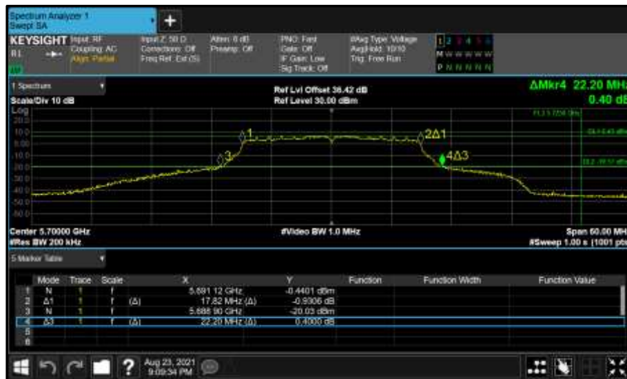
Figure 450 - Core 0 (A) 5700 MHz (CH140) 26 dB and 99% Bandwidth
