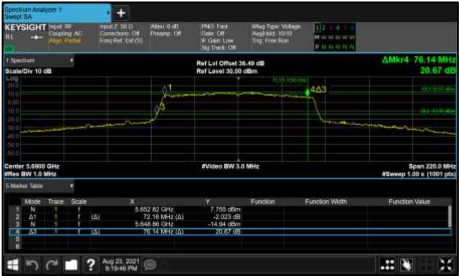
Figure 488 - Core 1 (B) 5690 MHz (CH138) 26 dB and 99% Bandwidth
