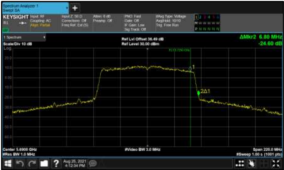
Figure 693 - Core 1 (B) 5690 MHz (CH138) 99% Bandwidth
