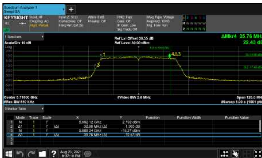
Figure 465 - Core 1 (B) 5710 MHz (CH142) 26 dB and 99% Bandwidth
