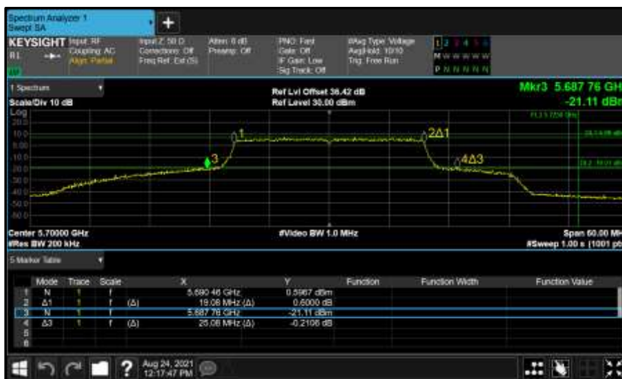
Figure 505 - Core 0 (A) 5700 MHz (CH140) 26 dB and 99% Bandwidth
