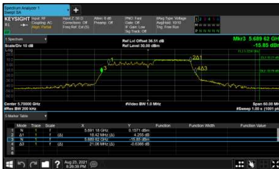
Figure 531 - Core 1 (B) 5700 MHz (CH140) 26 dB and 99% Bandwidth
