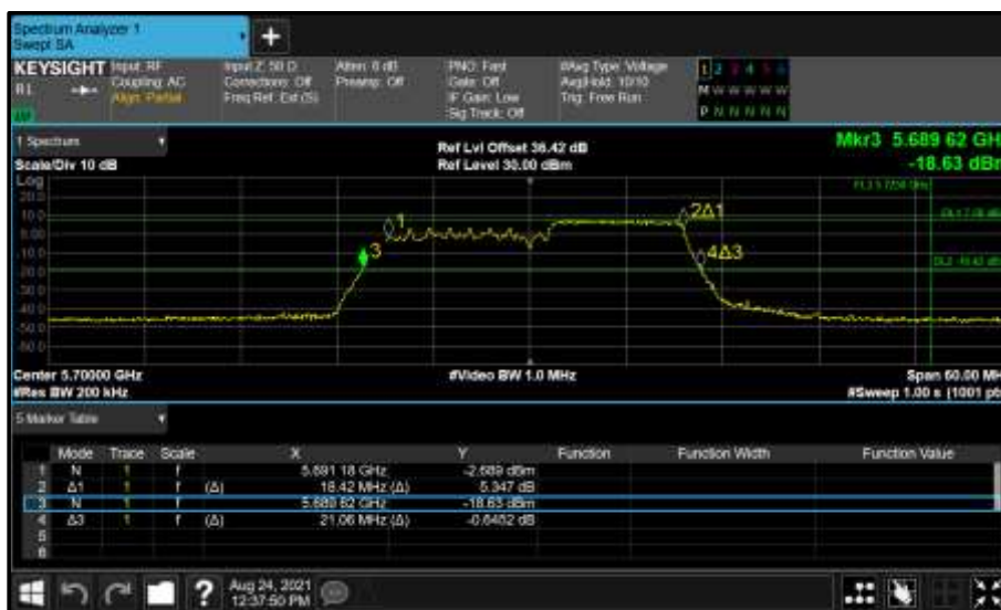
Figure 545 - Core 0 (A) 5700 MHz (CH140) 26 dB and 99% Bandwidth
