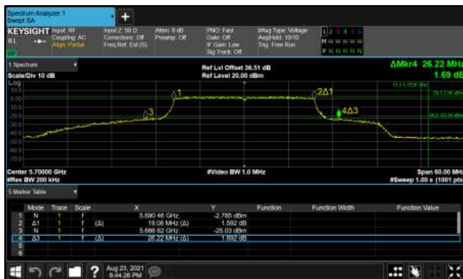
Figure 498 - Core 1 (B) 5700 MHz (CH140) 26 dB and 99% Bandwidth
