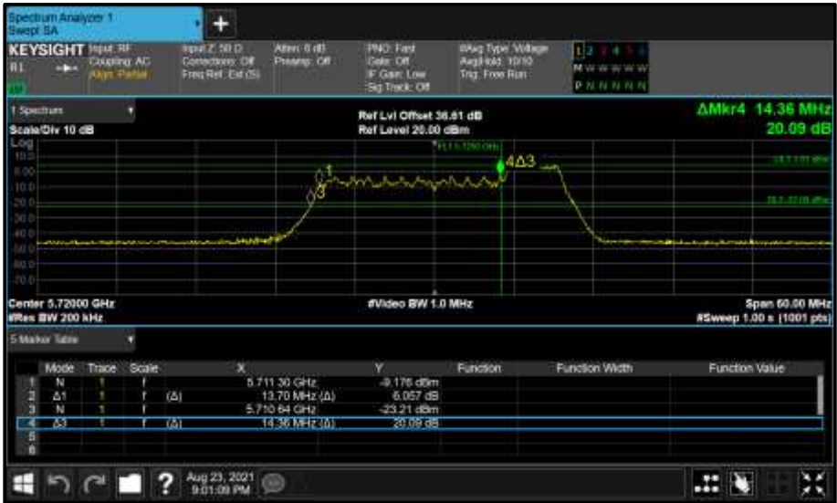
Figure 520 - Core 1 (B) 5720 MHz (CH144) 26 dB and 99% Bandwidth
