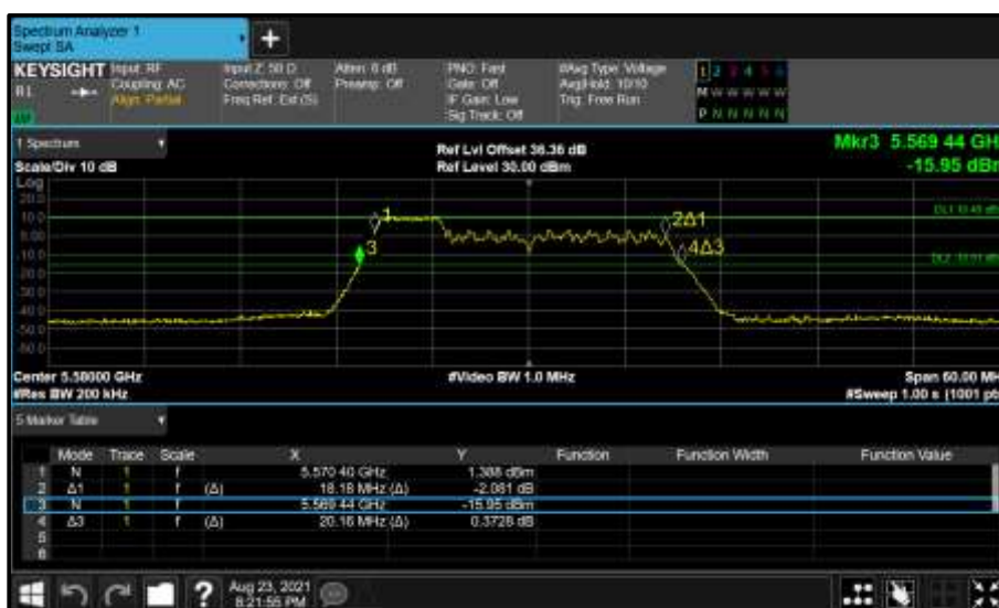
Figure 510 - Core 1 (B) 5580 MHz (CH116) 26 dB and 99% Bandwidth
