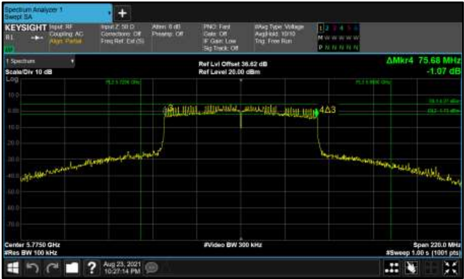
Figure 698 - Core 1 (B) 5775 MHz (CH155) 6 dB Bandwidth
