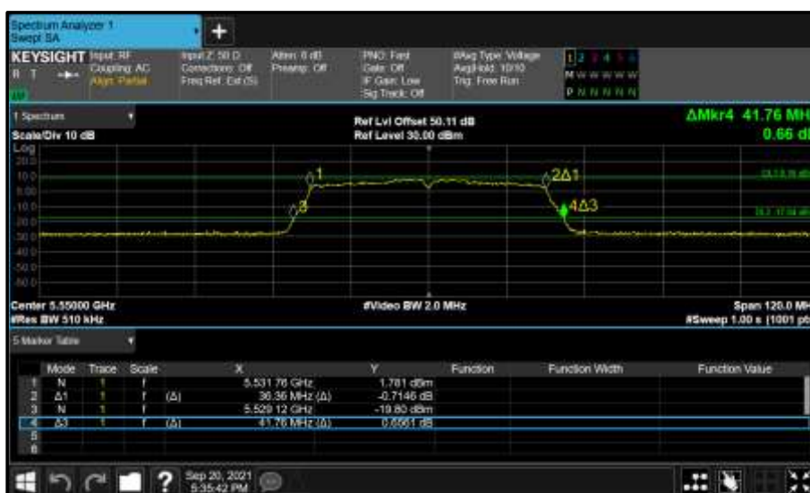
Figure 589 - Core 0 (A) 5550 MHz (CH110) 26 dB and 99% Bandwidth
