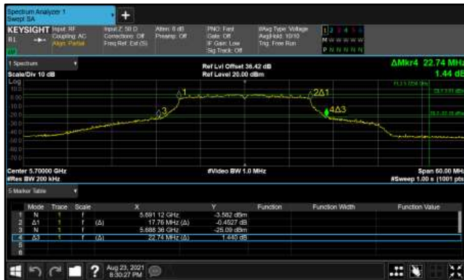
Figure 442 - Core 0 (A) 5700 MHz (CH140) 26 dB and 99% Bandwidth
