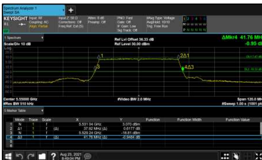
Figure 556 - Core 1 (B) 5550 MHz (CH110) 26 dB and 99% Bandwidth
