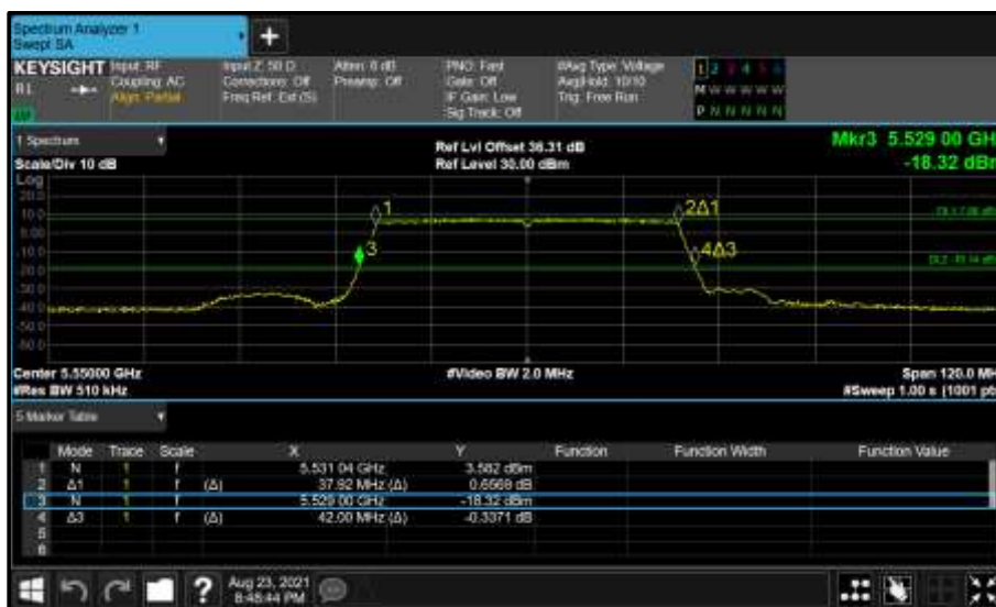
Figure 555 - Core 0 (A) 5550 MHz (CH110) 26 dB and 99% Bandwidth
