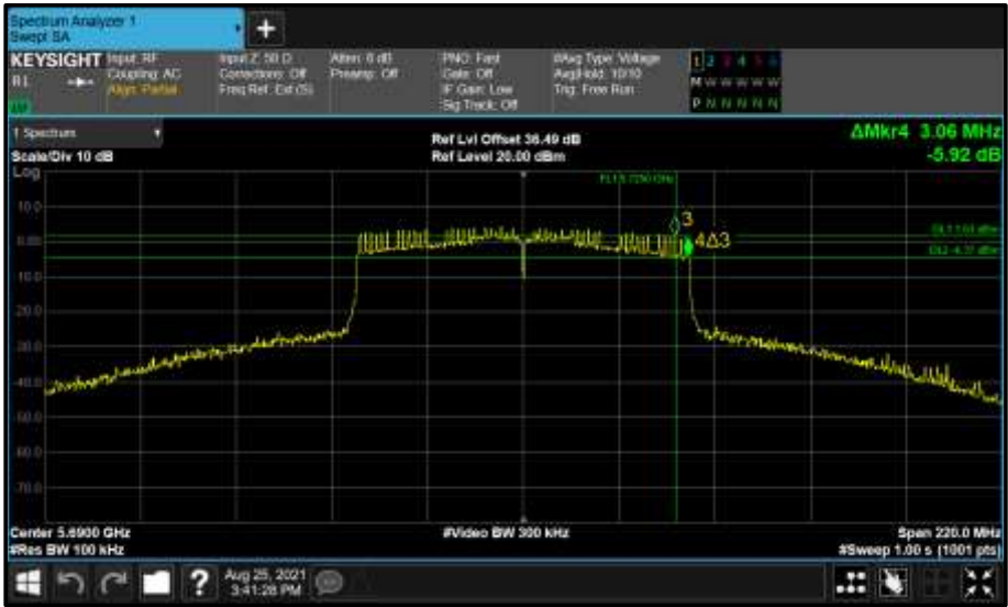
Figure 680 - Core 1 (B) 5690 MHz (CH138) 6 dB Bandwidth
