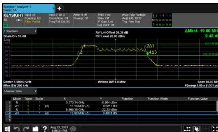
Figure 516 - Core 1 (B) 5580 MHz (CH116) 26 dB and 99% Bandwidth
