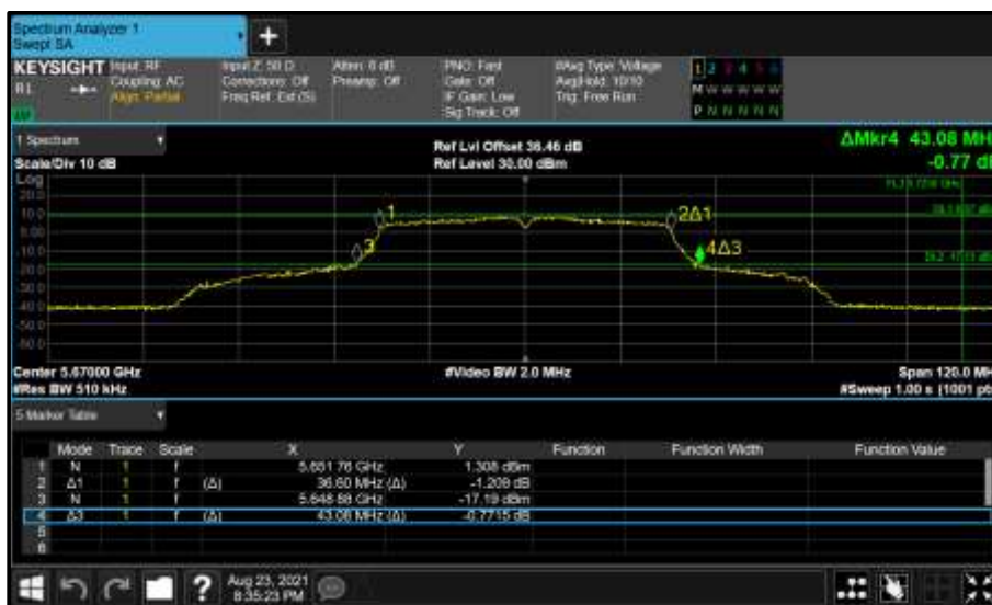
Figure 462 - Core 0 (A) 5670 MHz (CH134) 26 dB and 99% Bandwidth
