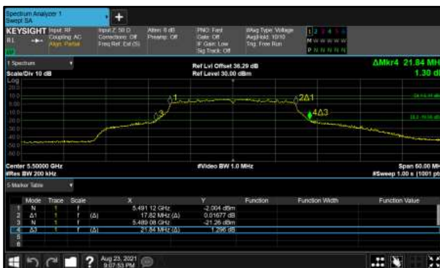
Figure 447 - Core 1 (B) 5500 MHz (CH100) 26 dB and 99% Bandwidth
