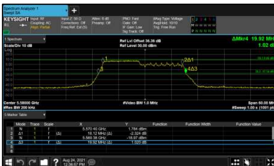
Figure 544 - Core 1 (B) 5580 MHz (CH116) 26 dB and 99% Bandwidth
