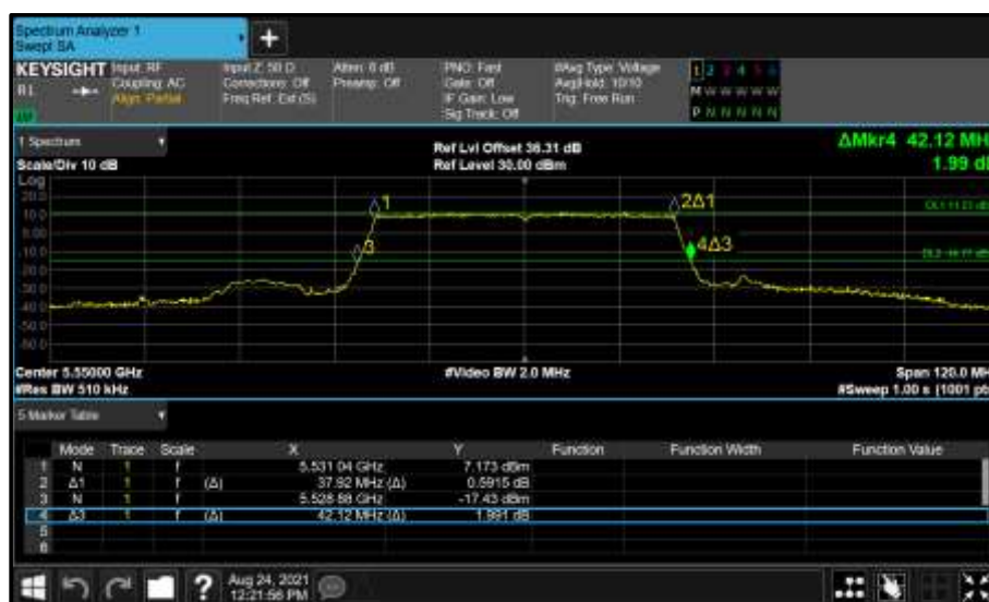
Figure 563 - Core 0 (A) 5550 MHz (CH110) 26 dB and 99% Bandwidth
