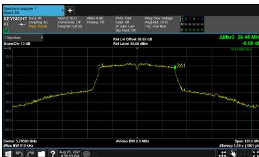
Figure 653 - Core 1 (B) 5795 MHz (CH159) 99% Bandwidth
