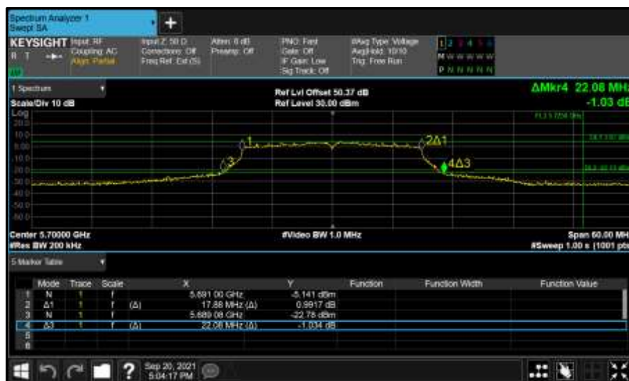
Figure 583 - Core 0 (A) 5700 MHz (CH140) 26 dB and 99% Bandwidth
