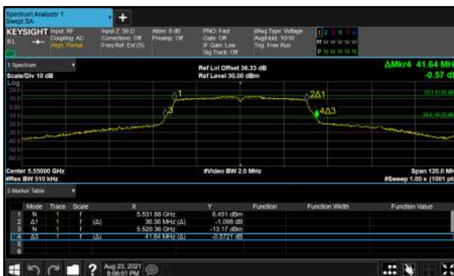
Figure 455 - Core 1 (B) 5550 MHz (CH110) 26 dB and 99% Bandwidth
