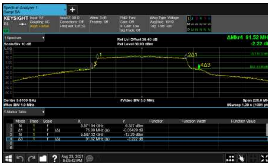
Figure 475 - Core 1 (B) 5610 MHz (CH122) 26 dB and 99% Bandwidth
