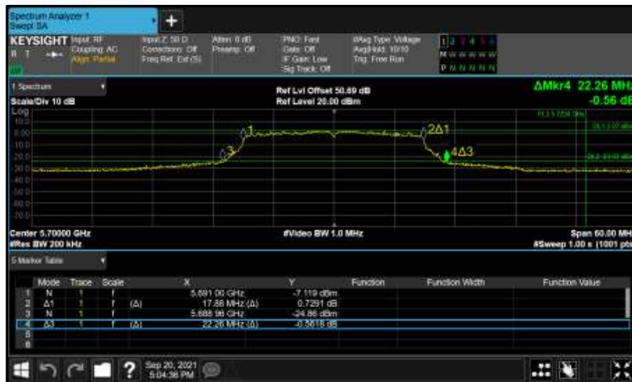
Figure 584 - Core 1 (B) 5700 MHz (CH140) 26 dB and 99% Bandwidth
