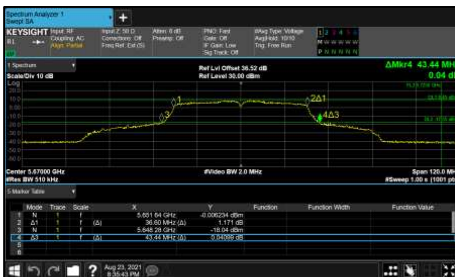
Figure 463 - Core 1 (B) 5670 MHz (CH134) 26 dB and 99% Bandwidth
