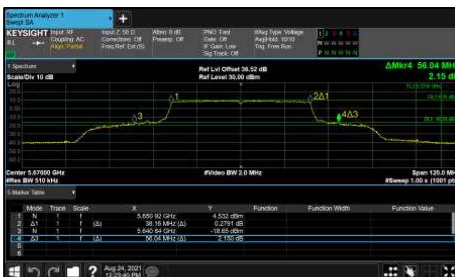
Figure 566 - Core 1 (B) 5670 MHz (CH134) 26 dB and 99% Bandwidth
