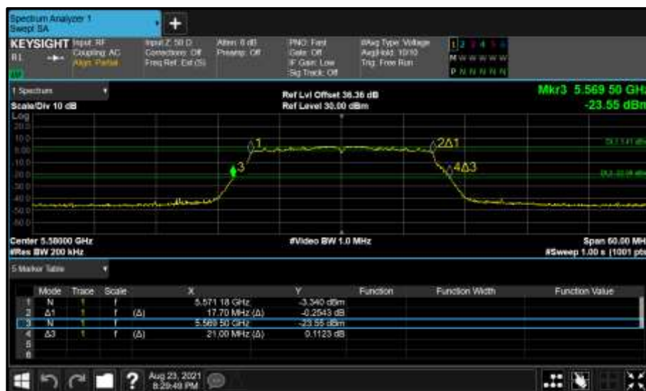
Figure 441 - Core 1 (B) 5580 MHz (CH116) 26 dB and 99% Bandwidth
