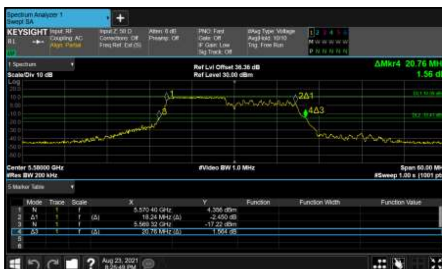
Figure 530 - Core 1 (B) 5580 MHz (CH116) 26 dB and 99% Bandwidth
