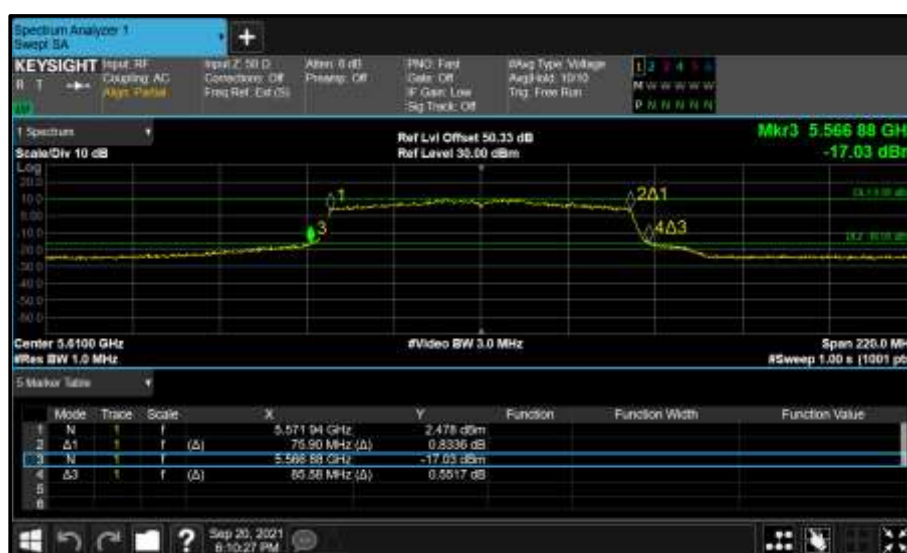
Figure 597 - Core 0 (A) 5610 MHz (CH122) 26 dB and 99% Bandwidth
