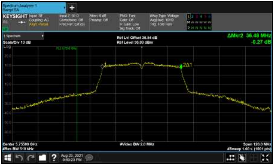
Figure 659 - Core 0 (A) 5755 MHz (CH151) 99% Bandwidth
