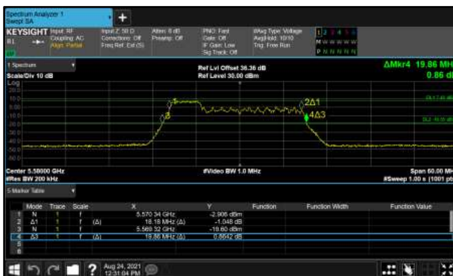
Figure 524 - Core 1 (B) 5580 MHz (CH116) 26 dB and 99% Bandwidth
