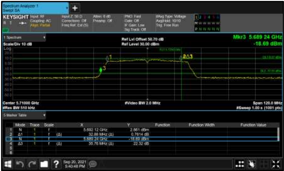
Figure 594 - Core 1 (B) 5710 MHz (CH142) 26 dB and 99% Bandwidth
