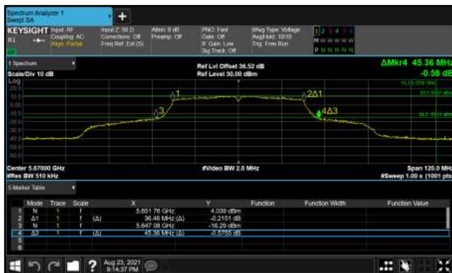
Figure 471 - Core 1 (B) 5670 MHz (CH134) 26 dB and 99% Bandwidth
