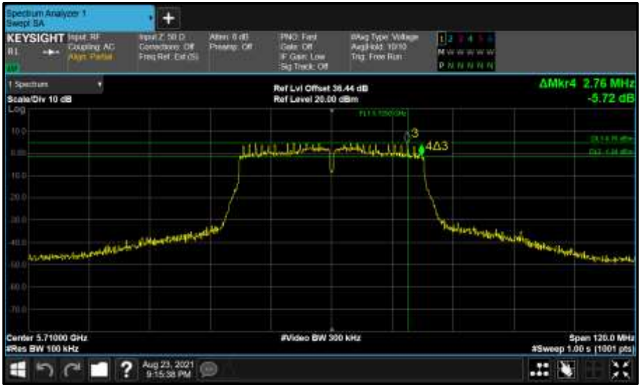
Figure 668 - Core 0 (A) 5710 MHz (CH142) 6 dB Bandwidth
