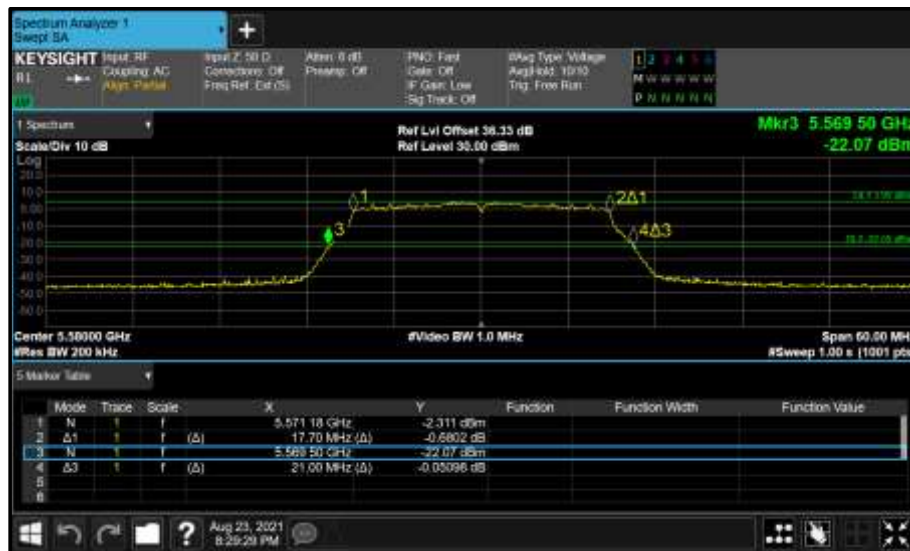
Figure 440 - Core 0 (A) 5580 MHz (CH116) 26 dB and 99% Bandwidth
