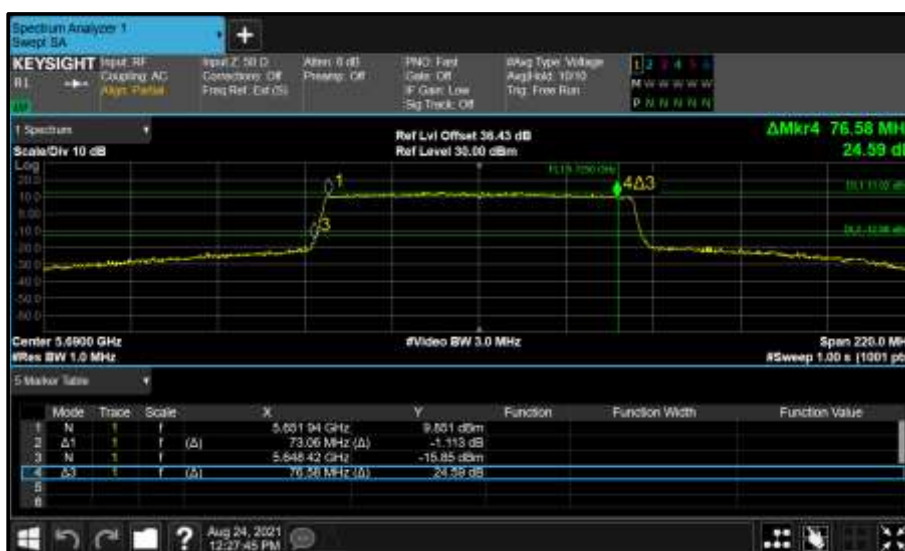
Figure 577 - Core 0 (A) 5690 MHz (CH138) 26 dB and 99% Bandwidth
