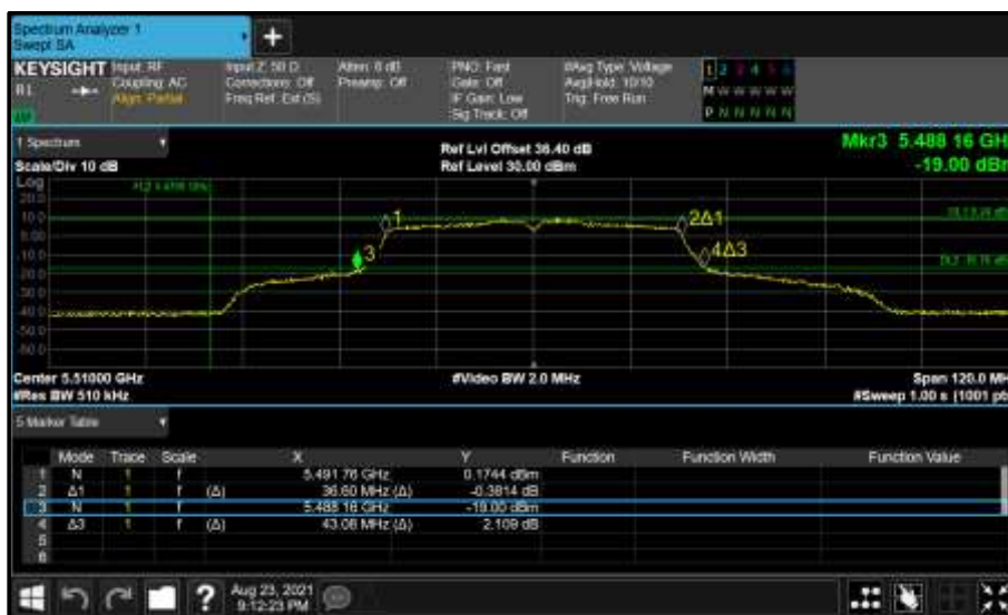
Figure 466 - Core 0 (A) 5510 MHz (CH102) 26 dB and 99% Bandwidth
