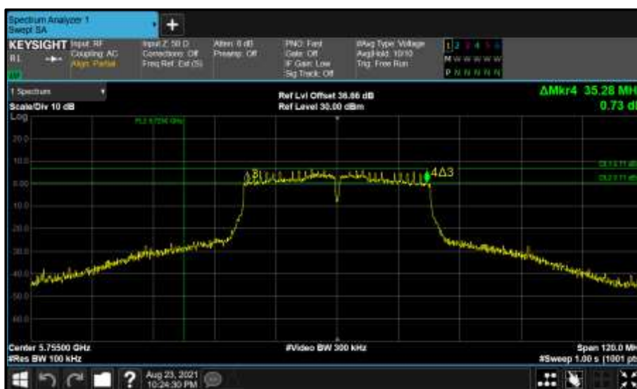
Figure 674 - Core 1 (B) 5755 MHz (CH151) 6 dB Bandwidth
