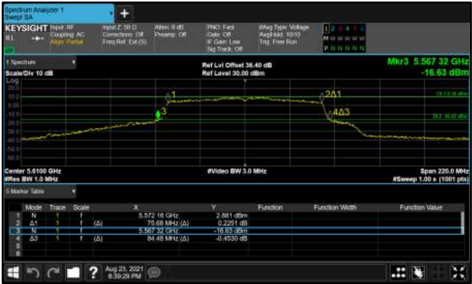
Figure 480 - Core 1 (B) 5610 MHz (CH122) 26 dB and 99% Bandwidth
