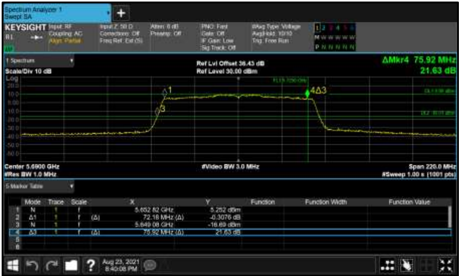
Figure 481 - Core 0 (A) 5690 MHz (CH138) 26 dB and 99% Bandwidth
