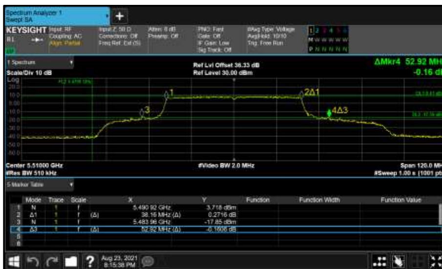
Figure 549 - Core 1 (B) 5510 MHz (CH102) 26 dB and 99% Bandwidth
