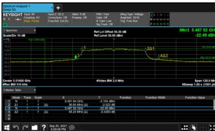
Figure 588 - Core 1 (B) 5510 MHz (CH102) 26 dB and 99% Bandwidth
