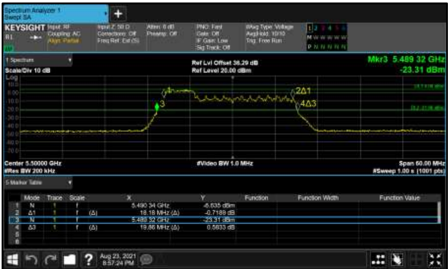
Figure 514 - Core 1 (B) 5500 MHz (CH100) 26 dB and 99% Bandwidth
