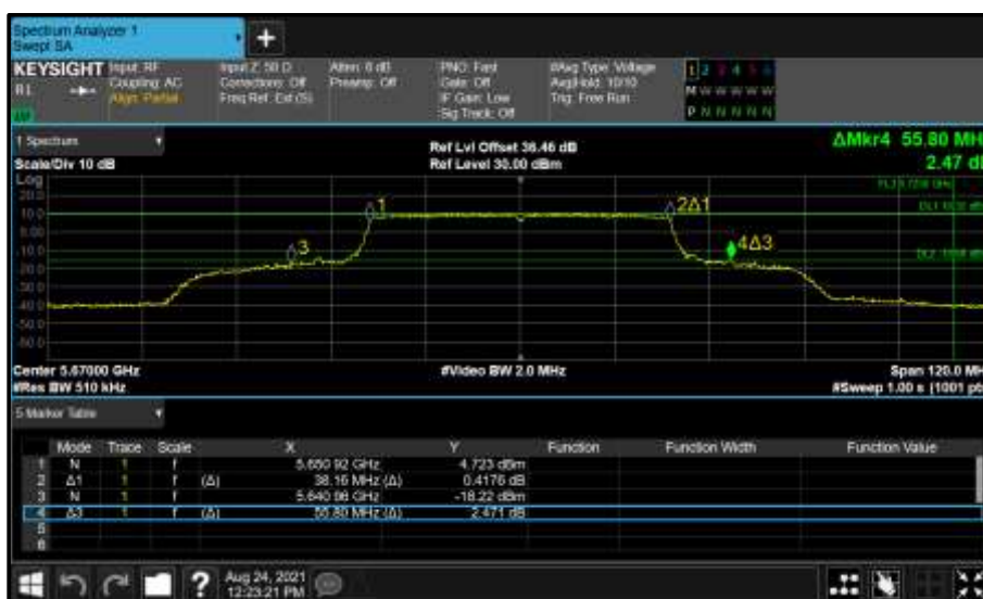
Figure 565 - Core 0 (A) 5670 MHz (CH134) 26 dB and 99% Bandwidth
