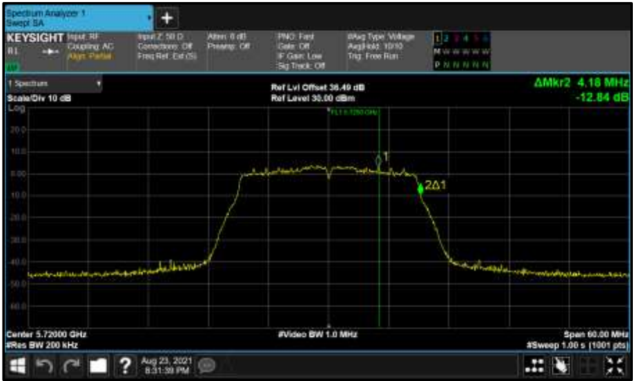
Figure 617 - Core 0 (A) 5720 MHz (CH144) 99% Bandwidth
