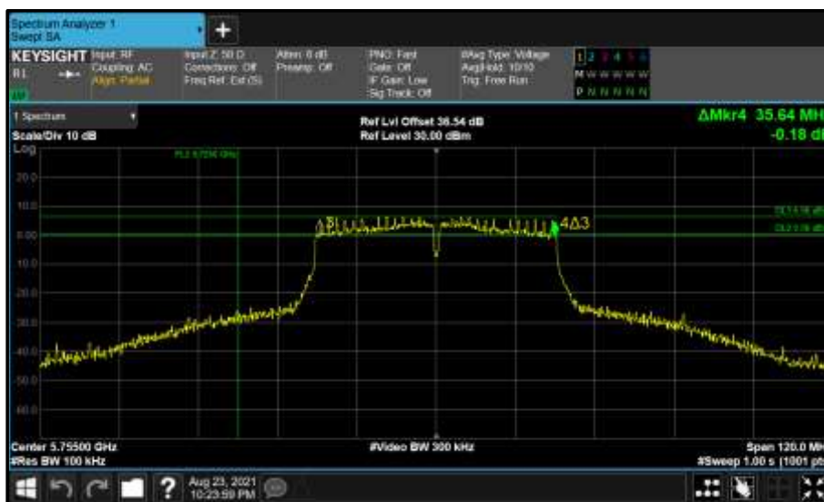
Figure 672 - Core 0 (A) 5755 MHz (CH151) 6 dB Bandwidth
