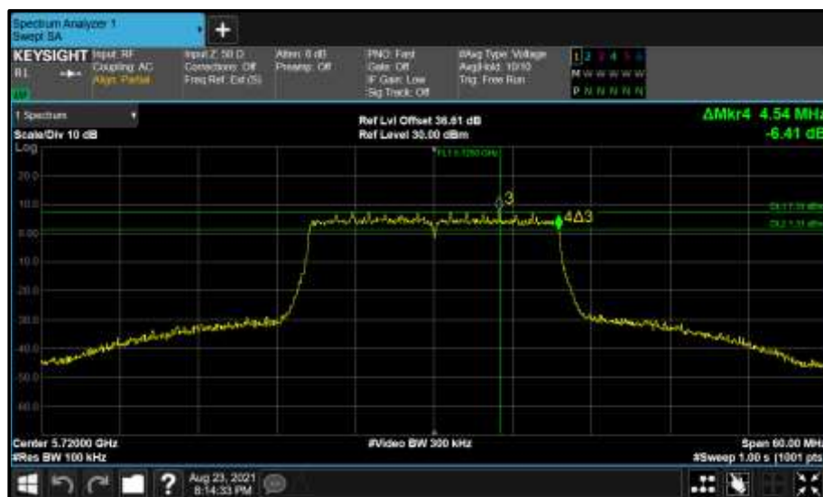
Figure 700 - Core 1 (B) 5720 MHz (CH144) 6 dB Bandwidth
