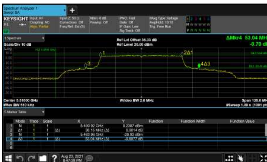
Figure 554 - Core 1 (B) 5510 MHz (CH102) 26 dB and 99% Bandwidth
