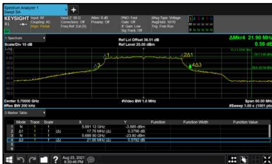
Figure 443 - Core 1 (B) 5700 MHz (CH140) 26 dB and 99% Bandwidth
