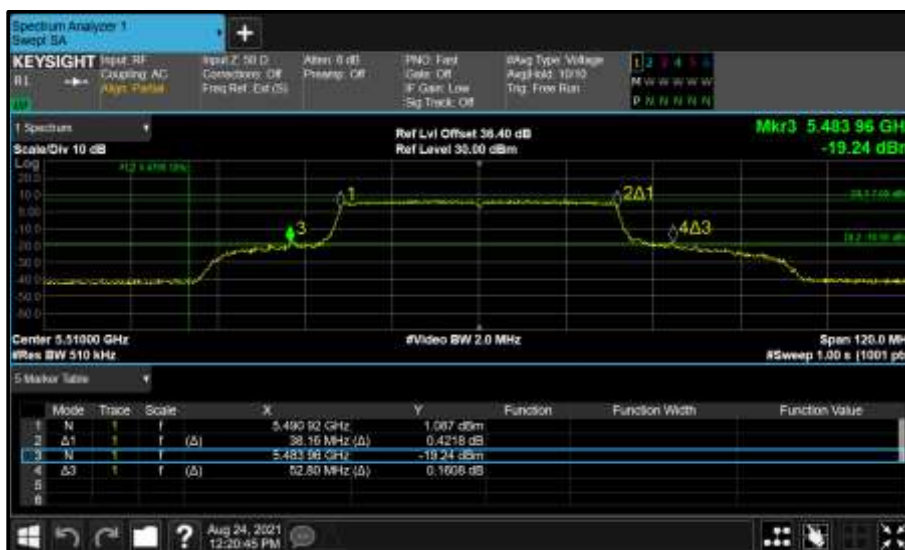
Figure 561 - Core 0 (A) 5510 MHz (CH102) 26 dB and 99% Bandwidth
