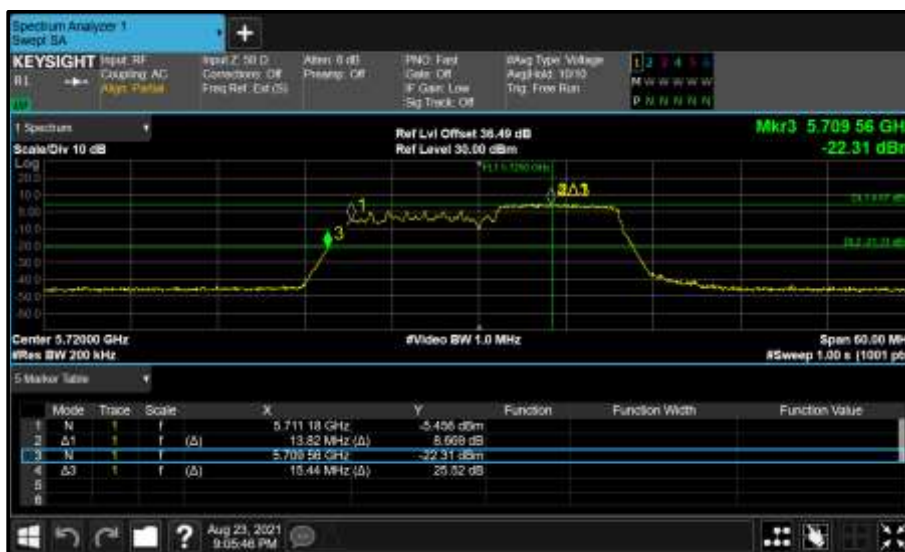
Figure 539 - Core 0 (A) 5720 MHz (CH144) 26 dB and 99% Bandwidth
