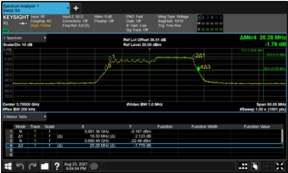
Figure 538 - Core 1 (B) 5700 MHz (CH140) 26 dB and 99% Bandwidth
