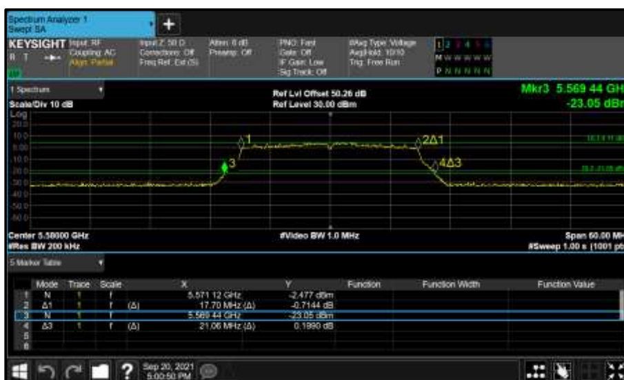
Figure 581 - Core 0 (A) 5580 MHz (CH116) 26 dB and 99% Bandwidth
