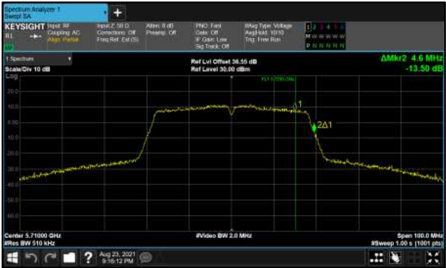
Figure 669 - Core 1 (B) 5710 MHz (CH142) 99% Bandwidth
