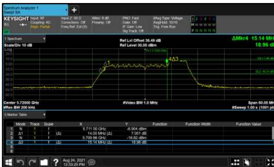
Figure 527 - Core 0 (A) 5720 MHz (CH144) 26 dB and 99% Bandwidth
