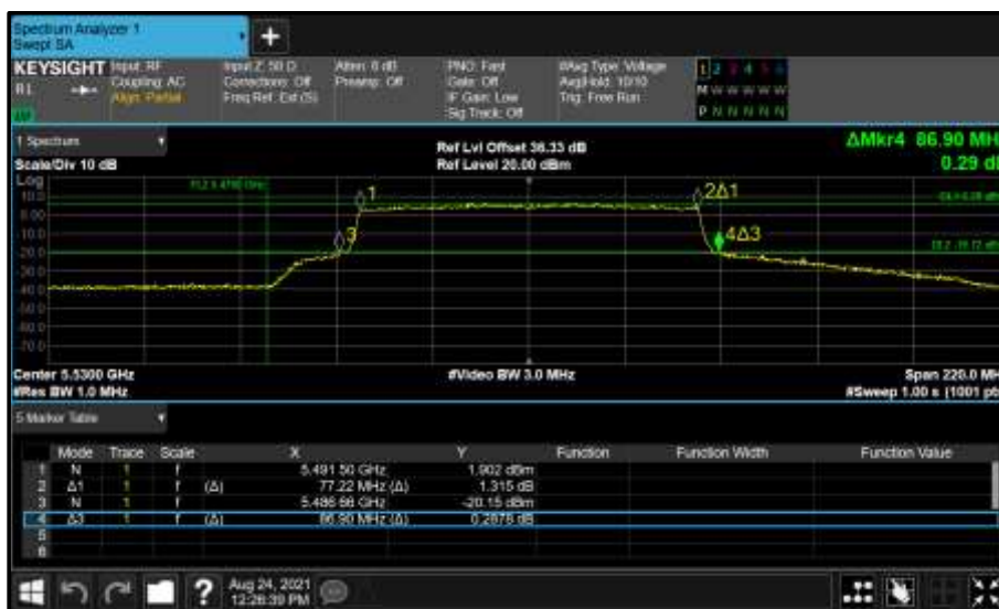
Figure 576 - Core 1 (B) 5530 MHz (CH106) 26 dB and 99% Bandwidth
