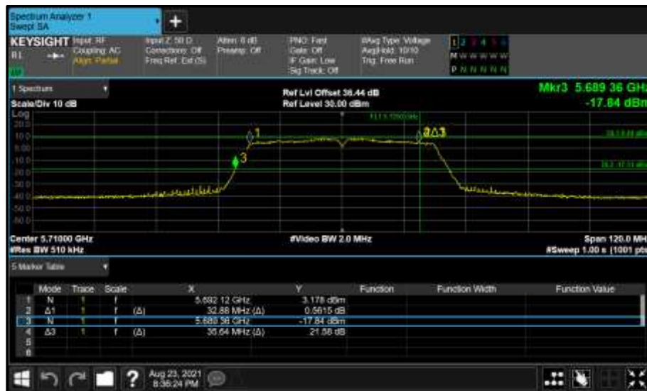
Figure 464 - Core 0 (A) 5710 MHz (CH142) 26 dB and 99% Bandwidth
