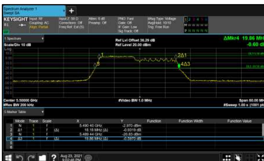
Figure 534 - Core 1 (B) 5500 MHz (CH100) 26 dB and 99% Bandwidth
