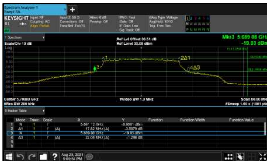
Figure 451 - Core 1 (B) 5700 MHz (CH140) 26 dB and 99% Bandwidth
