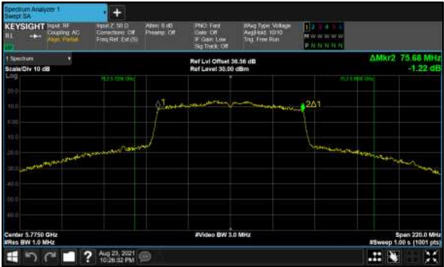
Figure 695 - Core 0 (A) 5775 MHz (CH155) 99% Bandwidth
