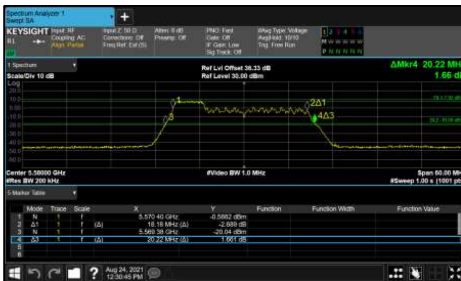
Figure 523 - Core 0 (A) 5580 MHz (CH116) 26 dB and 99% Bandwidth
