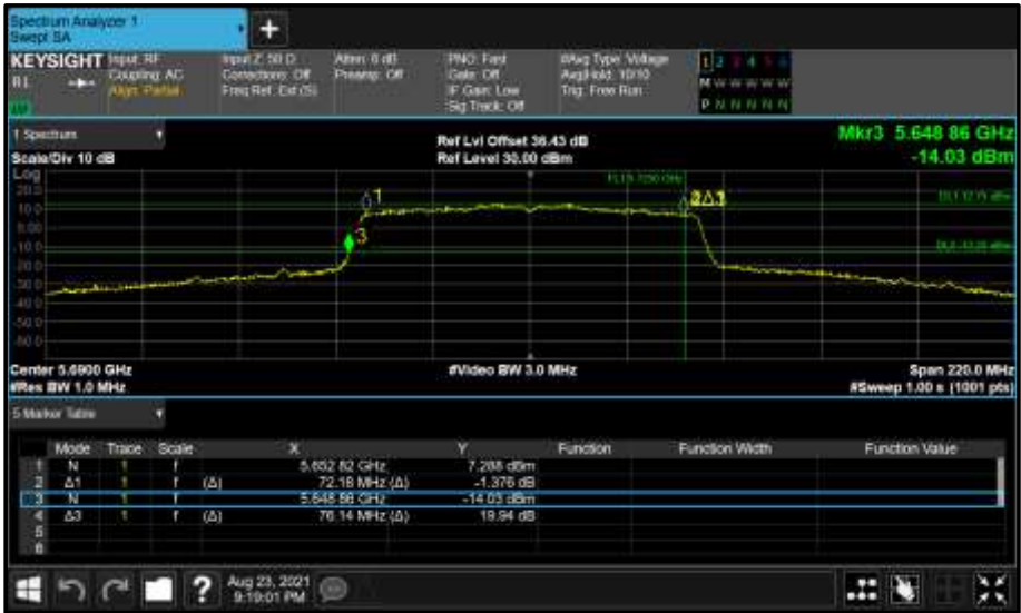
Figure 487 - Core 0 (A) 5690 MHz (CH138) 26 dB and 99% Bandwidth
