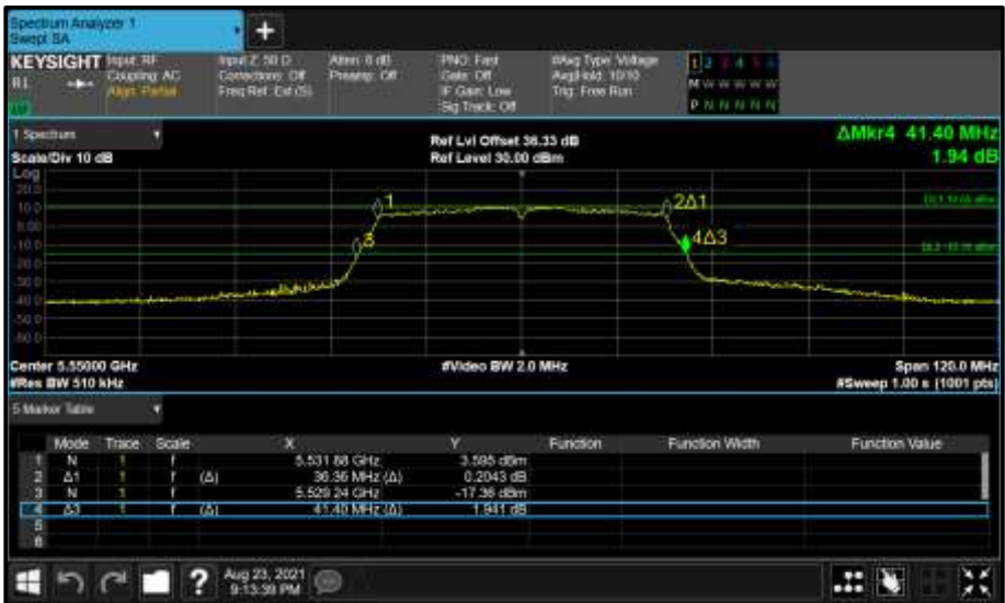
Figure 469 - Core 1 (B) 5550 MHz (CH110) 26 dB and 99% Bandwidth
