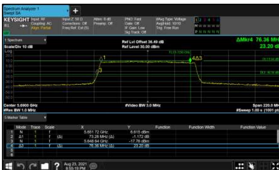
Figure 574 - Core 1 (B) 5690 MHz (CH138) 26 dB and 99% Bandwidth
