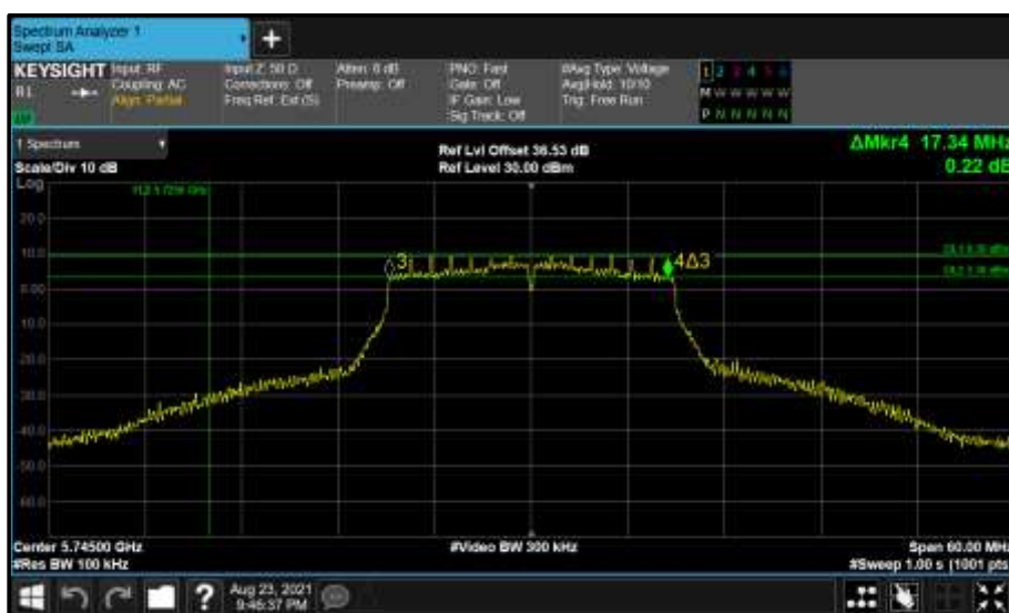
Figure 622 - Core 0 (A) 5745 MHz (CH149) 6 dB Bandwidth
