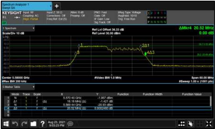
Figure 535 - Core 0 (A) 5580 MHz (CH116) 26 dB and 99% Bandwidth
