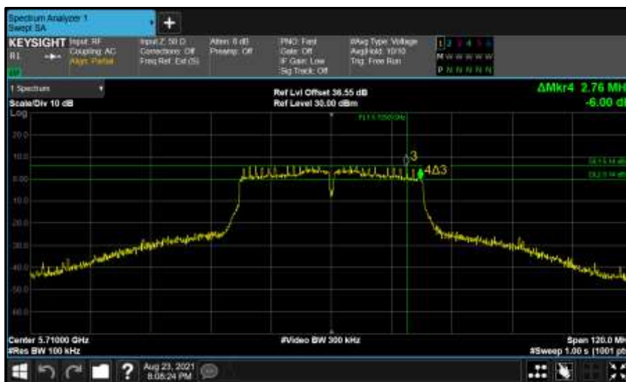
Figure 650 - Core 1 (B) 5710 MHz (CH142) 6 dB Bandwidth
