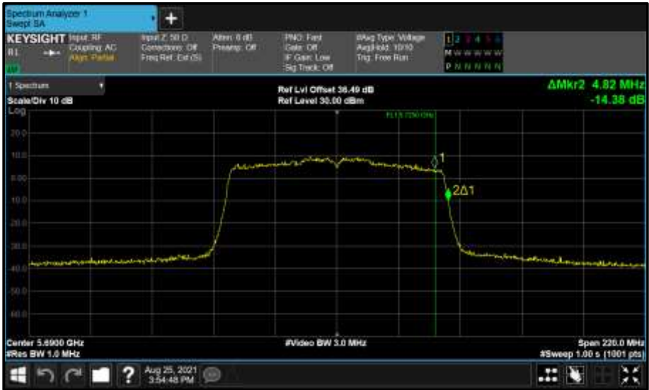
Figure 685 - Core 1 (B) 5690 MHz (CH138) 99% Bandwidth
