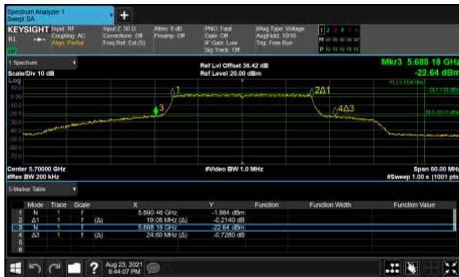
Figure 497 - Core 0 (A) 5700 MHz (CH140) 26 dB and 99% Bandwidth
