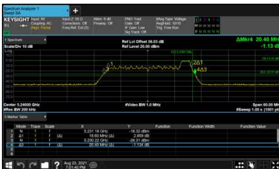
Figure 209 - Core 0 (A) 5240 MHz (CH48) 26 dB and 99% Bandwidth
