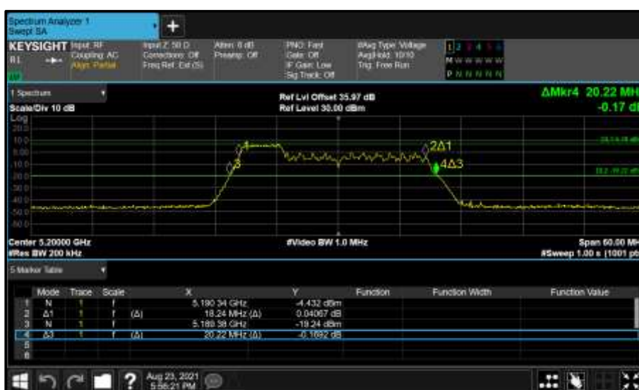
Figure 231 - Core 0 (A) 5200 MHz (CH40) 26 dB and 99% Bandwidth
