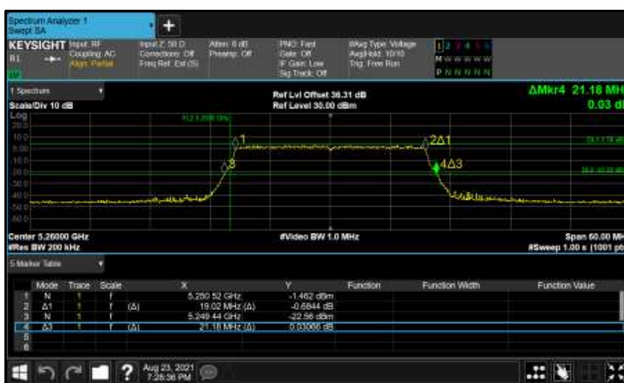
Figure 361 - Core 0 (A) 5260 MHz (CH52) 26 dB and 99% Bandwidth
