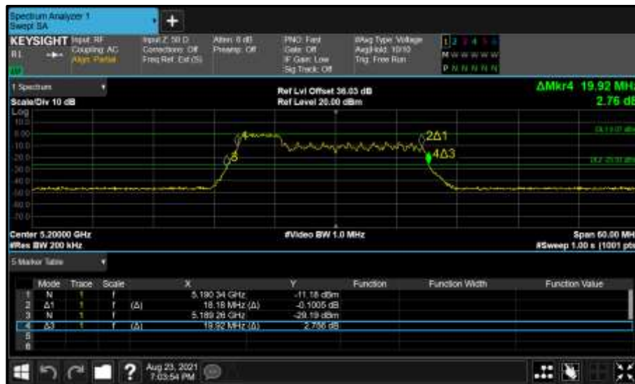
Figure 238 - Core 1 (B) 5200 MHz (CH40) 26 dB and 99% Bandwidth
