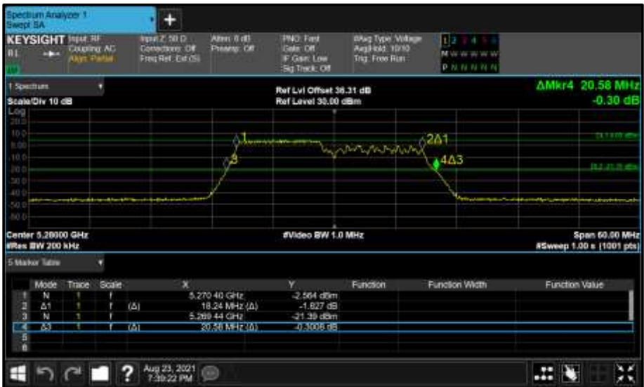
Figure 393 - Core 0 (A) 5280 MHz (CH56) 26 dB and 99% Bandwidth
