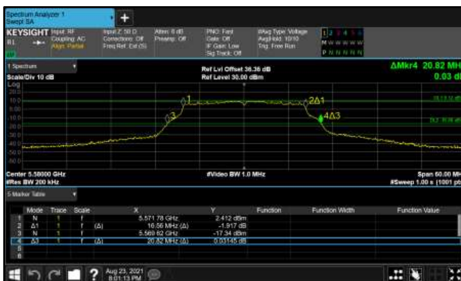
Figure 431 - Core 1 (B) 5580 MHz (CH116) 26 dB and 99% Bandwidth
