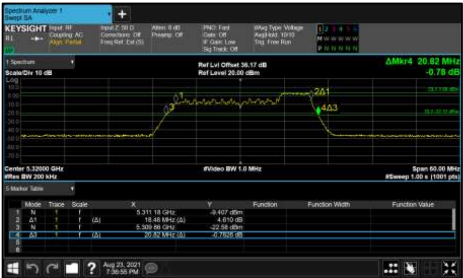
Figure 380 - Core 0 (A) 5320 MHz (CH64) 26 dB and 99% Bandwidth
