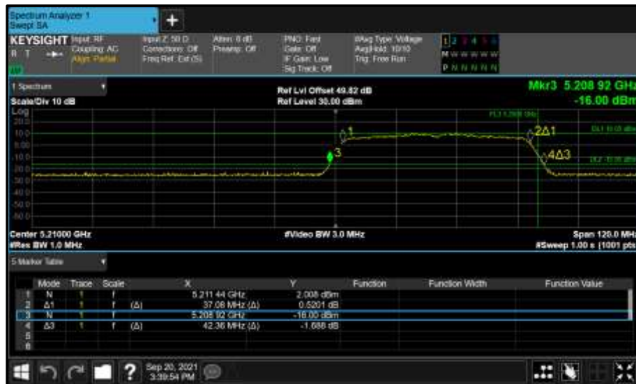
Figure 321 - Core 0 (A) 5210 MHz (CH42) 26 dB and 99% Bandwidth
