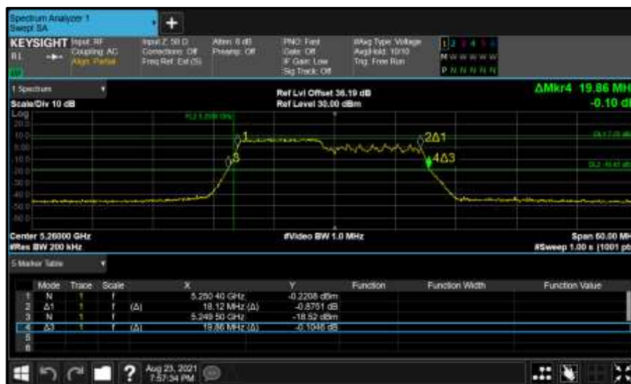
Figure 398 - Core 1 (B) 5260 MHz (CH52) 26 dB and 99% Bandwidth
