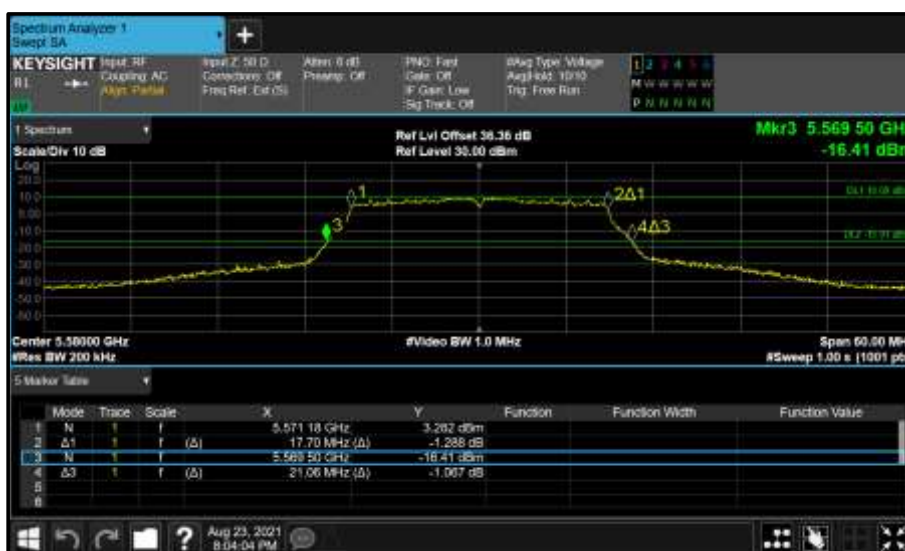
Figure 435 - Core 1 (B) 5580 MHz (CH116) 26 dB and 99% Bandwidth
