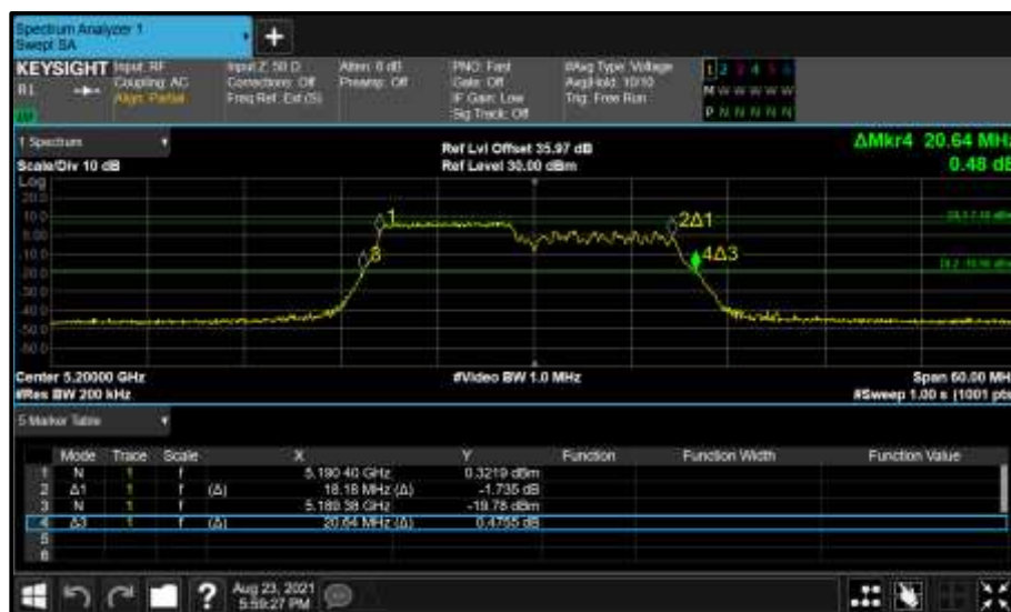
Figure 261 - Core 0 (A) 5200 MHz (CH40) 26 dB and 99% Bandwidth
