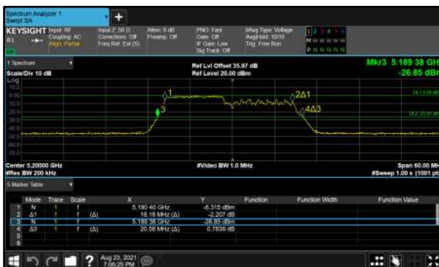
Figure 267 - Core 0 (A) 5200 MHz (CH40) 26 dB and 99% Bandwidth
