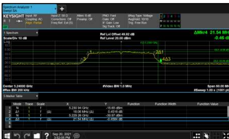
Figure 311 - Core 0 (A) 5240 MHz (CH48) 26 dB and 99% Bandwidth
