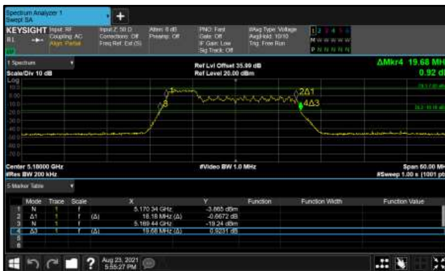
Figure 230 - Core 1 (B) 5180 MHz (CH36) 26 dB and 99% Bandwidth
