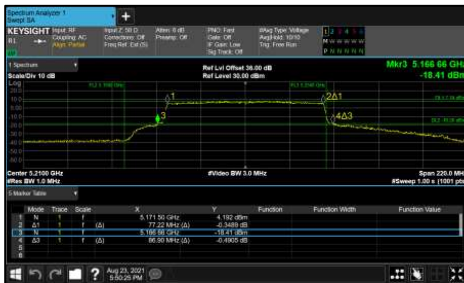
Figure 297 - Core 0 (A) 5210 MHz (CH42) 26 dB and 99% Bandwidth
