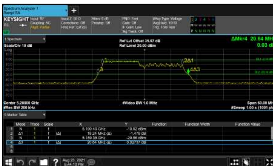
Figure 255 - Core 0 (A) 5200 MHz (CH40) 26 dB and 99% Bandwidth
