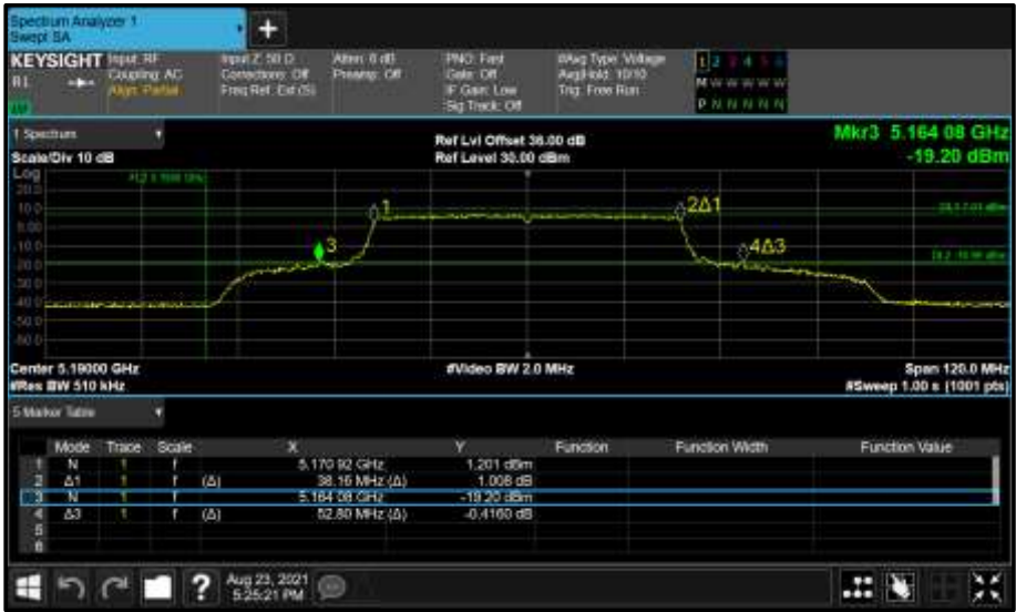
Figure 276 - Core 1 (B) 5190 MHz (CH38) 26 dB and 99% Bandwidth
