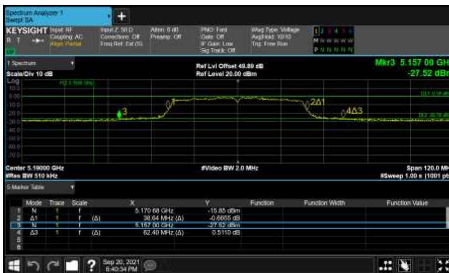
Figure 318 - Core 1 (B) 5190 MHz (CH38) 26 dB and 99% Bandwidth
