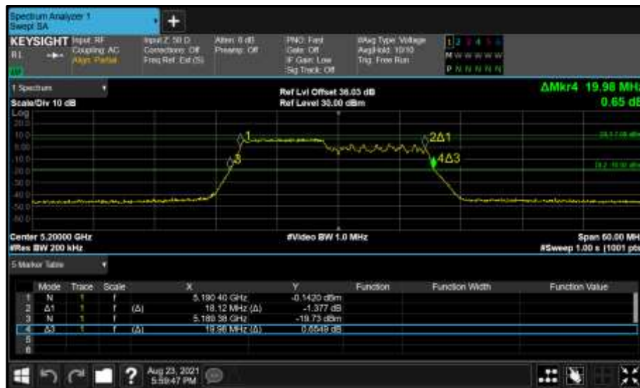
Figure 262 - Core 1 (B) 5200 MHz (CH40) 26 dB and 99% Bandwidth
