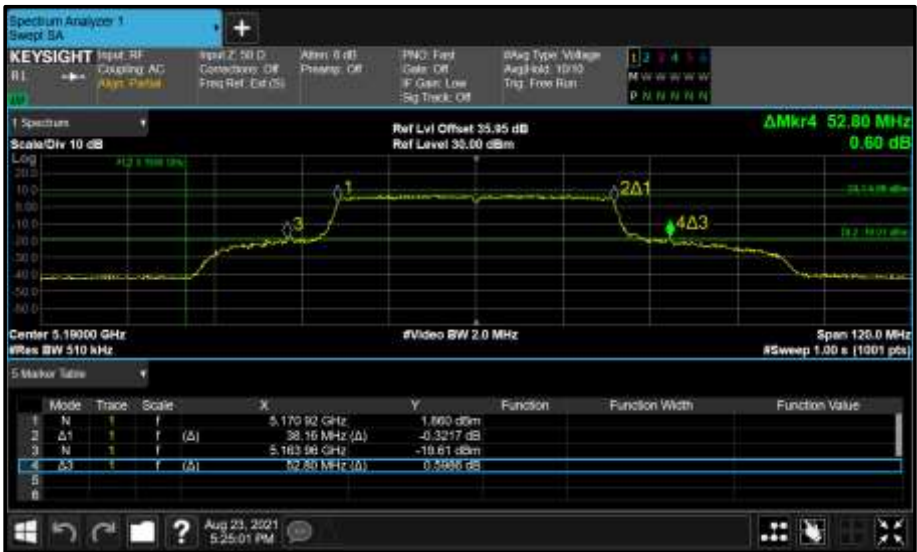
Figure 275 - Core 0 (A) 5190 MHz (CH38) 26 dB and 99% Bandwidth
