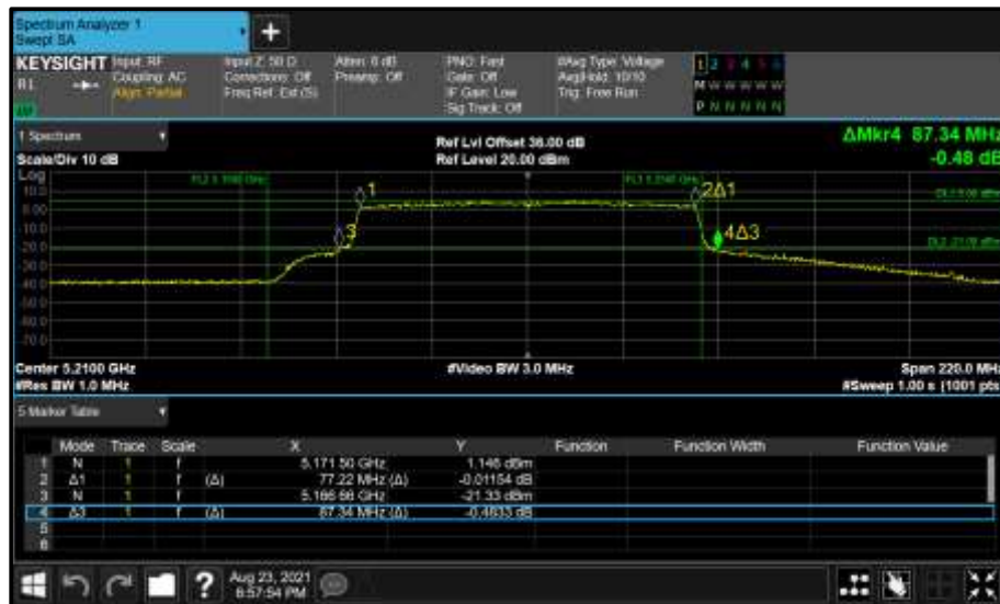
Figure 299 - Core 0 (A) 5210 MHz (CH42) 26 dB and 99% Bandwidth
