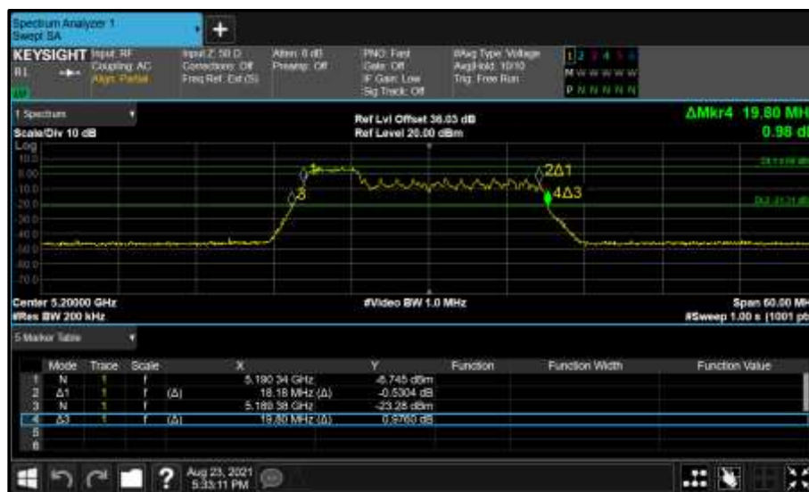
Figure 220 - Core 1 (B) 5200 MHz (CH40) 26 dB and 99% Bandwidth
