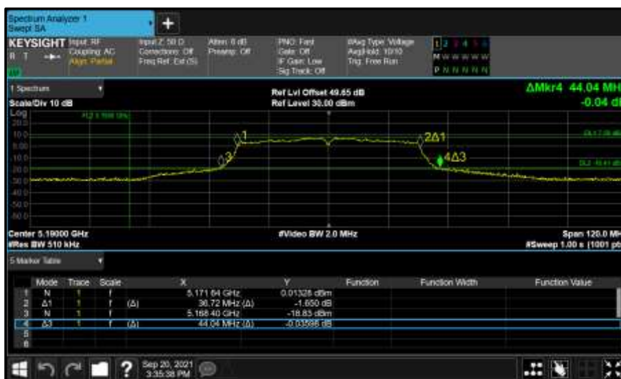
Figure 313 - Core 0 (A) 5190 MHz (CH38) 26 dB and 99% Bandwidth
