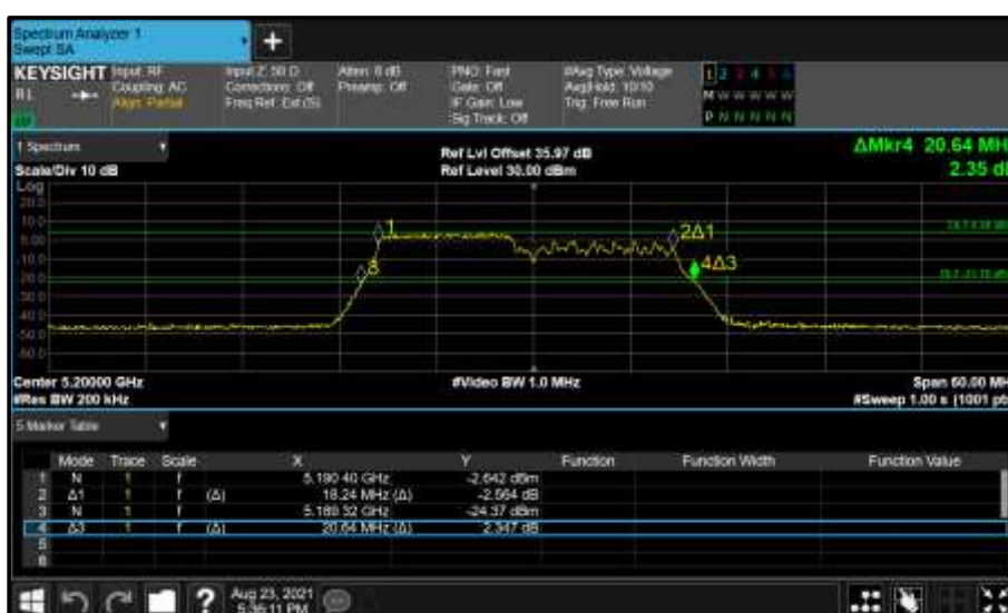
Figure 249 - Core 0 (A) 5200 MHz (CH40) 26 dB and 99% Bandwidth
