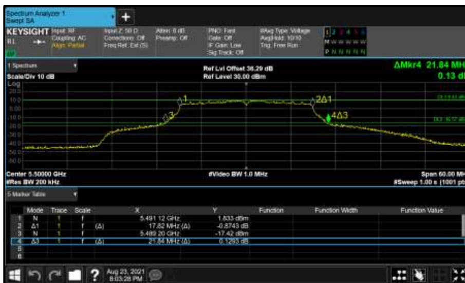
Figure 434 - Core 1 (B) 5500 MHz (CH100) 26 dB and 99% Bandwidth
