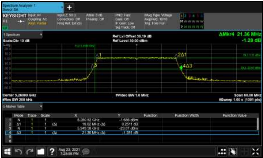
Figure 362 - Core 1 (B) 5260 MHz (CH52) 26 dB and 99% Bandwidth
