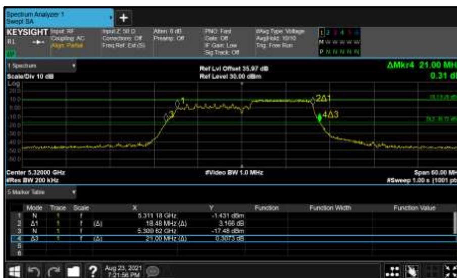
Figure 390 - Core 1 (B) 5320 MHz (CH64) 26 dB and 99% Bandwidth
