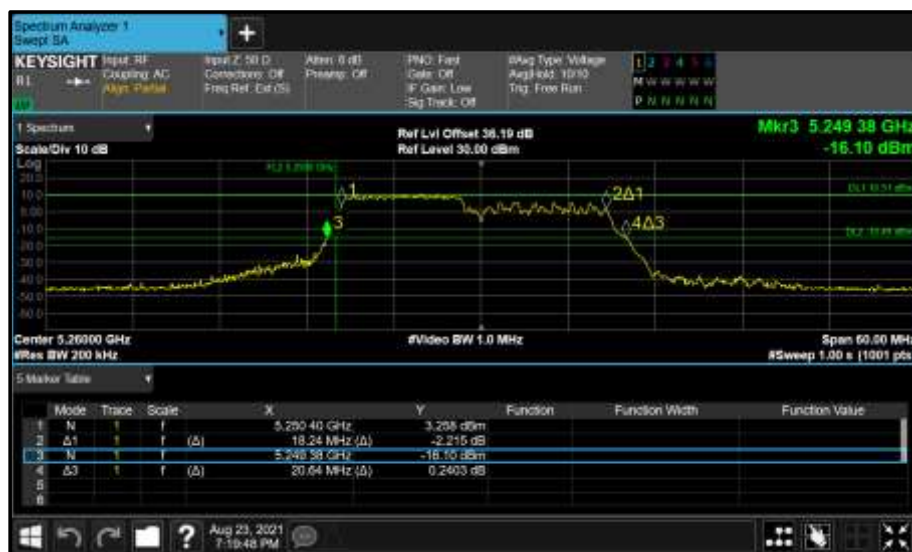
Figure 388 - Core 1 (B) 5260 MHz (CH52) 26 dB and 99% Bandwidth
