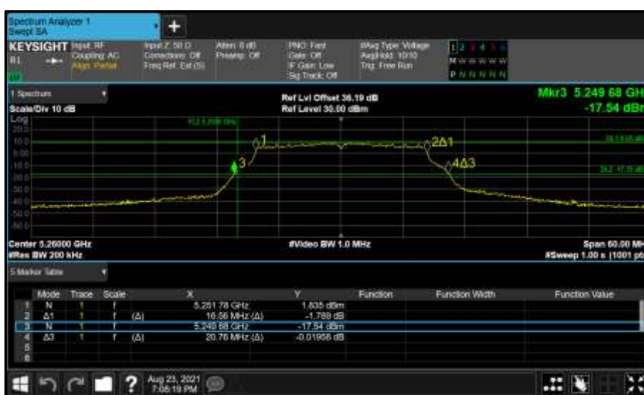
Figure 325 - Core 1 (B) 5260 MHz (CH52) 26 dB and 99% Bandwidth
