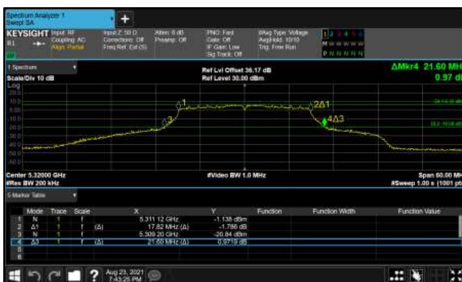
Figure 341 - Core 0 (A) 5320 MHz (CH64) 26 dB and 99% Bandwidth
