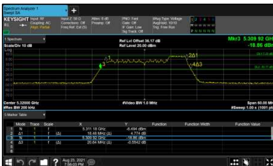
Figure 386 - Core 0 (A) 5320 MHz (CH64) 26 dB and 99% Bandwidth
