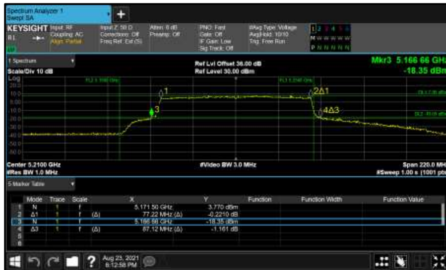
Figure 292 - Core 0 (A) 5210 MHz (CH42) 26 dB and 99% Bandwidth
