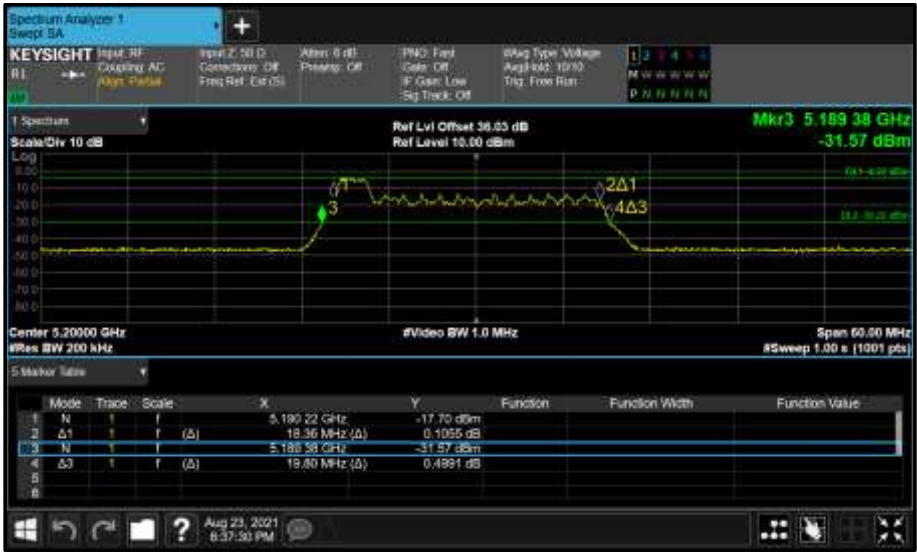
Figure 196 - Core 1 (B) 5200 MHz (CH40) 26 dB and 99% Bandwidth
