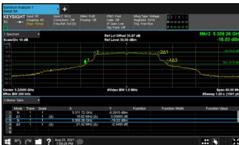
Figure 327 - Core 1 (B) 5320 MHz (CH64) 26 dB and 99% Bandwidth
