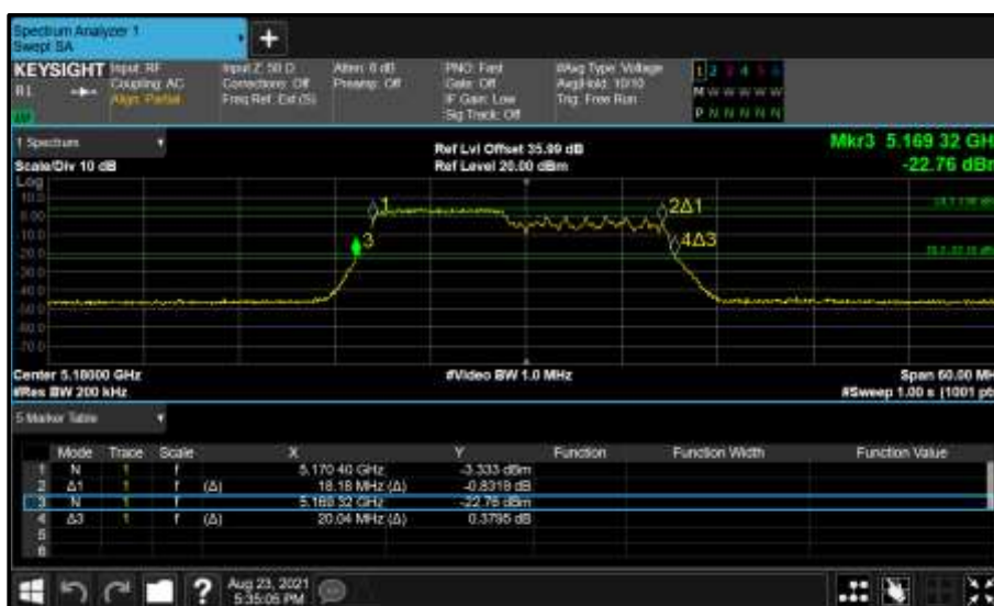
Figure 248 - Core 1 (B) 5180 MHz (CH36) 26 dB and 99% Bandwidth
