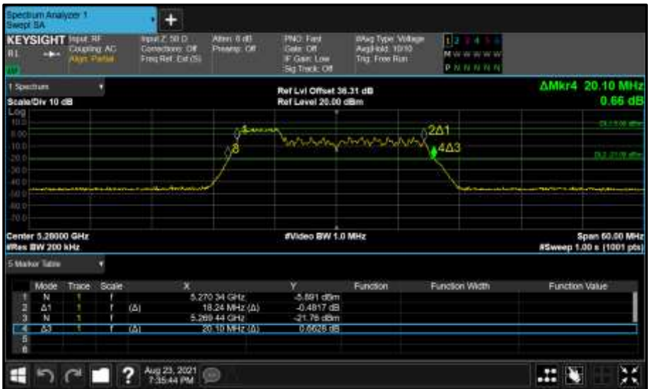
Figure 378 - Core 0 (A) 5280 MHz (CH56) 26 dB and 99% Bandwidth
