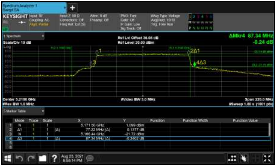
Figure 300 - Core 1 (B) 5210 MHz (CH42) 26 dB and 99% Bandwidth
