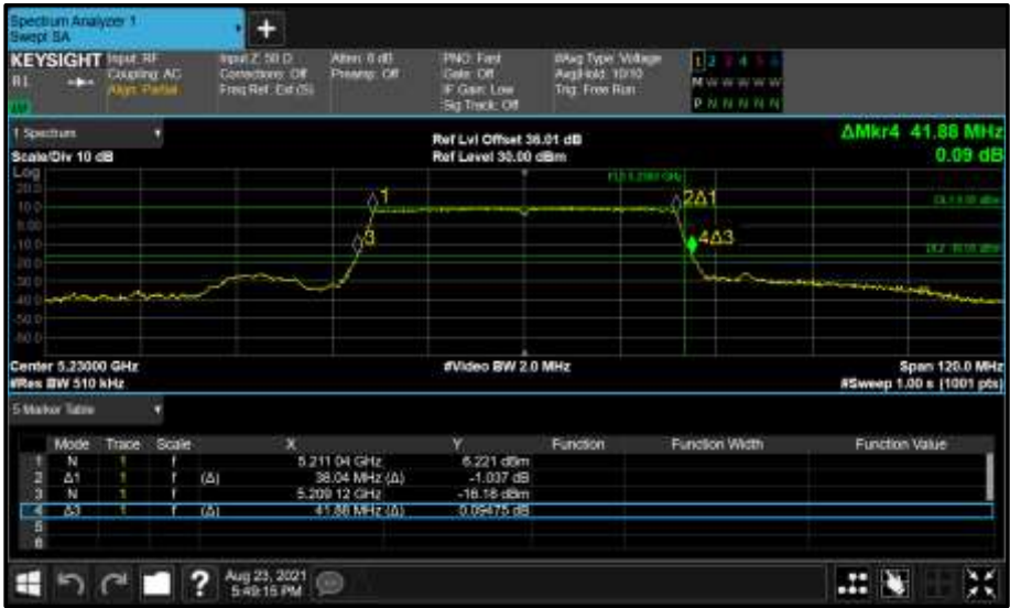
Figure 286 - Core 1 (B) 5230 MHz (CH46) 26 dB and 99% Bandwidth
