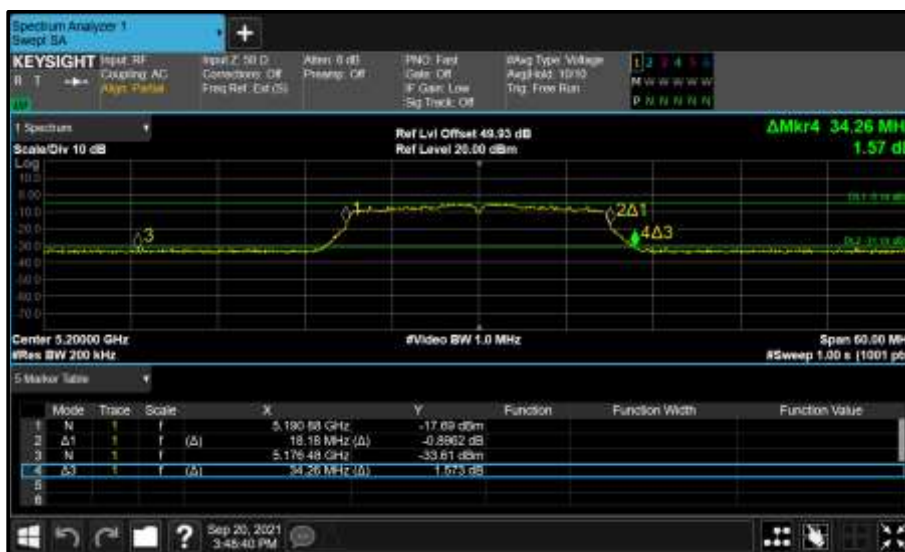
Figure 310 - Core 1 (B) 5200 MHz (CH40) 26 dB and 99% Bandwidth
