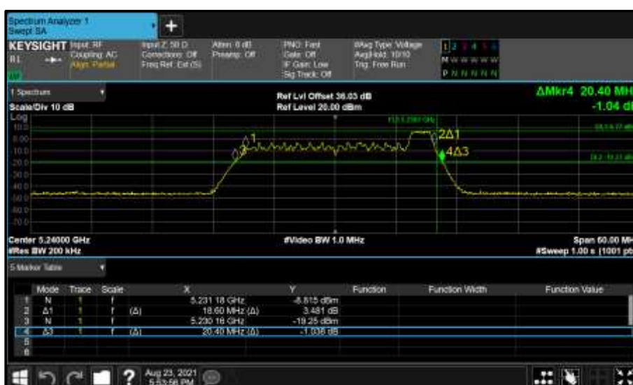
Figure 203 - Core 0 (A) 5240 MHz (CH48) 26 dB and 99% Bandwidth
