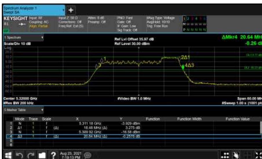
Figure 375 - Core 1 (B) 5320 MHz (CH64) 26 dB and 99% Bandwidth
