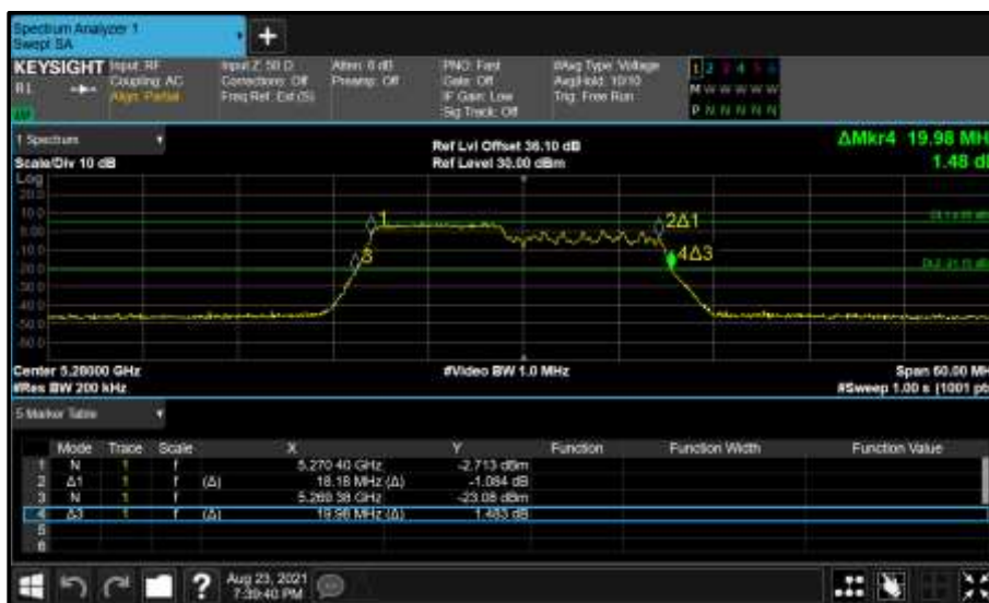
Figure 394 - Core 1 (B) 5280 MHz (CH56) 26 dB and 99% Bandwidth
