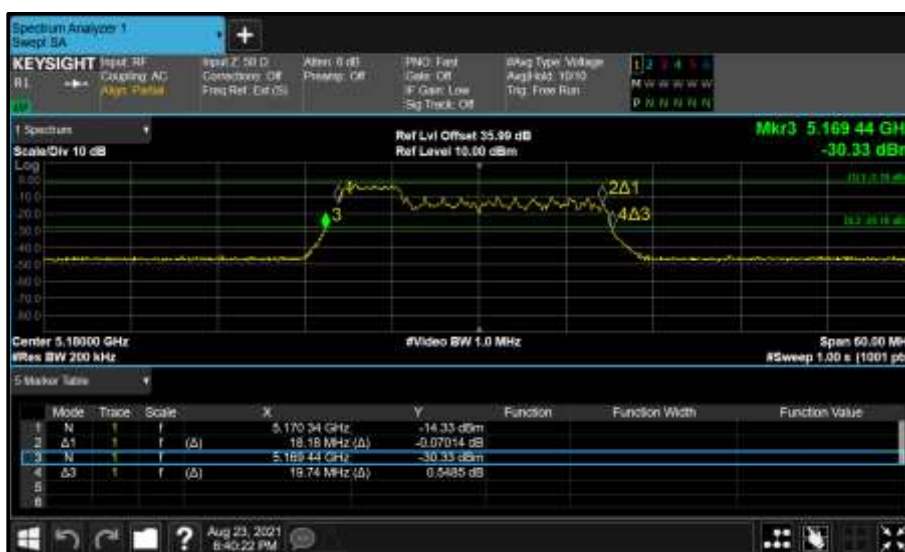
Figure 224 - Core 1 (B) 5180 MHz (CH36) 26 dB and 99% Bandwidth
