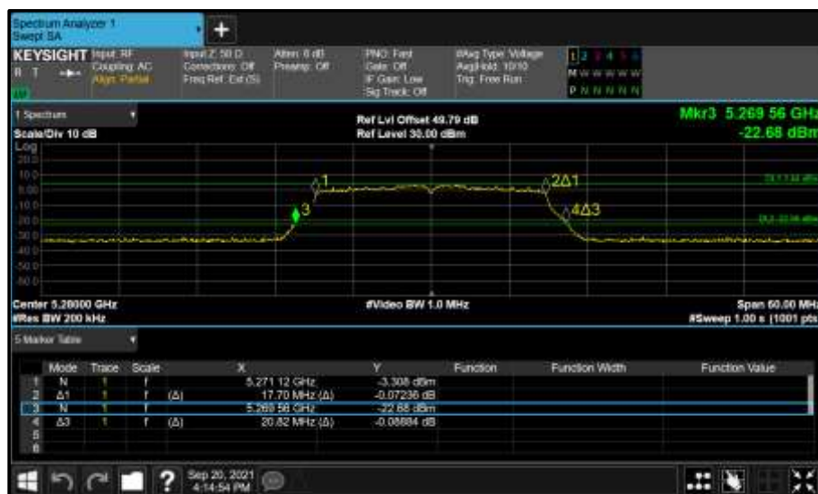
Figure 420 - Core 0 (A) 5280 MHz (CH56) 26 dB and 99% Bandwidth
