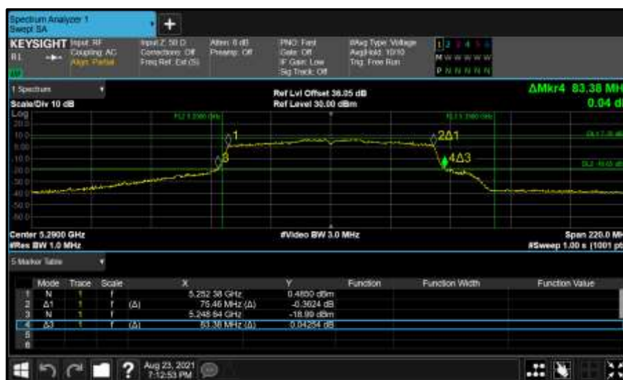
Figure 353 - Core 1 (B) 5290 MHz (CH58) 26 dB and 99% Bandwidth
