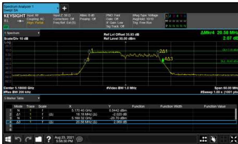
Figure 259 - Core 0 (A) 5180 MHz (CH36) 26 dB and 99% Bandwidth
