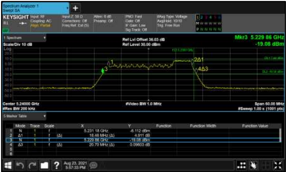
Figure 233 - Core 0 (A) 5240 MHz (CH48) 26 dB and 99% Bandwidth
