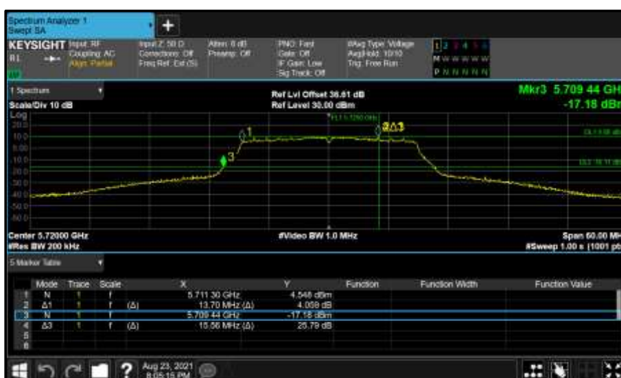
Figure 437 - Core 1 (B) 5720 MHz (CH144) 26 dB and 99% Bandwidth
