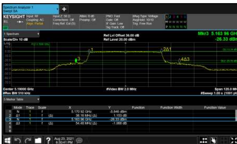
Figure 280 - Core 1 (B) 5190 MHz (CH38) 26 dB and 99% Bandwidth
