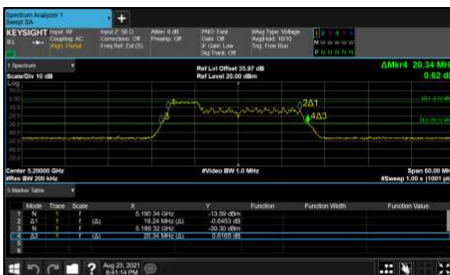
Figure 225 - Core 0 (A) 5200 MHz (CH40) 26 dB and 99% Bandwidth
