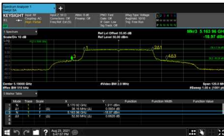
Figure 283 - Core 0 (A) 5190 MHz (CH38) 26 dB and 99% Bandwidth
