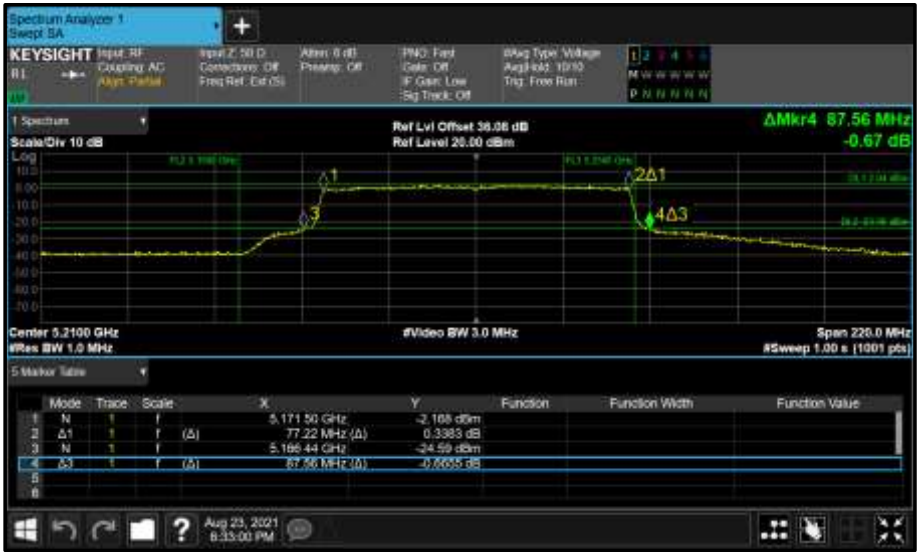
Figure 296 - Core 1 (B) 5210 MHz (CH42) 26 dB and 99% Bandwidth
