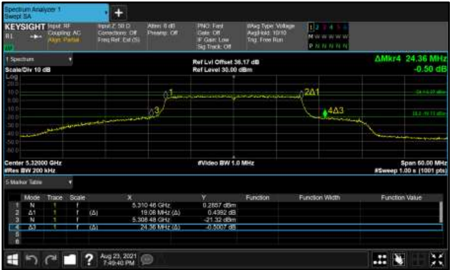
Figure 371 - Core 0 (A) 5320 MHz (CH64) 26 dB and 99% Bandwidth
