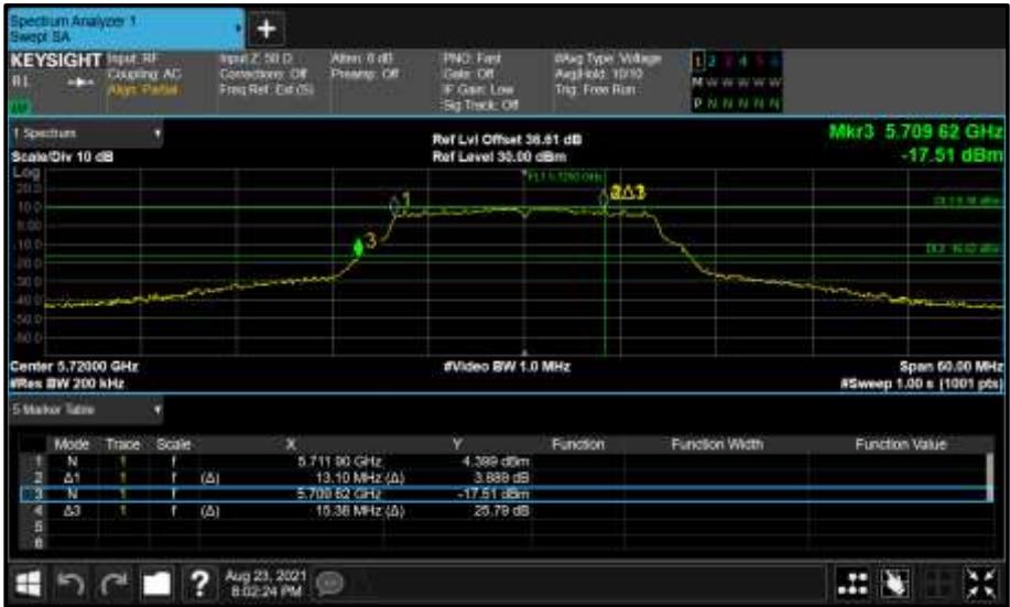
Figure 433 - Core 1 (B) 5720 MHz (CH144) 26 dB and 99% Bandwidth
