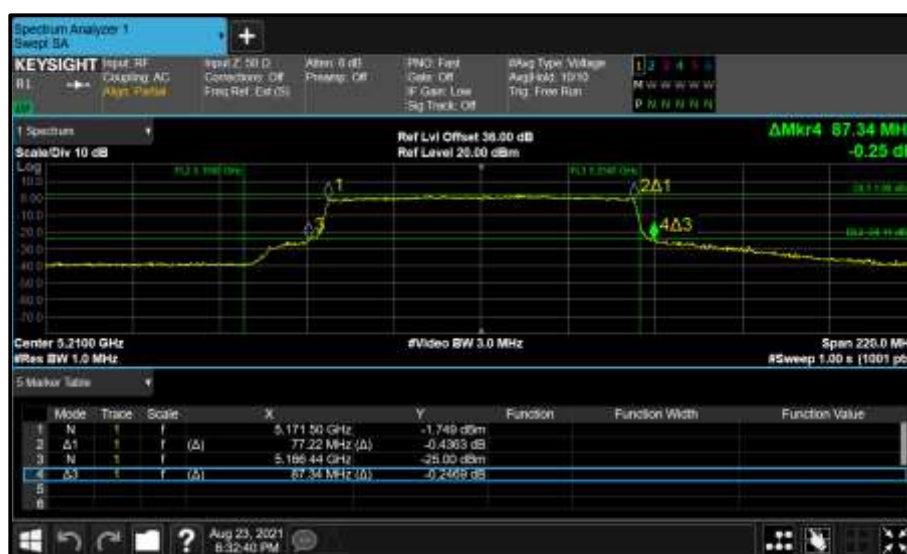
Figure 295 - Core 0 (A) 5210 MHz (CH42) 26 dB and 99% Bandwidth
