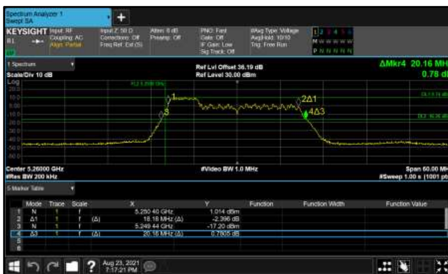
Figure 373 - Core 1 (B) 5260 MHz (CH52) 26 dB and 99% Bandwidth
