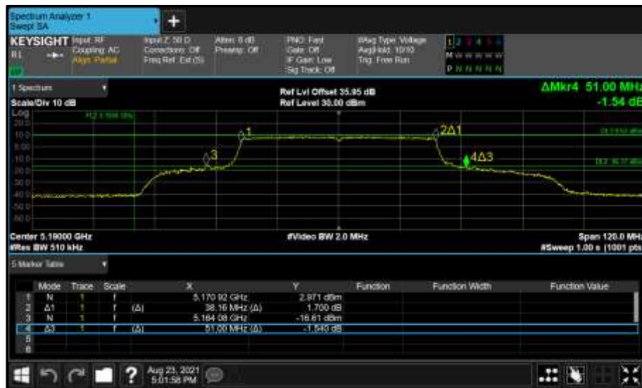
Figure 271 - Core 0 (A) 5190 MHz (CH38) 26 dB and 99% Bandwidth
