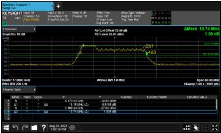
Figure 236 - Core 1 (B) 5180 MHz (CH36) 26 dB and 99% Bandwidth
