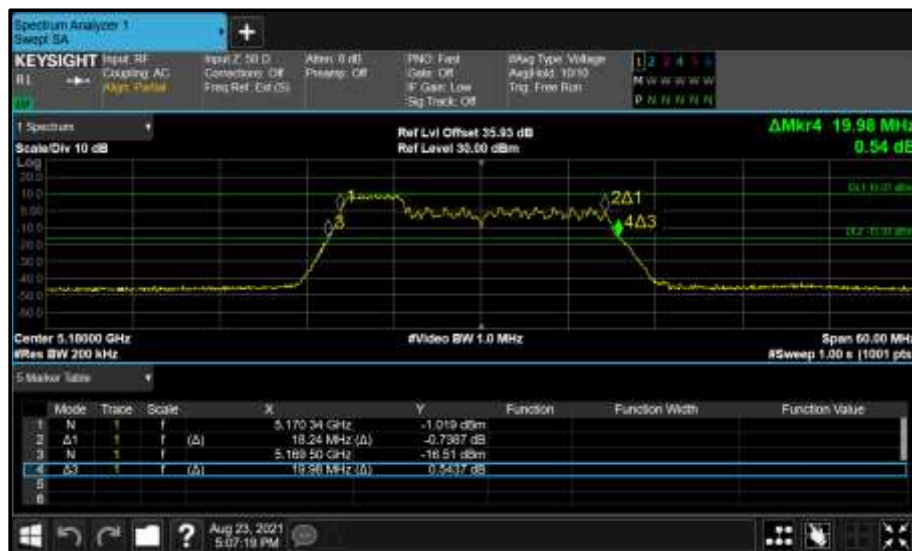
Figure 211 - Core 0 (A) 5180 MHz (CH36) 26 dB and 99% Bandwidth
