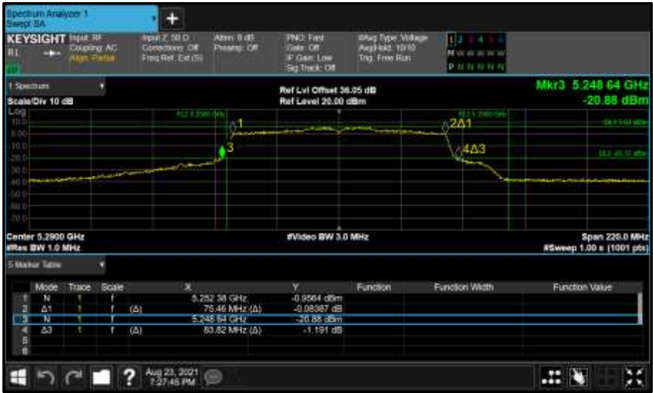
Figure 355 - Core 1 (B) 5290 MHz (CH58) 26 dB and 99% Bandwidth
