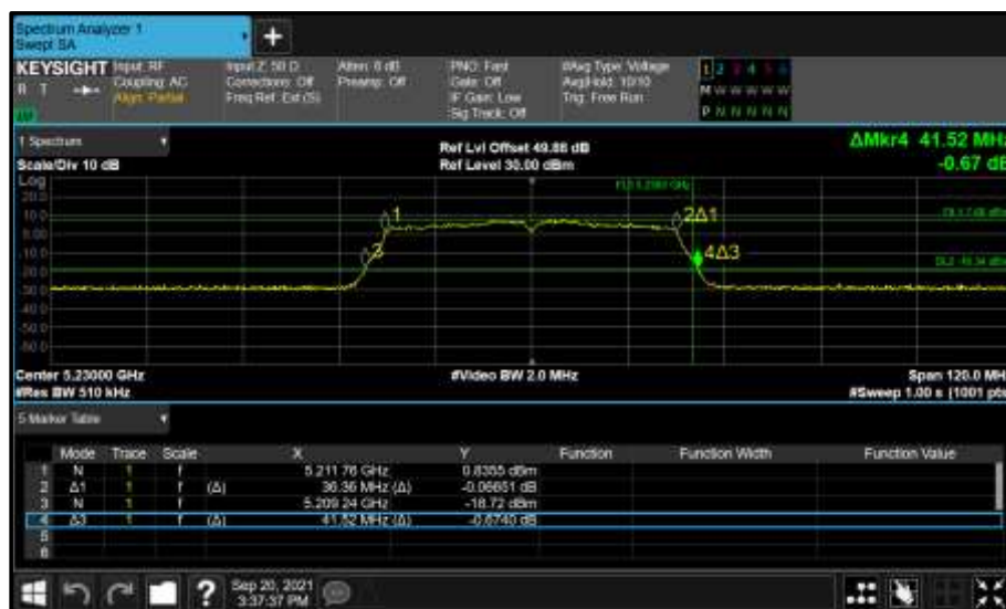
Figure 315 - Core 0 (A) 5230 MHz (CH46) 26 dB and 99% Bandwidth
