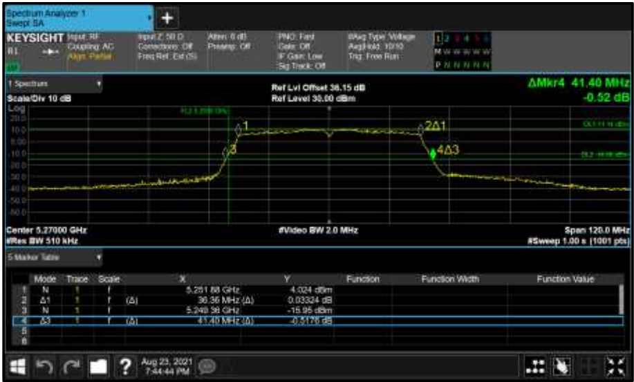
Figure 350 - Core 1 (B) 5270 MHz (CH54) 26 dB and 99% Bandwidth
