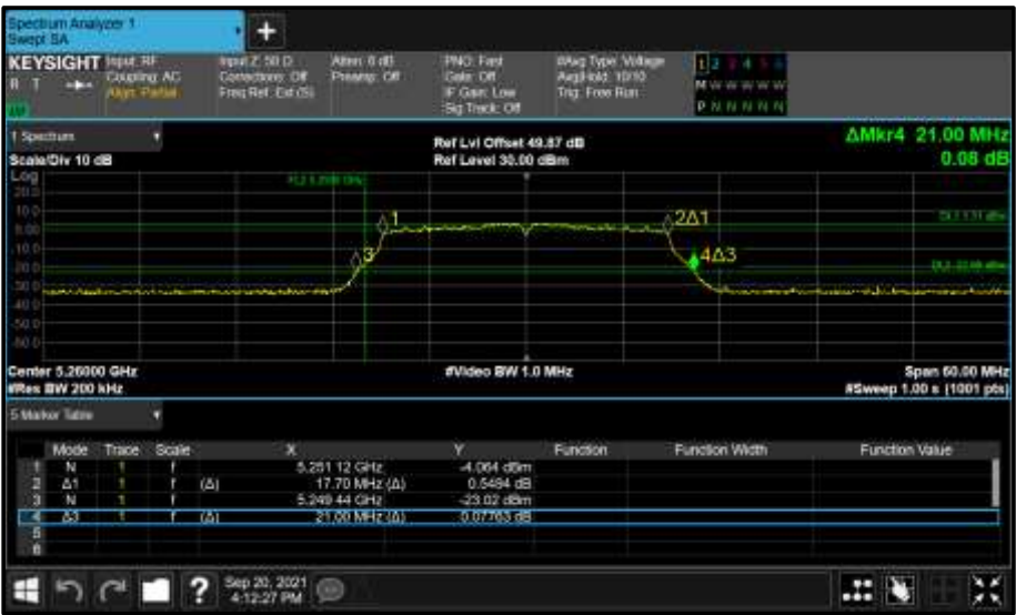
Figure 418 - Core 0 (A) 5260 MHz (CH52) 26 dB and 99% Bandwidth
