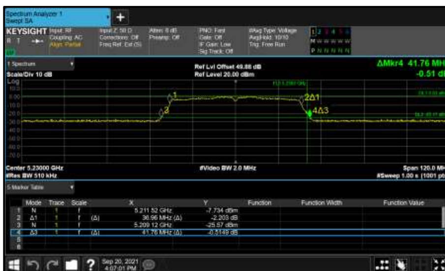
Figure 319 - Core 0 (A) 5230 MHz (CH46) 26 dB and 99% Bandwidth
