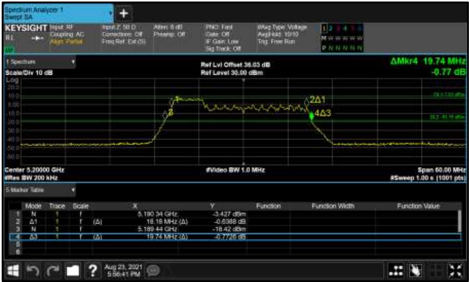
Figure 232 - Core 1 (B) 5200 MHz (CH40) 26 dB and 99% Bandwidth
