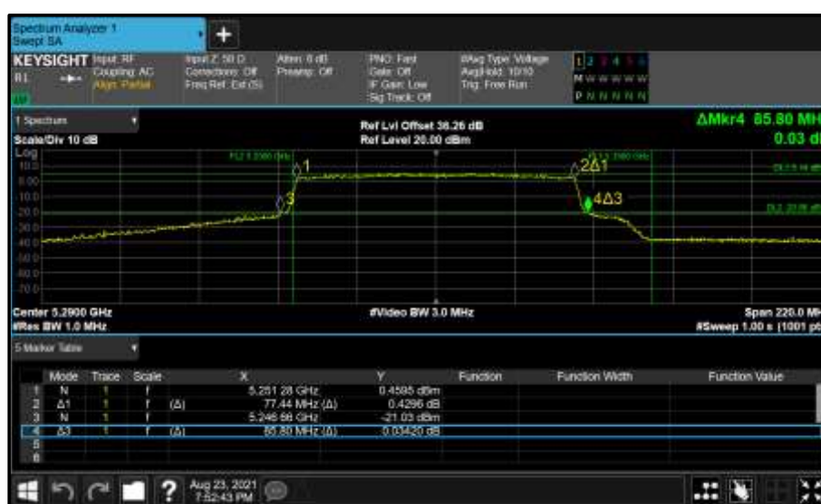
Figure 416 - Core 0 (A) 5290 MHz (CH58) 26 dB and 99% Bandwidth
