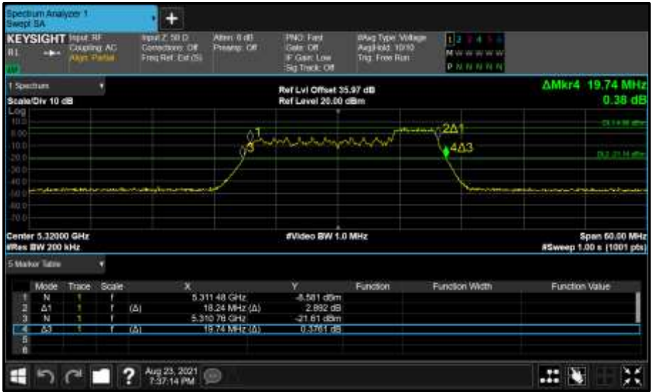
Figure 381 - Core 1 (B) 5320 MHz (CH64) 26 dB and 99% Bandwidth
