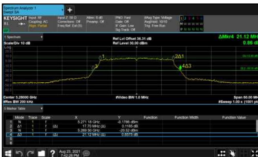
Figure 339 - Core 0 (A) 5280 MHz (CH56) 26 dB and 99% Bandwidth
