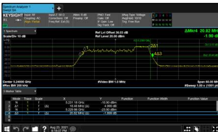
Figure 216 - Core 0 (A) 5240 MHz (CH48) 26 dB and 99% Bandwidth
