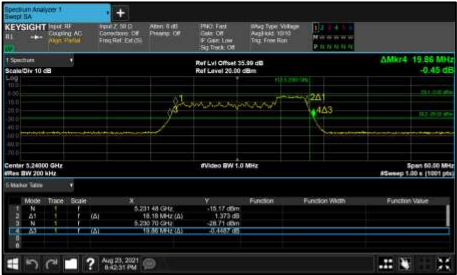
Figure 228 - Core 1 (B) 5240 MHz (CH48) 26 dB and 99% Bandwidth
