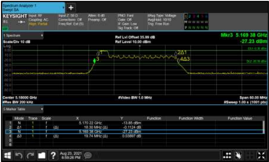
Figure 206 - Core 1 (B) 5180 MHz (CH36) 26 dB and 99% Bandwidth
