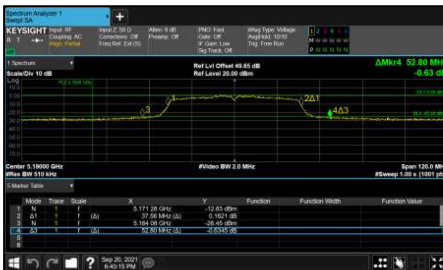
Figure 317 - Core 0 (A) 5190 MHz (CH38) 26 dB and 99% Bandwidth
