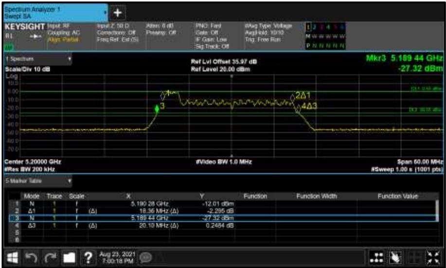
Figure 207 - Core 0 (A) 5200 MHz (CH40) 26 dB and 99% Bandwidth
