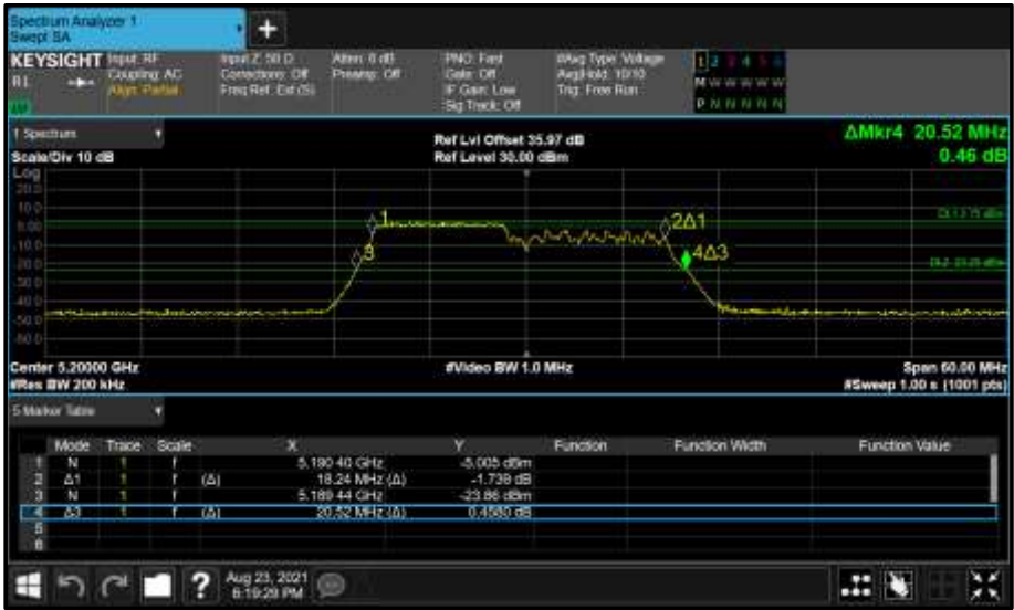
Figure 245 - Core 0 (A) 5200 MHz (CH40) 26 dB and 99% Bandwidth
