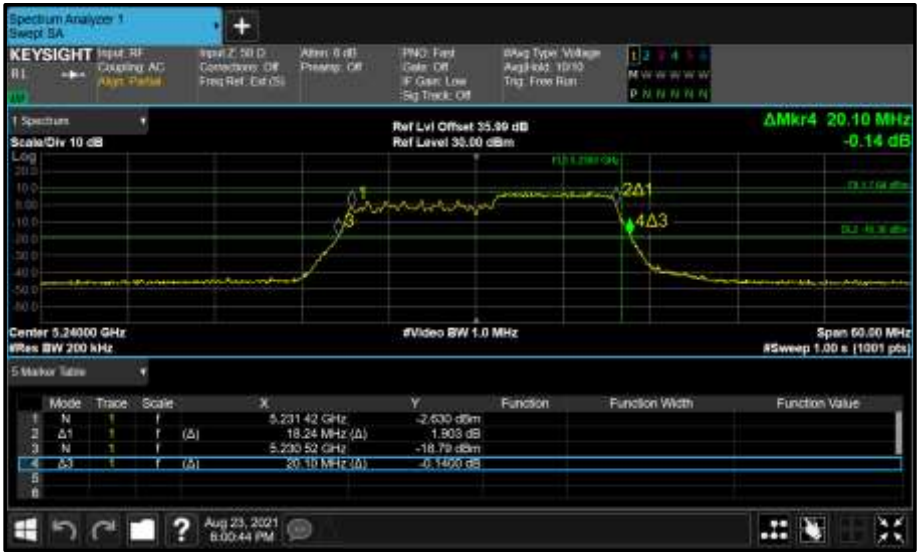
Figure 264 - Core 1 (B) 5240 MHz (CH48) 26 dB and 99% Bandwidth
