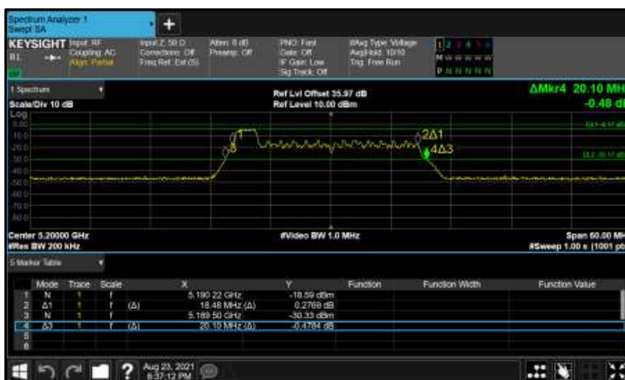
Figure 195 - Core 0 (A) 5200 MHz (CH40) 26 dB and 99% Bandwidth
