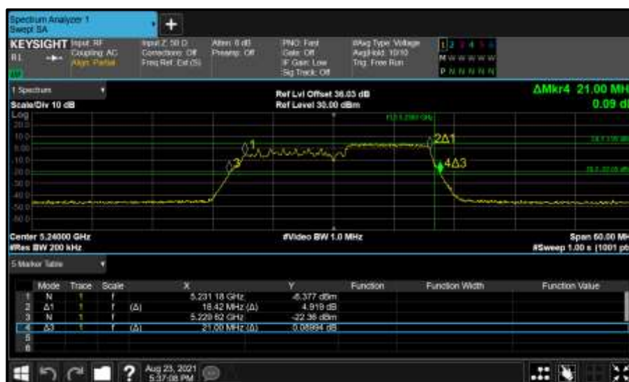
Figure 251 - Core 0 (A) 5240 MHz (CH48) 26 dB and 99% Bandwidth
