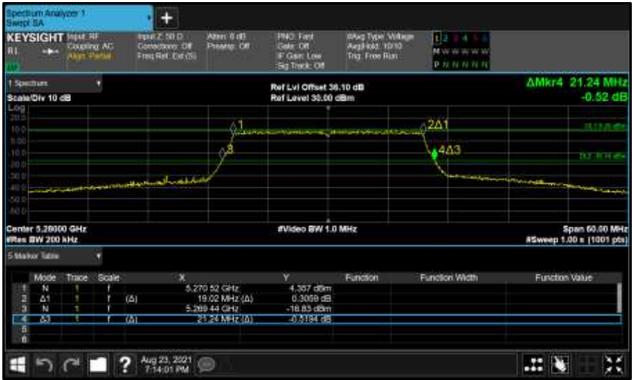
Figure 359 - Core 1 (B) 5280 MHz (CH56) 26 dB and 99% Bandwidth
