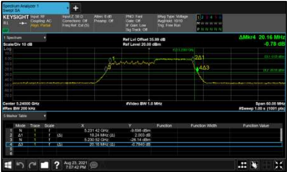
Figure 270 - Core 1 (B) 5240 MHz (CH48) 26 dB and 99% Bandwidth
