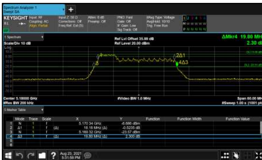
Figure 218 - Core 1 (B) 5180 MHz (CH36) 26 dB and 99% Bandwidth
