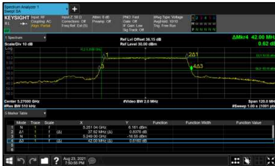
Figure 410 - Core 1 (B) 5270 MHz (CH54) 26 dB and 99% Bandwidth
