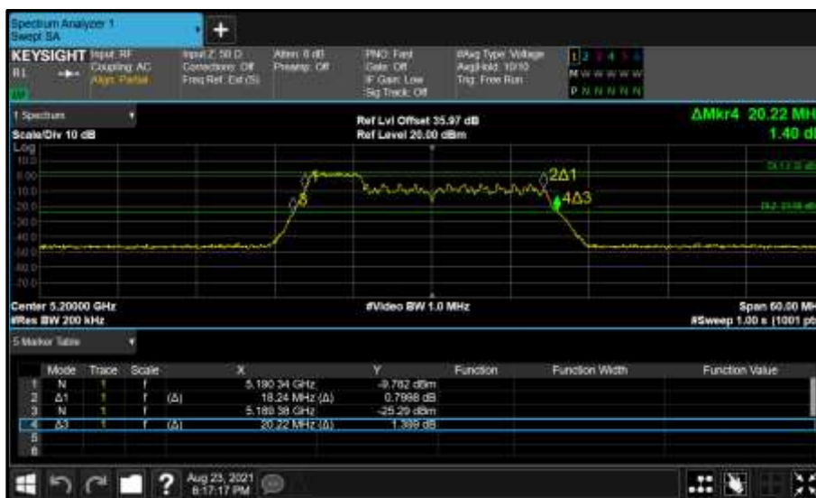
Figure 215 - Core 0 (A) 5200 MHz (CH40) 26 dB and 99% Bandwidth
