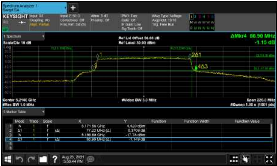
Figure 298 - Core 1 (B) 5210 MHz (CH42) 26 dB and 99% Bandwidth
