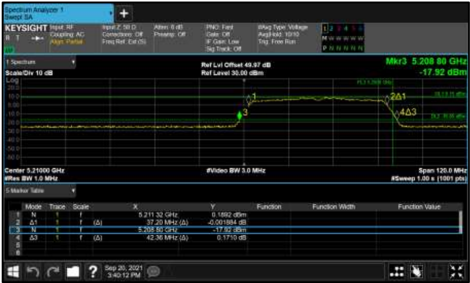
Figure 322 - Core 1 (B) 5210 MHz (CH42) 26 dB and 99% Bandwidth
