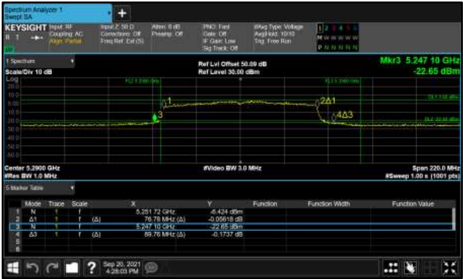
Figure 429 - Core 1 (B) 5290 MHz (CH58) 26 dB and 99% Bandwidth
