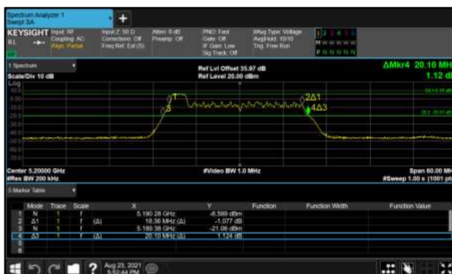
Figure 201 - Core 0 (A) 5200 MHz (CH40) 26 dB and 99% Bandwidth
