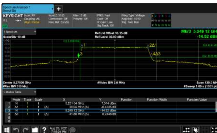
Figure 403 - Core 1 (B) 5270 MHz (CH54) 26 dB and 99% Bandwidth
