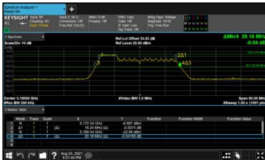
Figure 217 - Core 0 (A) 5180 MHz (CH36) 26 dB and 99% Bandwidth
