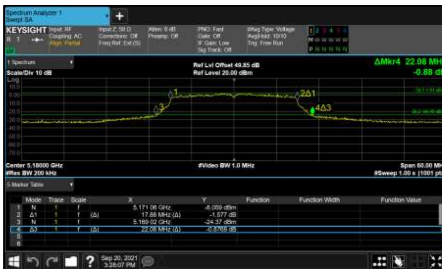
Figure 302 - Core 1 (B) 5180 MHz (CH36) 26 dB and 99% Bandwidth
