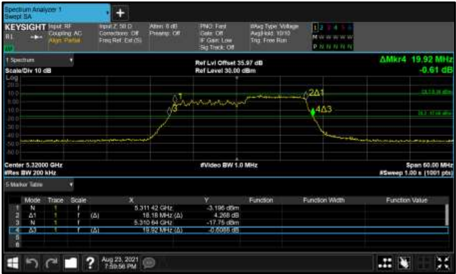
Figure 402 - Core 1 (B) 5320 MHz (CH64) 26 dB and 99% Bandwidth
