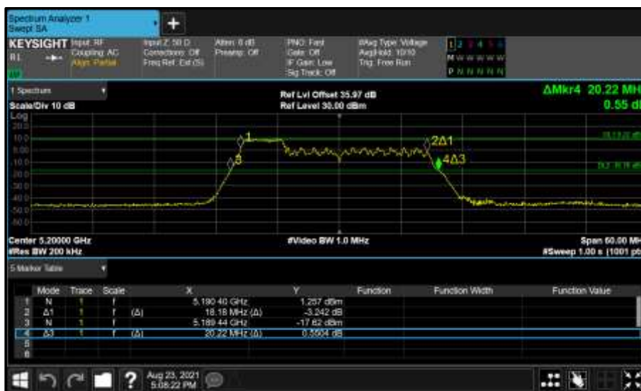
Figure 212 - Core 0 (A) 5200 MHz (CH40) 26 dB and 99% Bandwidth
