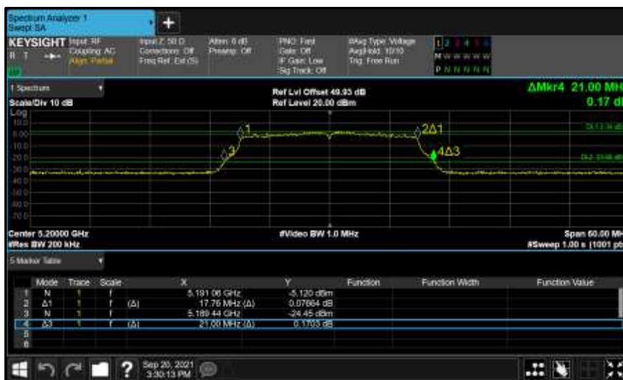
Figure 304 - Core 1 (B) 5200 MHz (CH40) 26 dB and 99% Bandwidth
