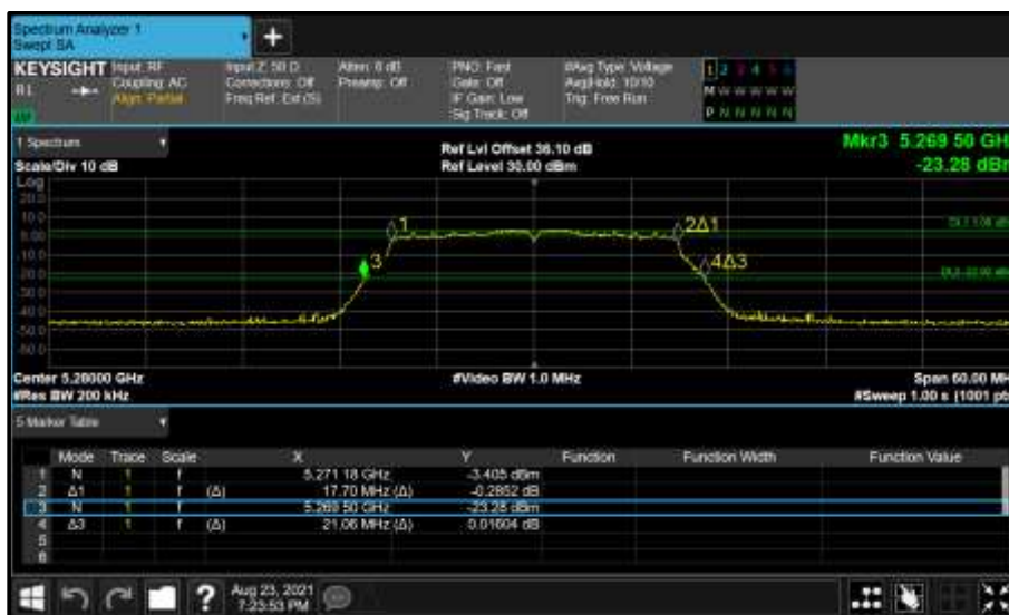
Figure 334 - Core 1 (B) 5280 MHz (CH56) 26 dB and 99% Bandwidth
