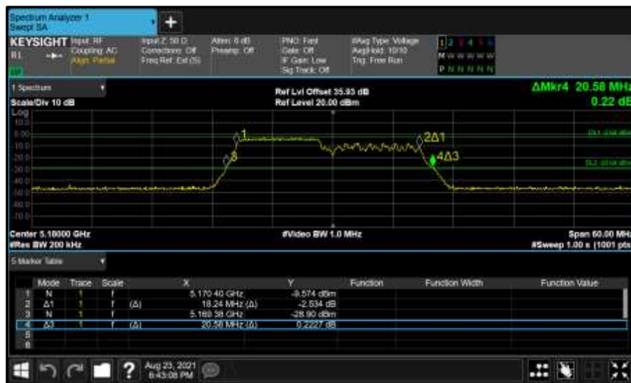
Figure 253 - Core 0 (A) 5180 MHz (CH36) 26 dB and 99% Bandwidth
