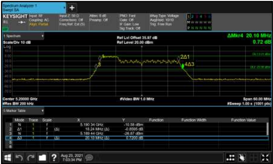
Figure 237 - Core 0 (A) 5200 MHz (CH40) 26 dB and 99% Bandwidth
