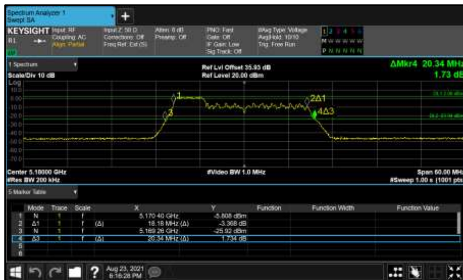
Figure 214 - Core 0 (A) 5180 MHz (CH36) 26 dB and 99% Bandwidth
