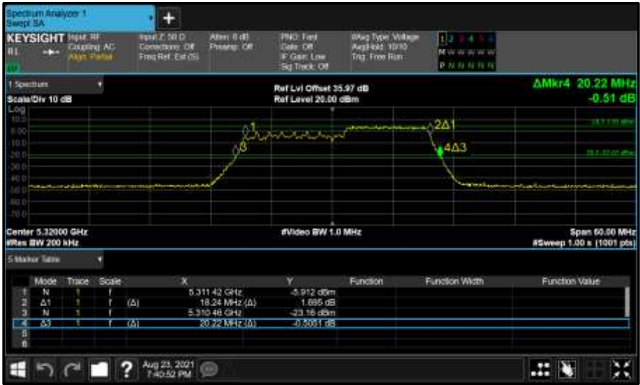
Figure 396 - Core 1 (B) 5320 MHz (CH64) 26 dB and 99% Bandwidth
