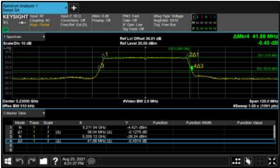
Figure 282 - Core 1 (B) 5230 MHz (CH46) 26 dB and 99% Bandwidth
