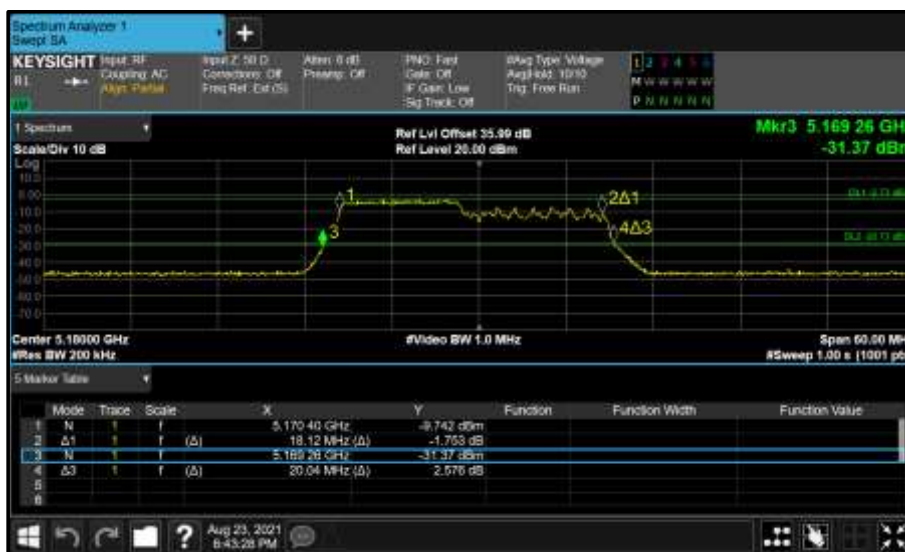
Figure 254 - Core 1 (B) 5180 MHz (CH36) 26 dB and 99% Bandwidth
