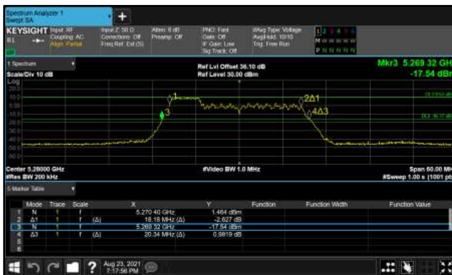
Figure 374 - Core 1 (B) 5280 MHz (CH56) 26 dB and 99% Bandwidth
