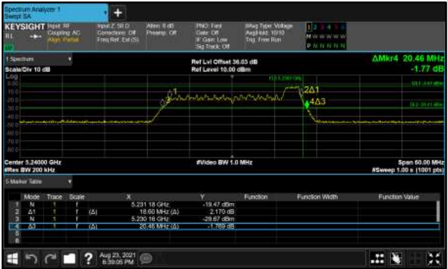
Figure 197 - Core 0 (A) 5240 MHz (CH48) 26 dB and 99% Bandwidth
