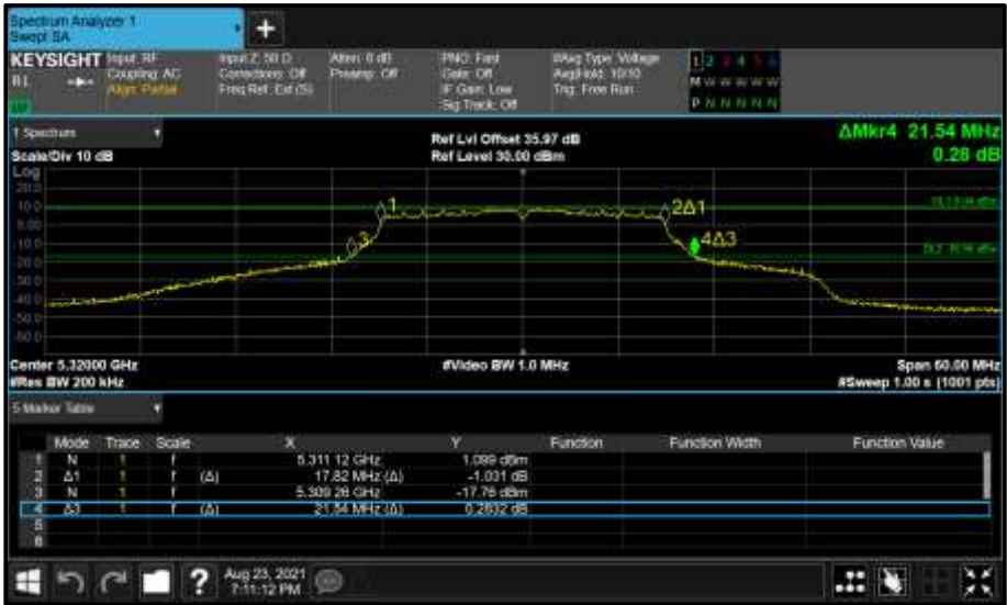
Figure 330 - Core 1 (B) 5320 MHz (CH64) 26 dB and 99% Bandwidth
