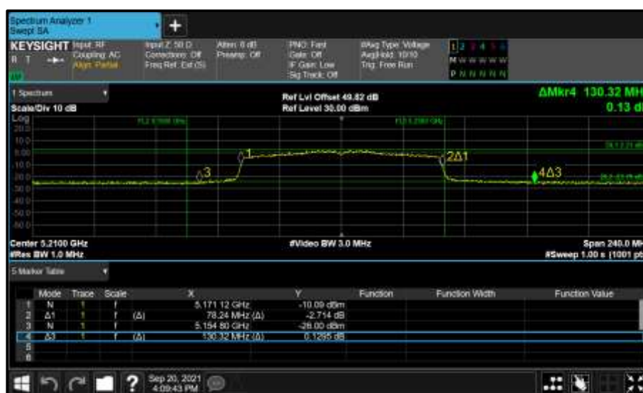
Figure 323 - Core 0 (A) 5210 MHz (CH42) 26 dB and 99% Bandwidth
