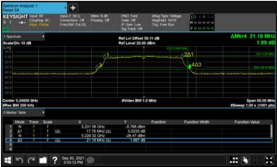
Figure 306 - Core 1 (B) 5240 MHz (CH48) 26 dB and 99% Bandwidth
