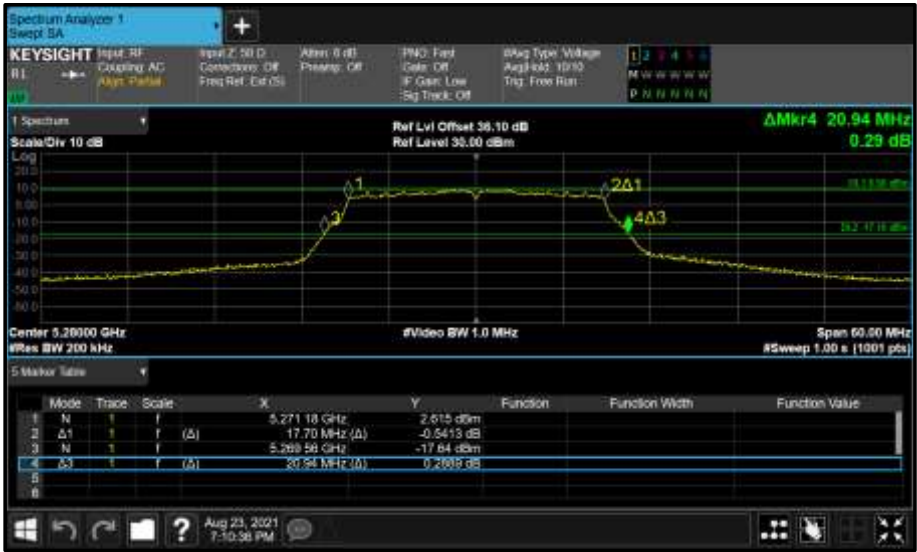
Figure 329 - Core 1 (B) 5280 MHz (CH56) 26 dB and 99% Bandwidth
