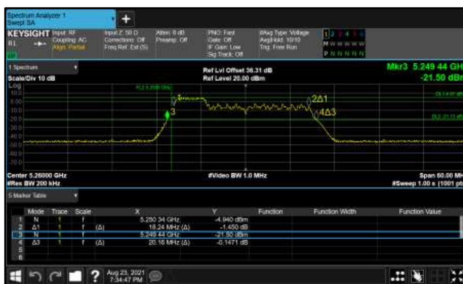
Figure 376 - Core 0 (A) 5260 MHz (CH52) 26 dB and 99% Bandwidth
