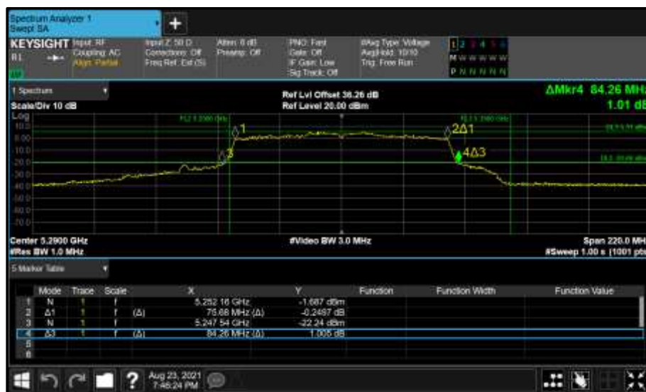
Figure 356 - Core 0 (A) 5290 MHz (CH58) 26 dB and 99% Bandwidth
