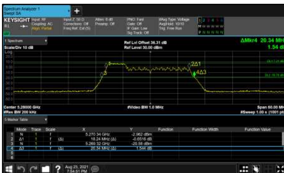
Figure 384 - Core 0 (A) 5280 MHz (CH56) 26 dB and 99% Bandwidth
