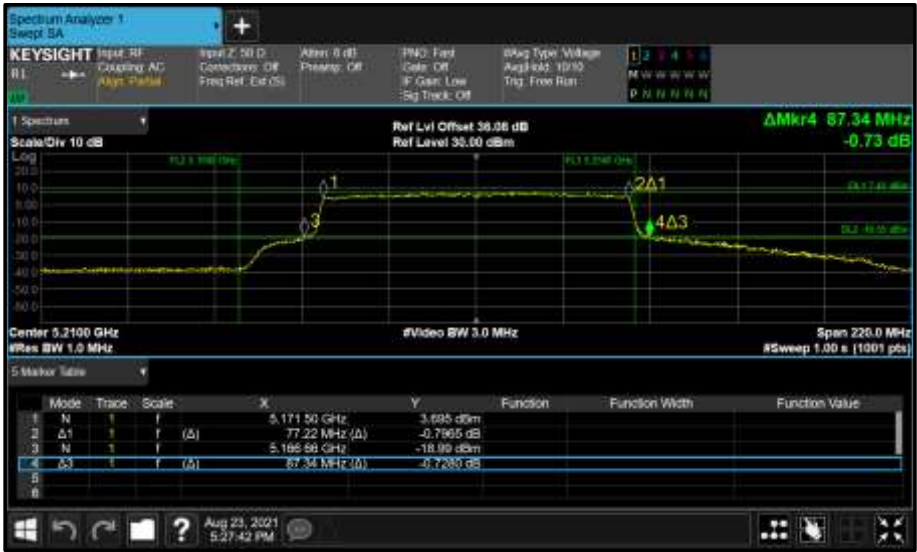
Figure 294 - Core 1 (B) 5210 MHz (CH42) 26 dB and 99% Bandwidth
