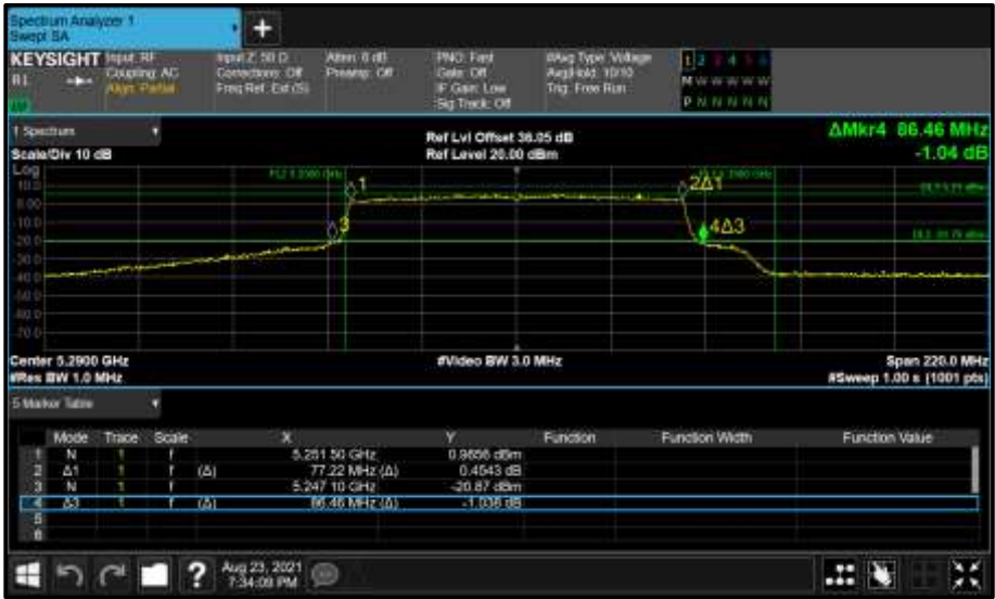
Figure 415 - Core 1 (B) 5290 MHz (CH58) 26 dB and 99% Bandwidth
