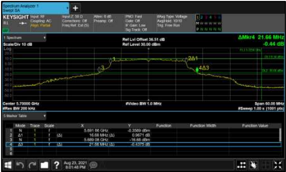
Figure 432 - Core 1 (B) 5700 MHz (CH140) 26 dB and 99% Bandwidth
