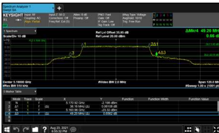
Figure 287 - Core 0 (A) 5190 MHz (CH38) 26 dB and 99% Bandwidth
