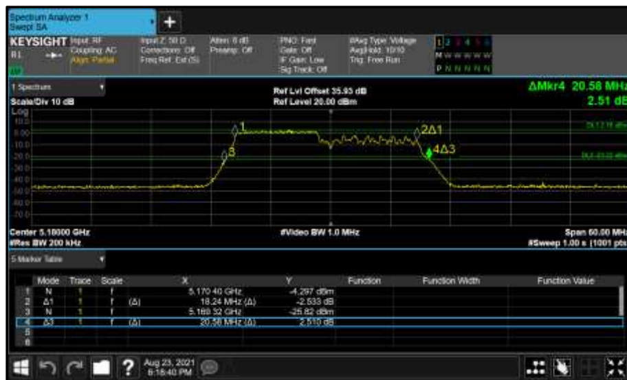
Figure 244 - Core 0 (A) 5180 MHz (CH36) 26 dB and 99% Bandwidth
