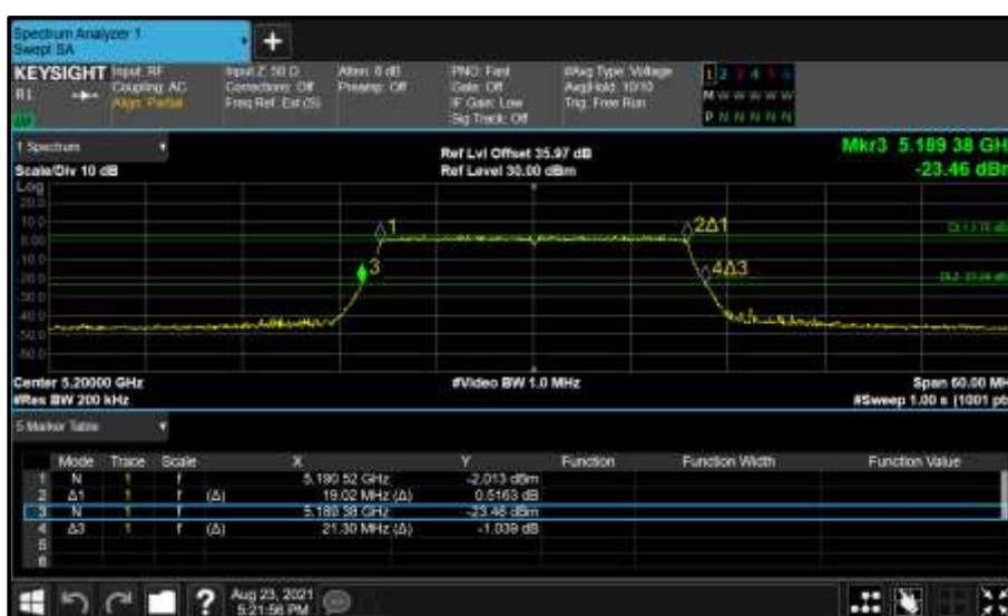
Figure 159 - Core 0 (A) 5200 MHz (CH40) 26 dB and 99% Bandwidth
