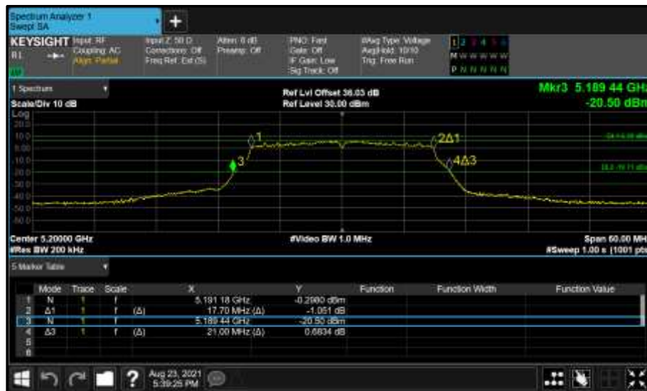
Figure 112 - Core 1 (B) 5200 MHz (CH40) 26 dB and 99% Bandwidth
