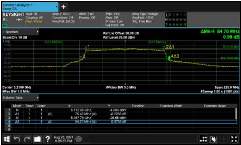
Figure 146 - Core 1 (B) 5210 MHz (CH42) 26 dB and 99% Bandwidth
