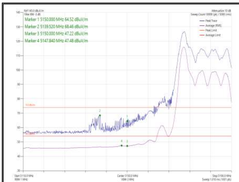
Figure 18 - 802.11ax HE20 SDM, Cores 0-1, 26-0 - 5180 MHz Band Edge Frequency 5150 MHz
