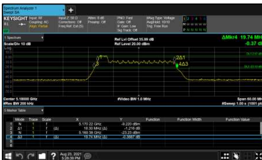
Figure 188 - Core 1 (B) 5180 MHz (CH36) 26 dB and 99% Bandwidth
