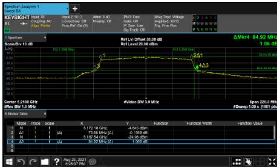
Figure 145 - Core 0 (A) 5210 MHz (CH42) 26 dB and 99% Bandwidth
