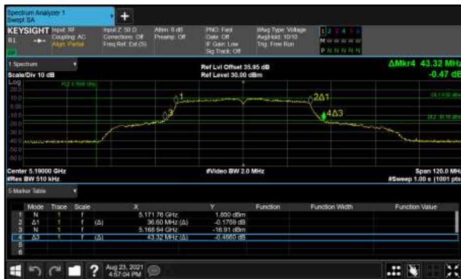
Figure 121 - Core 0 (A) 5190 MHz (CH38) 26 dB and 99% Bandwidth
