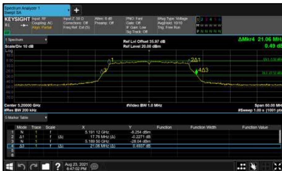
Figure 117 - Core 0 (A) 5200 MHz (CH40) 26 dB and 99% Bandwidth
