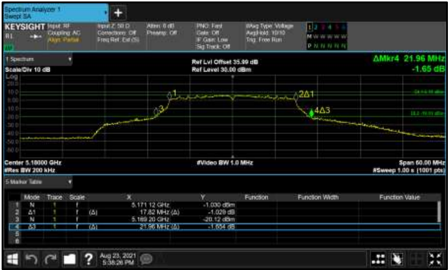
Figure 110 - Core 1 (B) 5180 MHz (CH36) 26 dB and 99% Bandwidth
