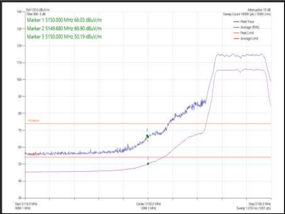
Figure 1 - 802.11a, Core 0 - 5180 MHz, Band Edge Frequency 5150 MHz
