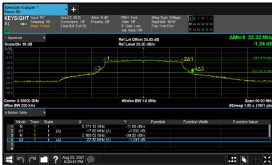
Figure 103 - Core 0 (A) 5180 MHz (CH36) 26 dB and 99% Bandwidth
