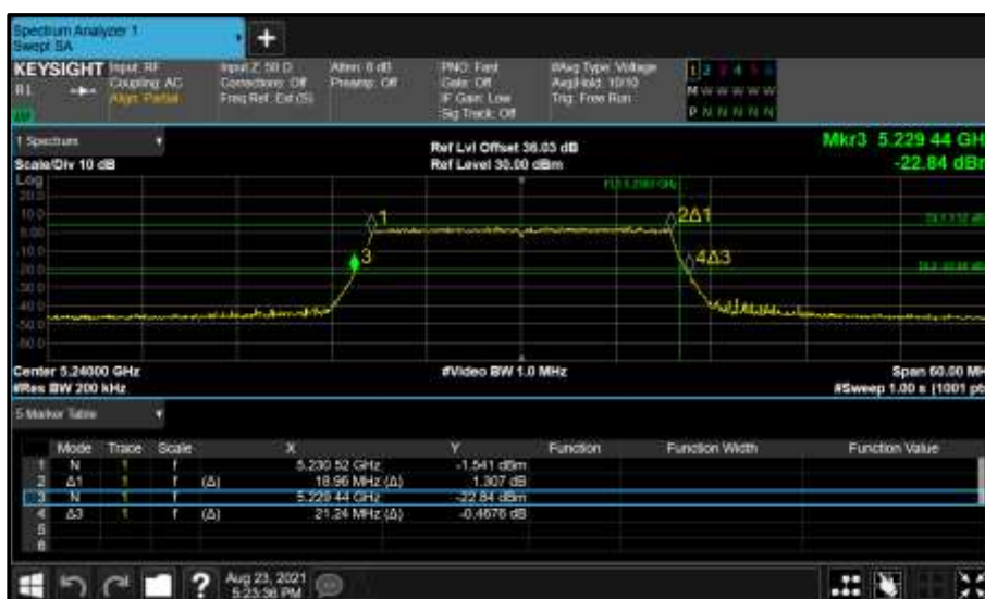
Figure 161 - Core 0 (A) 5240 MHz (CH48) 26 dB and 99% Bandwidth
