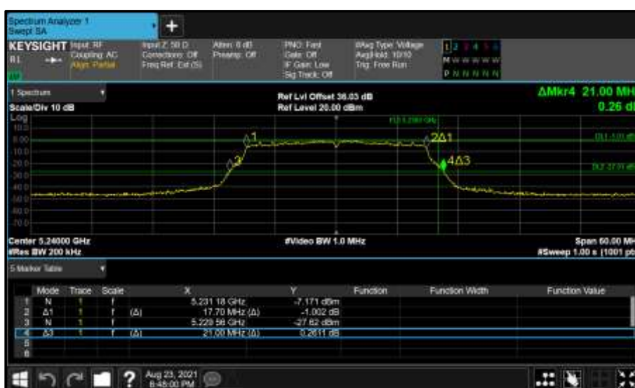
Figure 119 - Core 0 (A) 5240 MHz (CH48) 26 dB and 99% Bandwidth
