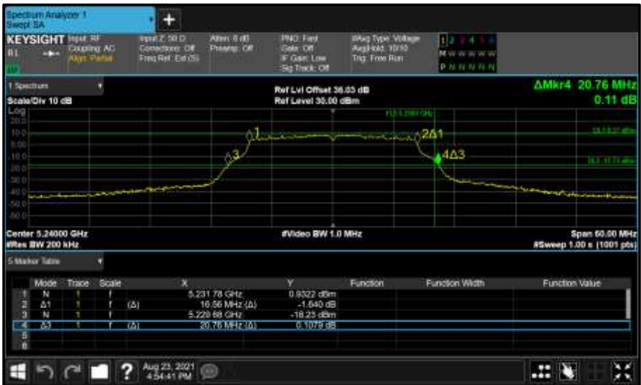
Figure 87 - Core 0 (A) 5240 MHz (CH48) 26 dB and 99% Bandwidth
