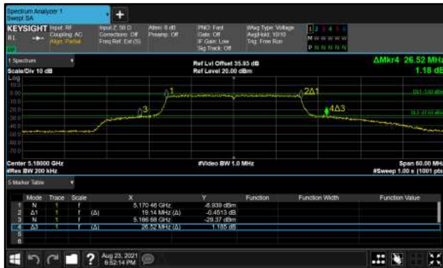
Figure 175 - Core 0 (A) 5180 MHz (CH36) 26 dB and 99% Bandwidth
