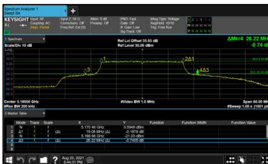
Figure 169 - Core 0 (A) 5180 MHz (CH36) 26 dB and 99% Bandwidth
