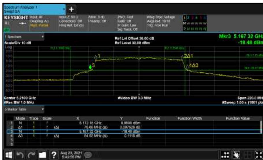
Figure 147 - Core 0 (A) 5210 MHz (CH42) 26 dB and 99% Bandwidth
