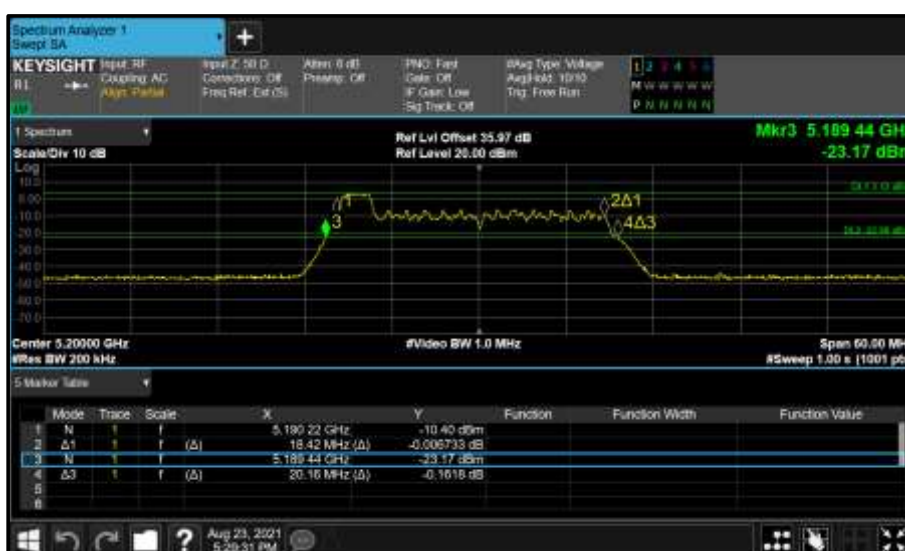
Figure 189 - Core 0 (A) 5200 MHz (CH40) 26 dB and 99% Bandwidth
