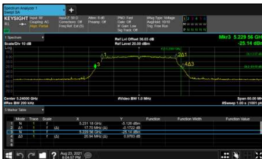
Figure 96 - Core 0 (A) 5240 MHz (CH48) 26 dB and 99% Bandwidth
