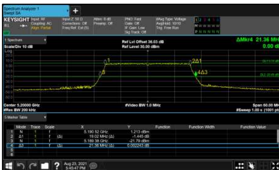
Figure 172 - Core 1 (B) 5200 MHz (CH40) 26 dB and 99% Bandwidth
