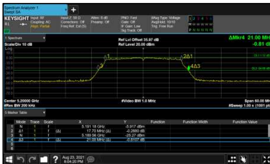
Figure 95 - Core 0 (A) 5200 MHz (CH40) 26 dB and 99% Bandwidth
