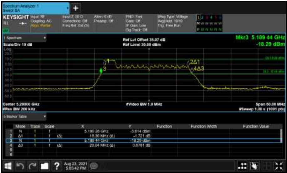
Figure 182 - Core 0 (A) 5200 MHz (CH40) 26 dB and 99% Bandwidth
