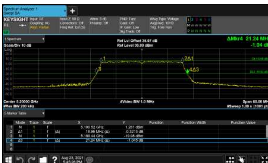
Figure 171 - Core 0 (A) 5200 MHz (CH40) 26 dB and 99% Bandwidth
