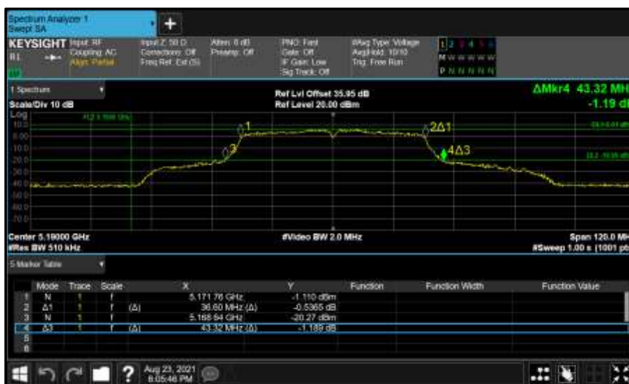
Figure 123 - Core 0 (A) 5190 MHz (CH38) 26 dB and 99% Bandwidth
