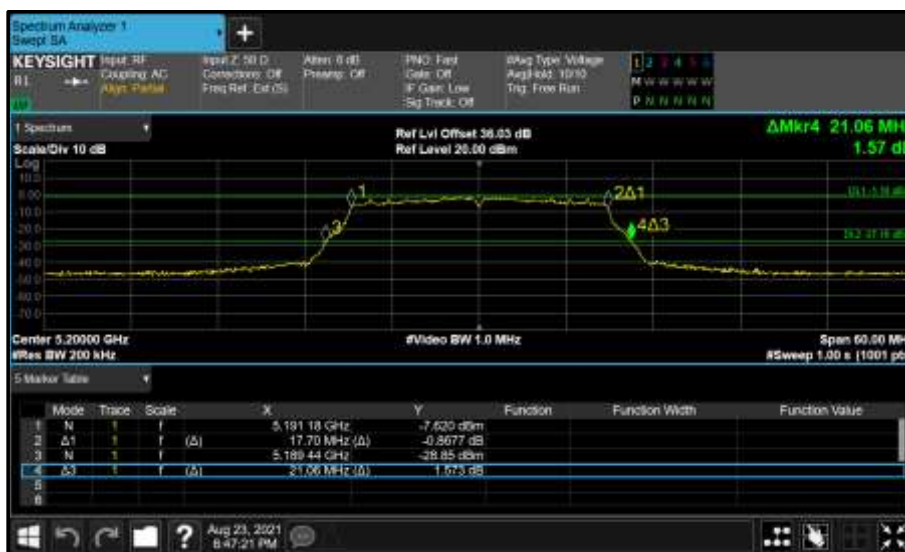
Figure 118 - Core 1 (B) 5200 MHz (CH40) 26 dB and 99% Bandwidth
