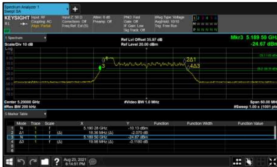
Figure 185 - Core 0 (A) 5200 MHz (CH40) 26 dB and 99% Bandwidth
