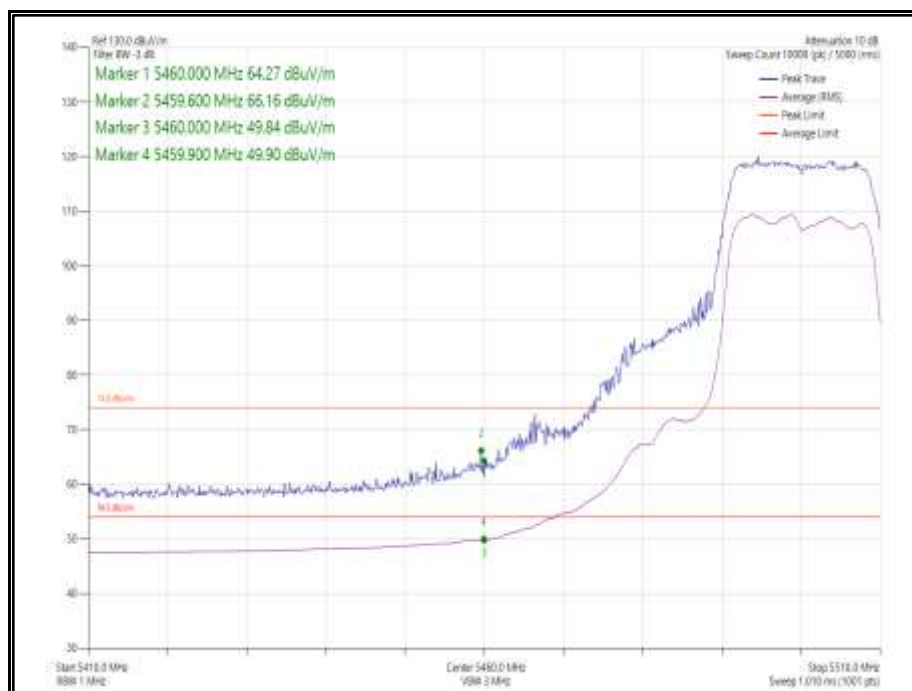
Figure 26 - 802.11n HT20 SDM, Cores 0-1 - 5500 MHz Band Edge Frequency 5460 MHz
