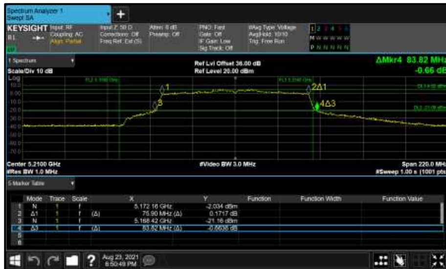
Figure 149 - Core 0 (A) 5210 MHz (CH42) 26 dB and 99% Bandwidth
