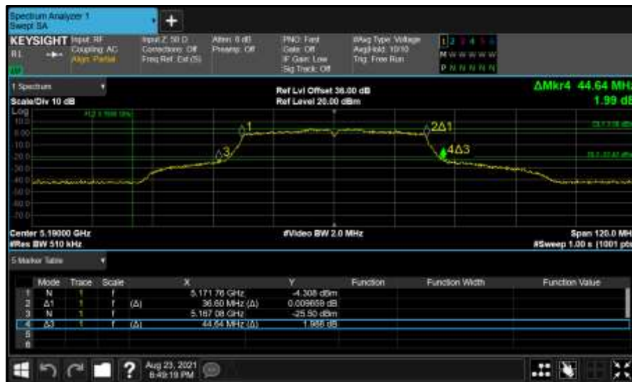
Figure 138 - Core 1 (B) 5190 MHz (CH38) 26 dB and 99% Bandwidth
