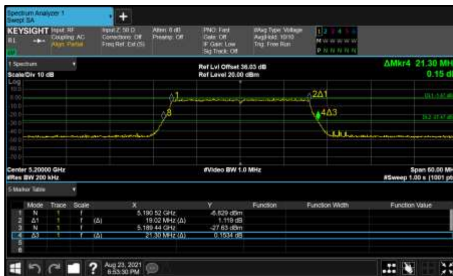
Figure 178 - Core 1 (B) 5200 MHz (CH40) 26 dB and 99% Bandwidth
