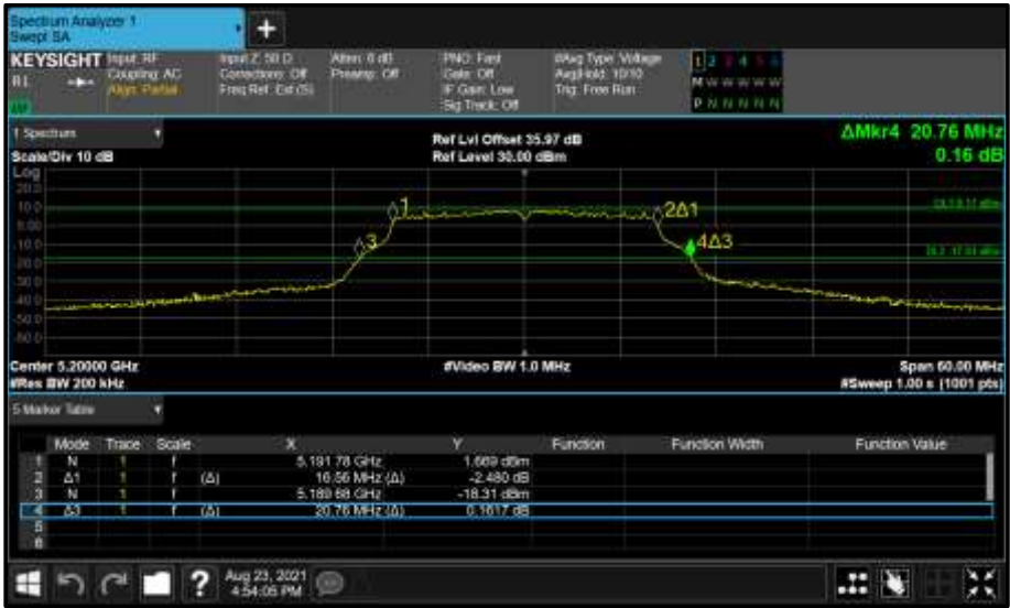
Figure 86 - Core 0 (A) 5200 MHz (CH40) 26 dB and 99% Bandwidth
