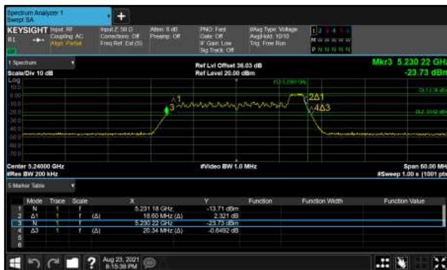
Figure 186 - Core 0 (A) 5240 MHz (CH48) 26 dB and 99% Bandwidth
