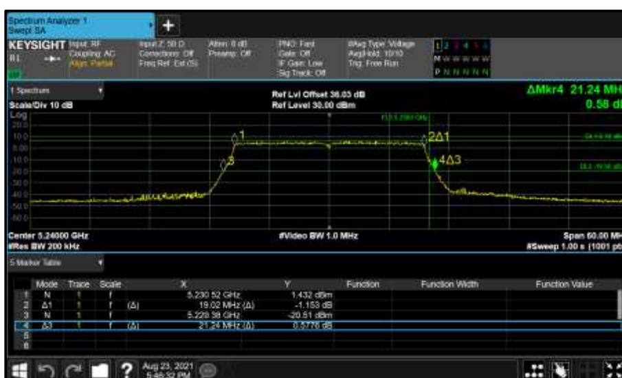
Figure 173 - Core 0 (A) 5240 MHz (CH48) 26 dB and 99% Bandwidth
