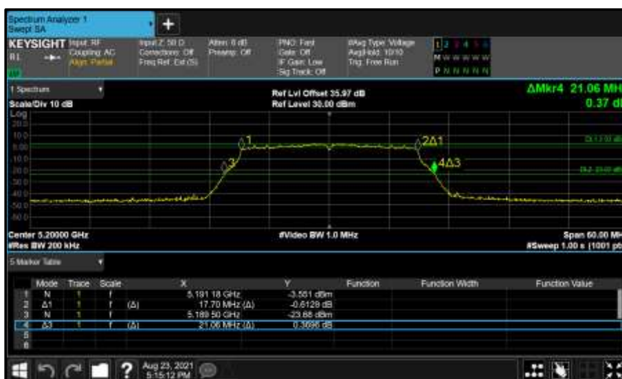
Figure 99 - Core 0 (A) 5200 MHz (CH40) 26 dB and 99% Bandwidth
