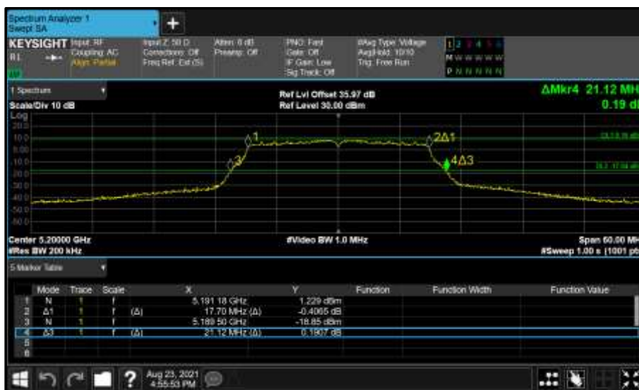
Figure 92 - Core 0 (A) 5200 MHz (CH40) 26 dB and 99% Bandwidth
