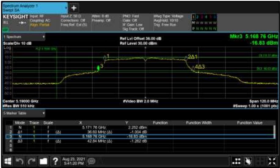
Figure 134 - Core 1 (B) 5190 MHz (CH38) 26 dB and 99% Bandwidth
