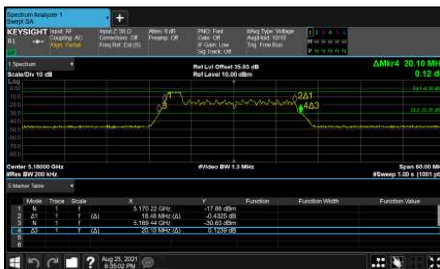
Figure 193 - Core 0 (A) 5180 MHz (CH36) 26 dB and 99% Bandwidth
