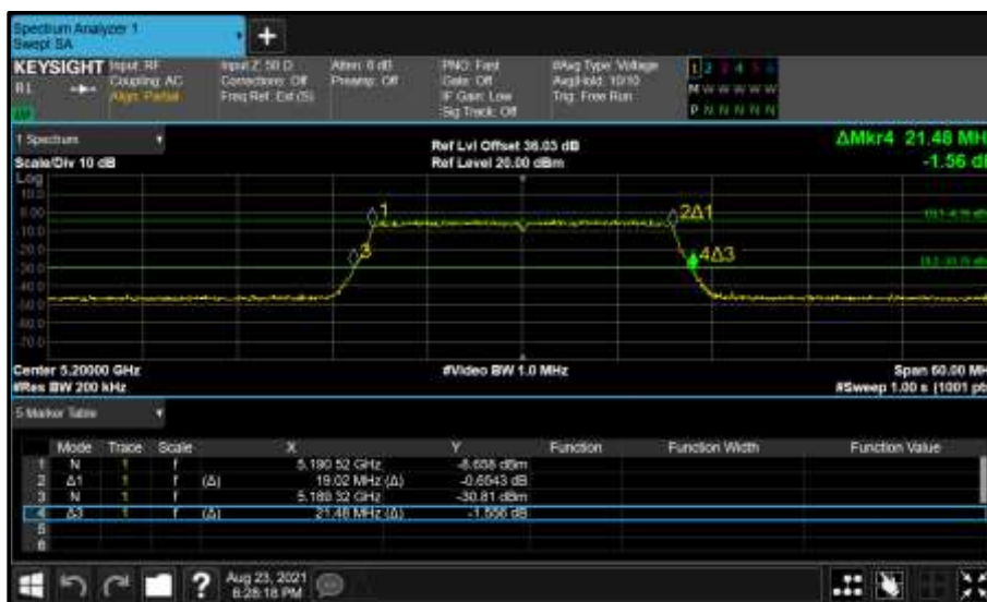
Figure 166 - Core 1 (B) 5200 MHz (CH40) 26 dB and 99% Bandwidth
