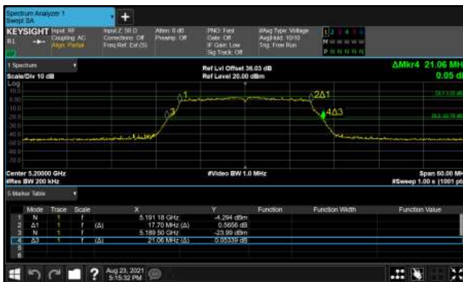
Figure 100 - Core 1 (B) 5200 MHz (CH40) 26 dB and 99% Bandwidth
