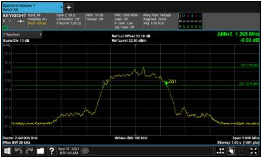
Figure 65 - Core 1 (B) 2441 MHz (CH39) 20 dB Bandwidth
