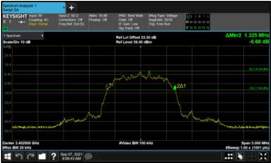
Figure 49 - Core 1 (B) 2402 MHz (CH0) 20 dB Bandwidth
