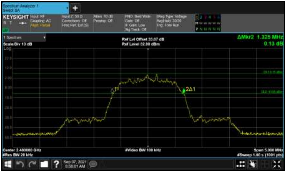
Figure 69 - Core 2 (C) 2480 MHz (CH78) 20 dB Bandwidth
