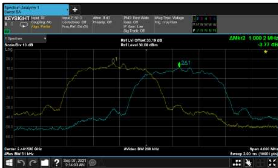
Figure 35 - \pi/4 DQPSK - 2441 MHz (CH39)
