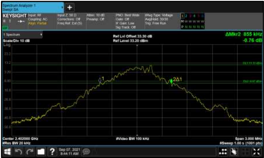
Figure 55 - Core 1 (B) 2402 MHz (CH0) 20 dB Bandwidth
