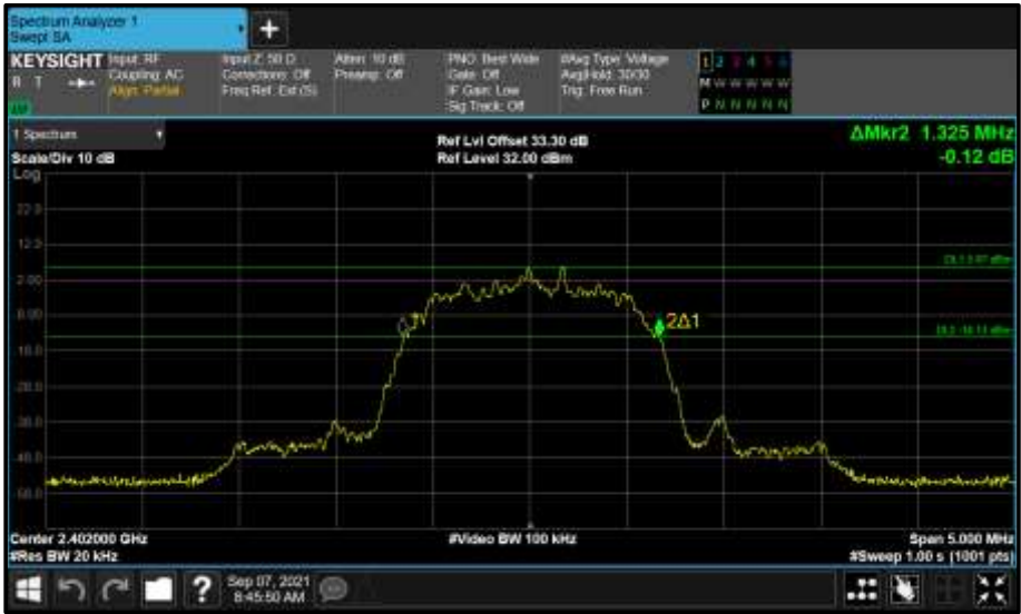
Figure 61 - Core 1 (B) 2402 MHz (CH0) 20 dB Bandwidth
