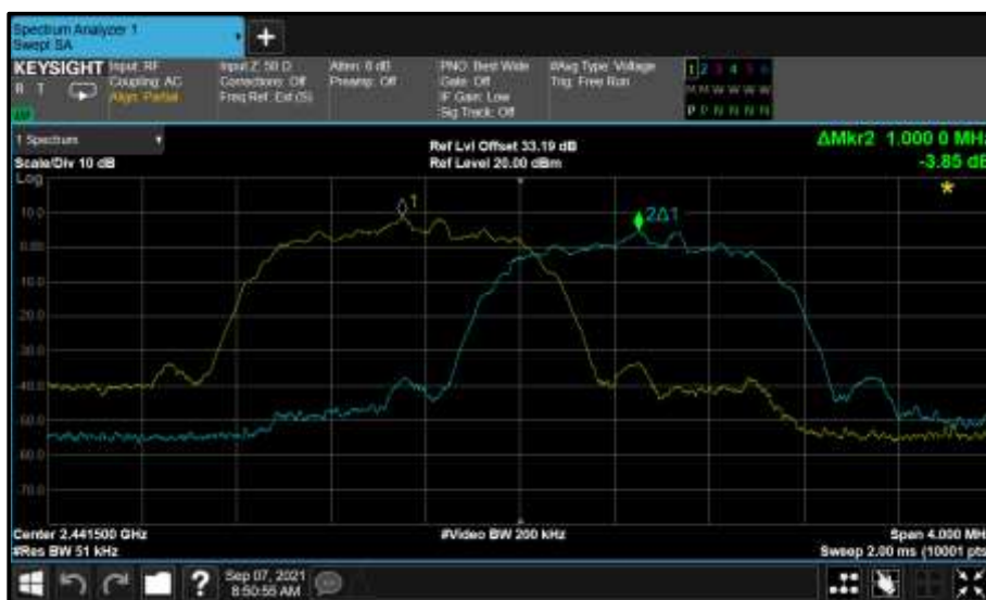
Figure 38 - \pi/4 DQPSK - 2441 MHz (CH39)
