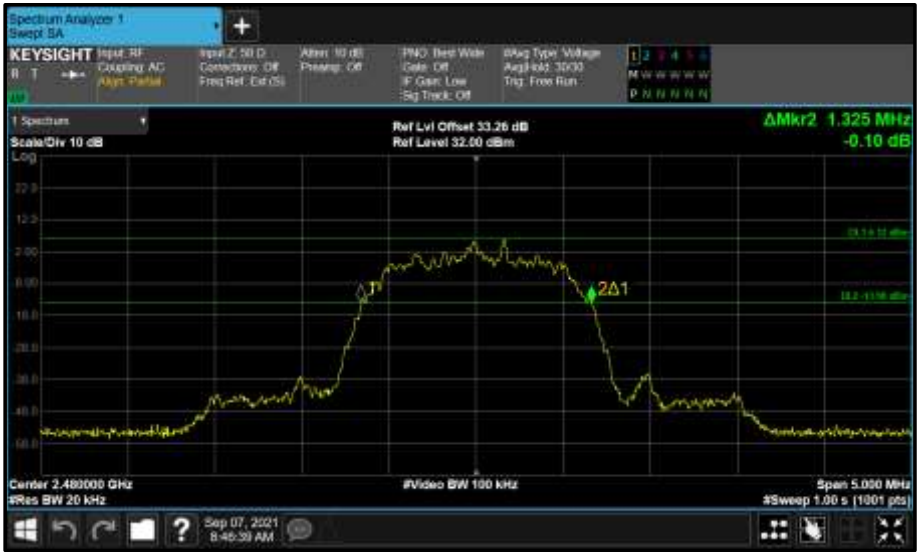
Figure 63 - Core 1 (B) 2480 MHz (CH78) 20 dB Bandwidth
