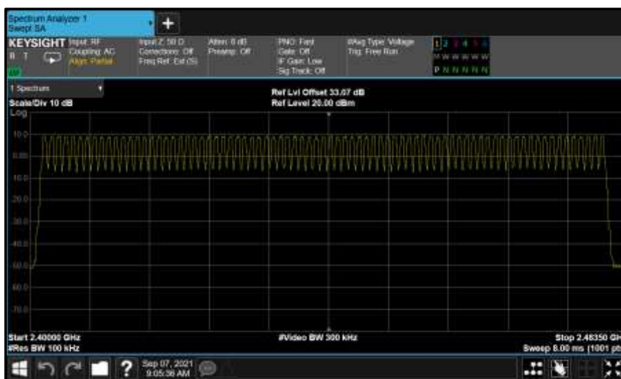
Figure 45 - GFSK (DH5) - Number of Hopping Channels
