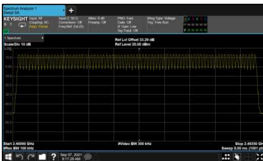
Figure 43 - GFSK (DH5) - Number of Hopping Channels
