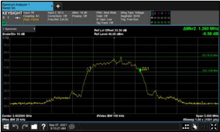
Figure 52 - Core 1 (B) 2402 MHz (CH0) 20 dB Bandwidth
