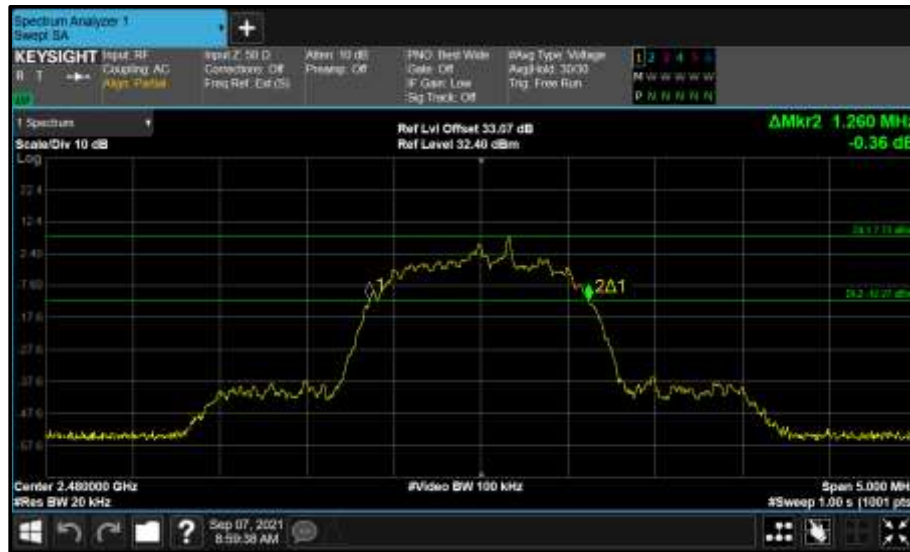
Figure 72 - Core 2 (C) 2480 MHz (CH78) 20 dB Bandwidth
