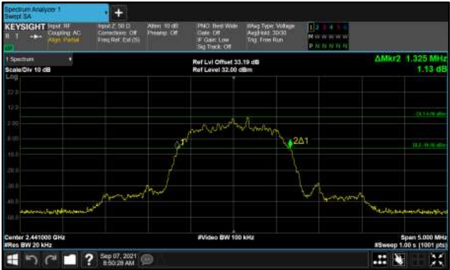
Figure 62 - Core 1 (B) 2441 MHz (CH39) 20 dB Bandwidth
