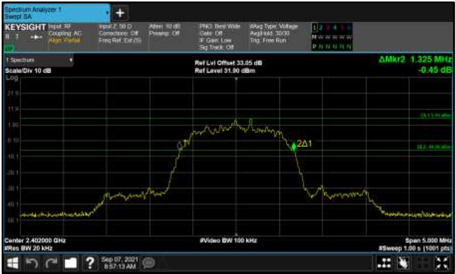
Figure 67 - Core 2 (C) 2402 MHz (CH0) 20 dB Bandwidth
