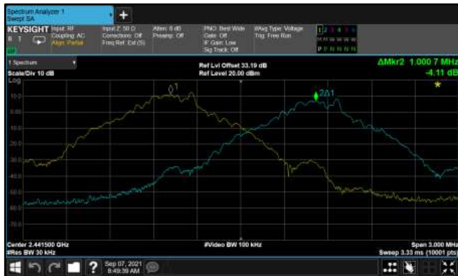
Figure 37 - GFSK - 2441 MHz (CH39)
