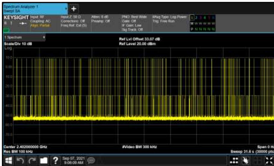
Figure 33 - GFSK - 2402 MHz Accumulated Transmit Time
