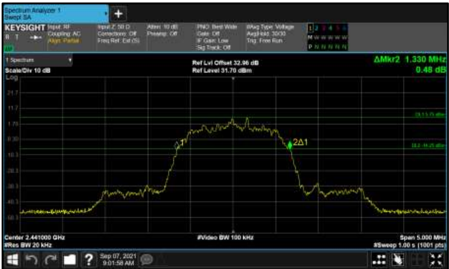
Figure 68 - Core 2 (C) 2441 MHz (CH39) 20 dB Bandwidth
