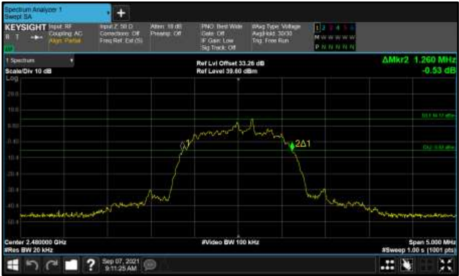
Figure 54 - Core 1 (B) 2480 MHz (CH78) 20 dB Bandwidth
