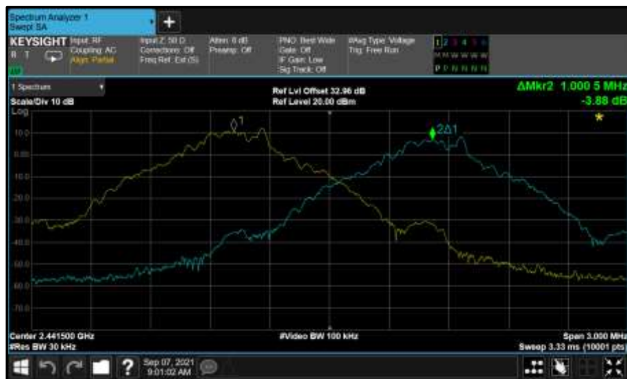
Figure 40 - GFSK - 2441 MHz (CH39)
