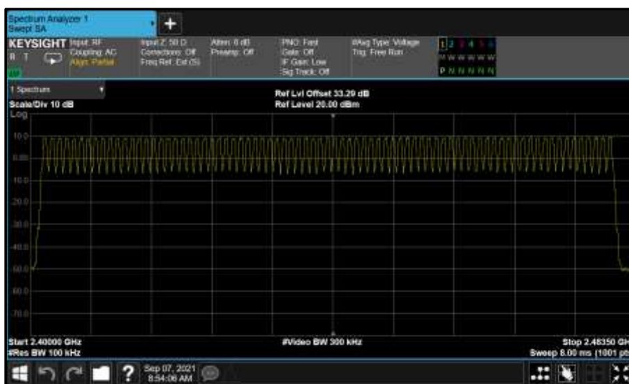
Figure 44 - GFSK (DH5) - Number of Hopping Channels
