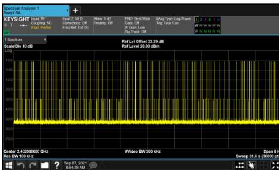
Figure 32 - GFSK - 2402 MHz Accumulated Transmit Time
