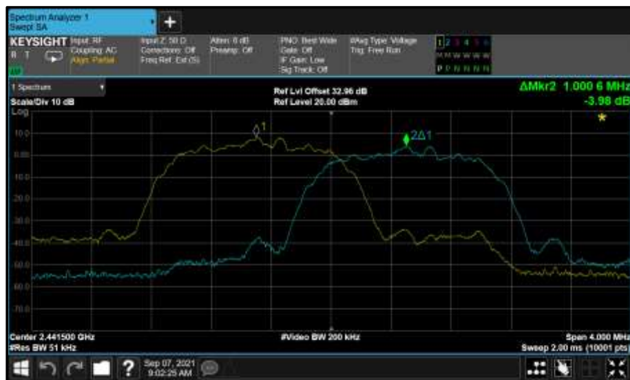
Figure 41 - \pi/4 DQPSK - 2441 MHz (CH39)
