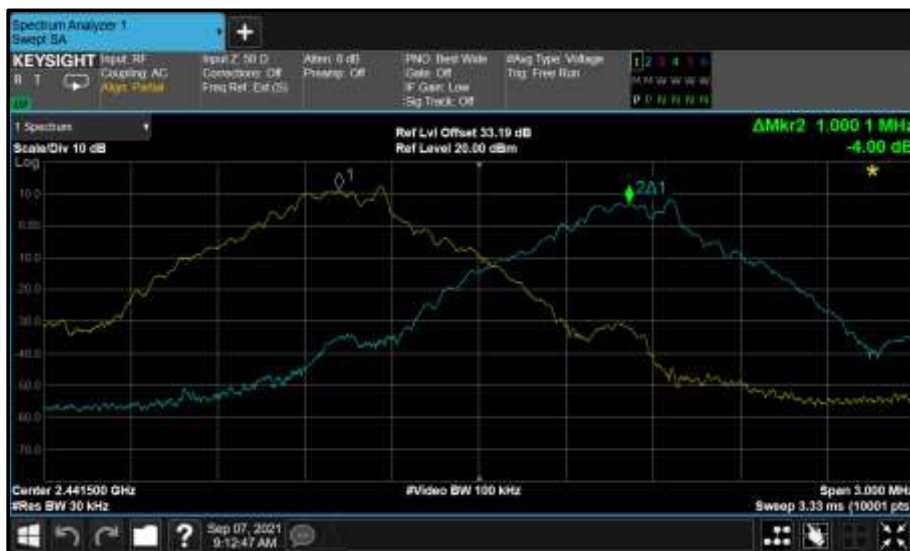
Figure 34 - GFSK - 2441 MHz (CH39)
