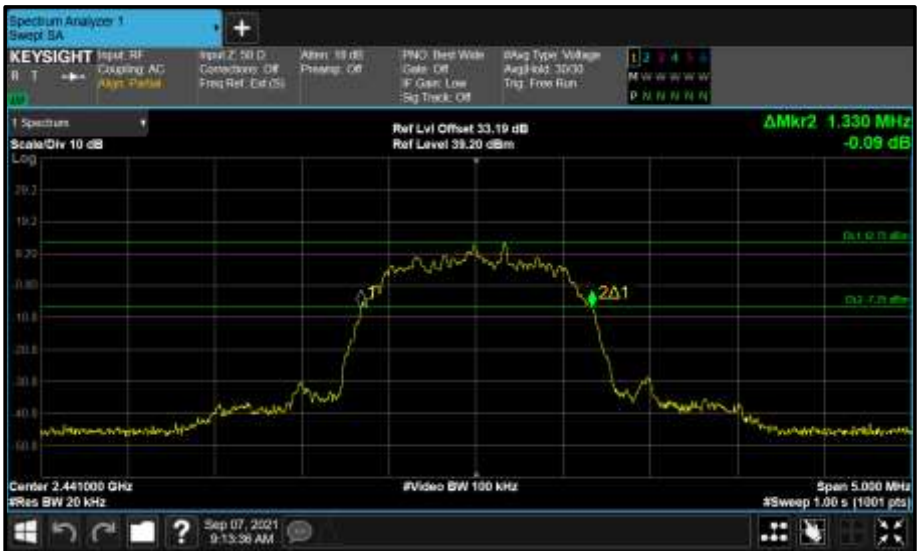
Figure 50 - Core 1 (B) 2441 MHz (CH39) 20 dB Bandwidth
