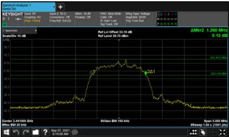
Figure 53 - Core 1 (B) 2441 MHz (CH39) 20 dB Bandwidth
