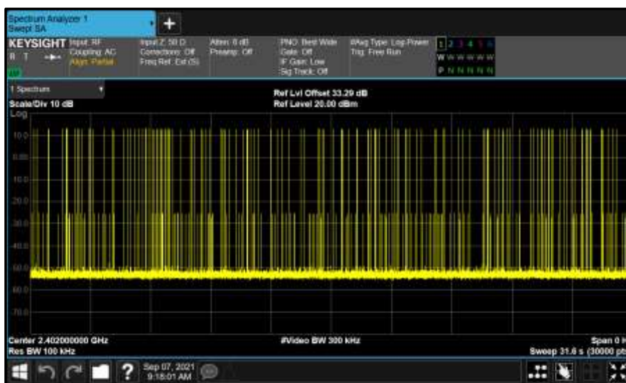
Figure 31 - GFSK - 2402 MHz Accumulated Transmit Time
