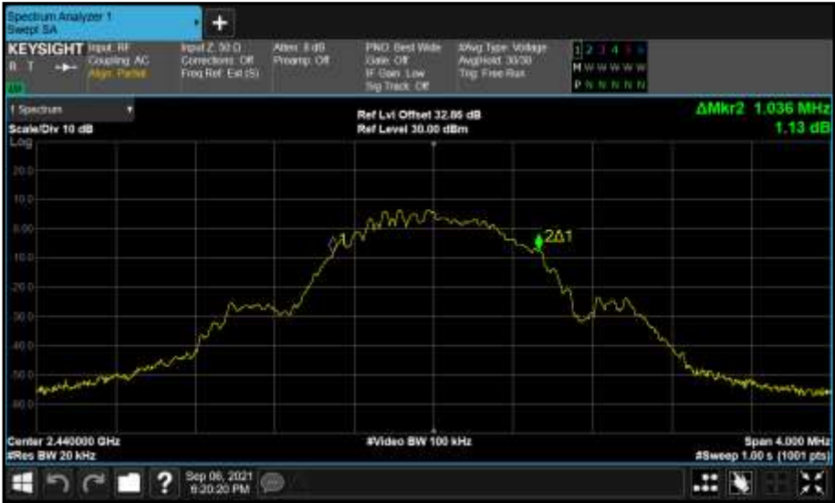
Figure 189 - Core 0 (A) 2440 MHz (CH17) 99% Bandwidth
