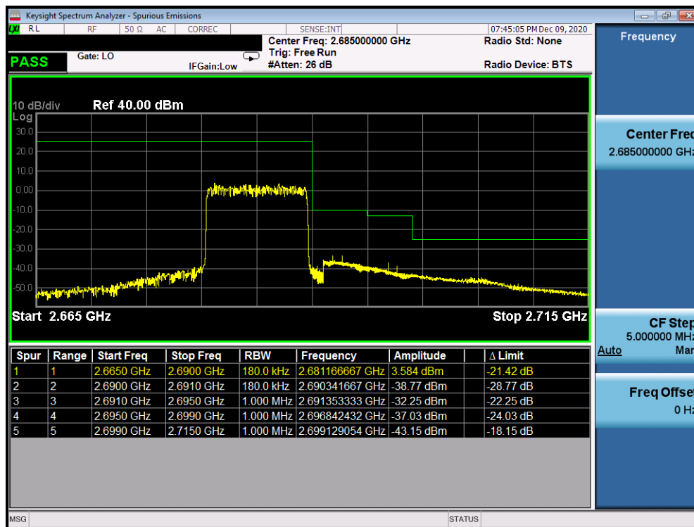
Plot 7-191. Upper ACP Plot (LTE Band 41 - 10MHz QPSK – Full RB Configuration)
