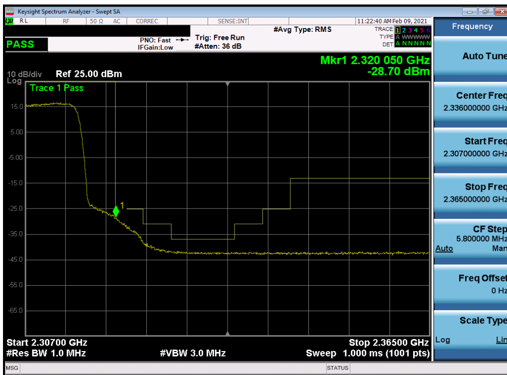
Plot 7-173. Upper Extended Band Edge Plot (Band 30 - 10.0MHz QPSK - Full RB Configuration)
