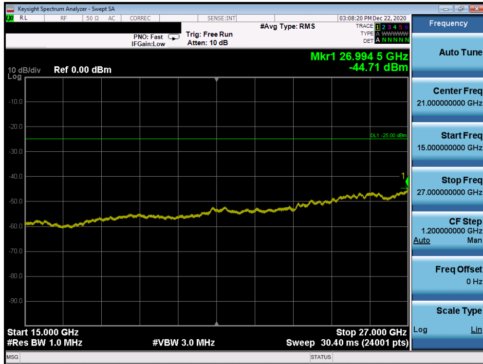
Plot 7-166. CSE (ULCA LTE Band 7 - (20 + 20)MHz QPSK - PCC 1/99 SCC 1/0, - Mid Channel)
