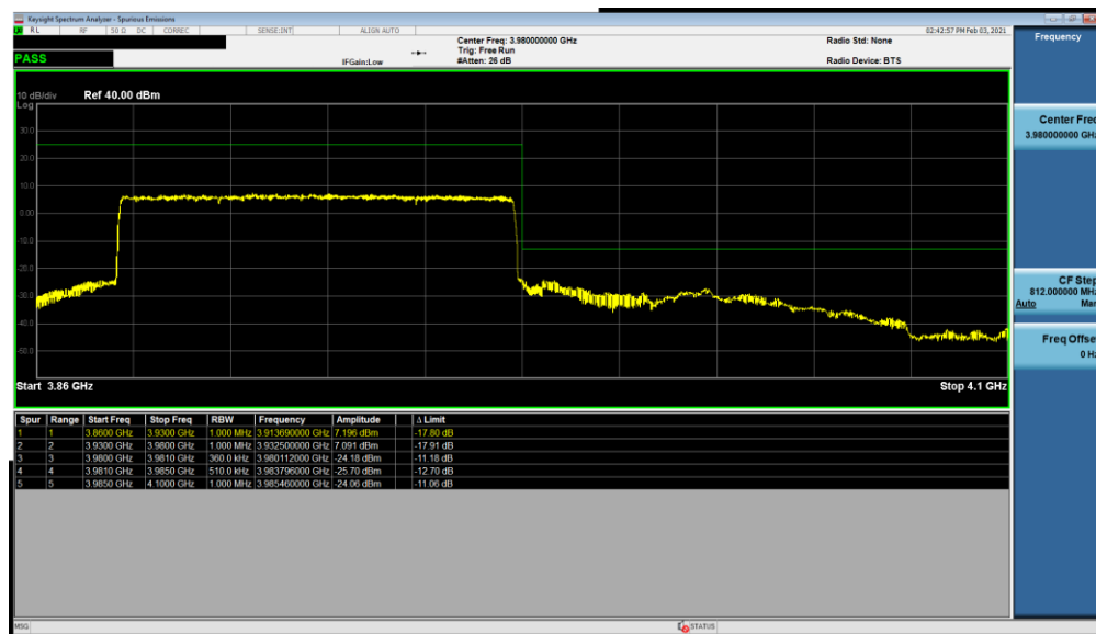
Plot 7-209. Upper ACP Plot (NR Band n77 - 100MHz DFT-s-OFDM \Pi/2 BPSK – Full RB Configuration)
