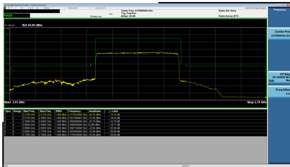
Plot 7-197. Upper ACP Plot (NR Band n41 - 90MHz DFT-s-OFDM \Pi/2 BPSK – Full RB Configuration)
