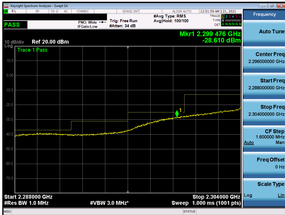
Plot 7-171. Lower Extended Band Edge Plot (Band 30 - 10.0MHz QPSK - Full RB Configuration)
