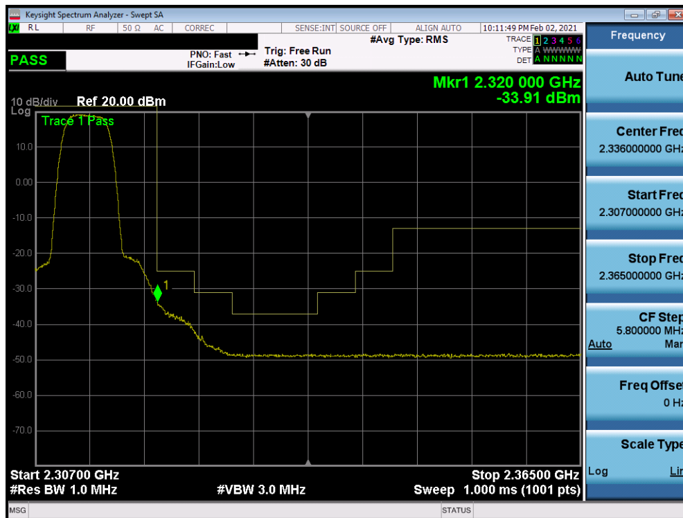
Plot 7-177. Upper Extended Band Edge Plot (Band 30 - 5.0MHz QPSK - Full RB Configuration)
