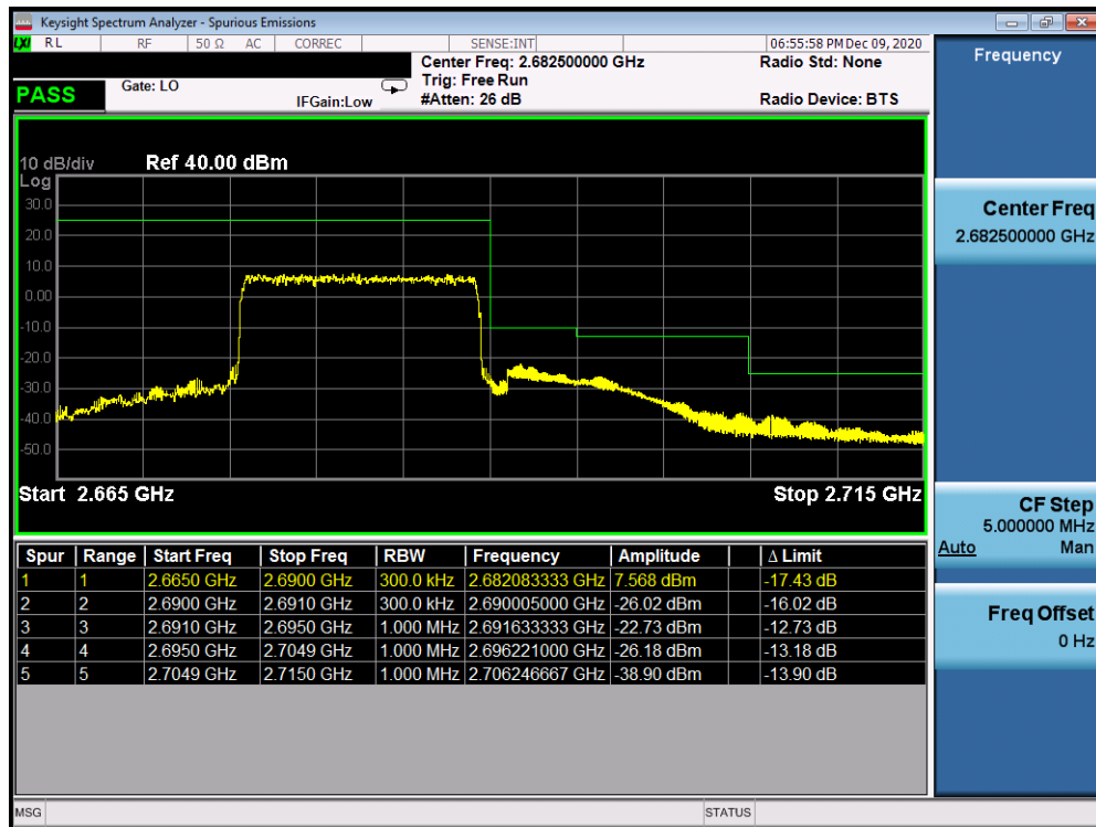
Plot 7-189. Upper ACP Plot (LTE Band 41 - 15MHz QPSK – Full RB Configuration)
