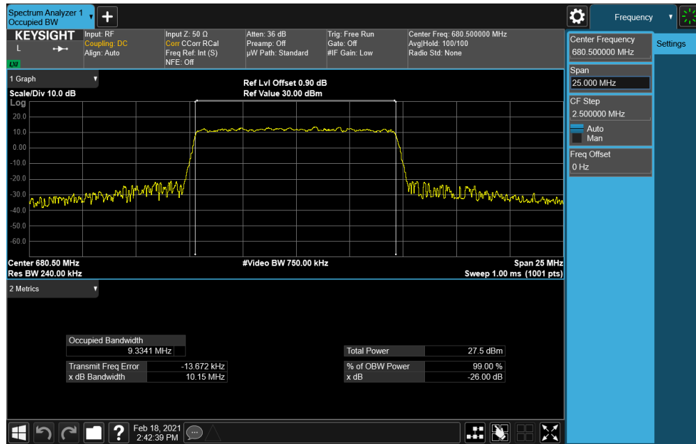
Plot 7-114. Occupied Bandwidth Plot (NR Band n71 - 10.0MHz CP-OFDM 256QAM - Full RB)
