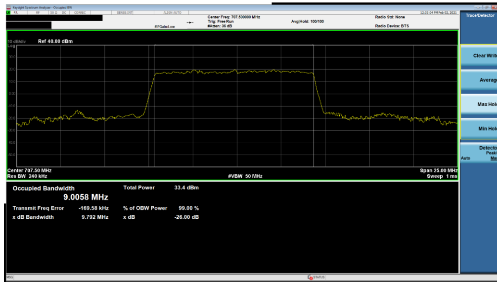
Plot 7-90. Occupied Bandwidth Plot (NR Band n12 - 10.0MHz DFT-s-OFDM \pi/2 BPSK - Full RB)
