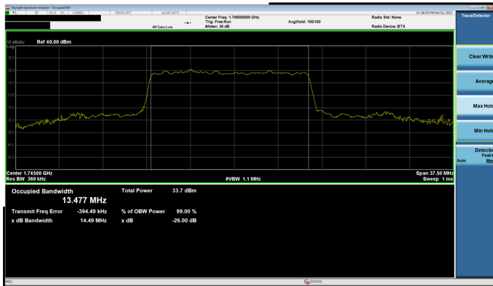
Plot 7-70. Occupied Bandwidth Plot (NR Band n66 - 15.0MHz DFT-s-OFDM \pi/2 BPSK - Full RB)
