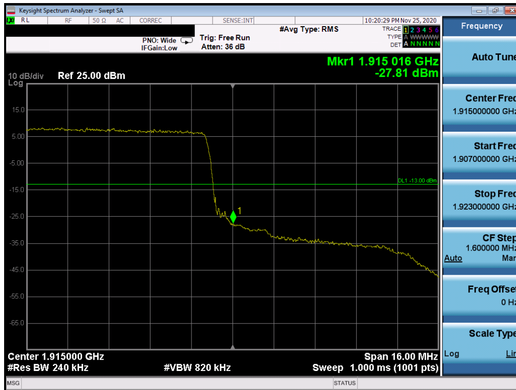
Plot 7-86. Upper Band Edge Plot (LTE Band 25 - 20MHz QPSK – Full RB Configuration)
