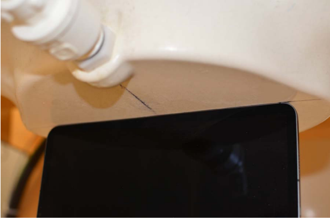
Test Setup Photo 8 – Right Edge SAR at 0 mm
