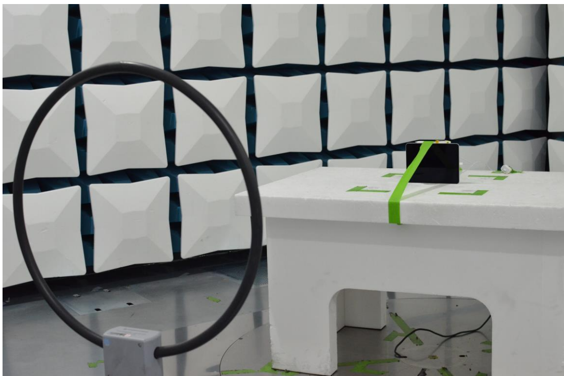
Figure 24: 9kHz-30MHz Test Setup (Front View)
