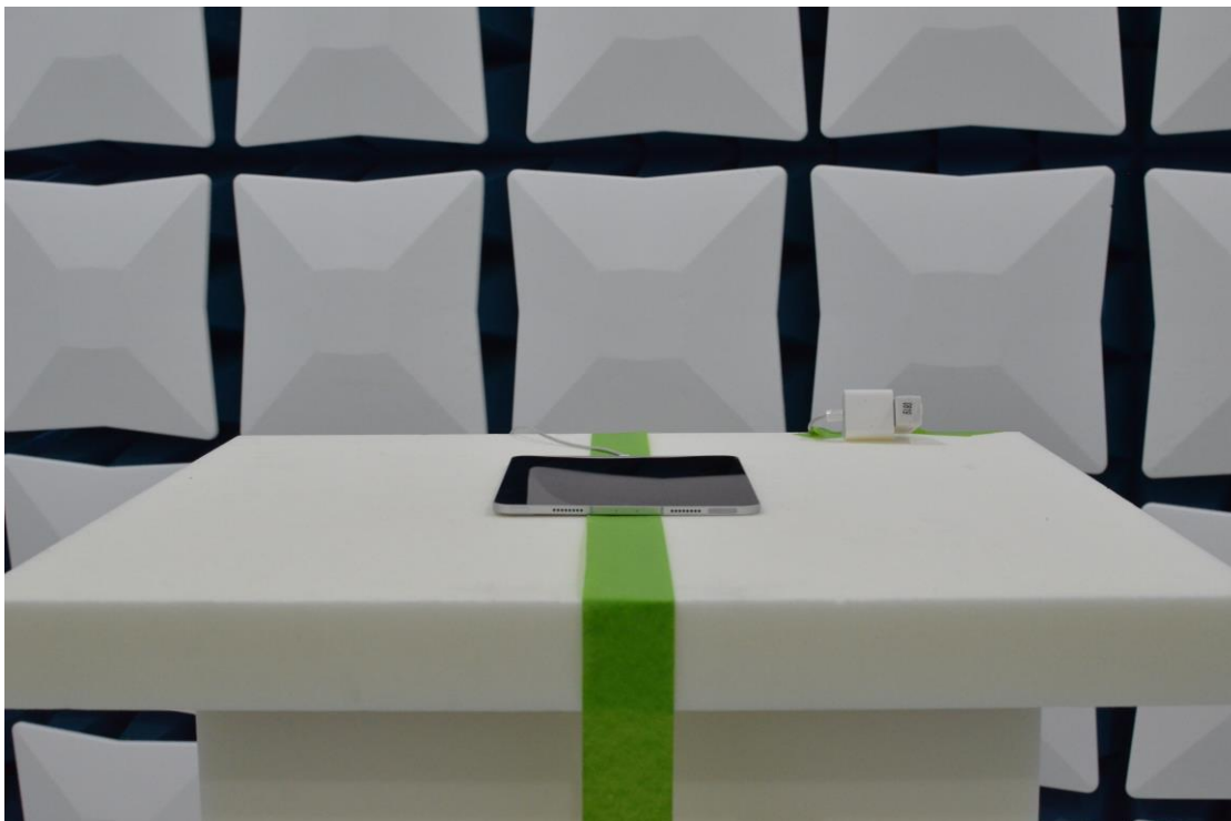
Figure 5: 1-18GHz Test Setup (Front View)
