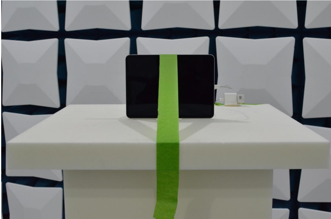
Figure 7: 1-18GHz Test Setup (Front View)
