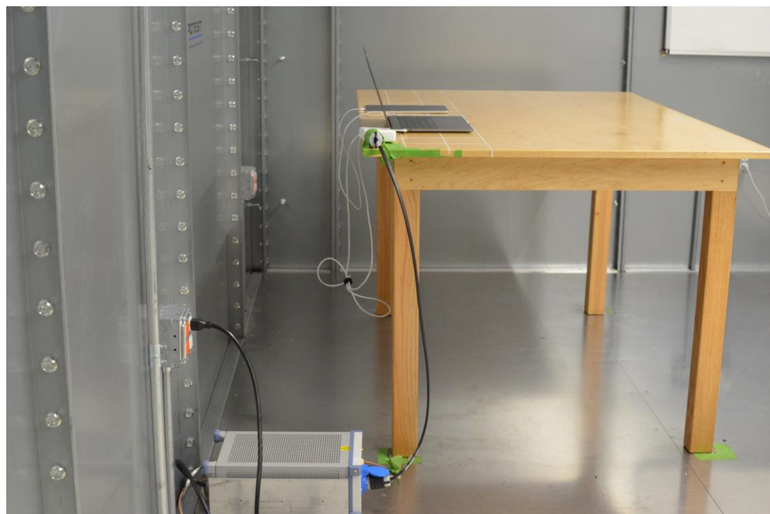
Figure 4: AC Line Conducted Emissions (Side View)
