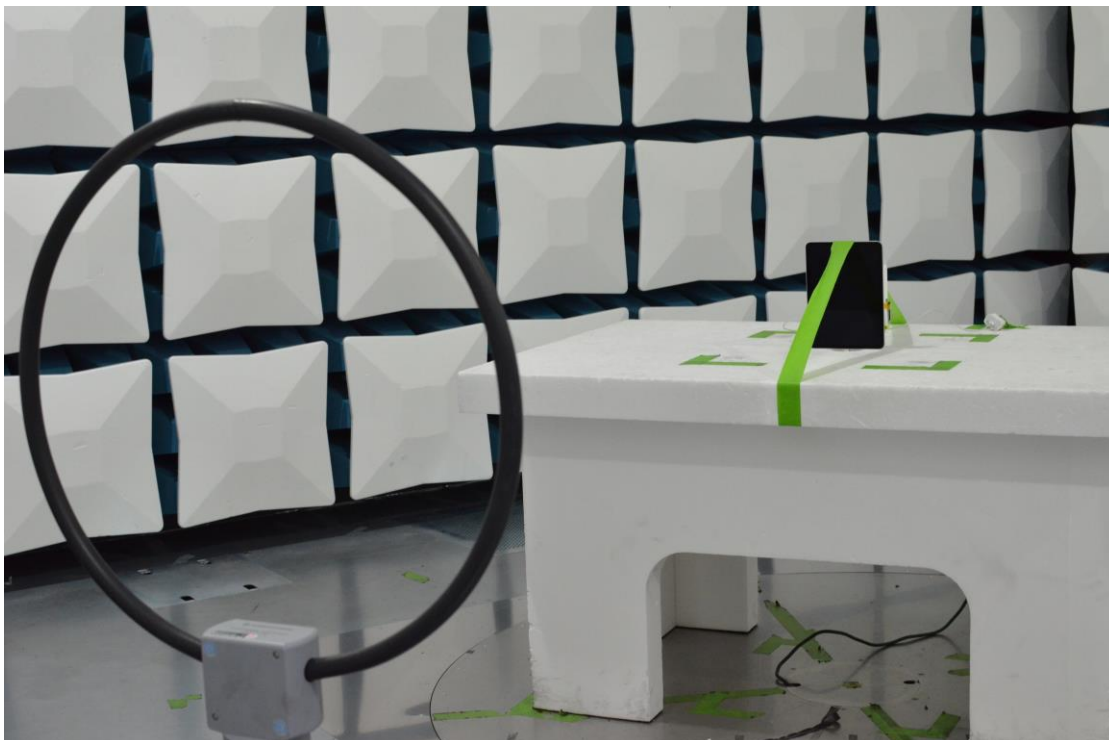
Figure 25: 9kHz-30MHz Test Setup (Front View)
