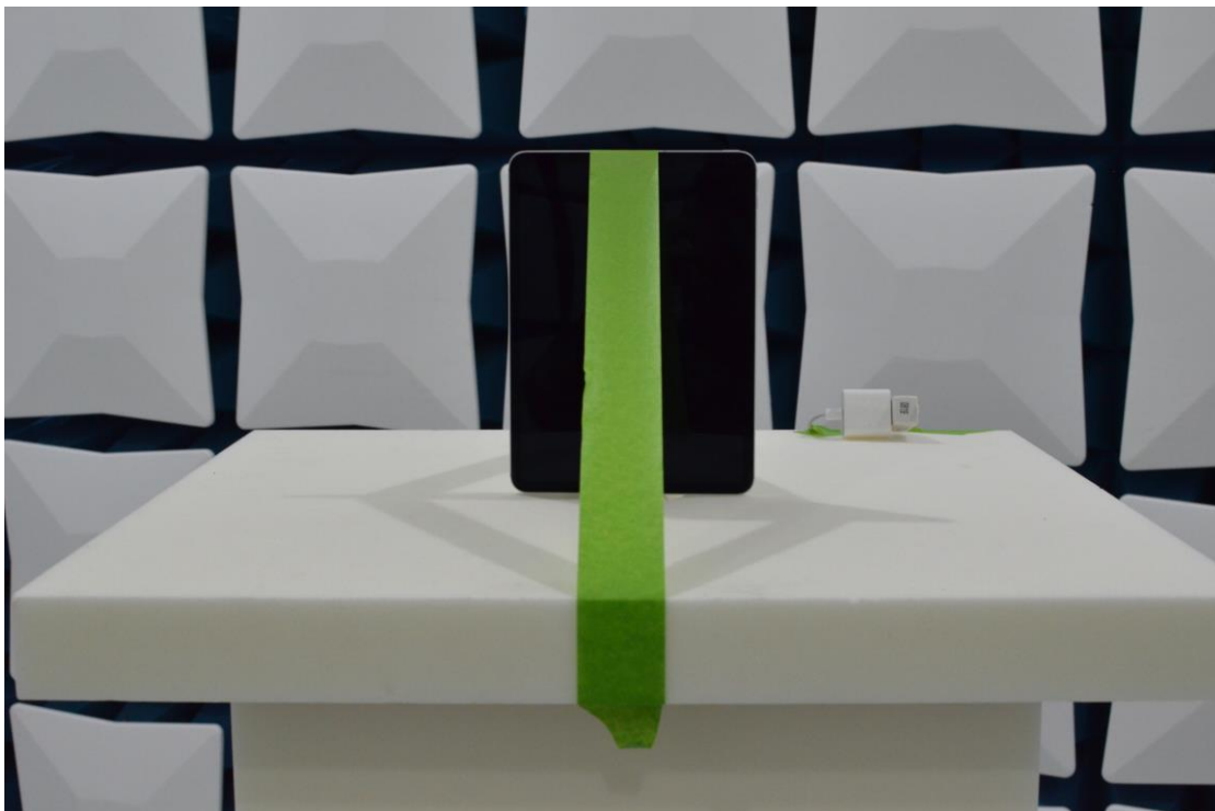
Figure 9: 1-18GHz Test Setup (Front View)
