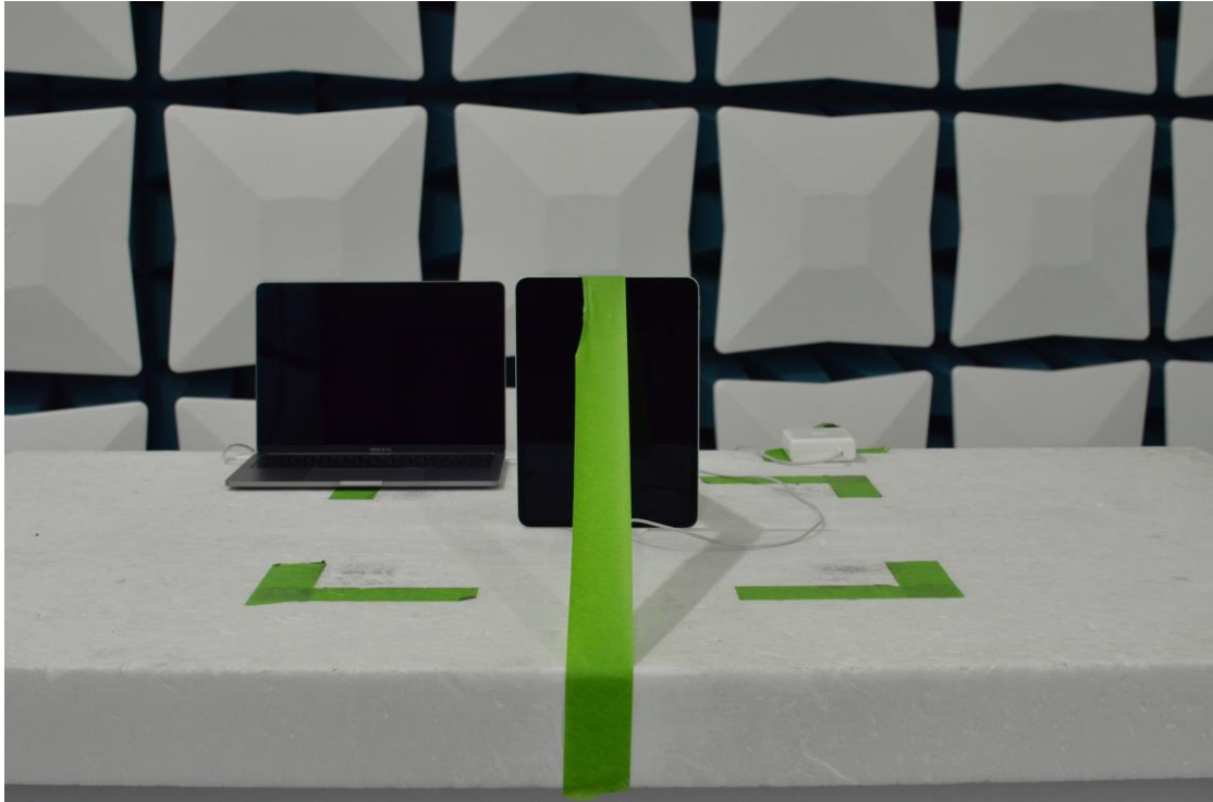
Figure 21: 30MHz-1GHz Test Setup (Front View)
