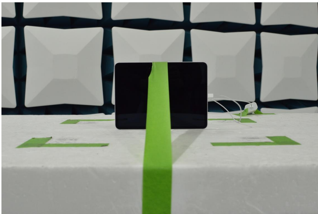
Figure 13: 30MHz-1GHz Test Setup (Front View)
