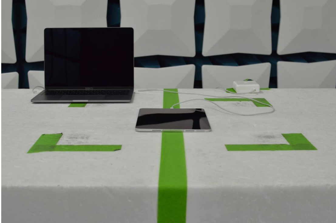
Figure 17: 30MHz-1GHz Test Setup (Front View)
