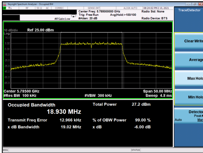
Plot 7-116. 6dB BW & 99% OBW Antenna 5b (20MHz BW 802.11ax(SU) – Ch. 157, MCS3)
