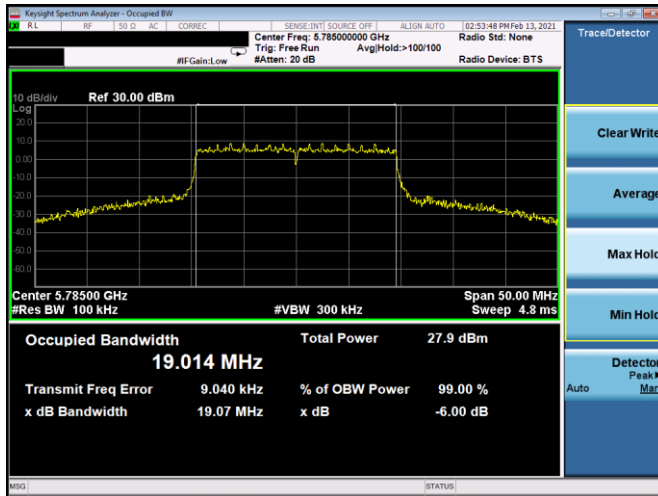
Plot 7-140. 6dB BW & 99% OBW Antenna 4b (20MHz BW 802.11ax(SU) – Ch. 157, MCS11)
