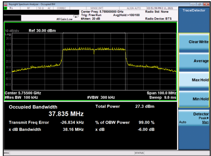
Plot 7-136. 6dB BW & 99% OBW Antenna 4b (40MHz BW 802.11ax (SU) – Ch. 151, MCS3)
