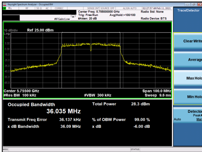
Plot 7-117. 6dB BW & 99% OBW Antenna 5b (40MHz BW 802.11n – Ch. 151, MCS3)
