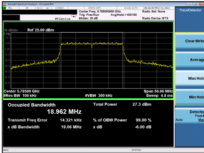
Plot 7-122. 6dB BW & 99% OBW Antenna 5b (20MHz BW 802.11ax(SU) – Ch. 157, MCS11)
