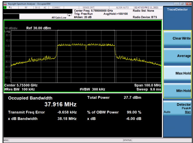
Plot 7-142. 6dB BW & 99% OBW Antenna 4b (40MHz BW 802.11ax(SU) – Ch. 151, MCS11)
