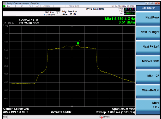
Plot 7-161. PSD Antenna 5b (80MHz BW 802.11ac – Ch. 106, MCS0)
