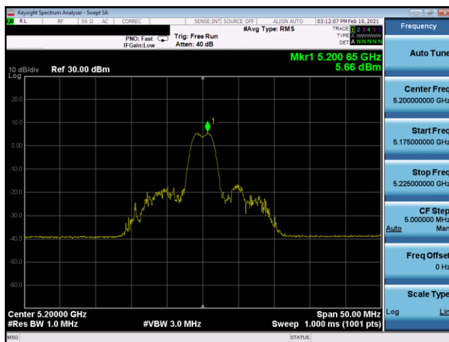
Plot 7-219. PSD SDM Antenna 5b (20MHz BW 11ax Index 4 – RU26 – Ch.40)
