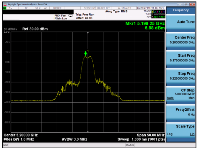
Plot 7-220. PSD SDM Antenna 4b (20MHz BW 11ax Index 4 – RU26 – Ch.40)
