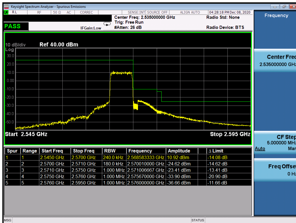
Plot 7-185. Upper ACP Plot (LTE Band 7 - 5MHz QPSK – Full RB Configuration)
