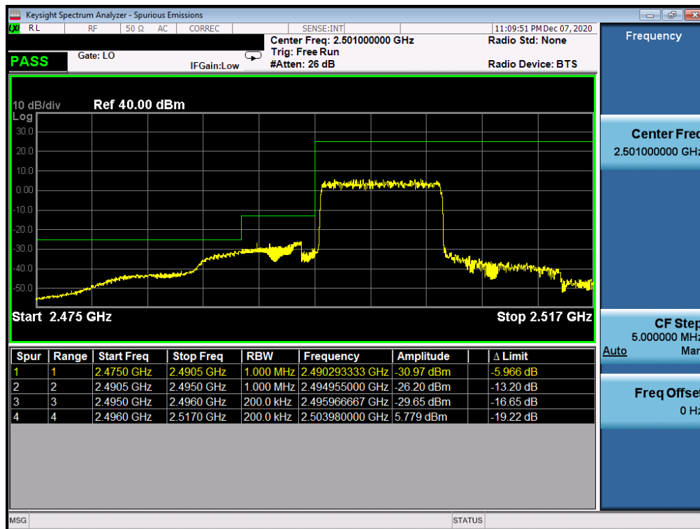
Plot 7-190. Lower ACP Plot (LTE Band 41 - 10MHz QPSK – Full RB Configuration)
