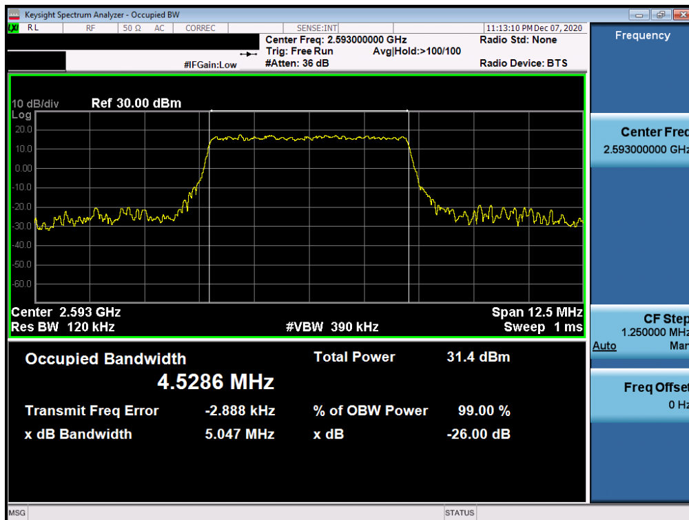
Plot 7-39. Occupied Bandwidth Plot (LTE Band 41 - 5MHz 64-QAM - Full RB Configuration)
