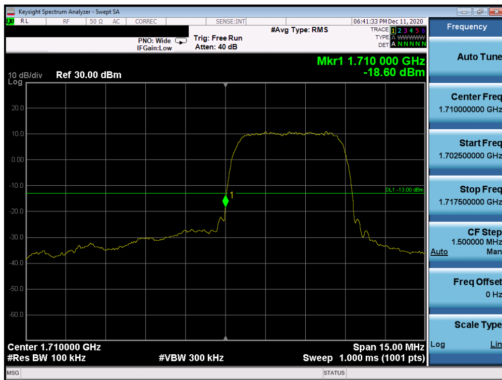
Plot 7-293. Band Edge Plot (AWS WCDMA Mode - Low Channel)
