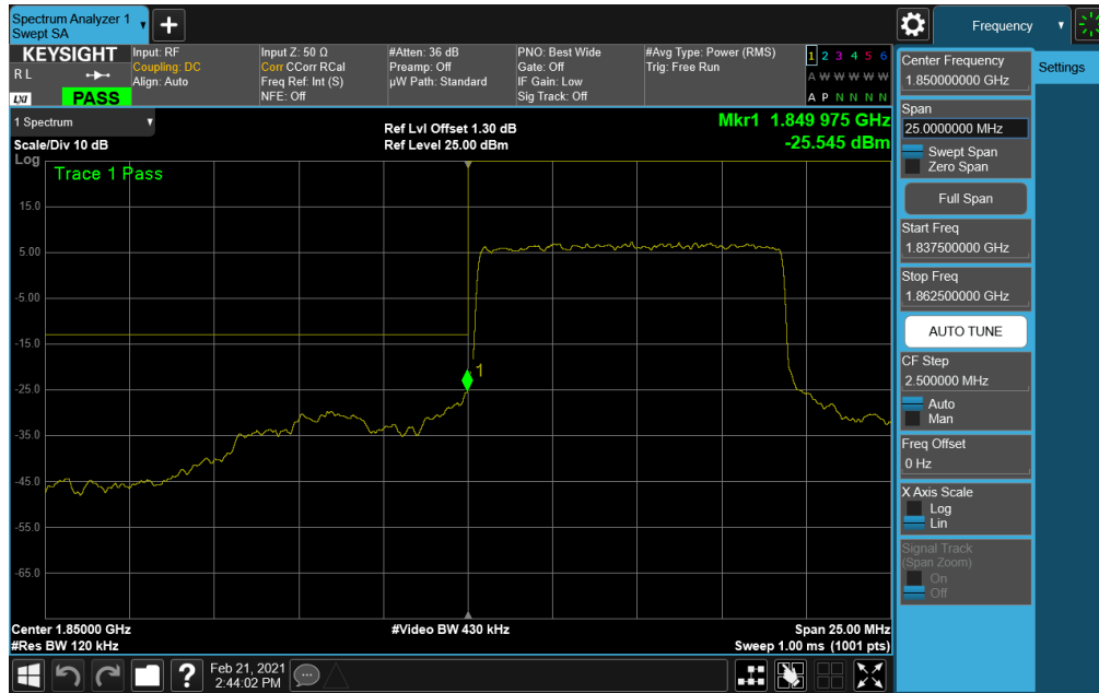
Plot 7-156. Lower Band Edge Plot (NR Band n2 – 10.0MHz DFT-s-OFDM \pi/2 BPSK - Full RB)
