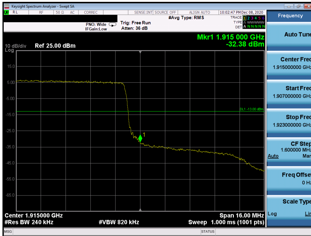
Plot 7-86. Upper Band Edge Plot (LTE Band 25 - 20MHz QPSK – Full RB Configuration)
