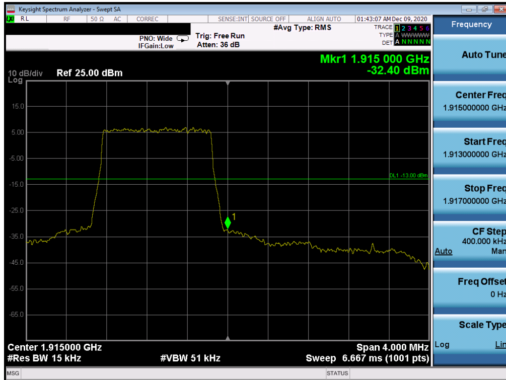
Plot 7-106. Upper Band Edge Plot (LTE Band 25 – 1.4MHz QPSK – Full RB Configuration)
