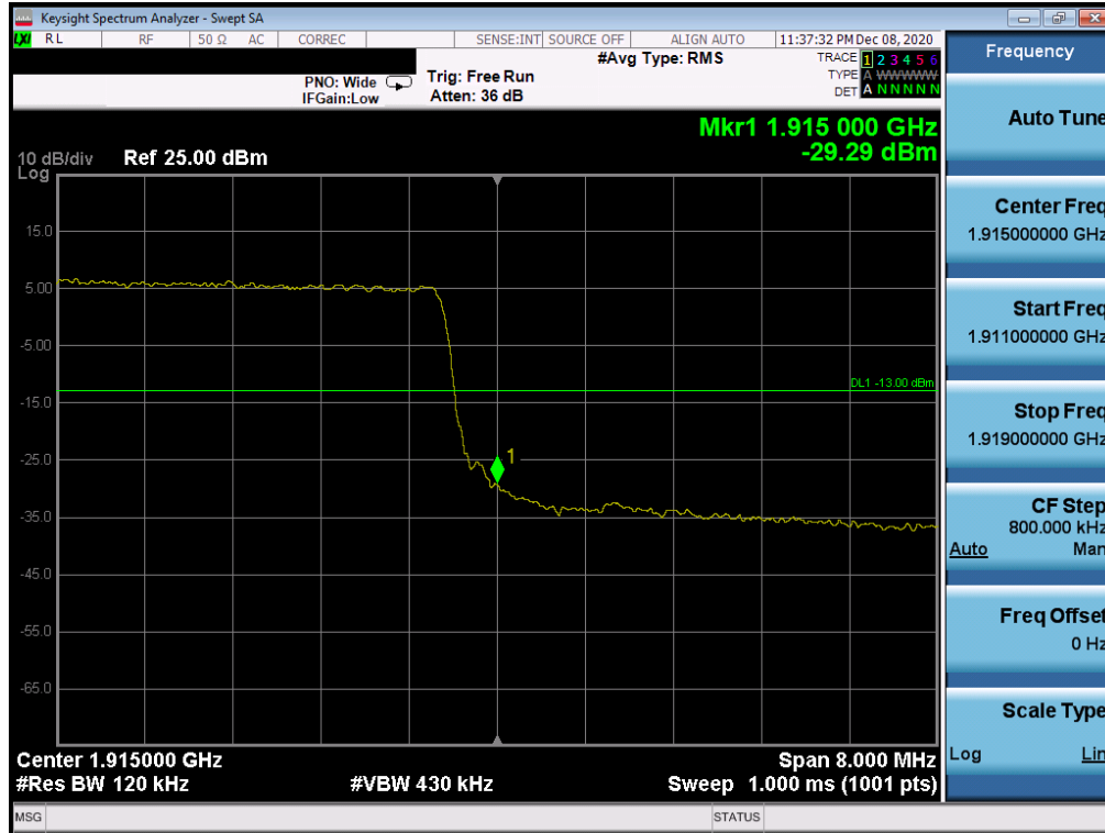
Plot 7-94. Upper Band Edge Plot (LTE Band 25 - 10MHz QPSK – Full RB Configuration)
