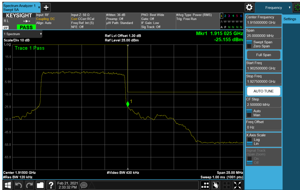
Plot 7-142. Upper Band Edge Plot (NR Band n25 – 10.0MHz DFT-s-OFDM \pi/2 BPSK - Full RB)
