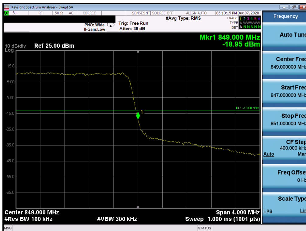
Plot 7-99. Upper Band Edge Plot (LTE Band 26 - 3MHz QPSK - Full RB Configuration)
