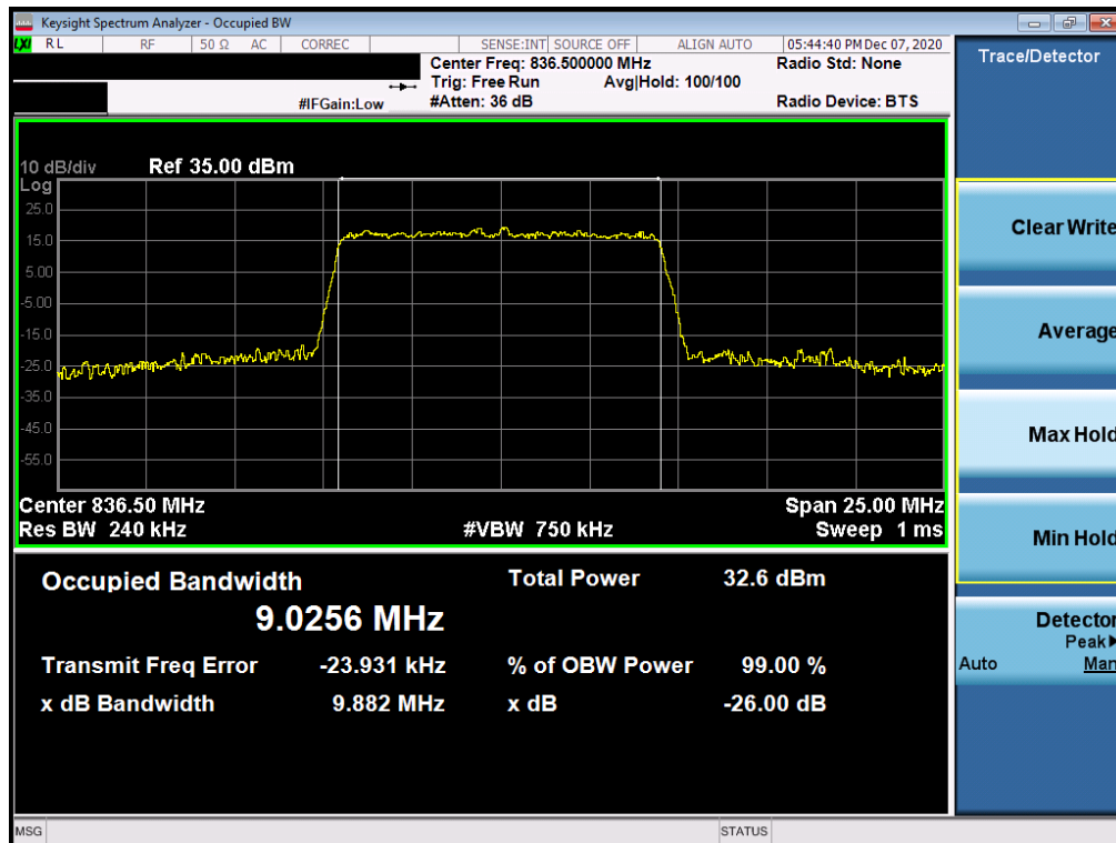
Plot 7-2. Occupied Bandwidth Plot (LTE Band 26/5 - 10MHz 16-QAM - Full RB Configuration)
