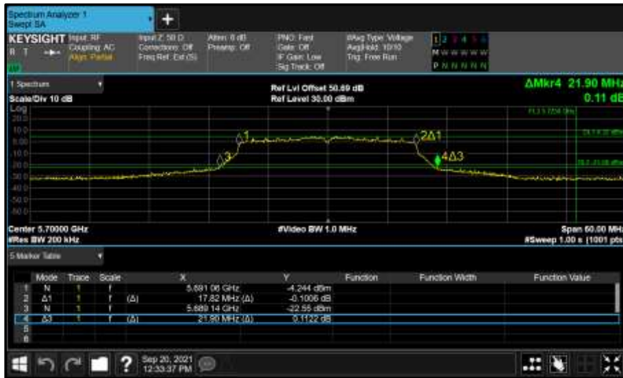
Figure 584 - Core 1 (B) 5700 MHz (CH140) 26 dB and 99% Bandwidth
