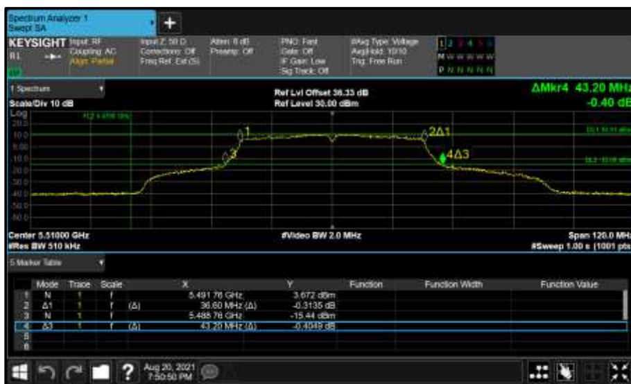
Figure 467 - Core 1 (B) 5510 MHz (CH102) 26 dB and 99% Bandwidth
