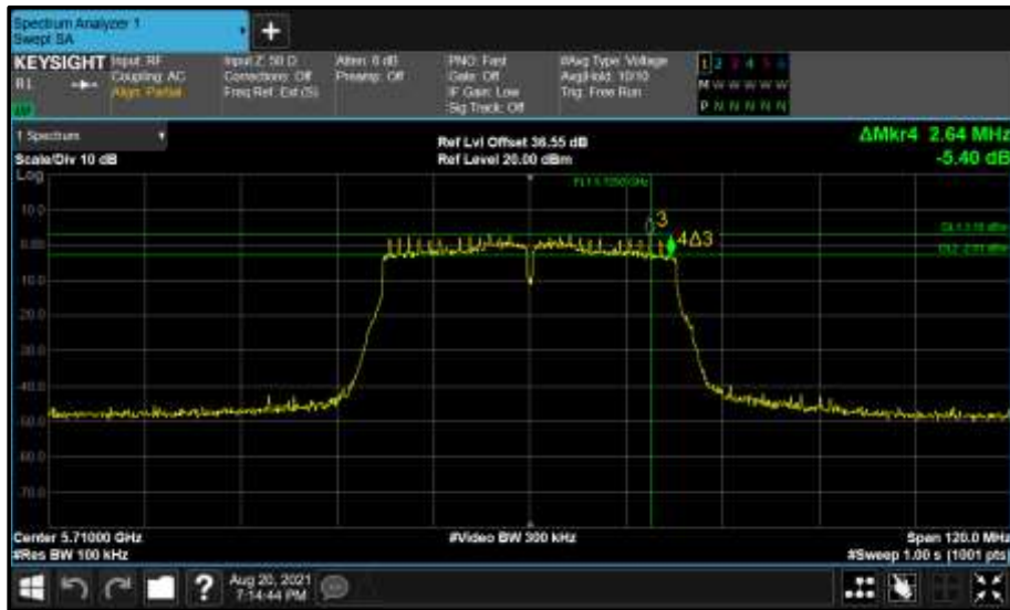
Figure 658 - Core 1 (B) 5710 MHz (CH142) 6 dB Bandwidth
