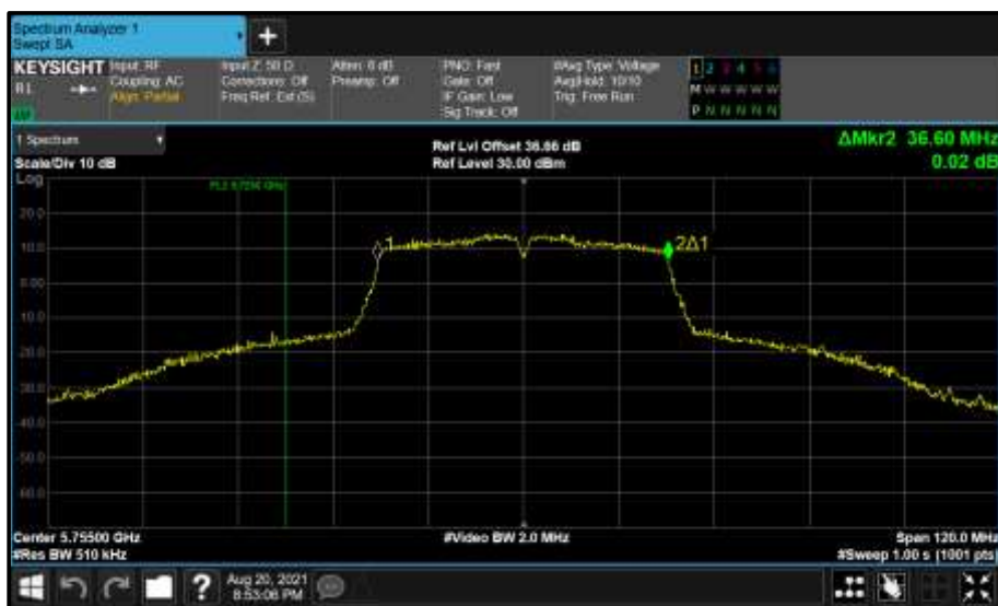
Figure 661 - Core 1 (B) 5755 MHz (CH151) 99% Bandwidth
