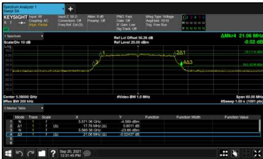
Figure 581 - Core 0 (A) 5580 MHz (CH116) 26 dB and 99% Bandwidth
