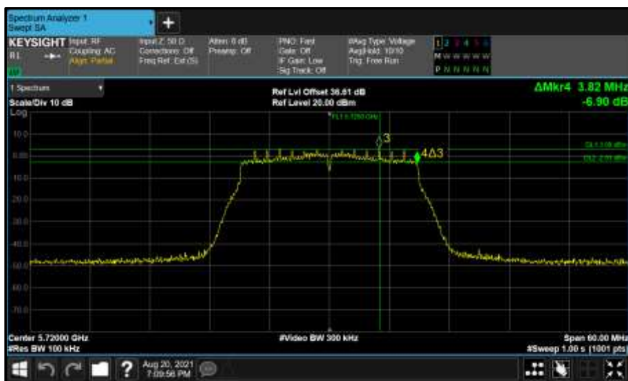
Figure 620 - Core 1 (B) 5720 MHz (CH144) 6 dB Bandwidth
