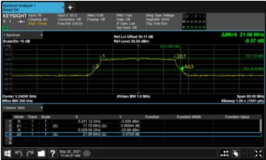
Figure 306 - Core 1 (B) 5240 MHz (CH48) 26 dB and 99% Bandwidth
