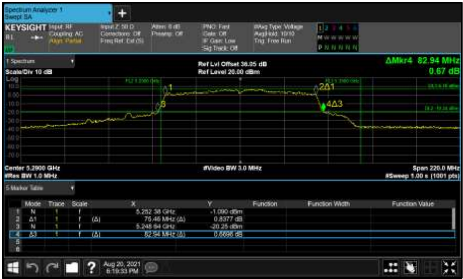
Figure 357 - Core 1 (B) 5290 MHz (CH58) 26 dB and 99% Bandwidth
