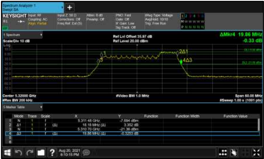
Figure 381 - Core 1 (B) 5320 MHz (CH64) 26 dB and 99% Bandwidth
