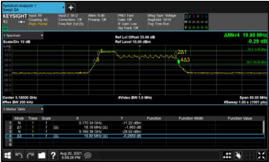
Figure 224 - Core 1 (B) 5180 MHz (CH36) 26 dB and 99% Bandwidth
