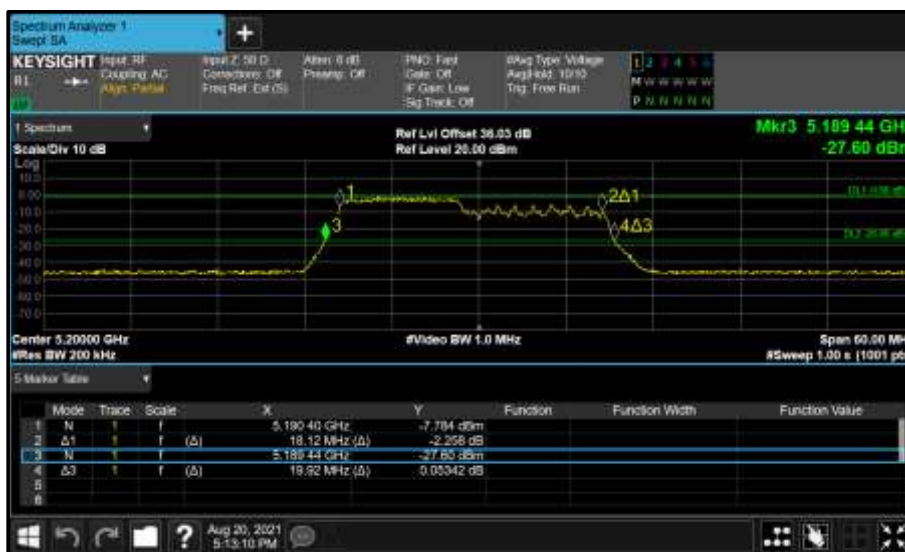
Figure 256 - Core 1 (B) 5200 MHz (CH40) 26 dB and 99% Bandwidth
