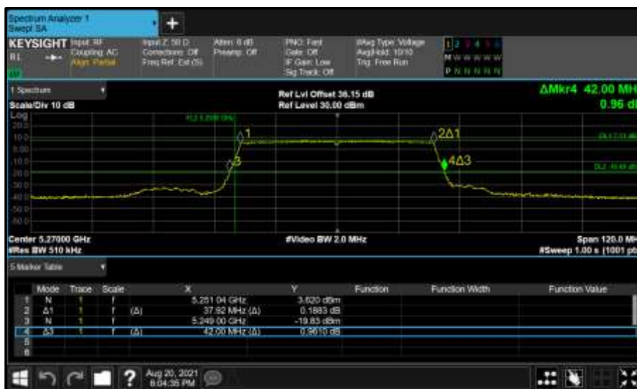
Figure 406 - Core 1 (B) 5270 MHz (CH54) 26 dB and 99% Bandwidth
