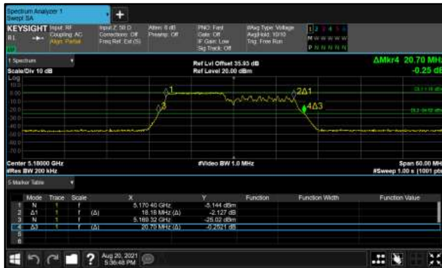
Figure 265 - Core 0 (A) 5180 MHz (CH36) 26 dB and 99% Bandwidth
