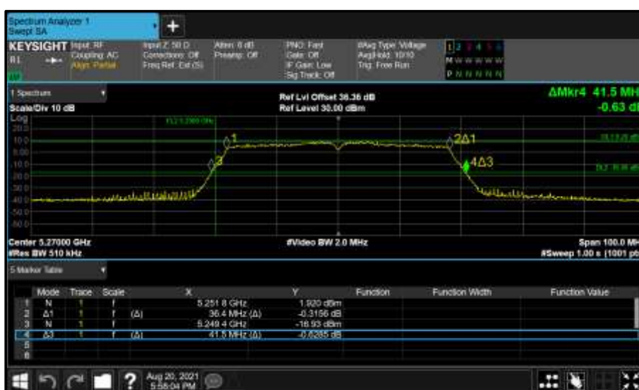
Figure 345 - Core 0 (A) 5270 MHz (CH54) 26 dB and 99% Bandwidth
