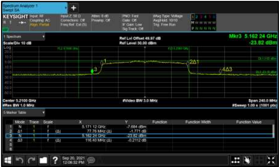
Figure 324 - Core 1 (B) 5210 MHz (CH42) 26 dB and 99% Bandwidth
