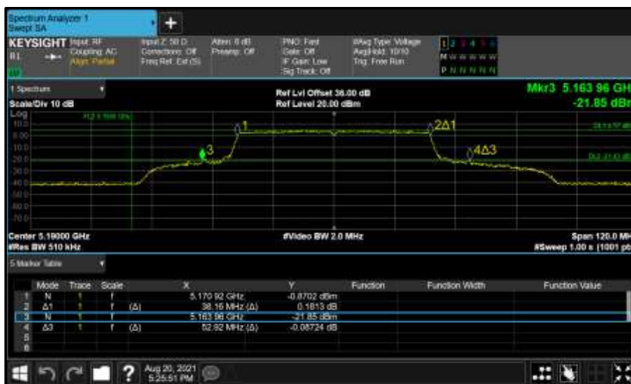
Figure 288 - Core 1 (B) 5190 MHz (CH38) 26 dB and 99% Bandwidth
