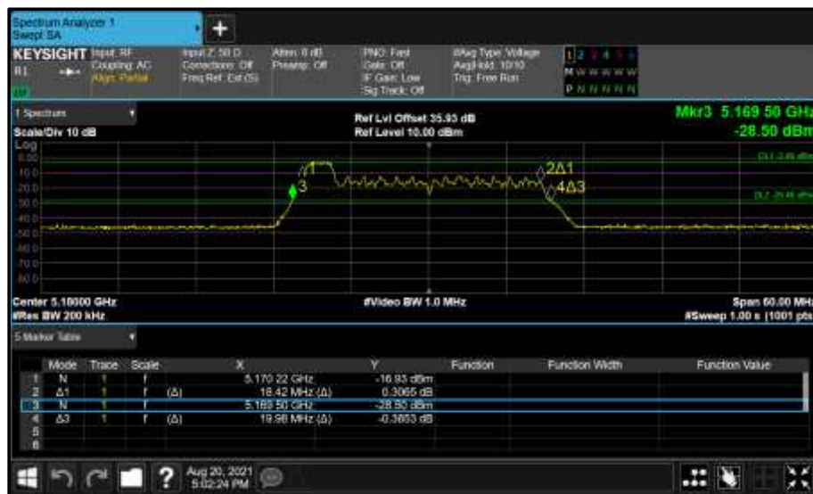
Figure 193 - Core 0 (A) 5180 MHz (CH36) 26 dB and 99% Bandwidth
