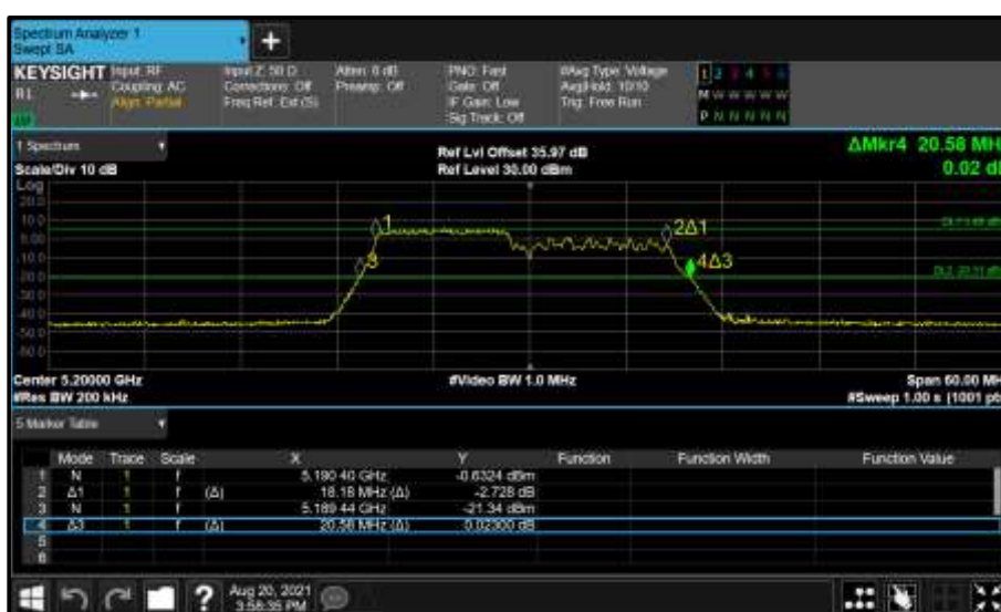
Figure 249 - Core 0 (A) 5200 MHz (CH40) 26 dB and 99% Bandwidth
