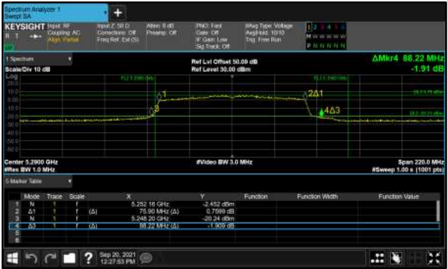
Figure 429 - Core 1 (B) 5290 MHz (CH58) 26 dB and 99% Bandwidth
