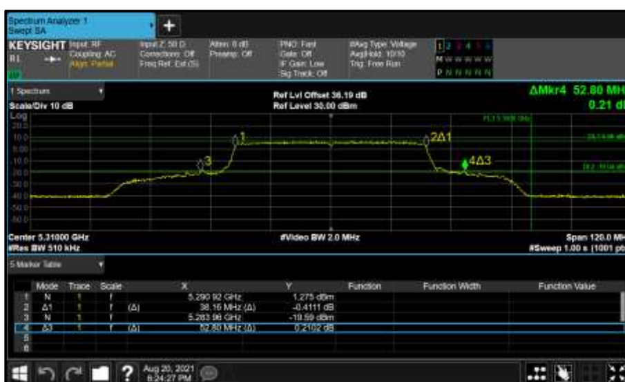
Figure 411 - Core 0 (A) 5310 MHz (CH62) 26 dB and 99% Bandwidth
