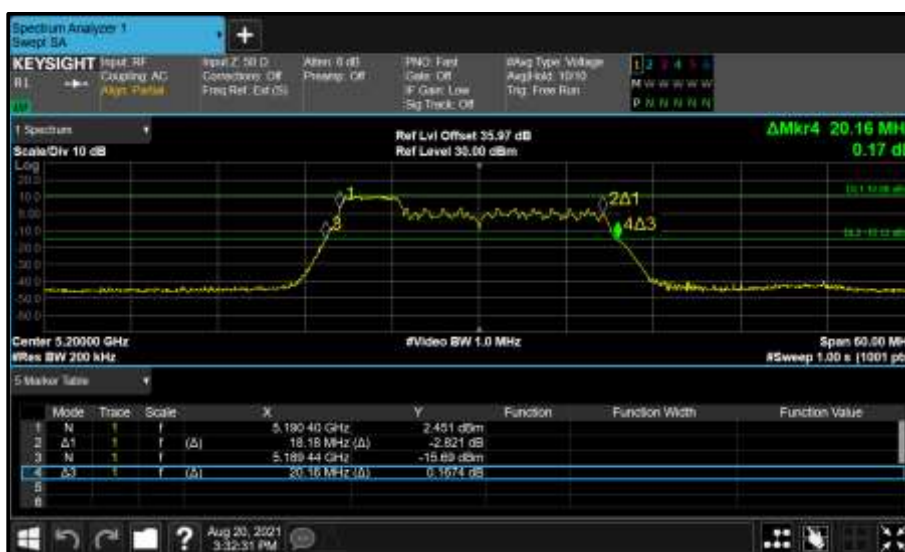
Figure 212 - Core 0 (A) 5200 MHz (CH40) 26 dB and 99% Bandwidth
