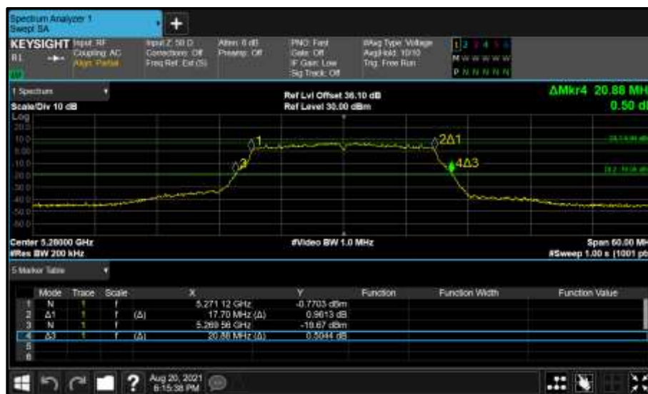
Figure 340 - Core 1 (B) 5280 MHz (CH56) 26 dB and 99% Bandwidth
