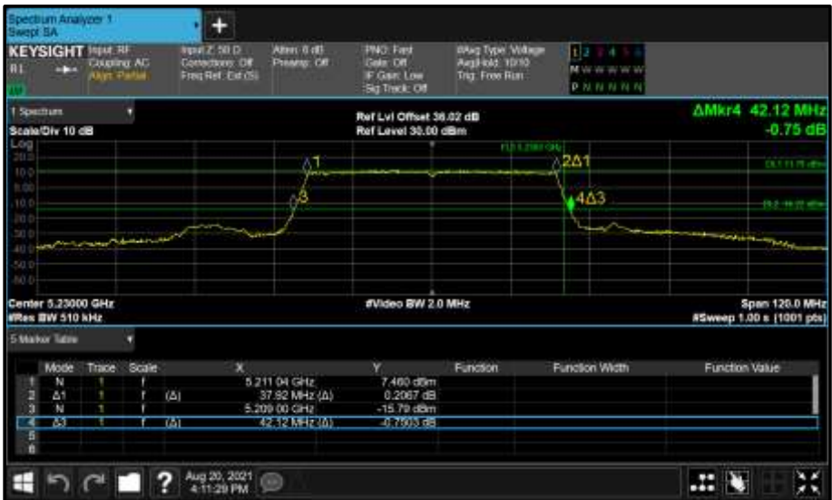
Figure 285 - Core 0 (A) 5230 MHz (CH46) 26 dB and 99% Bandwidth
