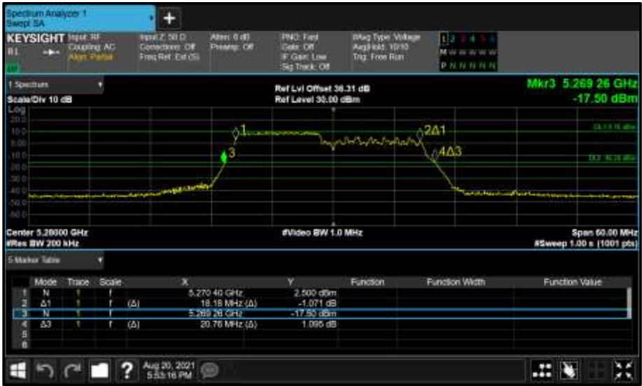
Figure 389 - Core 0 (A) 5280 MHz (CH56) 26 dB and 99% Bandwidth
