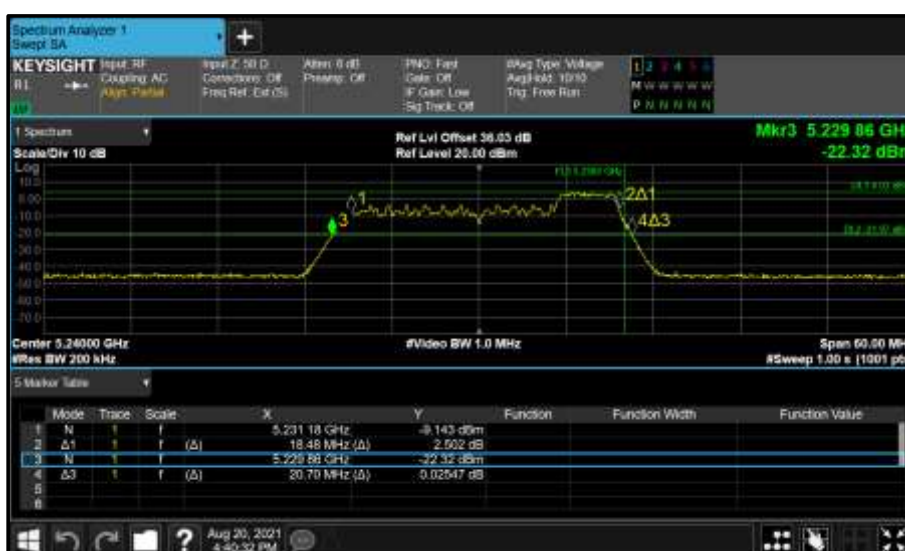
Figure 216 - Core 0 (A) 5240 MHz (CH48) 26 dB and 99% Bandwidth
