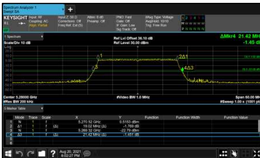
Figure 364 - Core 1 (B) 5280 MHz (CH56) 26 dB and 99% Bandwidth
