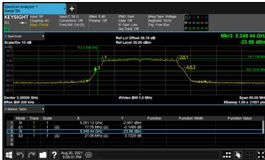
Figure 332 - Core 1 (B) 5260 MHz (CH52) 26 dB and 99% Bandwidth
