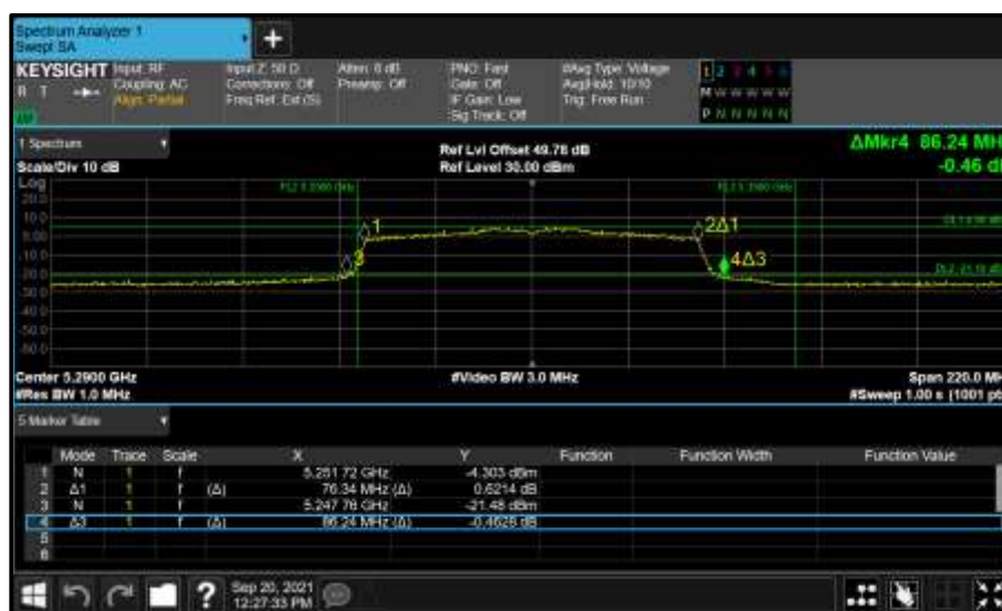
Figure 428 - Core 0 (A) 5290 MHz (CH58) 26 dB and 99% Bandwidth
