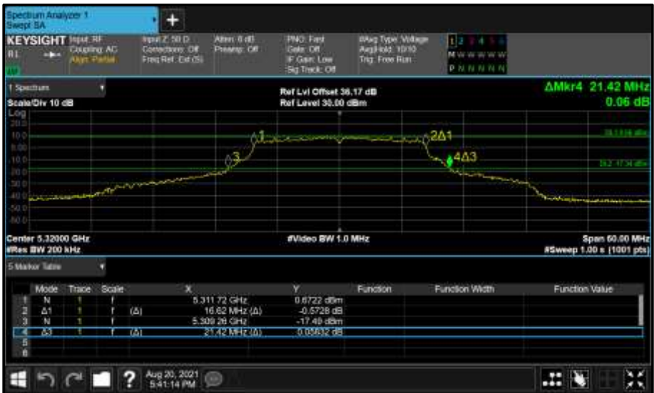
Figure 327 - Core 0 (A) 5320 MHz (CH64) 26 dB and 99% Bandwidth
