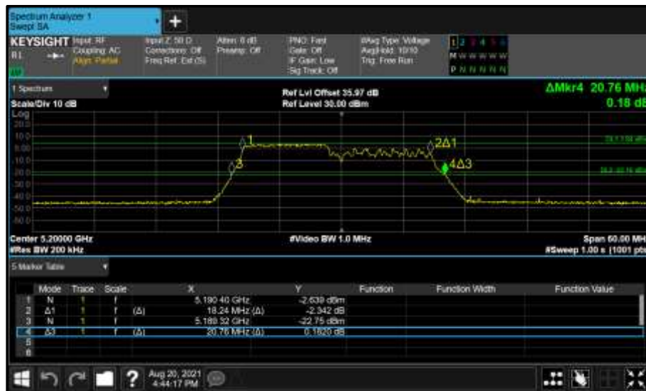
Figure 245 - Core 0 (A) 5200 MHz (CH40) 26 dB and 99% Bandwidth
