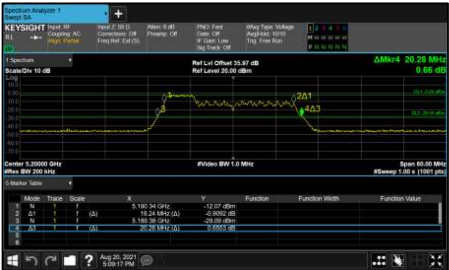
Figure 225 - Core 0 (A) 5200 MHz (CH40) 26 dB and 99% Bandwidth
