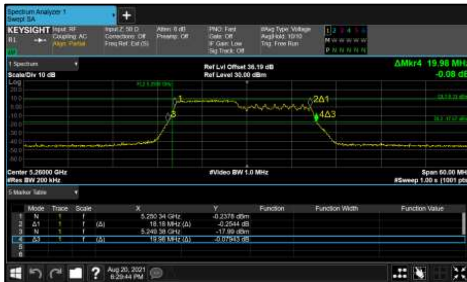
Figure 398 - Core 1 (B) 5260 MHz (CH52) 26 dB and 99% Bandwidth
