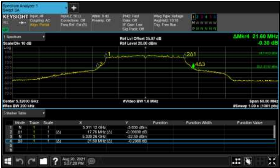
Figure 336 - Core 1 (B) 5320 MHz (CH64) 26 dB and 99% Bandwidth
