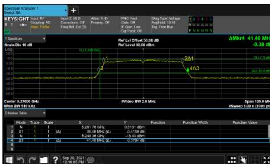
Figure 425 - Core 1 (B) 5270 MHz (CH54) 26 dB and 99% Bandwidth
