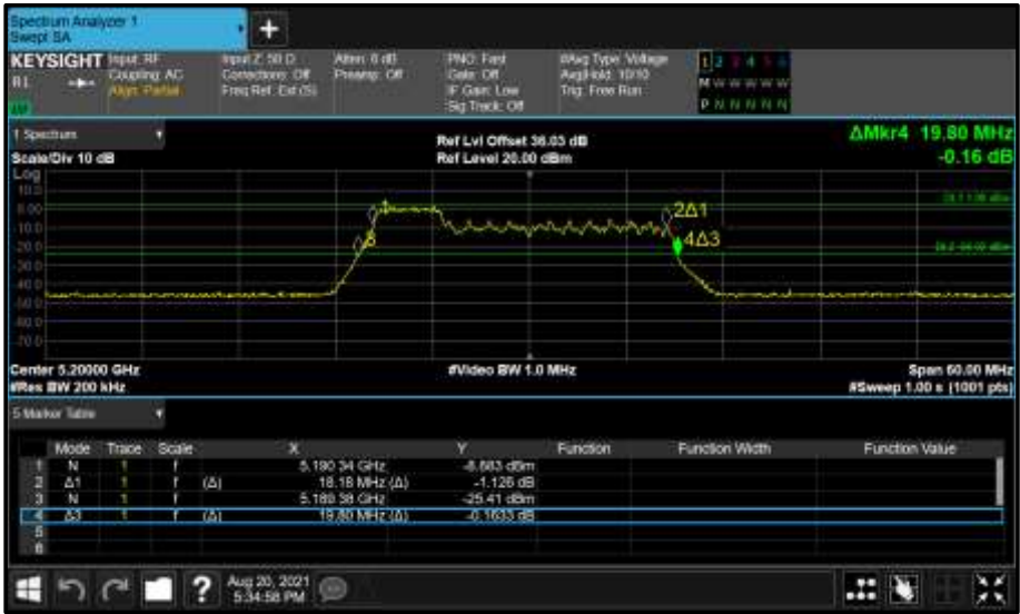
Figure 238 - Core 1 (B) 5200 MHz (CH40) 26 dB and 99% Bandwidth
