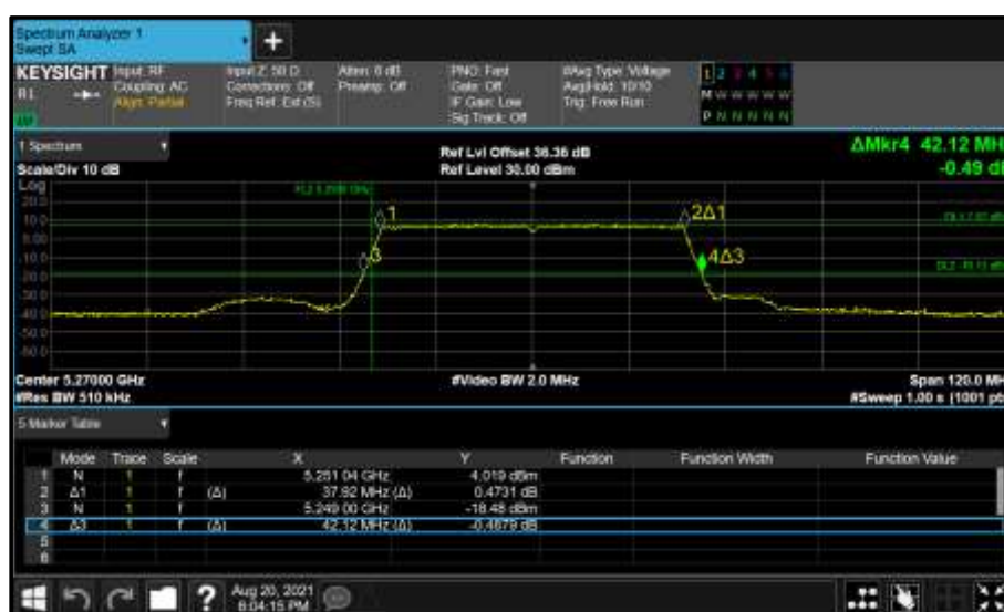
Figure 405 - Core 0 (A) 5270 MHz (CH54) 26 dB and 99% Bandwidth
