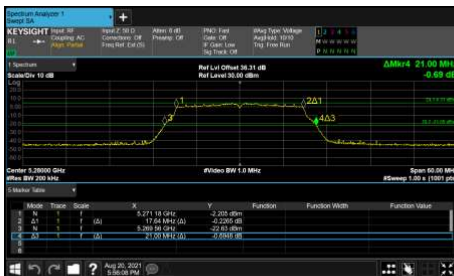
Figure 333 - Core 0 (A) 5280 MHz (CH56) 26 dB and 99% Bandwidth
