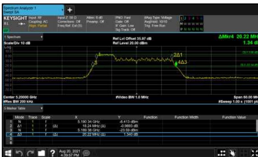
Figure 215 - Core 0 (A) 5200 MHz (CH40) 26 dB and 99% Bandwidth
