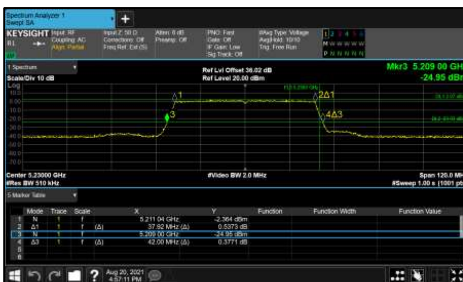
Figure 281 - Core 0 (A) 5230 MHz (CH46) 26 dB and 99% Bandwidth
