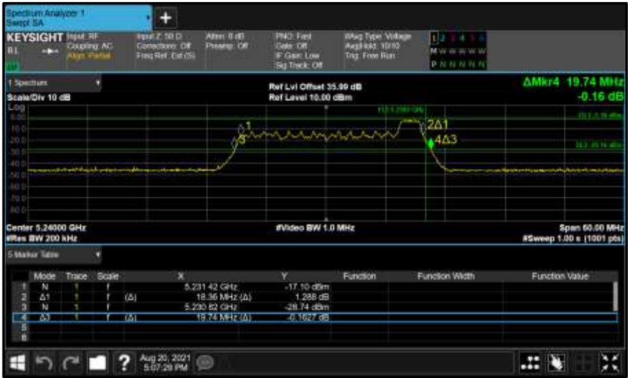
Figure 198 - Core 1 (B) 5240 MHz (CH48) 26 dB and 99% Bandwidth
