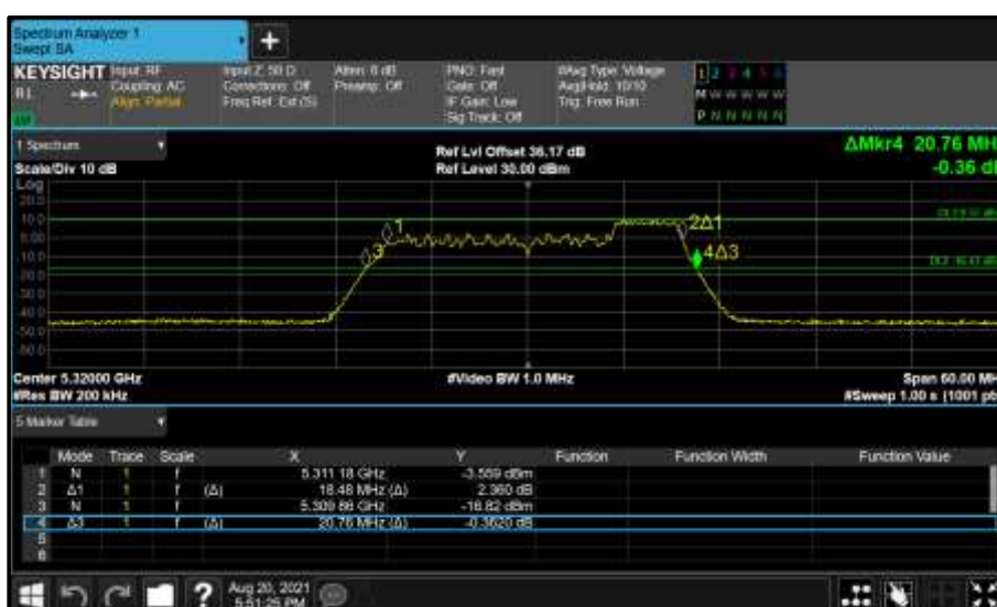
Figure 375 - Core 0 (A) 5320 MHz (CH64) 26 dB and 99% Bandwidth
