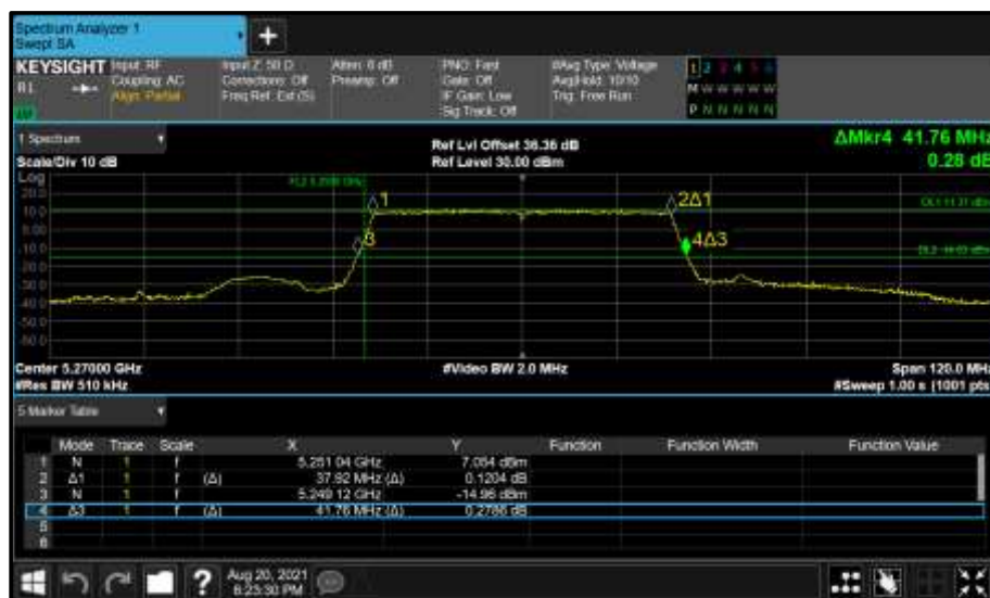
Figure 409 - Core 0 (A) 5270 MHz (CH54) 26 dB and 99% Bandwidth
