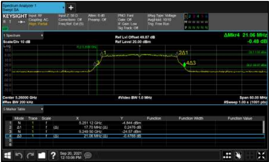
Figure 418 - Core 0 (A) 5260 MHz (CH52) 26 dB and 99% Bandwidth
