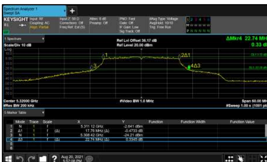
Figure 335 - Core 0 (A) 5320 MHz (CH64) 26 dB and 99% Bandwidth
