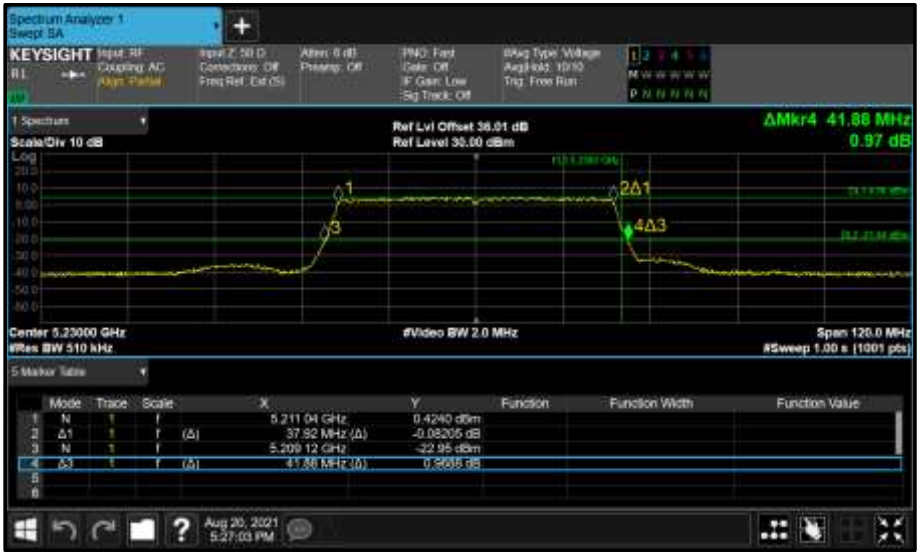
Figure 290 - Core 1 (B) 5230 MHz (CH46) 26 dB and 99% Bandwidth
