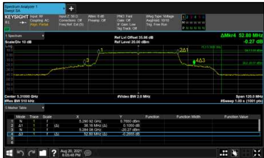
Figure 408 - Core 1 (B) 5310 MHz (CH62) 26 dB and 99% Bandwidth
