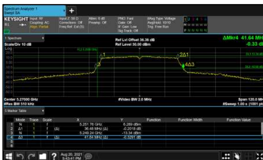
Figure 343 - Core 0 (A) 5270 MHz (CH54) 26 dB and 99% Bandwidth
