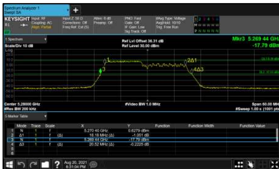
Figure 399 - Core 0 (A) 5280 MHz (CH56) 26 dB and 99% Bandwidth
