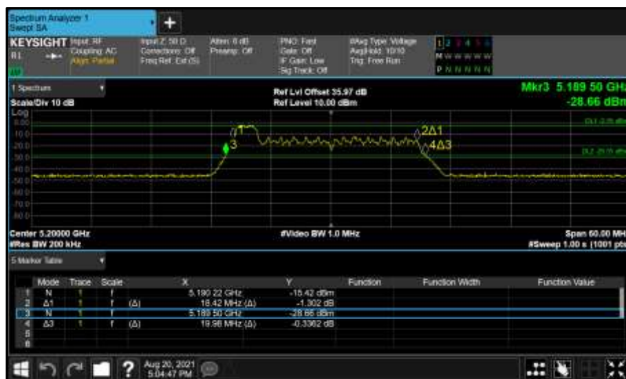
Figure 195 - Core 0 (A) 5200 MHz (CH40) 26 dB and 99% Bandwidth
