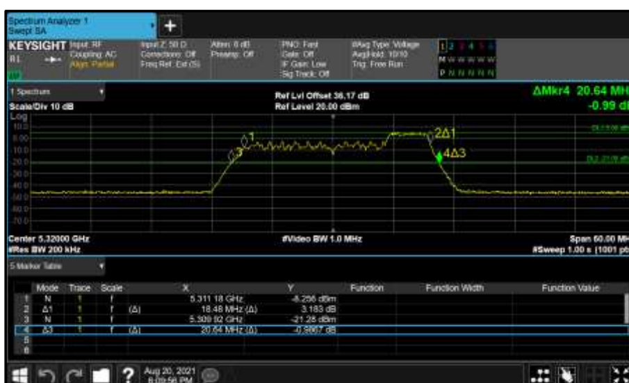
Figure 380 - Core 0 (A) 5320 MHz (CH64) 26 dB and 99% Bandwidth
