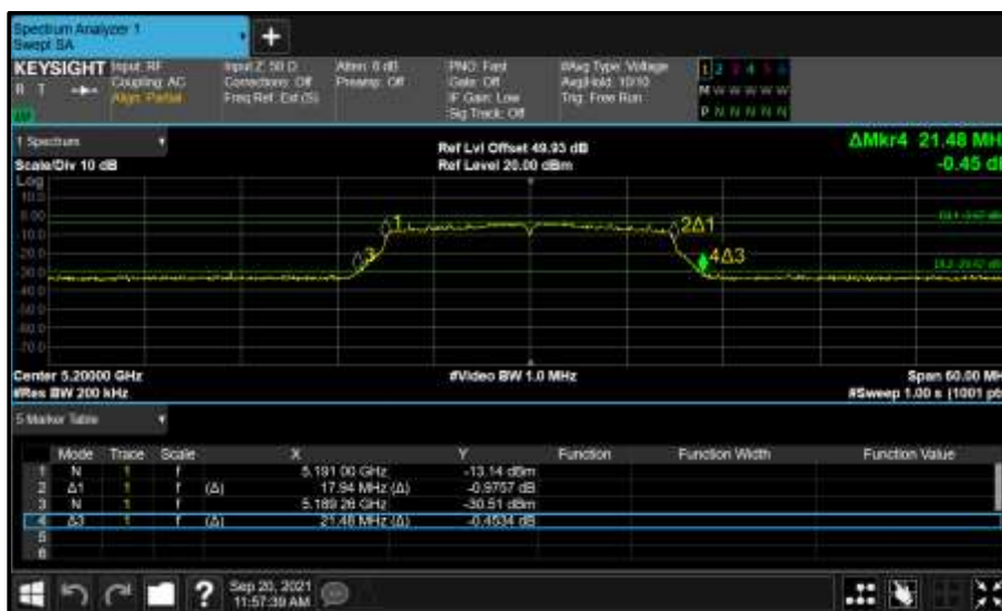
Figure 310 - Core 1 (B) 5200 MHz (CH40) 26 dB and 99% Bandwidth
