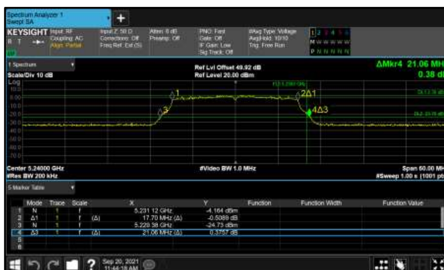
Figure 305 - Core 0 (A) 5240 MHz (CH48) 26 dB and 99% Bandwidth
