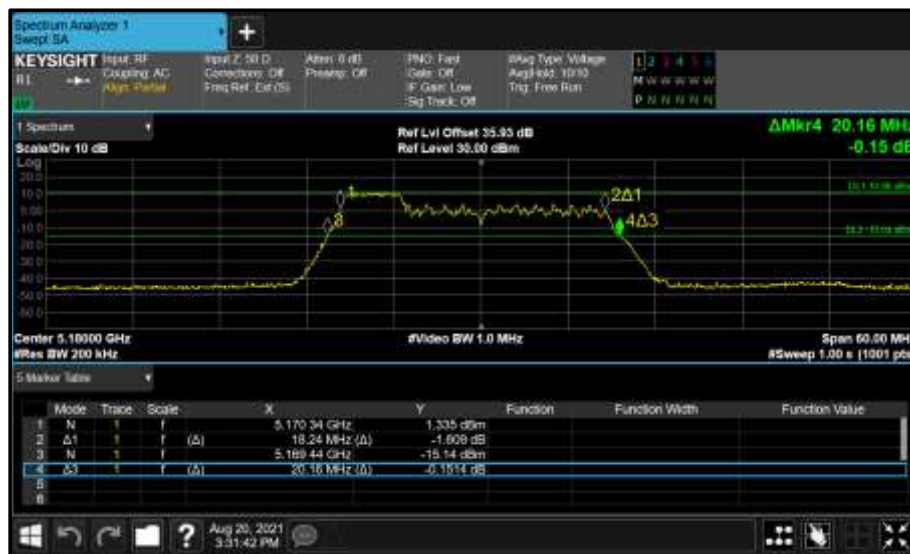
Figure 211 - Core 0 (A) 5180 MHz (CH36) 26 dB and 99% Bandwidth
