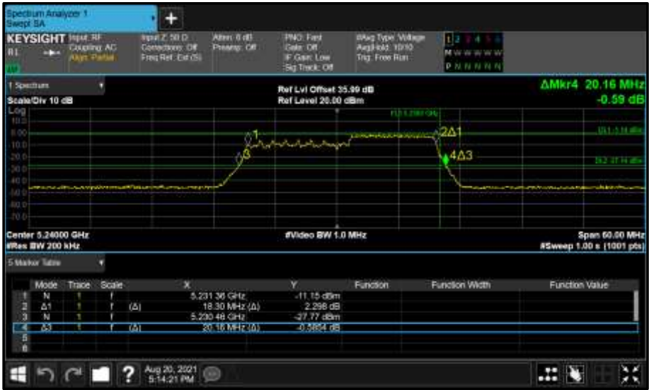
Figure 258 - Core 1 (B) 5240 MHz (CH48) 26 dB and 99% Bandwidth
