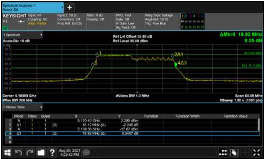
Figure 260 - Core 1 (B) 5180 MHz (CH36) 26 dB and 99% Bandwidth
