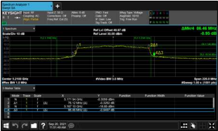
Figure 322 - Core 1 (B) 5210 MHz (CH42) 26 dB and 99% Bandwidth
