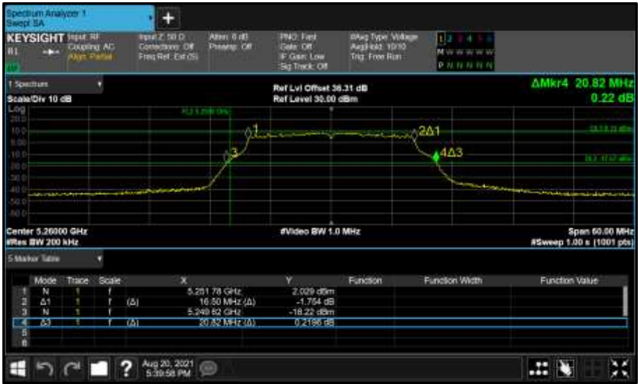
Figure 325 - Core 0 (A) 5260 MHz (CH52) 26 dB and 99% Bandwidth
