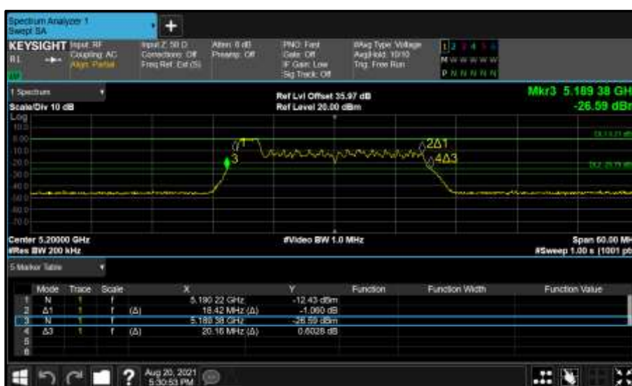
Figure 207 - Core 0 (A) 5200 MHz (CH40) 26 dB and 99% Bandwidth
