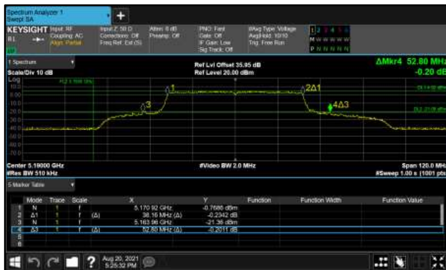
Figure 287 - Core 0 (A) 5190 MHz (CH38) 26 dB and 99% Bandwidth
