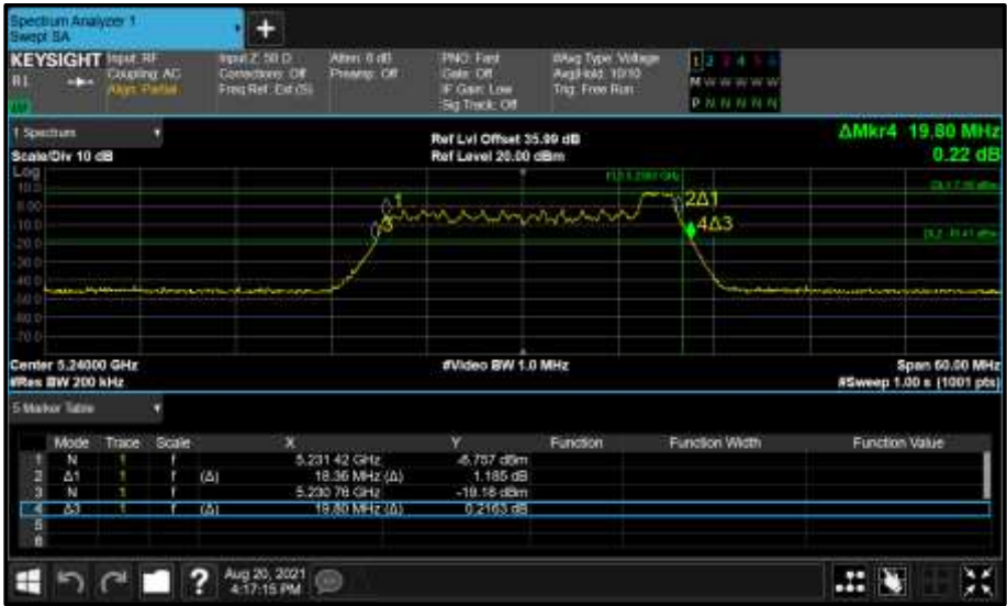
Figure 204 - Core 1 (B) 5240 MHz (CH48) 26 dB and 99% Bandwidth
