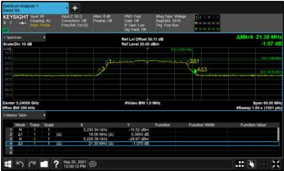
Figure 312 - Core 1 (B) 5240 MHz (CH48) 26 dB and 99% Bandwidth
