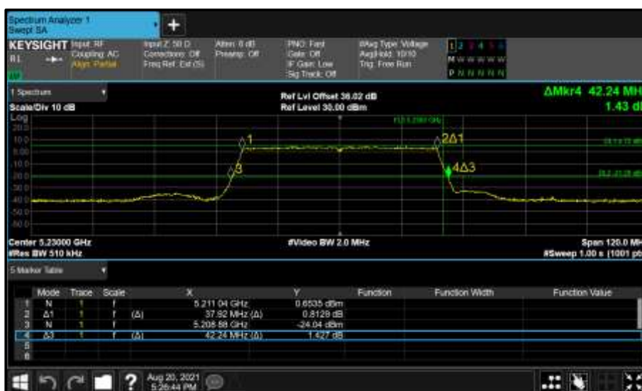
Figure 289 - Core 0 (A) 5230 MHz (CH46) 26 dB and 99% Bandwidth
