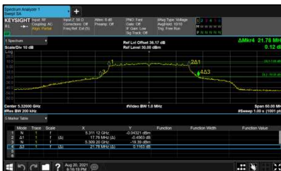
Figure 341 - Core 0 (A) 5320 MHz (CH64) 26 dB and 99% Bandwidth
