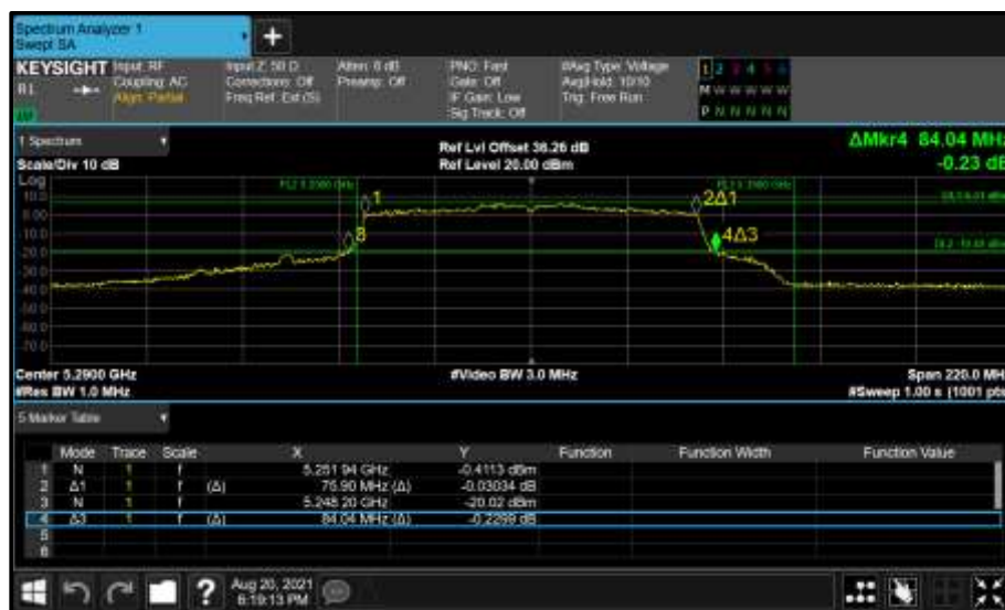
Figure 356 - Core 0 (A) 5290 MHz (CH58) 26 dB and 99% Bandwidth
