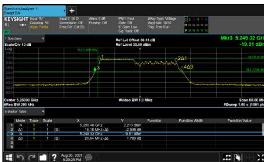
Figure 397 - Core 0 (A) 5260 MHz (CH52) 26 dB and 99% Bandwidth
