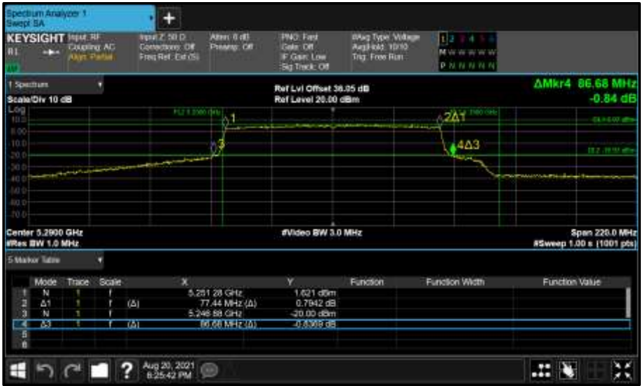
Figure 417 - Core 1 (B) 5290 MHz (CH58) 26 dB and 99% Bandwidth
