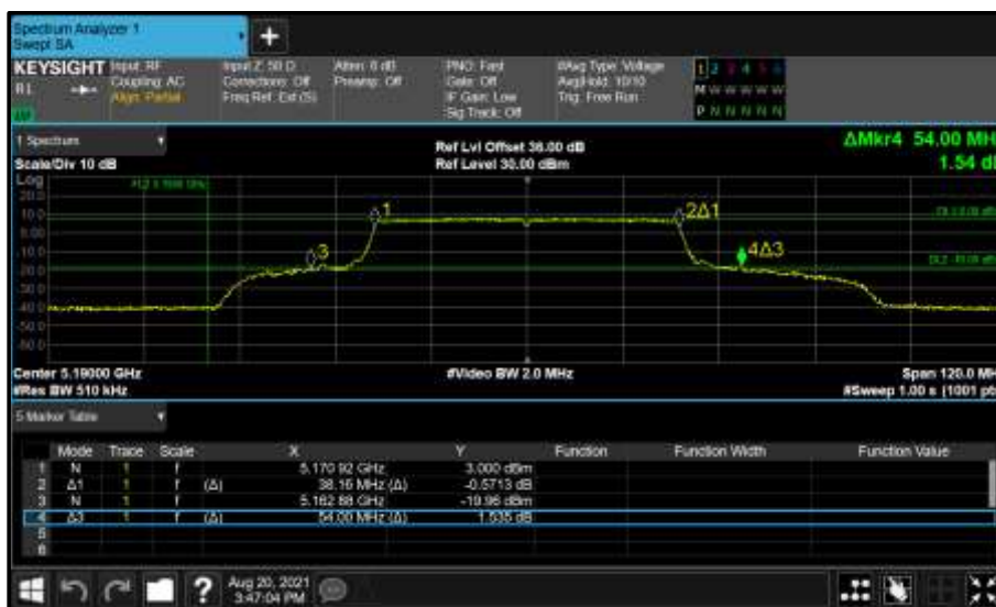
Figure 276 - Core 1 (B) 5190 MHz (CH38) 26 dB and 99% Bandwidth
