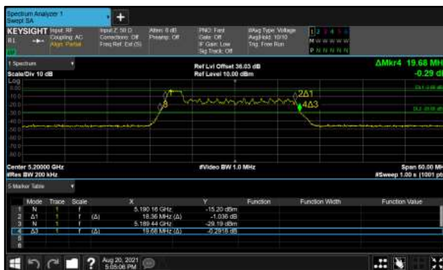
Figure 196 - Core 1 (B) 5200 MHz (CH40) 26 dB and 99% Bandwidth
