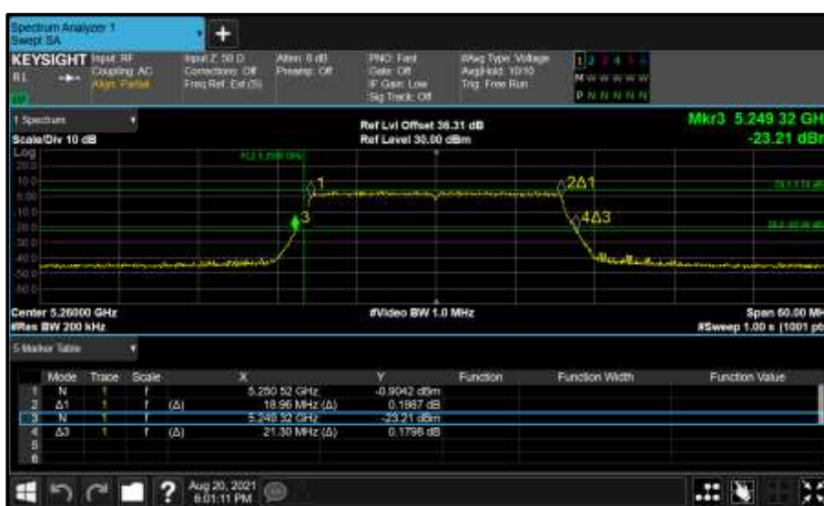
Figure 361 - Core 0 (A) 5260 MHz (CH52) 26 dB and 99% Bandwidth
