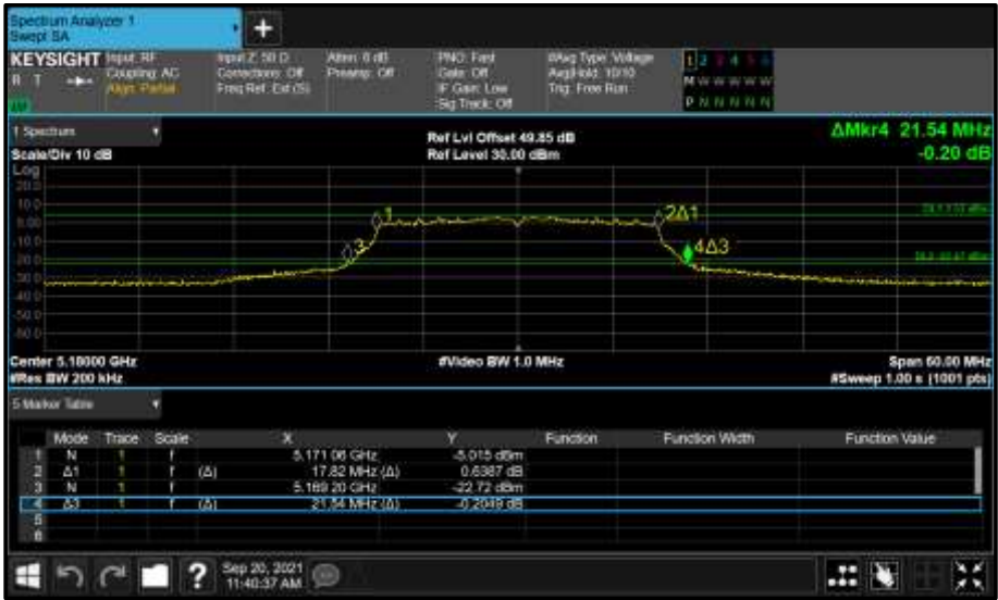
Figure 302 - Core 1 (B) 5180 MHz (CH36) 26 dB and 99% Bandwidth
