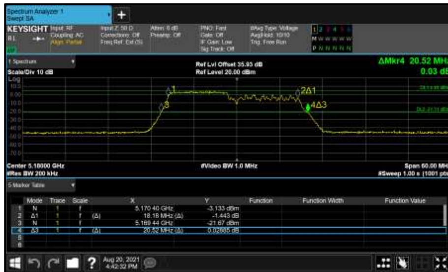
Figure 244 - Core 0 (A) 5180 MHz (CH36) 26 dB and 99% Bandwidth
