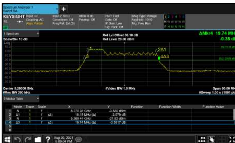
Figure 379 - Core 1 (B) 5280 MHz (CH56) 26 dB and 99% Bandwidth
