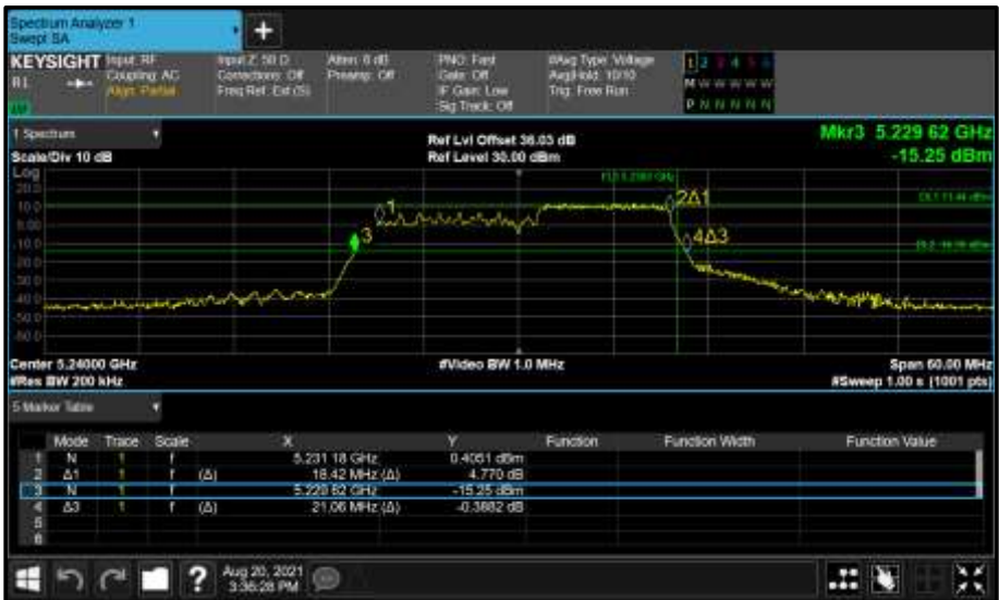
Figure 243 - Core 0 (A) 5240 MHz (CH48) 26 dB and 99% Bandwidth
