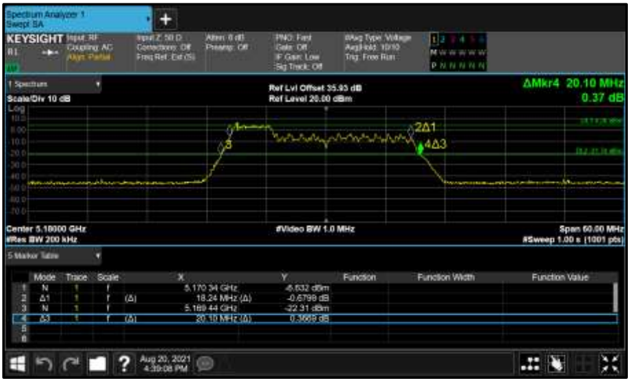
Figure 214 - Core 0 (A) 5180 MHz (CH36) 26 dB and 99% Bandwidth
