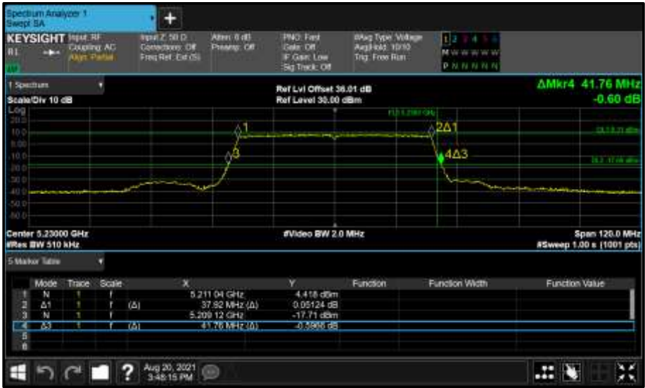
Figure 278 - Core 1 (B) 5230 MHz (CH46) 26 dB and 99% Bandwidth
