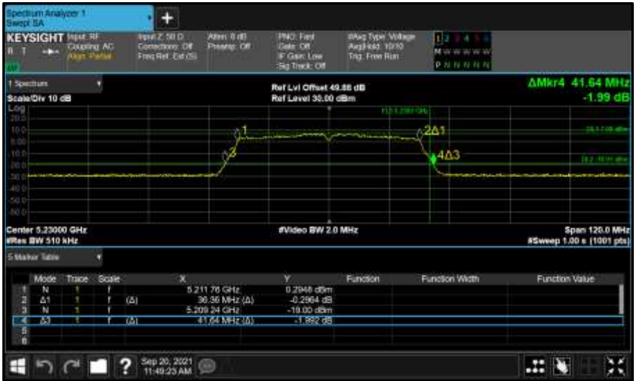
Figure 315 - Core 0 (A) 5230 MHz (CH46) 26 dB and 99% Bandwidth
