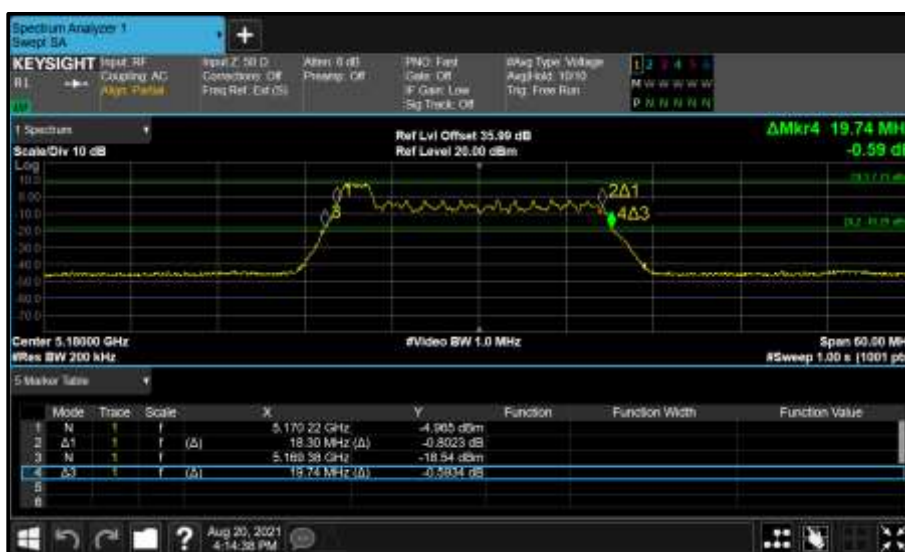
Figure 200 - Core 1 (B) 5180 MHz (CH36) 26 dB and 99% Bandwidth
