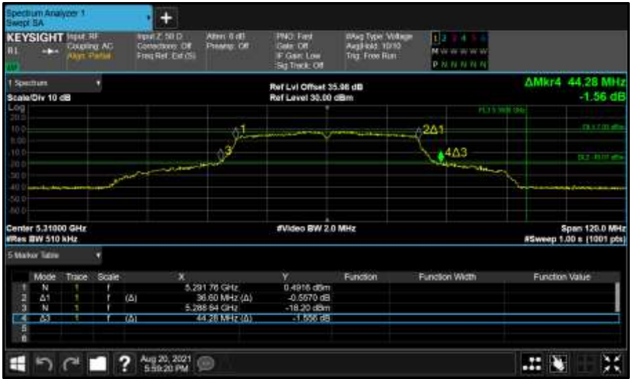
Figure 348 - Core 1 (B) 5310 MHz (CH62) 26 dB and 99% Bandwidth
