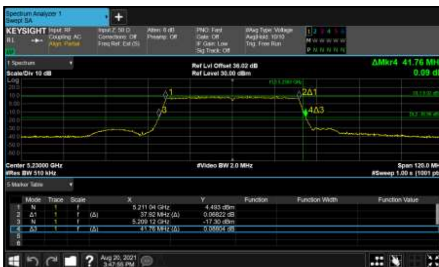
Figure 277 - Core 0 (A) 5230 MHz (CH46) 26 dB and 99% Bandwidth
