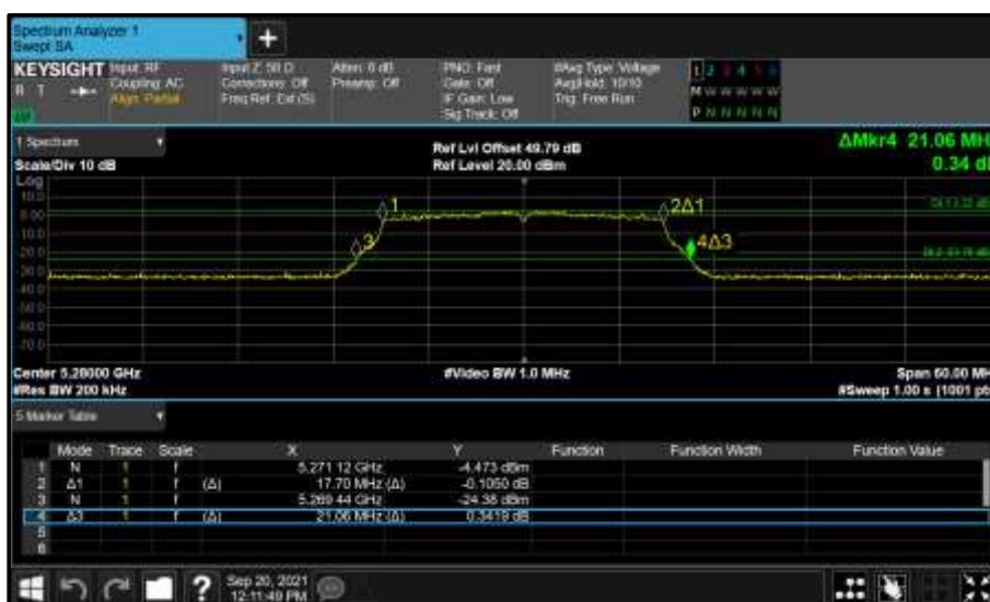
Figure 420 - Core 0 (A) 5280 MHz (CH56) 26 dB and 99% Bandwidth
