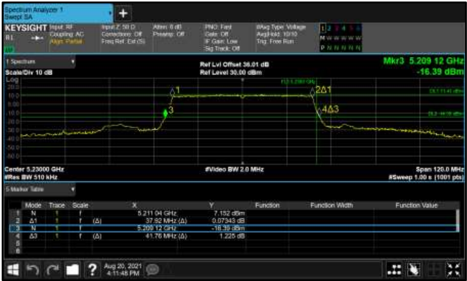
Figure 286 - Core 1 (B) 5230 MHz (CH46) 26 dB and 99% Bandwidth
