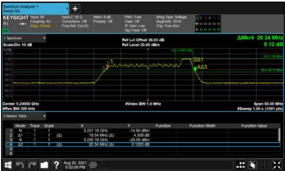
Figure 209 - Core 0 (A) 5240 MHz (CH48) 26 dB and 99% Bandwidth
