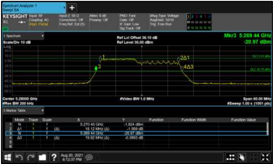
Figure 394 - Core 1 (B) 5280 MHz (CH56) 26 dB and 99% Bandwidth
