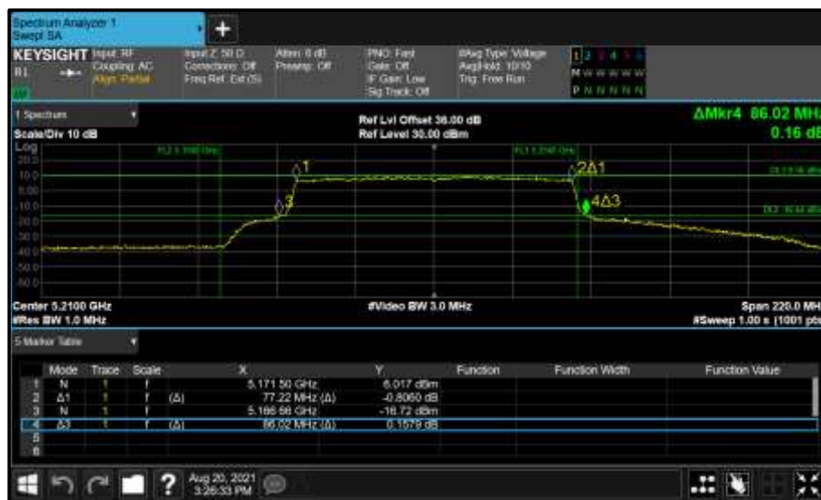
Figure 291 - Core 0 (A) 5210 MHz (CH42) 26 dB and 99% Bandwidth
