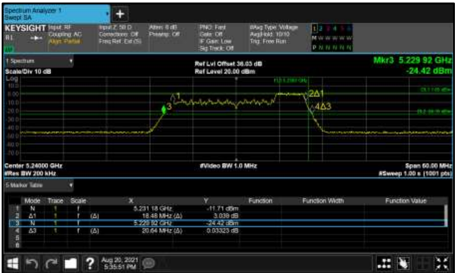
Figure 239 - Core 0 (A) 5240 MHz (CH48) 26 dB and 99% Bandwidth
