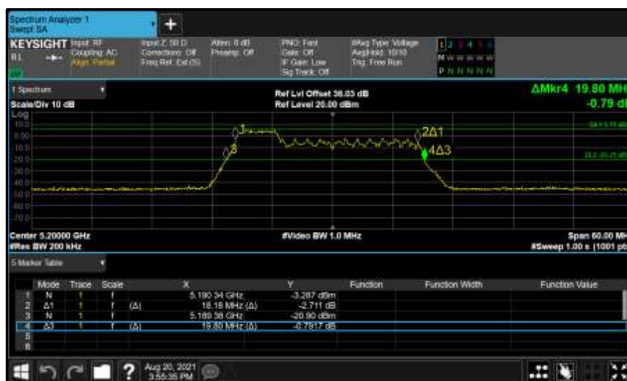
Figure 220 - Core 1 (B) 5200 MHz (CH40) 26 dB and 99% Bandwidth
