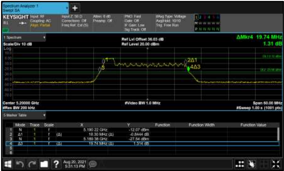
Figure 208 - Core 1 (B) 5200 MHz (CH40) 26 dB and 99% Bandwidth
