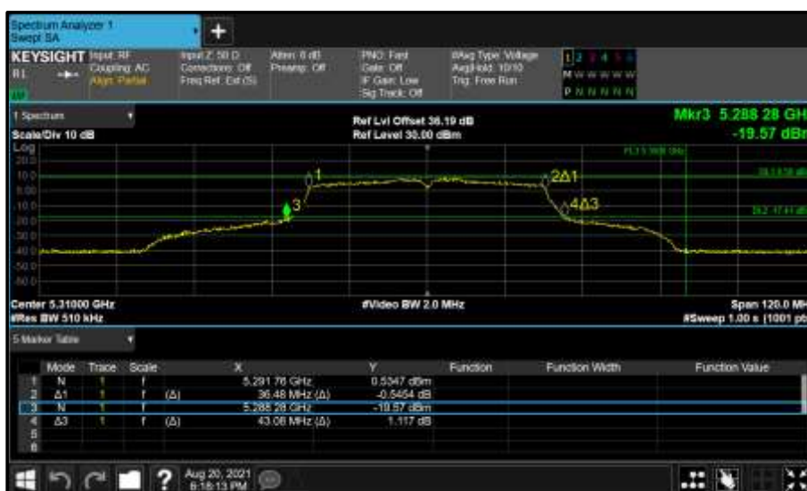
Figure 351 - Core 0 (A) 5310 MHz (CH62) 26 dB and 99% Bandwidth
