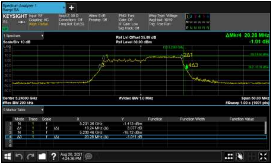
Figure 264 - Core 1 (B) 5240 MHz (CH48) 26 dB and 99% Bandwidth
