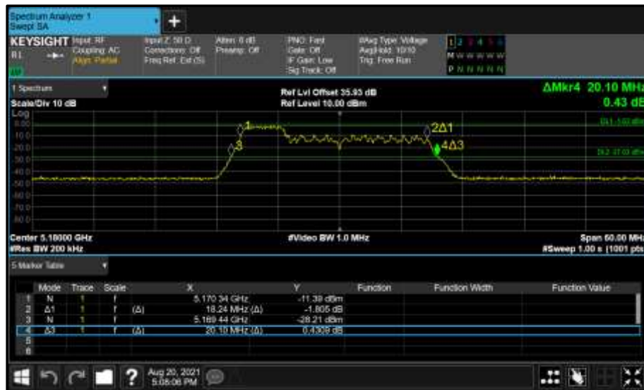
Figure 223 - Core 0 (A) 5180 MHz (CH36) 26 dB and 99% Bandwidth
