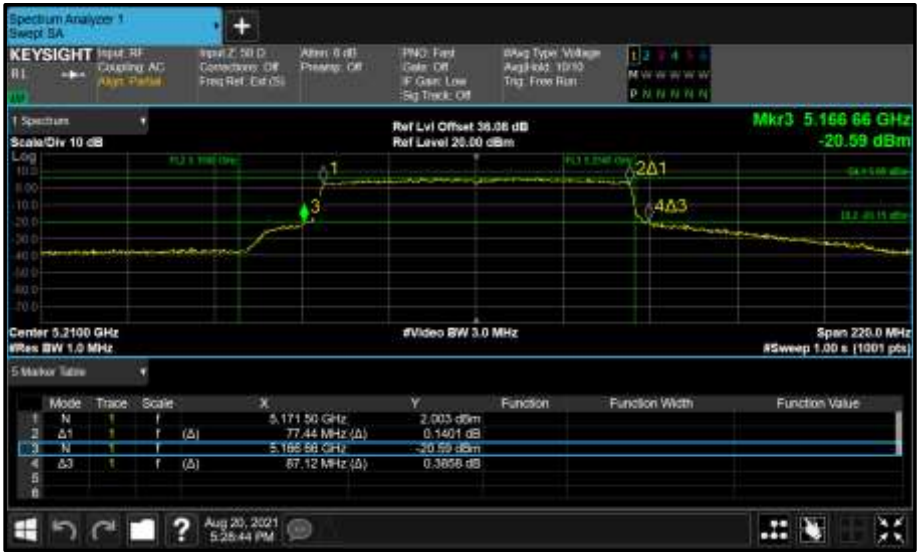
Figure 300 - Core 1 (B) 5210 MHz (CH42) 26 dB and 99% Bandwidth
