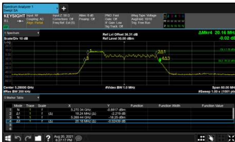
Figure 384 - Core 0 (A) 5280 MHz (CH56) 26 dB and 99% Bandwidth
