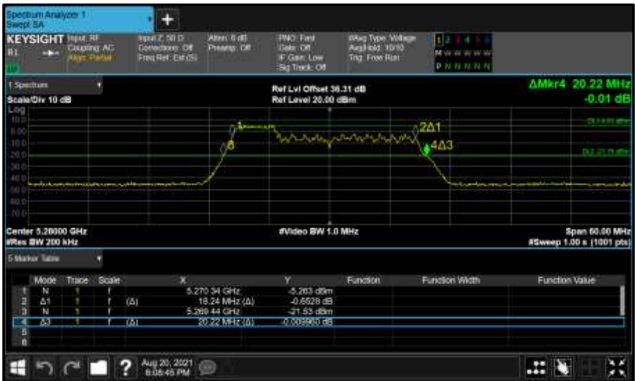
Figure 378 - Core 0 (A) 5280 MHz (CH56) 26 dB and 99% Bandwidth
