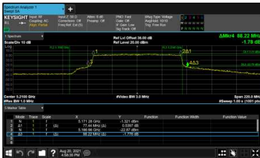
Figure 295 - Core 0 (A) 5210 MHz (CH42) 26 dB and 99% Bandwidth
