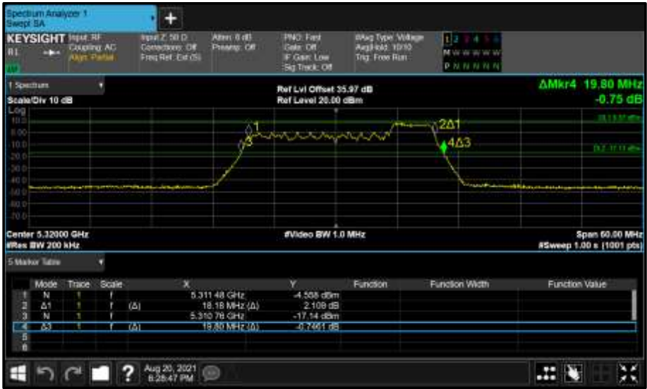
Figure 387 - Core 1 (B) 5320 MHz (CH64) 26 dB and 99% Bandwidth
