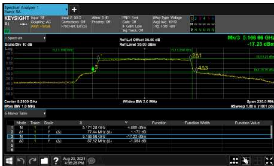
Figure 292 - Core 0 (A) 5210 MHz (CH42) 26 dB and 99% Bandwidth
