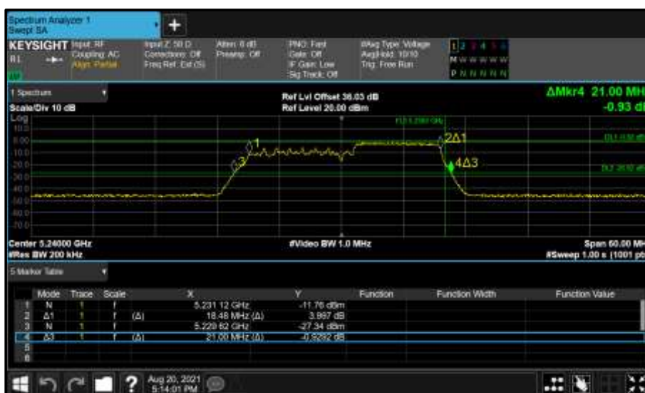
Figure 257 - Core 0 (A) 5240 MHz (CH48) 26 dB and 99% Bandwidth
