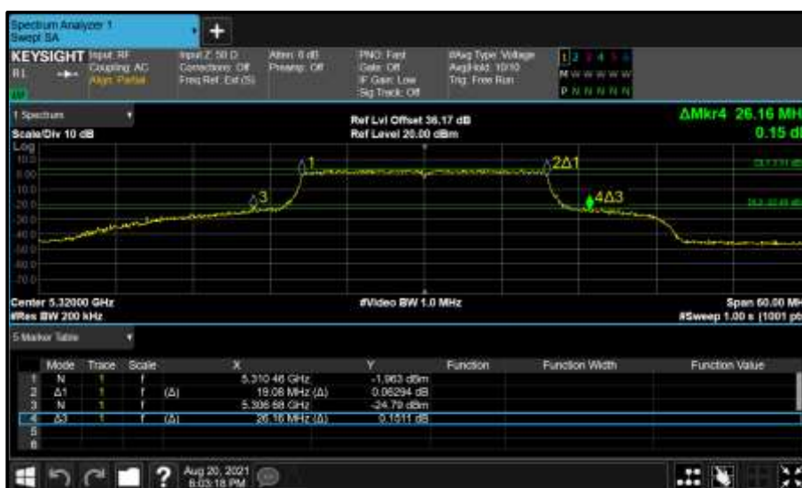
Figure 365 - Core 0 (A) 5320 MHz (CH64) 26 dB and 99% Bandwidth
