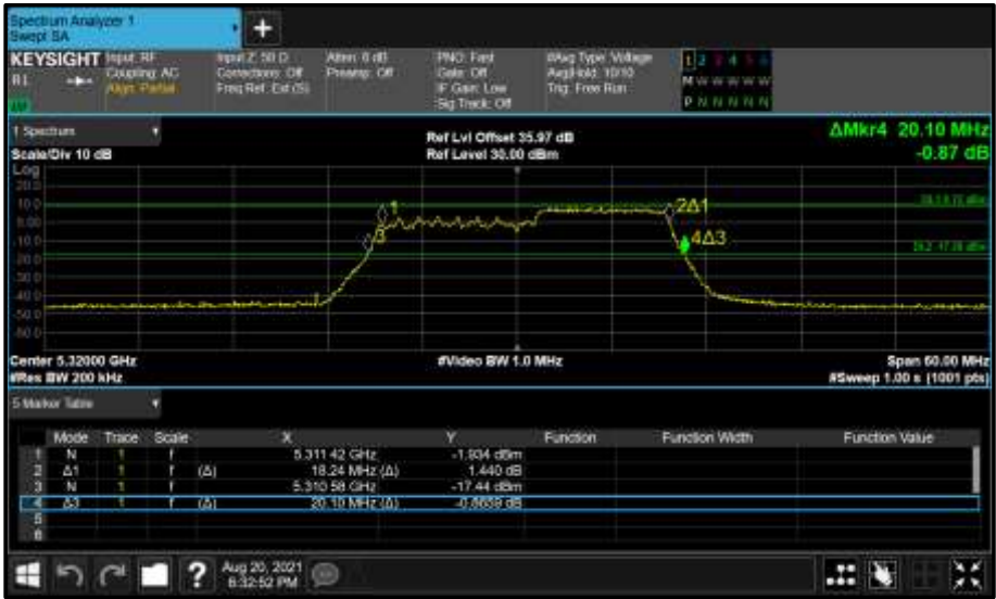
Figure 402 - Core 1 (B) 5320 MHz (CH64) 26 dB and 99% Bandwidth
