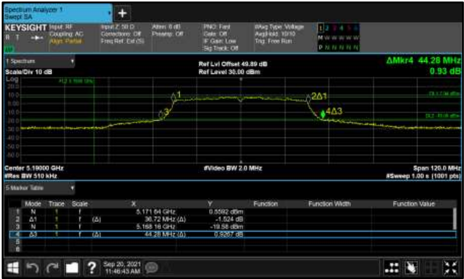
Figure 314 - Core 1 (B) 5190 MHz (CH38) 26 dB and 99% Bandwidth
