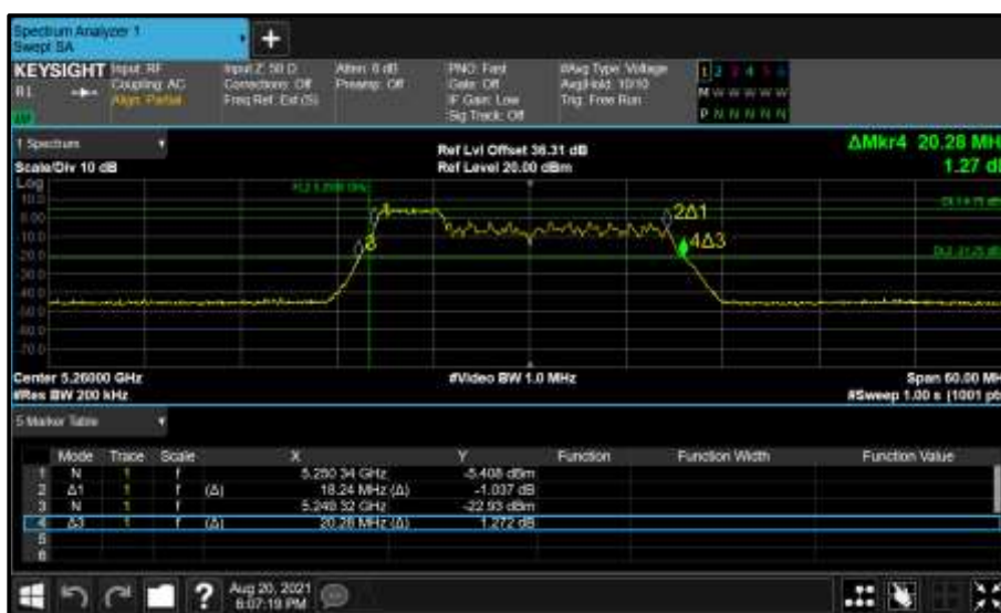
Figure 376 - Core 0 (A) 5260 MHz (CH52) 26 dB and 99% Bandwidth
