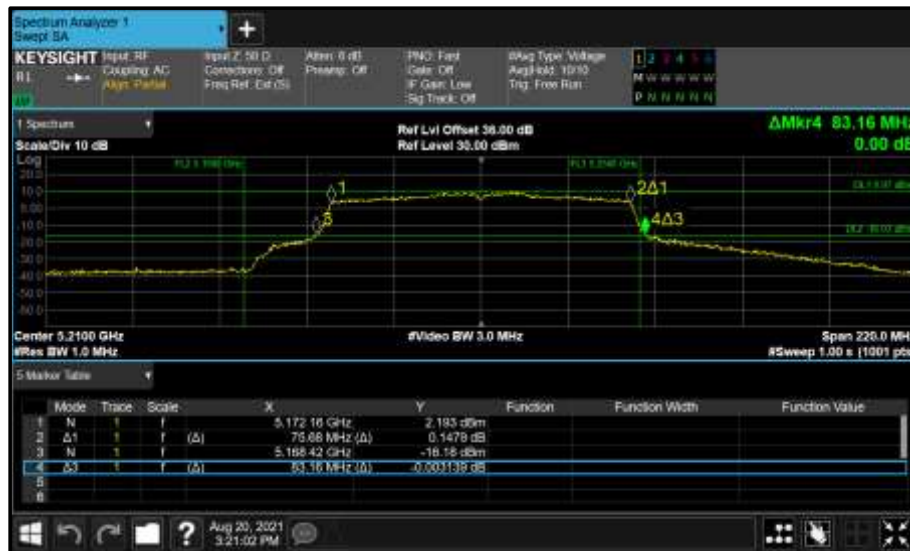
Figure 141 - Core 0 (A) 5210 MHz (CH42) 26 dB and 99% Bandwidth
