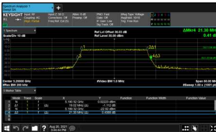
Figure 160 - Core 1 (B) 5200 MHz (CH40) 26 dB and 99% Bandwidth
