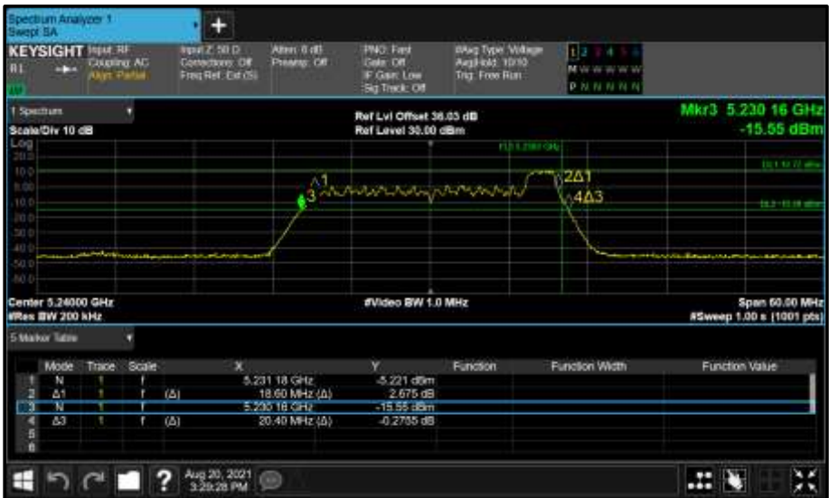
Figure 183 - Core 0 (A) 5240 MHz (CH48) 26 dB and 99% Bandwidth
