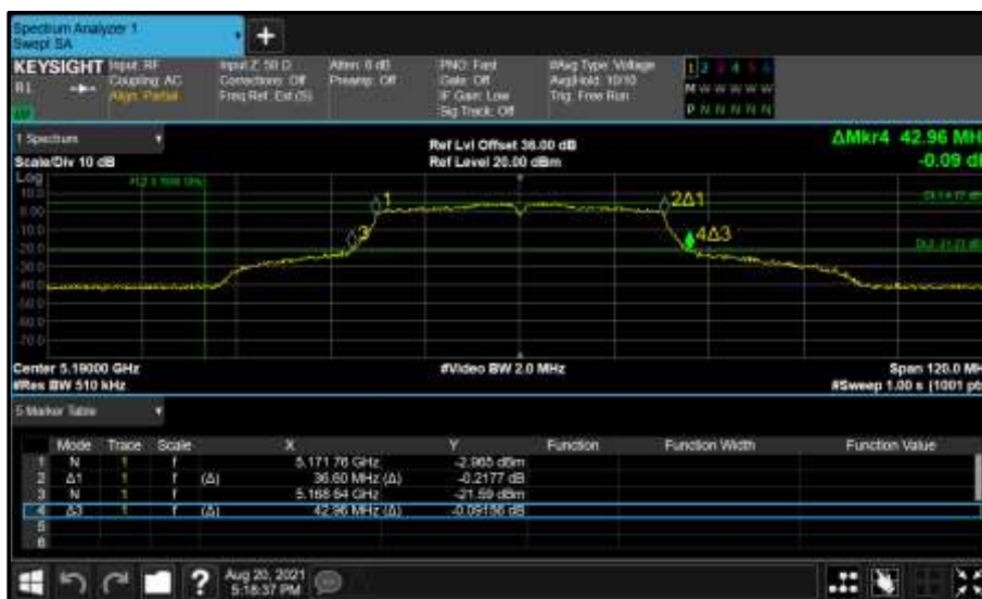
Figure 138 - Core 1 (B) 5190 MHz (CH38) 26 dB and 99% Bandwidth
