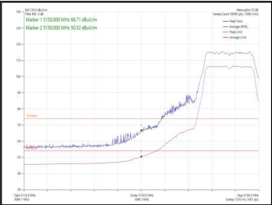
Figure 1 - 802.11a, Core 0 - 5180 MHz, Band Edge Frequency 5150 MHz
