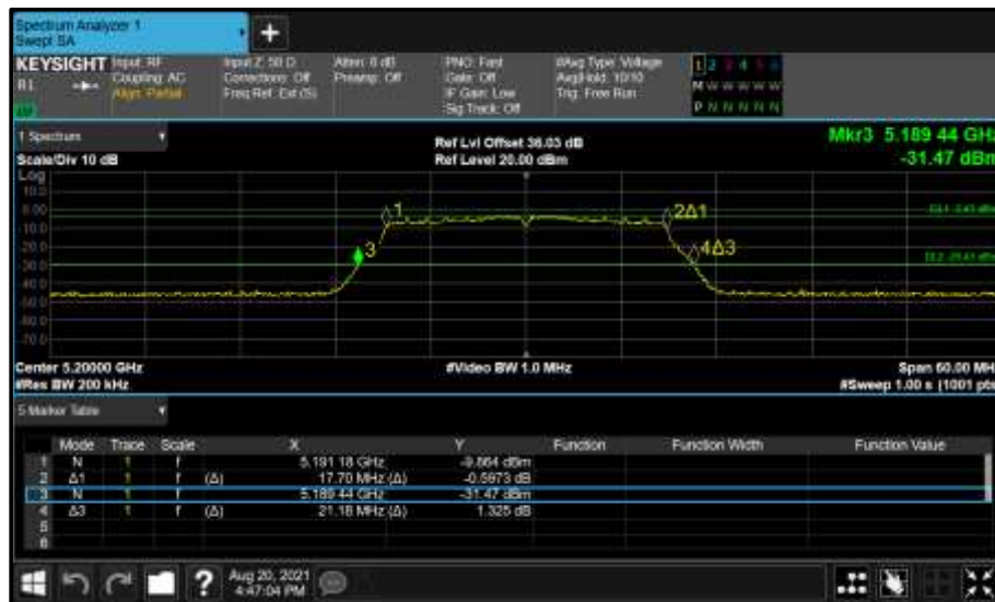
Figure 106 - Core 1 (B) 5200 MHz (CH40) 26 dB and 99% Bandwidth
