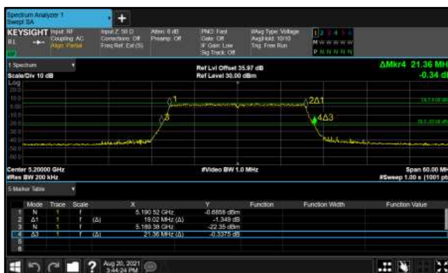
Figure 159 - Core 0 (A) 5200 MHz (CH40) 26 dB and 99% Bandwidth
