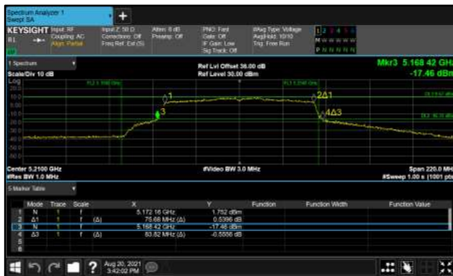
Figure 143 - Core 0 (A) 5210 MHz (CH42) 26 dB and 99% Bandwidth
