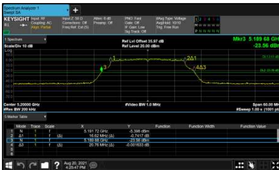
Figure 89 - Core 0 (A) 5200 MHz (CH40) 26 dB and 99% Bandwidth
