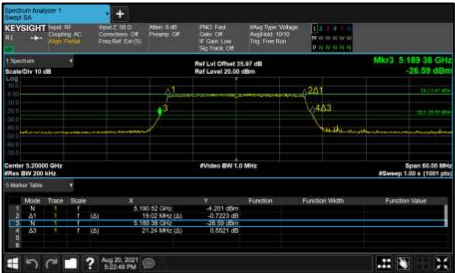
Figure 177 - Core 0 (A) 5200 MHz (CH40) 26 dB and 99% Bandwidth
