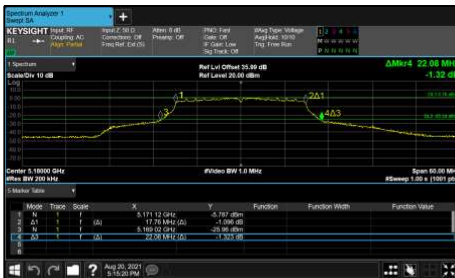
Figure 116 - Core 1 (B) 5180 MHz (CH36) 26 dB and 99% Bandwidth
