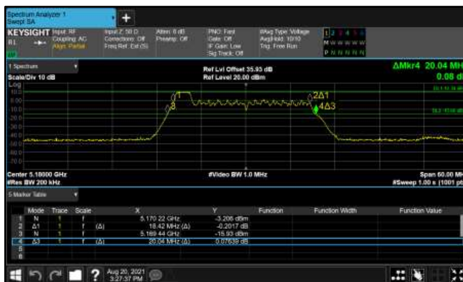
Figure 181 - Core 0 (A) 5180 MHz (CH36) 26 dB and 99% Bandwidth
