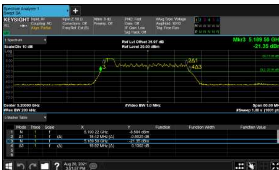
Figure 189 - Core 0 (A) 5200 MHz (CH40) 26 dB and 99% Bandwidth
