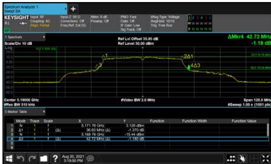
Figure 121 - Core 0 (A) 5190 MHz (CH38) 26 dB and 99% Bandwidth
