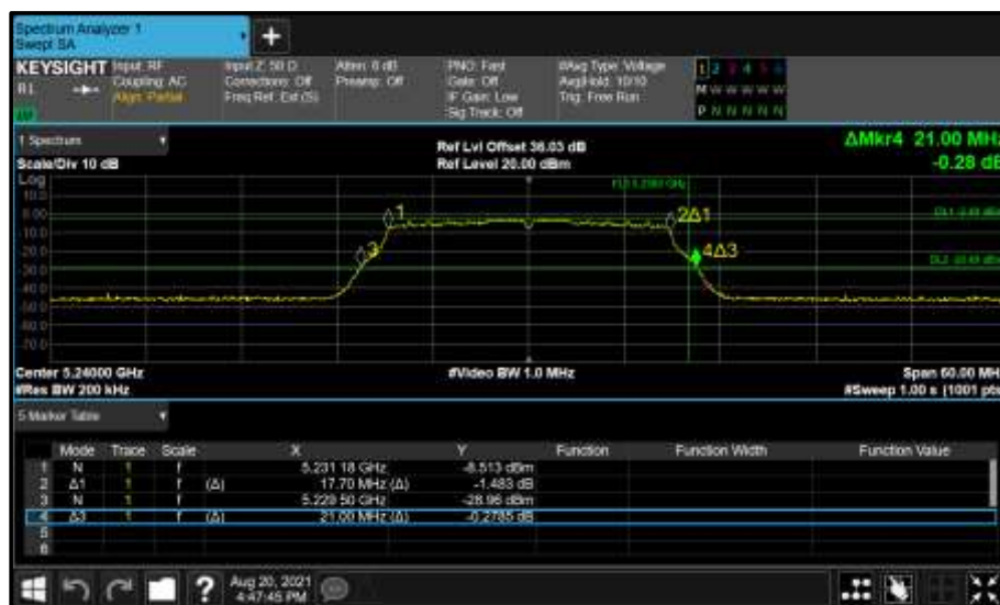
Figure 107 - Core 0 (A) 5240 MHz (CH48) 26 dB and 99% Bandwidth
