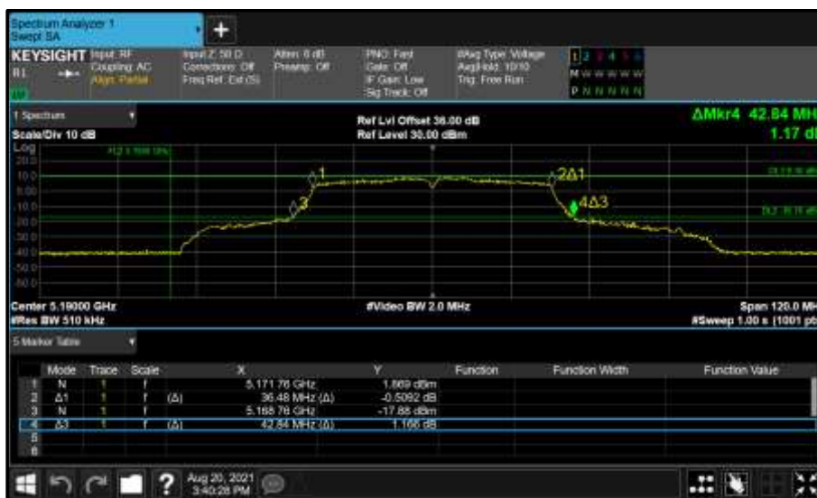
Figure 126 - Core 1 (B) 5190 MHz (CH38) 26 dB and 99% Bandwidth
