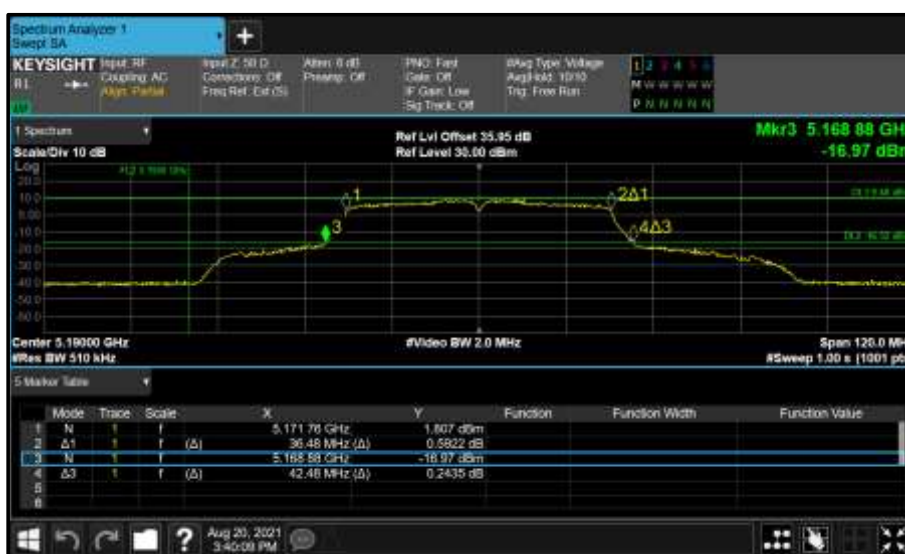
Figure 125 - Core 0 (A) 5190 MHz (CH38) 26 dB and 99% Bandwidth
