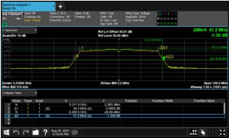
Figure 140 - Core 1 (B) 5230 MHz (CH46) 26 dB and 99% Bandwidth
