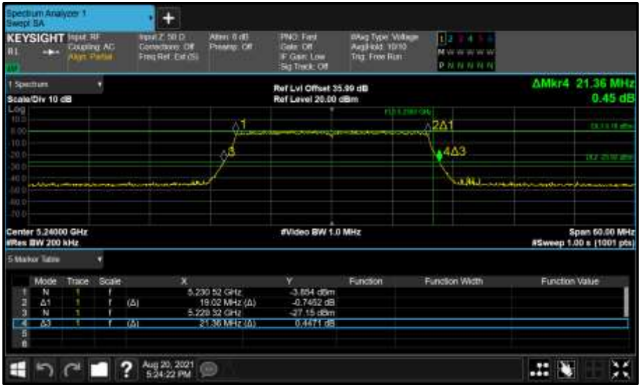
Figure 180 - Core 1 (B) 5240 MHz (CH48) 26 dB and 99% Bandwidth
