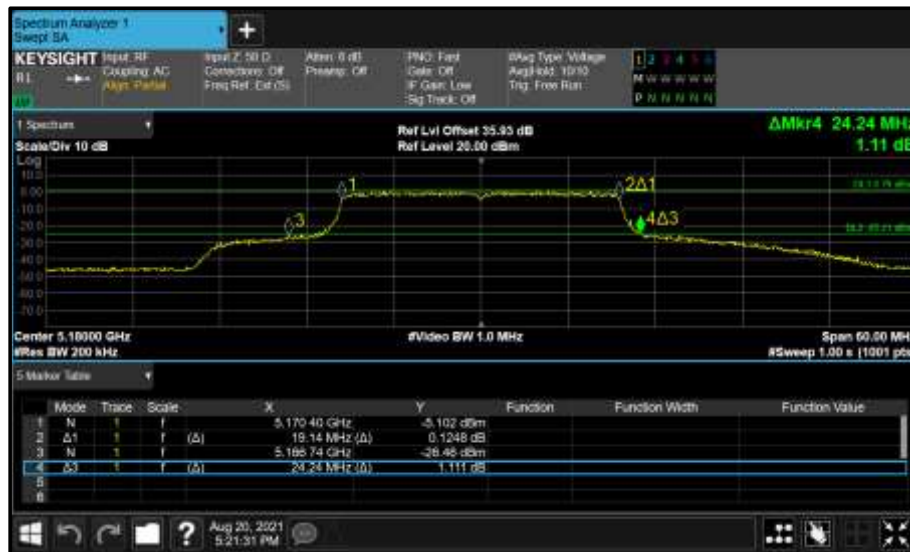
Figure 175 - Core 0 (A) 5180 MHz (CH36) 26 dB and 99% Bandwidth
