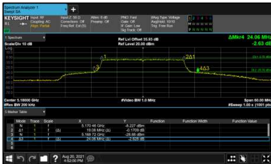
Figure 163 - Core 0 (A) 5180 MHz (CH36) 26 dB and 99% Bandwidth
