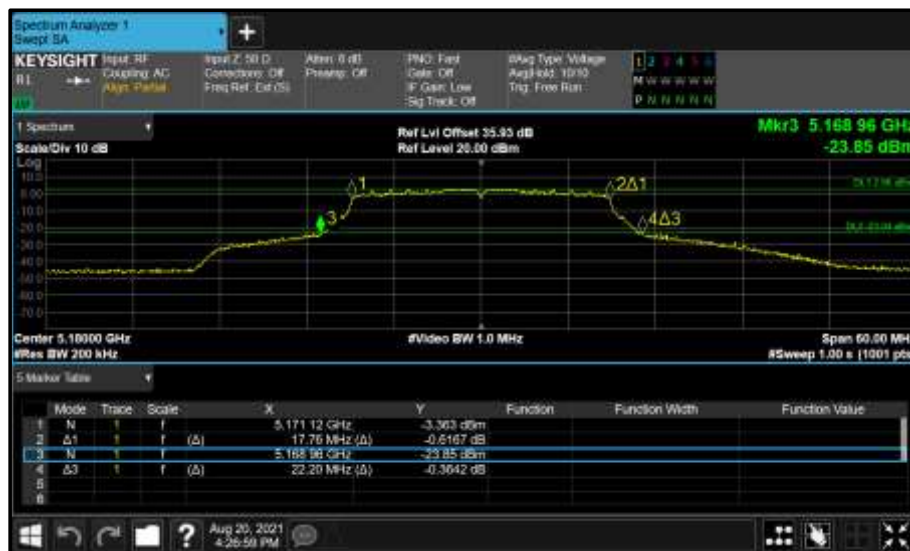
Figure 94 - Core 0 (A) 5180 MHz (CH36) 26 dB and 99% Bandwidth
