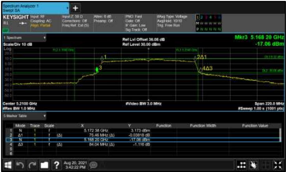
Figure 144 - Core 1 (B) 5210 MHz (CH42) 26 dB and 99% Bandwidth
