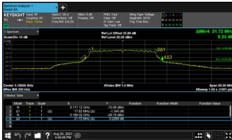
Figure 104 - Core 1 (B) 5180 MHz (CH36) 26 dB and 99% Bandwidth
