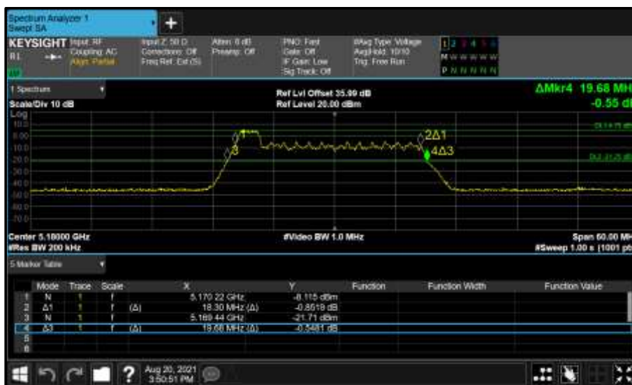
Figure 188 - Core 1 (B) 5180 MHz (CH36) 26 dB and 99% Bandwidth
