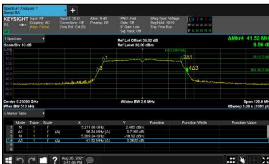
Figure 127 - Core 0 (A) 5230 MHz (CH46) 26 dB and 99% Bandwidth
