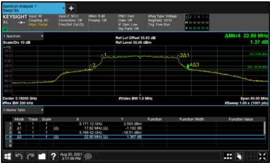
Figure 91 - Core 0 (A) 5180 MHz (CH36) 26 dB and 99% Bandwidth
