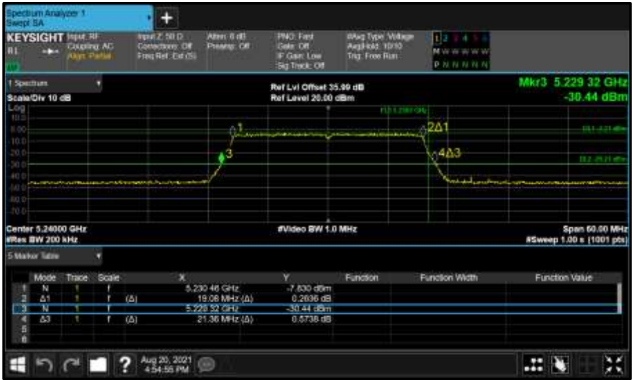
Figure 168 - Core 1 (B) 5240 MHz (CH48) 26 dB and 99% Bandwidth
