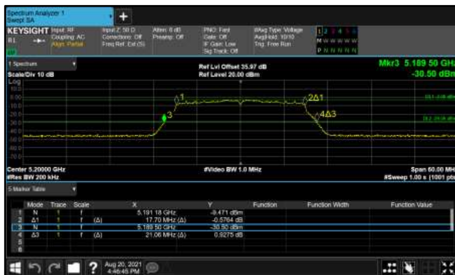
Figure 105 - Core 0 (A) 5200 MHz (CH40) 26 dB and 99% Bandwidth
