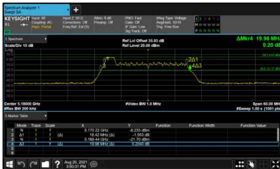
Figure 187 - Core 0 (A) 5180 MHz (CH36) 26 dB and 99% Bandwidth
