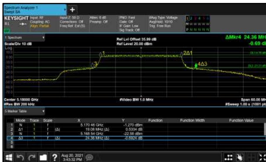
Figure 158 - Core 1 (B) 5180 MHz (CH36) 26 dB and 99% Bandwidth
