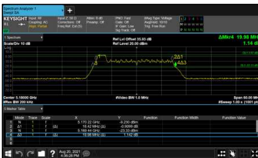
Figure 184 - Core 0 (A) 5180 MHz (CH36) 26 dB and 99% Bandwidth
