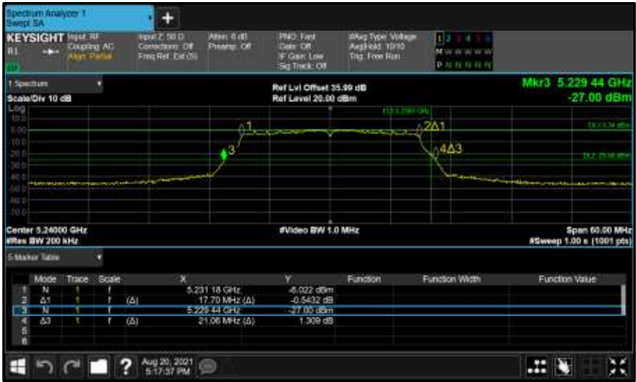
Figure 120 - Core 1 (B) 5240 MHz (CH48) 26 dB and 99% Bandwidth
