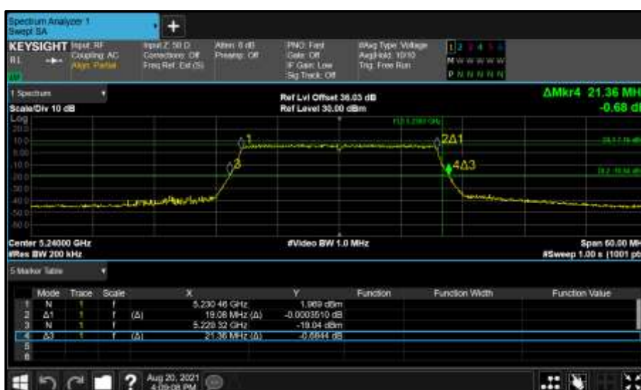
Figure 173 - Core 0 (A) 5240 MHz (CH48) 26 dB and 99% Bandwidth
