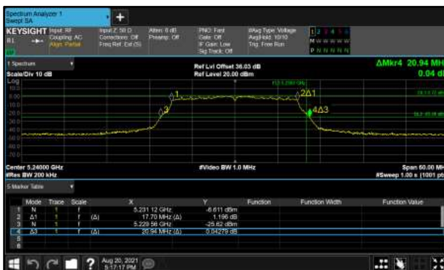
Figure 119 - Core 0 (A) 5240 MHz (CH48) 26 dB and 99% Bandwidth
