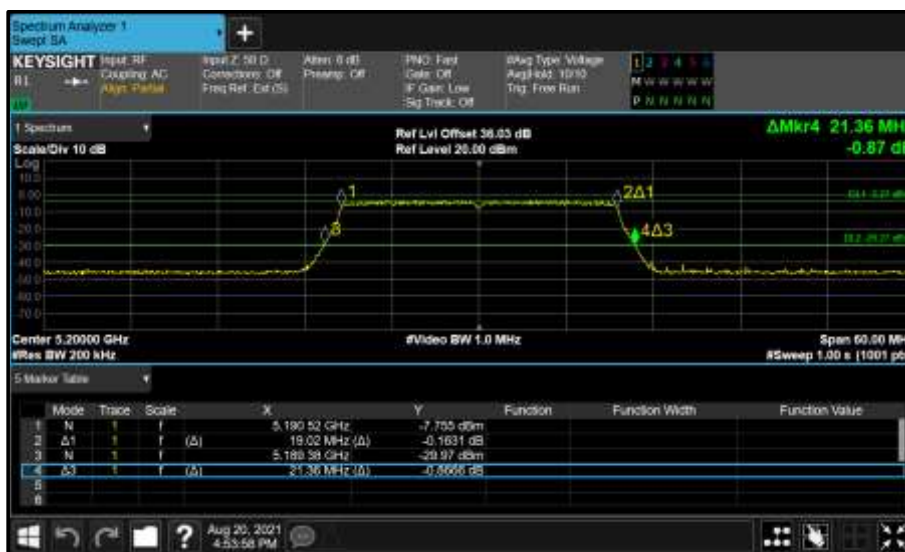
Figure 166 - Core 1 (B) 5200 MHz (CH40) 26 dB and 99% Bandwidth
