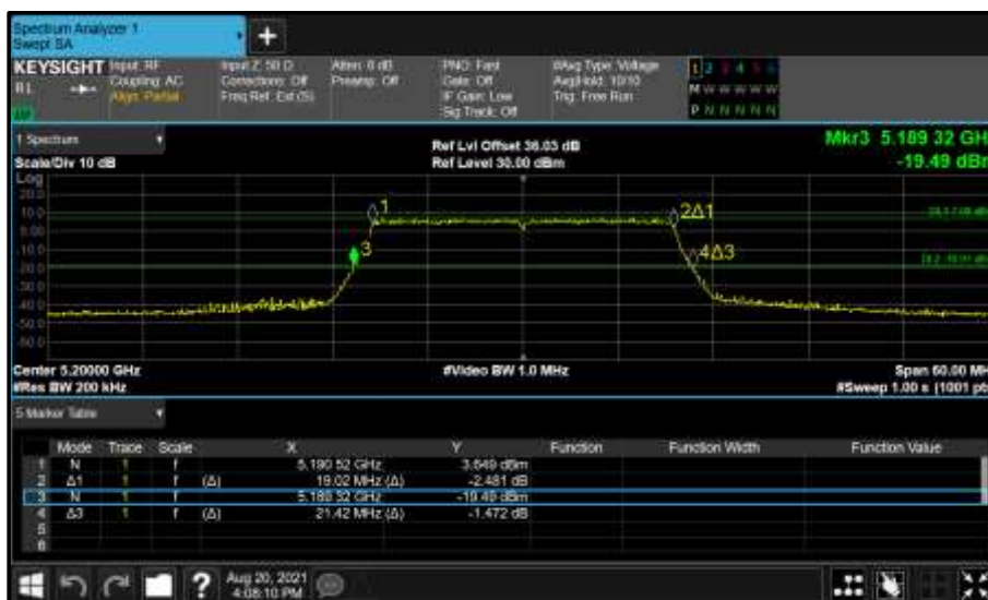
Figure 172 - Core 1 (B) 5200 MHz (CH40) 26 dB and 99% Bandwidth
