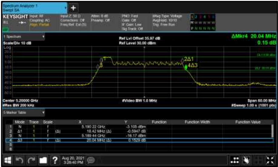
Figure 182 - Core 0 (A) 5200 MHz (CH40) 26 dB and 99% Bandwidth
