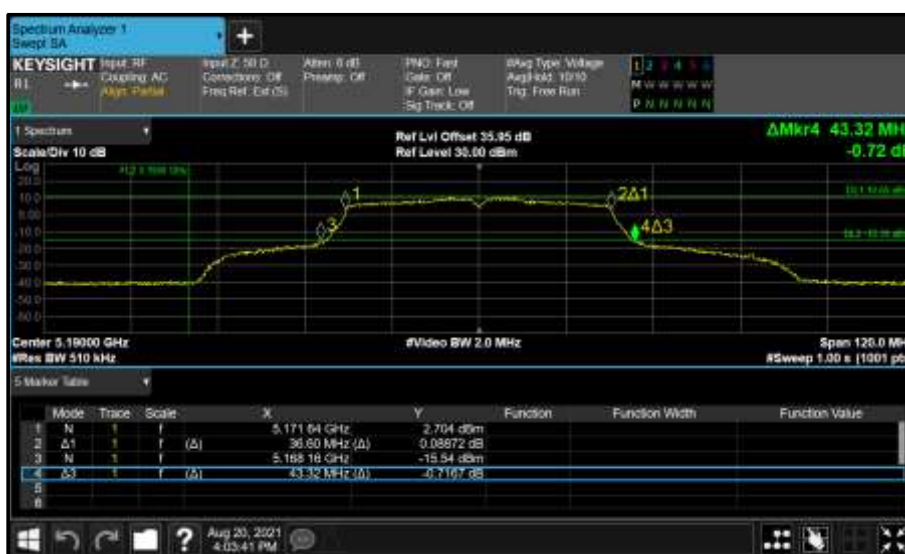
Figure 133 - Core 0 (A) 5190 MHz (CH38) 26 dB and 99% Bandwidth
