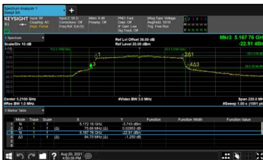
Figure 145 - Core 0 (A) 5210 MHz (CH42) 26 dB and 99% Bandwidth
