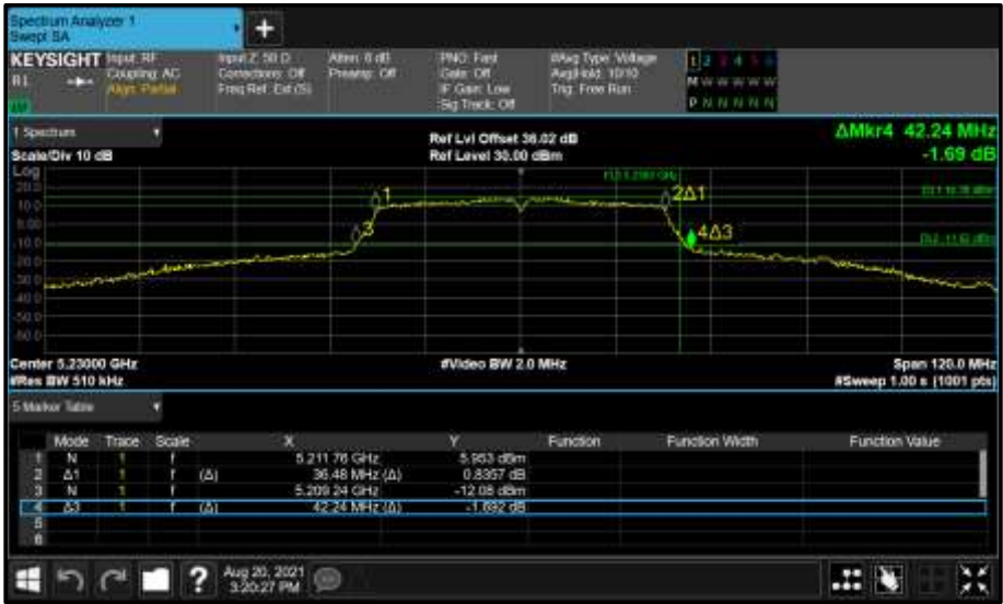
Figure 122 - Core 0 (A) 5230 MHz (CH46) 26 dB and 99% Bandwidth
