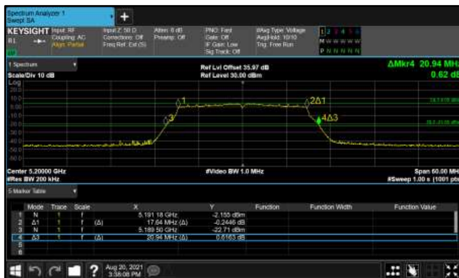
Figure 99 - Core 0 (A) 5200 MHz (CH40) 26 dB and 99% Bandwidth
