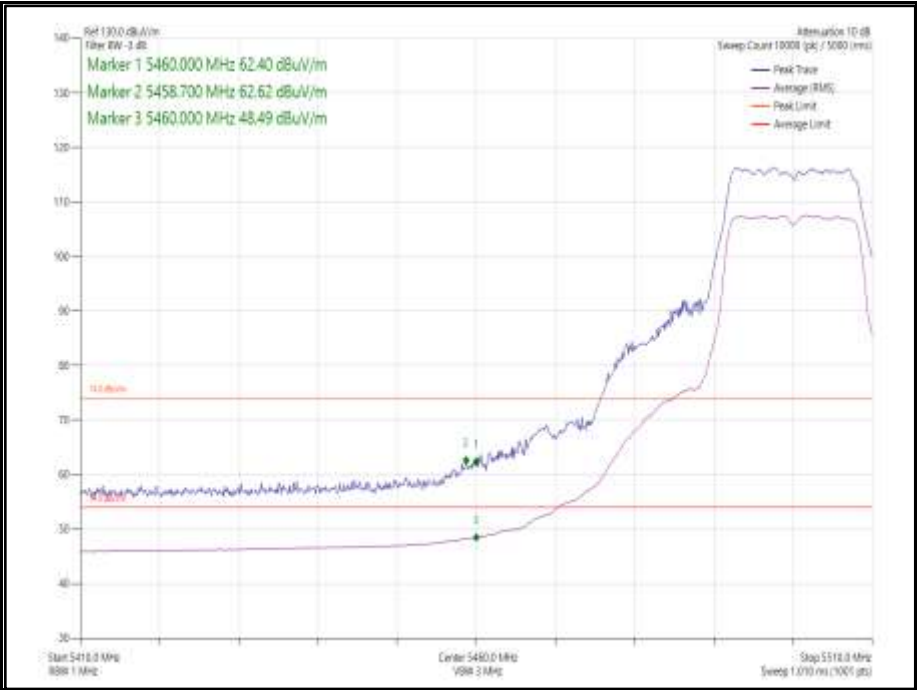
Figure 9 - 802.11a, Core 0 - 5500 MHz, Band Edge Frequency 5460 MHz
