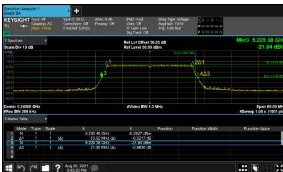
Figure 161 - Core 0 (A) 5240 MHz (CH48) 26 dB and 99% Bandwidth
