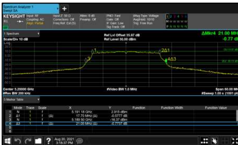
Figure 92 - Core 0 (A) 5200 MHz (CH40) 26 dB and 99% Bandwidth
