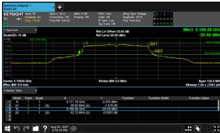
Figure 137 - Core 0 (A) 5190 MHz (CH38) 26 dB and 99% Bandwidth
