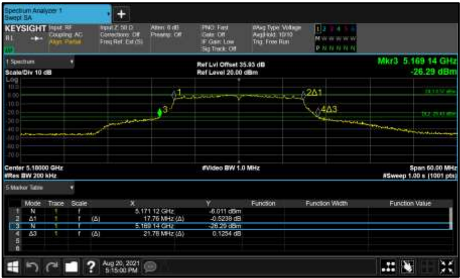
Figure 115 - Core 0 (A) 5180 MHz (CH36) 26 dB and 99% Bandwidth
