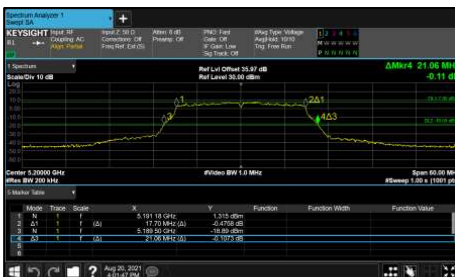
Figure 111 - Core 0 (A) 5200 MHz (CH40) 26 dB and 99% Bandwidth
