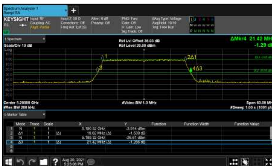
Figure 178 - Core 1 (B) 5200 MHz (CH40) 26 dB and 99% Bandwidth
