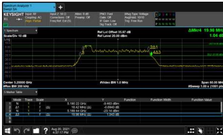
Figure 185 - Core 0 (A) 5200 MHz (CH40) 26 dB and 99% Bandwidth
