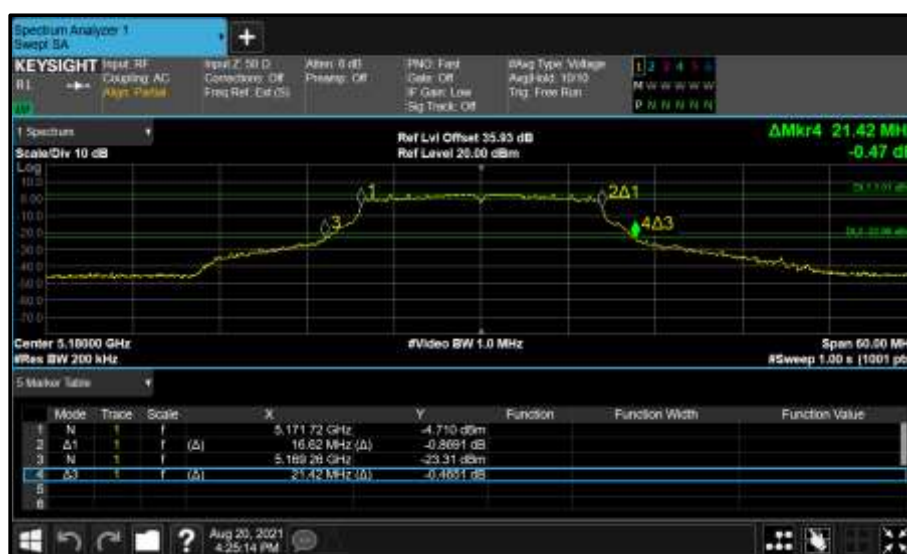
Figure 88 - Core 0 (A) 5180 MHz (CH36) 26 dB and 99% Bandwidth
