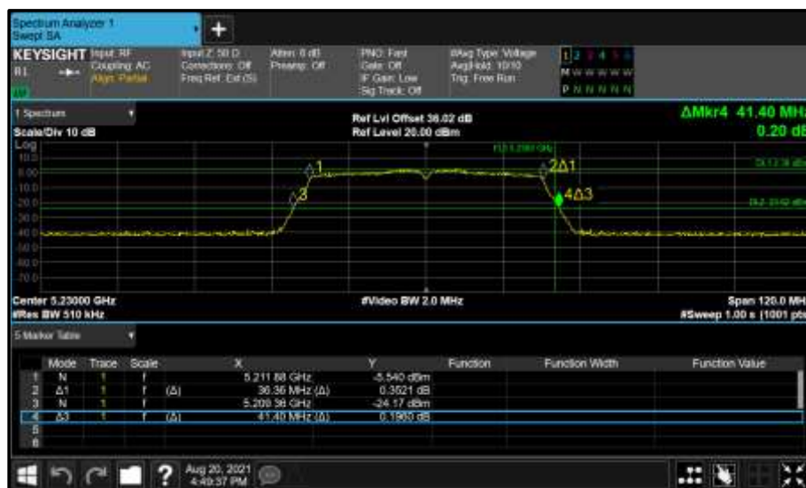
Figure 131 - Core 0 (A) 5230 MHz (CH46) 26 dB and 99% Bandwidth
