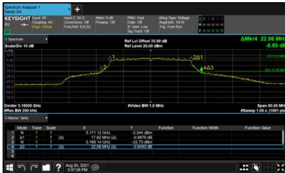
Figure 98 - Core 1 (B) 5180 MHz (CH36) 26 dB and 99% Bandwidth
