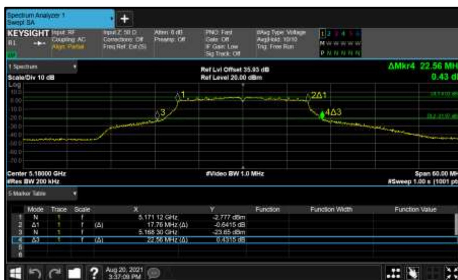
Figure 97 - Core 0 (A) 5180 MHz (CH36) 26 dB and 99% Bandwidth
