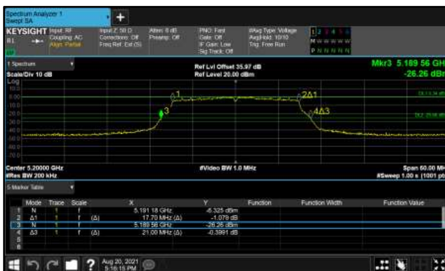
Figure 117 - Core 0 (A) 5200 MHz (CH40) 26 dB and 99% Bandwidth
