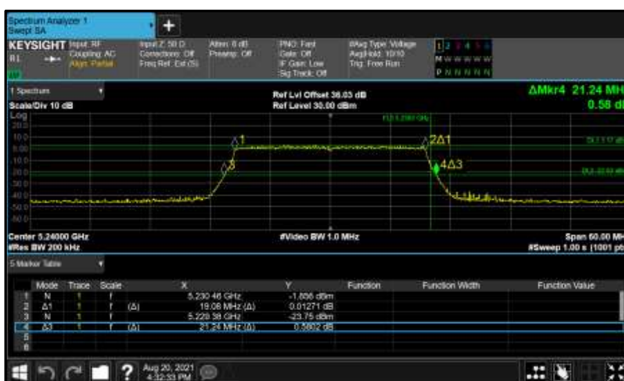
Figure 156 - Core 0 (A) 5240 MHz (CH48) 26 dB and 99% Bandwidth
