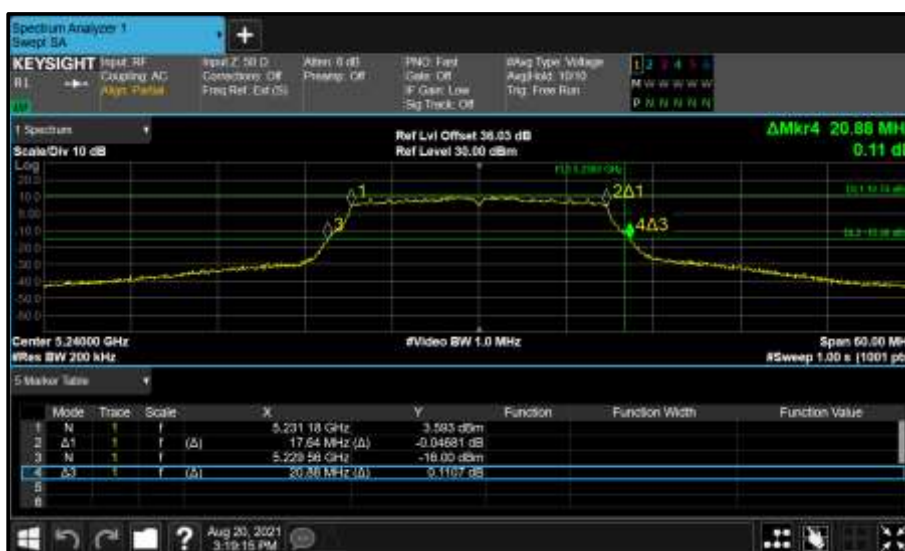
Figure 93 - Core 0 (A) 5240 MHz (CH48) 26 dB and 99% Bandwidth
