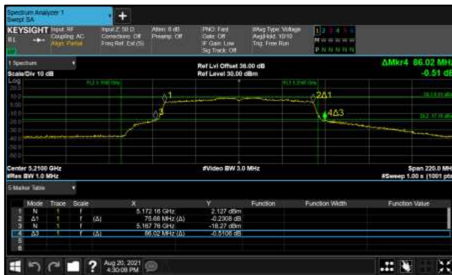
Figure 142 - Core 0 (A) 5210 MHz (CH42) 26 dB and 99% Bandwidth
