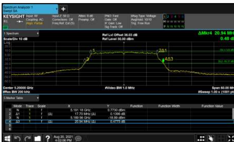
Figure 112 - Core 1 (B) 5200 MHz (CH40) 26 dB and 99% Bandwidth
