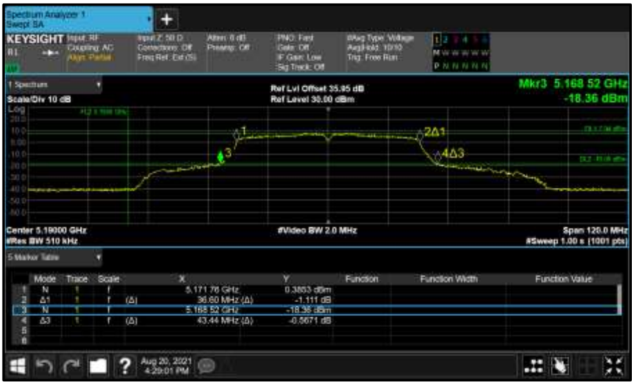
Figure 123 - Core 0 (A) 5190 MHz (CH38) 26 dB and 99% Bandwidth
