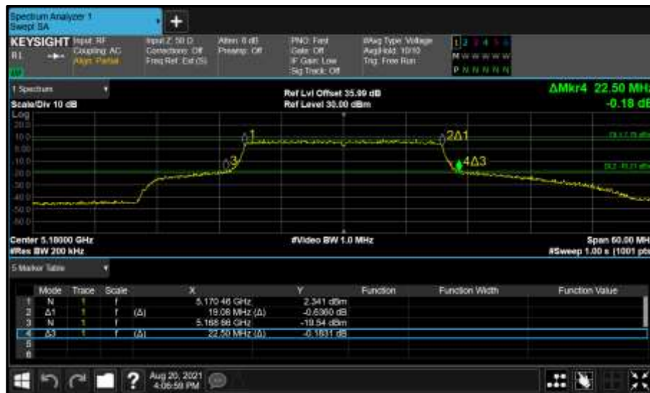
Figure 170 - Core 1 (B) 5180 MHz (CH36) 26 dB and 99% Bandwidth
