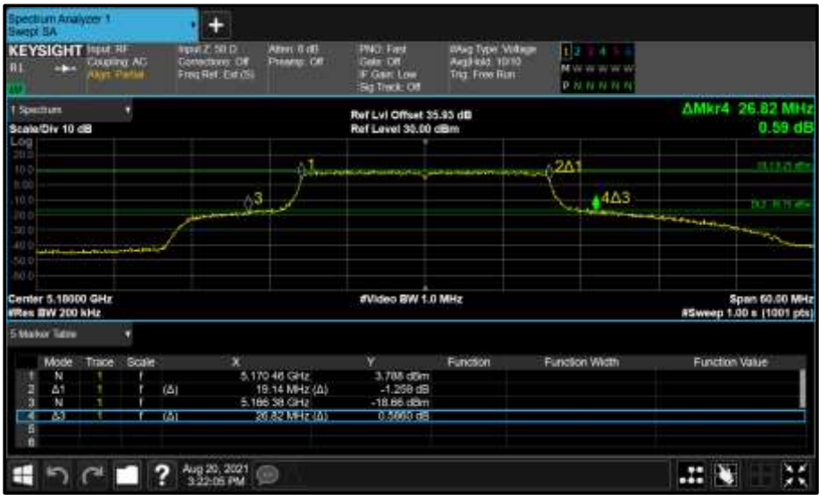
Figure 151 - Core 0 (A) 5180 MHz (CH36) 26 dB and 99% Bandwidth
