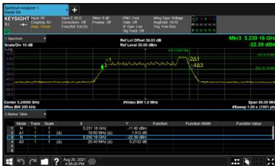
Figure 186 - Core 0 (A) 5240 MHz (CH48) 26 dB and 99% Bandwidth
