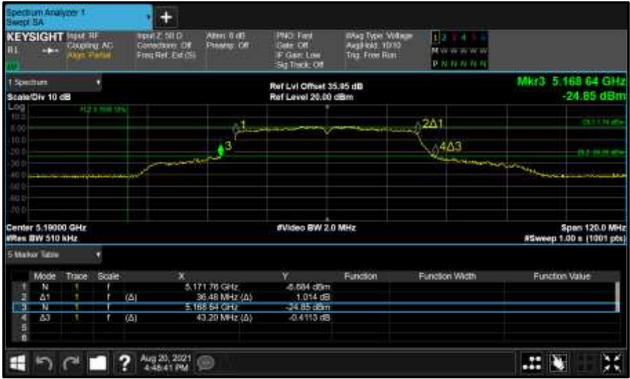
Figure 129 - Core 0 (A) 5190 MHz (CH38) 26 dB and 99% Bandwidth
