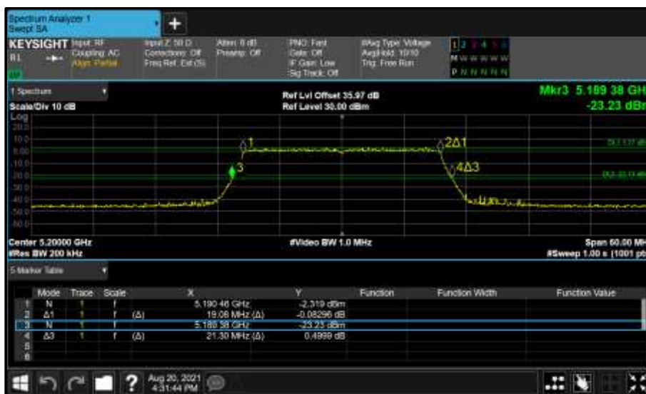
Figure 155 - Core 0 (A) 5200 MHz (CH40) 26 dB and 99% Bandwidth
