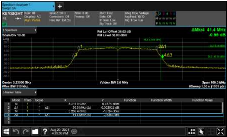
Figure 124 - Core 0 (A) 5230 MHz (CH46) 26 dB and 99% Bandwidth
