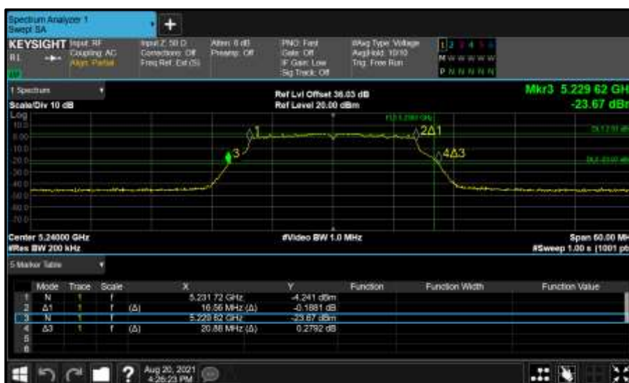
Figure 90 - Core 0 (A) 5240 MHz (CH48) 26 dB and 99% Bandwidth
