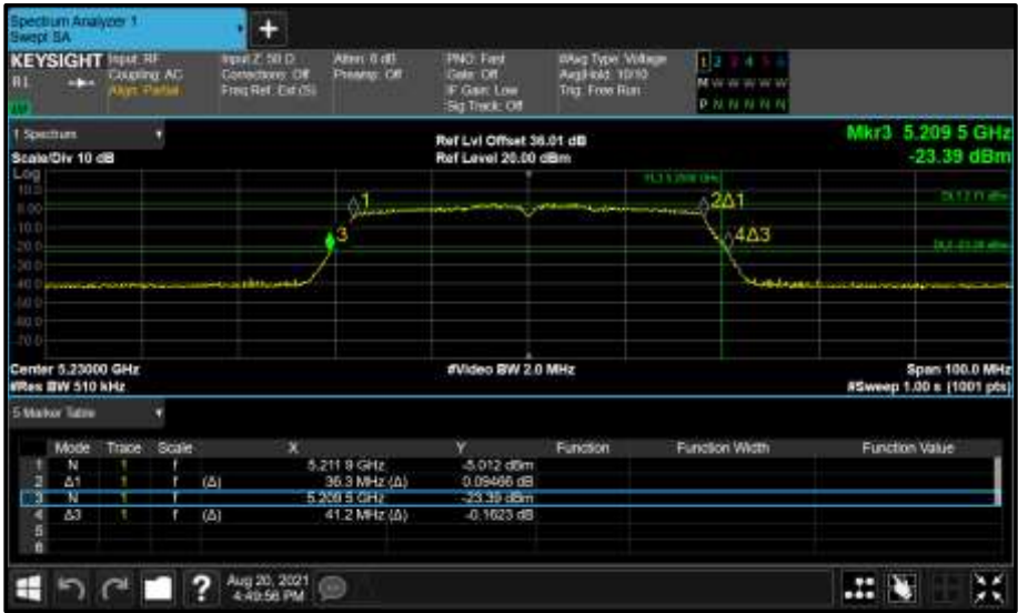
Figure 132 - Core 1 (B) 5230 MHz (CH46) 26 dB and 99% Bandwidth
