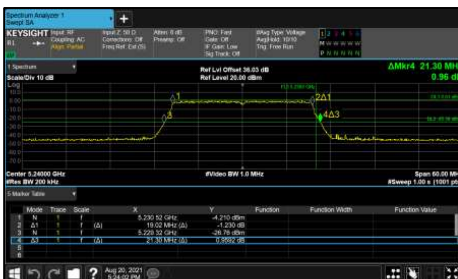
Figure 179 - Core 0 (A) 5240 MHz (CH48) 26 dB and 99% Bandwidth
