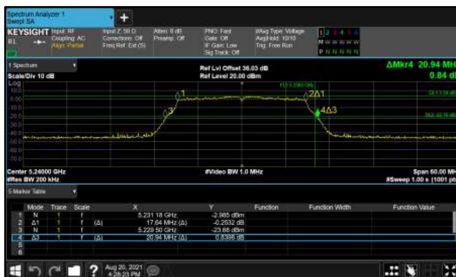
Figure 96 - Core 0 (A) 5240 MHz (CH48) 26 dB and 99% Bandwidth
