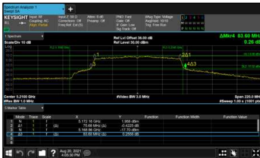
Figure 147 - Core 0 (A) 5210 MHz (CH42) 26 dB and 99% Bandwidth
