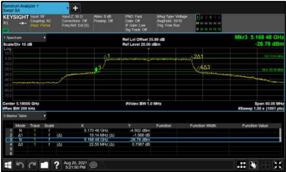
Figure 176 - Core 1 (B) 5180 MHz (CH36) 26 dB and 99% Bandwidth
