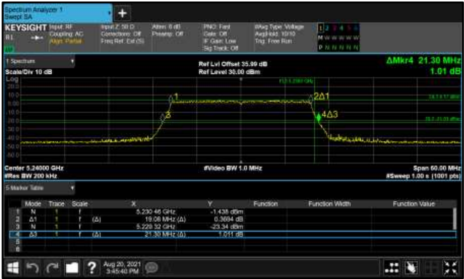
Figure 162 - Core 1 (B) 5240 MHz (CH48) 26 dB and 99% Bandwidth
