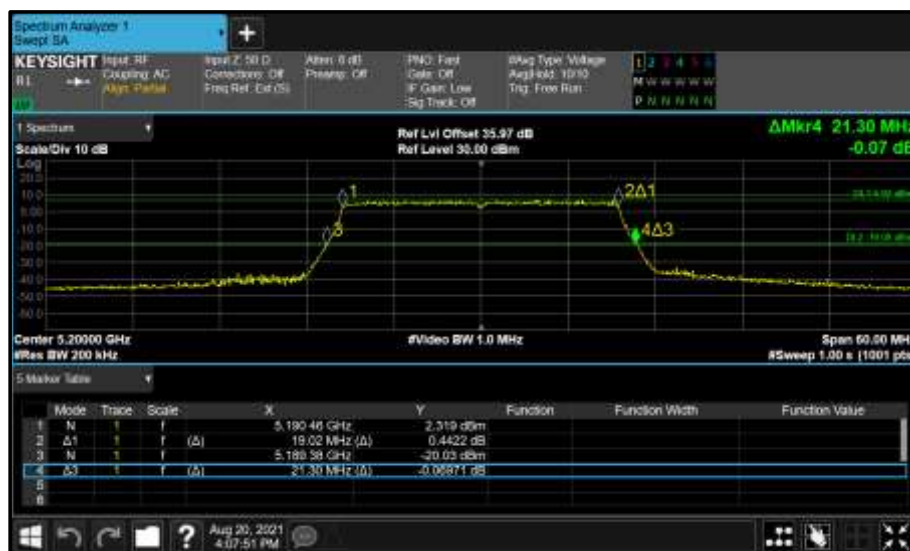
Figure 171 - Core 0 (A) 5200 MHz (CH40) 26 dB and 99% Bandwidth
