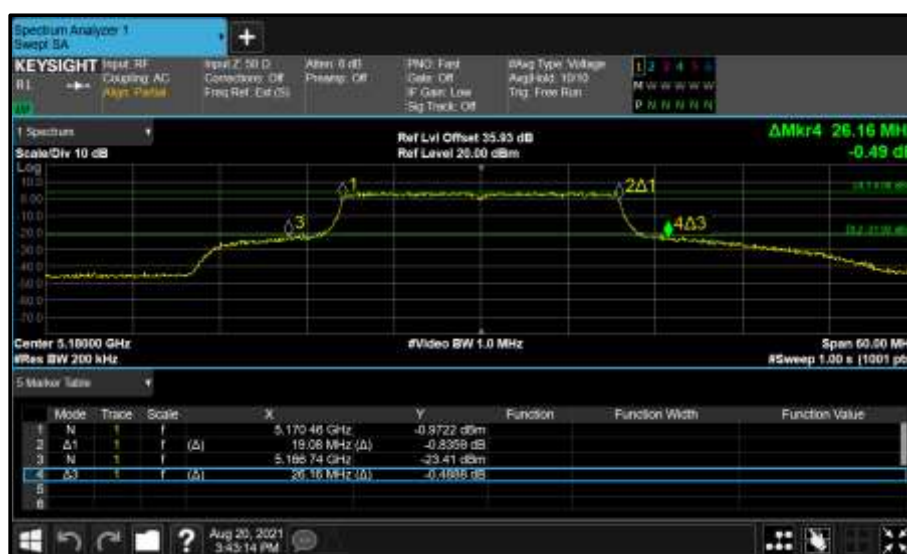
Figure 157 - Core 0 (A) 5180 MHz (CH36) 26 dB and 99% Bandwidth
