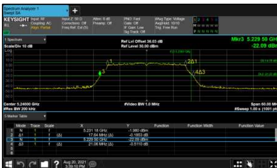
Figure 101 - Core 0 (A) 5240 MHz (CH48) 26 dB and 99% Bandwidth
