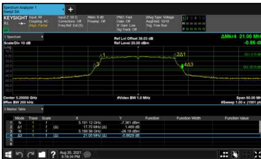
Figure 118 - Core 1 (B) 5200 MHz (CH40) 26 dB and 99% Bandwidth
