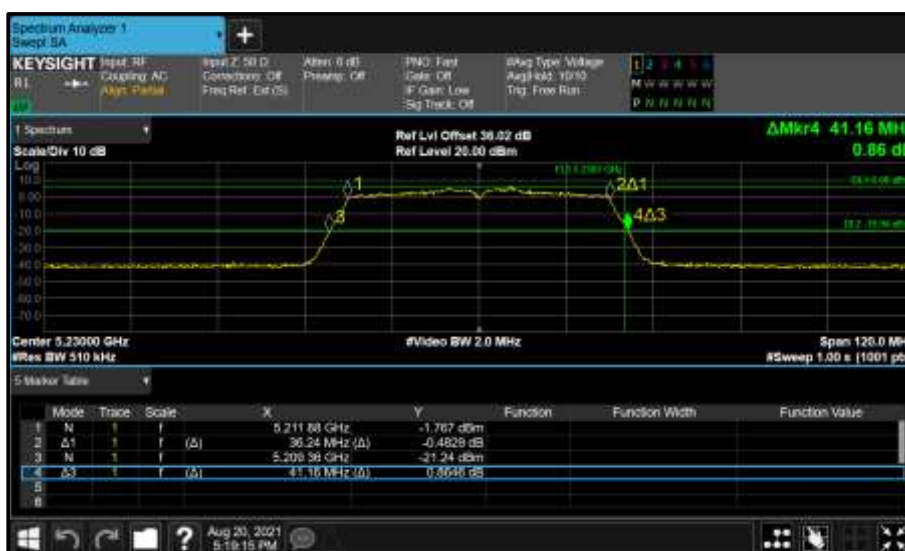
Figure 139 - Core 0 (A) 5230 MHz (CH46) 26 dB and 99% Bandwidth
