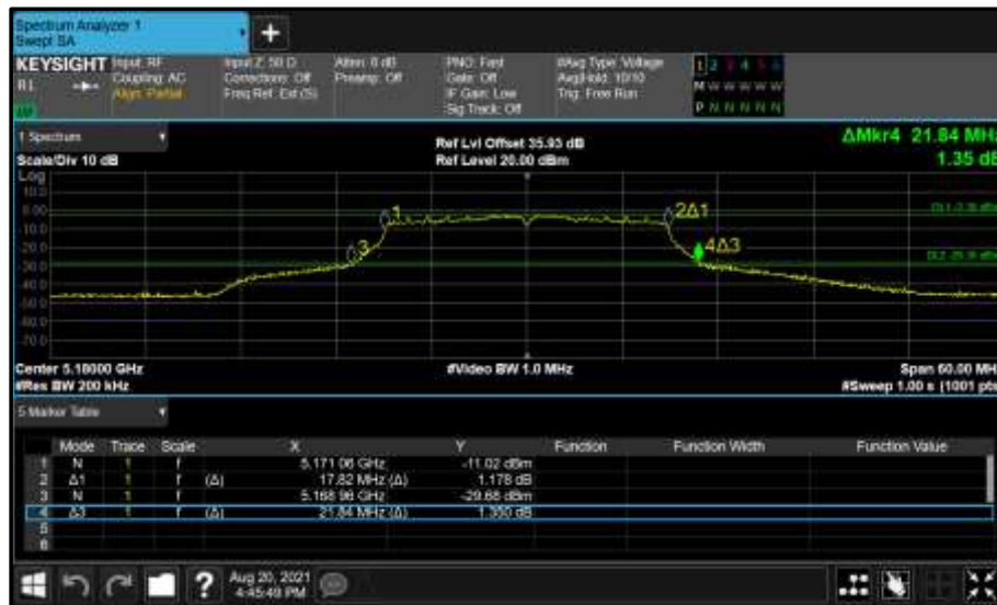
Figure 103 - Core 0 (A) 5180 MHz (CH36) 26 dB and 99% Bandwidth
