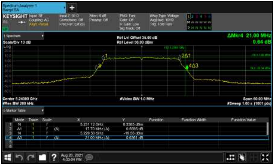
Figure 114 - Core 1 (B) 5240 MHz (CH48) 26 dB and 99% Bandwidth
