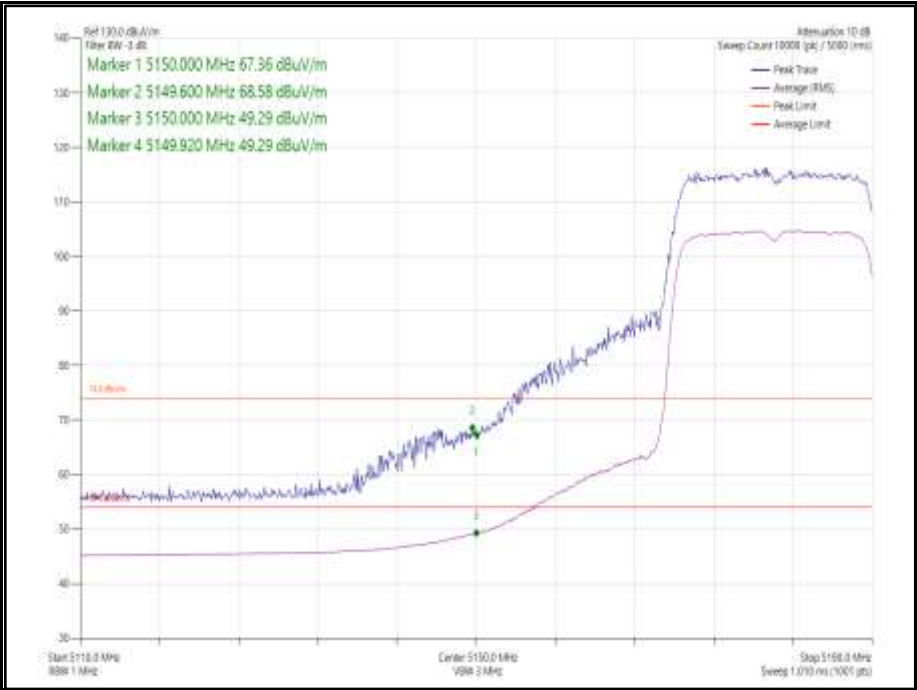
Figure 3 - 802.11ax HE20, Core 0, SU - 5180 MHz, Band Edge Frequency 5150 MHz
