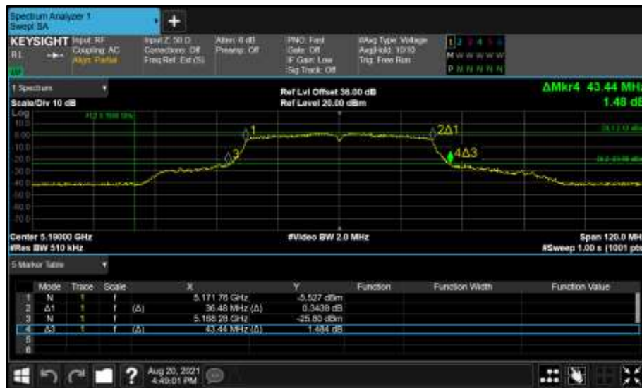
Figure 130 - Core 1 (B) 5190 MHz (CH38) 26 dB and 99% Bandwidth
