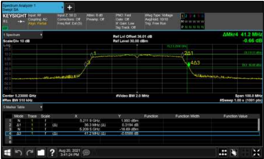
Figure 128 - Core 1 (B) 5230 MHz (CH46) 26 dB and 99% Bandwidth
