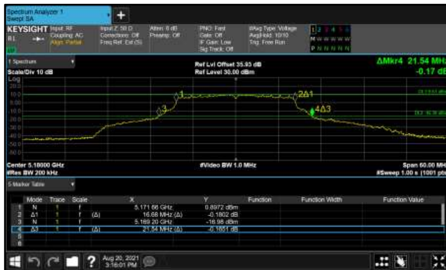
Figure 85 - Core 0 (A) 5180 MHz (CH36) 26 dB and 99% Bandwidth
