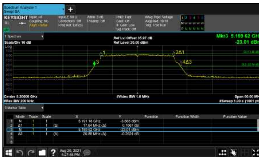
Figure 95 - Core 0 (A) 5200 MHz (CH40) 26 dB and 99% Bandwidth
