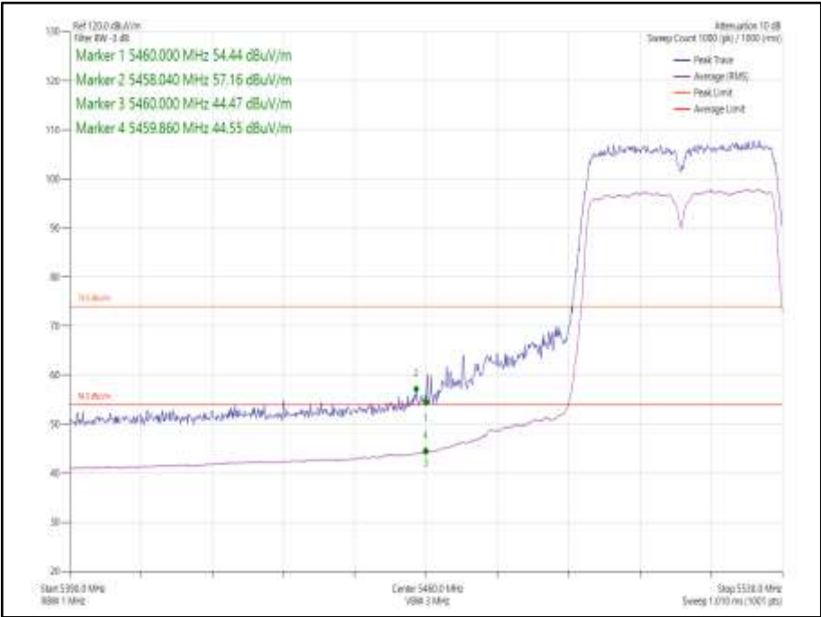
Figure 1053 - 802.11n HT40 CDD, Cores 0-1 - 5510 MHz Band Edge Frequency 5460 MHz
