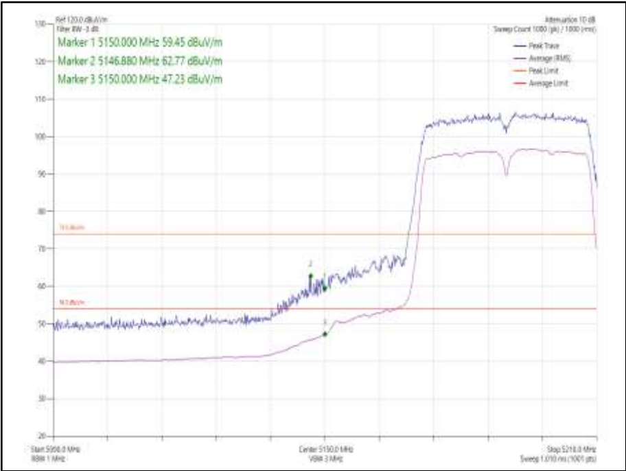
Figure 1041 - 802.11n HT40 CDD Cores 0-1 - 5190 MHz Band Edge Frequency 5150 MHz
