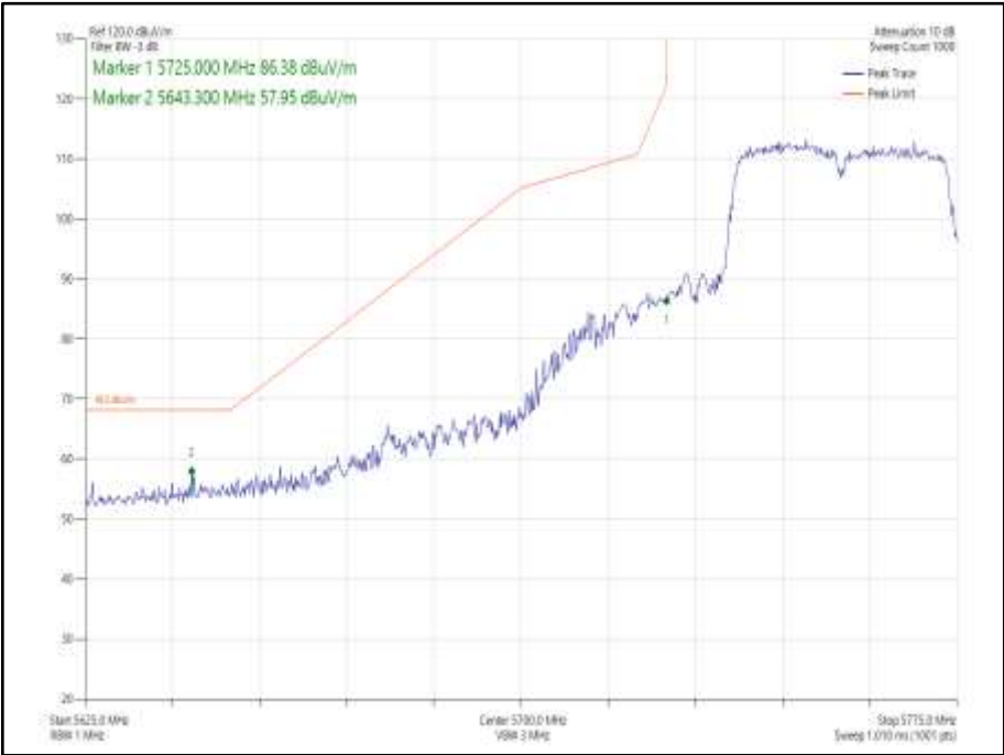
Figure 954 - 802.11n HT40 CDD, Cores 0-1 - 5755 MHz Band Edge Frequency 5725 MHz
