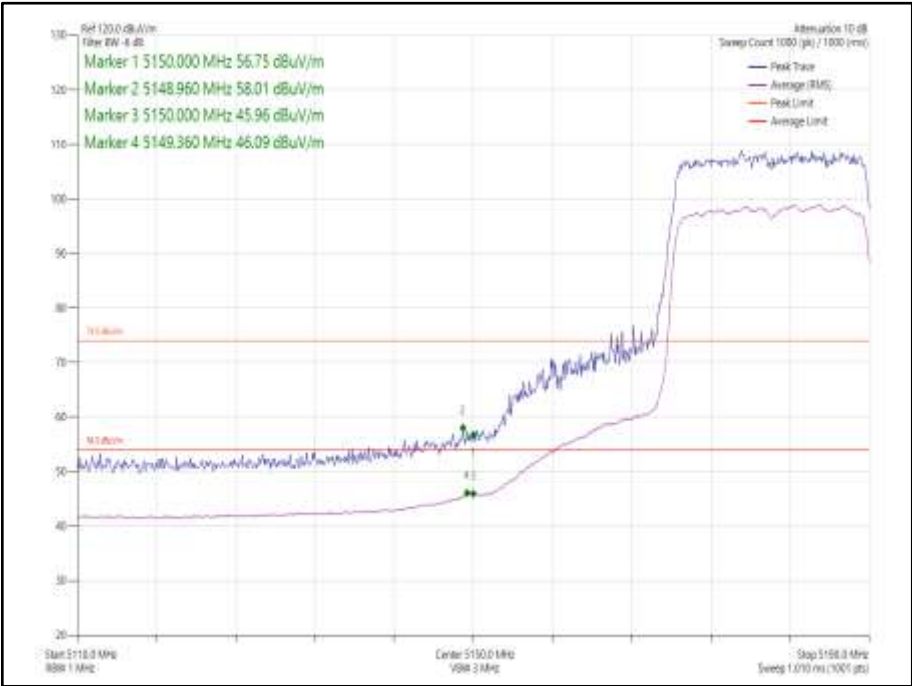
Figure 1016 - 802.11ax HE20 CDD, Cores 0-1 SU - 5180 MHz Band Edge Frequency 5150 MHz
