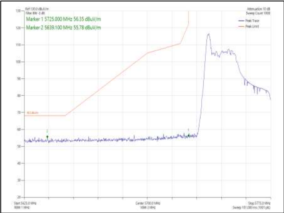
Figure 939 - 802.11ax HE40, Core 0, 26-0 - 5755 MHz Band Edge Frequency 5725 MHz
