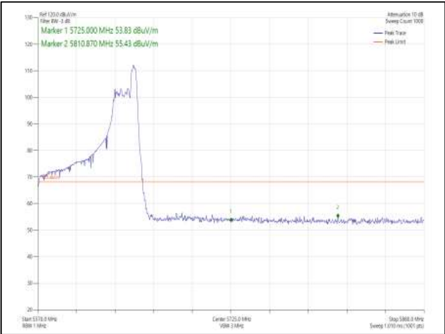
Figure 987 - 802.11ax HE80 CDD, Cores 0-1, 52-52- 5610 MHz Band Edge Frequency 5725 MHz
