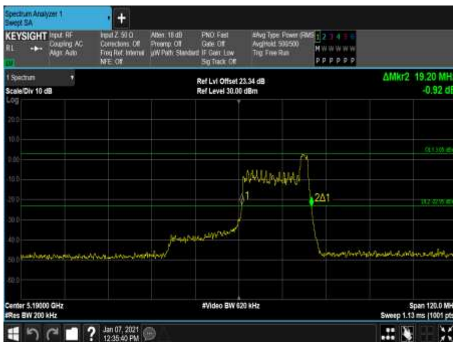
Figure 237 - 5190 MHz - 26 dB Emission Bandwidth
