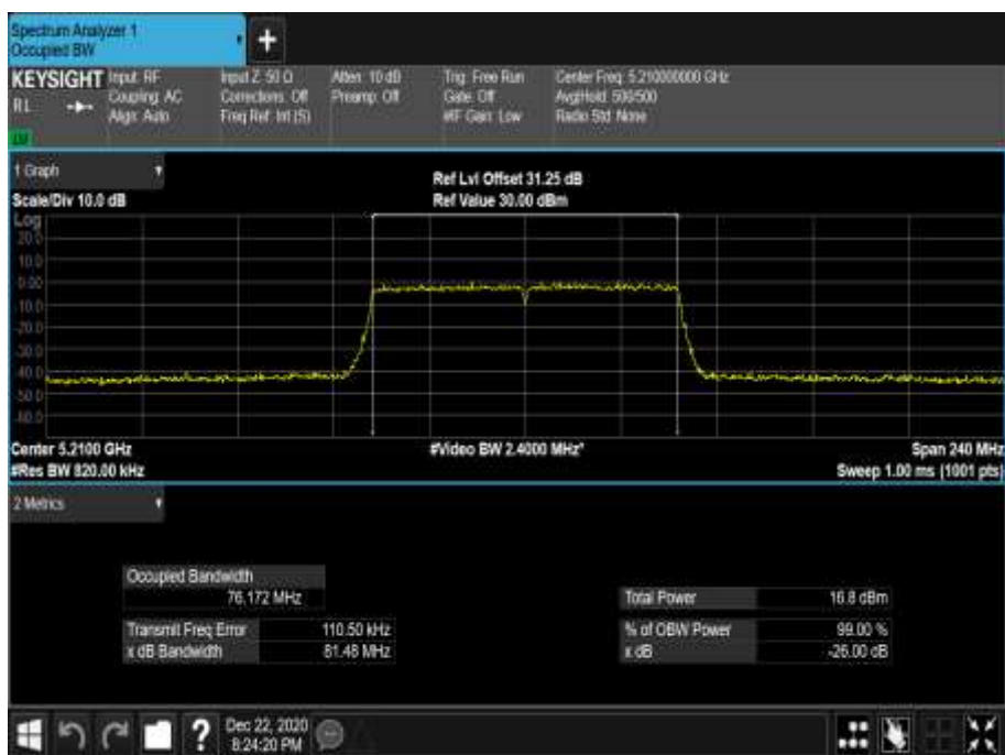
Figure 294 - 5210 MHz - 99% Occupied Bandwidth
