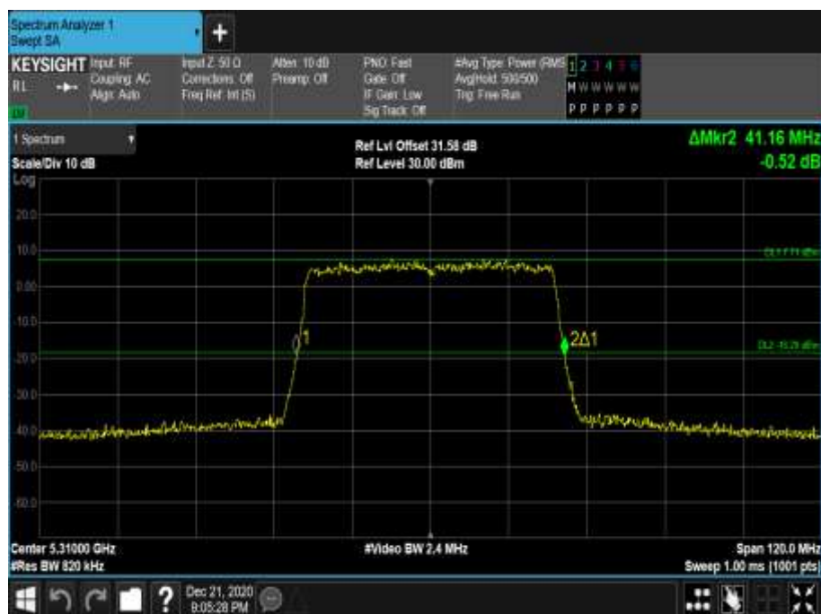
Figure 407 - 5310 MHz - 26 dB Emission Bandwidth
