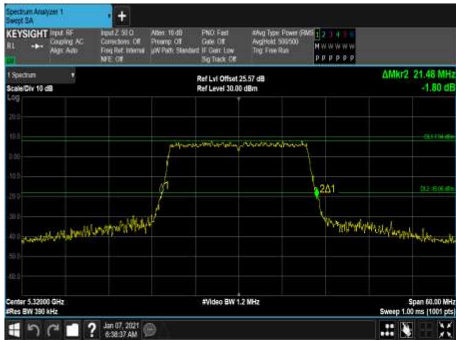
Figure 387 - 5320 MHz - 26 dB Emission Bandwidth
