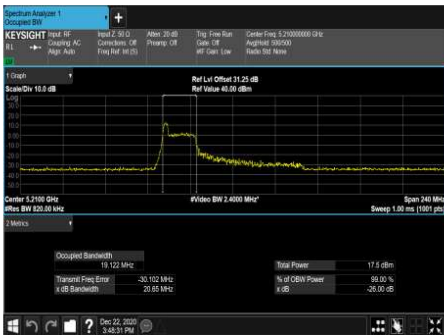
Figure 310 - 5210 MHz - 99% Occupied Bandwidth
