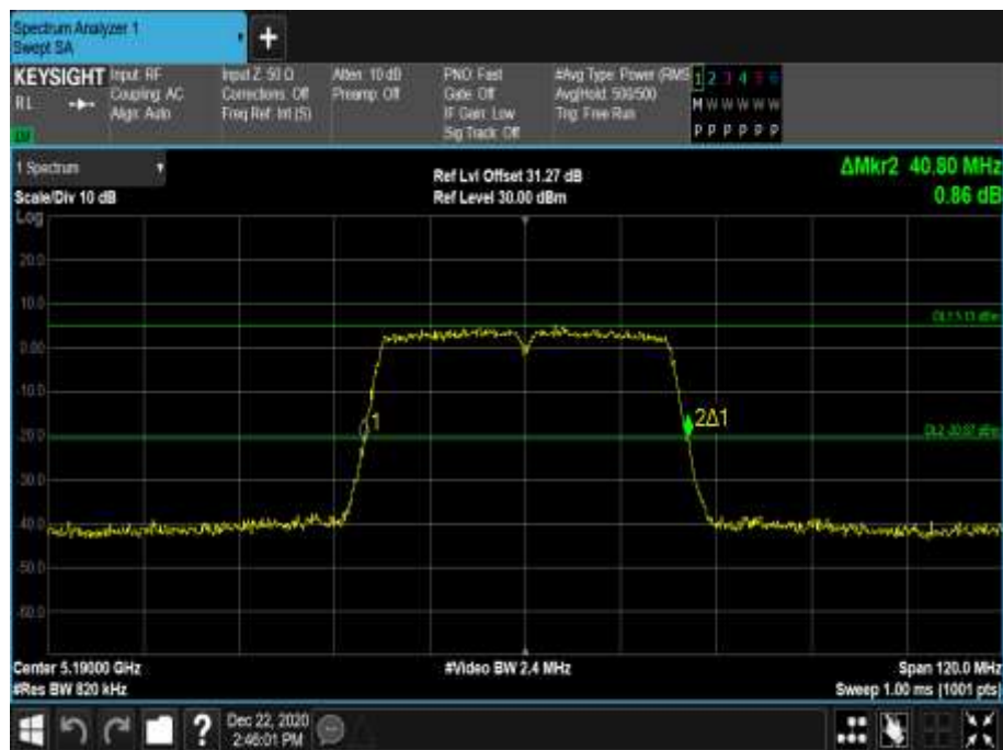
Figure 185 - 5190 MHz - 26 dB Emission Bandwidth
