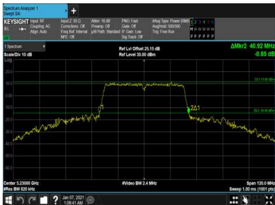
Figure 187 - 5230 MHz - 26 dB Emission Bandwidth
