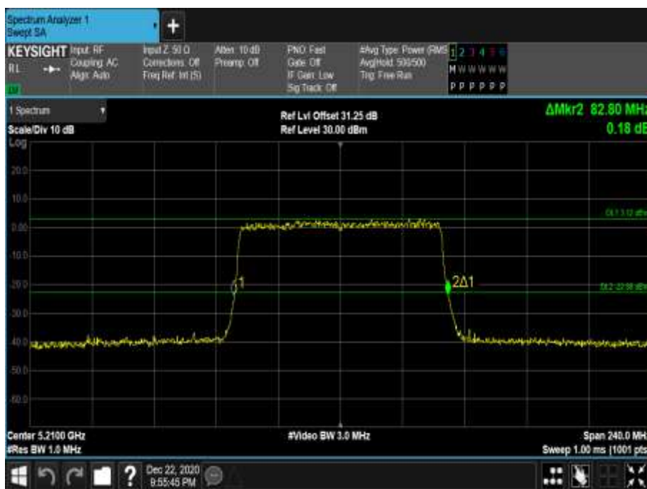
Figure 317 - 5210 MHz - 26 dB Emission Bandwidth
