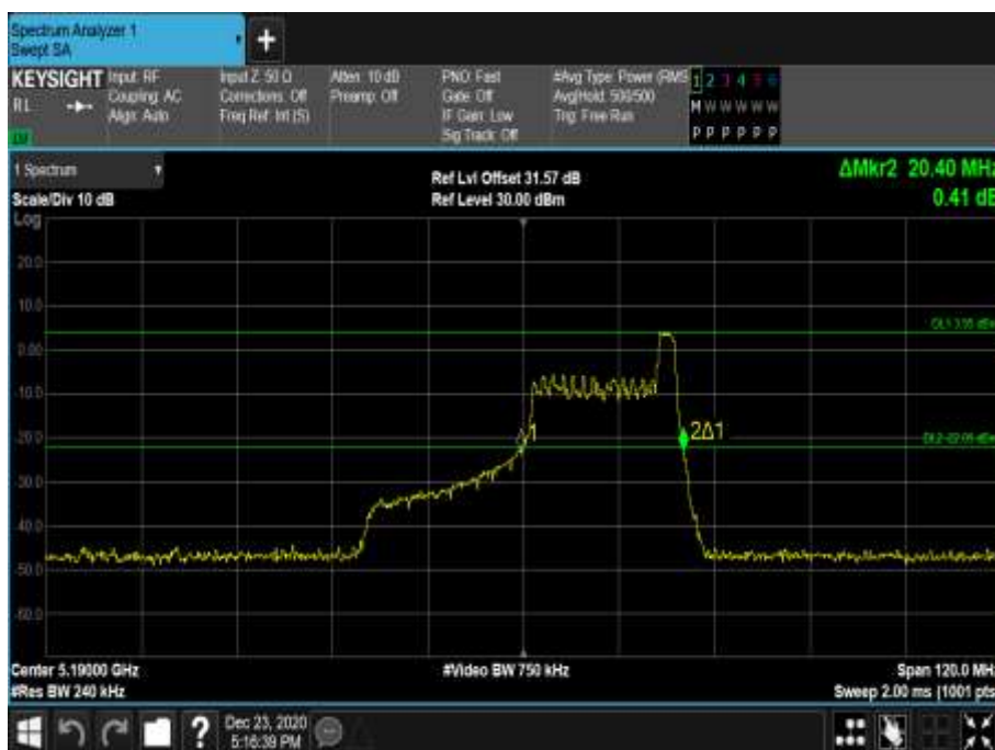
Figure 257 - 5190 MHz - 26 dB Emission Bandwidth
