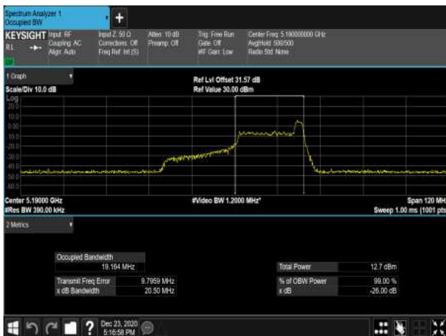
Figure 258 - 5190 MHz - 99% Occupied Bandwidth
