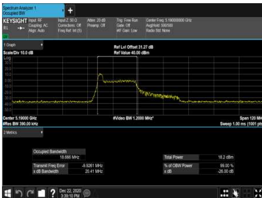
Figure 226 - 5190 MHz - 99% Occupied Bandwidth
