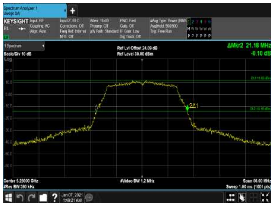
Figure 343 - 5280 MHz - 26 dB Emission Bandwidth
