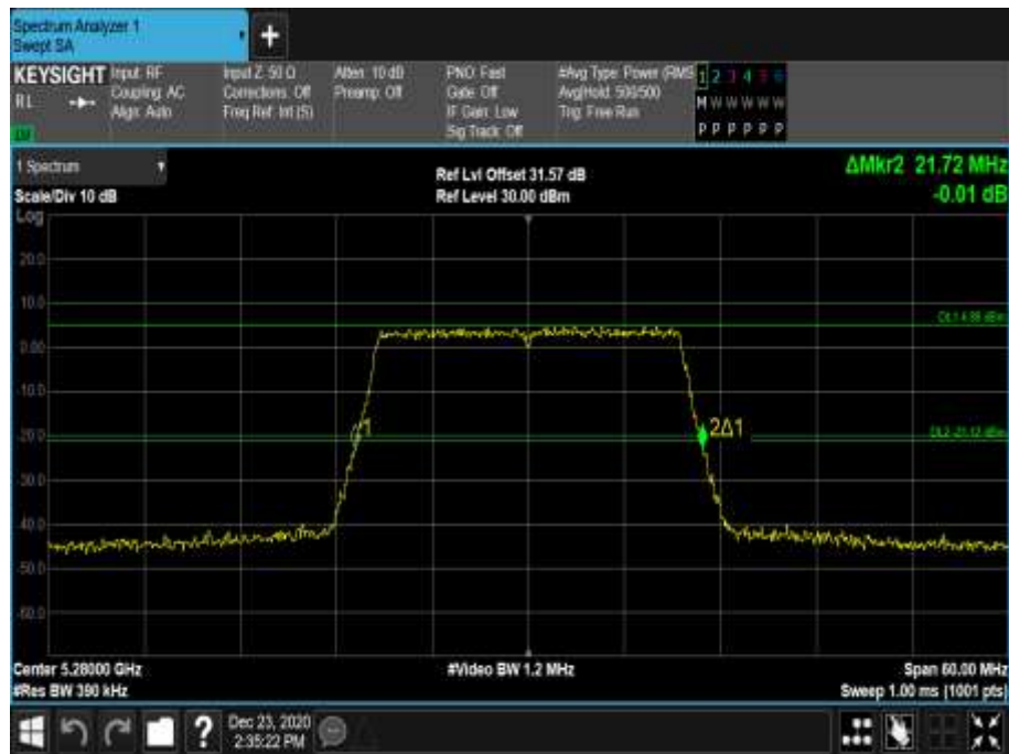
Figure 379 - 5280 MHz - 26 dB Emission Bandwidth
