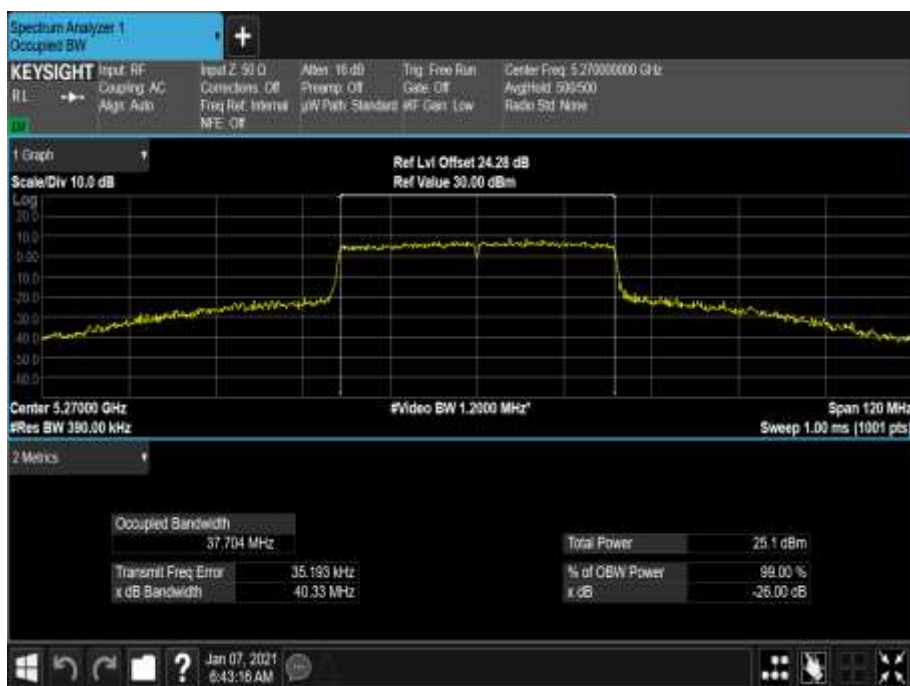
Figure 406 - 5270 MHz - 99% Occupied Bandwidth
