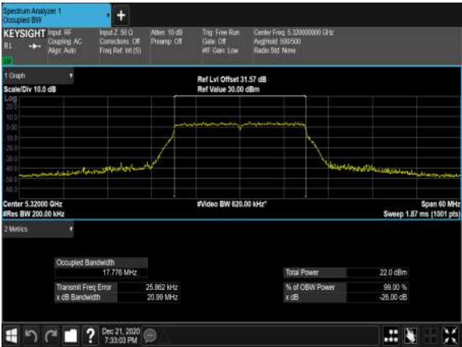
Figure 352 - 5320 MHz - 99% Occupied Bandwidth
