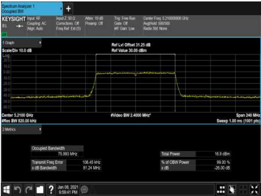
Figure 304 - 5210 MHz - 99% Occupied Bandwidth
