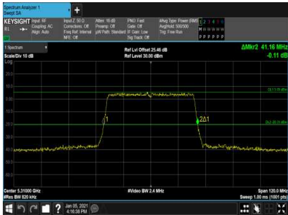
Figure 415 - 5310 MHz - 26 dB Emission Bandwidth
