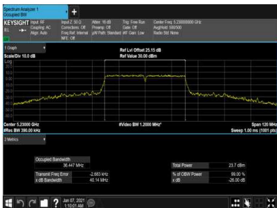
Figure 188 - 5230 MHz - 99% Occupied Bandwidth
