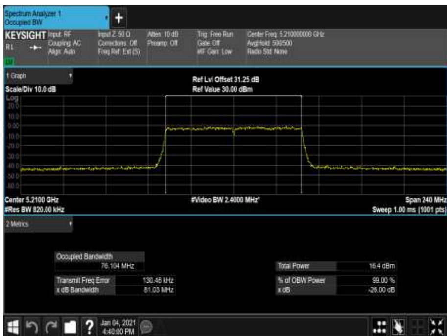
Figure 298 - 5210 MHz - 99% Occupied Bandwidth
