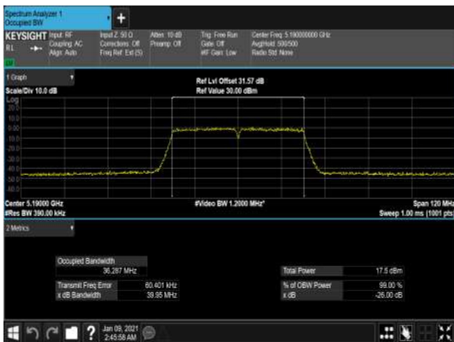
Figure 210 - 5190 MHz - 99% Occupied Bandwidth
