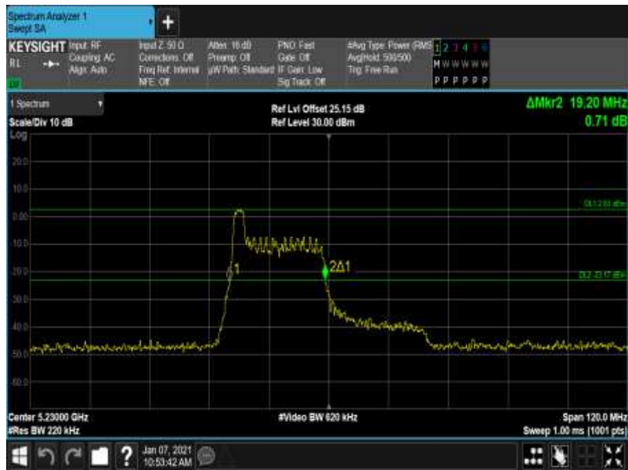
Figure 231 - 5230 MHz - 26 dB Emission Bandwidth
