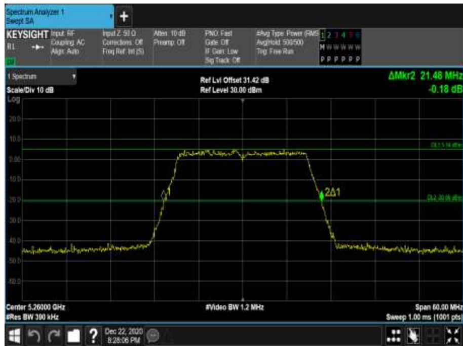
Figure 353 - 5260 MHz - 26 dB Emission Bandwidth
