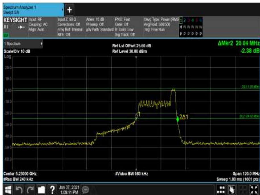
Figure 287 - 5230 MHz - 26 dB Emission Bandwidth
