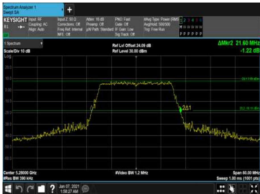
Figure 361 - 5280 MHz - 26 dB Emission Bandwidth
