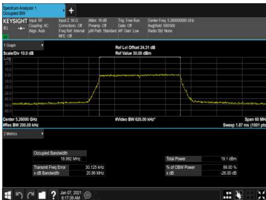
Figure 378 - 5260 MHz - 99% Occupied Bandwidth
