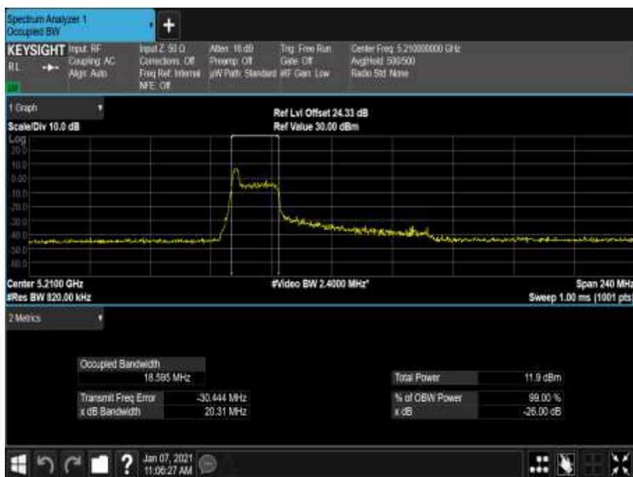
Figure 312 - 5210 MHz - 99% Occupied Bandwidth
