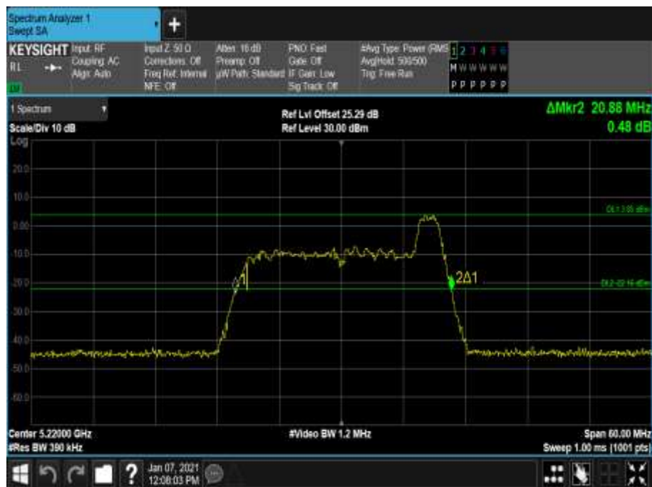
Figure 181 - 5220 MHz - 26 dB Emission Bandwidth
