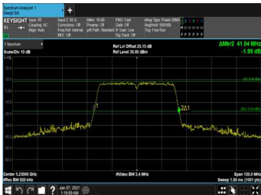
Figure 191 - 5230 MHz - 26 dB Emission Bandwidth
