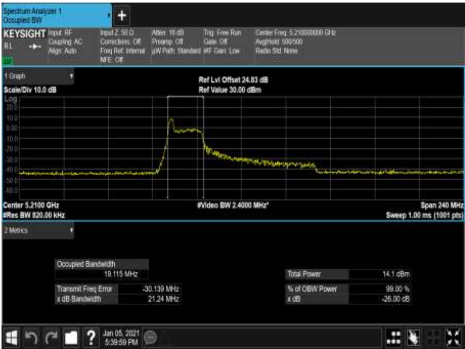
Figure 334 - 5210 MHz - 99% Occupied Bandwidth
