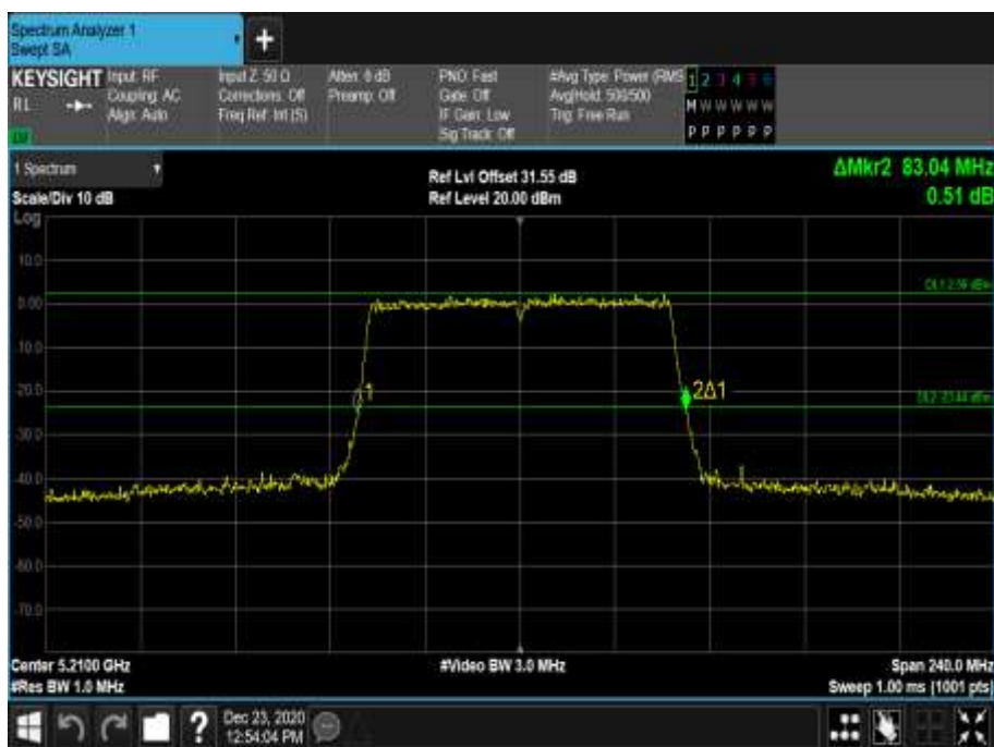
Figure 293 - 5210 MHz - 26 dB Emission Bandwidth
