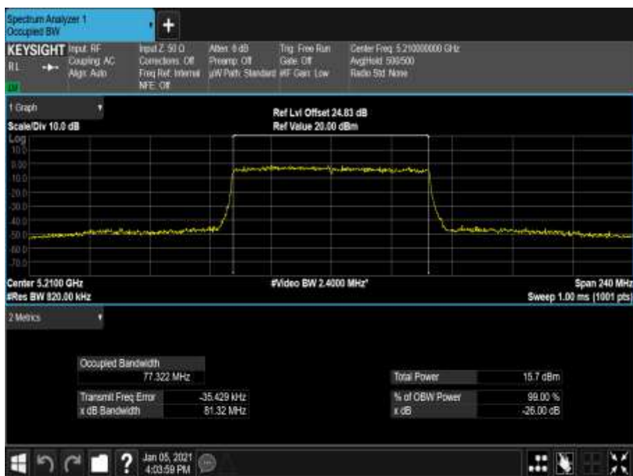
Figure 332 - 5210 MHz - 99% Occupied Bandwidth
