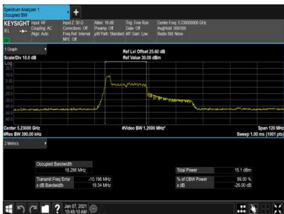
Figure 276 - 5230 MHz - 99% Occupied Bandwidth
