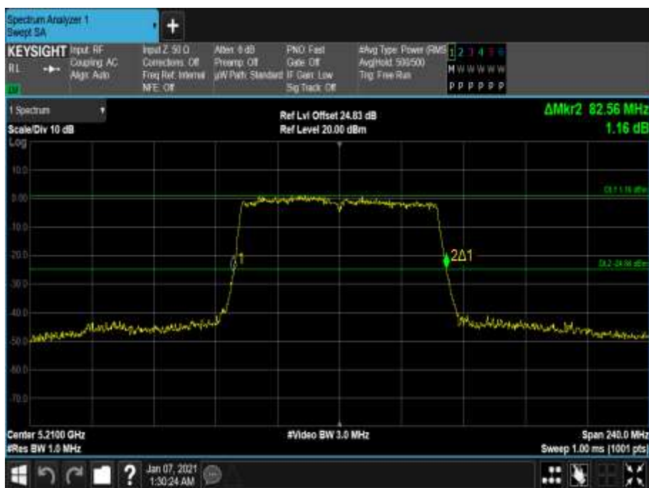
Figure 295 - 5210 MHz - 26 dB Emission Bandwidth
