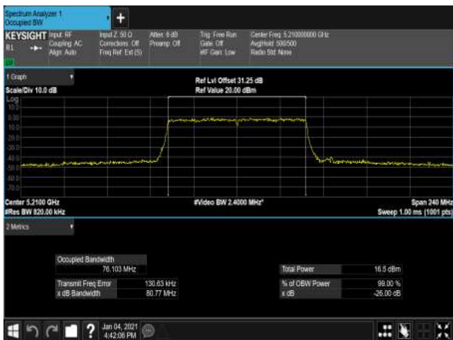
Figure 300 - 5210 MHz - 99% Occupied Bandwidth
