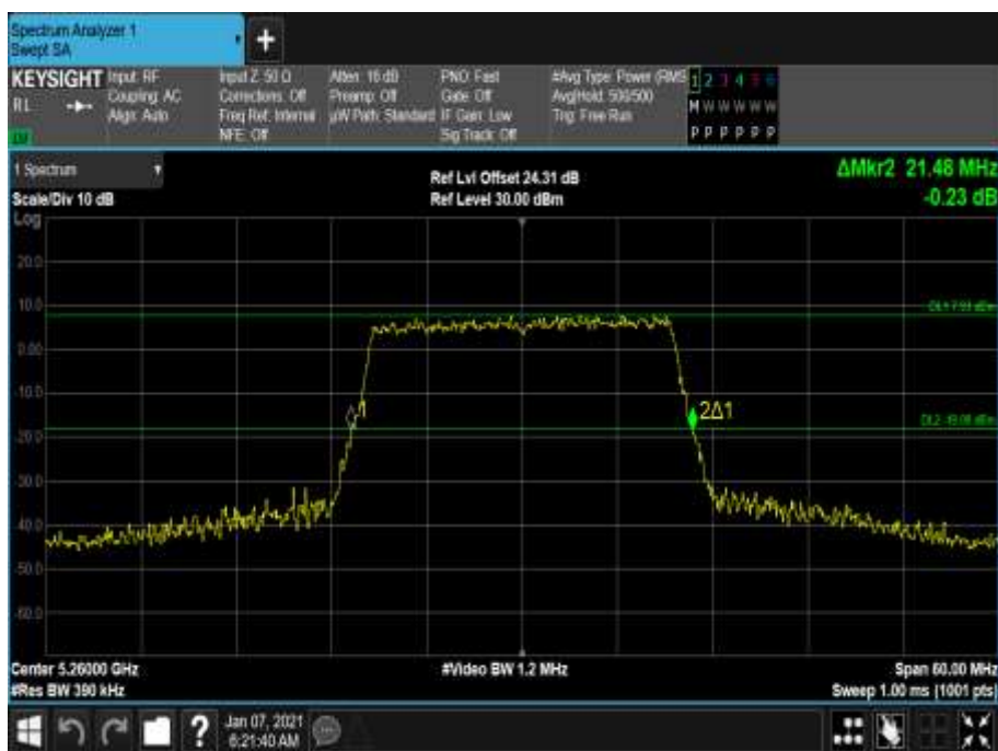
Figure 383 - 5260 MHz - 26 dB Emission Bandwidth
