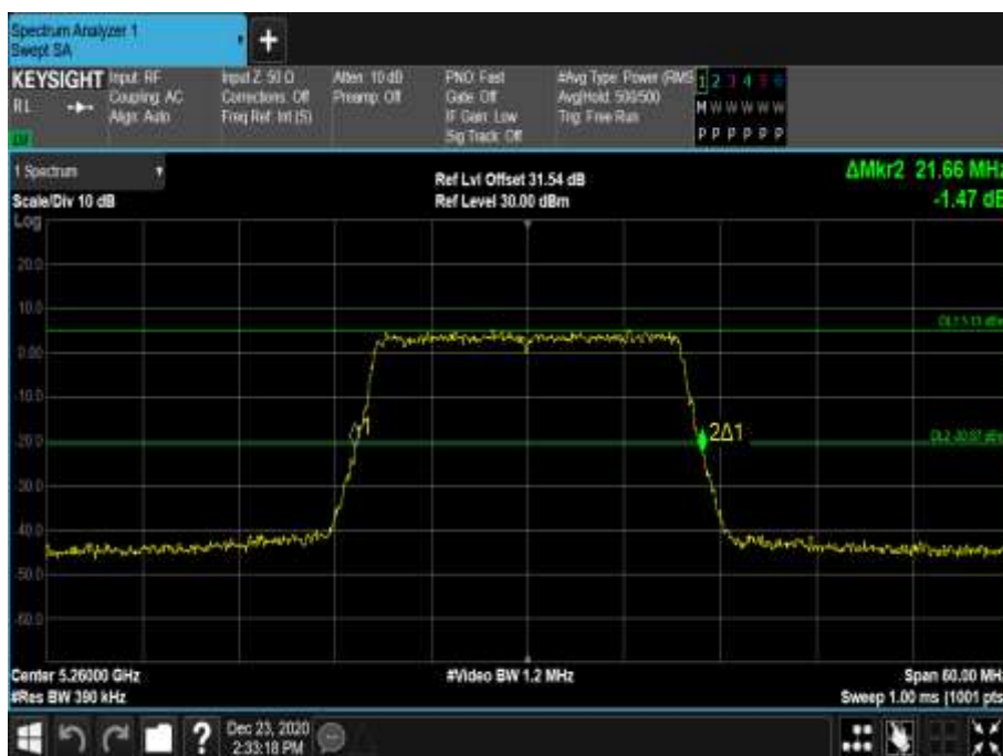
Figure 377 - 5260 MHz - 26 dB Emission Bandwidth
