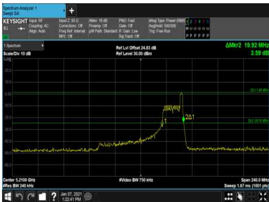
Figure 339 - 5210 MHz - 26 dB Emission Bandwidth
