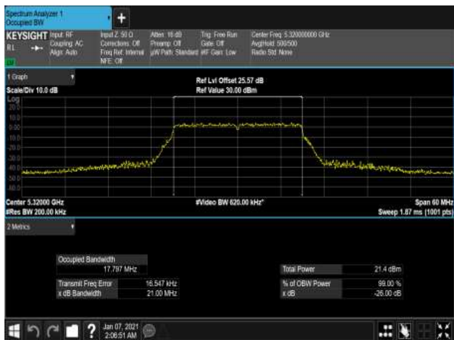
Figure 364 - 5320 MHz - 99% Occupied Bandwidth
