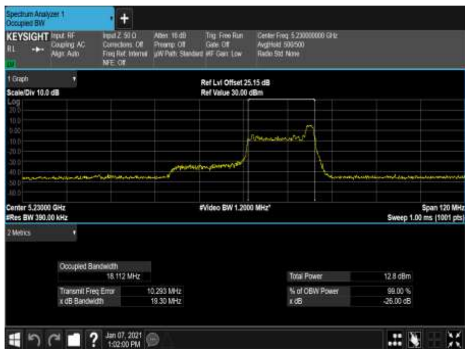
Figure 240 - 5230 MHz - 99% Occupied Bandwidth
