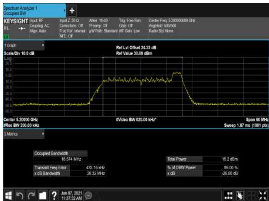
Figure 172 - 5200 MHz - 99% Occupied Bandwidth
