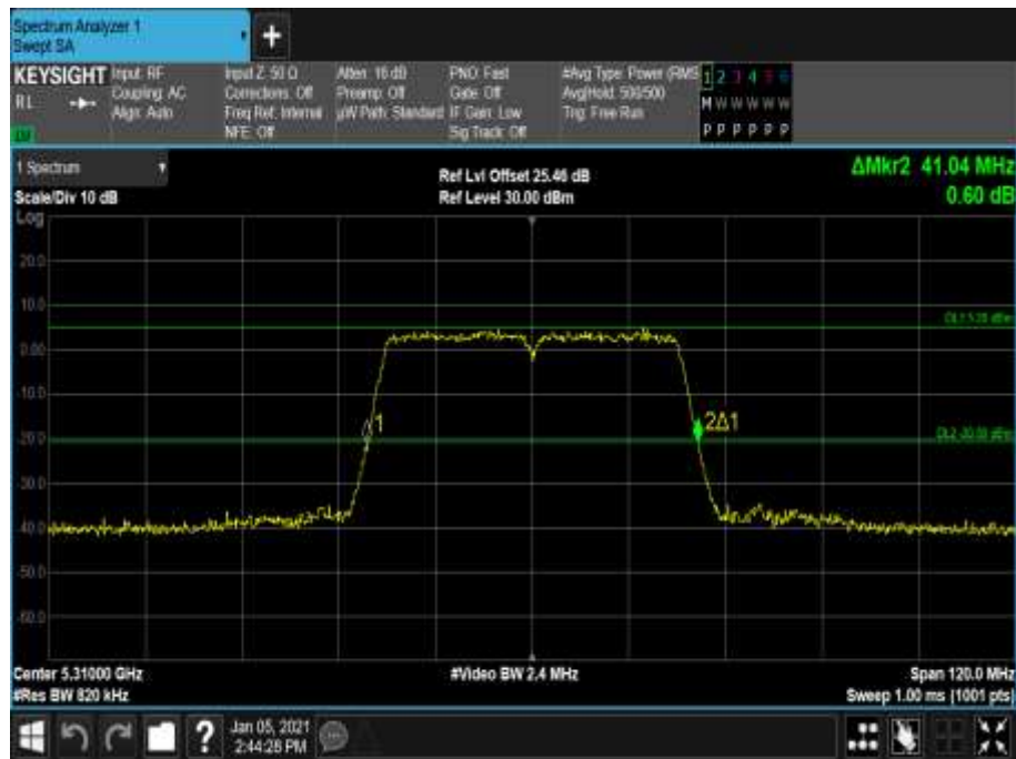
Figure 399 - 5310 MHz - 26 dB Emission Bandwidth
