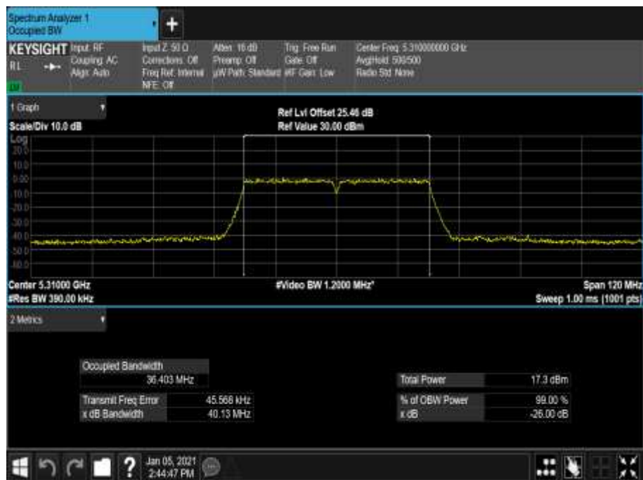
Figure 400 - 5310 MHz - 99% Occupied Bandwidth
