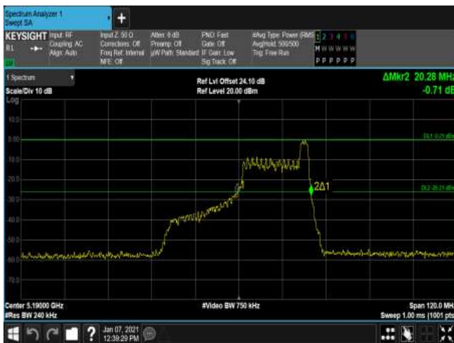
Figure 261 - 5190 MHz - 26 dB Emission Bandwidth
