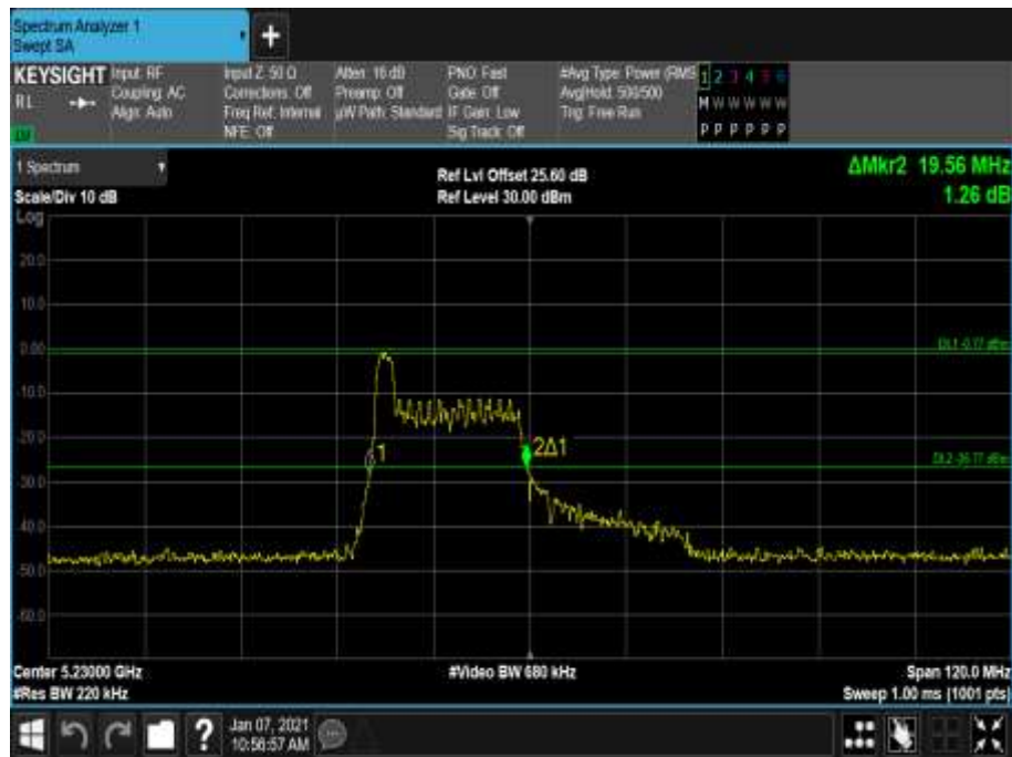
Figure 255 - 5230 MHz - 26 dB Emission Bandwidth
