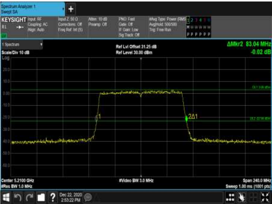
Figure 289 - 5210 MHz - 26 dB Emission Bandwidth
