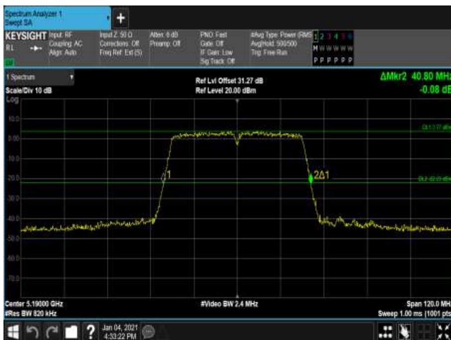
Figure 205 - 5190 MHz - 26 dB Emission Bandwidth
