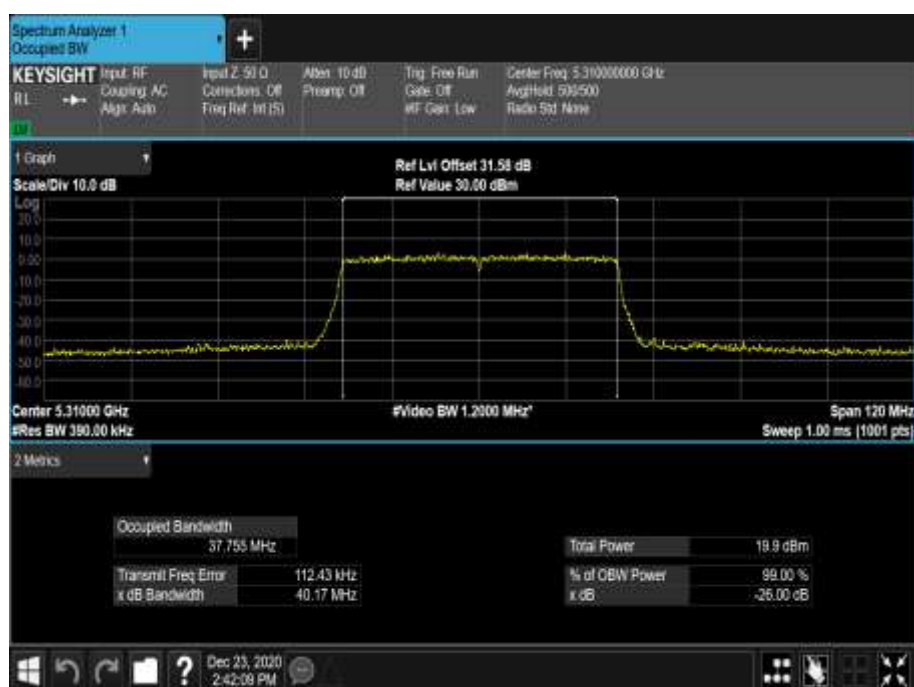
Figure 412 - 5310 MHz - 99% Occupied Bandwidth
