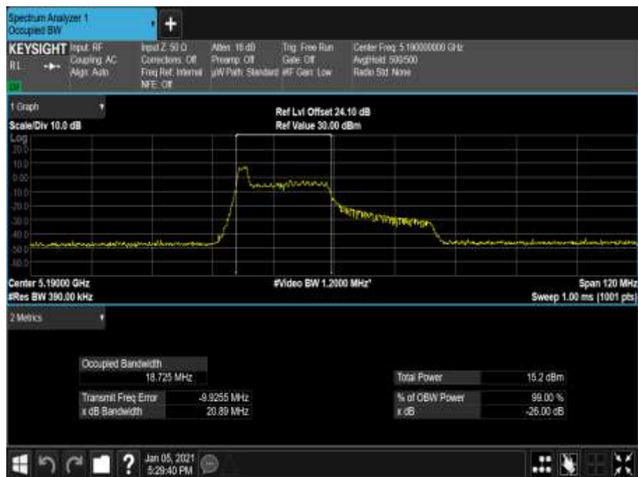
Figure 274 - 5190 MHz - 99% Occupied Bandwidth
