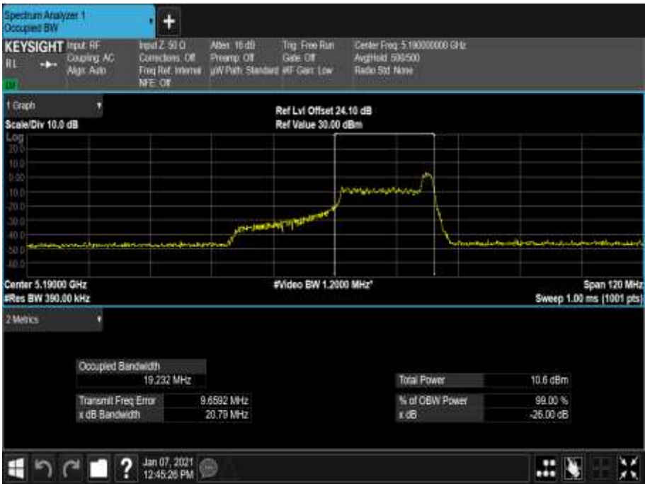
Figure 286 - 5190 MHz - 99% Occupied Bandwidth
