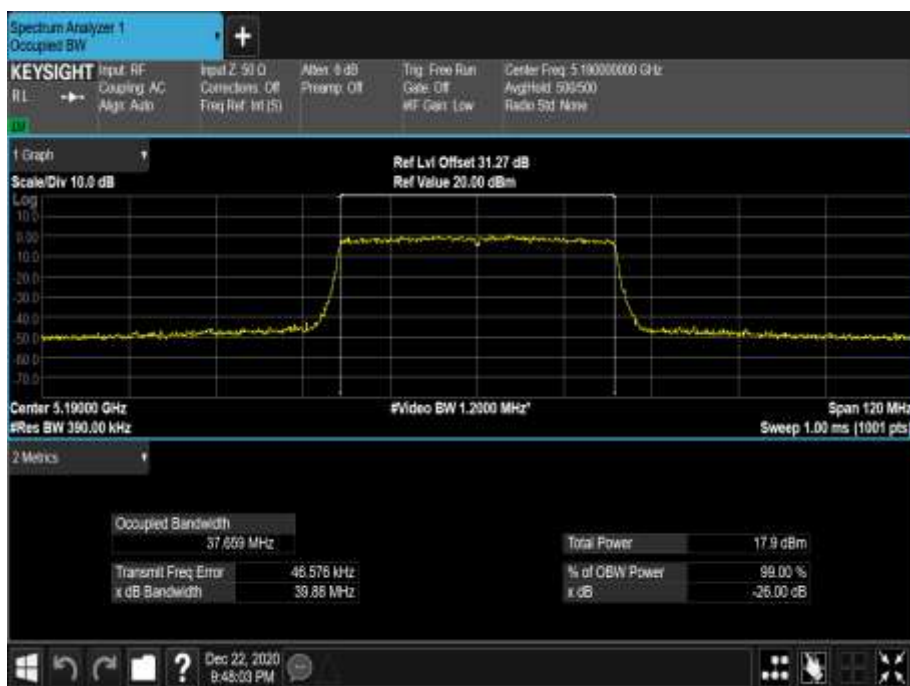
Figure 242 - 5190 MHz - 99% Occupied Bandwidth
