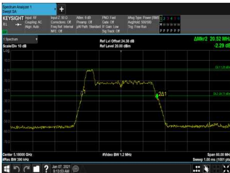
Figure 117 - 5180 MHz - 26 dB Emission Bandwidth
