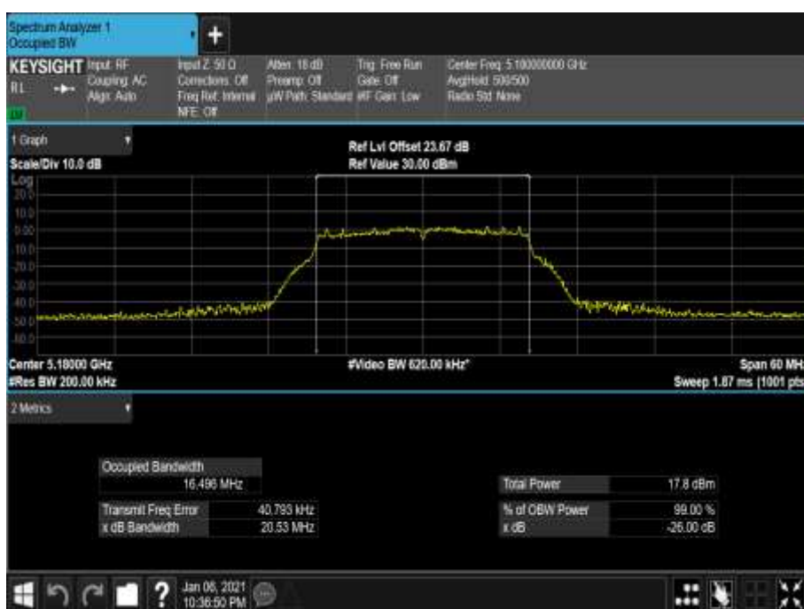
Figure 8 - 5180 MHz - 99% Occupied Bandwidth
