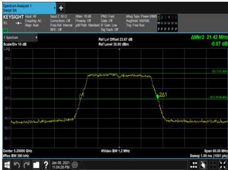
Figure 21 - 5200 MHz - 26 dB Emission Bandwidth
