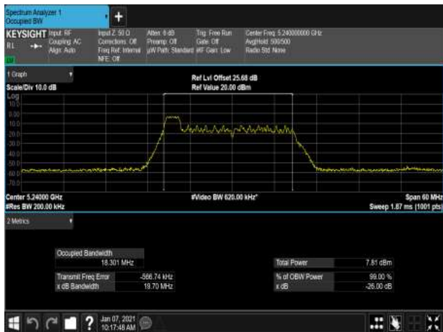
Figure 124 - 5240 MHz - 99% Occupied Bandwidth
