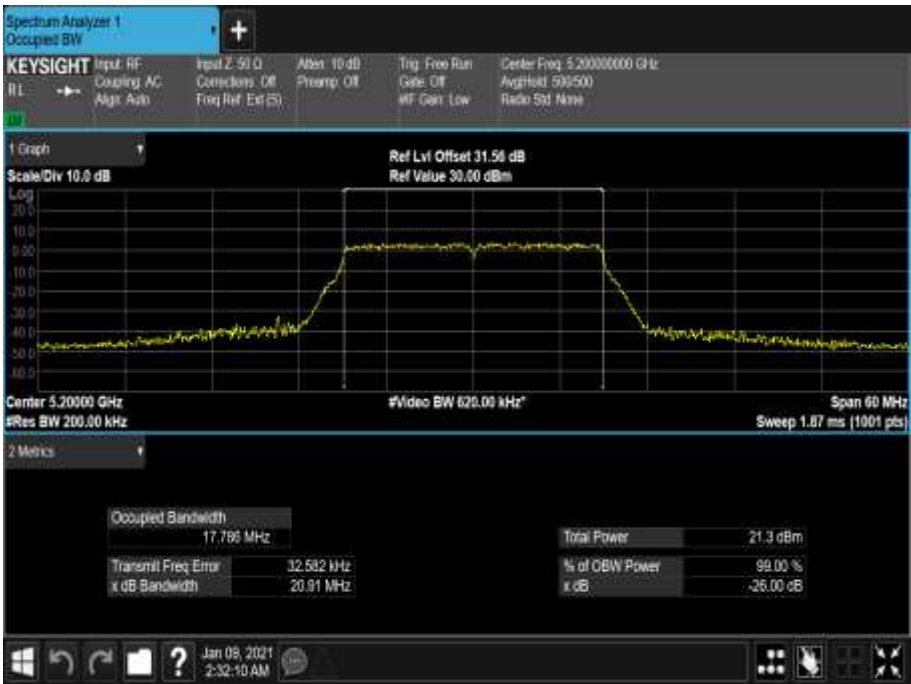
Figure 52 - 5200 MHz - 99% Occupied Bandwidth
