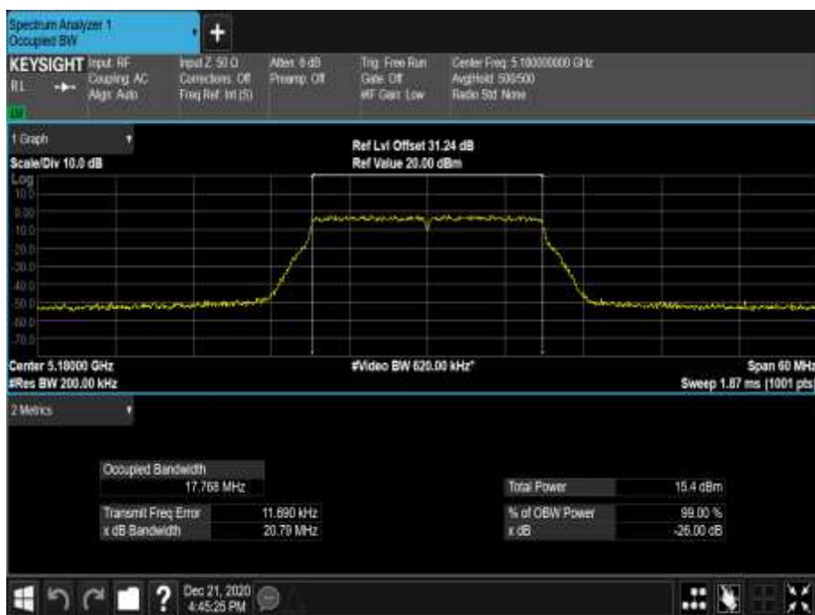
Figure 50 - 5180 MHz - 99% Occupied Bandwidth
