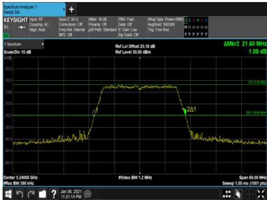
Figure 29 - 5240 MHz - 26 dB Emission Bandwidth
