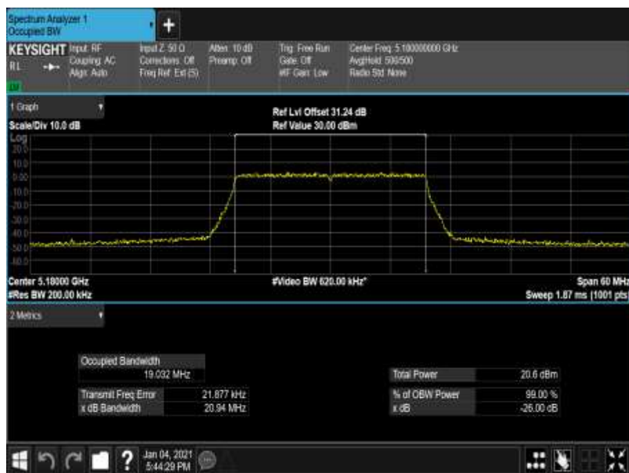
Figure 142 - 5180 MHz - 99% Occupied Bandwidth
