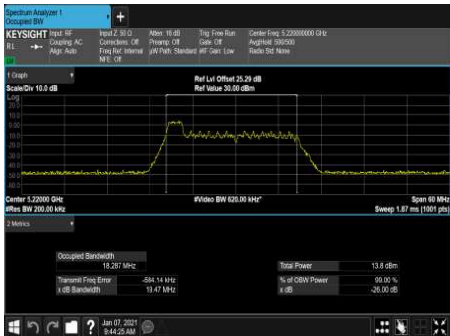
Figure 114 - 5220 MHz - 99% Occupied Bandwidth
