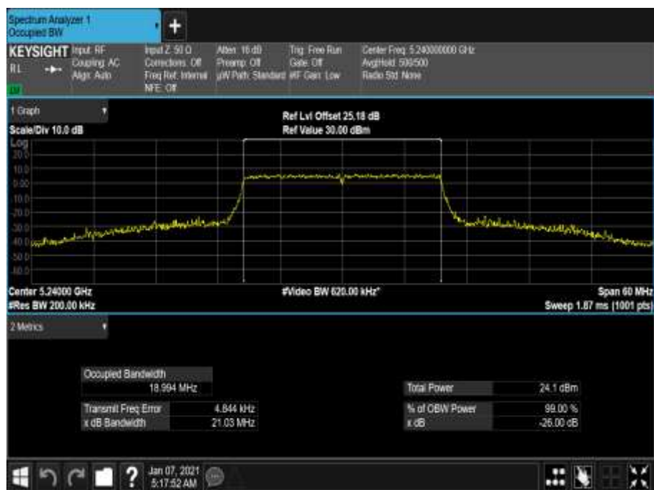
Figure 66 - 5240 MHz - 99% Occupied Bandwidth
