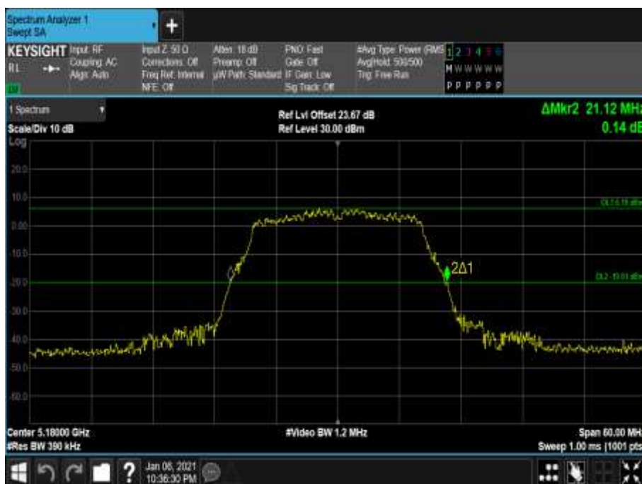
Figure 7 - 5180 MHz - 26 dB Emission Bandwidth
