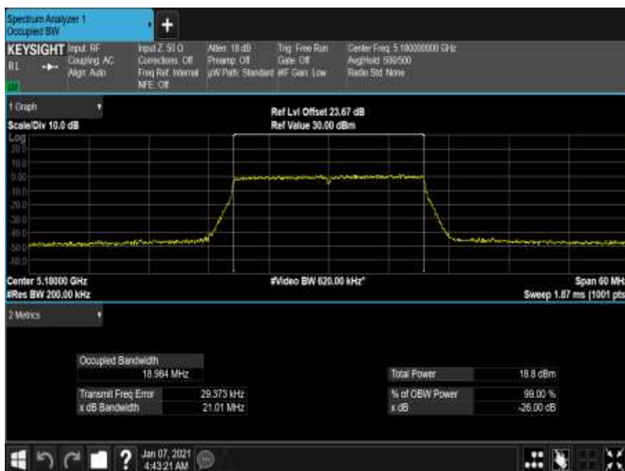
Figure 68 - 5180 MHz - 99% Occupied Bandwidth
