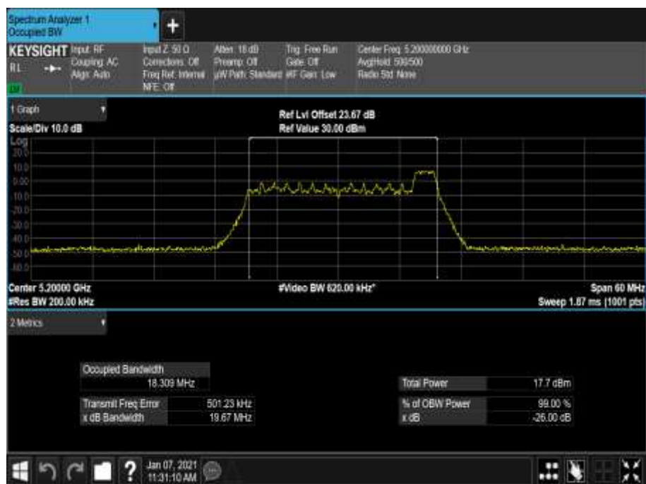
Figure 88 - 5200 MHz - 99% Occupied Bandwidth
