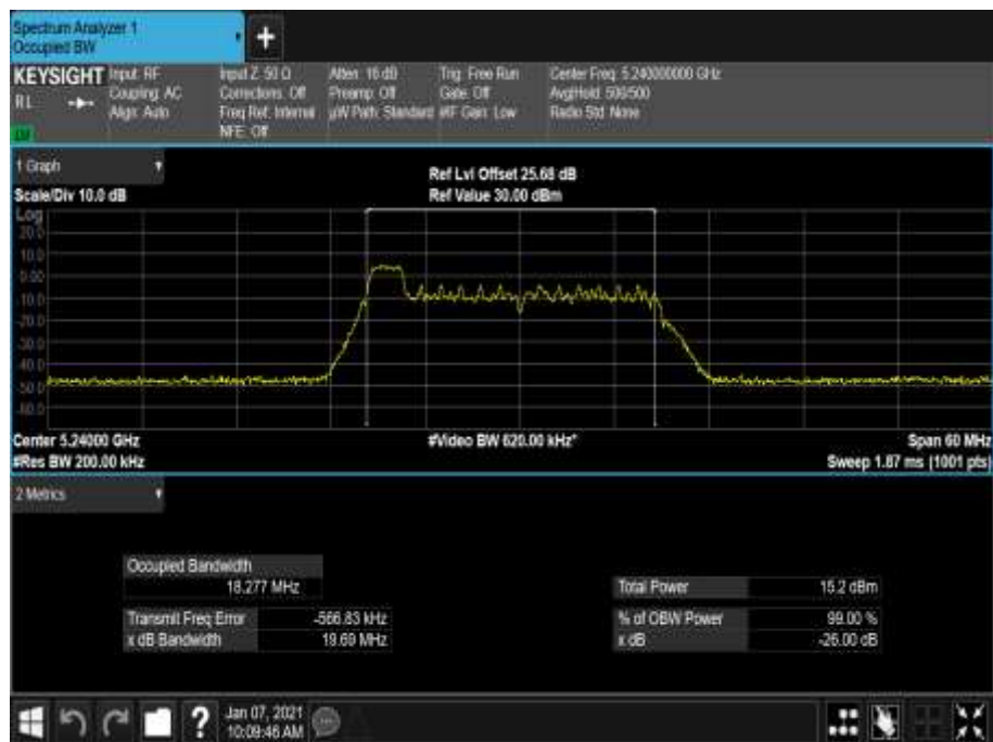
Figure 160 - 5240 MHz - 99% Occupied Bandwidth
