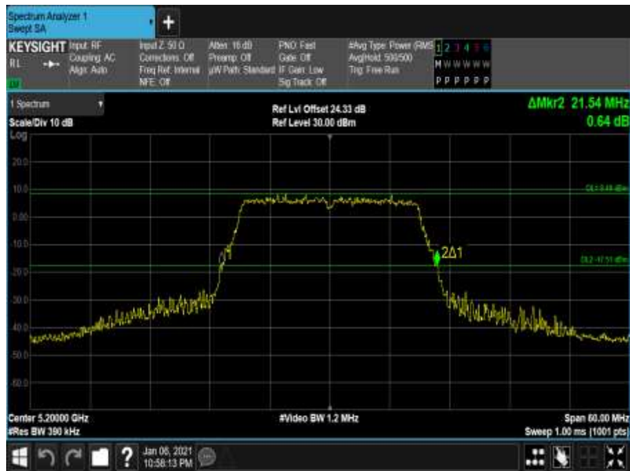
Figure 39 - 5200 MHz - 26 dB Emission Bandwidth
