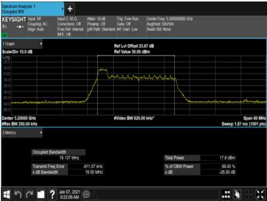
Figure 76 - 5200 MHz - 99% Occupied Bandwidth
