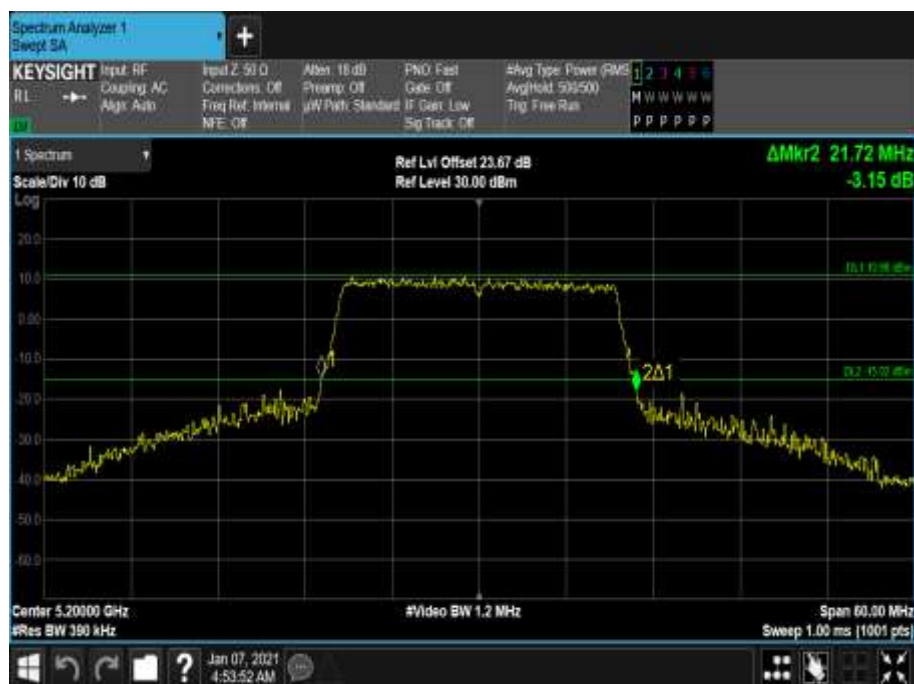
Figure 63 - 5200 MHz - 26 dB Emission Bandwidth
