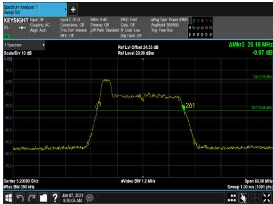
Figure 119 - 5200 MHz - 26 dB Emission Bandwidth
