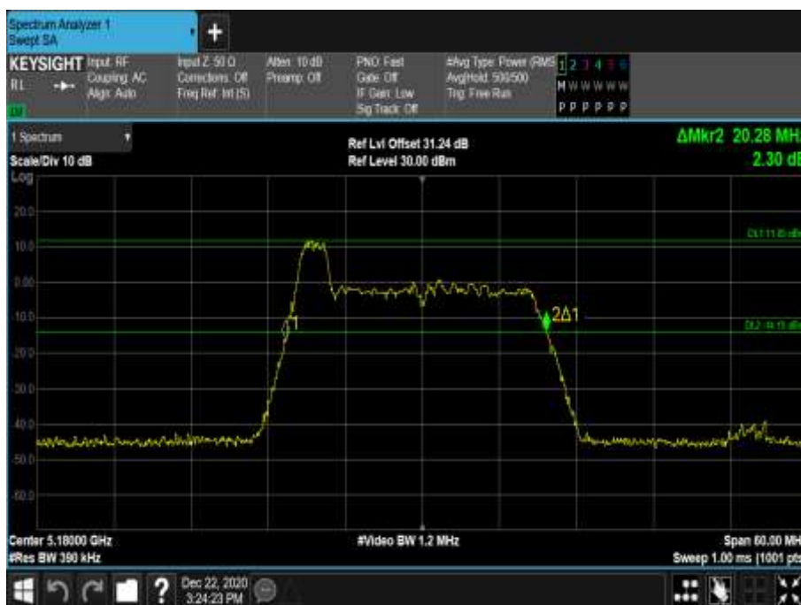
Figure 73 - 5180 MHz - 26 dB Emission Bandwidth
