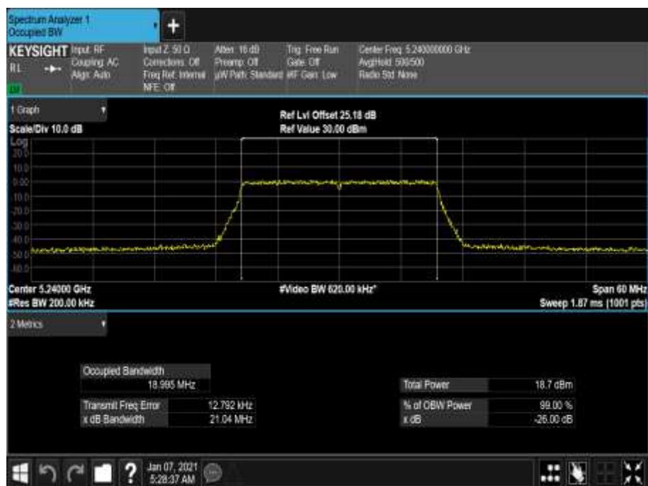
Figure 72 - 5240 MHz - 99% Occupied Bandwidth
