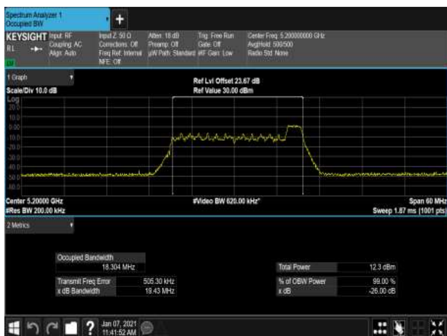
Figure 94 - 5200 MHz - 99% Occupied Bandwidth
