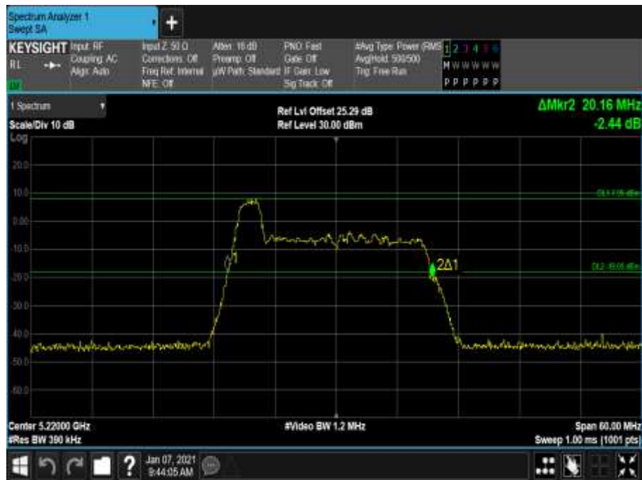
Figure 113 - 5220 MHz - 26 dB Emission Bandwidth
