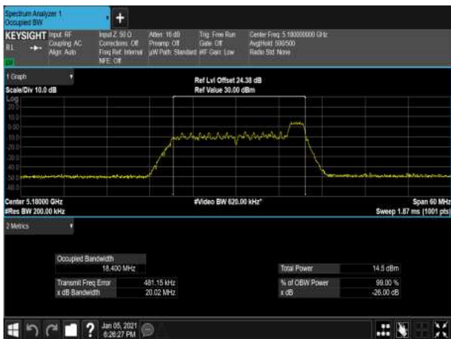
Figure 170 - 5180 MHz - 99% Occupied Bandwidth
