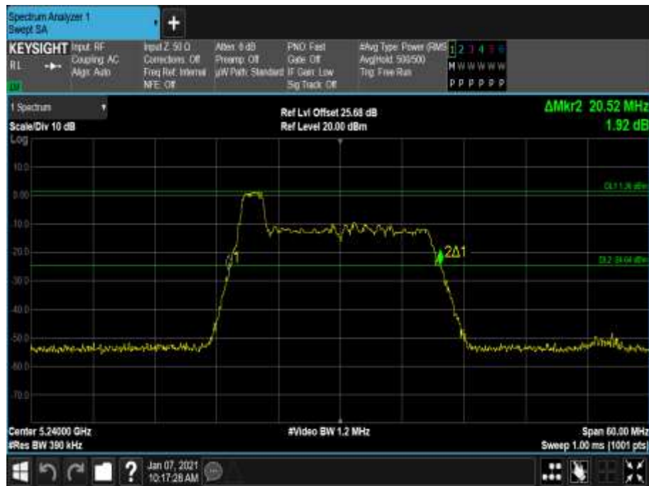
Figure 123 - 5240 MHz - 26 dB Emission Bandwidth
