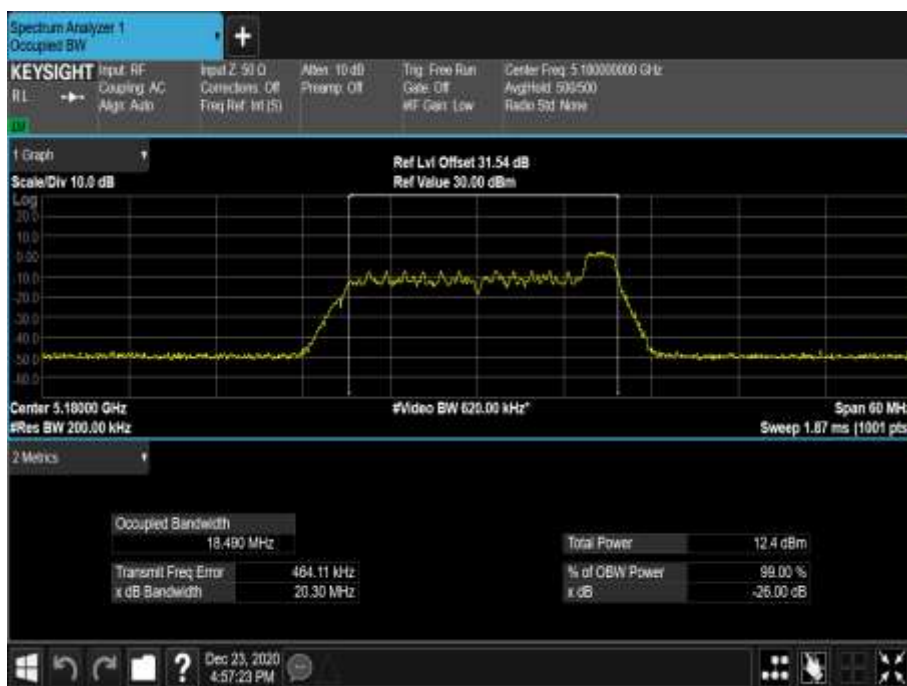
Figure 126 - 5180 MHz - 99% Occupied Bandwidth
