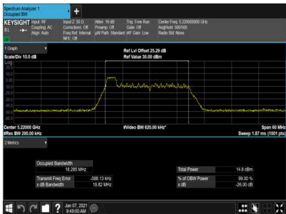
Figure 158 - 5220 MHz - 99% Occupied Bandwidth
