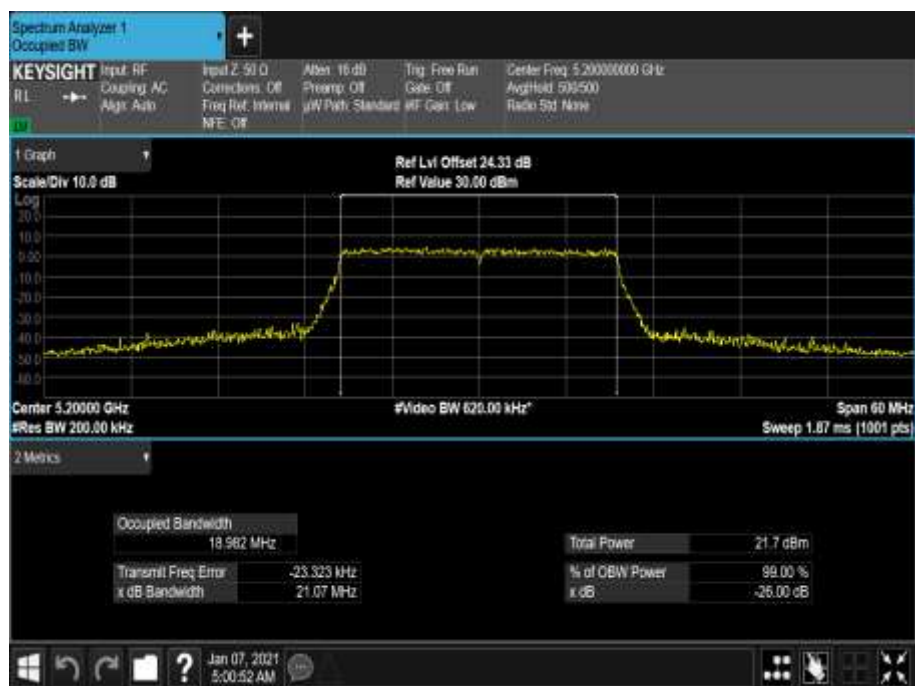
Figure 144 - 5200 MHz - 99% Occupied Bandwidth
