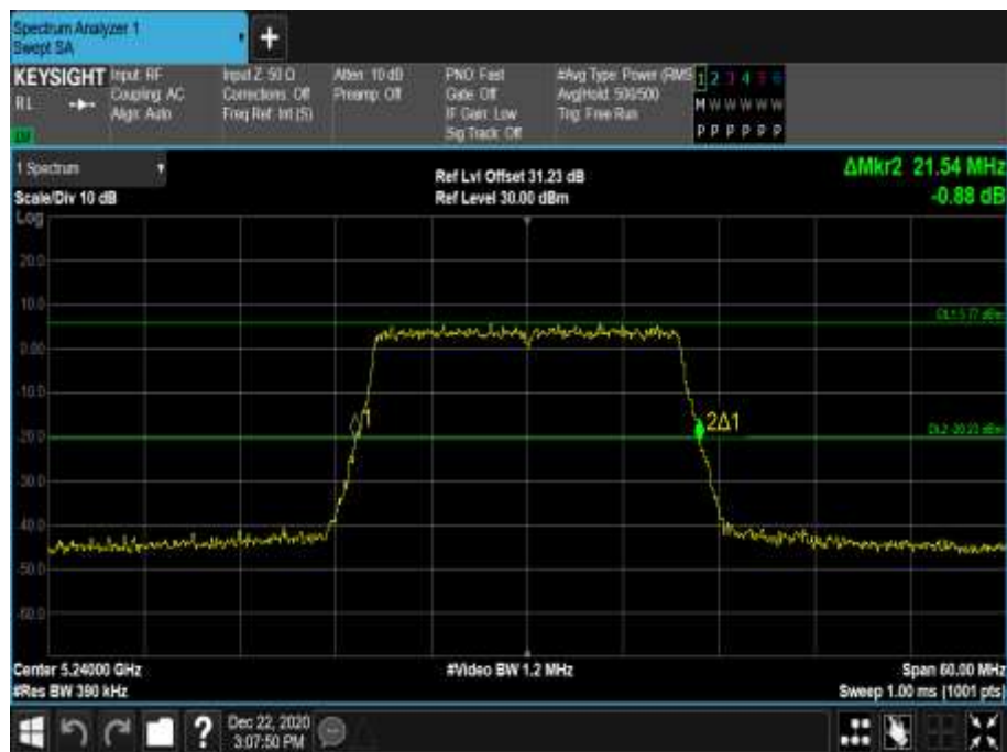
Figure 71 - 5240 MHz - 26 dB Emission Bandwidth
