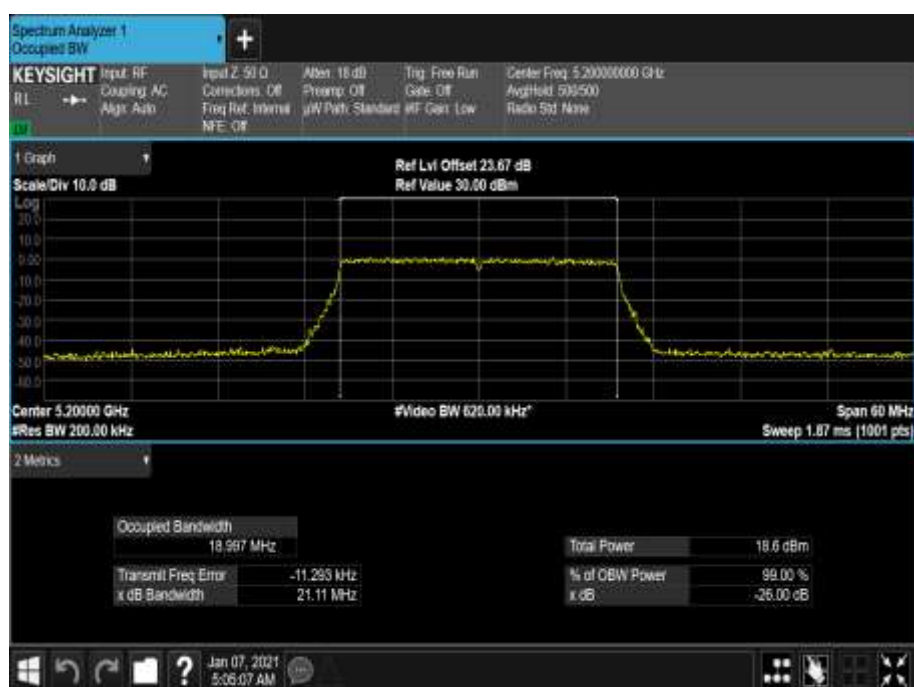
Figure 70 - 5200 MHz - 99% Occupied Bandwidth
