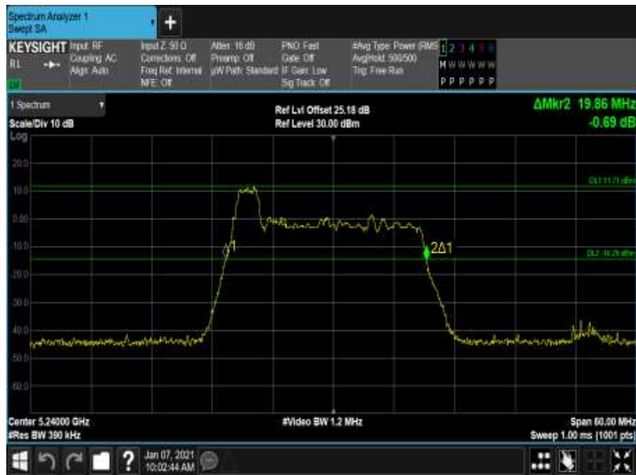
Figure 77 - 5240 MHz - 26 dB Emission Bandwidth
