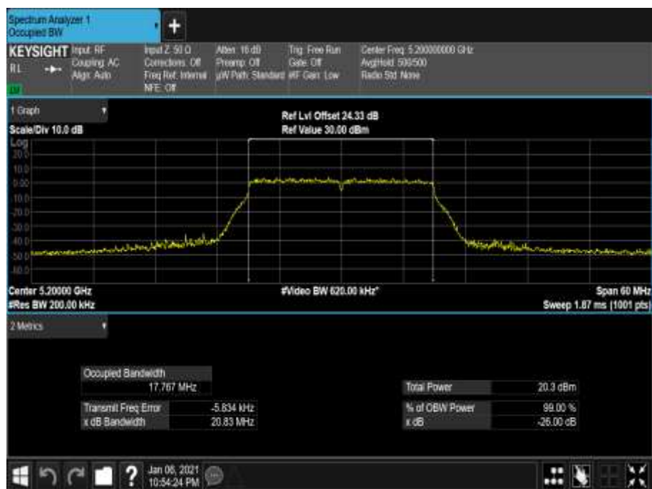
Figure 28 - 5200 MHz - 99% Occupied Bandwidth
