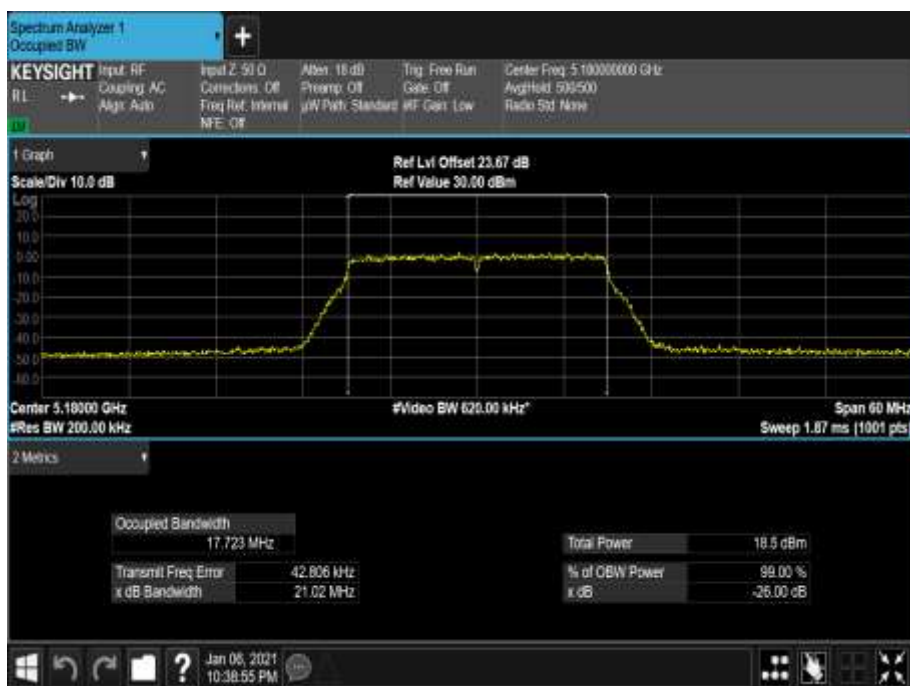
Figure 20 - 5180 MHz - 99% Occupied Bandwidth
