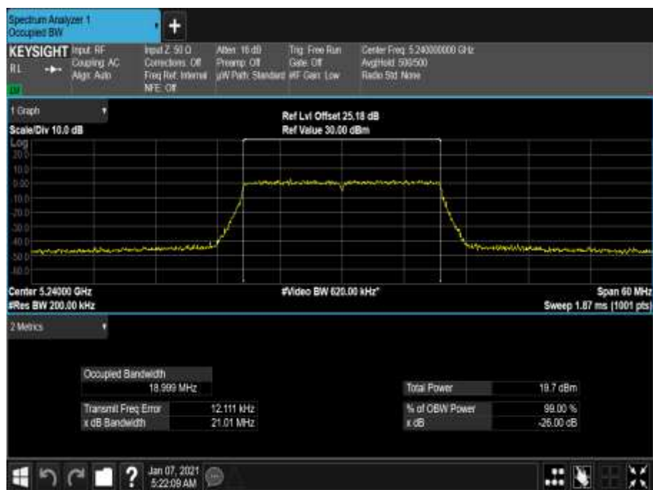
Figure 102 - 5240 MHz - 99% Occupied Bandwidth
