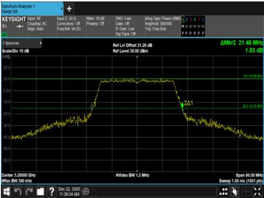
Figure 15 - 5200 MHz - 26 dB Emission Bandwidth
