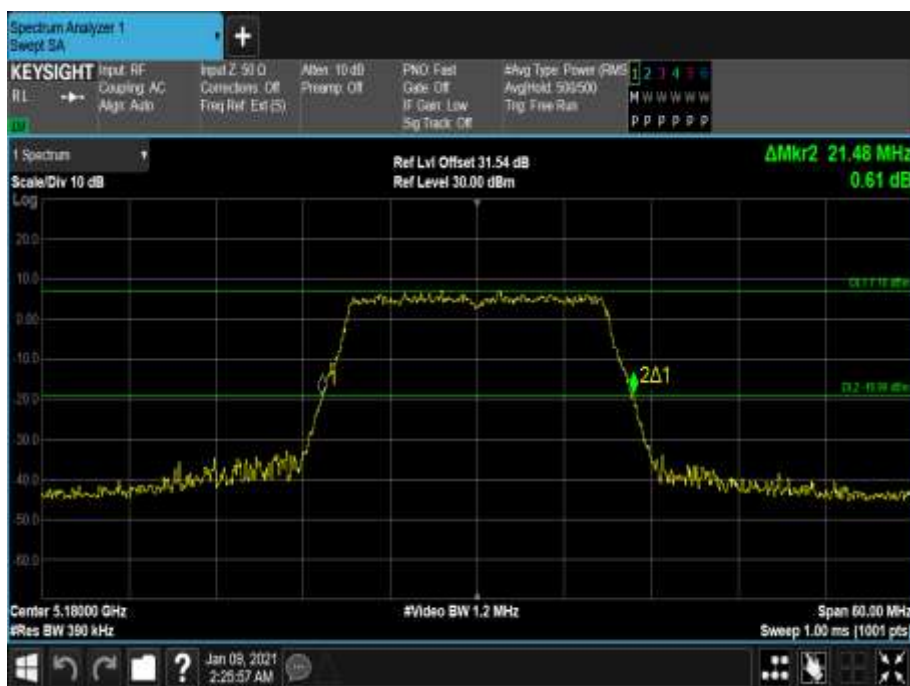
Figure 49 - 5180 MHz - 26 dB Emission Bandwidth
