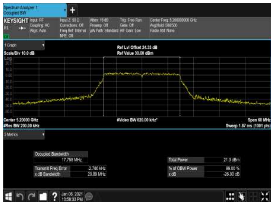
Figure 40 - 5200 MHz - 99% Occupied Bandwidth
