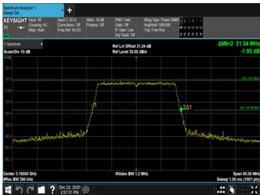
Figure 61 - 5180 MHz - 26 dB Emission Bandwidth
