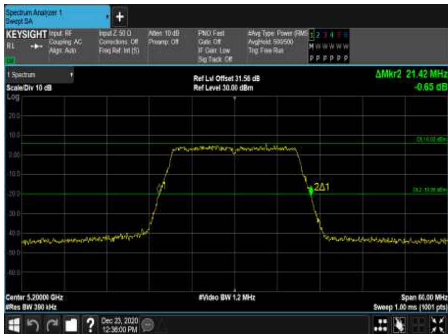
Figure 27 - 5200 MHz - 26 dB Emission Bandwidth
