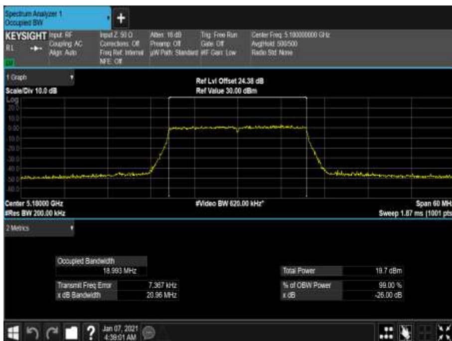
Figure 98 - 5180 MHz - 99% Occupied Bandwidth
