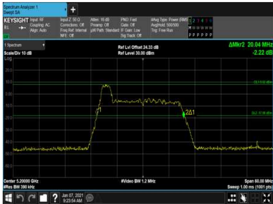
Figure 111 - 5200 MHz - 26 dB Emission Bandwidth
