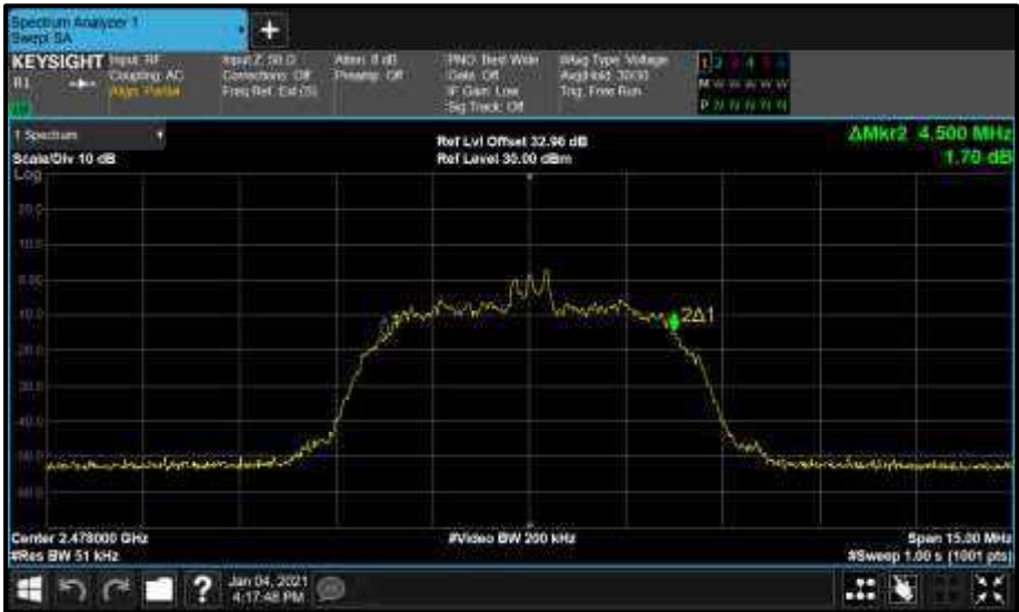
Figure 119 - Core0 (C) 2478 MHz (CH76) 99% Bandwidth
