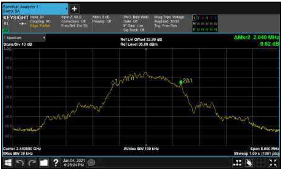
Figure 67 - Core0 (C) 2440 MHz (CH19) 99% Bandwidth
