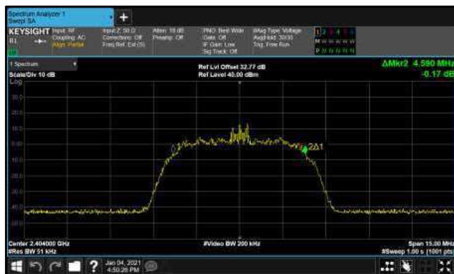
Figure 25 - Core1 (B) 2404 MHz (CH2) 99% Bandwidth
