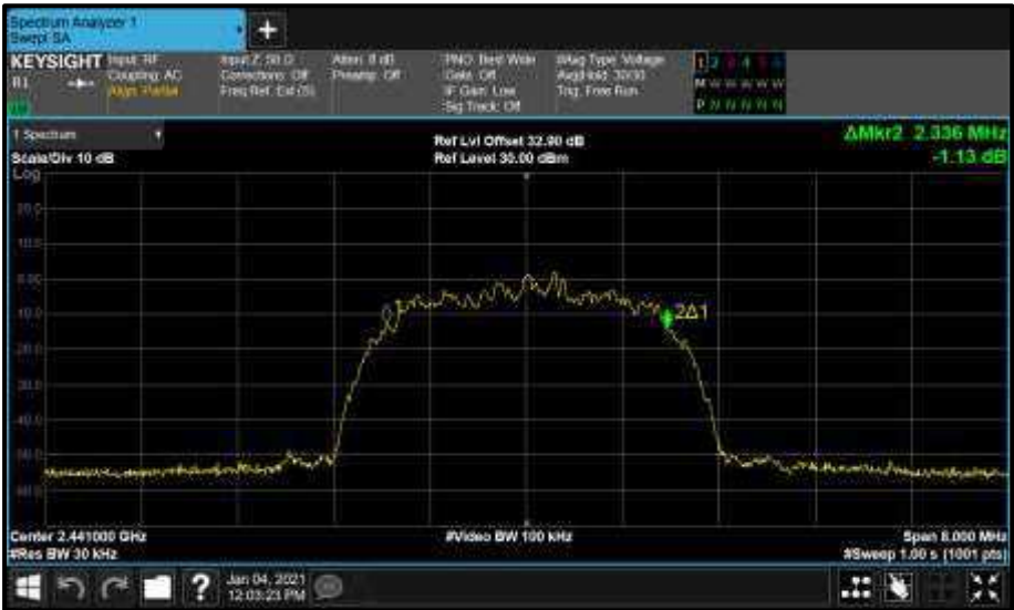
Figure 87 - Core0 (C) 2441 MHz (CH39) 99% Band width h
