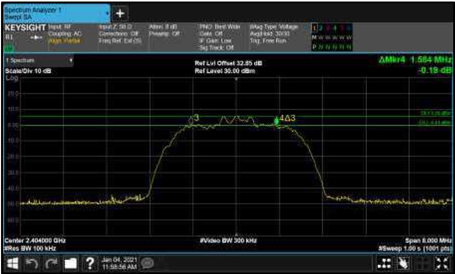
Figure 86 - Core0 (C) 2404 MHz (CH2) 6 dB Bandwidth
