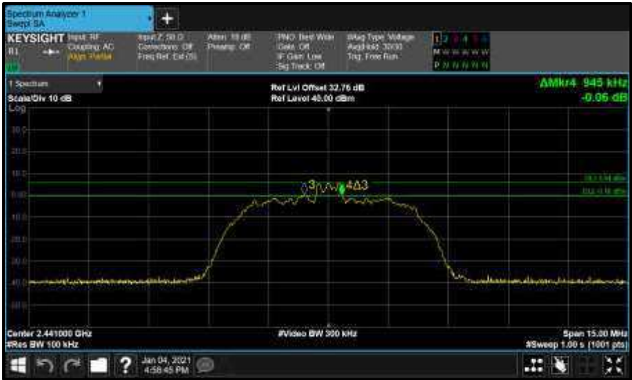
Figure 30 - Core1 (B) 2441 MHz (CH39) 6 dB Bandwidth
