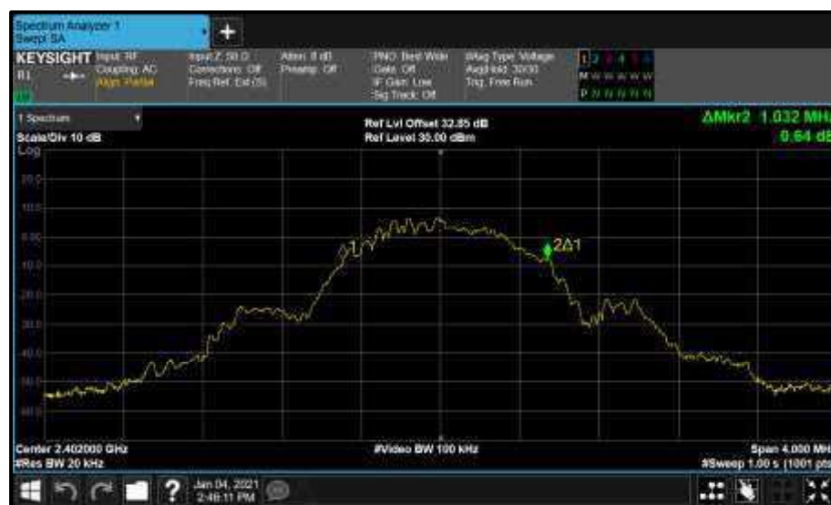
Figure 37 - Core0 (C) 2402 MHz (CH0) 99% Bandwidth
