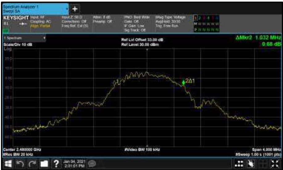
Figure 125 - Core2 (A) 2480 MHz (CH39) 99% Bandwidth
