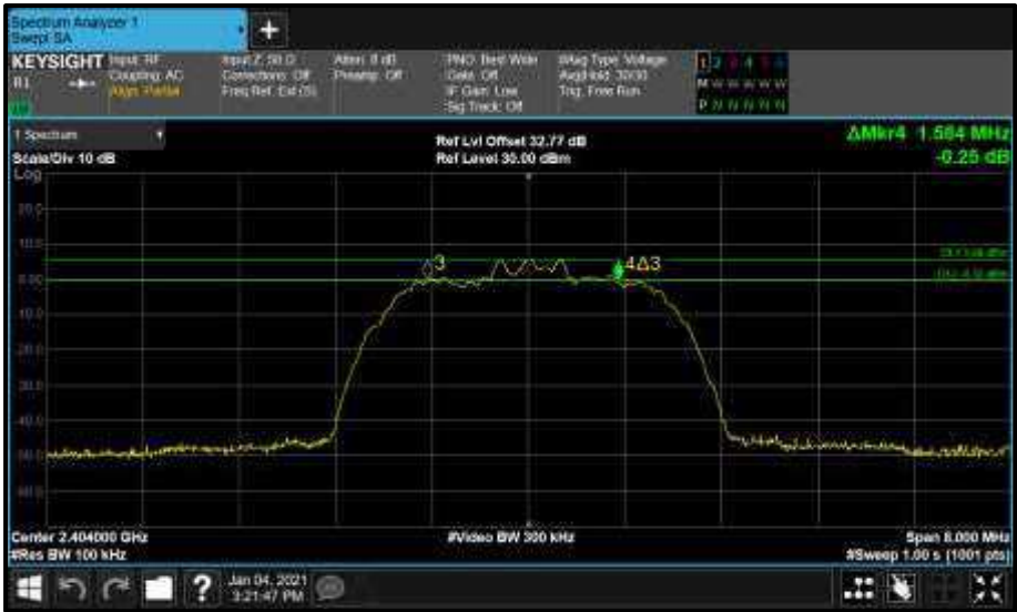
Figure 98 - Core1 (B) 2404 MHz (CH2) 6 dB Bandwidth
