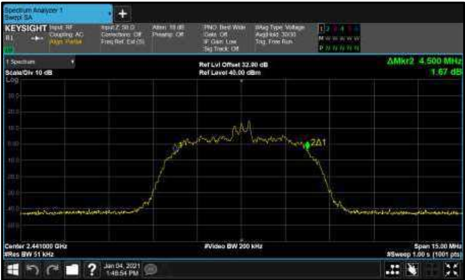
Figure 9 - Core0 (C) 2441 MHz (CH39) 99 % Bandwidth
