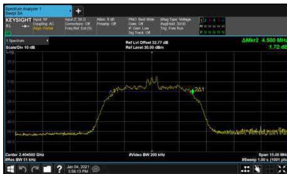
Figure 109 - Core1 (B) 2404 MHz (CH2) 99% Bandwidth
