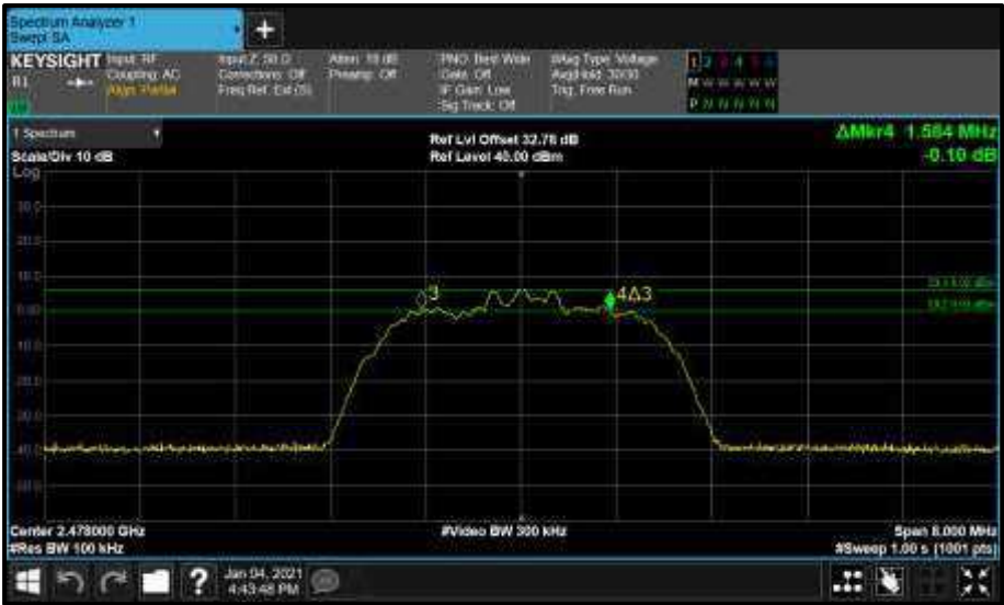
Figure 22 - Core1 (B) 2478 MHz (CH76) 6 dB Bandwidth
