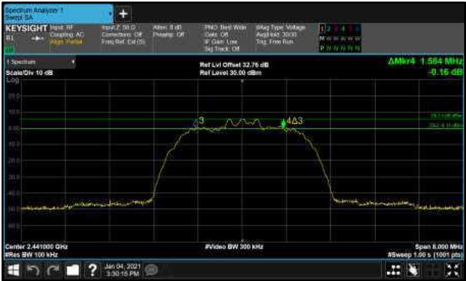
Figure 102 - Core1 (B) 2441 MHz (CH39) 6 dB Bandwidth
