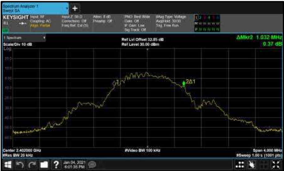
Figure 51 - Core0 (C) 2402 MHz (CH0) 99% Bandwidth
