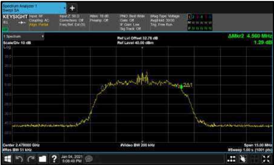
Figure 33 - Core1 (B) 2478 MHz (CH76) 99% Bandwidth
