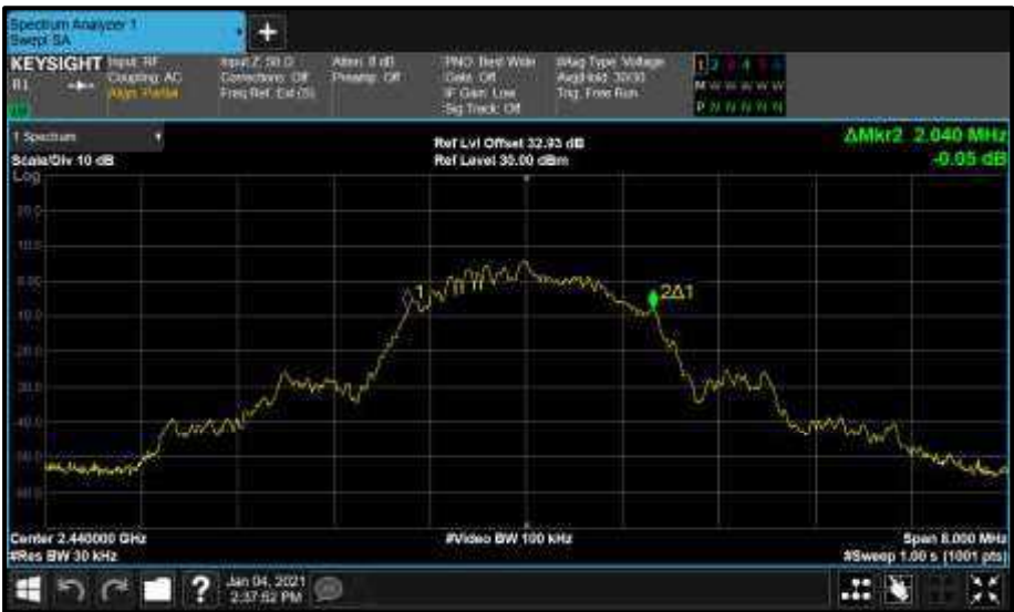
Figure 129 - Core2 (A) 2440 MHz (CH19) 99% Bandwidth
