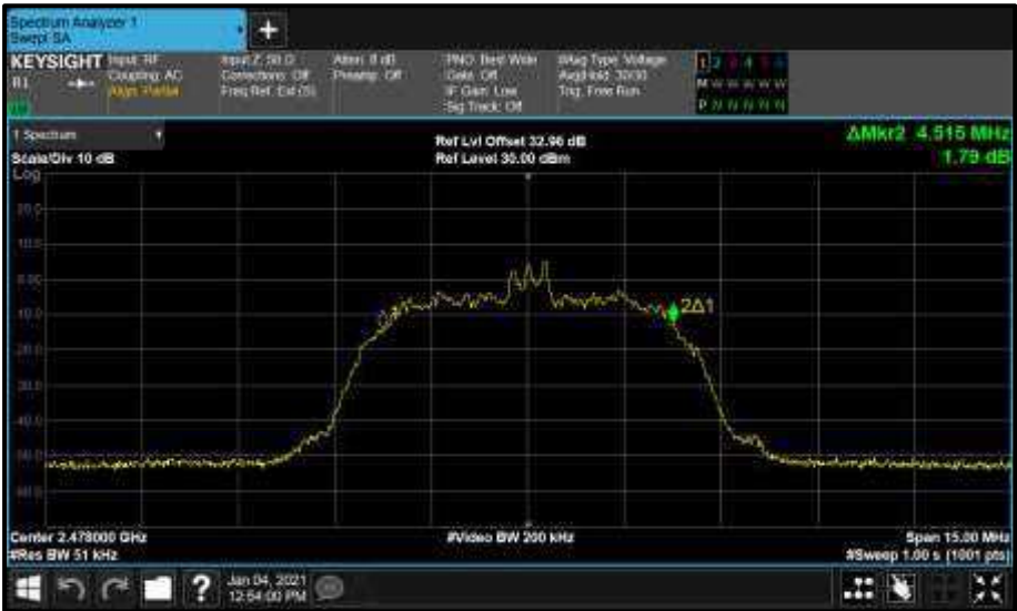
Figure 95 - Core0 (C) 2478 MHz (CH76) 99% Bandwidth
