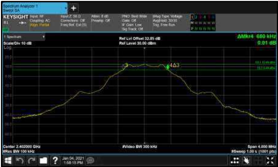
Figure 134 - Core0 (C) 2402 MHz (CH0) 6 dB Bandwidth
