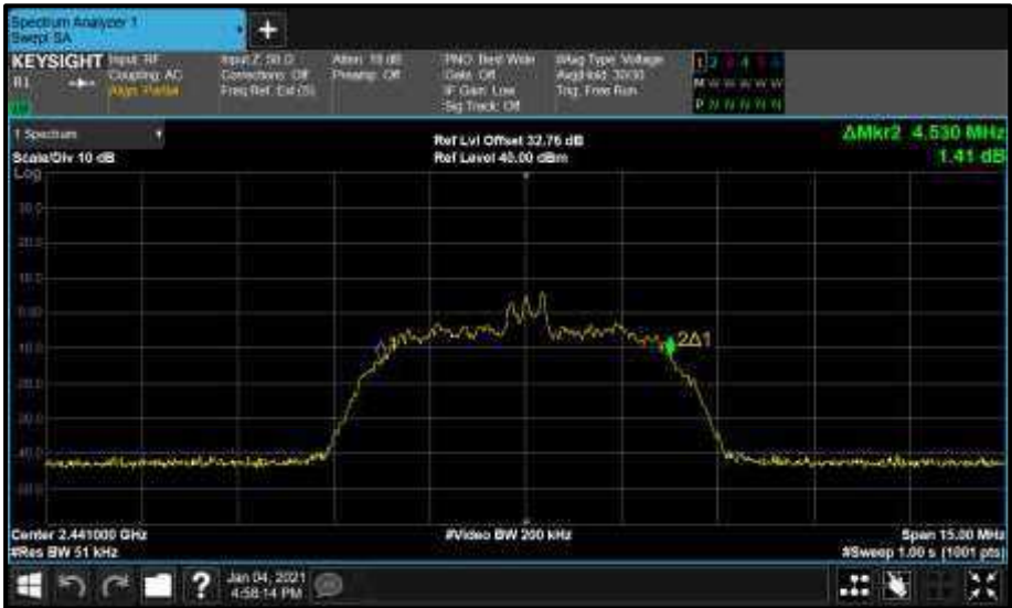
Figure 29 - Core1 (B) 2441 MHz (CH39) 99% Bandwidth
