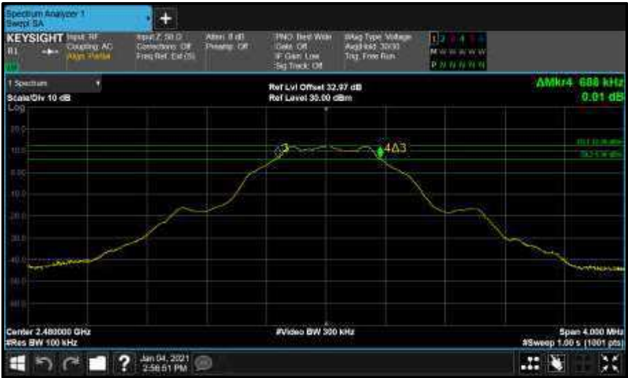
Figure 42 - Core0 (C) 2480 MHz (CH39) 6 dB Bandwidth
