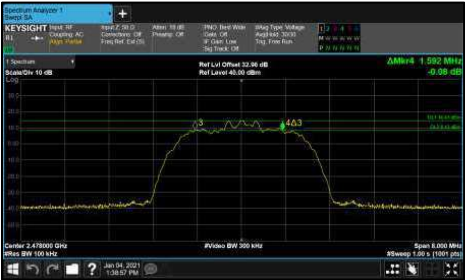
Figure 6 - Core0 (C) 247.8 MHz (CH76) 6 dB Bandwidth
