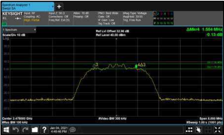
Figure 24 - Core0 (C) 2478 MHz (CH76) 6 dB Bandwidth
