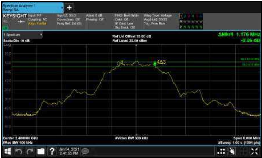
Figure 132 - Core2 (A) 2480 MHz (CH39) 6 dB Bandwidth
