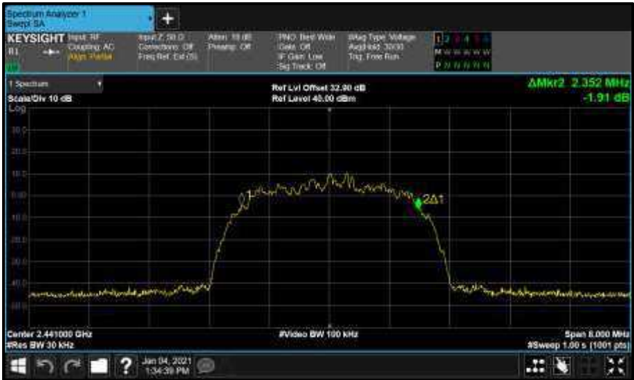
Figure 3 - Core0 (C) 2441 MHz (CH39) 99 % Bandwidth
