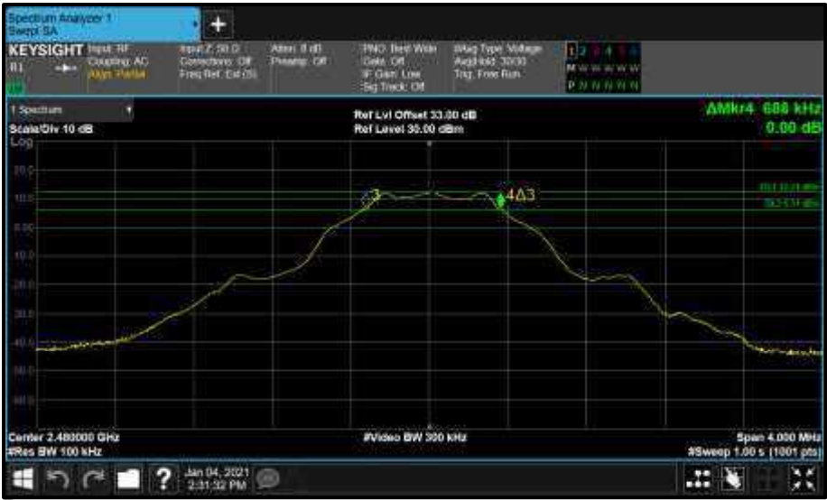
Figure 126 - Core2 (A) 2480 MHz (CH39) 6 dB Bandwidth
