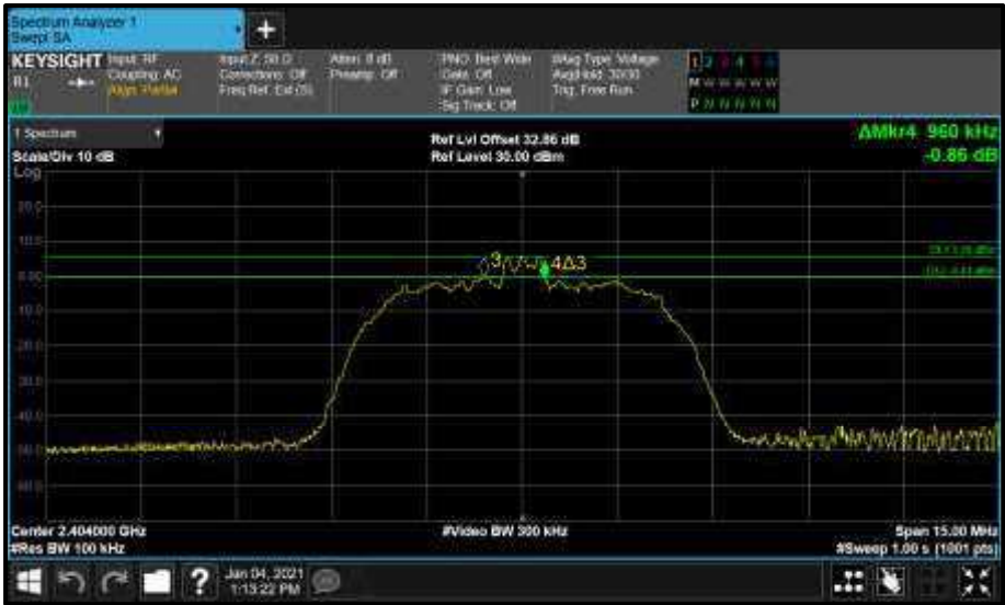
Figure 80 - Core2 (A) 2404 MHz (CH2) 6 dB Bandwidth
