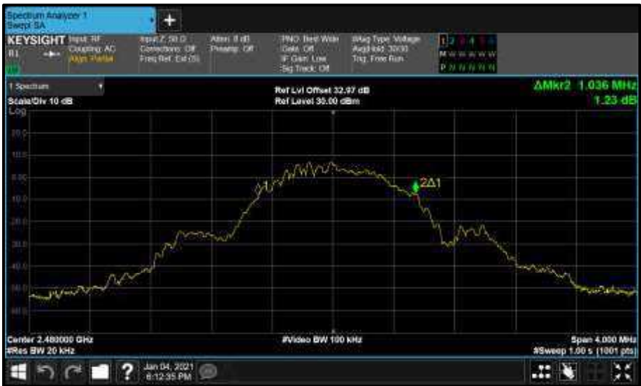
Figure 59 - Core0 (C) 2480 MHz (CH39) 99% Bandwidth
