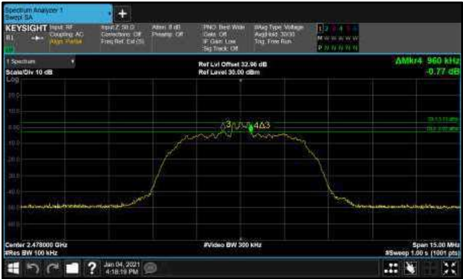
Figure 120 - Core0 (C) 2478 MHz (CH76) 6 dB Bandwidth
