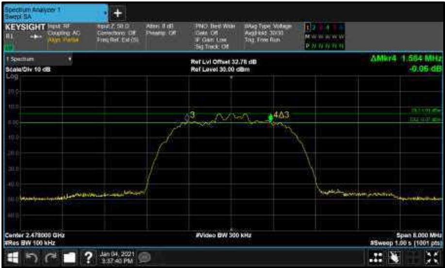
Figure 106 - Core1 (B) 24 78 MHz (CH76) 6 dB Bandwidth
