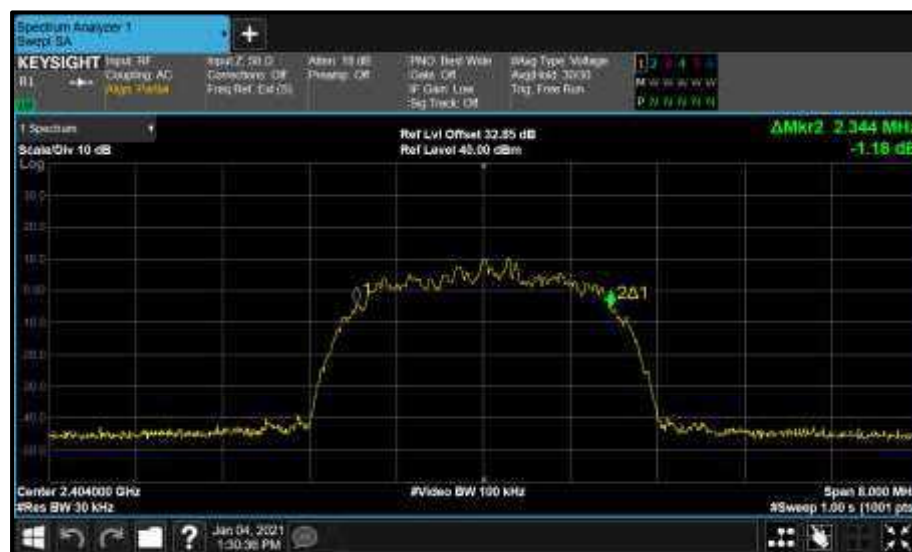
Figure 1 - Core0 (C) 2404 MHz (CH2) 99% Bandwidth
