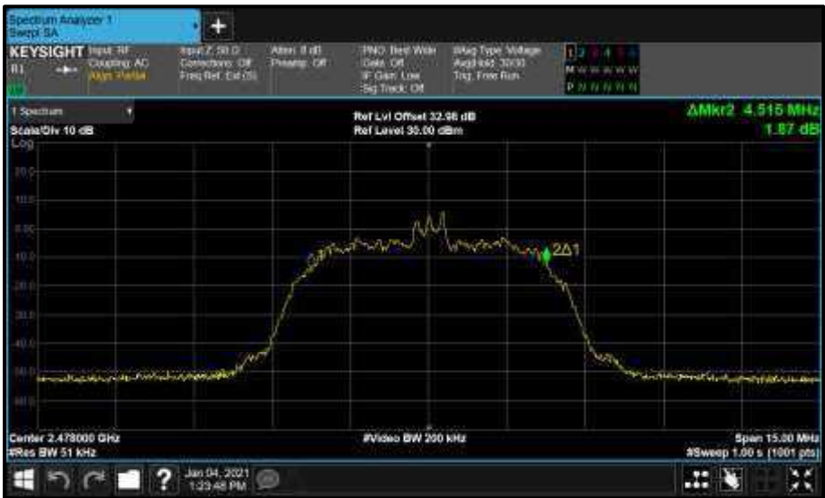
Figure 83 - Core2 (A) 2478 MHz (CH76) 99% Bandwidth
