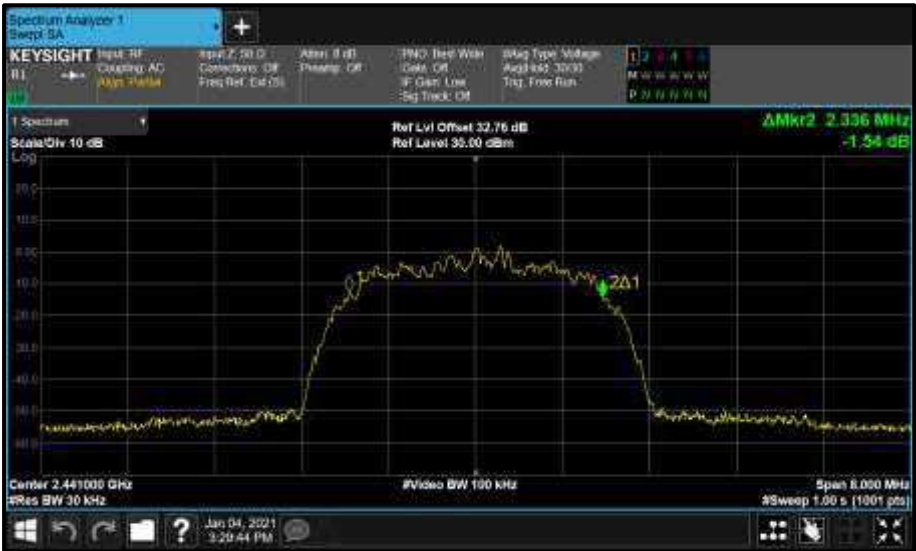
Figure 101 - Core1 (B) 2441 MHz (CH39) 99% Bandwidth
