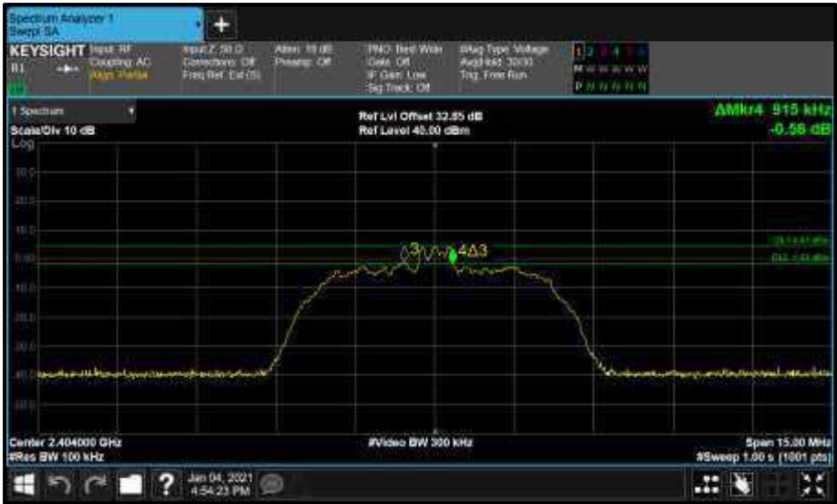
Figure 28 - Core0 (C) 2404 MHz (CH2) 6 dB Bandwidth
