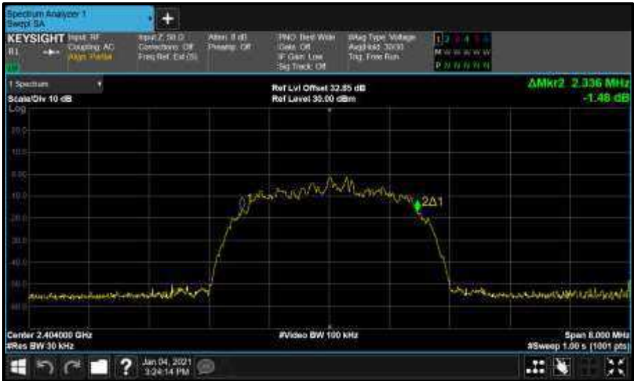
Figure 99 - Core0 (C) 2404 MHz (CH2) 99% Bandwidth
