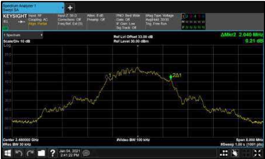
Figure 131 - Core2 (A) 2480 MHz (CH39) 99% Bandwidth
