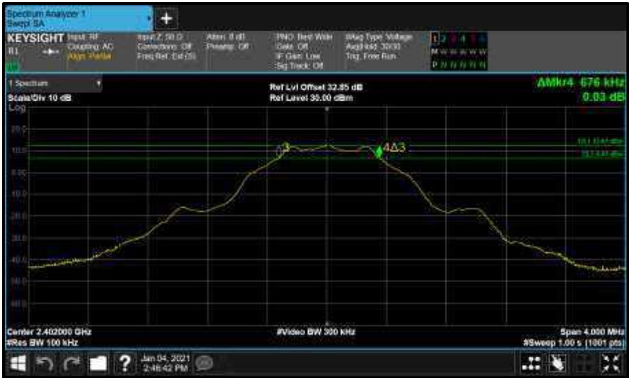
Figure 38 - Core0 (C) 2402 MHz (CH0) 6 dB Bandwidth
