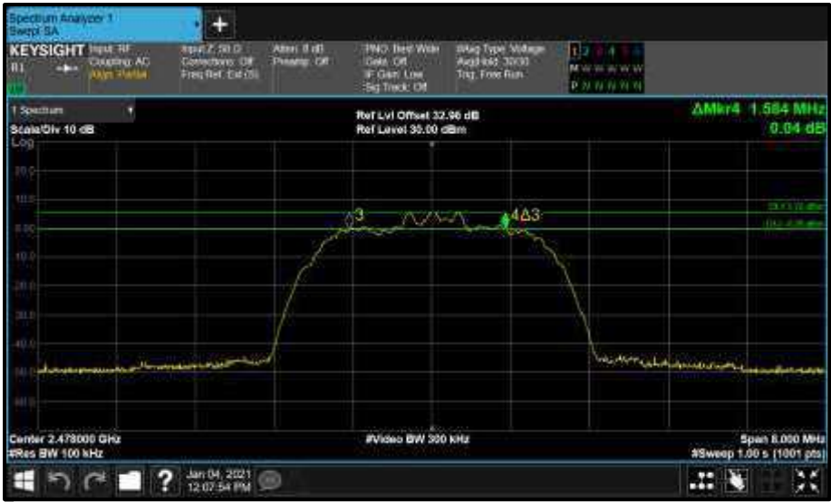
Figure 90 - Core0 (C) 2478 MHz (CH76) 6 dB Bandwidth
