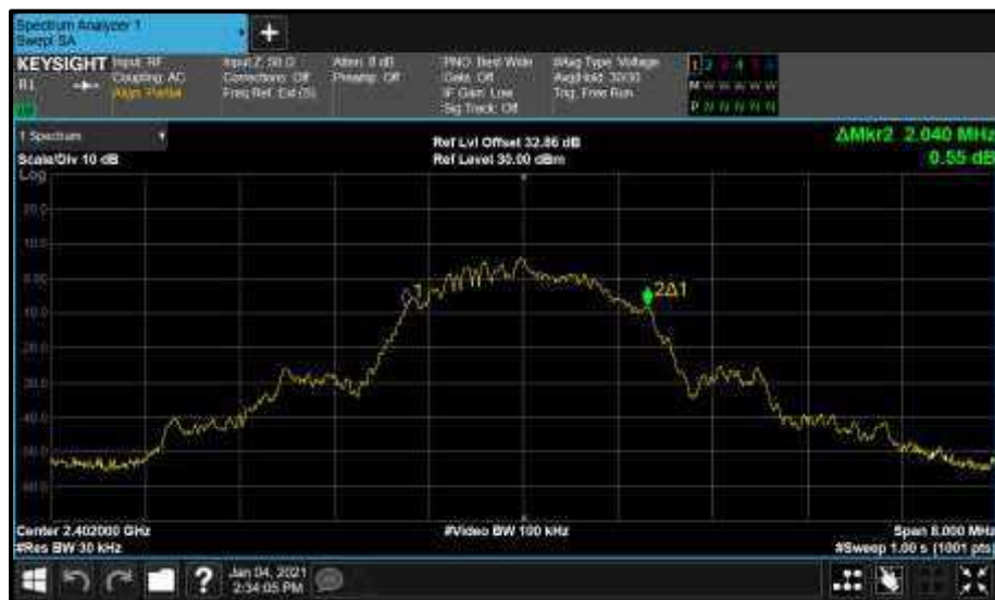
Figure 127 - Core2 (A) 2402 MHz (CH0) 99% Bandwidth
