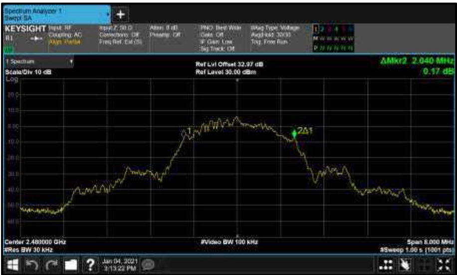
Figure 47 - Core0 (C) 2480 MHz (CH39) 99% Bandwidth
