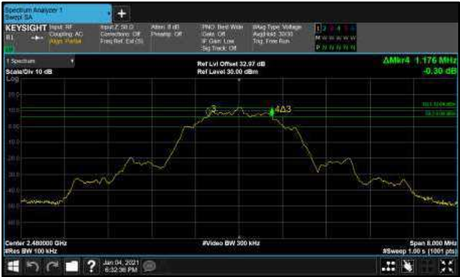
Figure 72 - Core0 (C) 2480 MHz (CH39) 6 dB Bandwidth
