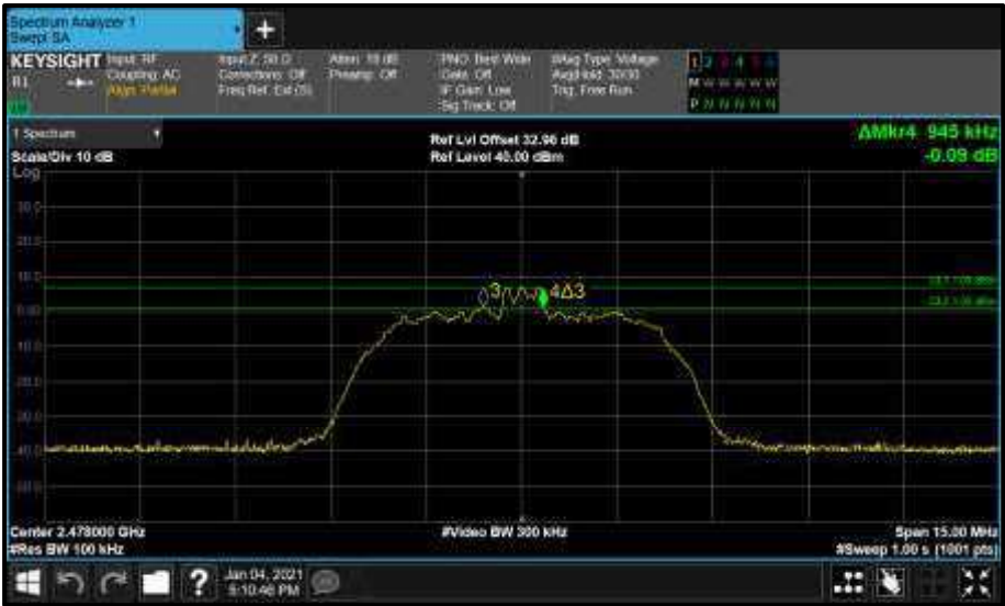
Figure 36 - Core0 (C) 2478 MHz (CH76) 6 dB Bandwidth
