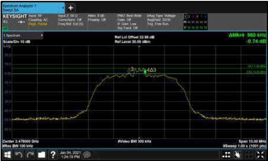
Figure 84 - Core2 (A) 2478 MHz (CH76) 6 dB Bandwidth
