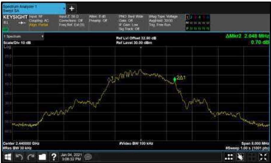
Figure 45 - Core0 (C) 2440 MHz (CH19) 99% Bandwidth
