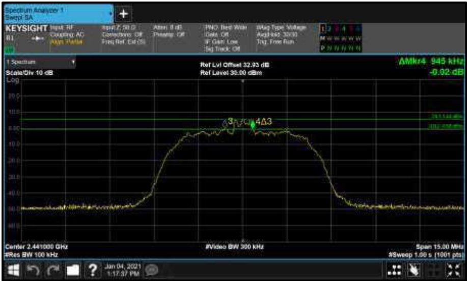
Figure 82 - Core2 (A) 2441 MHz (CH39) 6 dB Bandwidth
