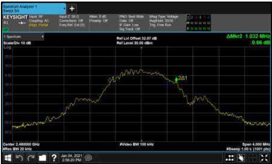
Figure 41 - Core0 (C) 2480 MHz (CH39) 99% Bandwidth
