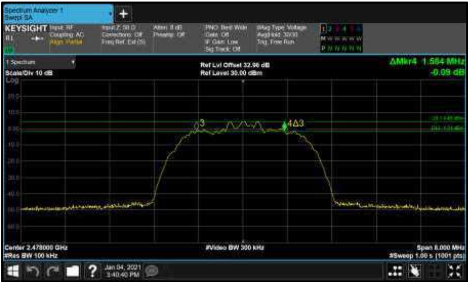
Figure 108 - Core0 (C) 2478 MHz (CH76) 6 dB Bandwidth
