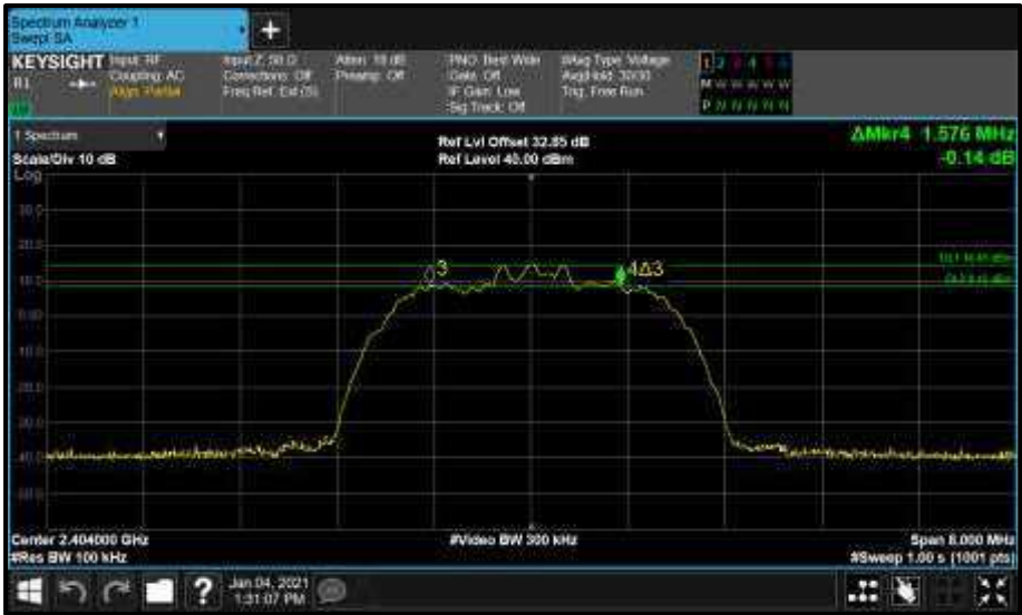
Figure 2 - Core0 (C) 2404 MHz (CH2) 6 d B Bandwidth
