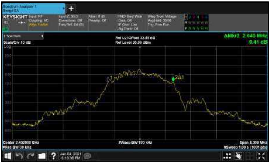
Figure 63 - Core0 (C) 2402 MHz (CH0) 99% Bandwidth
