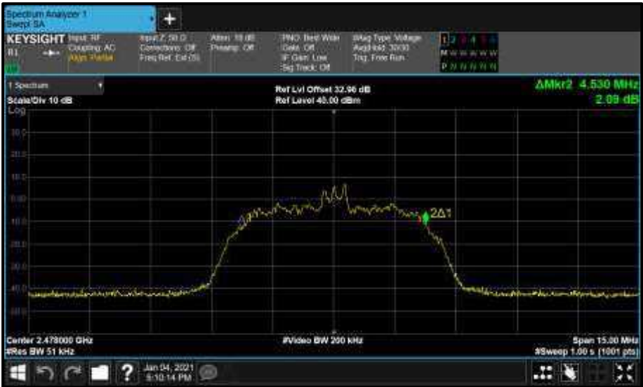
Figure 35 - Core0 (C) 2478 MHz (CH76) 99% Bandwidth
