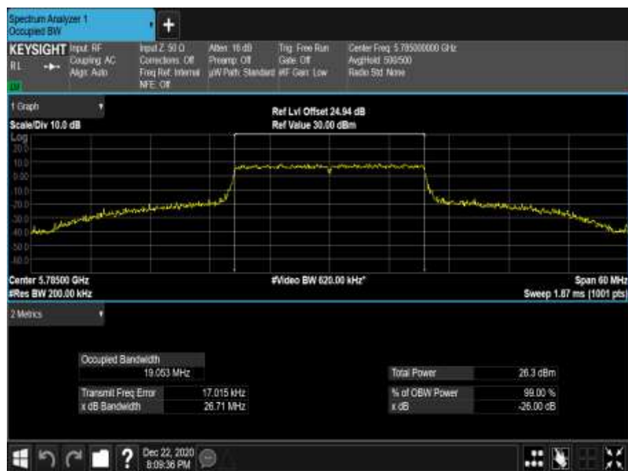
Figure 681 - 5785 MHz - 99% Occupied Bandwidth
