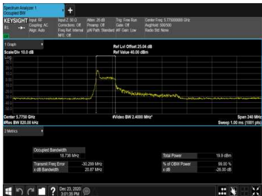
Figure 888 - 5775 MHz - 99% Occupied Bandwidth
