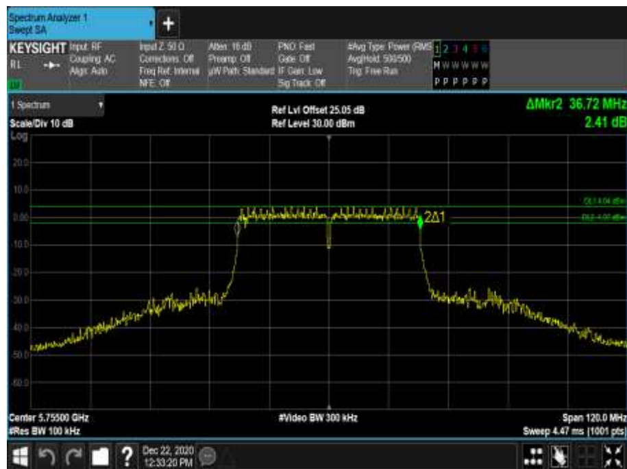
Figure 754 - 5755 MHz - 6 dB DTS Bandwidth
