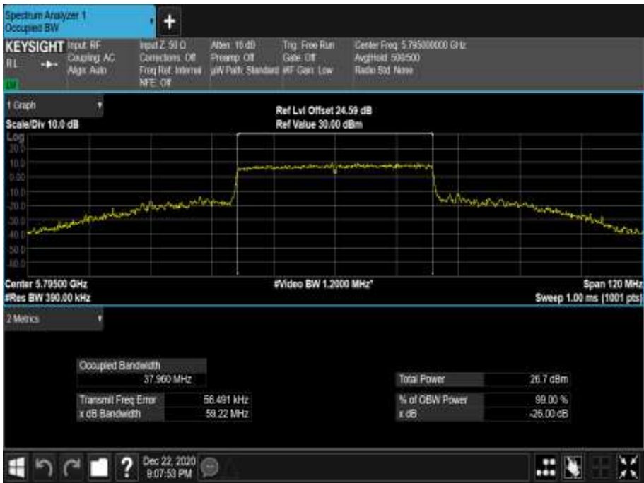
Figure 819 - 5795 MHz - 99% Occupied Bandwidth
