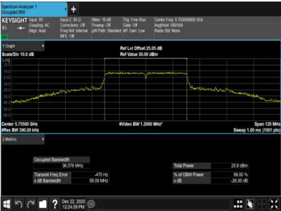
Figure 738 - 5755 MHz - 99% Occupied Bandwidth
