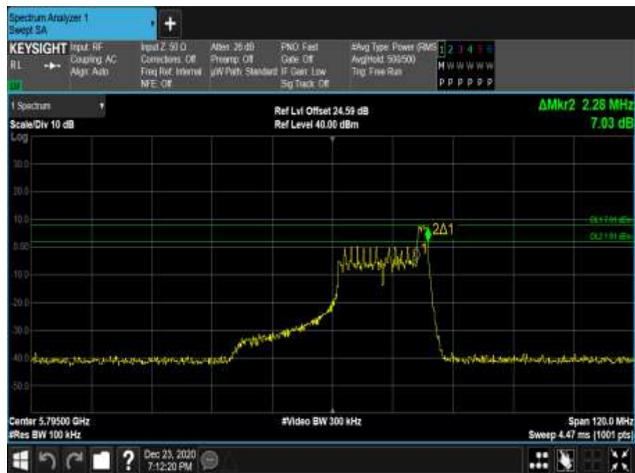
Figure 808 - 5795 MHz - 6 dB DTS Bandwidth
