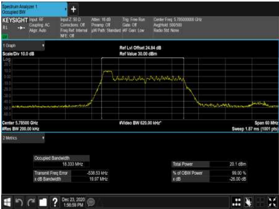
Figure 720 - 5785 MHz - 99% Occupied Bandwidth
