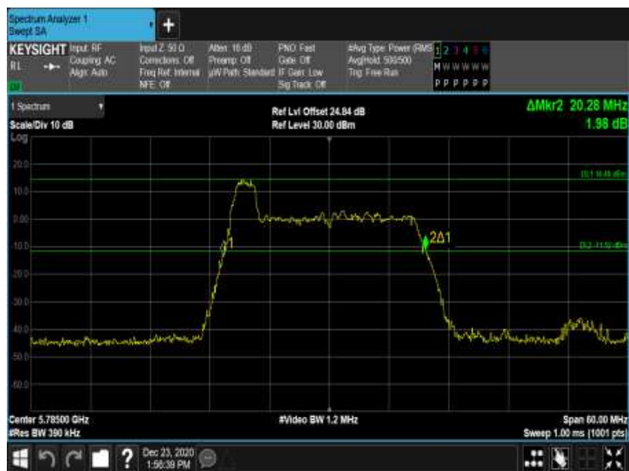
Figure 719 - 5785 MHz - 26 dB Emission Bandwidth
