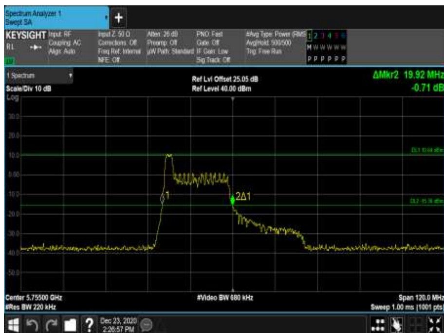
Figure 821 - 5755 MHz - 26 dB Emission Bandwidth
