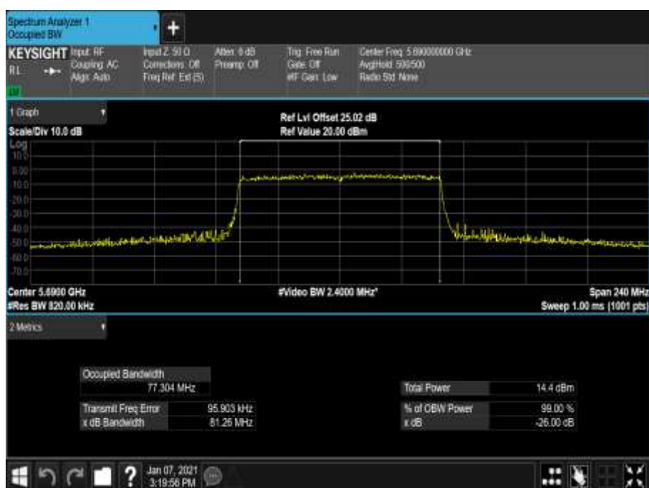
Figure 870 - 5690 MHz - 99% Occupied Bandwidth
