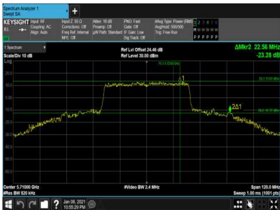
Figure 812 - 5710 MHz - 26 dB Emission Bandwidth
