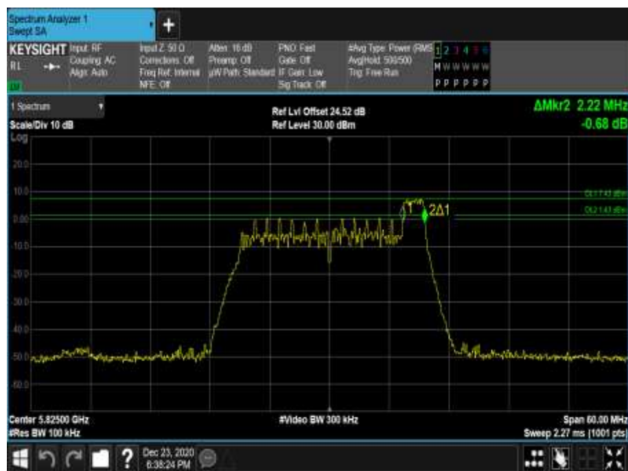
Figure 670 - 5825 MHz - 6 dB DTS Bandwidth
