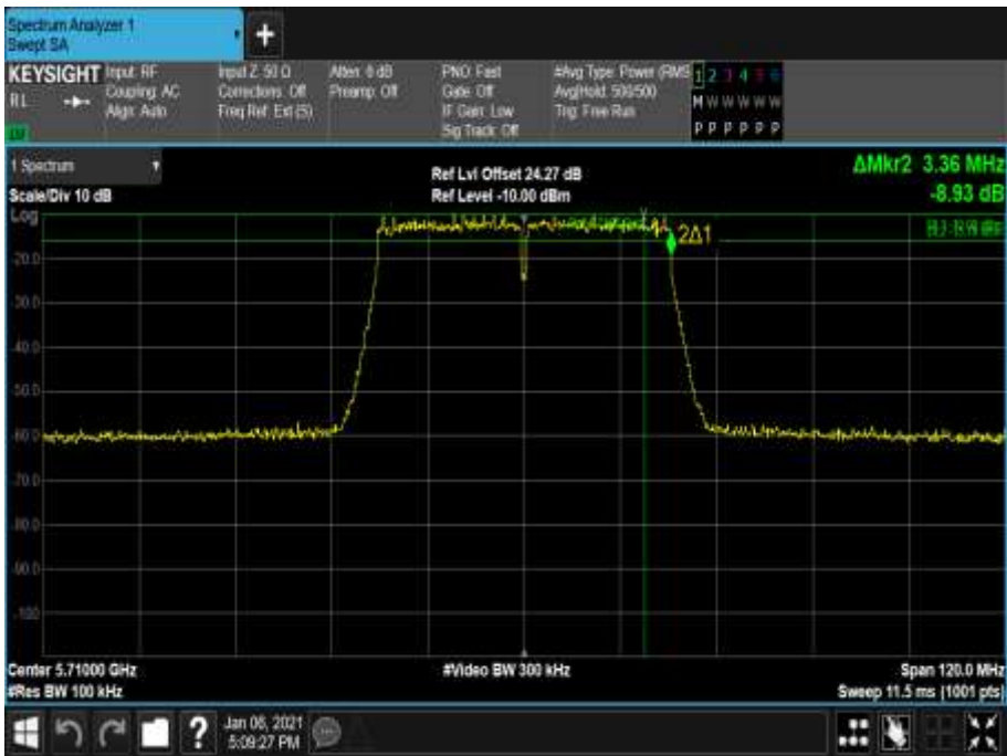
Figure 760 - 5710 MHz - 6 dB DTS Bandwidth
