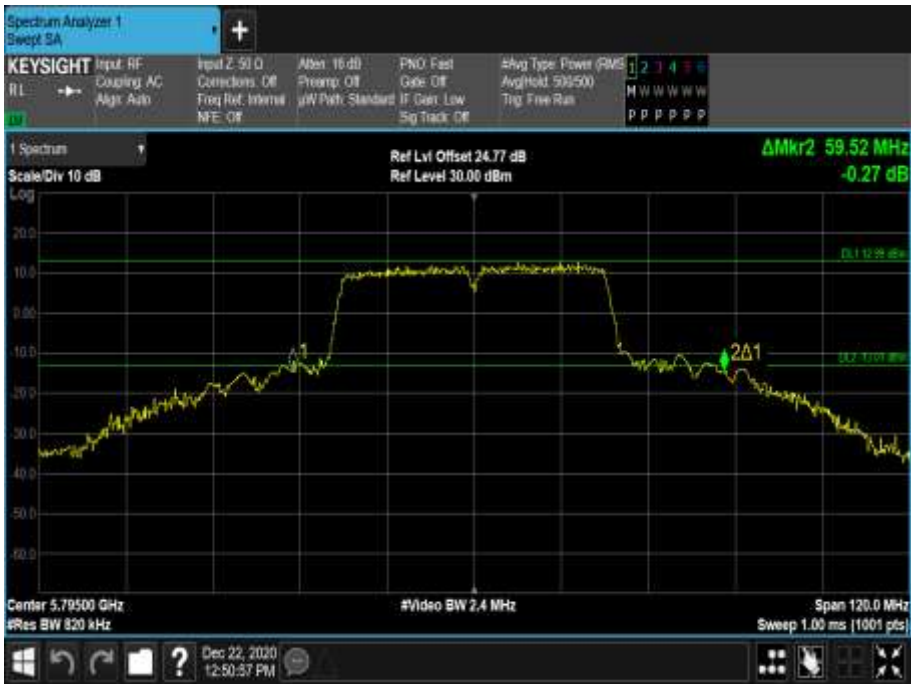
Figure 758 - 5795 MHz - 26 dB Emission Bandwidth
