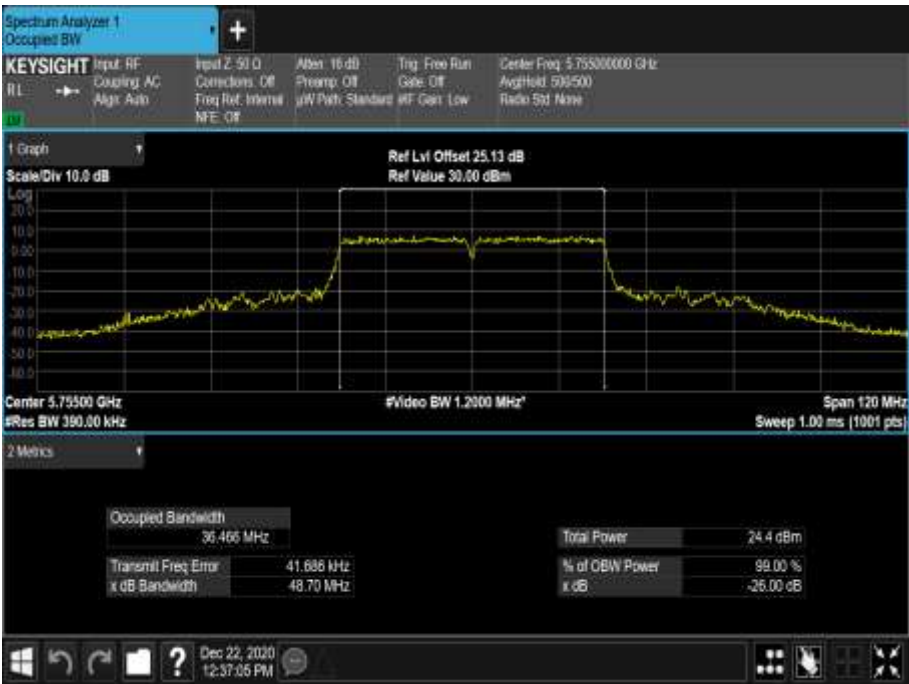
Figure 756 - 5755 MHz - 99% Occupied Bandwidth
