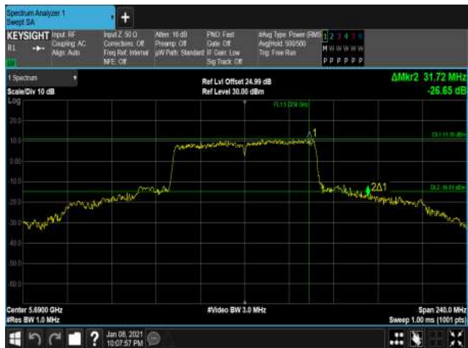
Figure 845 - 5690 MHz - 26 dB Emission Bandwidth
