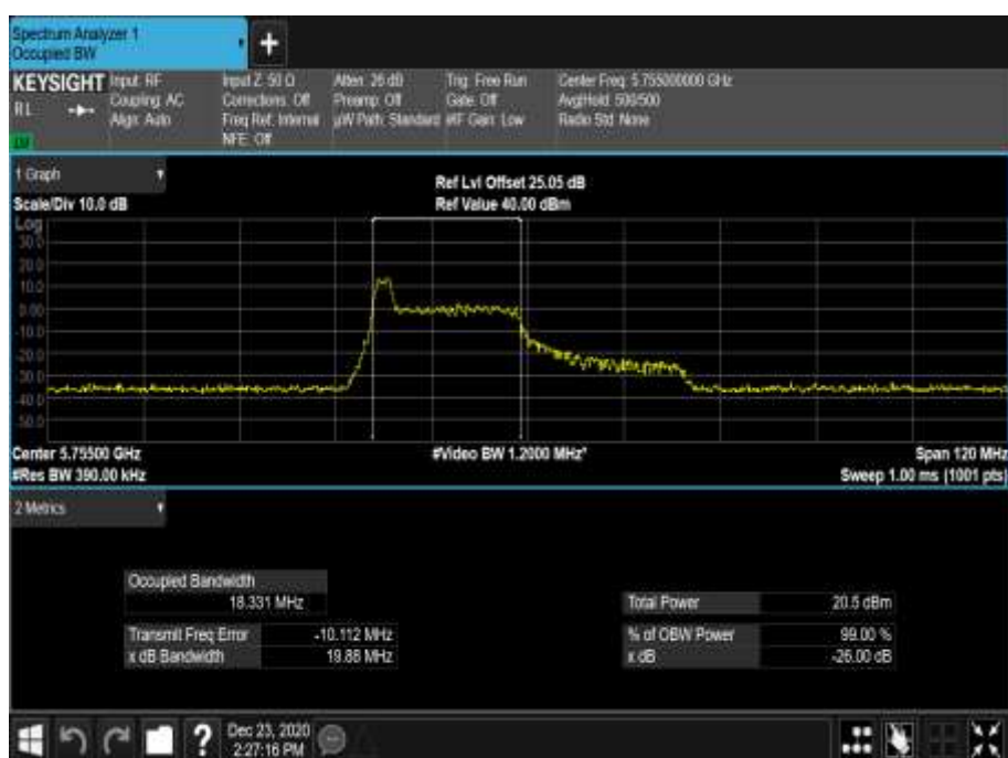
Figure 822 - 5755 MHz - 99% Occupied Bandwidth
