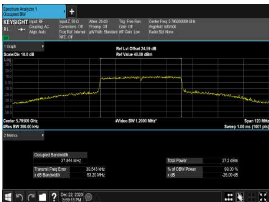
Figure 777 - 5795 MHz - 99% Occupied Bandwidth
