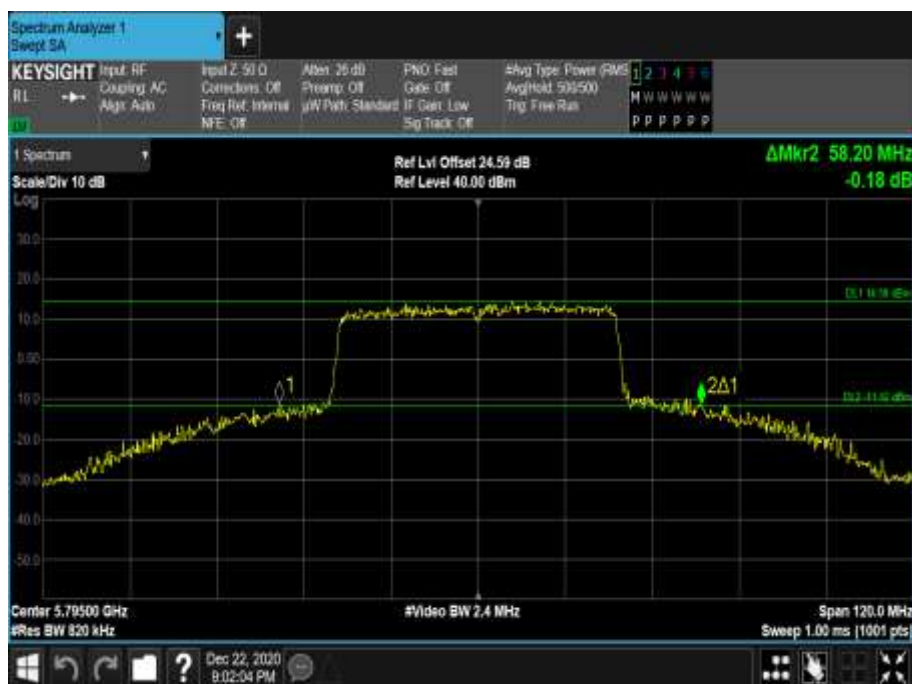
Figure 797 - 5795 MHz - 26 dB Emission Bandwidth
