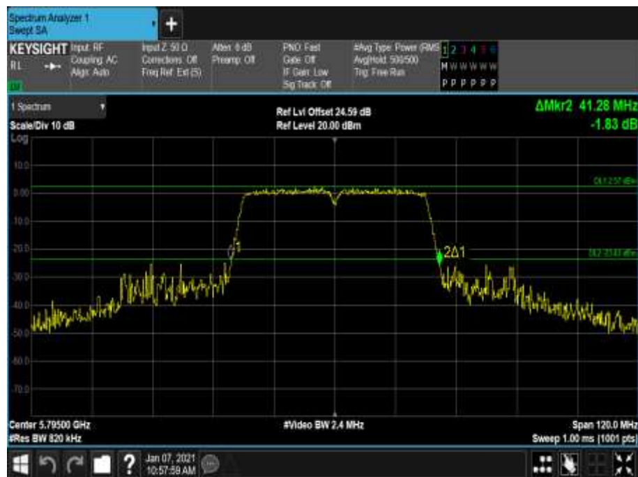
Figure 767 - 5795 MHz - 26 dB Emission Bandwidth
