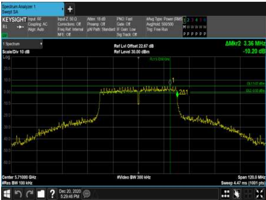
Figure 751 - 5710 MHz - 6 dB DTS Bandwidth
