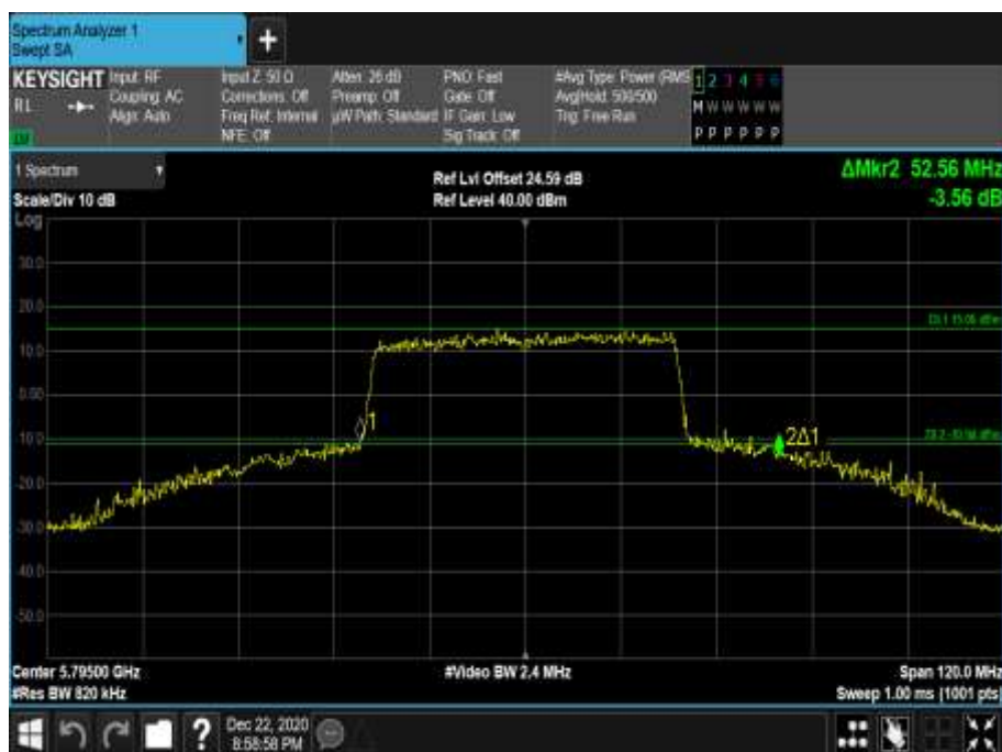
Figure 776 - 5795 MHz - 26 dB Emission Bandwidth
