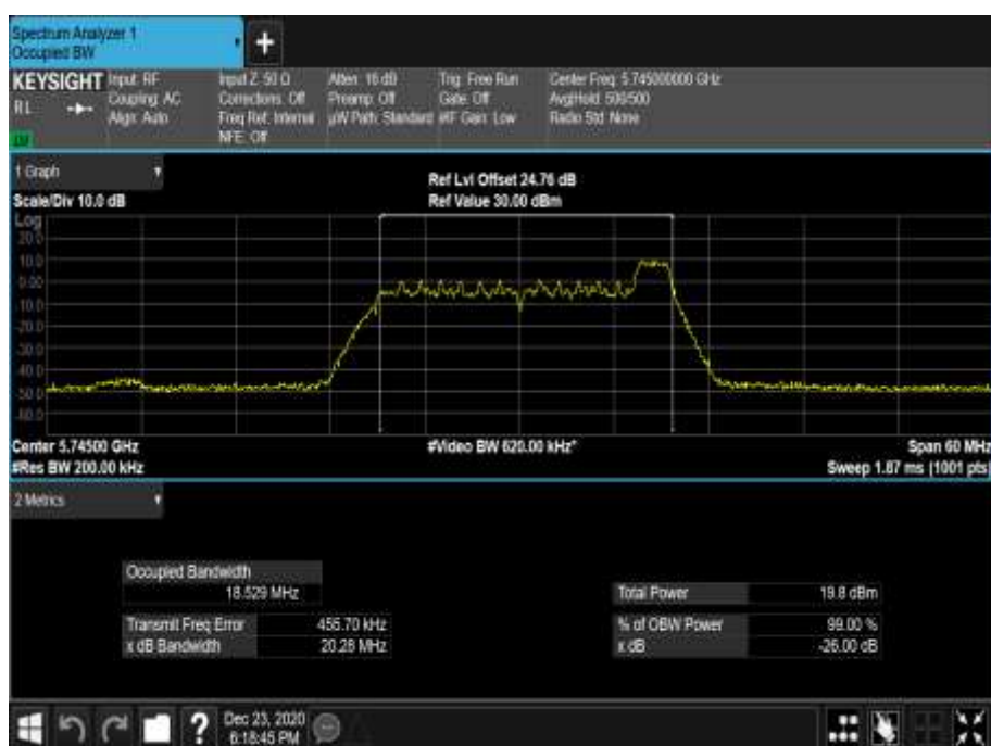
Figure 726 - 5745 MHz - 99% Occupied Bandwidth
