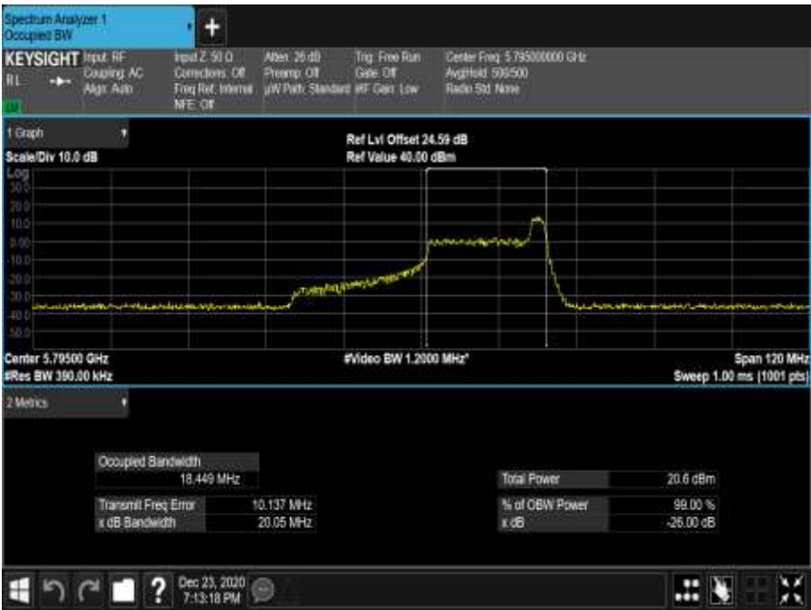
Figure 810 - 5795 MHz - 99% Occupied Bandwidth
