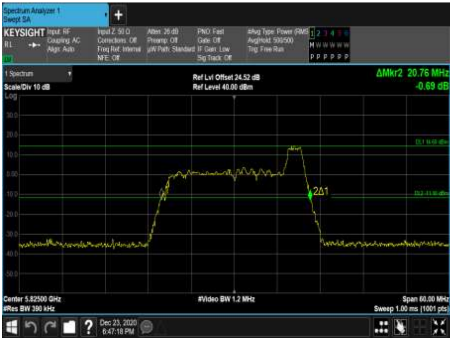
Figure 731 - 5825 MHz - 26 dB Emission Bandwidth
