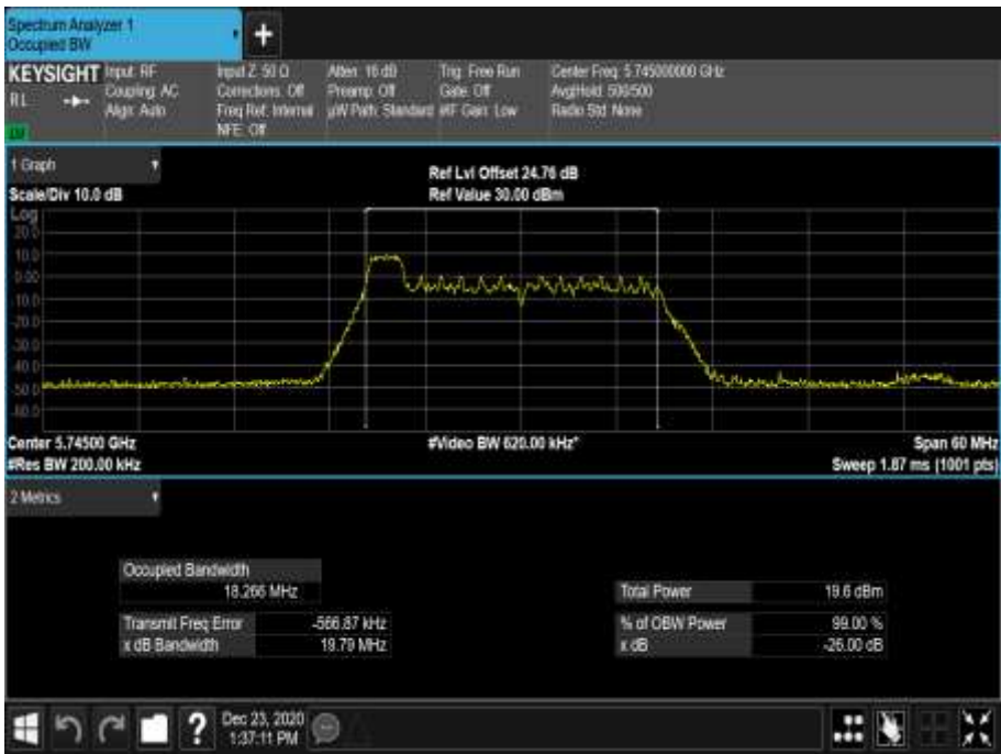
Figure 687 - 5745 MHz - 99% Occupied Bandwidth
