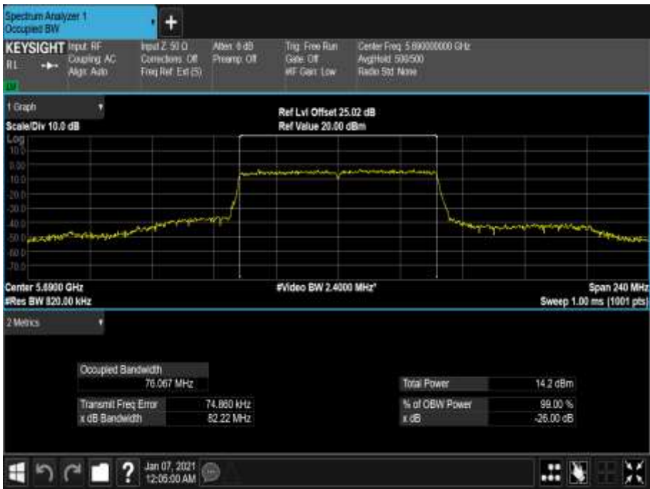
Figure 834 - 5690 MHz - 99% Occupied Bandwidth
