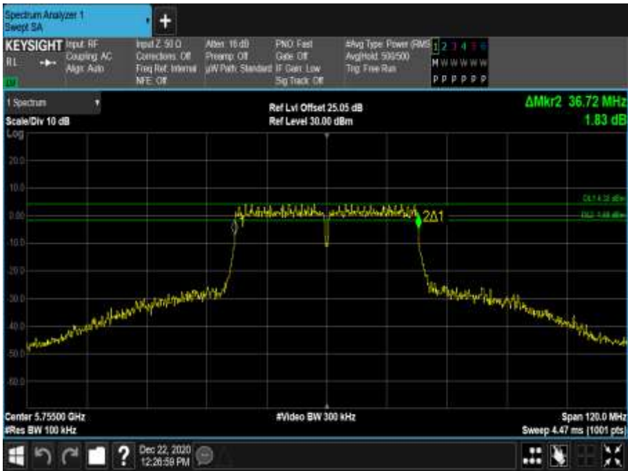
Figure 745 - 5755 MHz - 6 dB DTS Bandwidth
