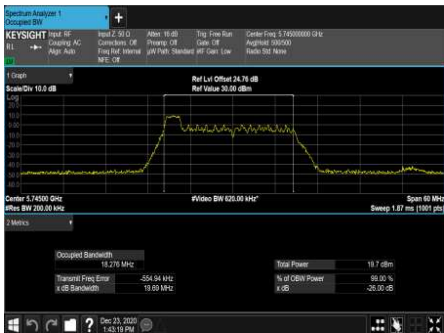
Figure 717 - 5745 MHz - 99% Occupied Bandwidth
