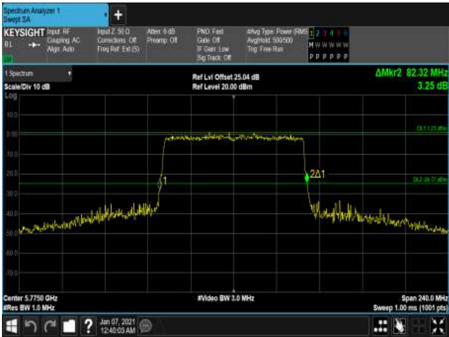
Figure 860 - 5775 MHz - 26 dB Emission Bandwidth
