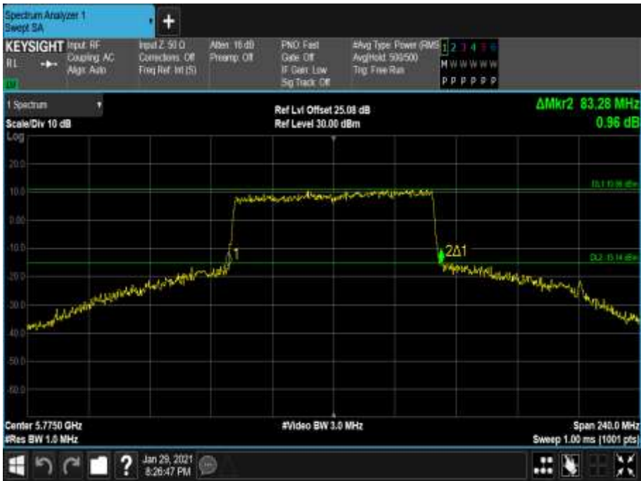
Figure 884 - 5775 MHz - 26 dB Emission Bandwidth
