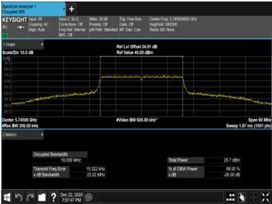
Figure 708 - 5745 MHz - 99% Occupied Bandwidth
