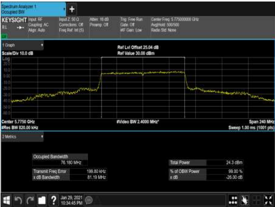
Figure 849 - 5775 MHz - 99% Occupied Bandwidth
