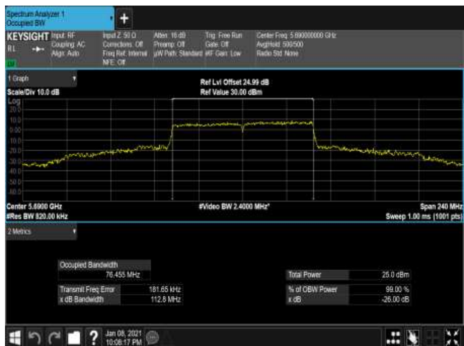
Figure 846 - 5690 MHz - 99% Occupied Bandwidth
