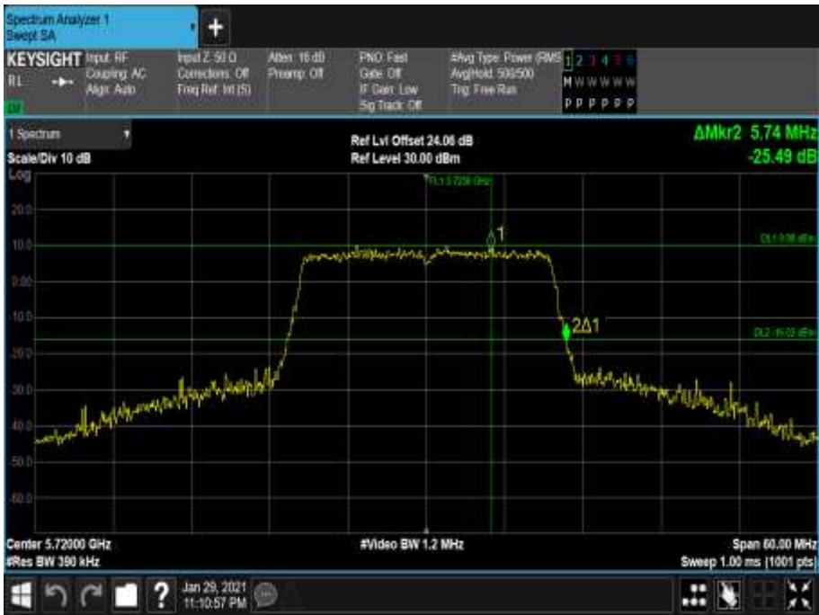
Figure 704 - 5720 MHz - 26 dB Emission Bandwidth
