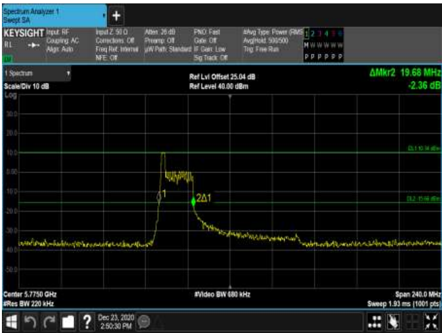
Figure 863 - 5775 MHz - 26 dB Emission Bandwidth
