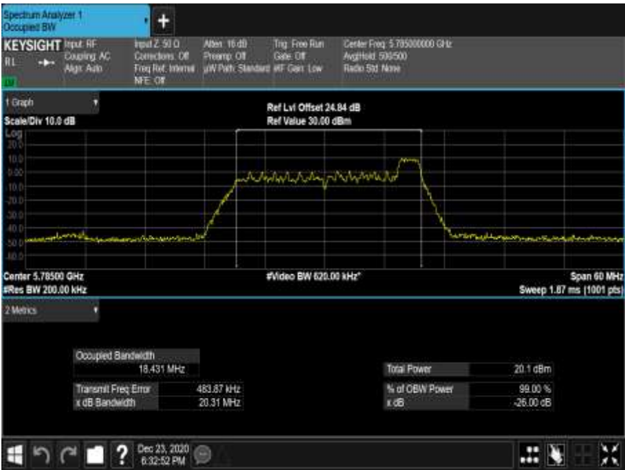
Figure 729 - 5785 MHz - 99% Occupied Bandwidth
