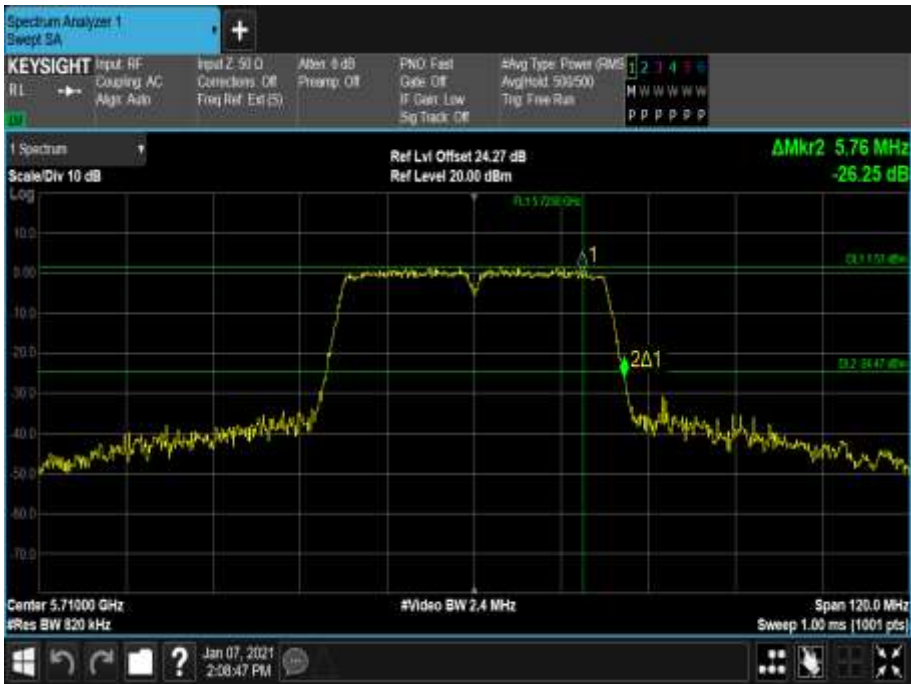
Figure 743 - 5710 MHz - 26 dB Emission Bandwidth
