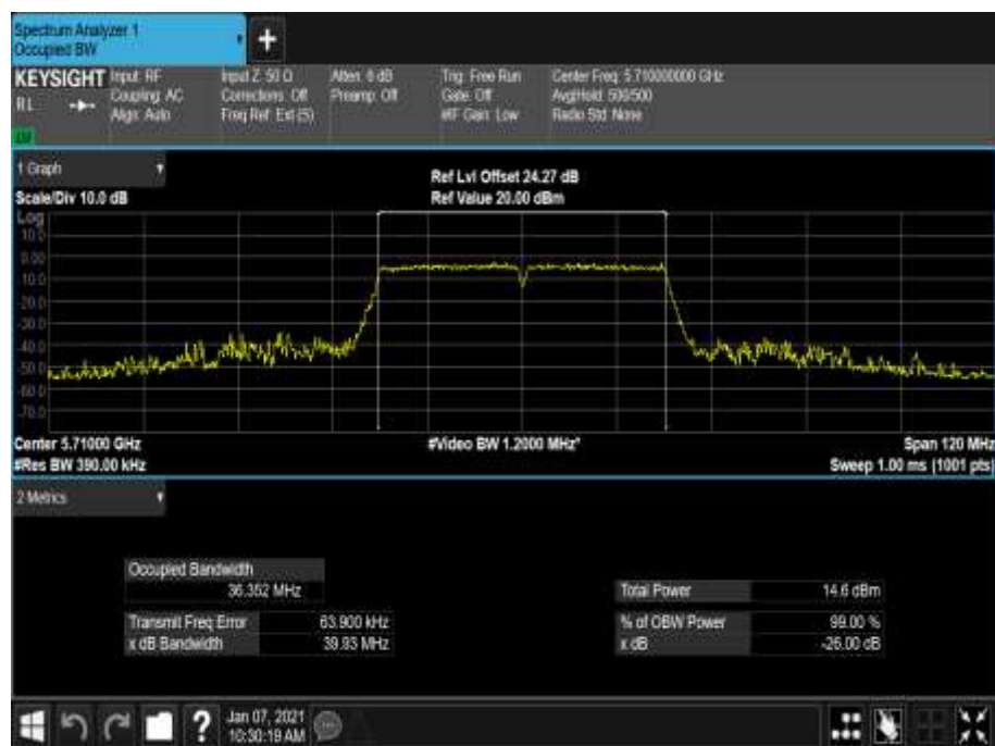
Figure 762 - 5710 MHz - 99% Occupied Bandwidth
