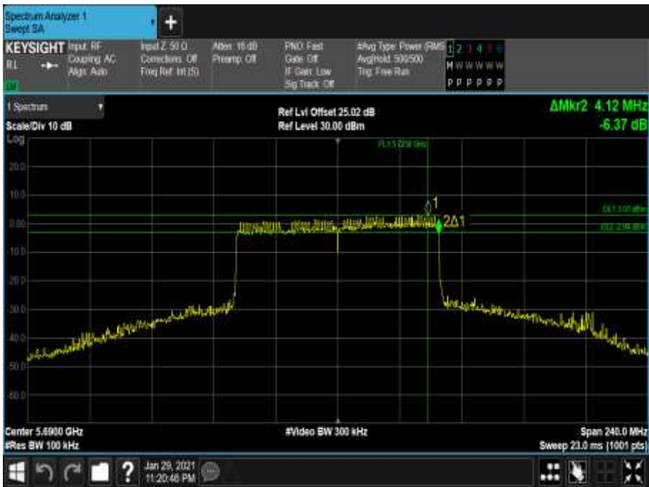
Figure 880 - 5690 MHz - 6 dB DTS Bandwidth
