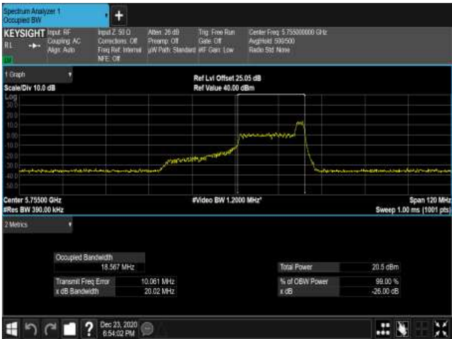
Figure 786 - 5755 MHz - 99% Occupied Bandwidth
