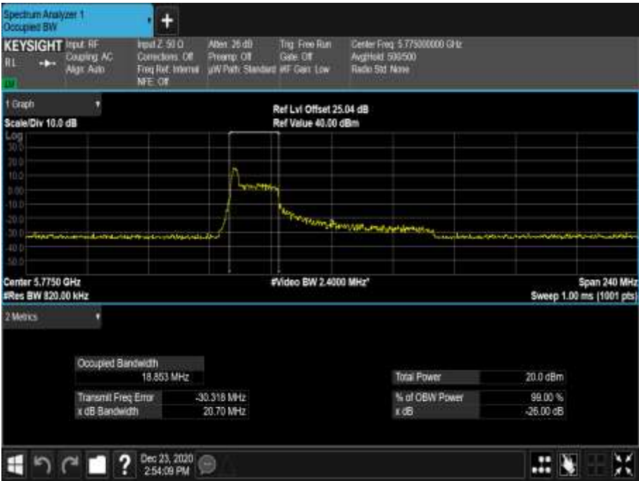
Figure 876 - 5775 MHz - 99% Occupied Bandwidth
