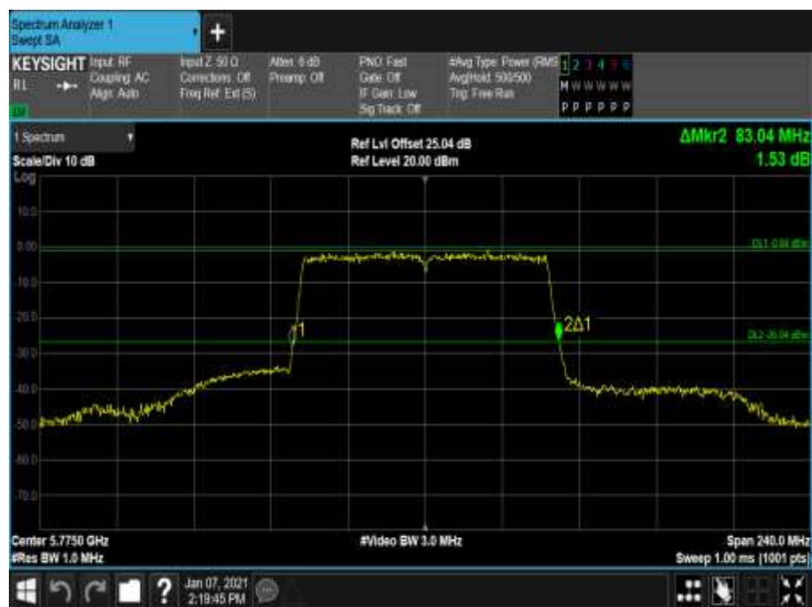
Figure 842 - 5775 MHz - 26 dB Emission Bandwidth
