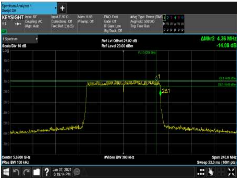
Figure 868 - 5690 MHz - 6 dB DTS Bandwidth
