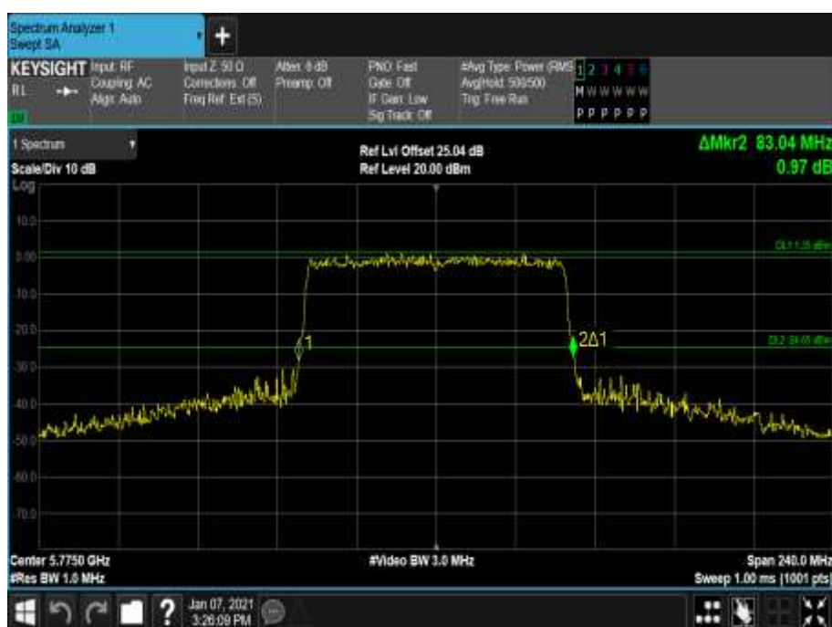
Figure 872 - 5775 MHz - 26 dB Emission Bandwidth
