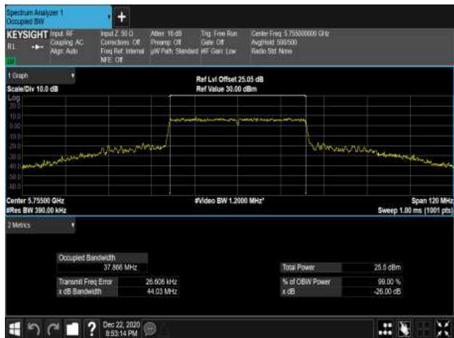
Figure 816 - 5755 MHz - 99% Occupied Bandwidth
