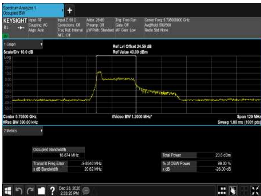
Figure 783 - 5795 MHz - 99% Occupied Bandwidth
