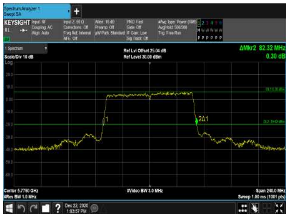
Figure 848 - 5775 MHz - 26 dB Emission Bandwidth
