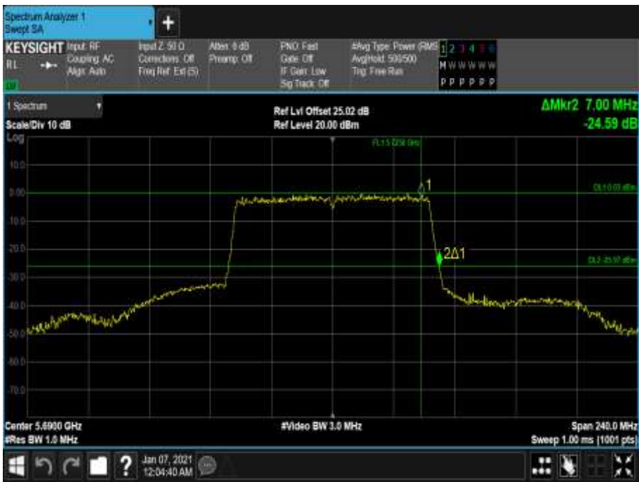
Figure 833 - 5690 MHz - 26 dB Emission Bandwidth
