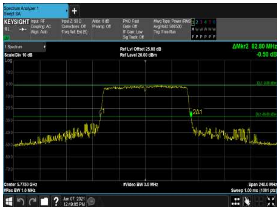
Figure 854 - 5775 MHz - 26 dB Emission Bandwidth
