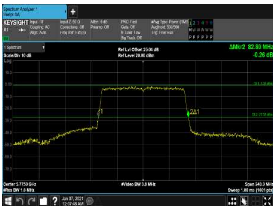
Figure 836 - 5775 MHz - 26 dB Emission Bandwidth
