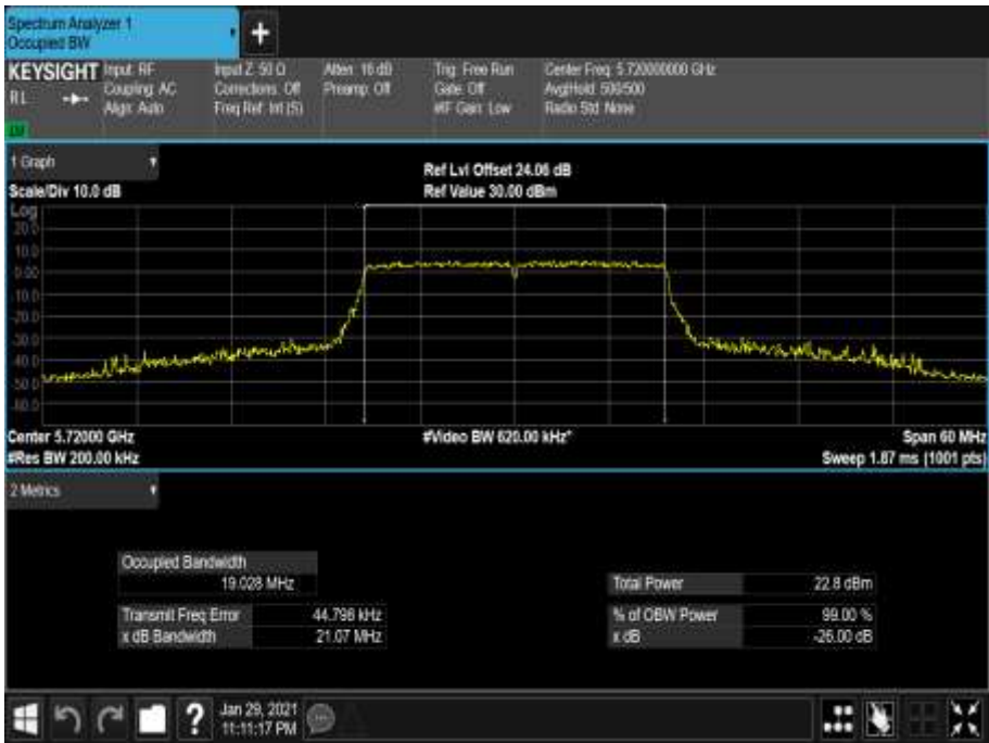
Figure 705 - 5720 MHz - 99% Occupied Bandwidth
