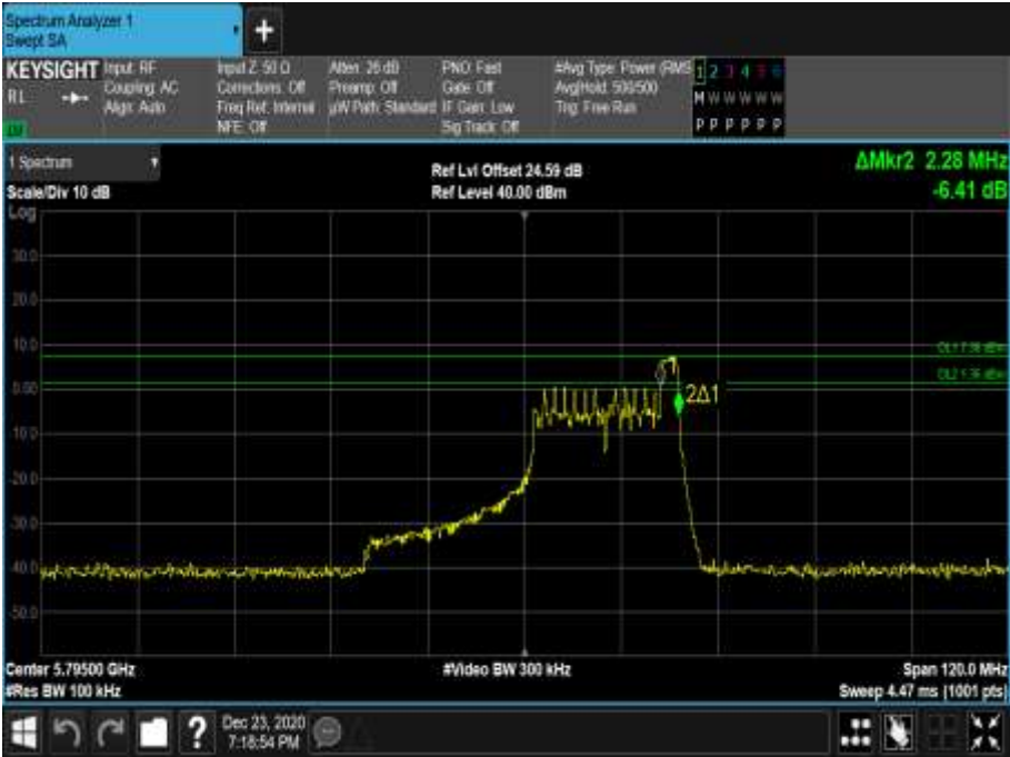
Figure 829 - 5795 MHz - 6 dB DTS Bandwidth
