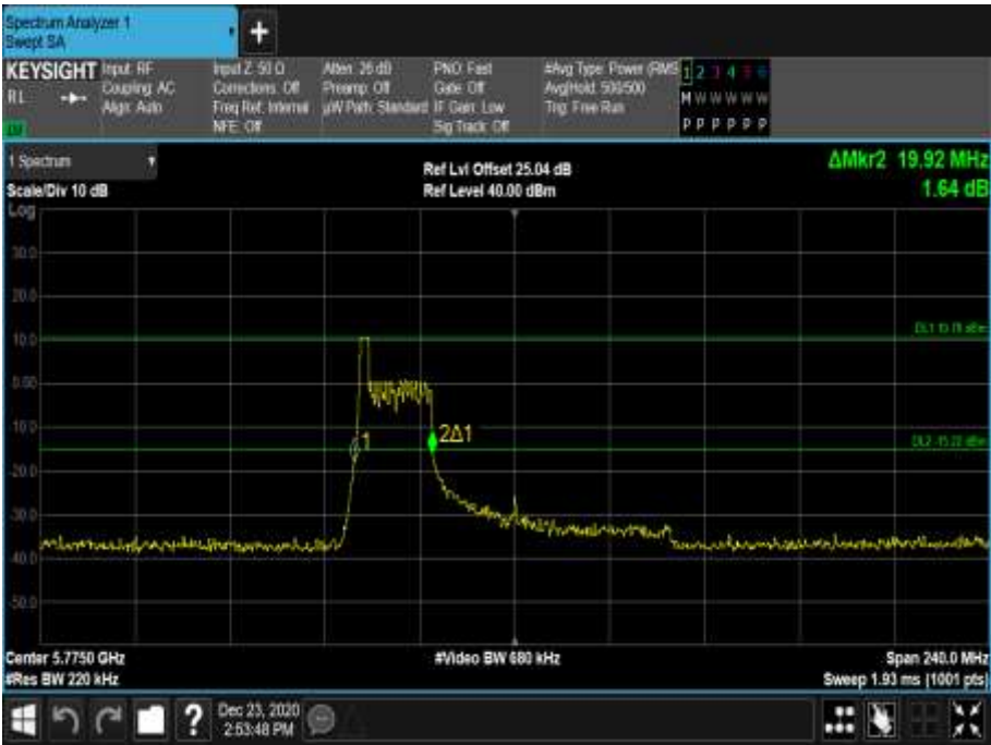
Figure 875 - 5775 MHz - 26 dB Emission Bandwidth
