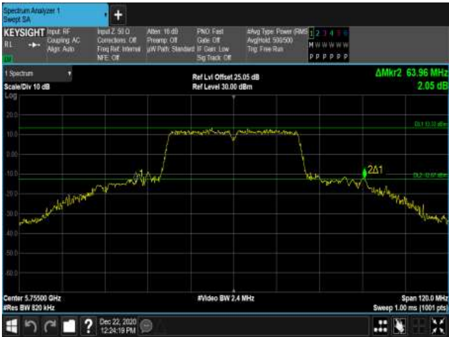
Figure 737 - 5755 MHz - 26 dB Emission Bandwidth
