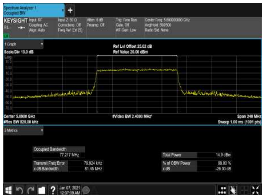
Figure 858 - 5690 MHz - 99% Occupied Bandwidth
