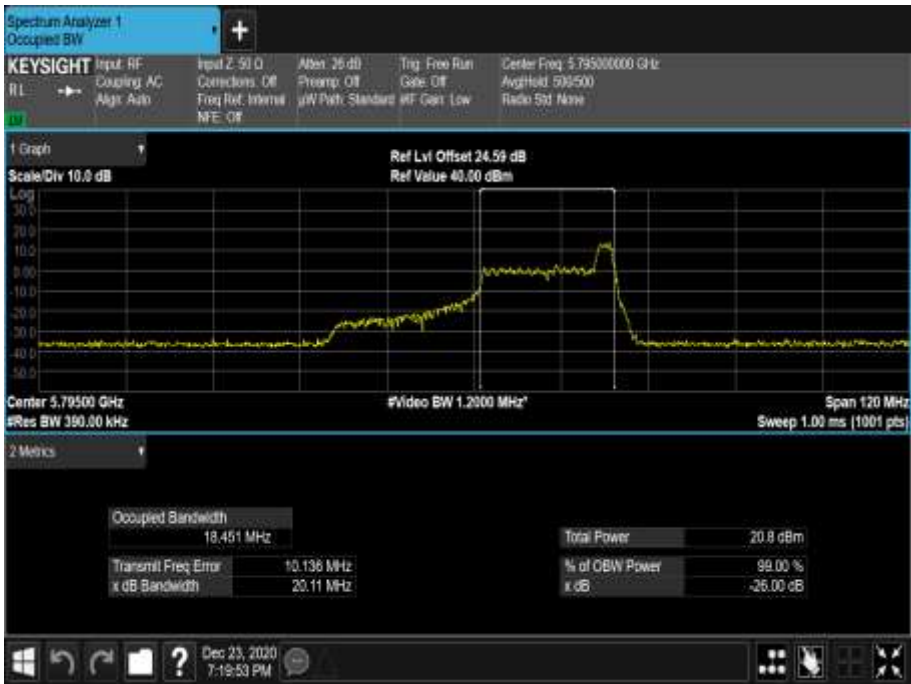
Figure 831 - 5795 MHz - 99% Occupied Bandwidth
