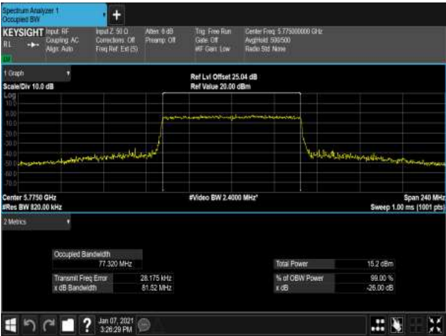
Figure 873 - 5775 MHz - 99% Occupied Bandwidth
