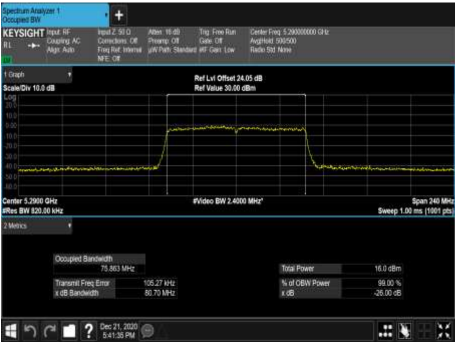
Figure 424 - 5290 MHz - 99% Occupied Bandwidth
