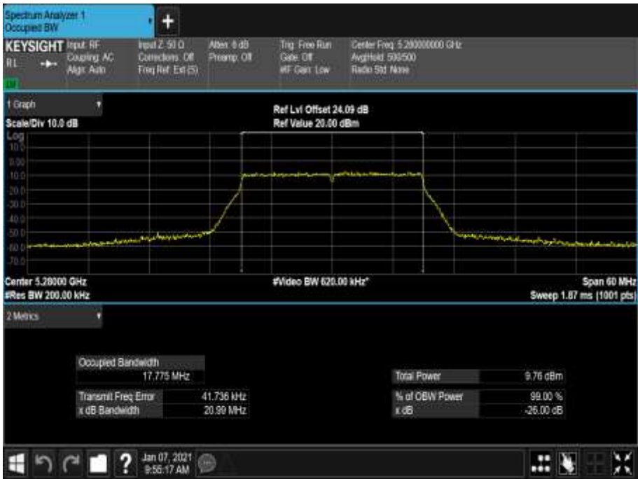
Figure 370 - 5280 MHz - 99% Occupied Bandwidth
