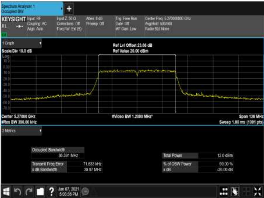
Figure 396 - 5270 MHz - 99% Occupied Bandwidth
