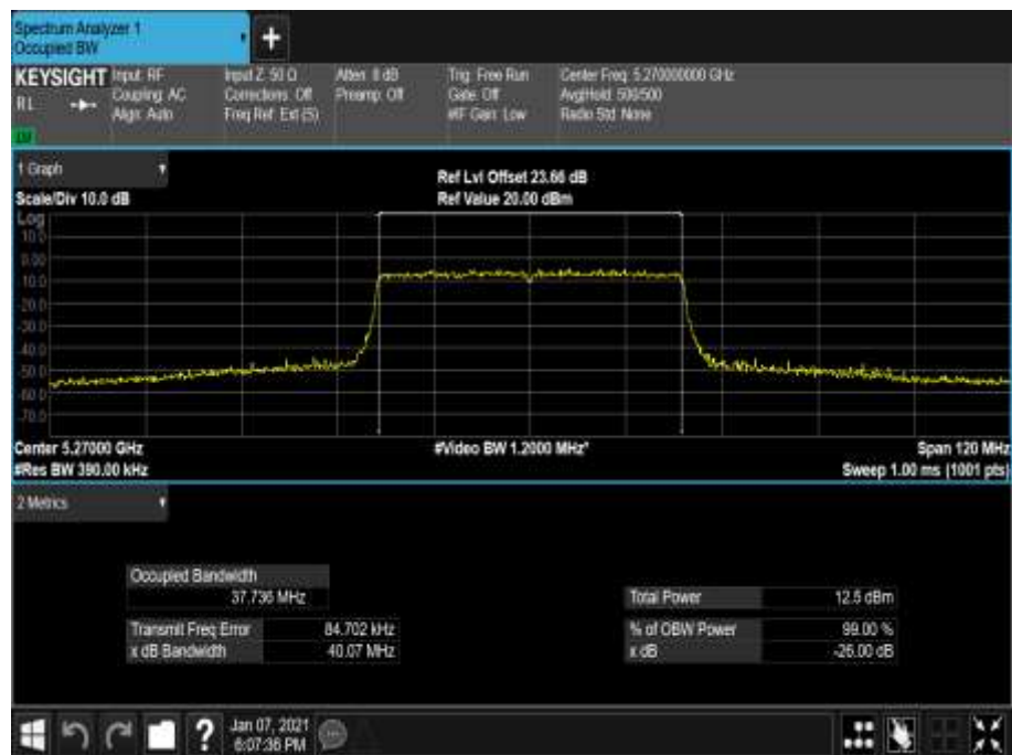
Figure 412 - 5270 MHz - 99% Occupied Bandwidth
