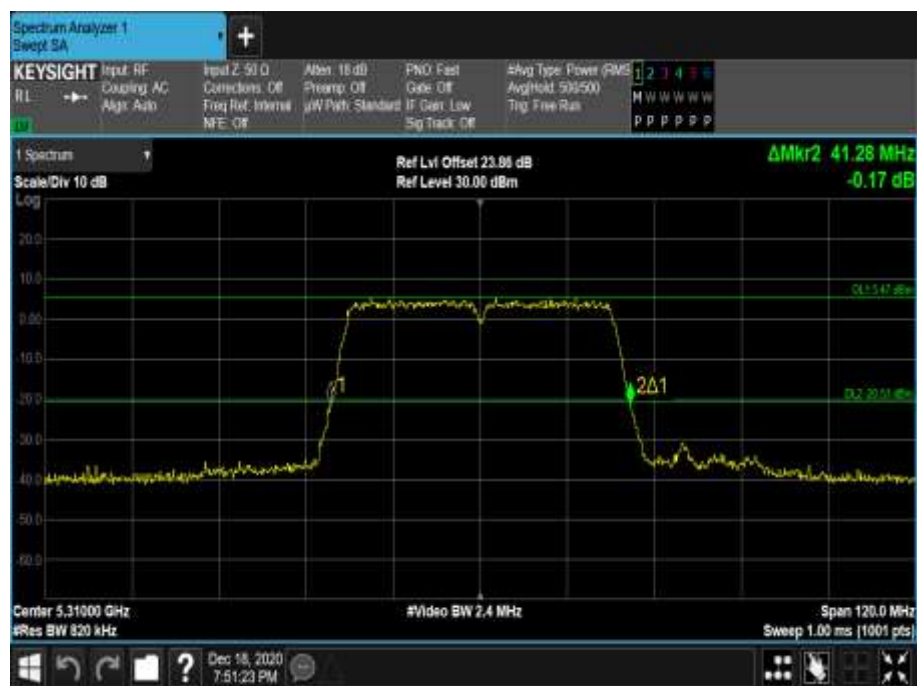
Figure 401 - 5310 MHz - 26 dB Emission Bandwidth
