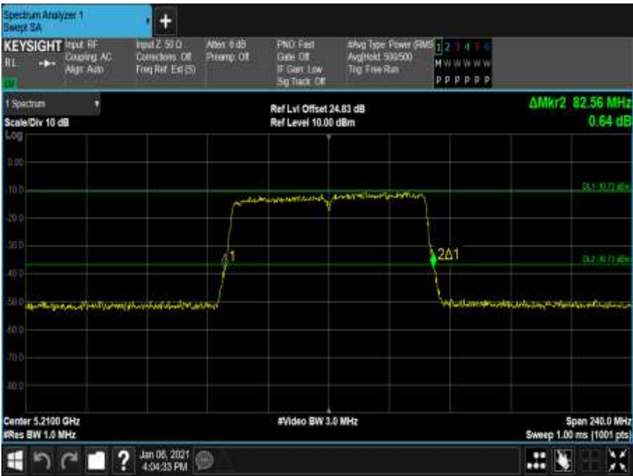
Figure 305 - 5210 MHz - 26 dB Emission Bandwidth
