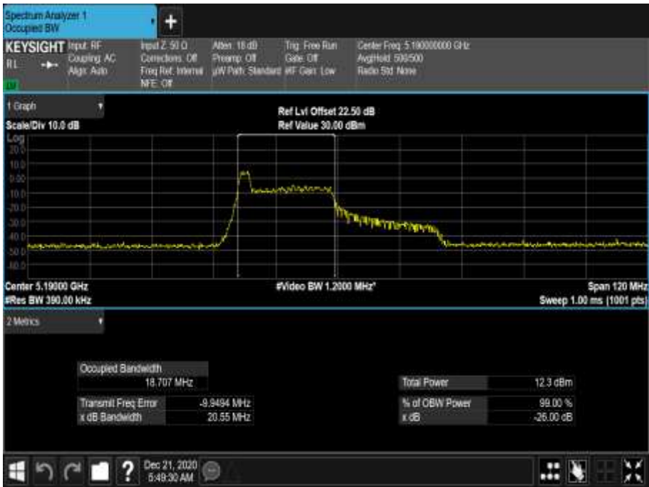
Figure 232 - 5190 MHz - 99% Occupied Bandwidth
