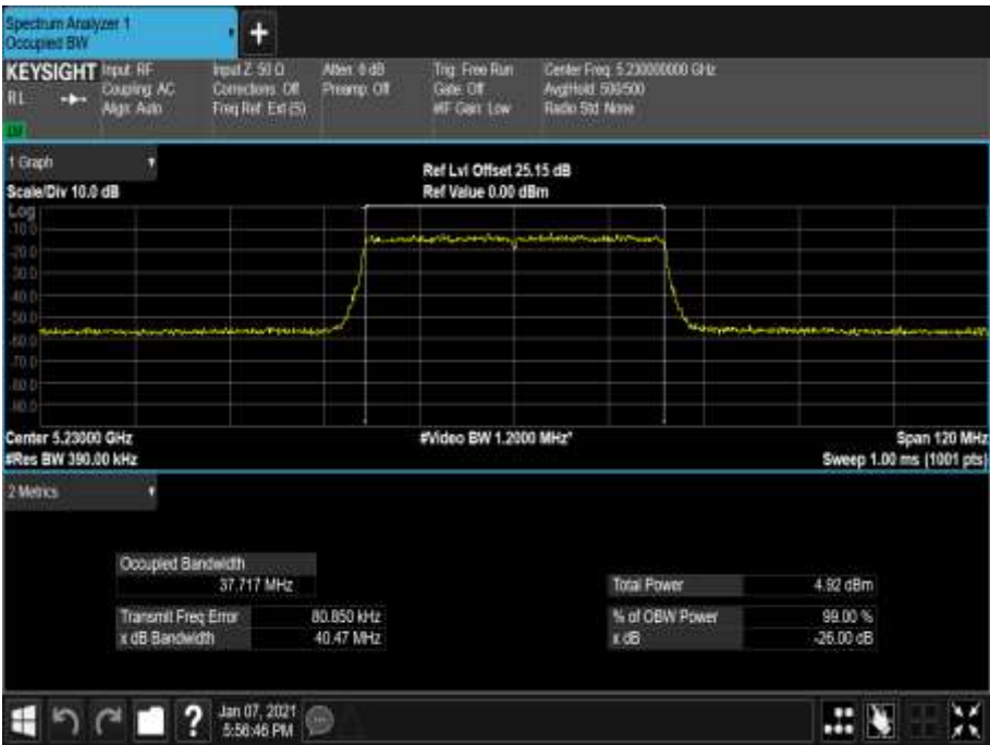
Figure 250 - 5230 MHz - 99% Occupied Bandwidth
