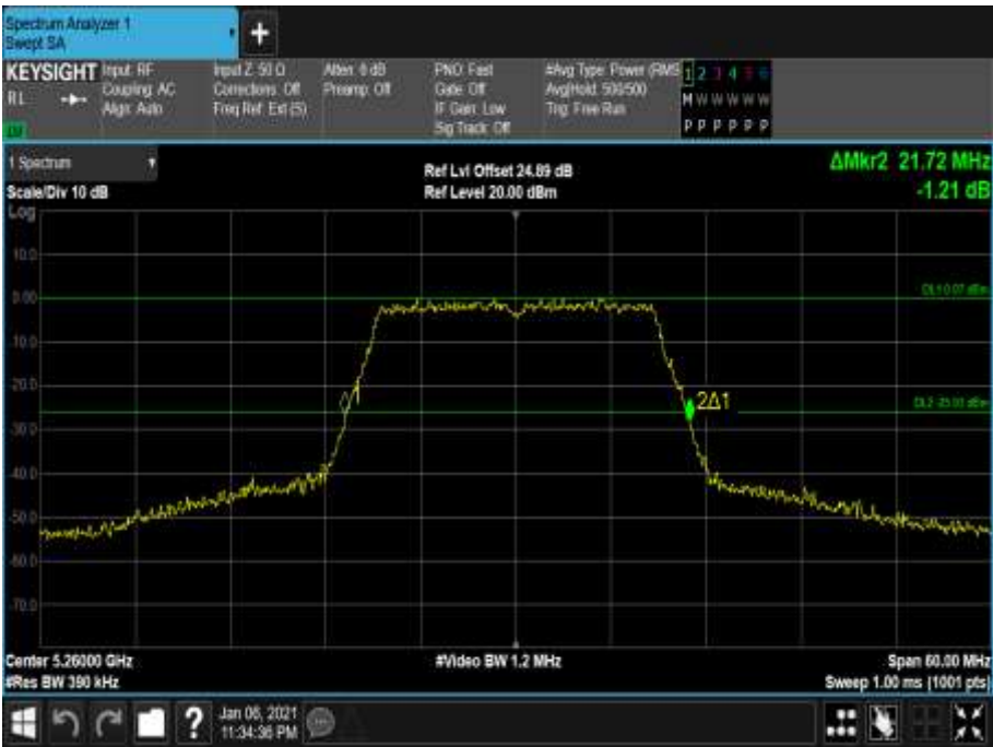
Figure 349 - 5260 MHz - 26 dB Emission Bandwidth
