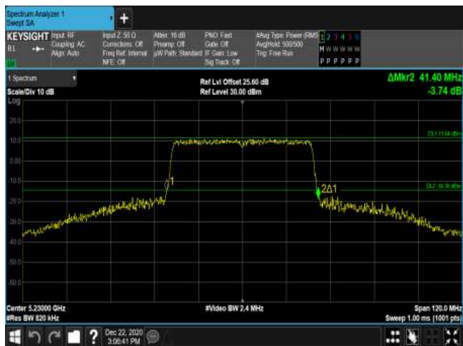
Figure 221 - 5230 MHz - 26 dB Emission Bandwidth
