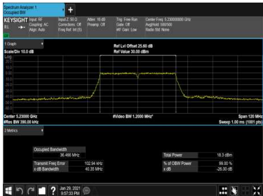
Figure 210 - 5230 MHz - 99% Occupied Bandwidth
