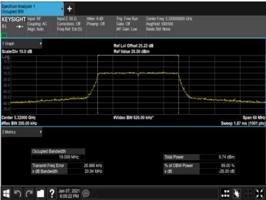
Figure 384 - 5320 MHz - 99% Occupied Bandwidth
