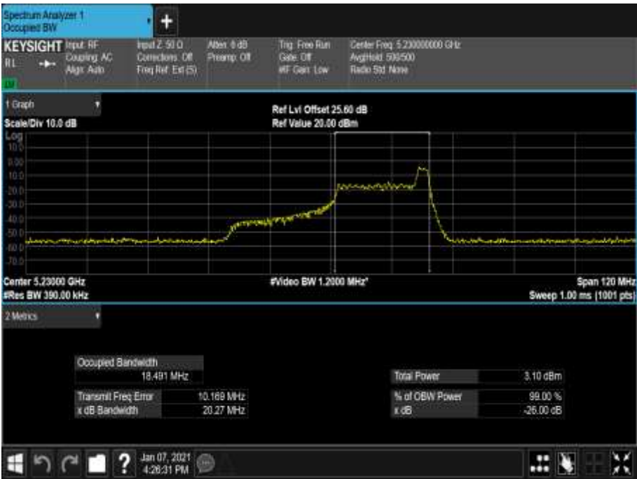
Figure 266 - 5230 MHz - 99% Occupied Bandwidth
