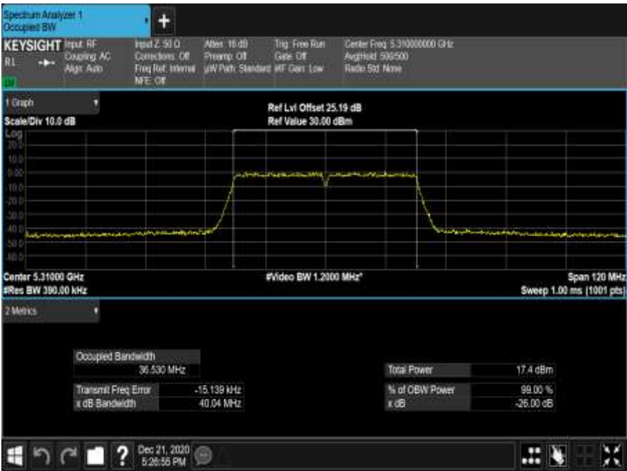
Figure 398 - 5310 MHz - 99% Occupied Bandwidth
