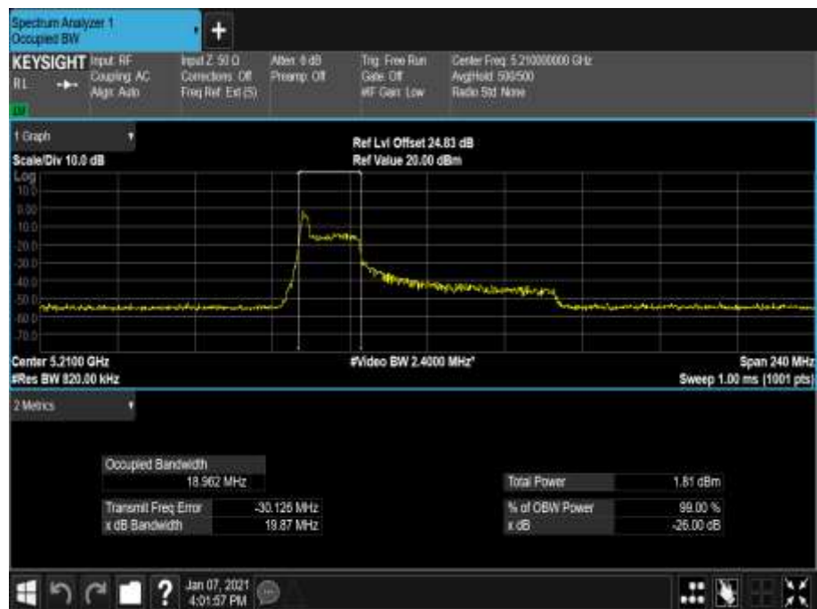
Figure 326 - 5210 MHz - 99% Occupied Bandwidth
