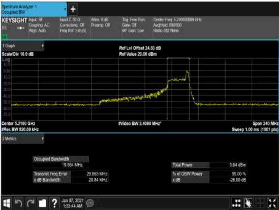
Figure 318 - 5210 MHz - 99% Occupied Bandwidth
