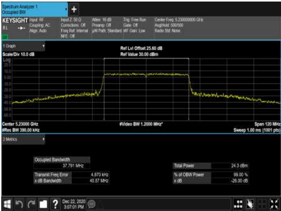
Figure 222 - 5230 MHz - 99% Occupied Bandwidth
