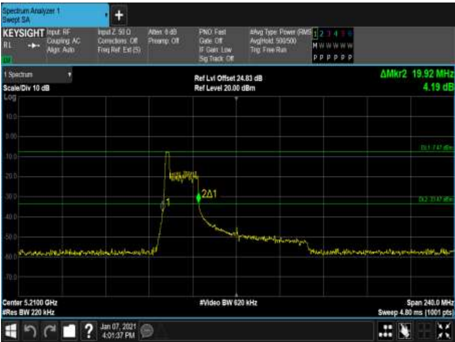
Figure 325 - 5210 MHz - 26 dB Emission Bandwidth
