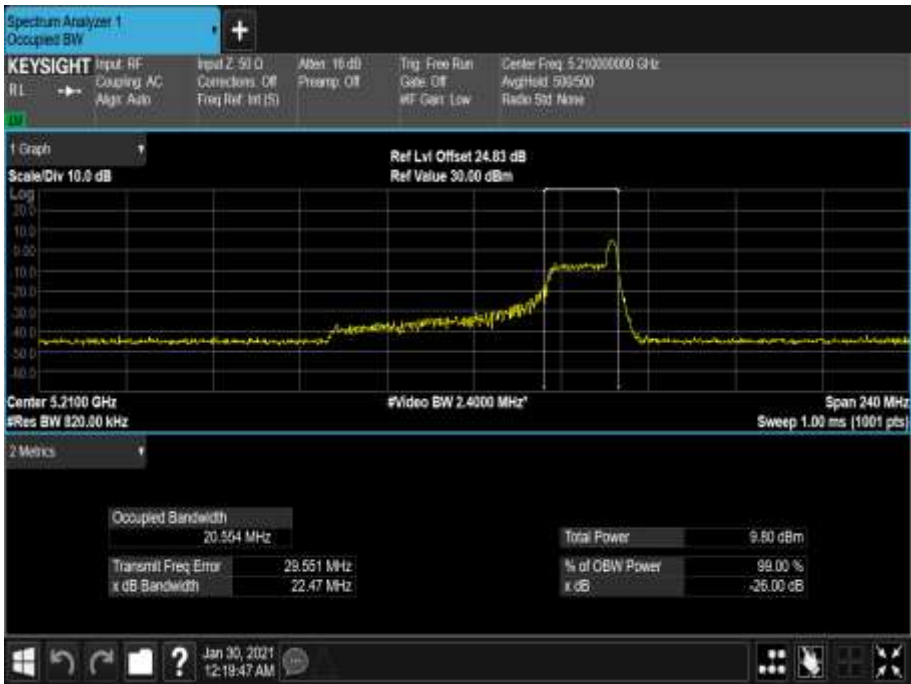
Figure 342 - 5210 MHz - 99% Occupied Bandwidth
