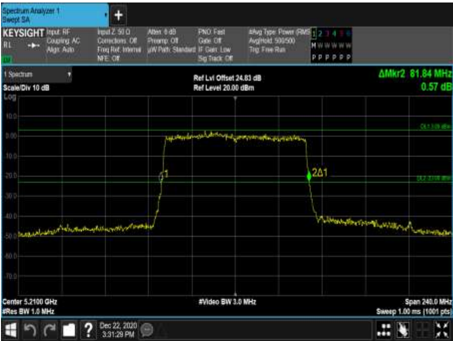
Figure 307 - 5210 MHz - 26 dB Emission Bandwidth
