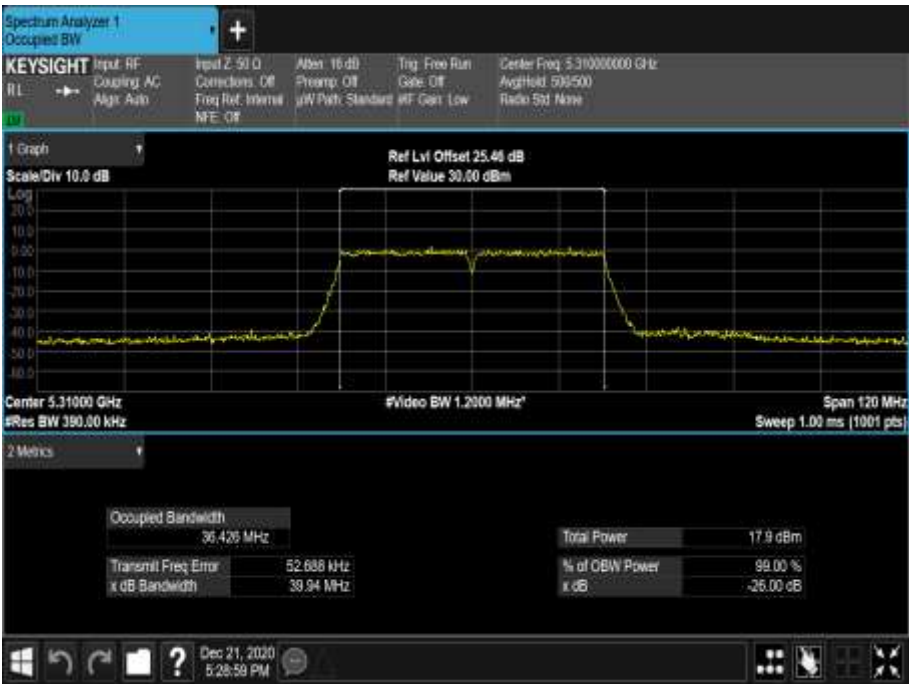
Figure 402 - 5310 MHz - 99% Occupied Bandwidth
