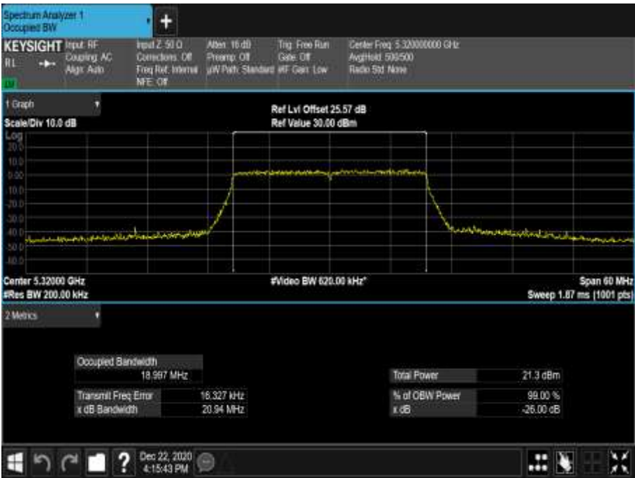
Figure 378 - 5320 MHz - 99% Occupied Bandwidth
