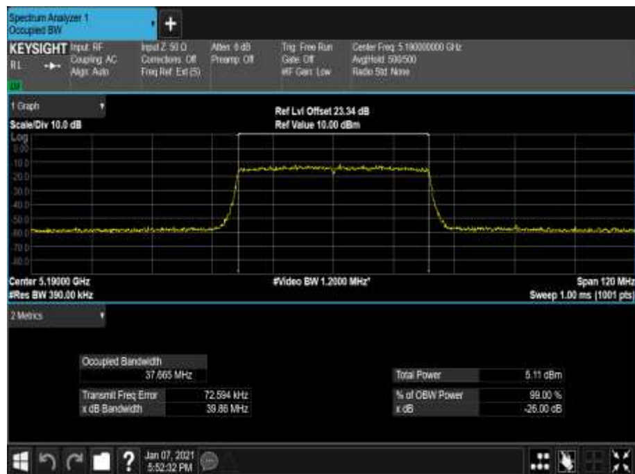
Figure 248 - 5190 MHz - 99% Occupied Bandwidth
