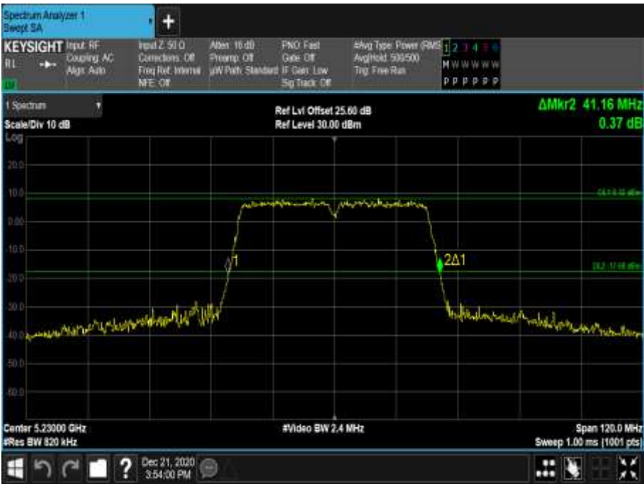
Figure 197 - 5230 MHz - 26 dB Emission Bandwidth
