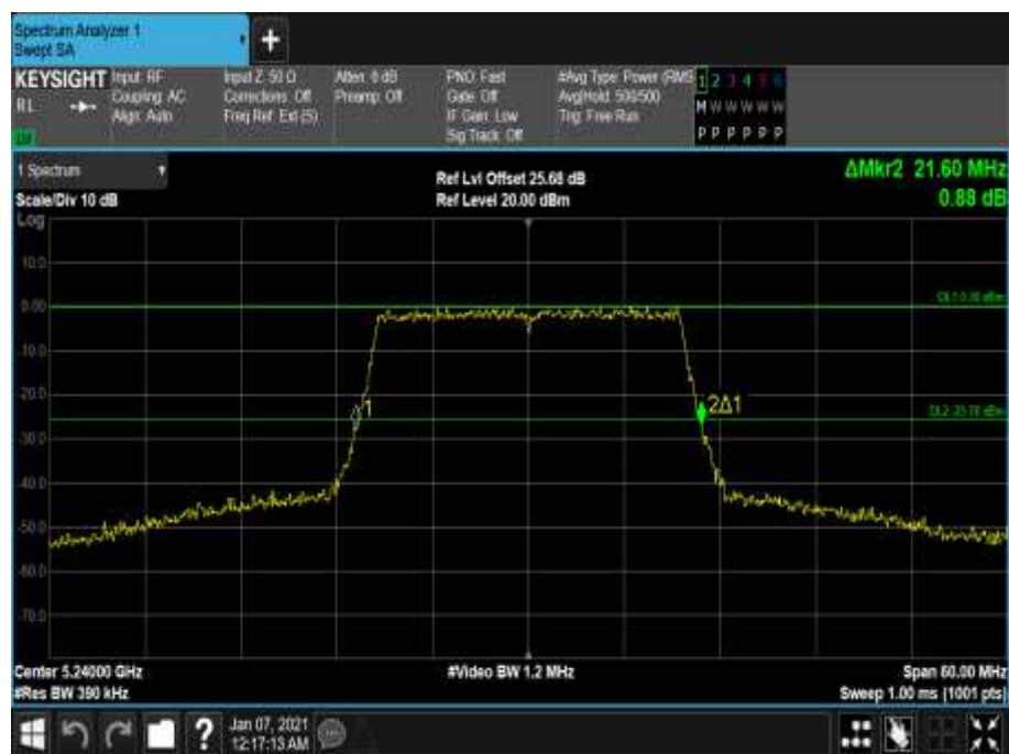
Figure 65 - 5240 MHz - 26 dB Emission Bandwidth
