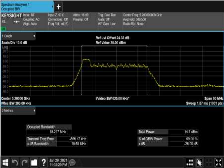
Figure 158 - 5200 MHz - 99% Occupied Bandwidth
