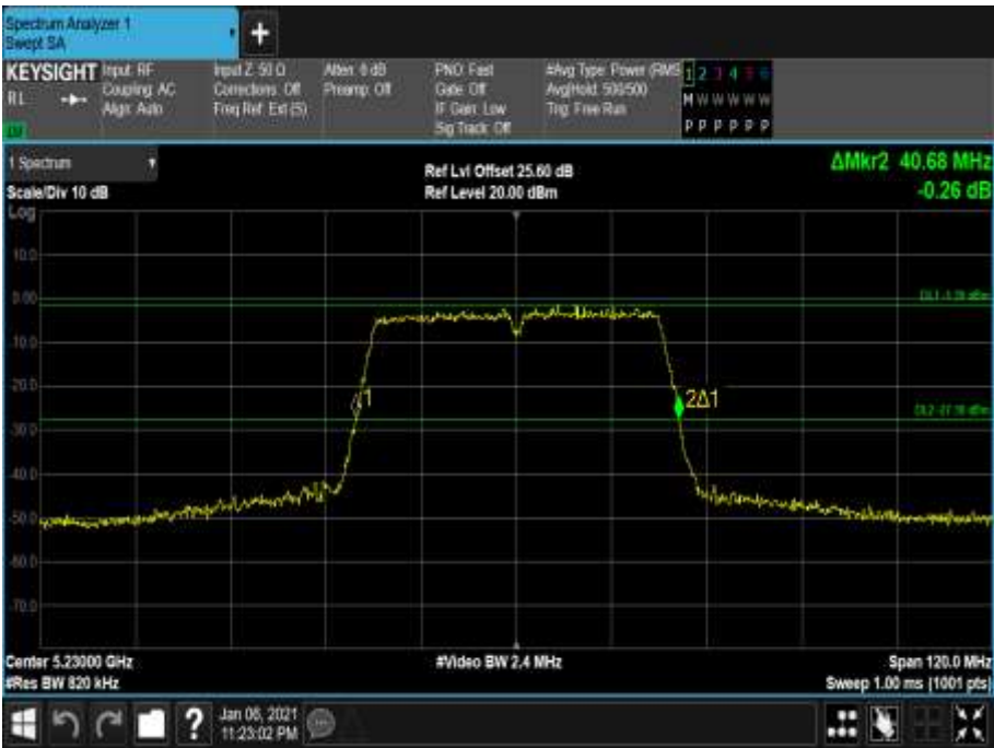
Figure 193 - 5230 MHz - 26 dB Emission Bandwidth
