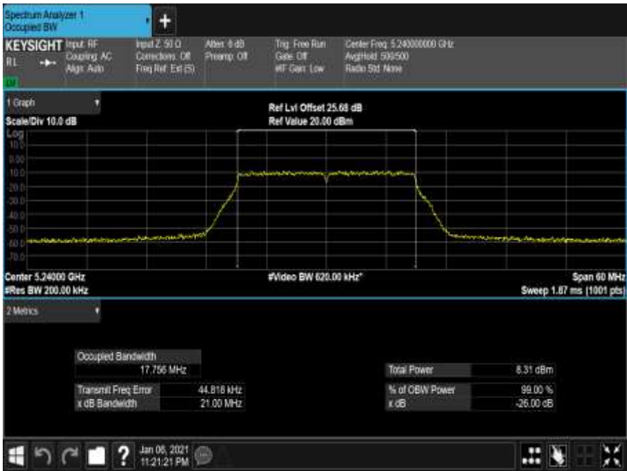
Figure 24 - 5240 MHz - 99% Occupied Bandwidth
