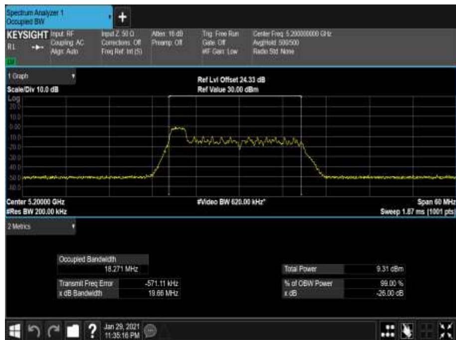
Figure 166 - 5200 MHz - 99% Occupied Bandwidth
