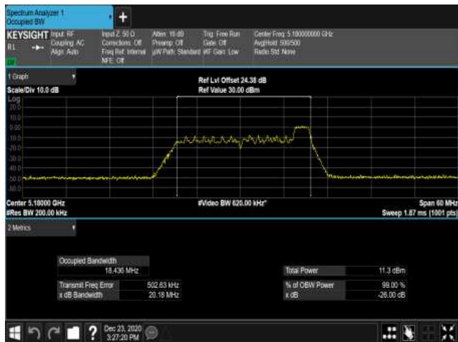
Figure 128 - 5180 MHz - 99% Occupied Bandwidth
