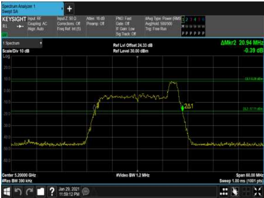
Figure 173 - 5200 MHz - 26 dB Emission Bandwidth
