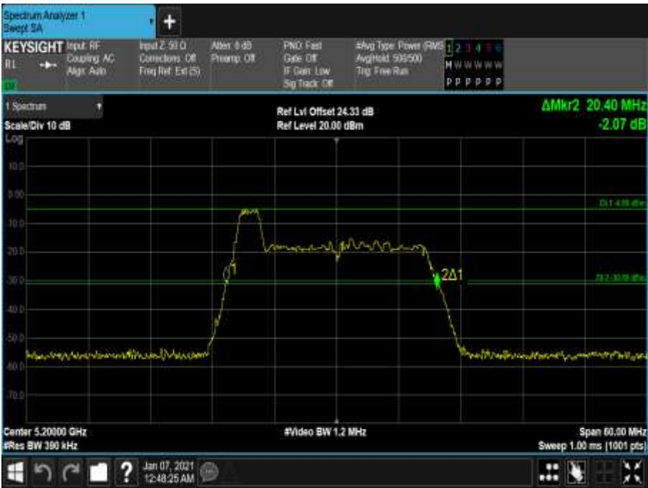
Figure 83 - 5200 MHz - 26 dB Emission Bandwidth
