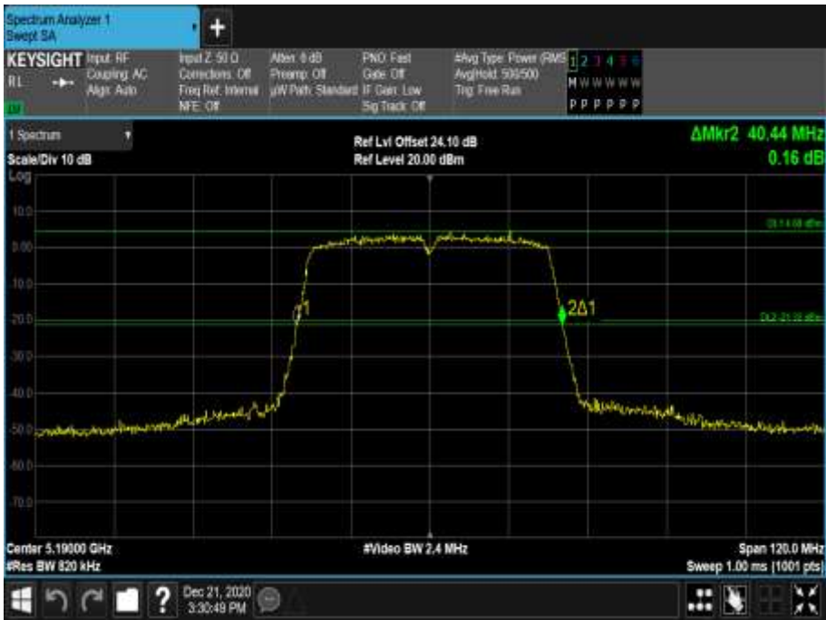
Figure 187 - 5190 MHz - 26 dB Emission Bandwidth
