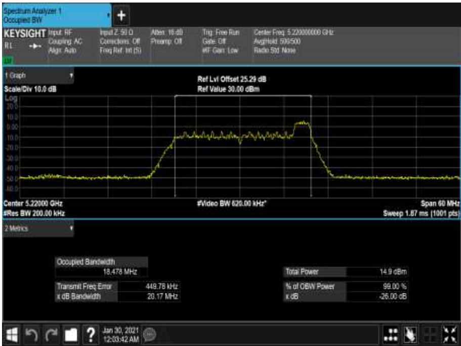
Figure 176 - 5220 MHz - 99% Occupied Bandwidth
