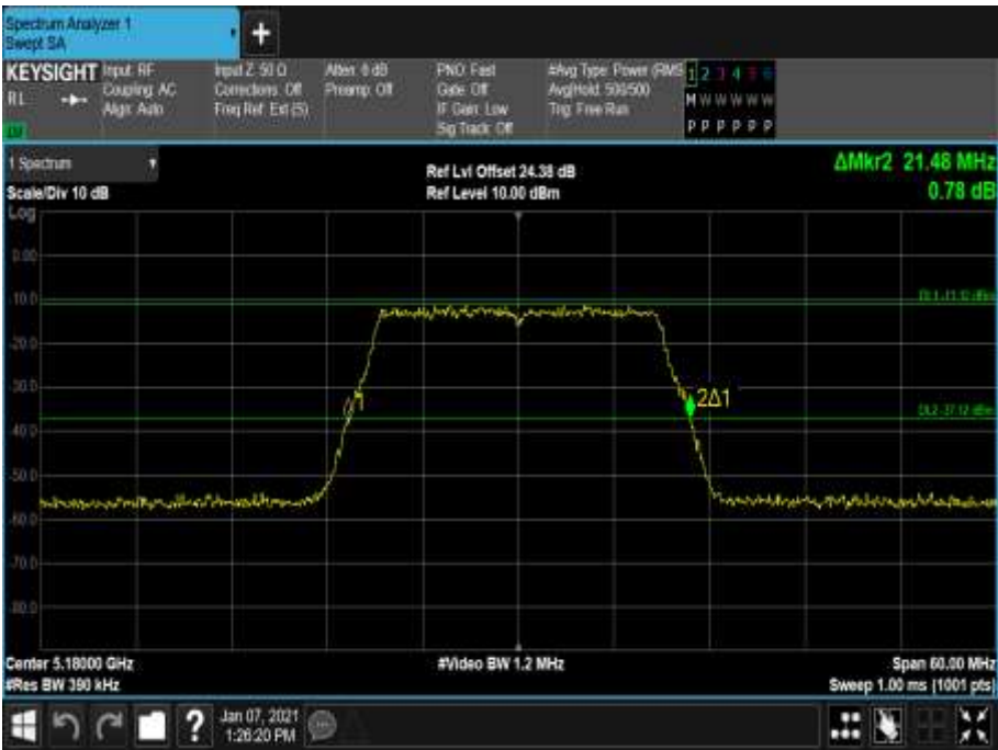
Figure 31 - 5180 MHz - 26 dB Emission Bandwidth
