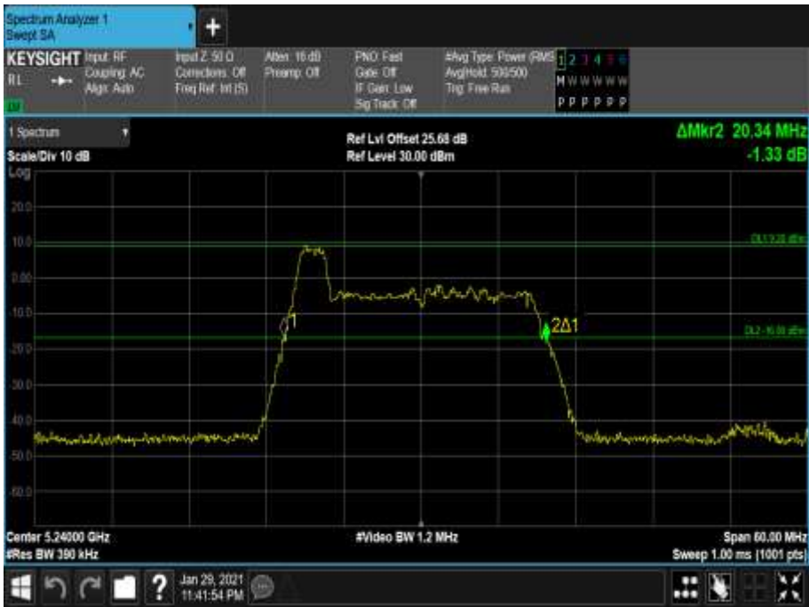
Figure 161 - 5240 MHz - 26 dB Emission Bandwidth
