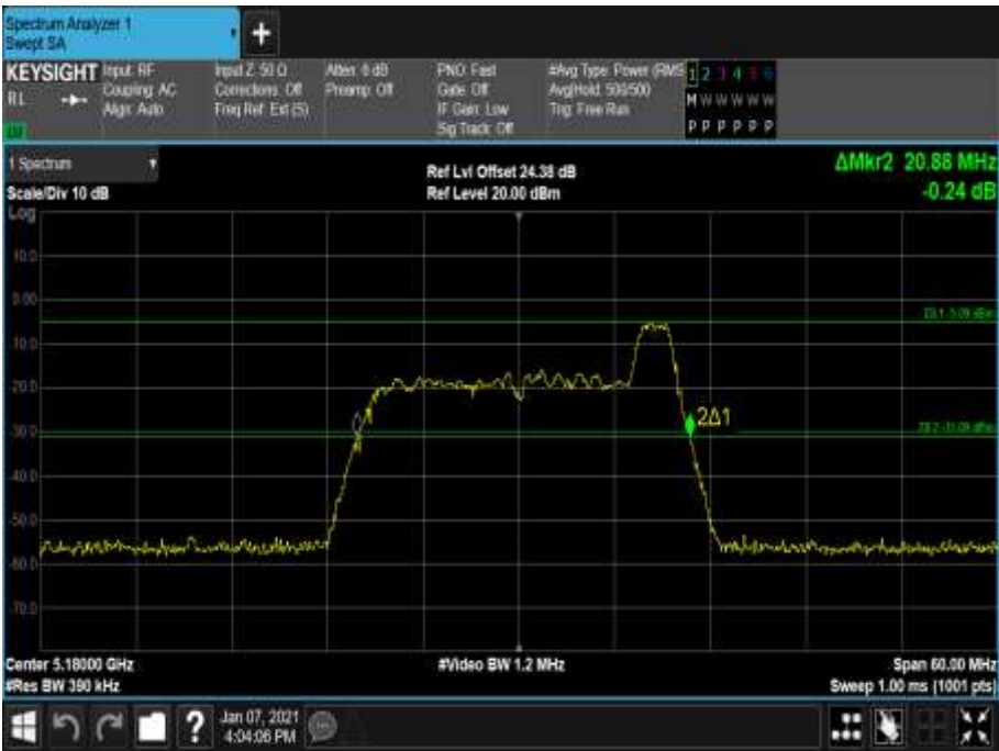
Figure 135 - 5180 MHz - 26 dB Emission Bandwidth
