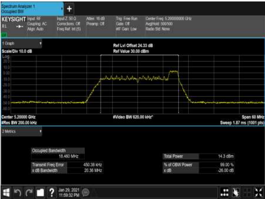
Figure 174 - 5200 MHz - 99% Occupied Bandwidth
