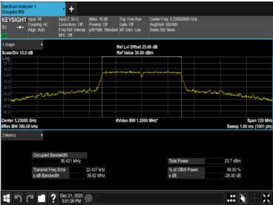
Figure 190 - 5230 MHz - 99% Occupied Bandwidth
