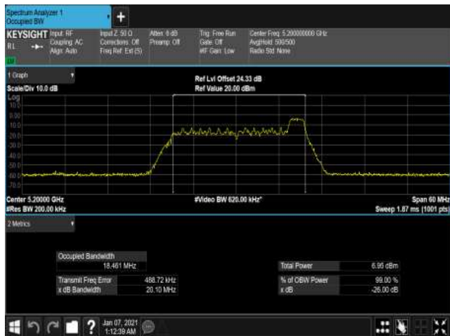
Figure 90 - 5200 MHz - 99% Occupied Bandwidth
