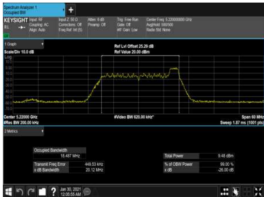
Figure 184 - 5220 MHz - 99% Occupied Bandwidth
