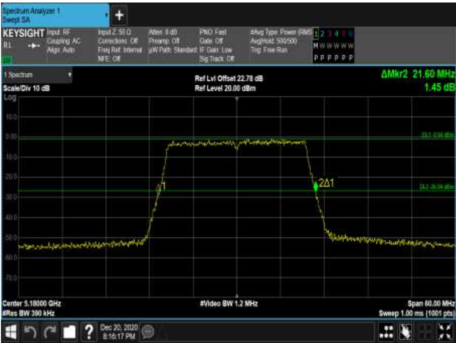
Figure 105 - 5180 MHz - 26 dB Emission Bandwidth
