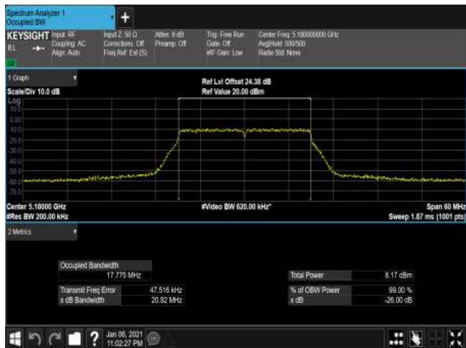
Figure 20 - 5180 MHz - 99% Occupied Bandwidth
