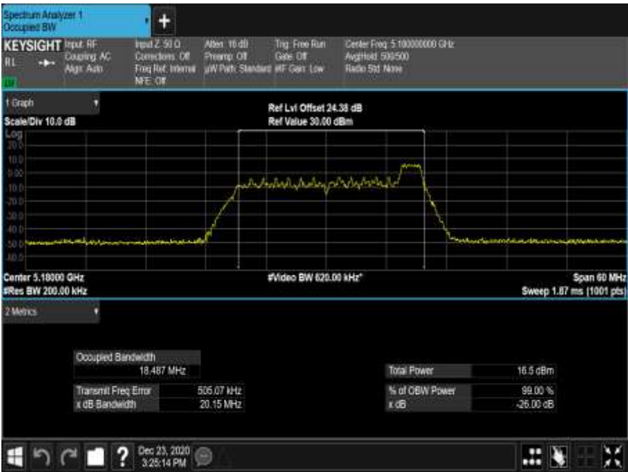
Figure 88 - 5180 MHz - 99% Occupied Bandwidth
