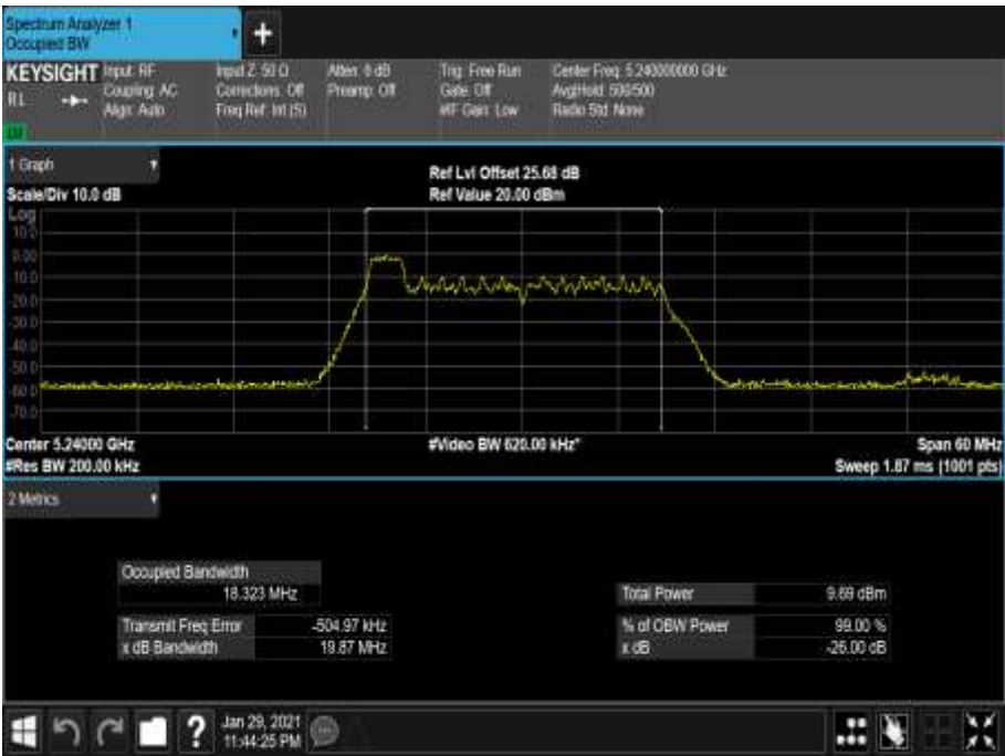
Figure 170 - 5240 MHz - 99% Occupied Bandwidth
