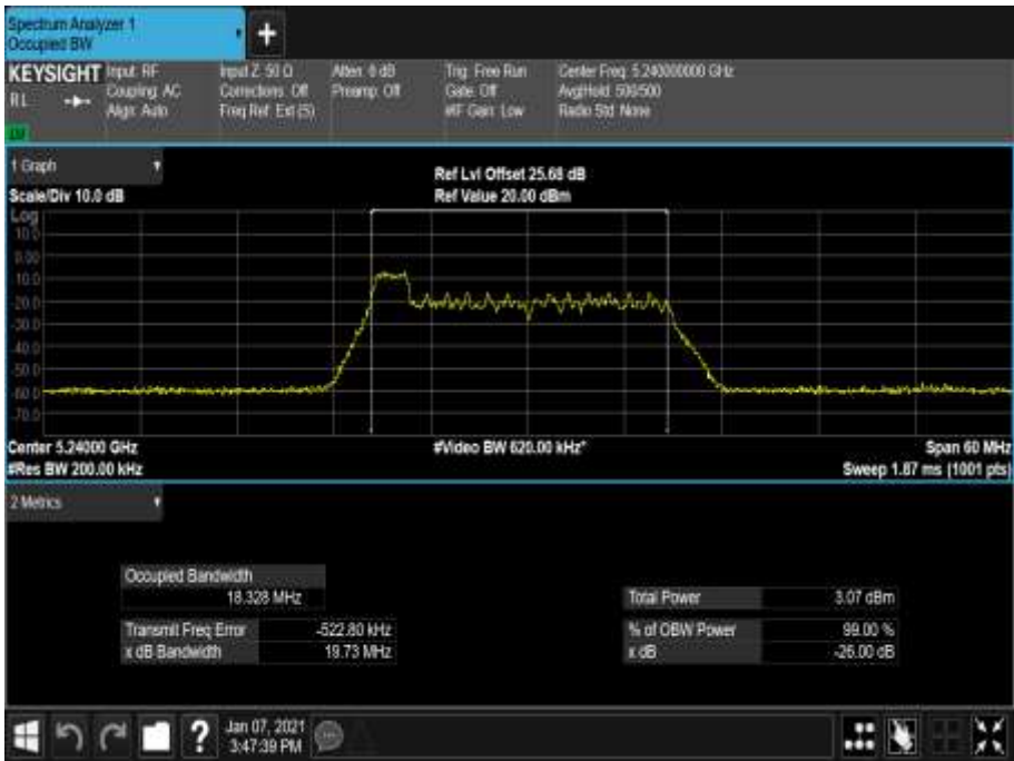
Figure 118 - 5240 MHz - 99% Occupied Bandwidth
