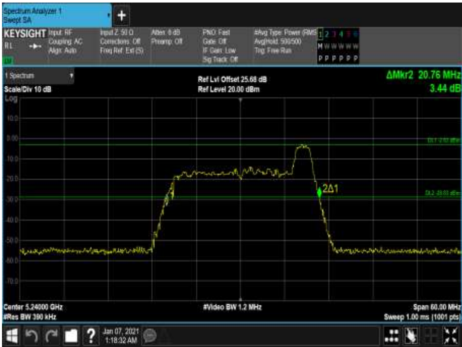
Figure 97 - 5240 MHz - 26 dB Emission Bandwidth
