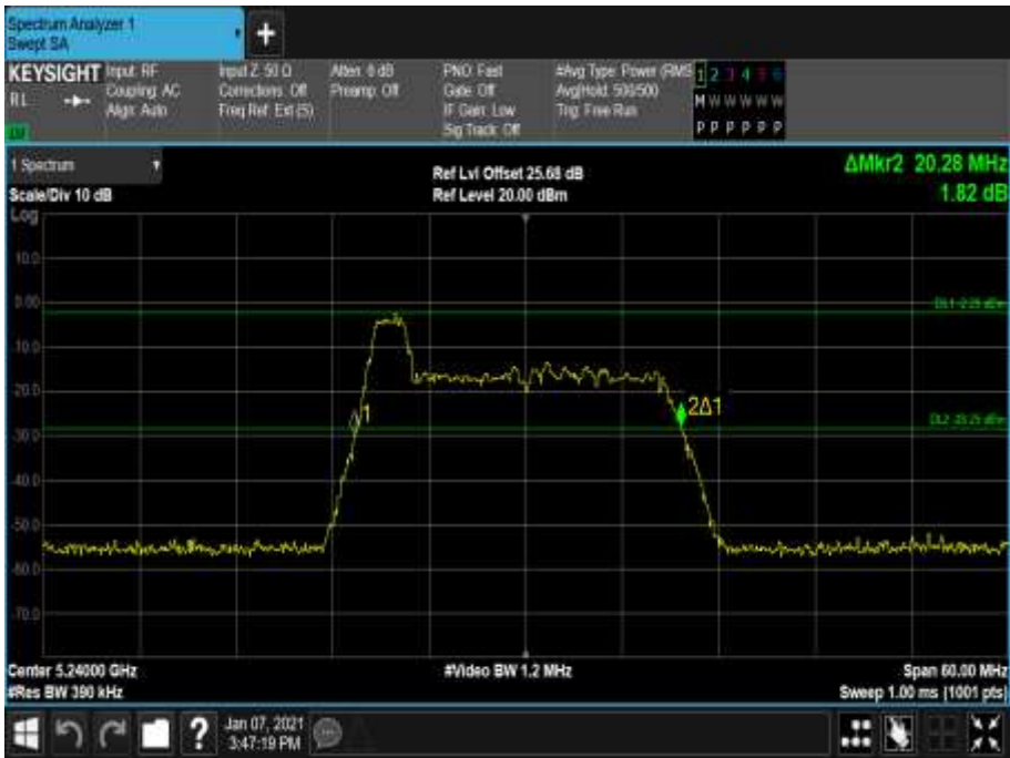
Figure 117 - 5240 MHz - 26 dB Emission Bandwidth
