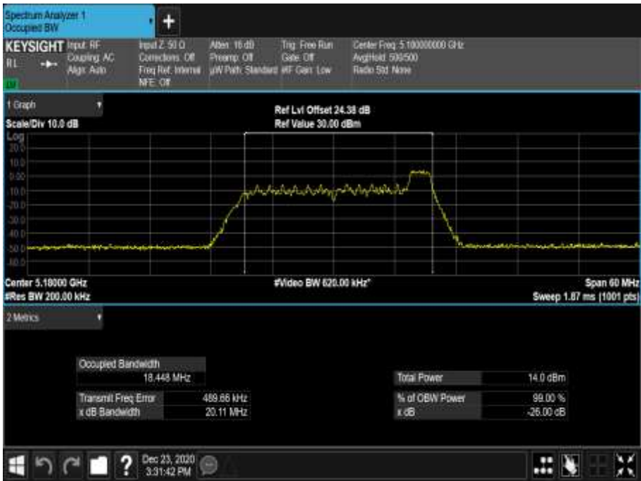
Figure 172 - 5180 MHz - 99% Occupied Bandwidth
