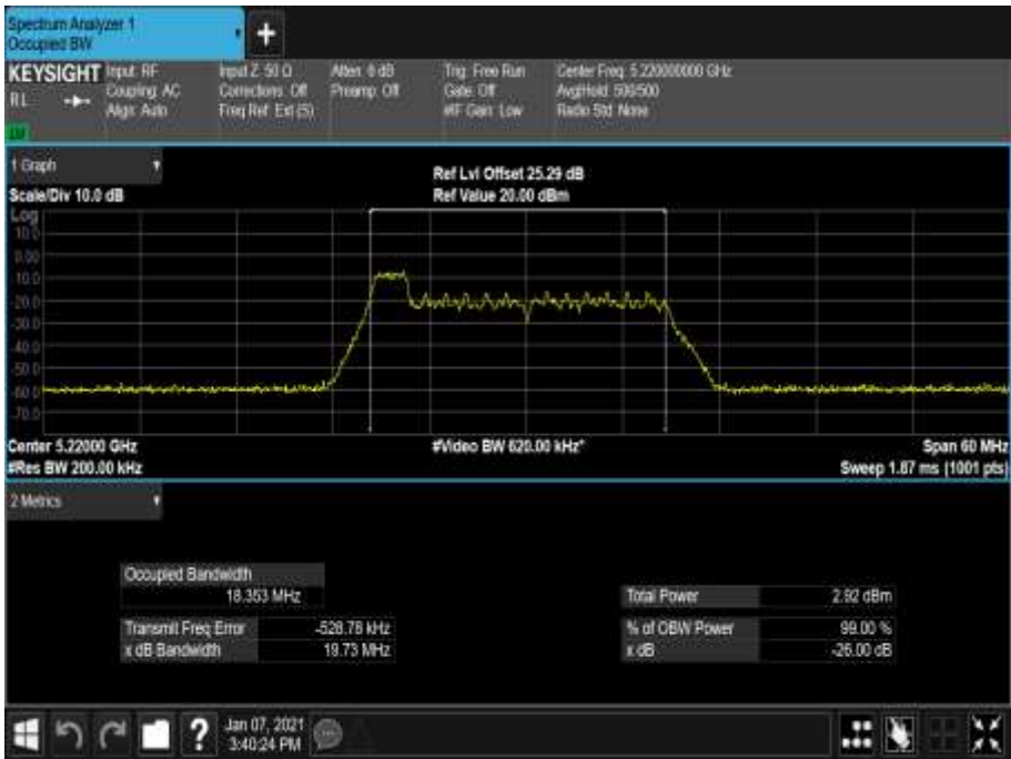
Figure 116 - 5220 MHz - 99% Occupied Bandwidth
