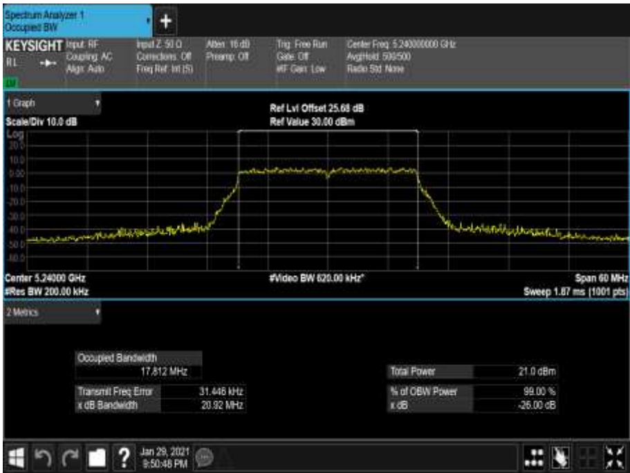
Figure 42 - 5240 MHz - 99% Occupied Bandwidth
