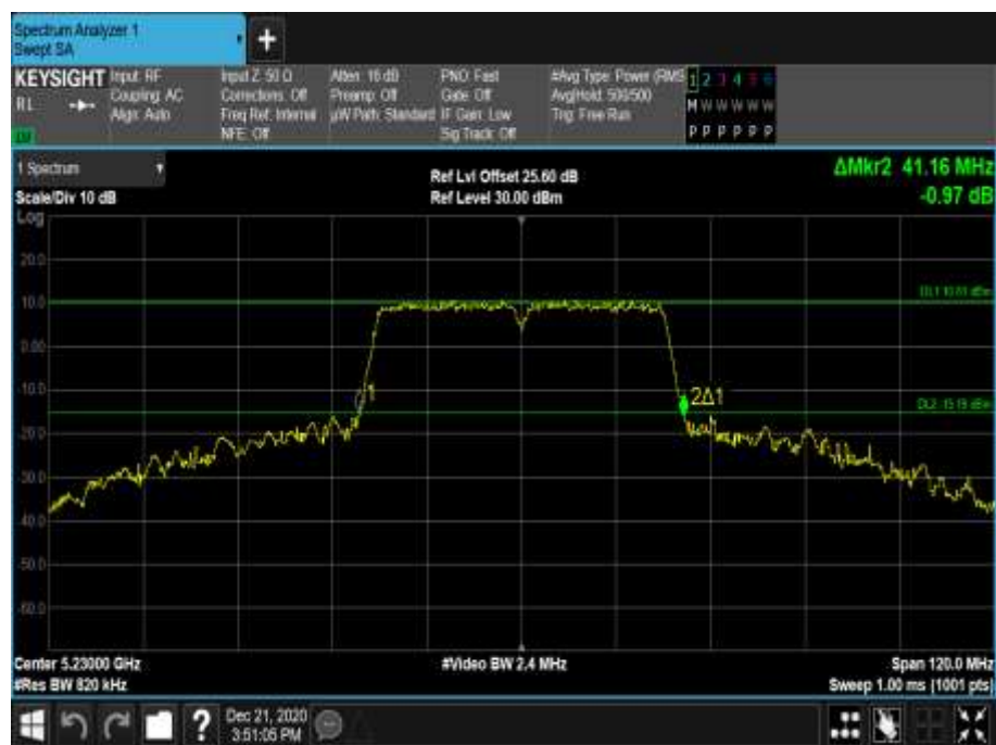
Figure 189 - 5230 MHz - 26 dB Emission Bandwidth
