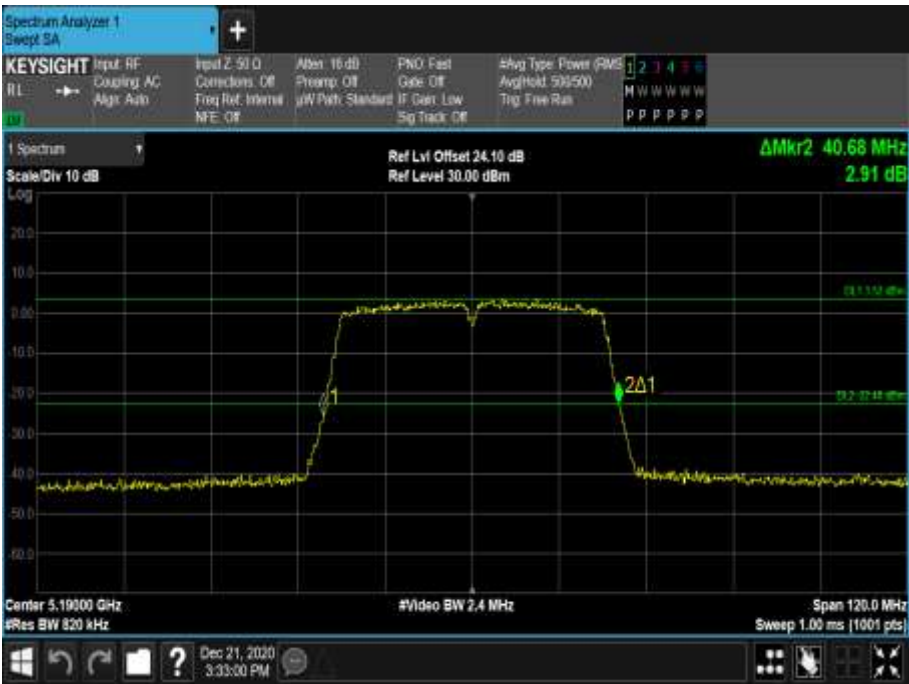
Figure 195 - 5190 MHz - 26 dB Emission Bandwidth
