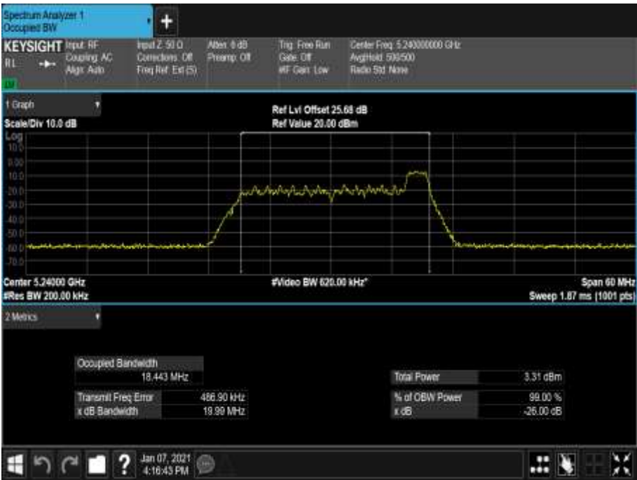
Figure 134 - 5240 MHz - 99% Occupied Bandwidth
