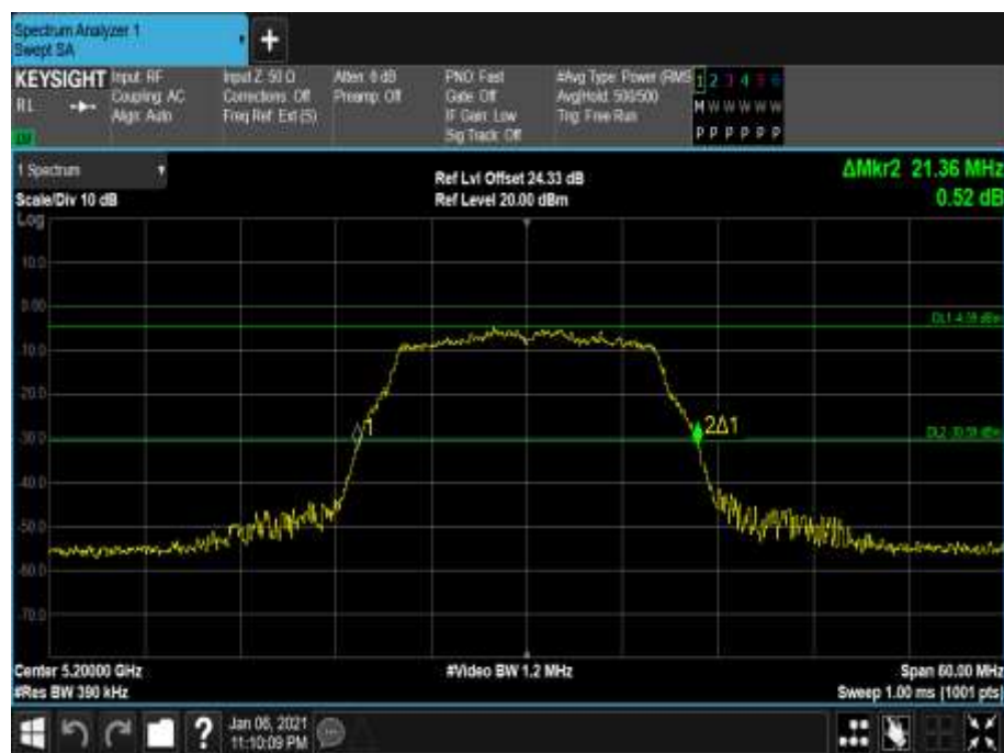
Figure 9 - 5200 MHz - 26 dB Emission Bandwidth
