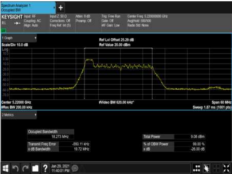
Figure 168 - 5220 MHz - 99% Occupied Bandwidth
