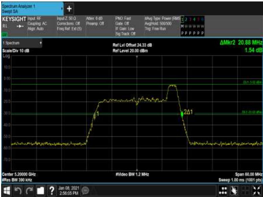
Figure 181 - 5200 MHz - 26 dB Emission Bandwidth
