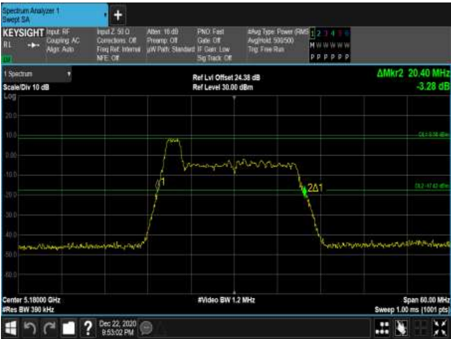
Figure 155 - 5180 MHz - 26 dB Emission Bandwidth
