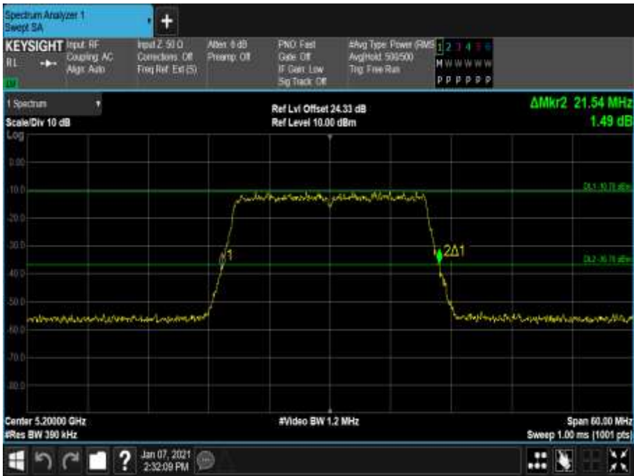
Figure 107 - 5200 MHz - 26 dB Emission Bandwidth
