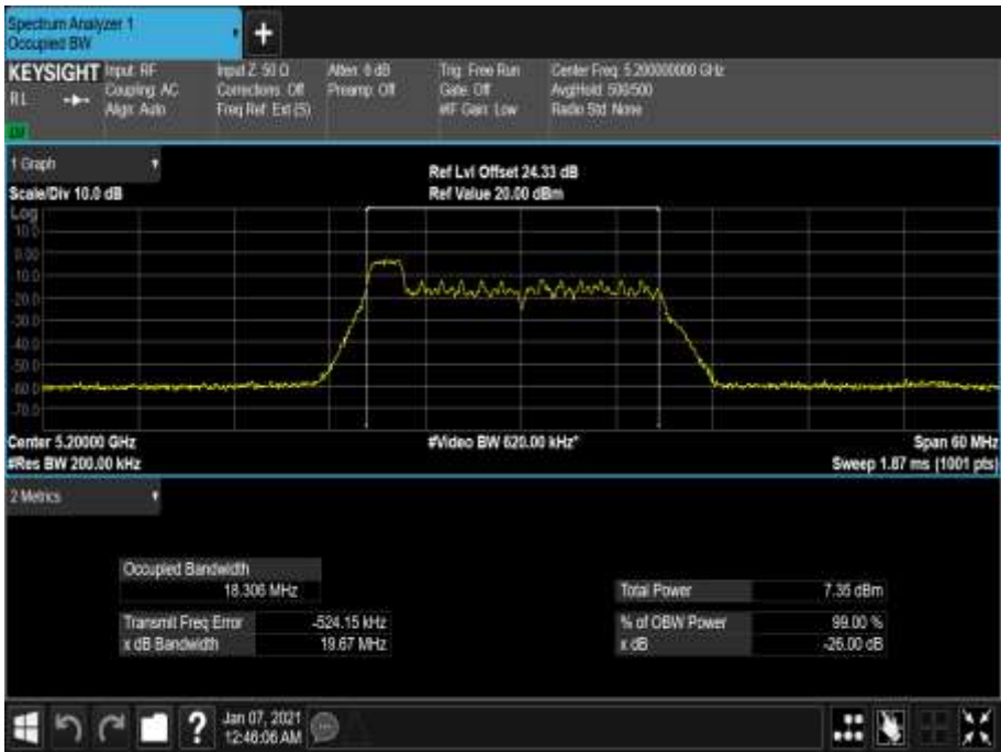
Figure 78 - 5200 MHz - 99% Occupied Bandwidth
