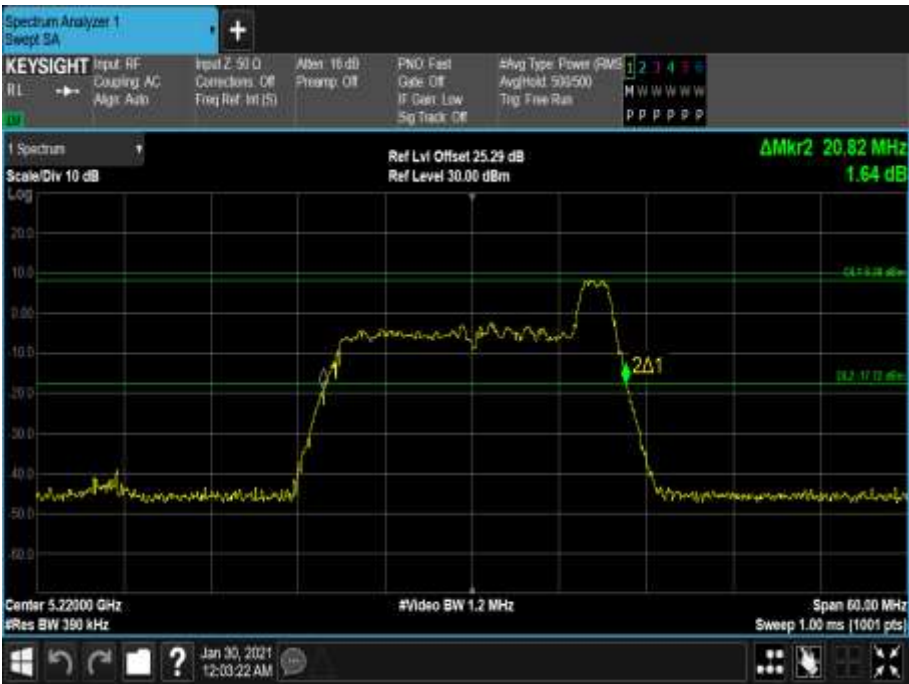
Figure 175 - 5220 MHz - 26 dB Emission Bandwidth
