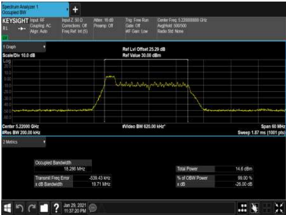
Figure 160 - 5220 MHz - 99% Occupied Bandwidth
