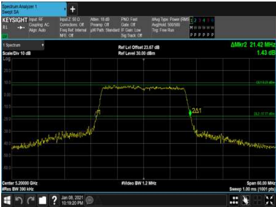
Figure 145 - 5200 MHz - 26 dB Emission Bandwidth
