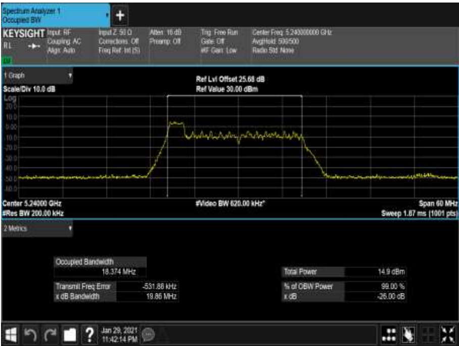
Figure 162 - 5240 MHz - 99% Occupied Bandwidth
