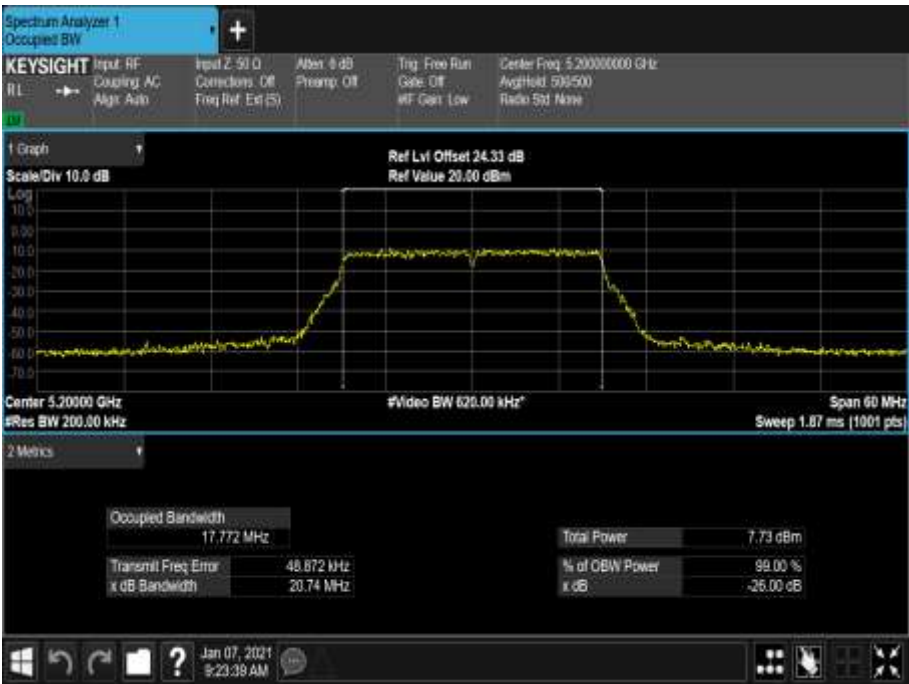
Figure 52 - 5200 MHz - 99% Occupied Bandwidth
