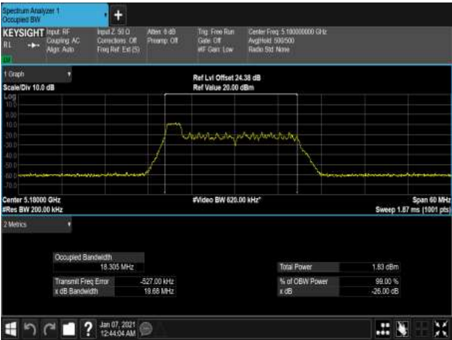
Figure 82 - 5180 MHz - 99% Occupied Bandwidth
