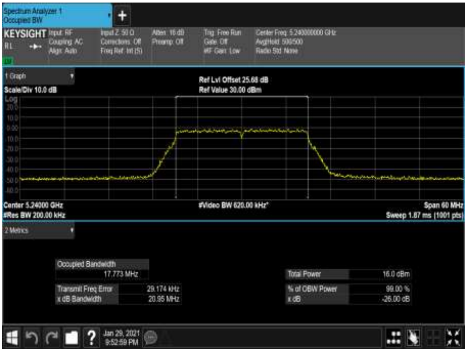
Figure 48 - 5240 MHz - 99% Occupied Bandwidth
