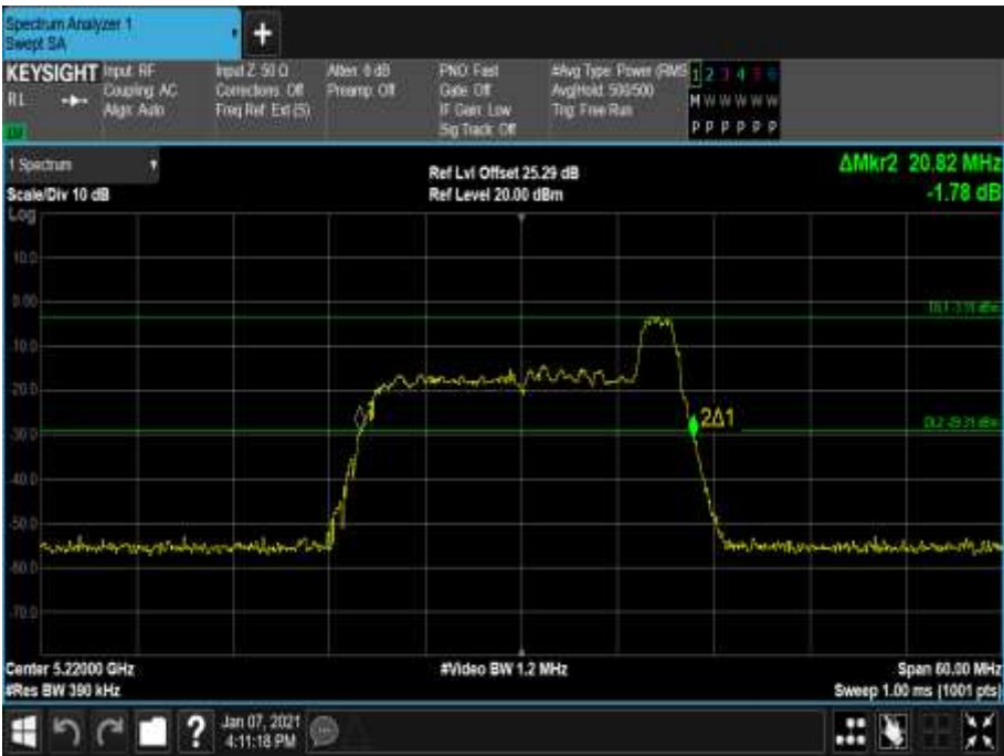
Figure 131 - 5220 MHz - 26 dB Emission Bandwidth
