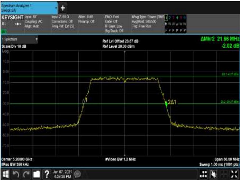
Figure 27 - 5200 MHz - 26 dB Emission Bandwidth
