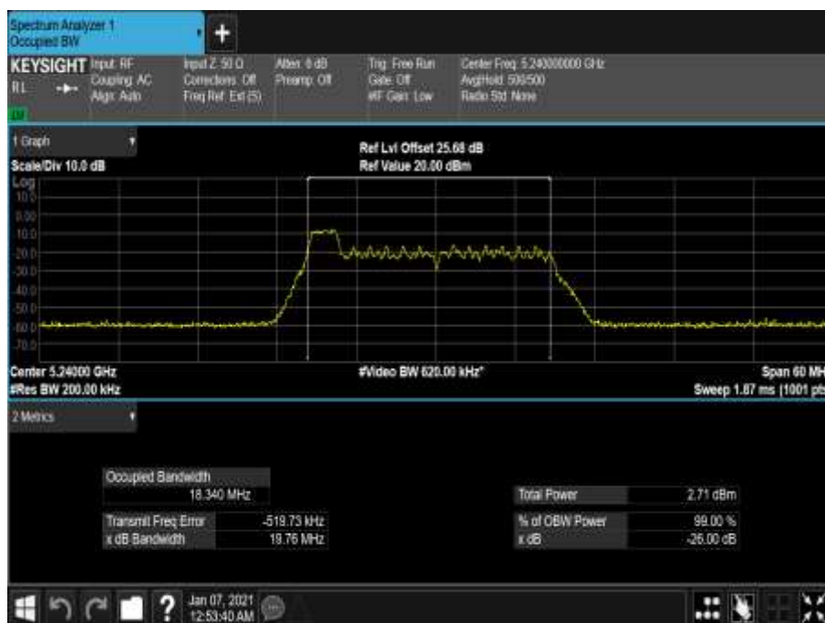
Figure 86 - 5240 MHz - 99% Occupied Bandwidth
