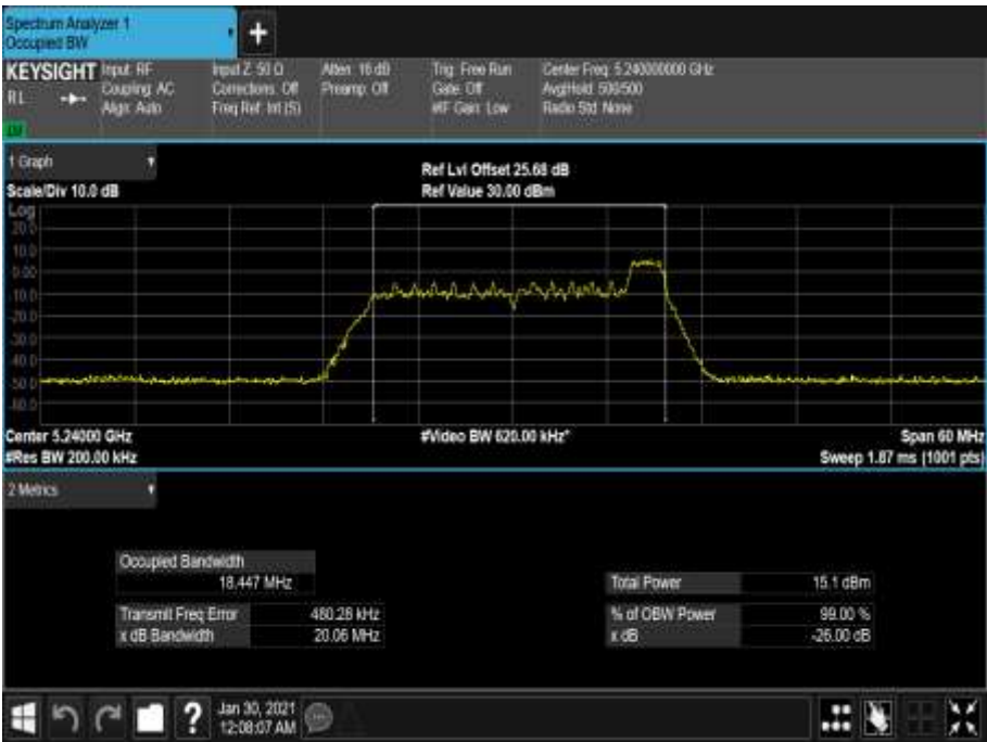
Figure 178 - 5240 MHz - 99% Occupied Bandwidth
