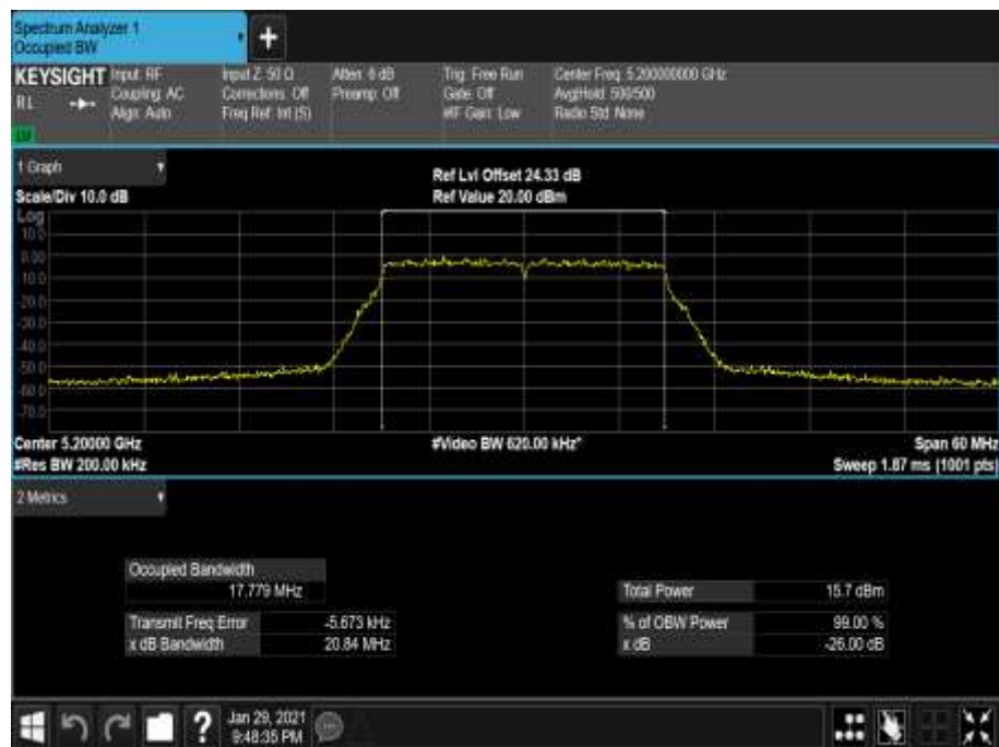
Figure 46 - 5200 MHz - 99% Occupied Bandwidth
