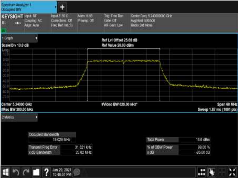
Figure 154 - 5240 MHz - 99% Occupied Bandwidth
