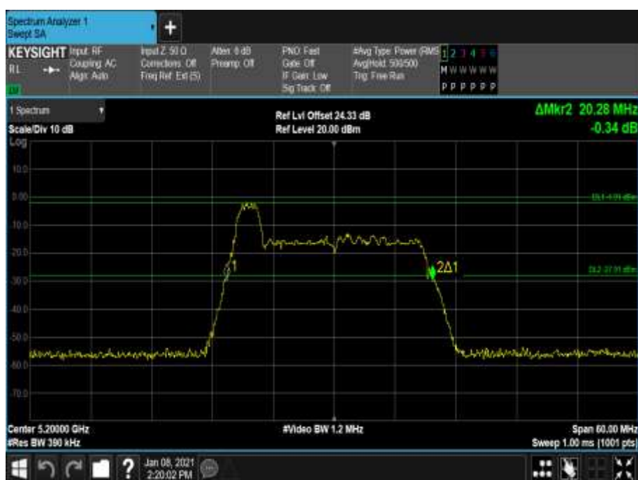
Figure 157 - 5200 MHz - 26 dB Emission Bandwidth
