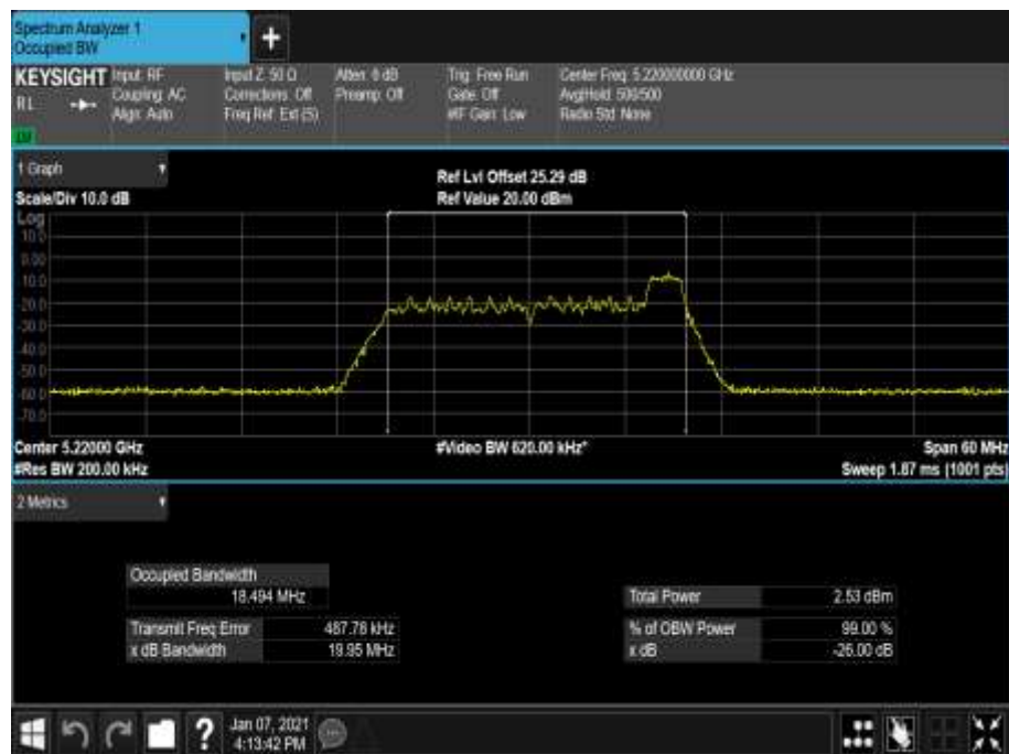
Figure 140 - 5220 MHz - 99% Occupied Bandwidth
