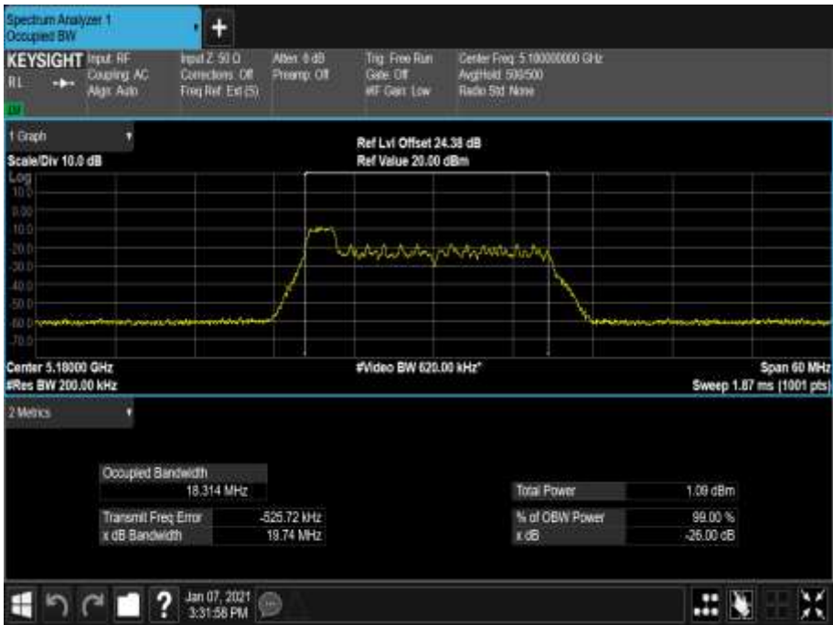
Figure 120 - 5180 MHz - 99% Occupied Bandwidth
