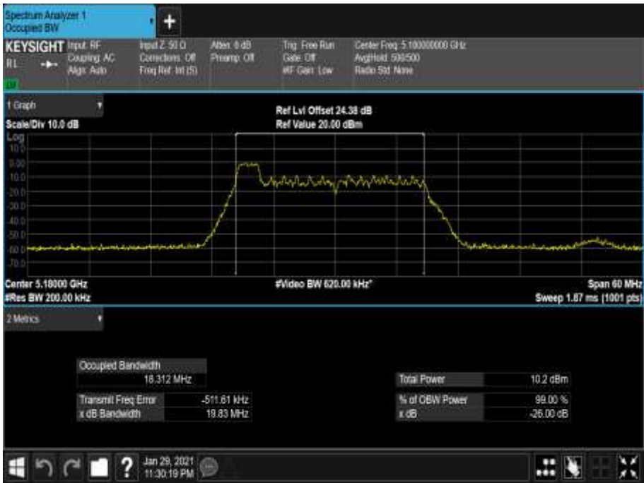
Figure 164 - 5180 MHz - 99% Occupied Bandwidth
