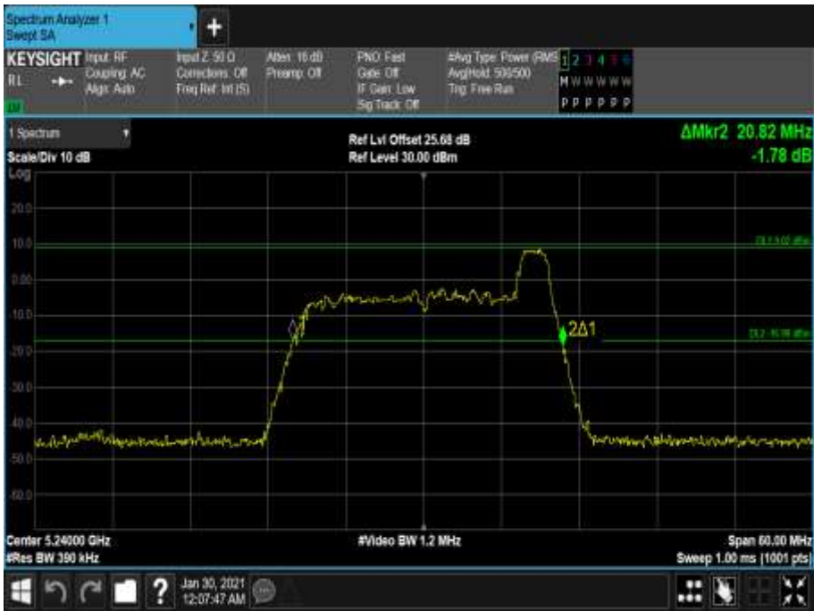
Figure 177 - 5240 MHz - 26 dB Emission Bandwidth
