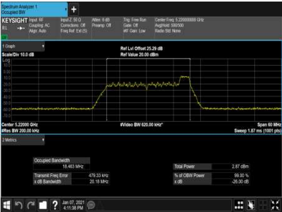
Figure 132 - 5220 MHz - 99% Occupied Bandwidth
