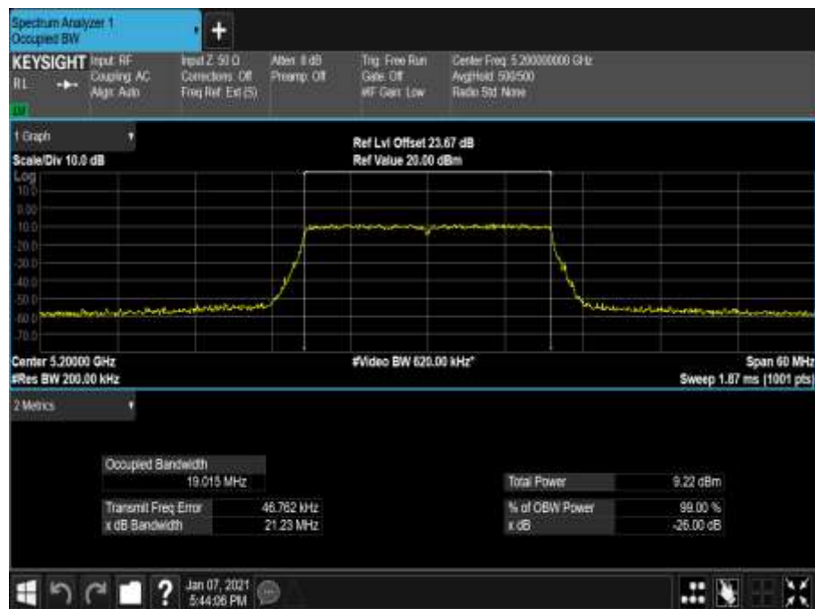
Figure 102 - 5200 MHz - 99% Occupied Bandwidth
