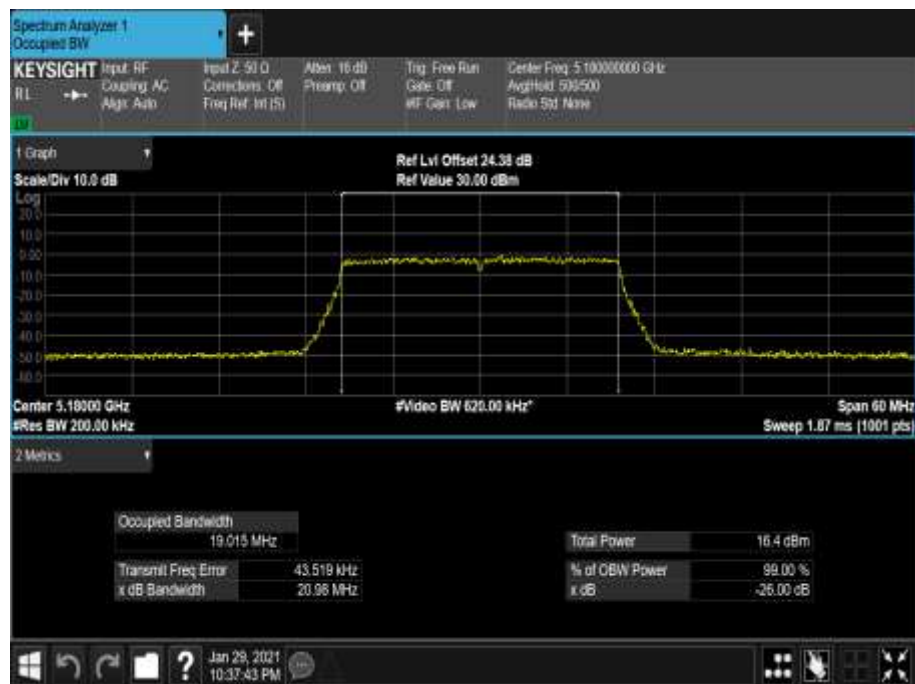
Figure 150 - 5180 MHz - 99% Occupied Bandwidth
