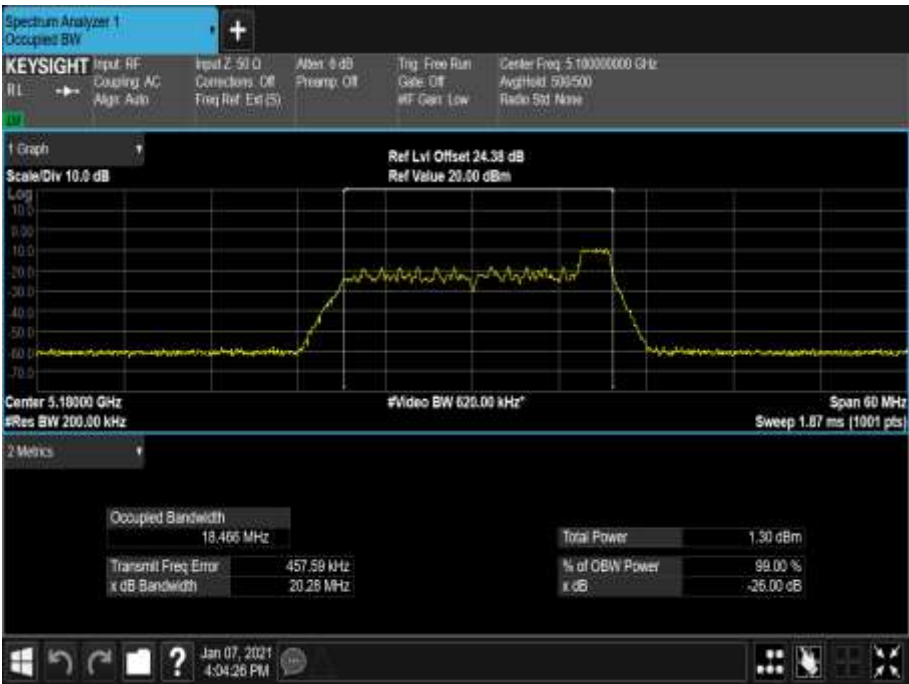
Figure 136 - 5180 MHz - 99% Occupied Bandwidth
