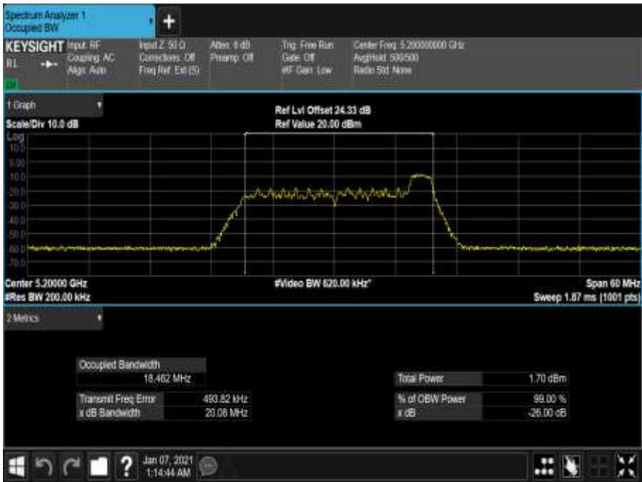
Figure 96 - 5200 MHz - 99% Occupied Bandwidth
