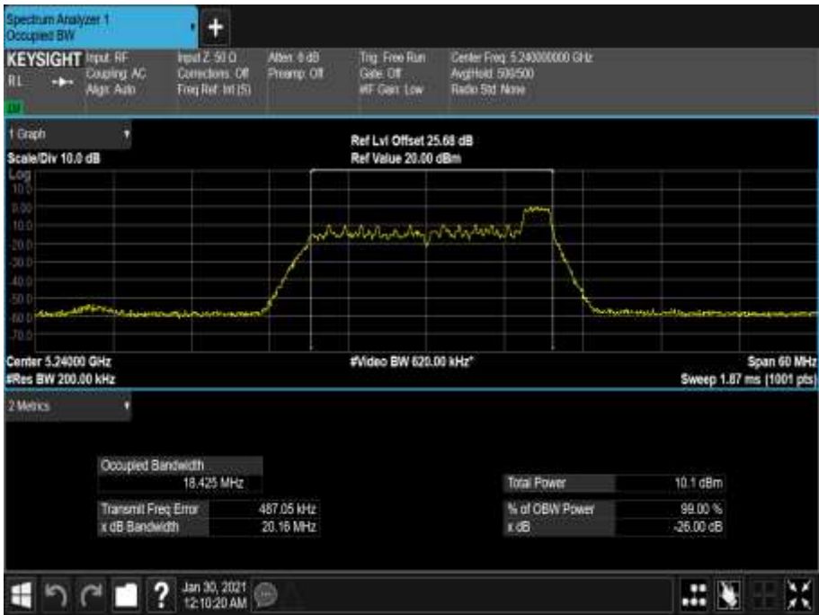
Figure 186 - 5240 MHz - 99% Occupied Bandwidth
