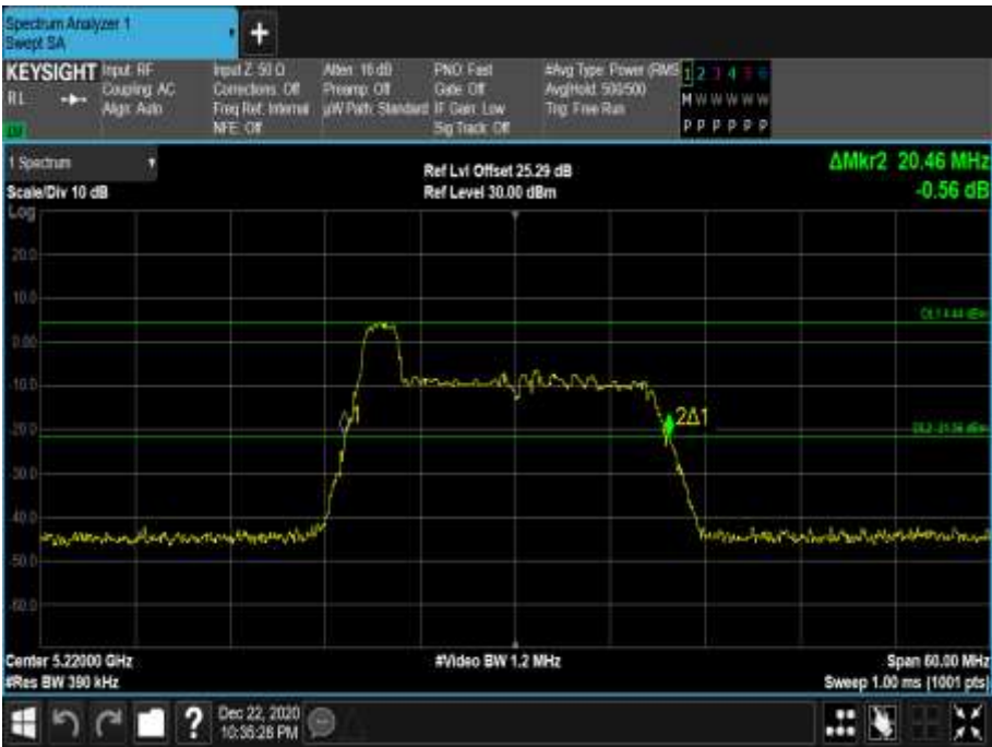
Figure 115 - 5220 MHz - 26 dB Emission Bandwidth
