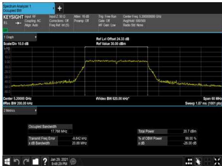
Figure 40 - 5200 MHz - 99% Occupied Bandwidth
