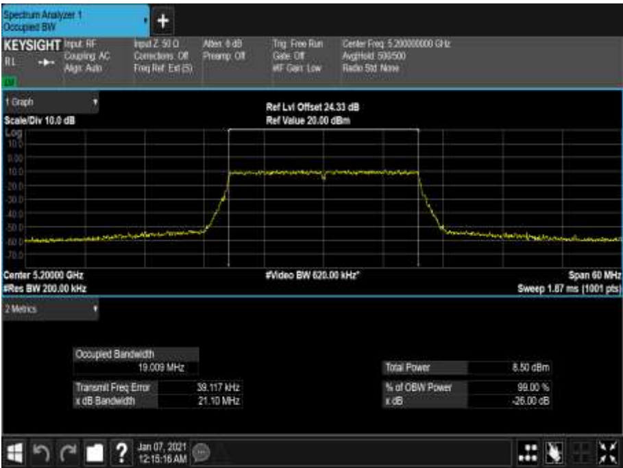
Figure 70 - 5200 MHz - 99% Occupied Bandwidth
