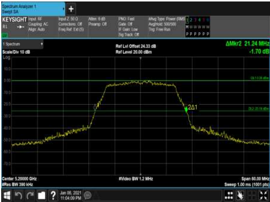
Figure 3 - 5200 MHz - 26 dB Emission Bandwidth
