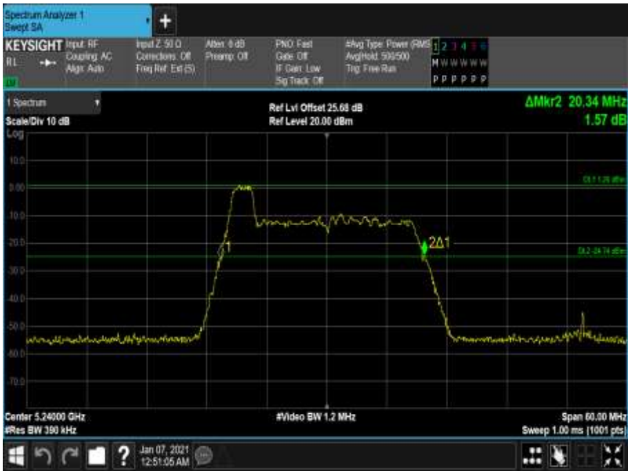
Figure 79 - 5240 MHz - 26 dB Emission Bandwidth
