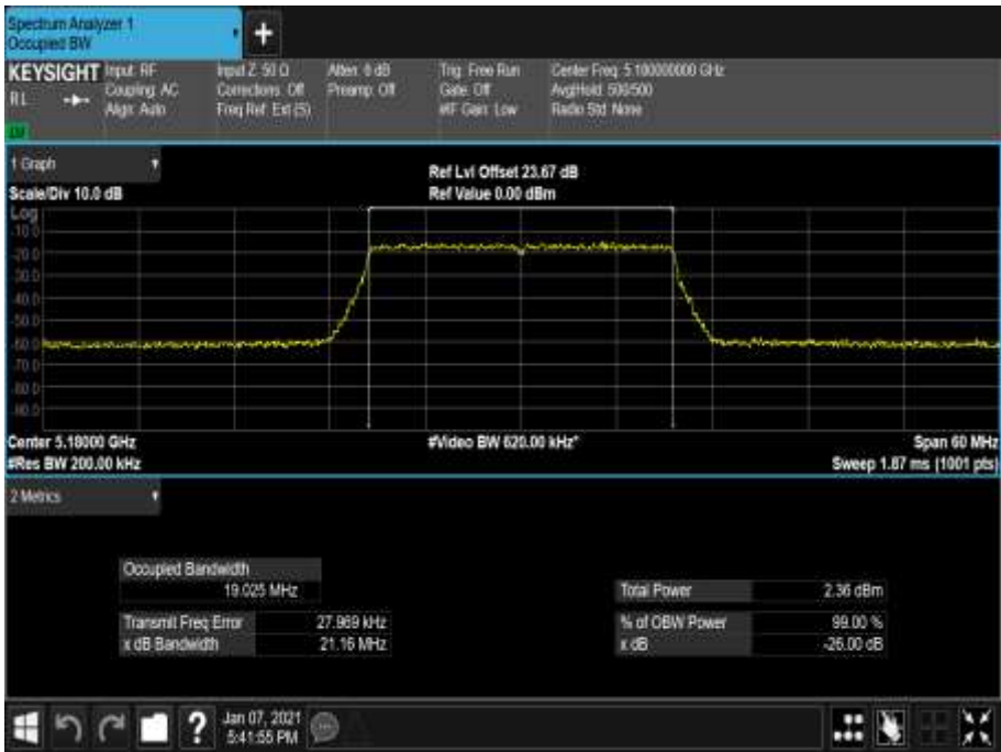
Figure 106 - 5180 MHz - 99% Occupied Bandwidth
