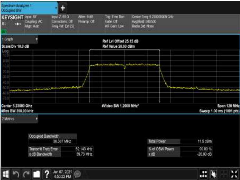
Figure 198 - 5230 MHz - 99% Occupied Bandwidth
