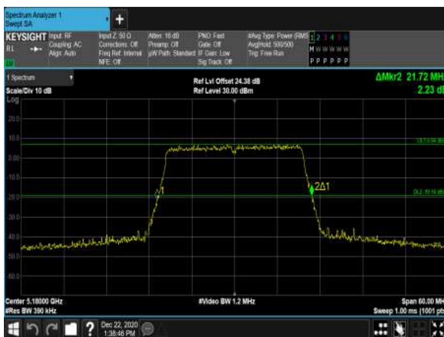
Figure 61 - 5180 MHz - 26 dB Emission Bandwidth
