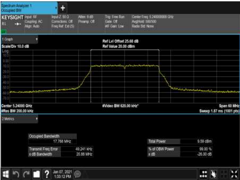
Figure 30 - 5240 MHz - 99% Occupied Bandwidth
