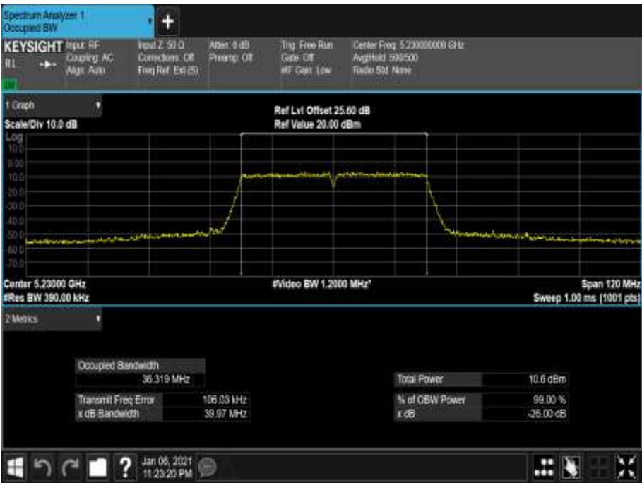
Figure 194 - 5230 MHz - 99% Occupied Bandwidth
