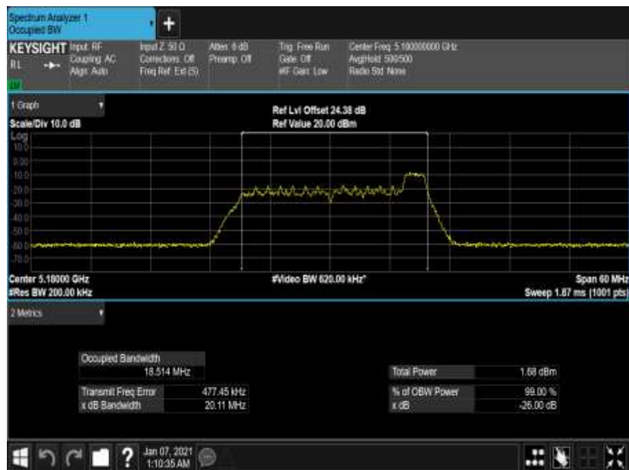
Figure 94 - 5180 MHz - 99% Occupied Bandwidth
