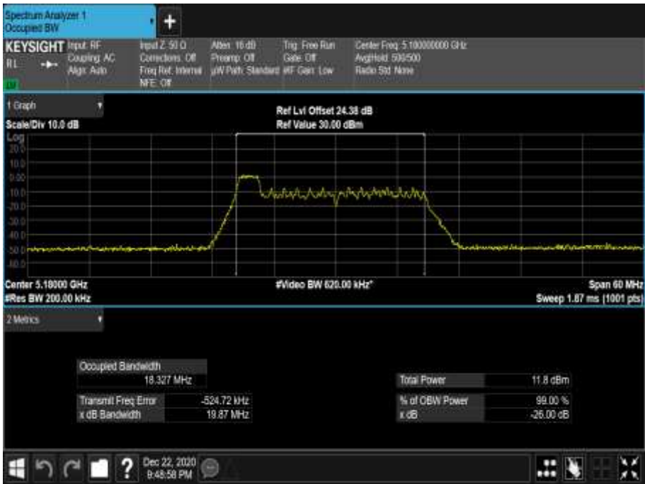
Figure 112 - 5180 MHz - 99% Occupied Bandwidth
