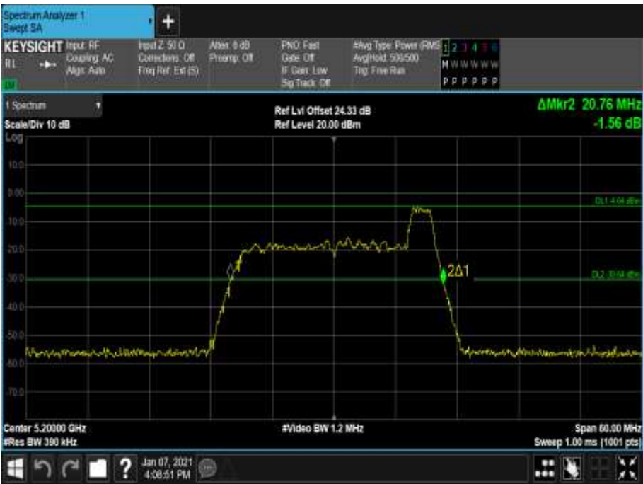
Figure 137 - 5200 MHz - 26 dB Emission Bandwidth
