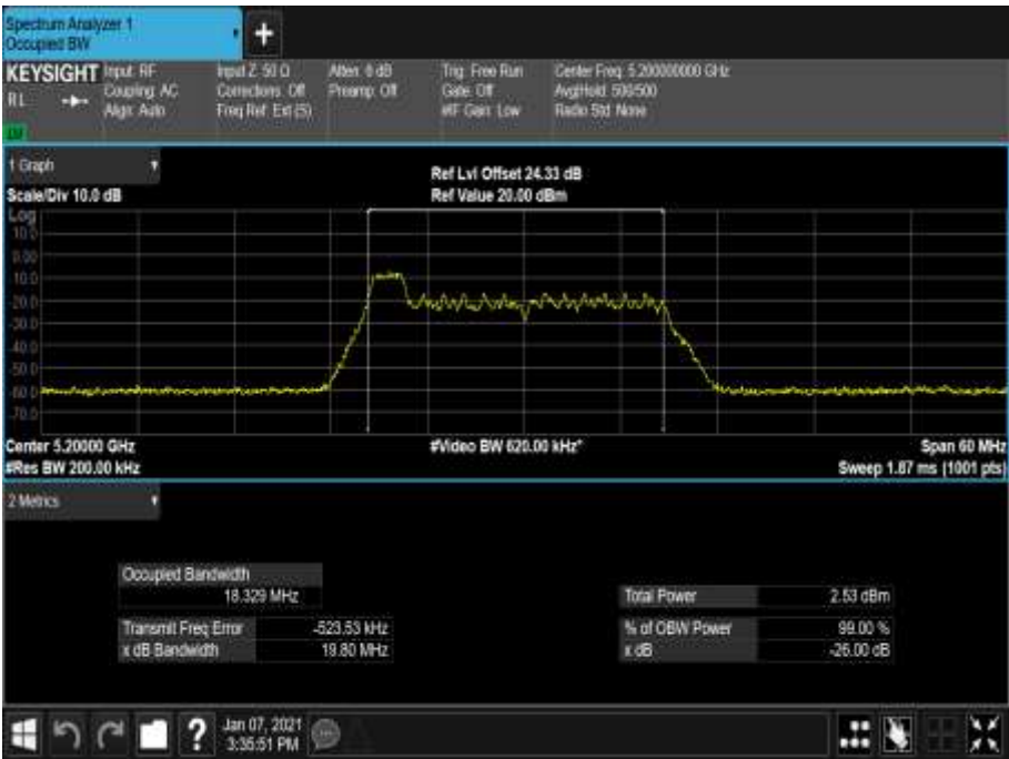
Figure 114 - 5200 MHz - 99% Occupied Bandwidth
