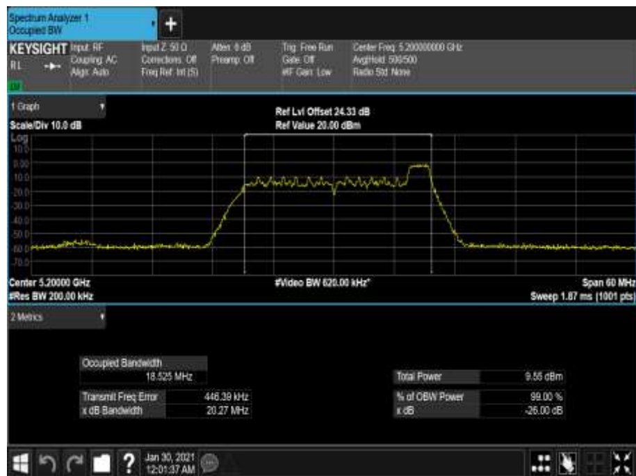
Figure 182 - 5200 MHz - 99% Occupied Bandwidth
