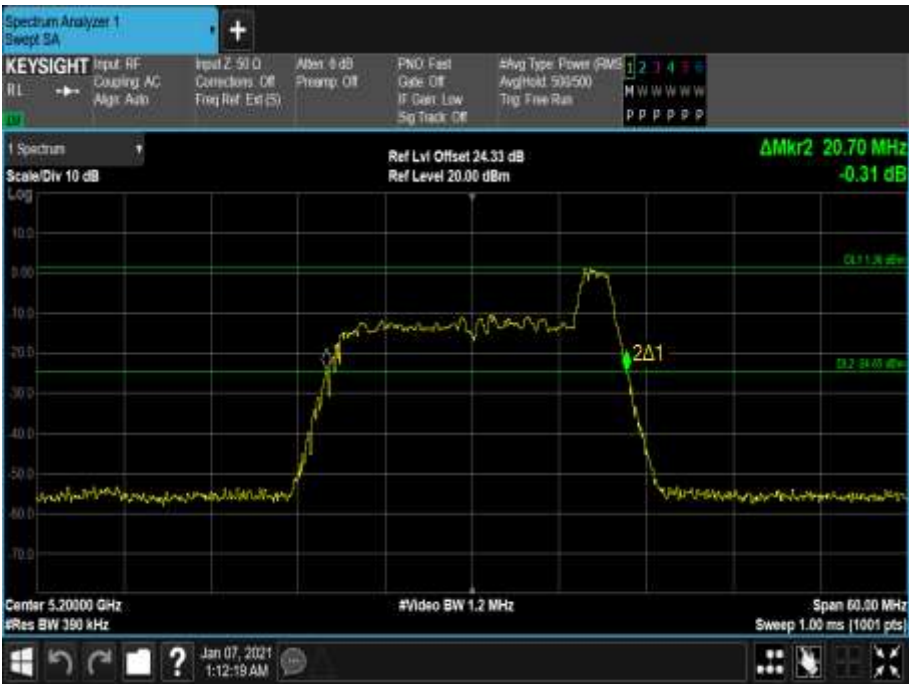
Figure 89 - 5200 MHz - 26 dB Emission Bandwidth
