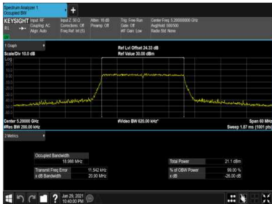
Figure 146 - 5200 MHz - 99% Occupied Bandwidth
