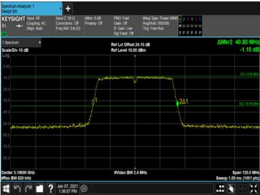
Figure 199 - 5190 MHz - 26 dB Emission Bandwidth
