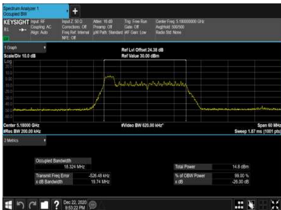
Figure 156 - 5180 MHz - 99% Occupied Bandwidth
