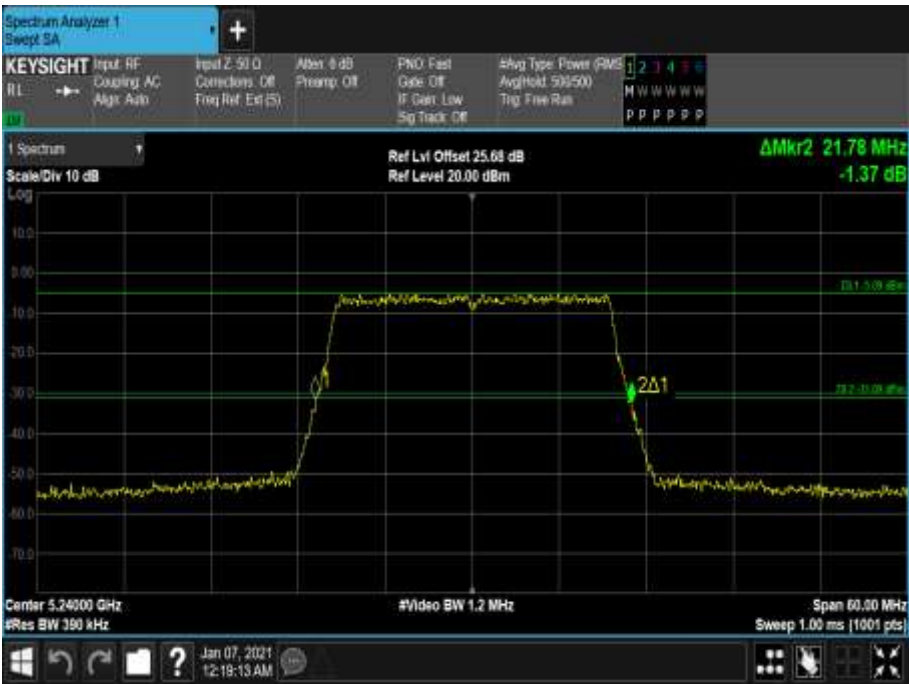
Figure 71 - 5240 MHz - 26 dB Emission Bandwidth
