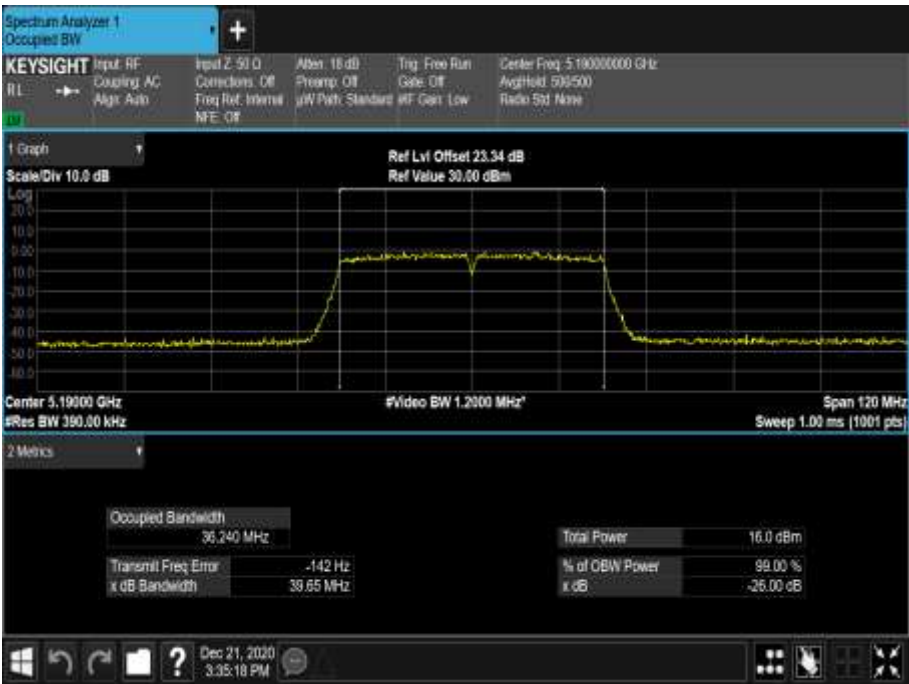
Figure 196 - 5190 MHz - 99% Occupied Bandwidth
