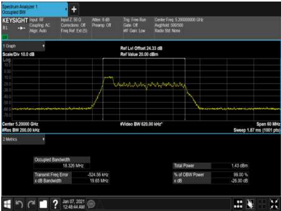
Figure 84 - 5200 MHz - 99% Occupied Bandwidth
