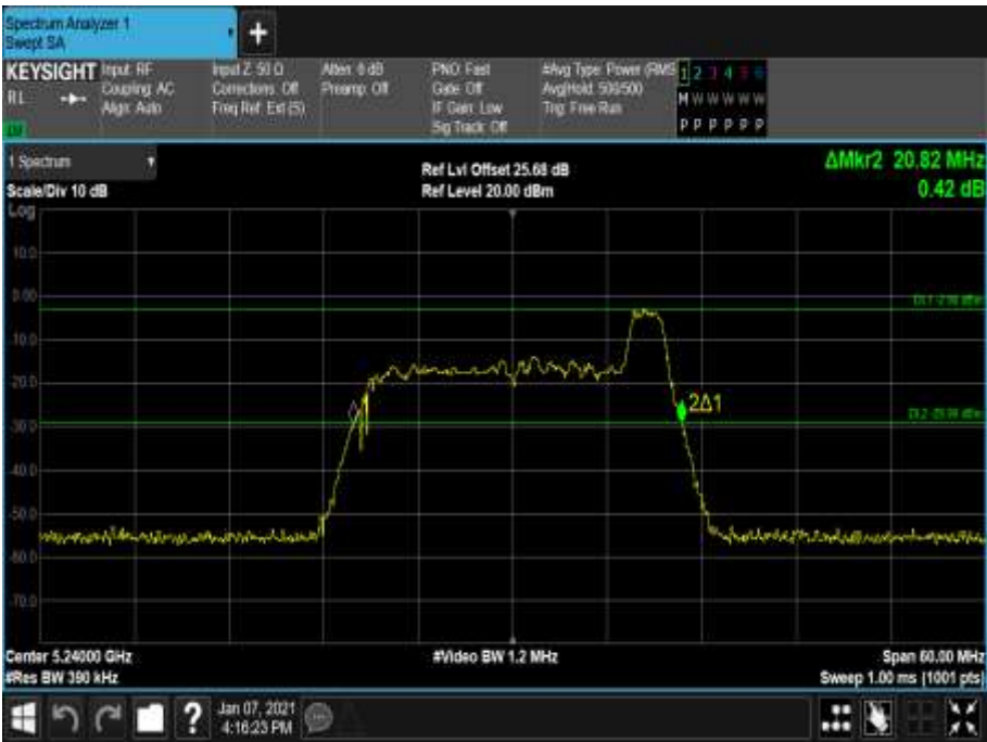
Figure 133 - 5240 MHz - 26 dB Emission Bandwidth
