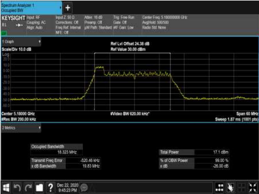
Figure 74 - 5180 MHz - 99% Occupied Bandwidth
