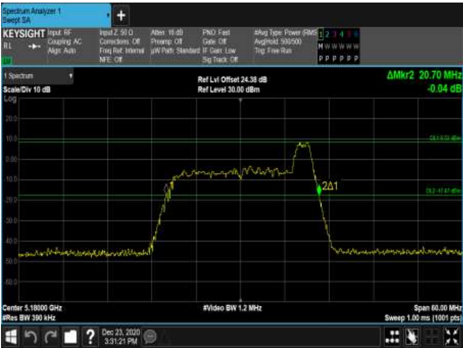
Figure 171 - 5180 MHz - 26 dB Emission Bandwidth
