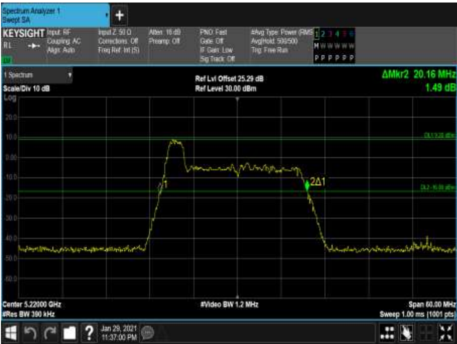
Figure 159 - 5220 MHz - 26 dB Emission Bandwidth
