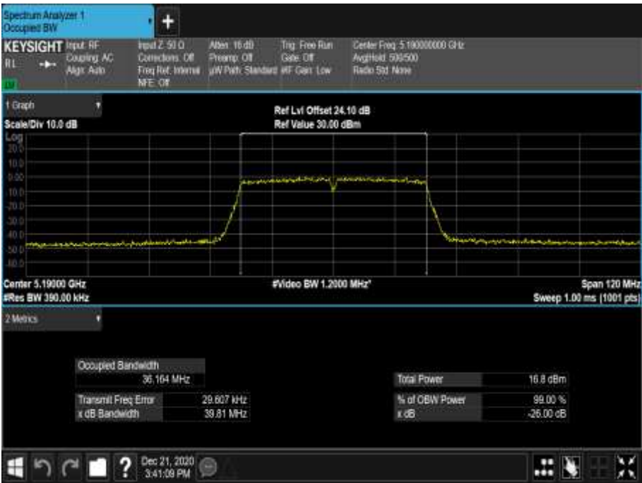
Figure 192 - 5190 MHz - 99% Occupied Bandwidth
