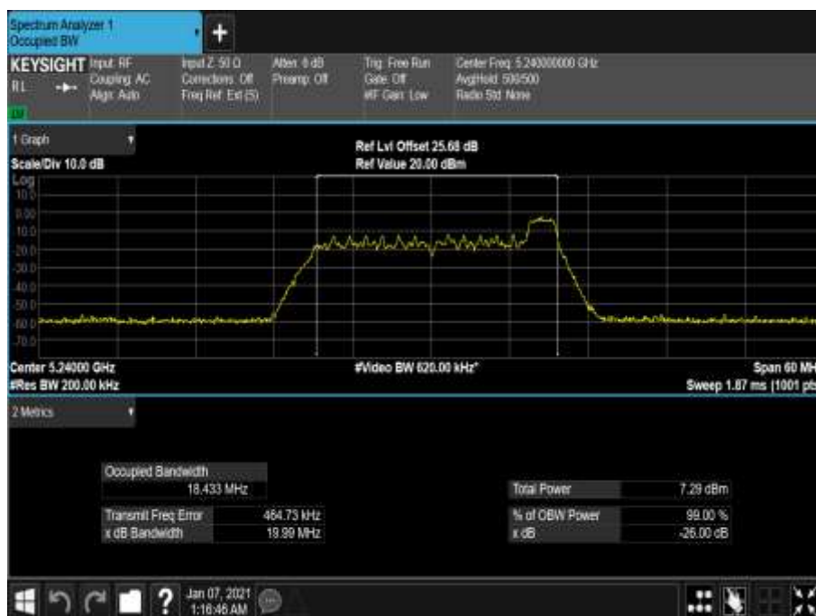
Figure 92 - 5240 MHz - 99% Occupied Bandwidth
