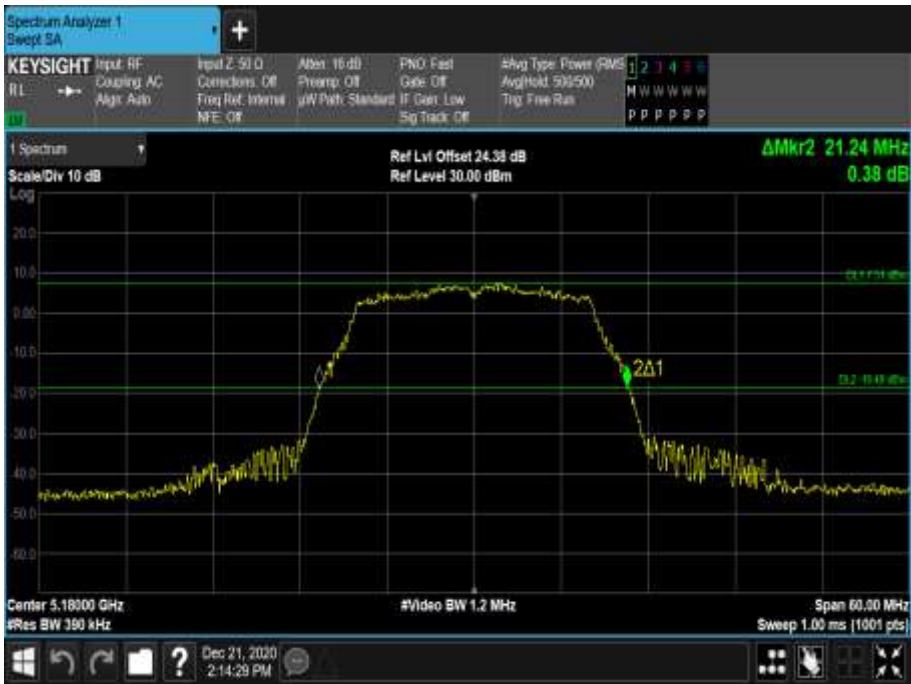
Figure 1 - 5180 MHz - 26 dB Emission Bandwidth
