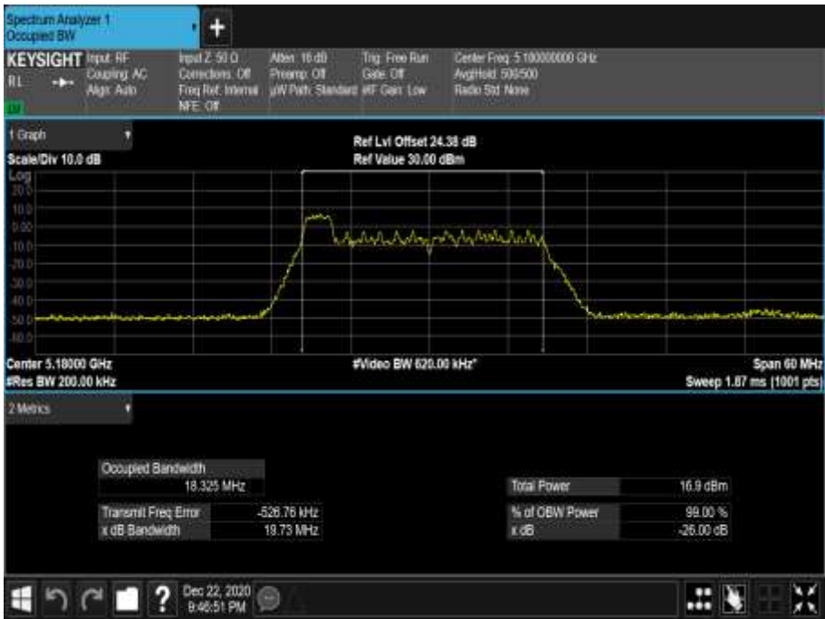
Figure 76 - 5180 MHz - 99% Occupied Bandwidth
