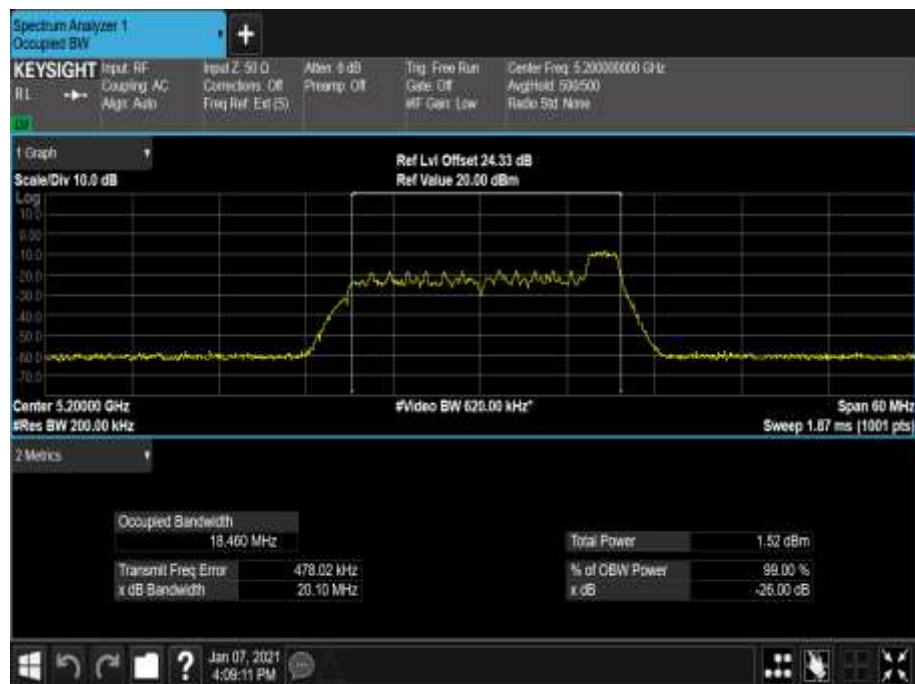
Figure 138 - 5200 MHz - 99% Occupied Bandwidth
