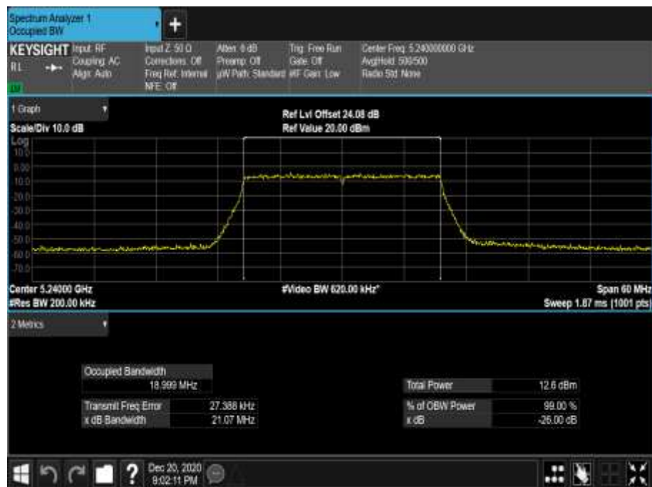
Figure 110 - 5240 MHz - 99% Occupied Bandwidth
