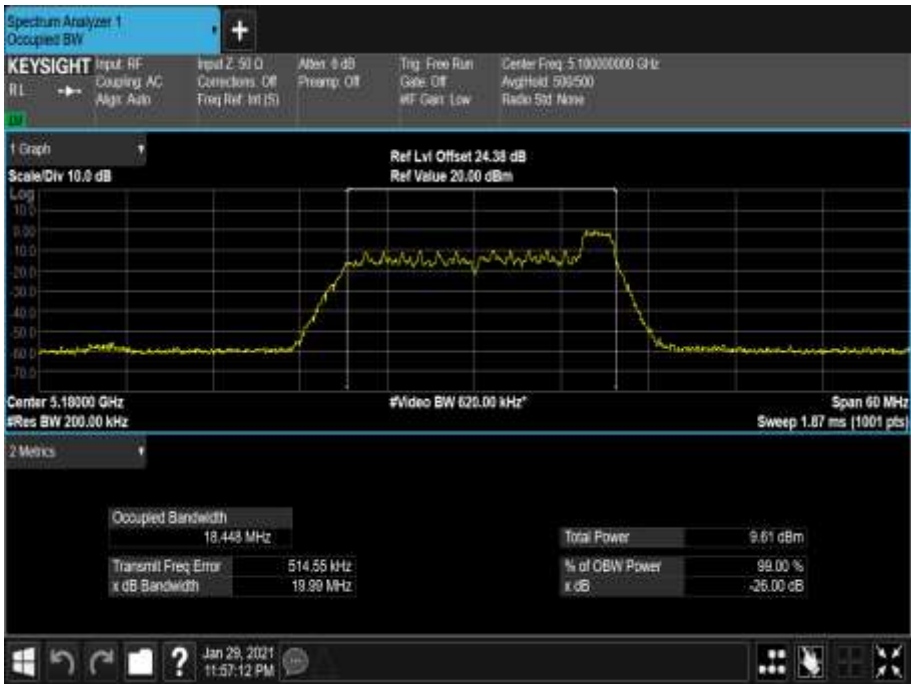
Figure 180 - 5180 MHz - 99% Occupied Bandwidth
