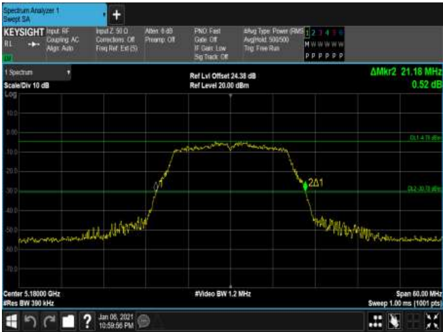
Figure 7 - 5180 MHz - 26 dB Emission Bandwidth
