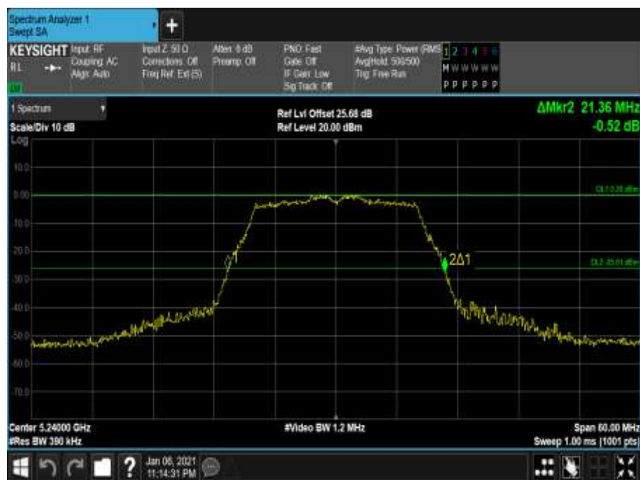
Figure 5 - 5240 MHz - 26 dB Emission Bandwidth
