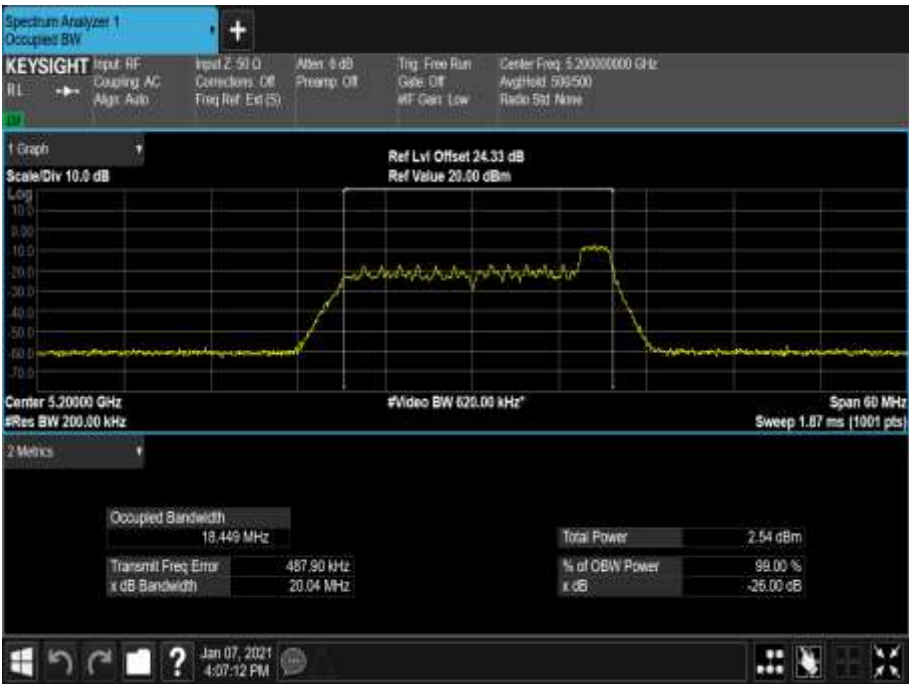
Figure 130 - 5200 MHz - 99% Occupied Bandwidth
