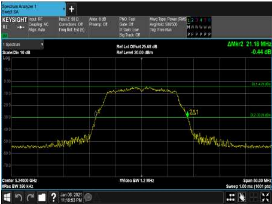
Figure 11 - 5240 MHz - 26 dB Emission Bandwidth
