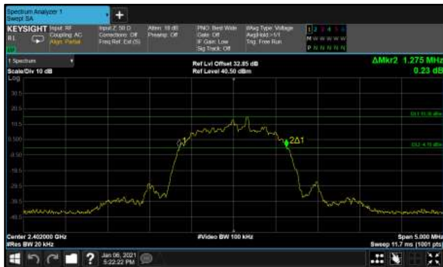
Figure 28 - Core0 (C) 2402 MHz (CH0) 20 dB Bandwidth
