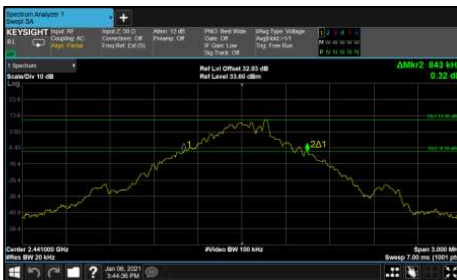
Figure 44 - Core2 (A) 2441 MHz (CH39) 20 dB Bandwidth
