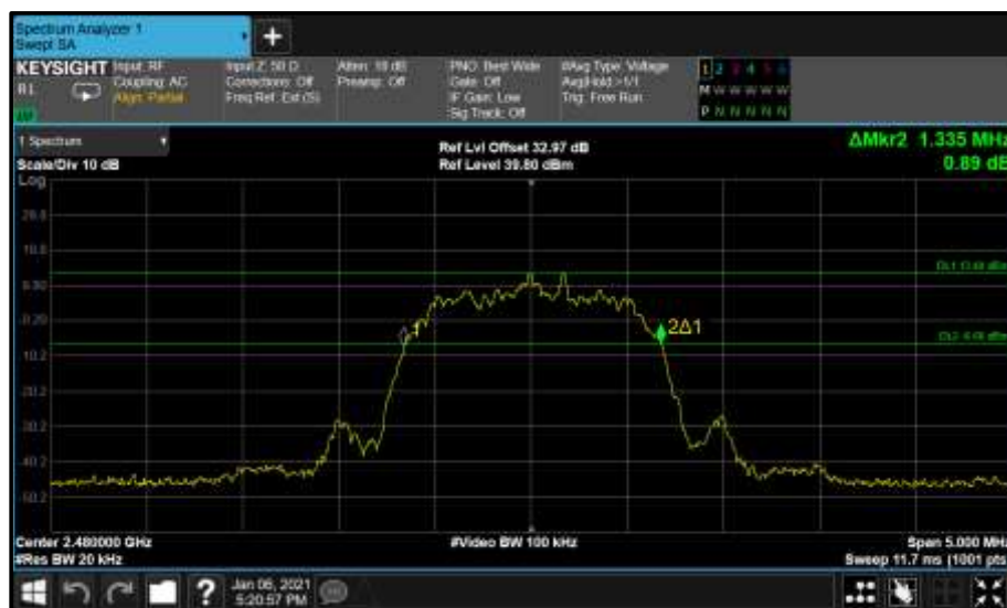
Figure 27 - Core0 (C) 2480 MHz (CH78) 20 dB Bandwidth
