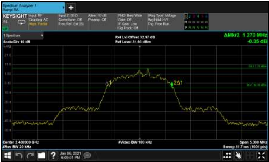
Figure 78 - Core0 (C) 2480 MHz (CH78) 20 dB Bandwidth
