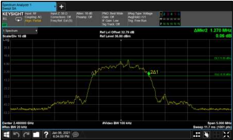
Figure 41 - Core1 (B) 2480 MHz (CH78) 20 dB Bandwidth
