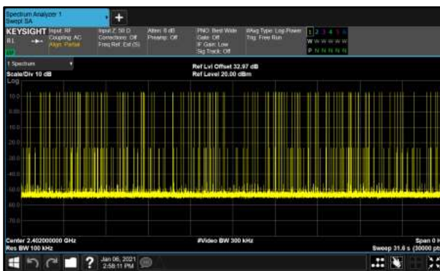
Figure 3 - GFSK - 2402 MHz Accumulated Transmit Time
