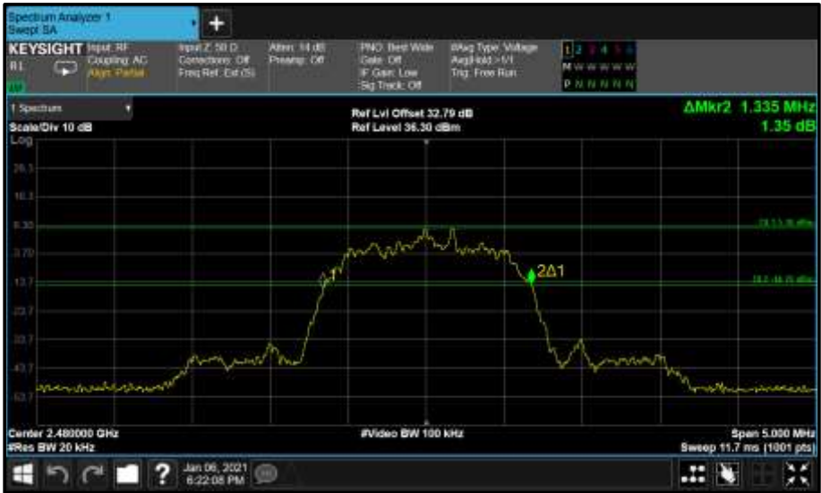
Figure 35 - Core1 (B) 2480 MHz (CH78) 20 dB Bandwidth
