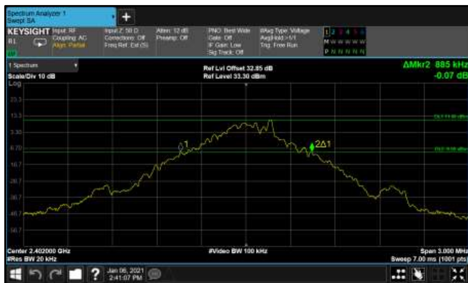
Figure 46 - Core0 (C) 2402 MHz (CH0) 20 dB Bandwidth
