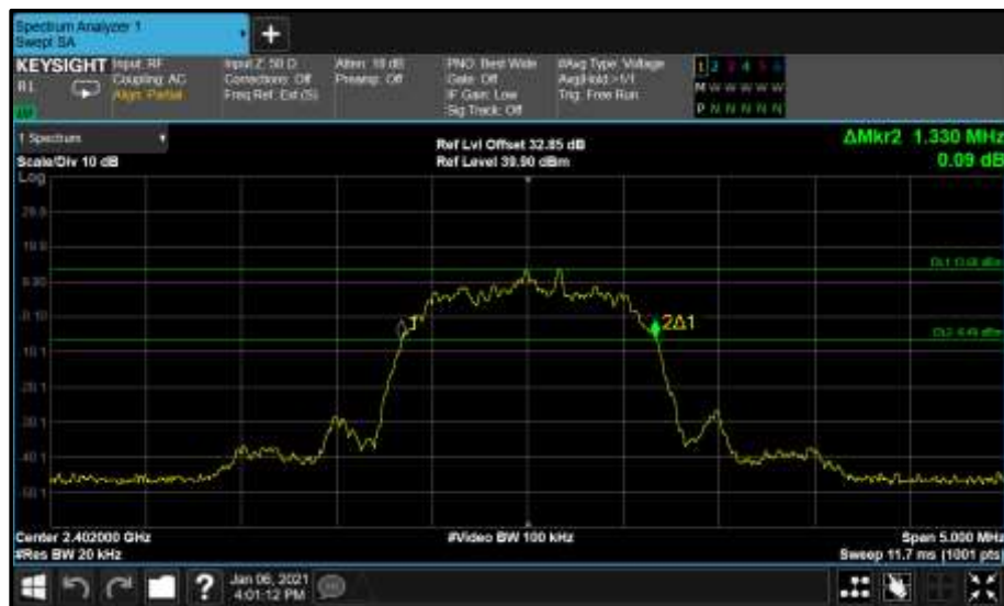
Figure 25 - Core0 (C) 2402 MHz (CH0) 20 dB Bandwidth
