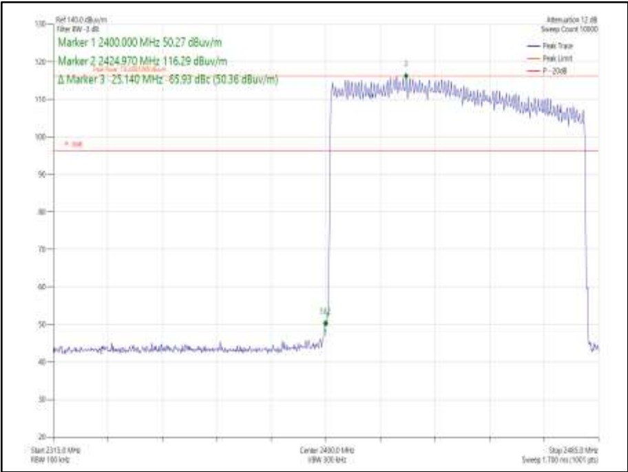
Figure 102 - Hopping - Core 0, 8-DPSK/3DH5 - Band Edge Frequency 2400.0 MHz
