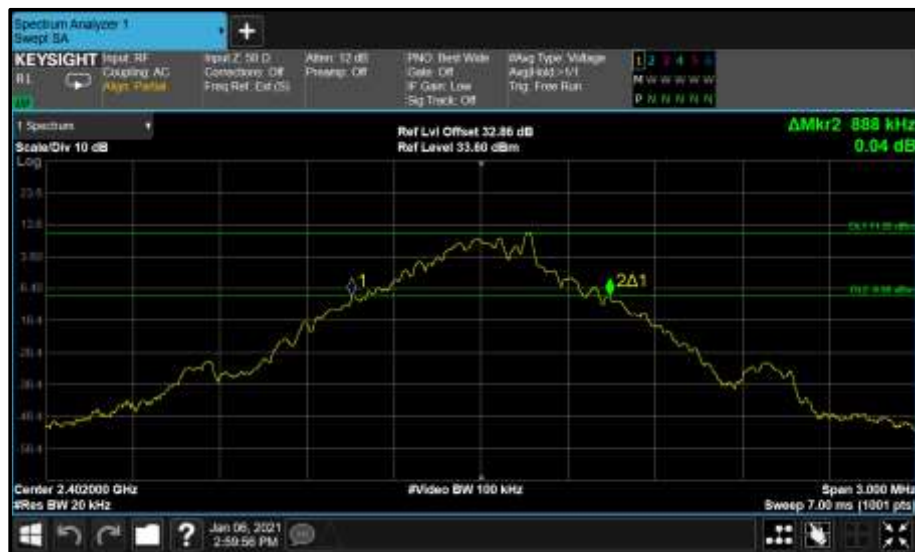
Figure 43 - Core2 (A) 2402 MHz (CH0) 20 dB Bandwidth
