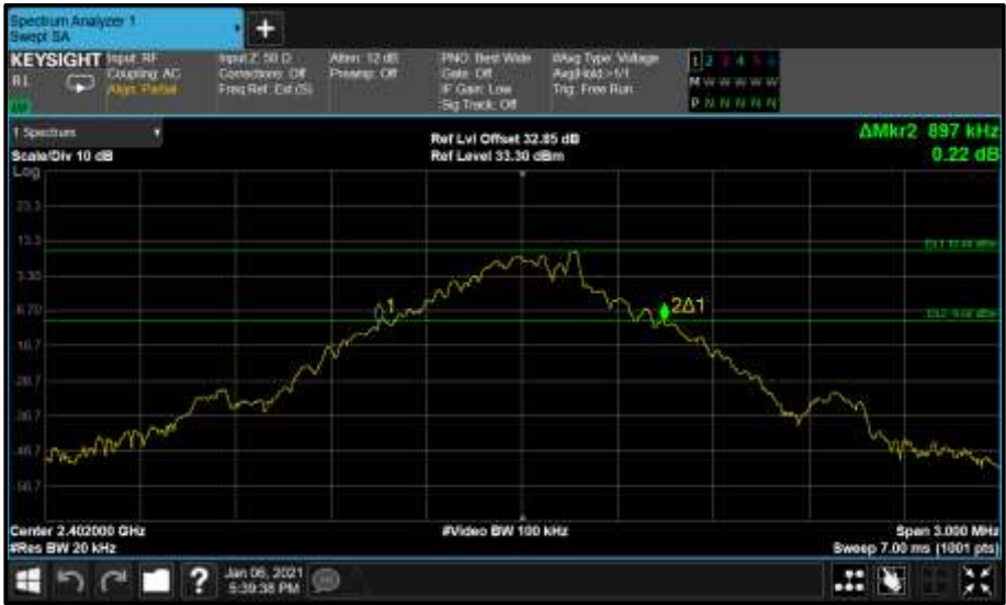
Figure 50 - Core0 (C) 2402 MHz (CH0) 20 dB Bandwidth
