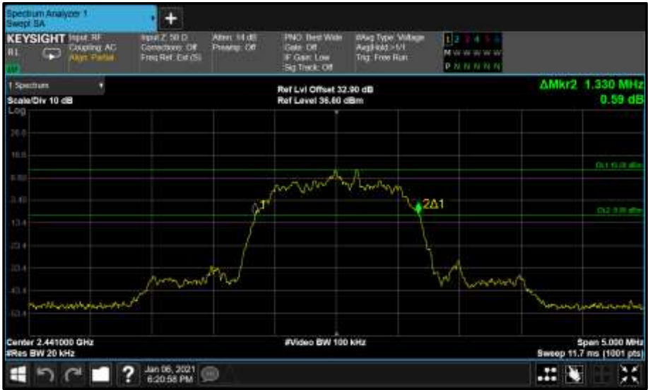
Figure 34 - Core0 (C) 2441 MHz (CH39) 20 dB Bandwidth
