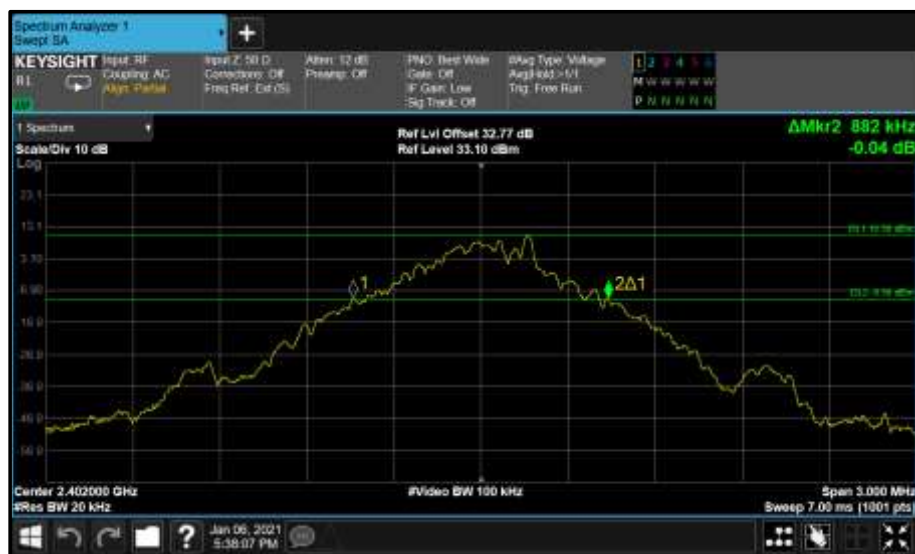
Figure 49 - Core1 (B) 2402 MHz (CH0) 20 dB Bandwidth
