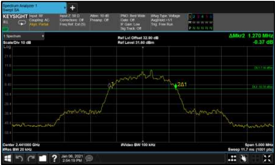
Figure 65 - Core0 (C) 2441 MHz (CH39) 20 dB Bandwidth
