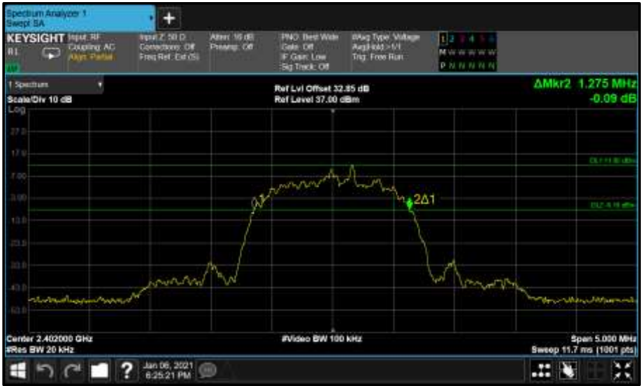
Figure 38 - Core0 (C) 2402 MHz (CH0) 20 dB Bandwidth
