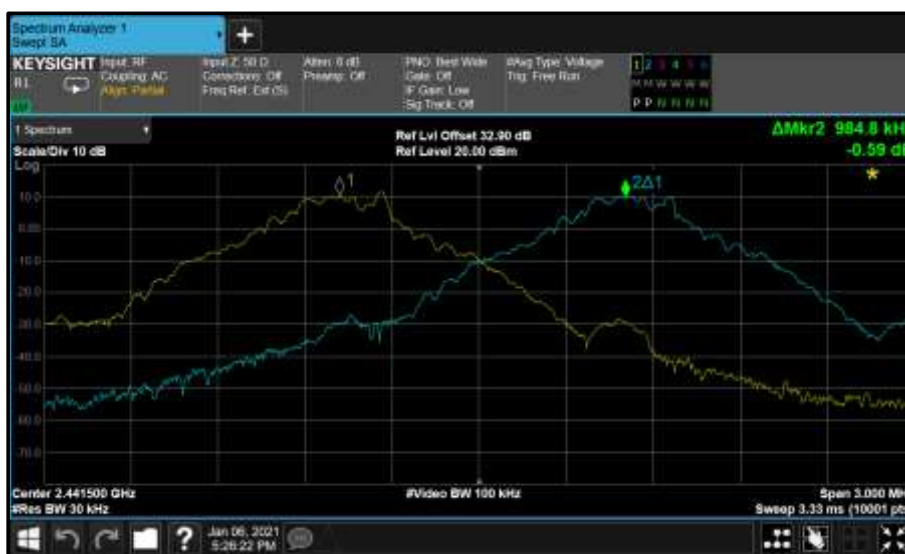
Figure 4 - GFSK - 2441 MHz (CH39)
