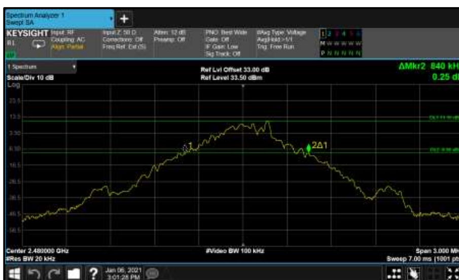
Figure 45 - Core2 (A) 2480 MHz (CH78) 20 dB Bandwidth
