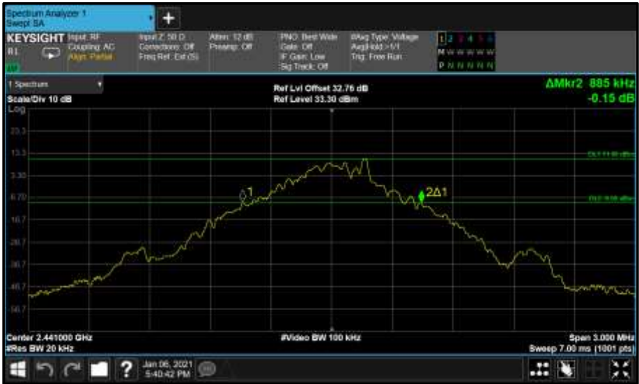
Figure 51 - Core1 (B) 2441 MHz (CH39) 20 dB Bandwidth
