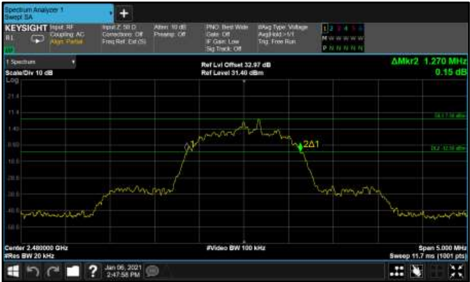
Figure 66 - Core0 (C) 2480 MHz (CH78) 20 dB Bandwidth
