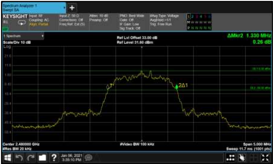
Figure 57 - Core2 (A) 2480 MHz (CH78) 20 dB Bandwidth
