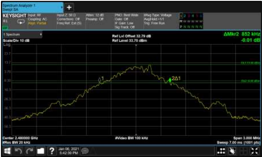
Figure 53 - Core1 (B) 2480 MHz (CH78) 20 dB Bandwidth
