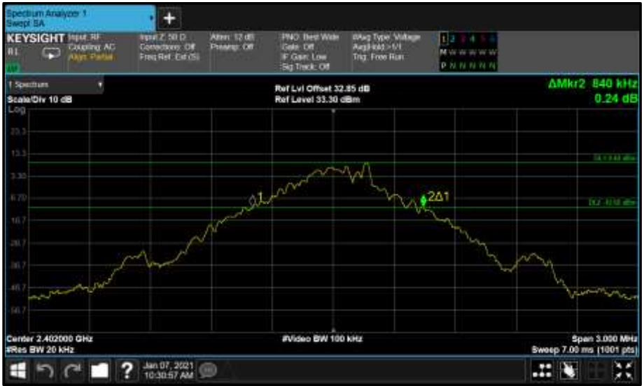
Figure 20 - Core0 (C) 2402 MHz (CH0) 20 dB Bandwidth
