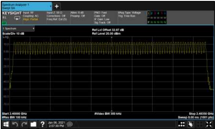
Figure 15 - GFSK (DH5) - Number of Hopping Channels
