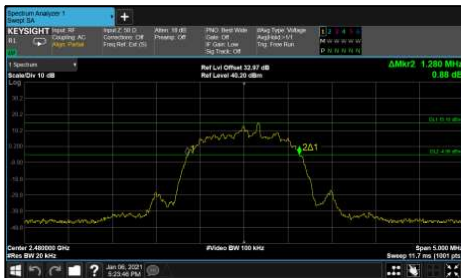
Figure 30 - Core0 (C) 2480 MHz (CH78) 20 dB Bandwidth
