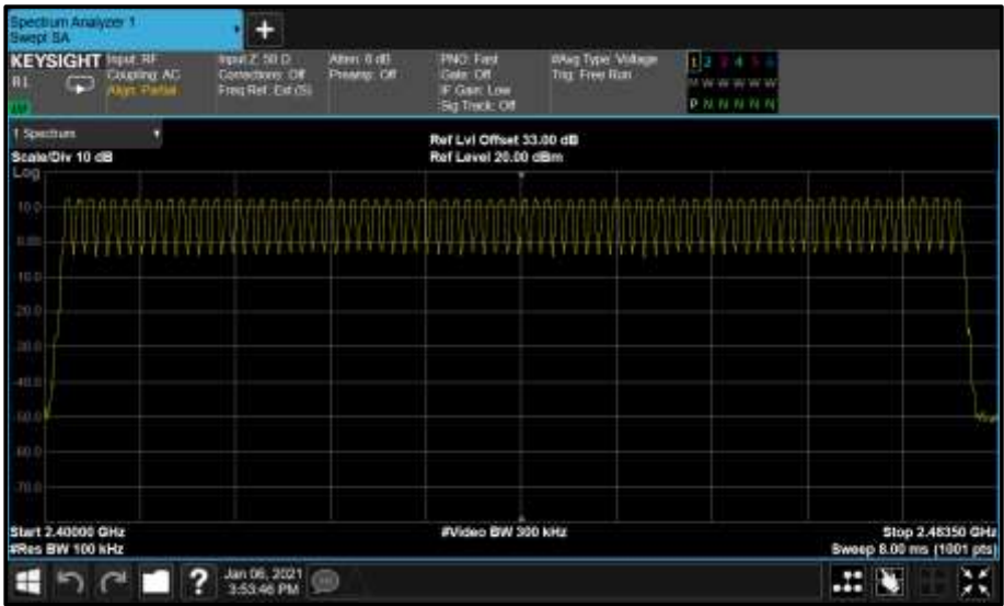
Figure 14 - GFSK (DH5) - Number of Hopping Channels
