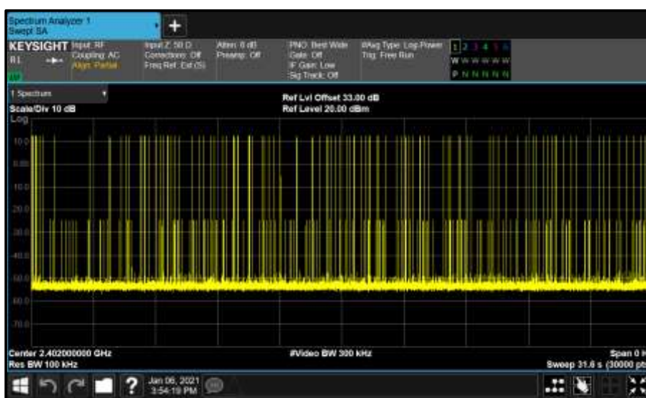
Figure 2 - GFSK - 2402 MHz Accumulated Transmit Time
