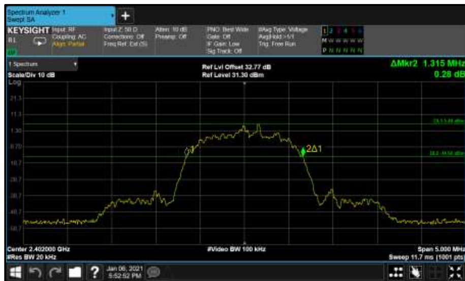
Figure 73 - Core1 (B) 2402 MHz (CH0) 20 dB Bandwidth
