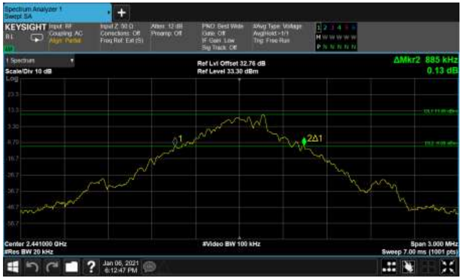
Figure 21 - Core1 (B) 2441 MHz (CH39) 20 dB Bandwidth
