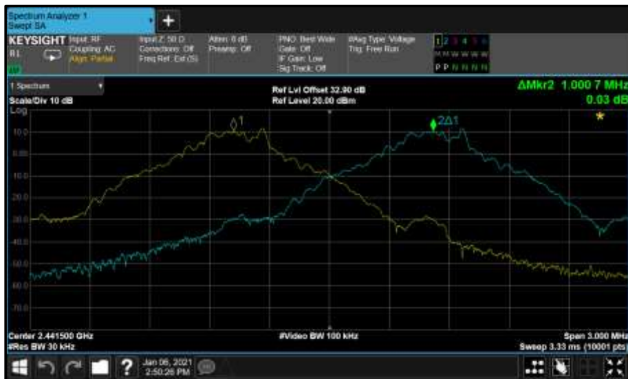
Figure 10 - GFSK - 2441 MHz (CH39)
