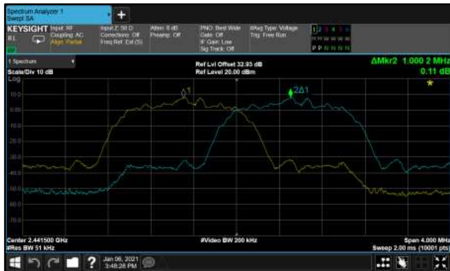
Figure 8 - \pi/4 DQPSK - 2441 MHz (CH39)
