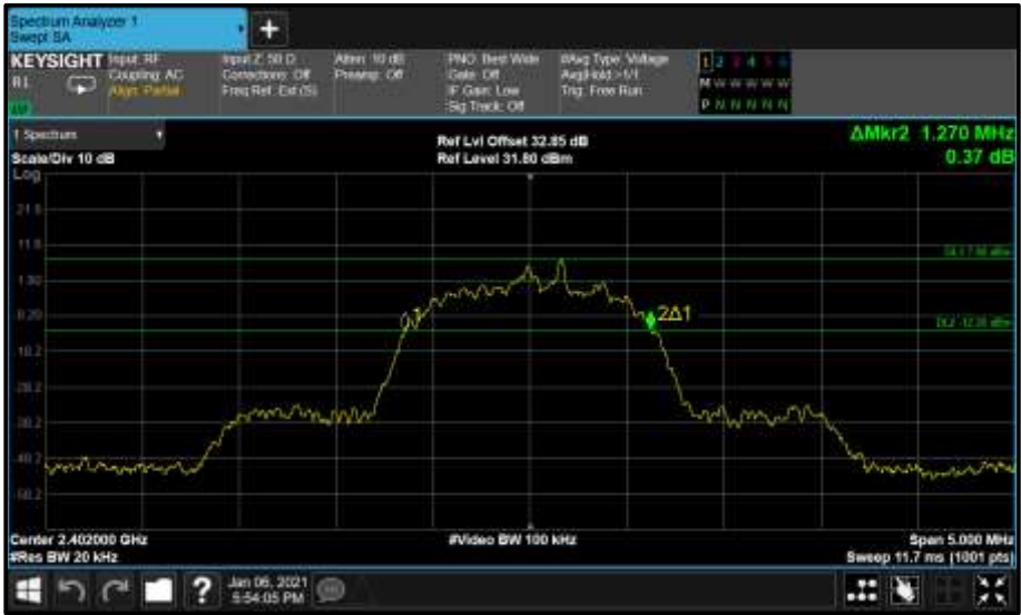
Figure 74 - Core0 (C) 2402 MHz (CH0) 20 dB Bandwidth
