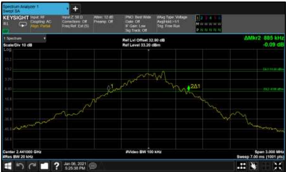
Figure 17 - Core0 (C) 2441 MHz (CH39) 20 dB Bandwidth
