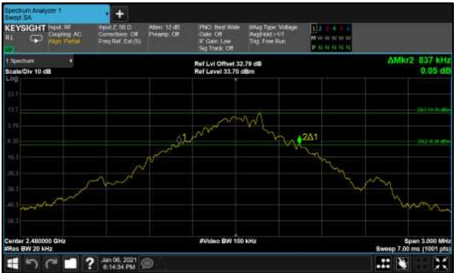
Figure 23 - Core1 (B) 2480 MHz (CH78) 20 dB Bandwidth
