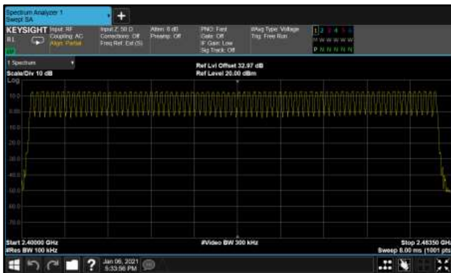
Figure 13 - GFSK (DH5) - Number of Hopping Channels
