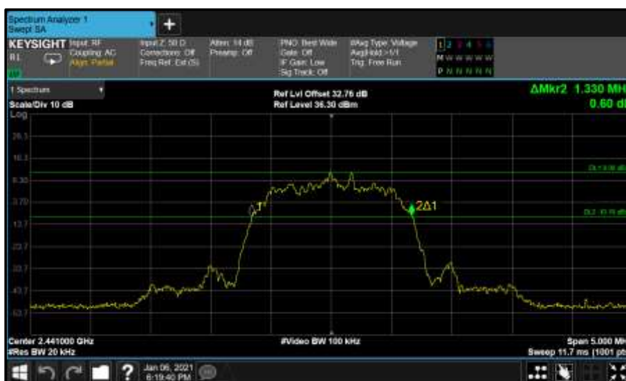
Figure 33 - Core1 (B) 2441 MHz (CH39) 20 dB Bandwidth
