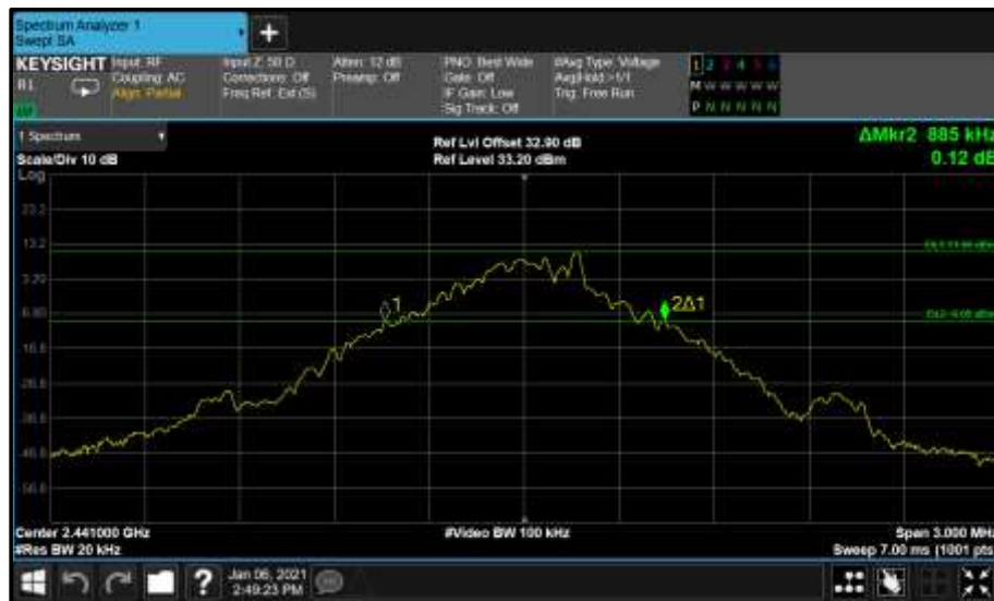
Figure 47 - Core0 (C) 2441 MHz (CH39) 20 dB Bandwidth
