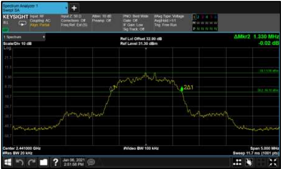
Figure 62 - Core0 (C) 2441 MHz (CH39) 20 dB Bandwidth
