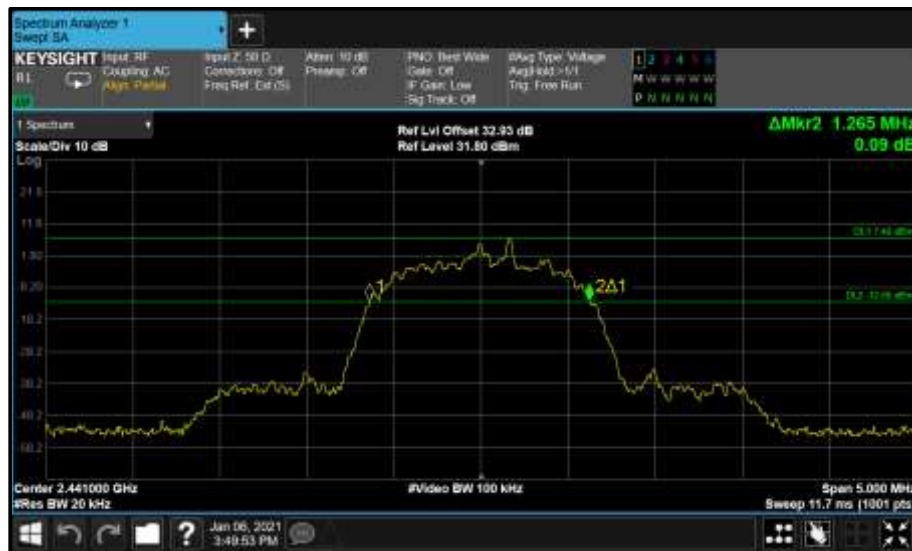
Figure 59 - Core2 (A) 2441 MHz (CH39) 20 dB Bandwidth
