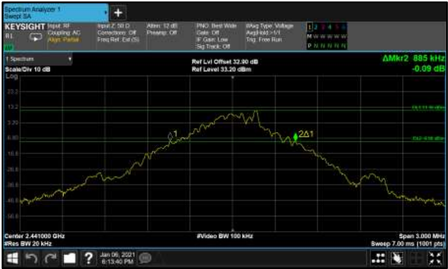
Figure 22 - Core0 (C) 2441 MHz (CH39) 20 dB Bandwidth
