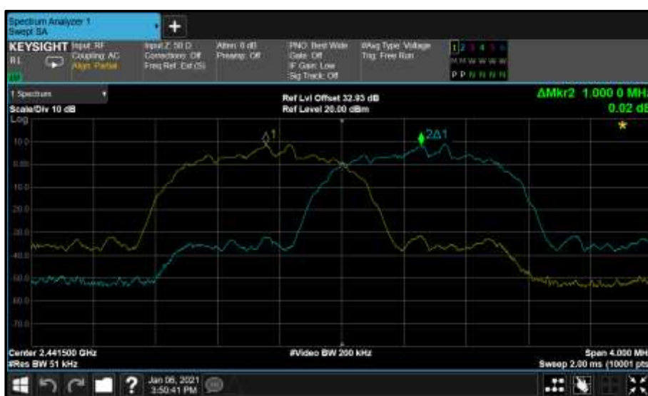
Figure 9 - 8-DPSK - 2441 MHz (CH39)
