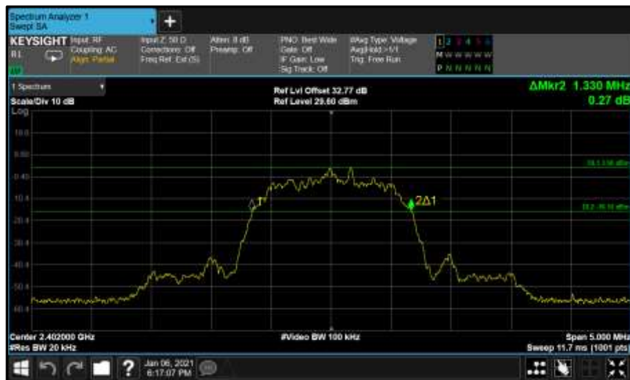
Figure 31 - Core1 (B) 2402 MHz (CH0) 20 dB Bandwidth
