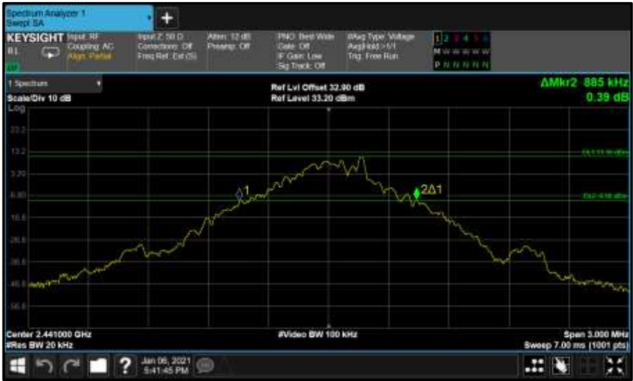
Figure 52 - Core0 (C) 2441 MHz (CH39) 20 dB Bandwidth
