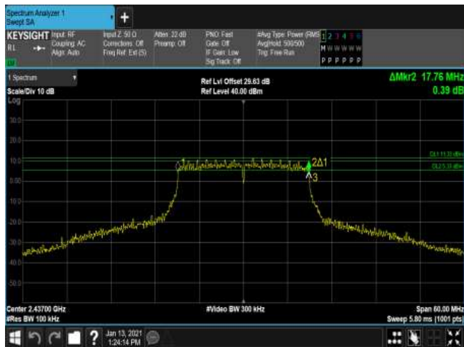
Figure 21 - 2437 MHz - 6 dB DTS Bandwidth
