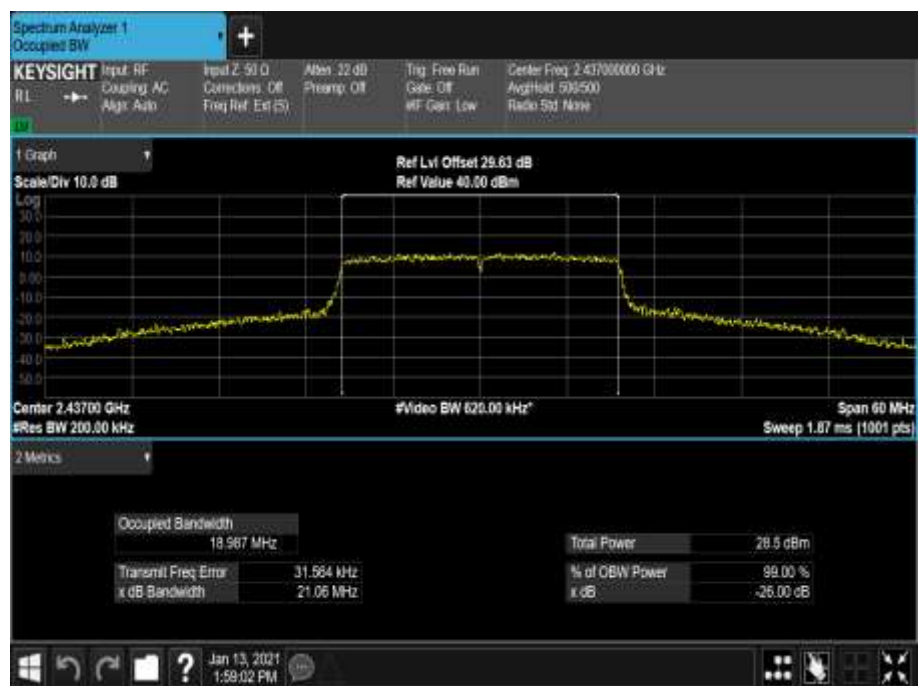
Figure 46 - 2437 MHz - 99% Occupied Bandwidth
