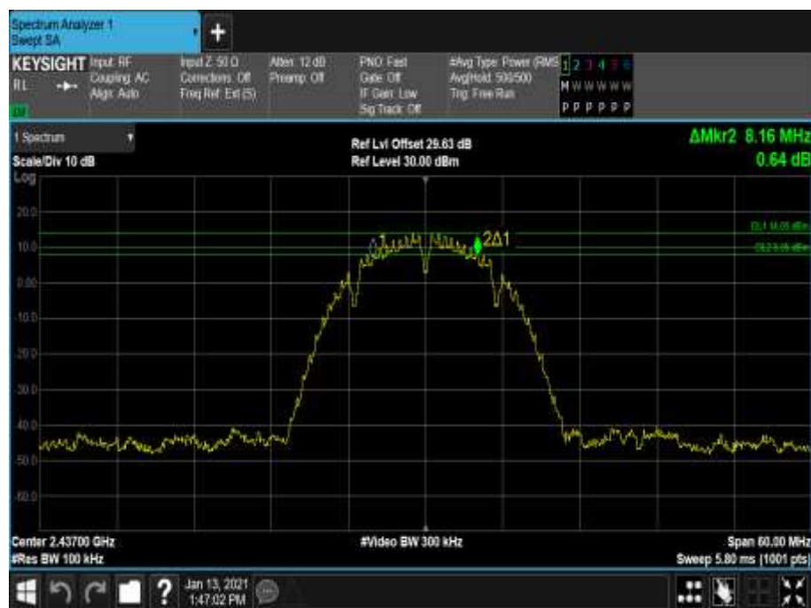
Figure 3 - 2437 MHz - 6 dB DTS Bandwidth
