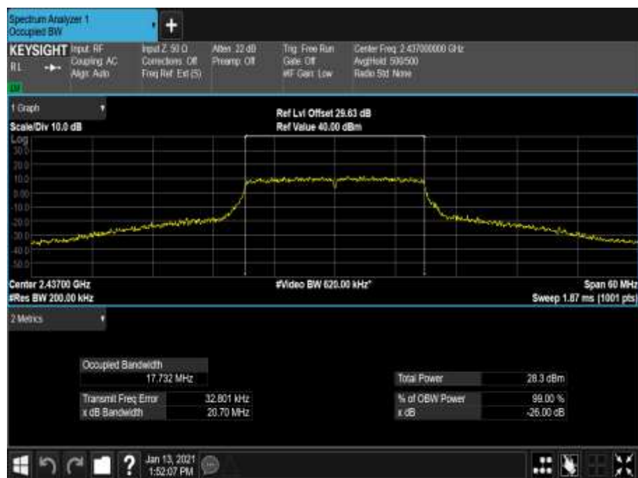
Figure 16 - 2437 MHz - 99% Occupied Bandwidth
