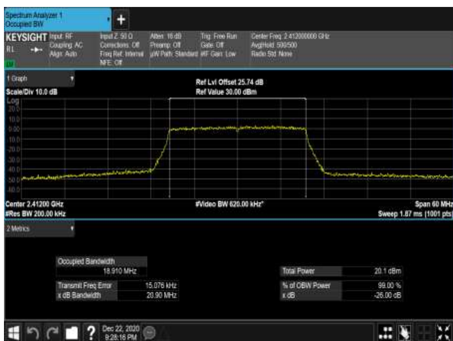
Figure 26 - 2412 MHz - 99% Occupied Bandwidth
