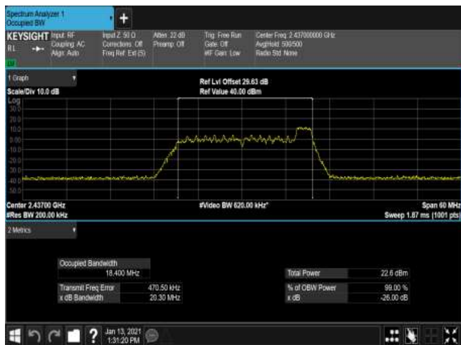
Figure 58 - 2437 MHz - 99% Occupied Bandwidth
