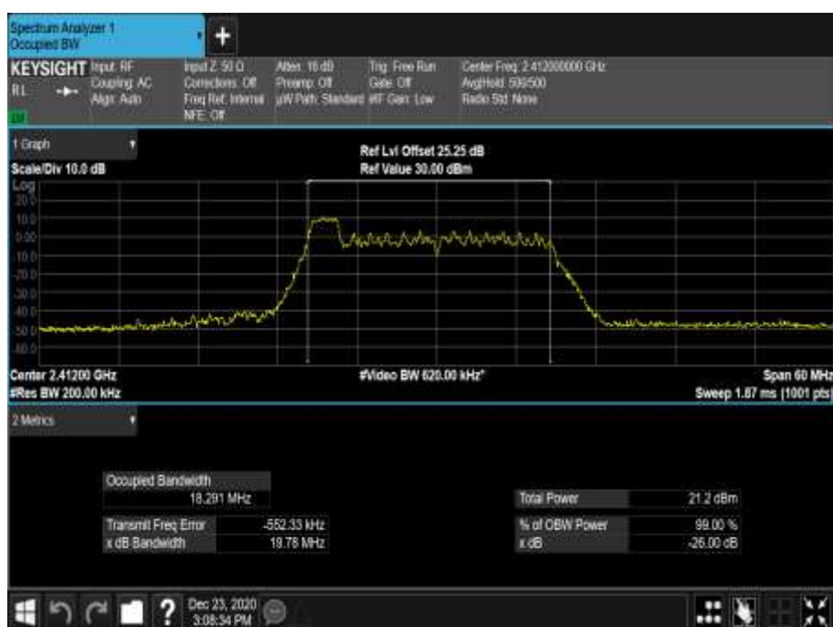
Figure 50 - 2412 MHz - 99% Occupied Bandwidth
