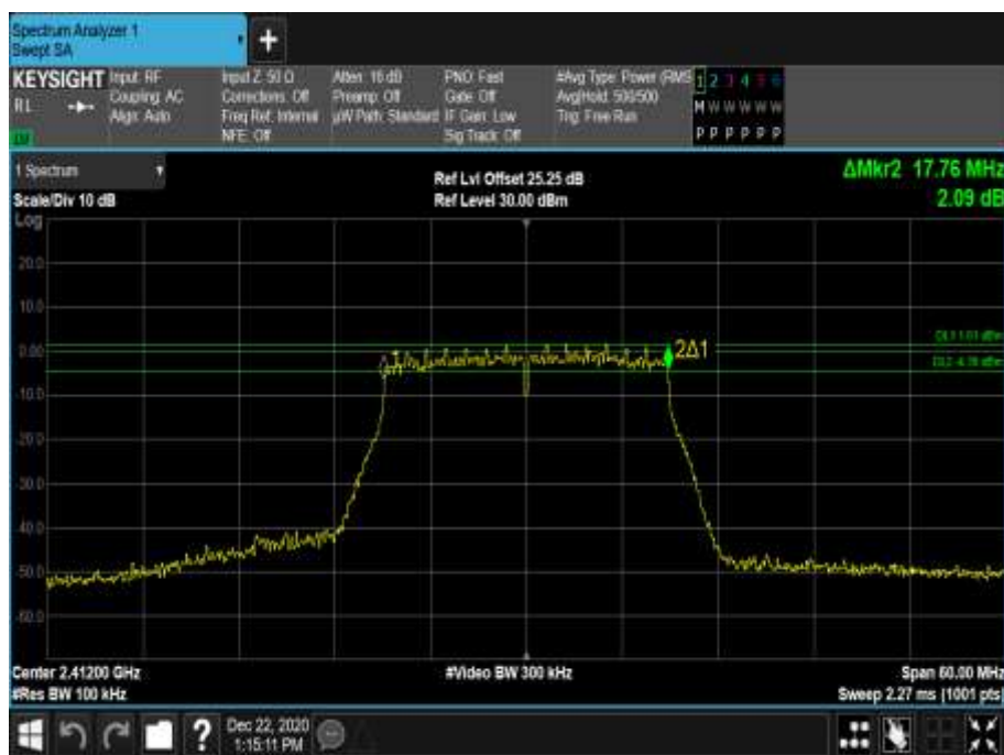
Figure 19 - 2412 MHz - 6 dB DTS Bandwidth
