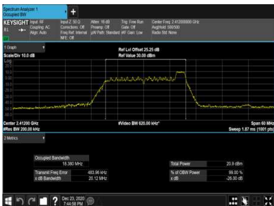
Figure 56 - 2412 MHz - 99% Occupied Bandwidth
