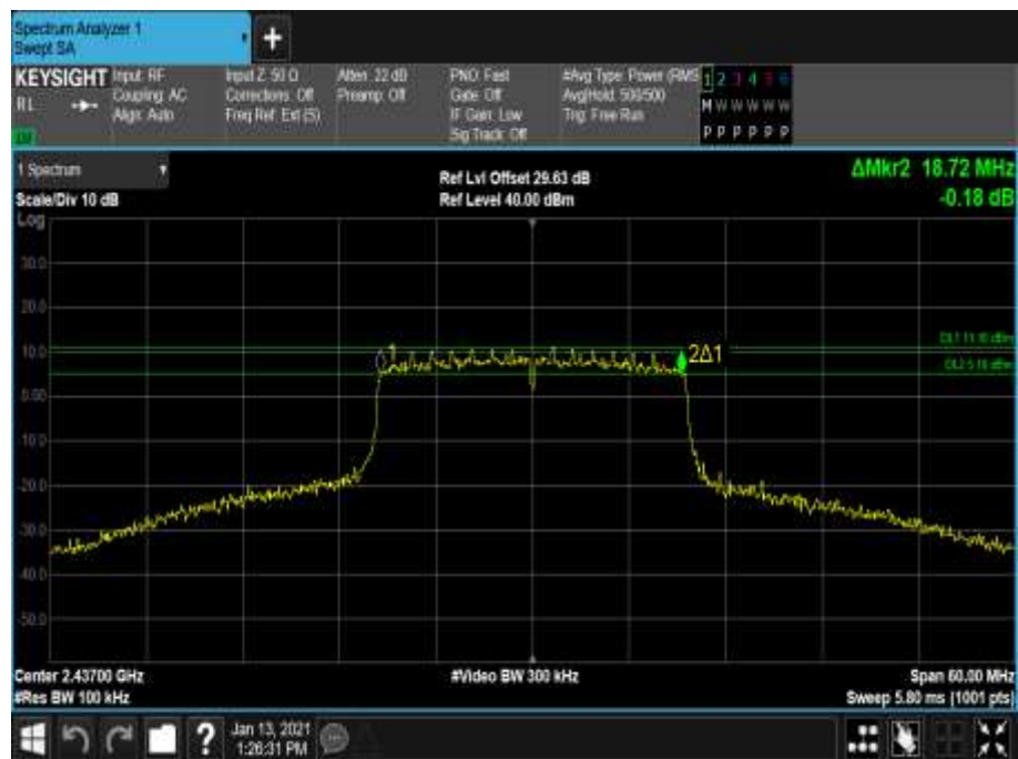
Figure 45 - 2437 MHz - 6 dB DTS Bandwidth
