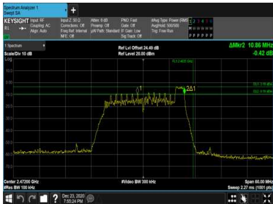
Figure 59 - 2472 MHz - 6 dB DTS Bandwidth
