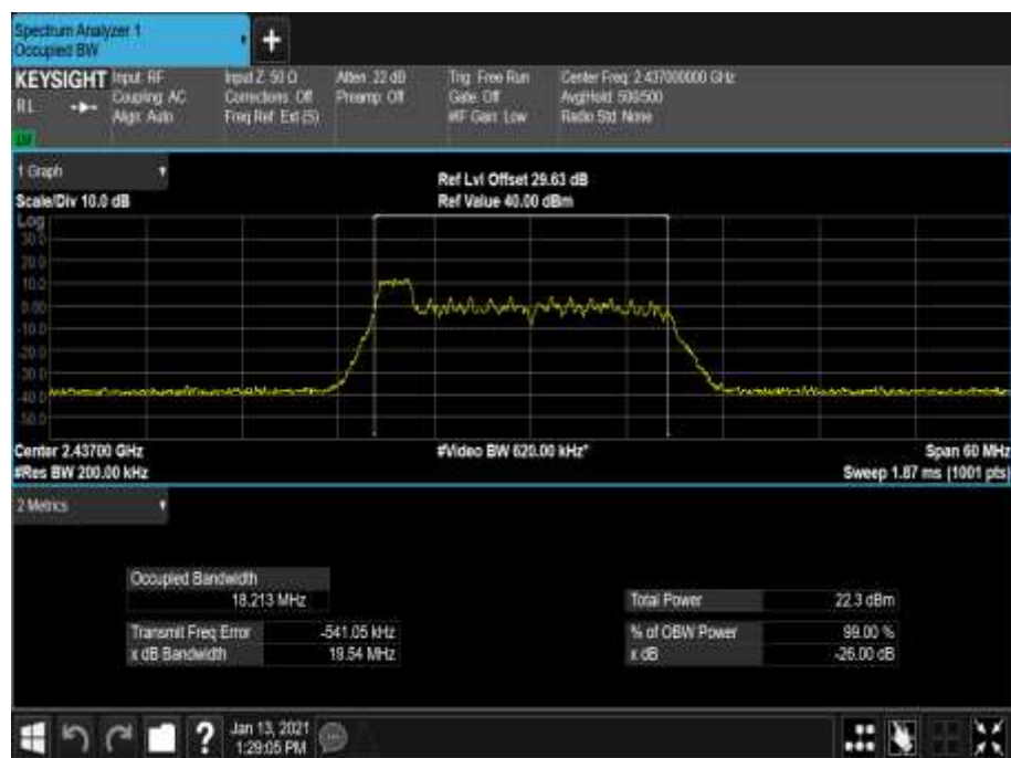
Figure 52 - 2437 MHz - 99% Occupied Bandwidth
