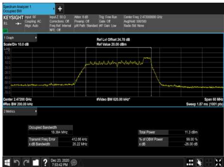
Figure 42 - 2472 MHz - 99% Occupied Bandwidth
