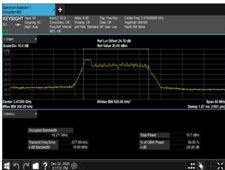
Figure 36 - 2472 MHz - 99% Occupied Bandwidth
