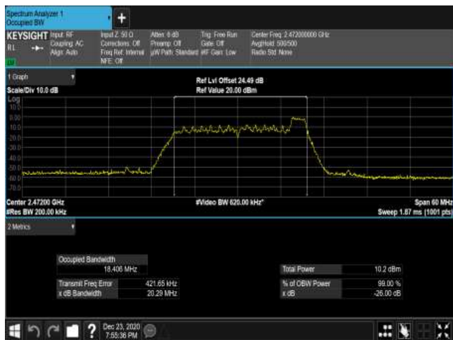
Figure 60 - 2472 MHz - 99% Occupied Bandwidth
