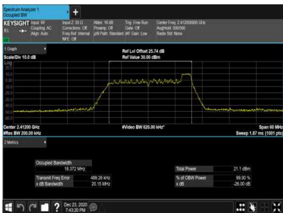
Figure 38 - 2412 MHz - 99% Occupied Bandwidth
