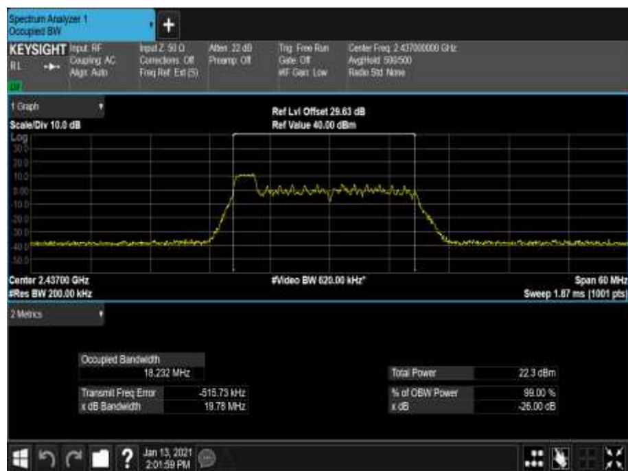
Figure 34 - 2437 MHz - 99% Occupied Bandwidth
