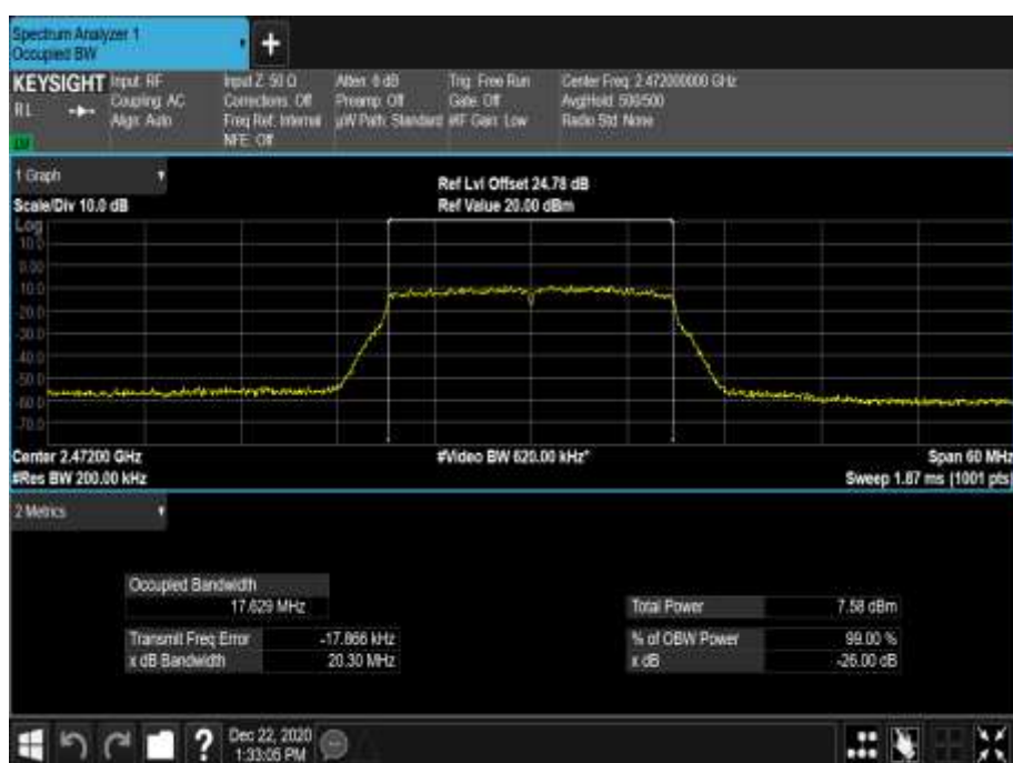
Figure 18 - 2472 MHz - 99% Occupied Bandwidth
