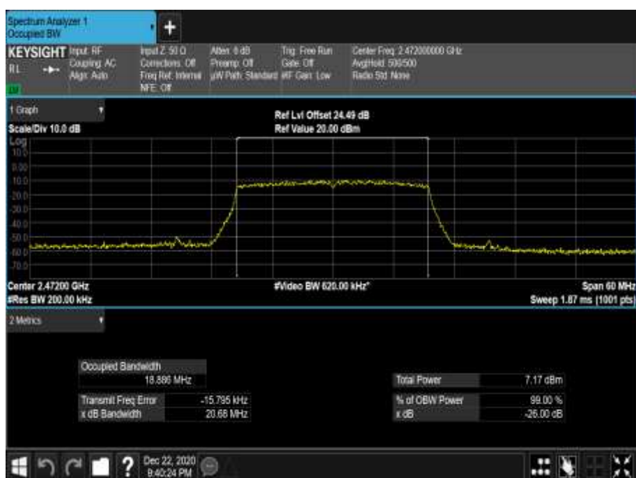
Figure 48 - 2472 MHz - 99% Occupied Bandwidth
