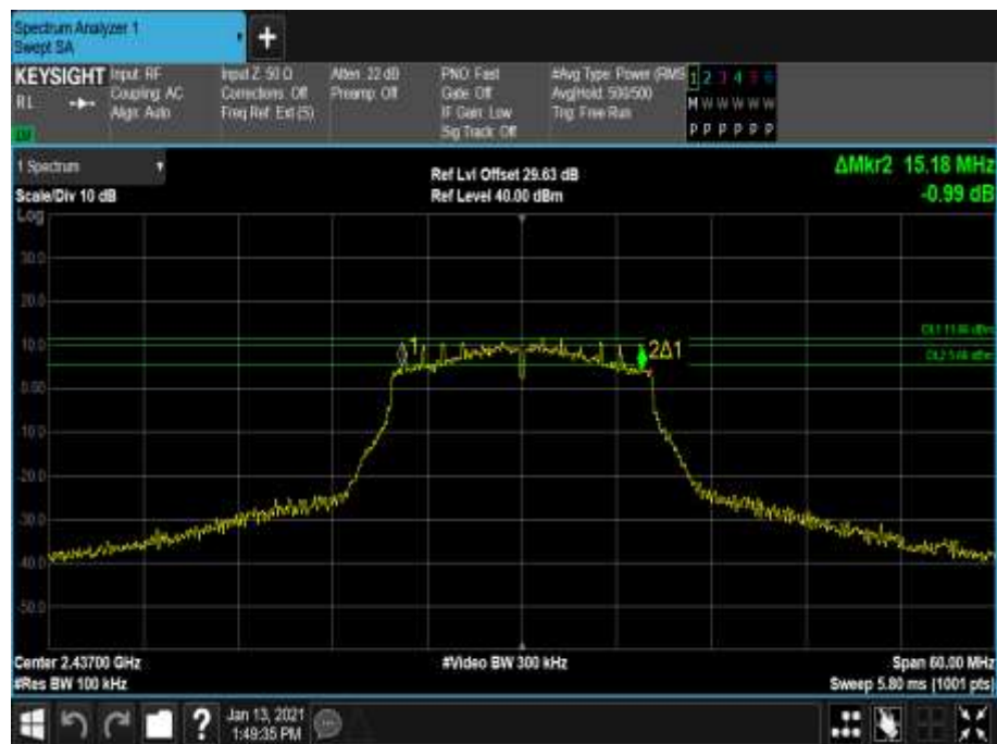
Figure 9 - 2437 MHz - 6 dB DTS Bandwidth
