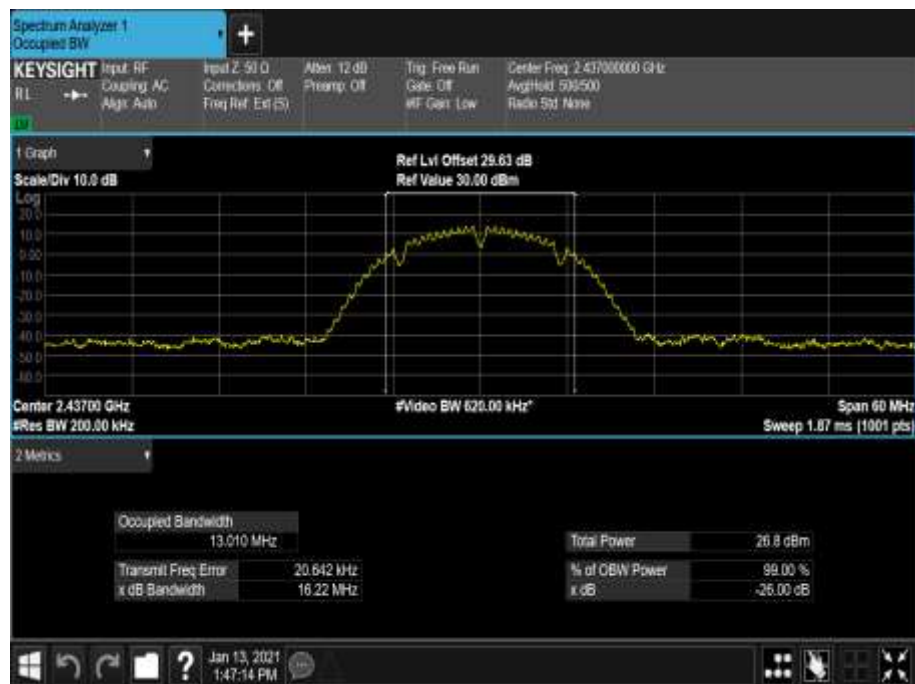
Figure 4 - 2437 MHz - 99% Occupied Bandwidth
