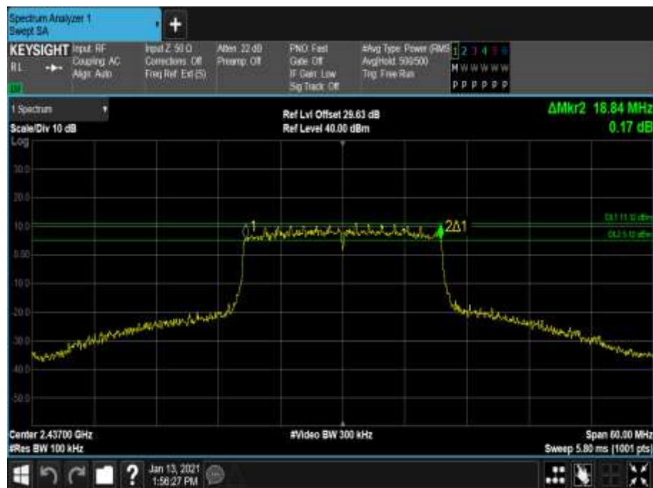
Figure 27 - 2437 MHz - 6 dB DTS Bandwidth
