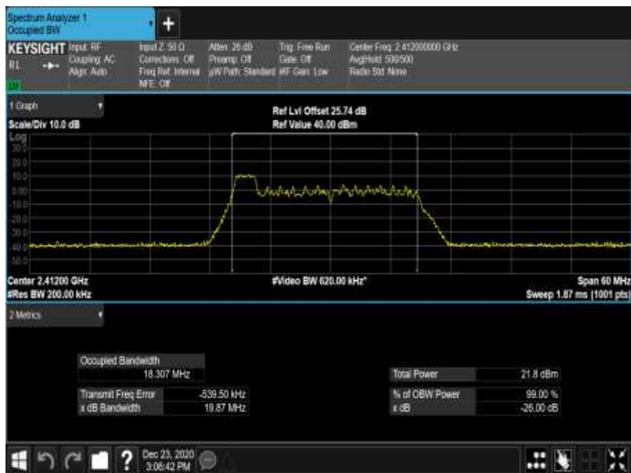
Figure 32 - 2412 MHz - 99% Occupied Bandwidth
