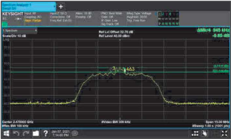
Figure 34 - Core1 (B) 2478 MHz (CH76) 6 dB Bandwidth
