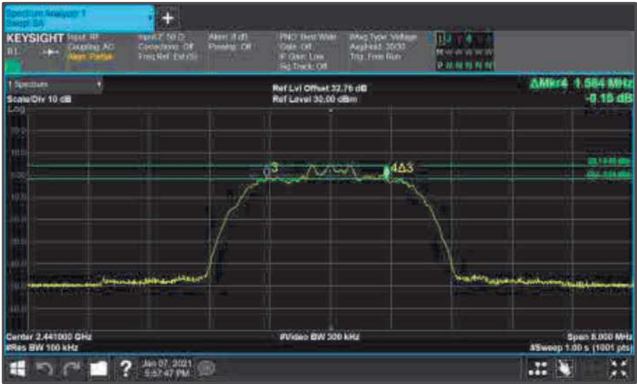
Figure 102 - Core1 (B) 2441 MHz (CH39) 6 dB Bandwidth
