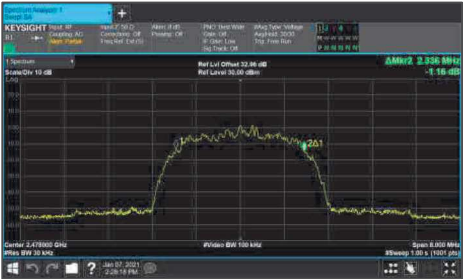
Figure 89 - Core0 (C) 2478 MHz (CH76) 99% Bandwidth
