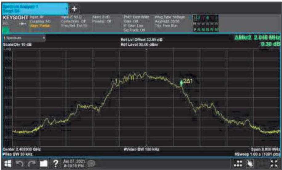
Figure 63 - Core0 (C) 2402 MHz (CH0) 99% Bandwidth
