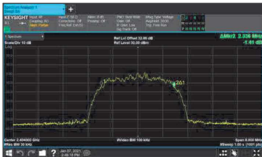
Figure 73 - Core2 (A) 2404 MHz (CH2) 99% Bandwidth
