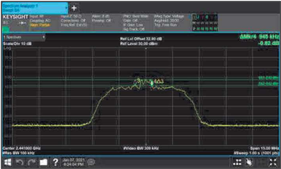
Figure 116 - Core0 (C) 2441 MHz (CH39) 6 dB Bandwidth
