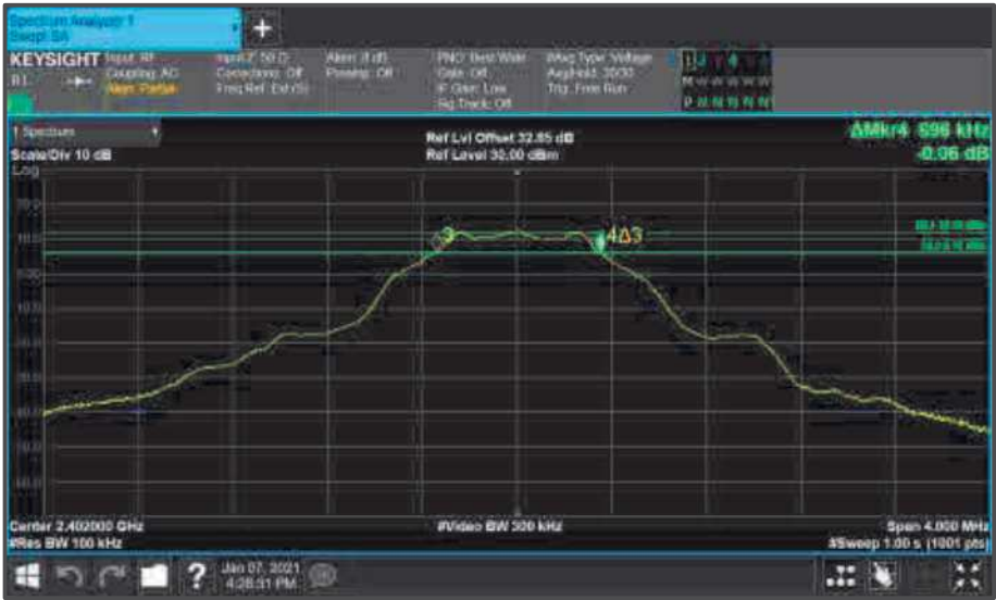
Figure 134 - Core0 (C) 2402 MHz (CH0) 6 dB Bandwidth
