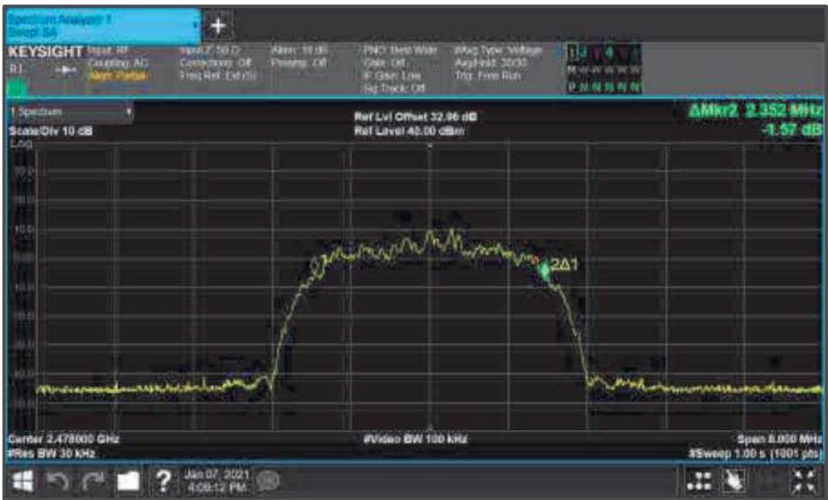
Figure 5 - Core0 (C) 2478 MHz (CH76) 99% Bandwidth
