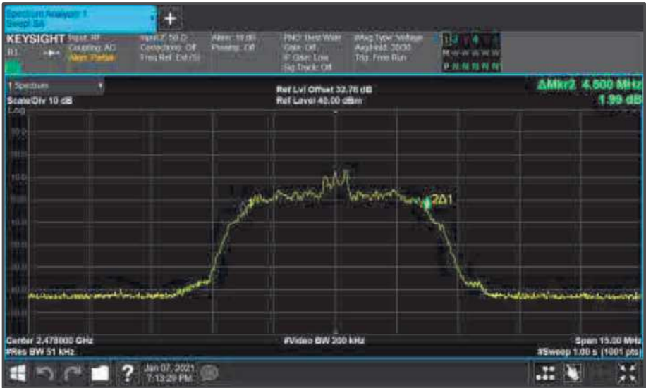
Figure 33 - Core1 (B) 2478 MHz (CH76) 99% Bandwidth
