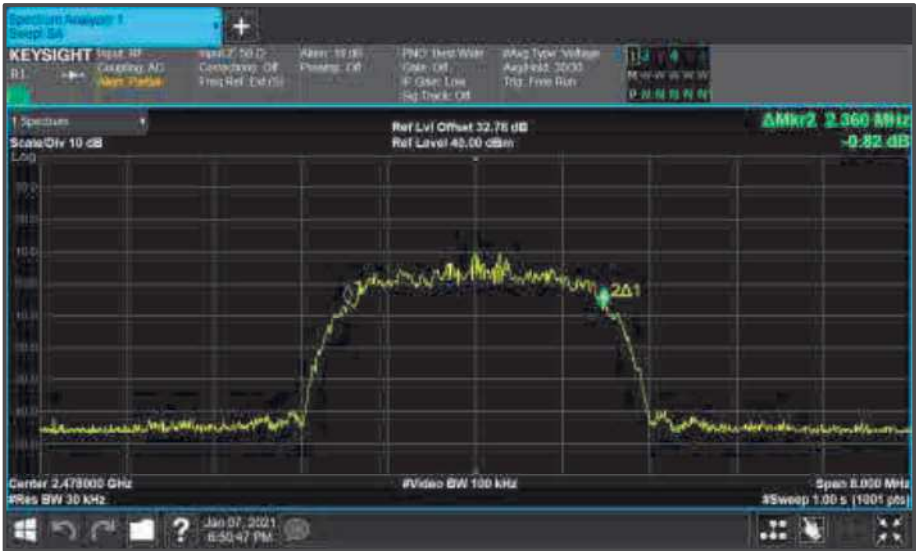
Figure 21 - Core1 (B) 2478 MHz (CH76) 99% Bandwidth
