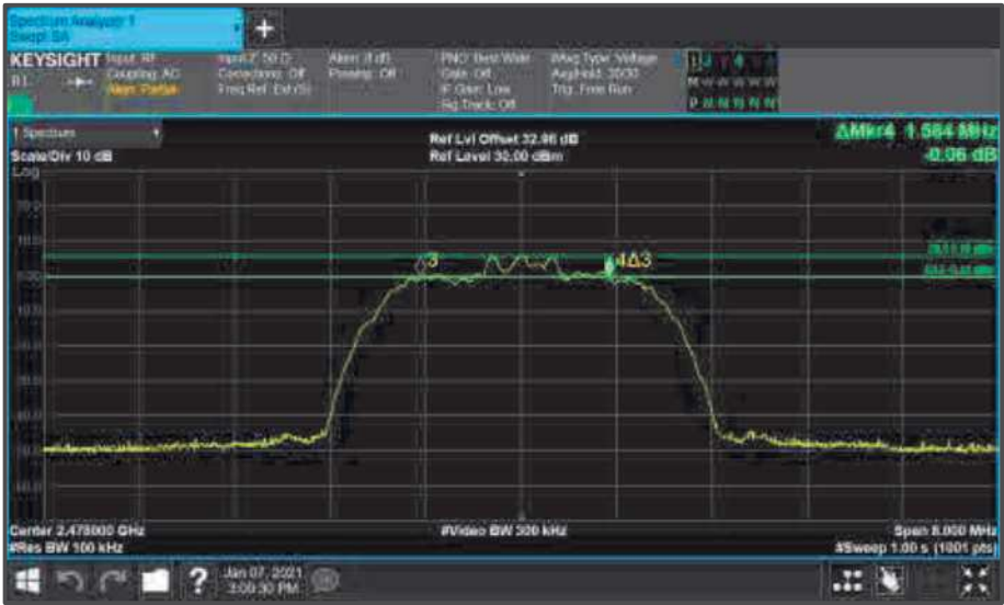
Figure 78 - Core2 (A) 2478 MHz (CH76) 6 dB Bandwidth
