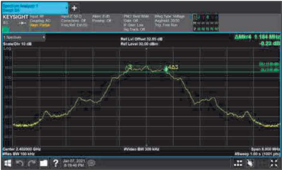
Figure 64 - Core0 (C) 2402 MHz (CH0) 6 dB Bandwidth
