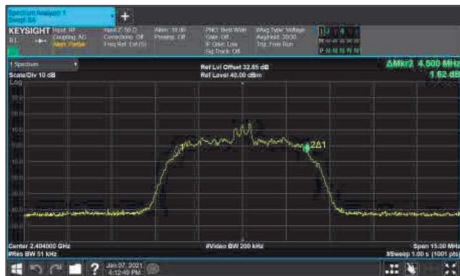
Figure 7 - Core0 (C) 2404 MHz (CH2) 99% Bandwidth
