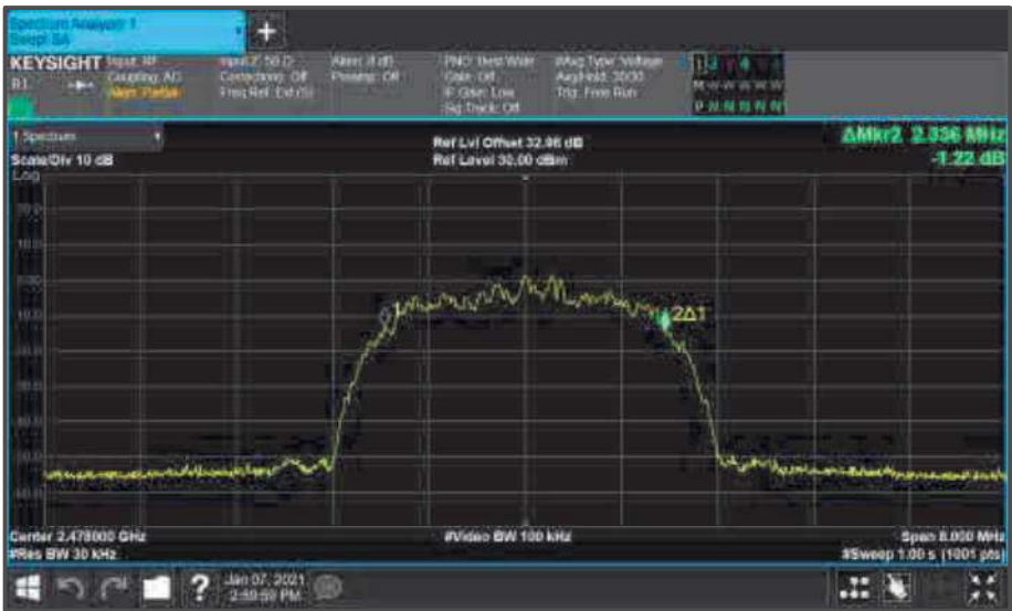
Figure 77 - Core2 (A) 2478 MHz (CH76) 99% Bandwidth
