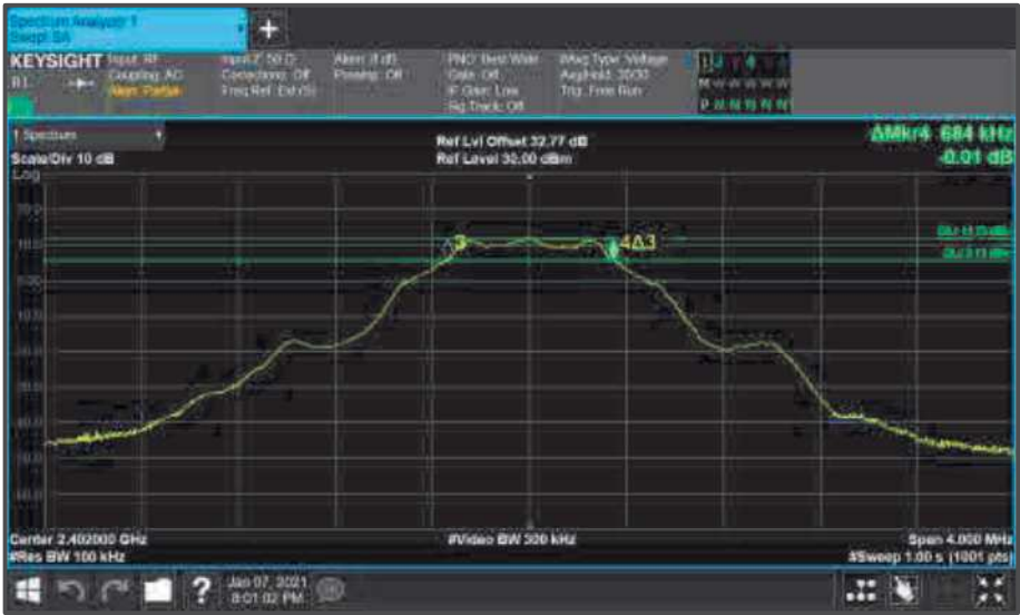
Figure 50 - Core1 (B) 2402 MHz (CH0) 6 dB Bandwidth
