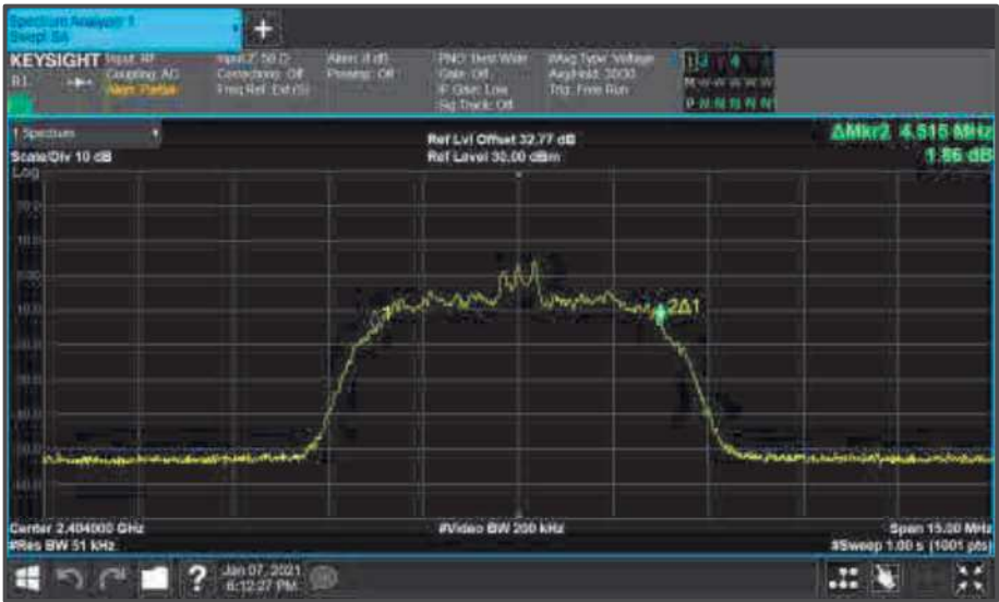
Figure 109 - Core1 (B) 2404 MHz (CH2) 99% Bandwidth
