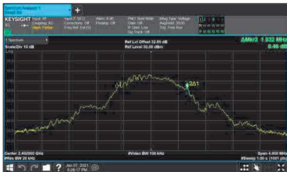
Figure 37 - Core0 (C) 2402 MHz (CH0) 99% Bandwidth
