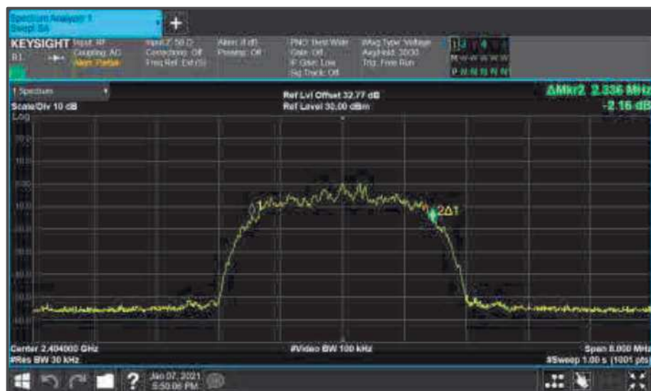
Figure 97 - Core1 (B) 2404 MHz (CH2) 99% Bandwidth
