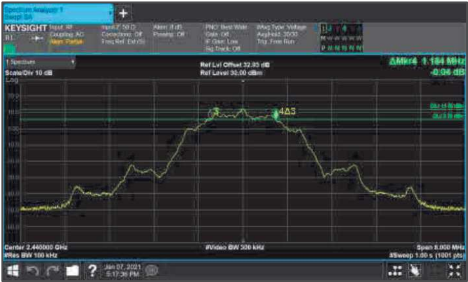
Figure 130 - Core2 (A) 2440 MHz (CH19) 6 dB Bandwidth
