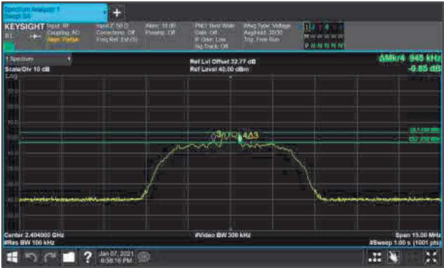
Figure 26 - Core1 (B) 2404 MHz (CH2) 6 dB Bandwidth
