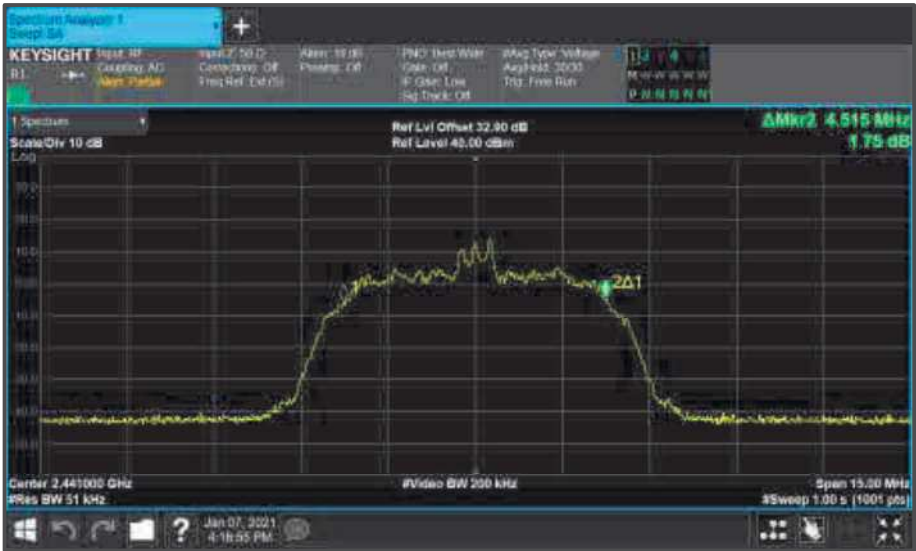
Figure 9 - Core0 (C) 2441 MHz (CH39) 99% Bandwidth
