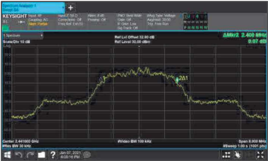
Figure 103 - Core0 (C) 2441 MHz (CH39) 99% Bandwidth
