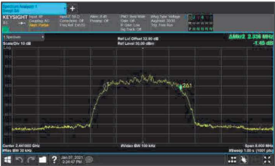
Figure 87 - Core0 (C) 2441 MHz (CH39) 99% Bandwidth
