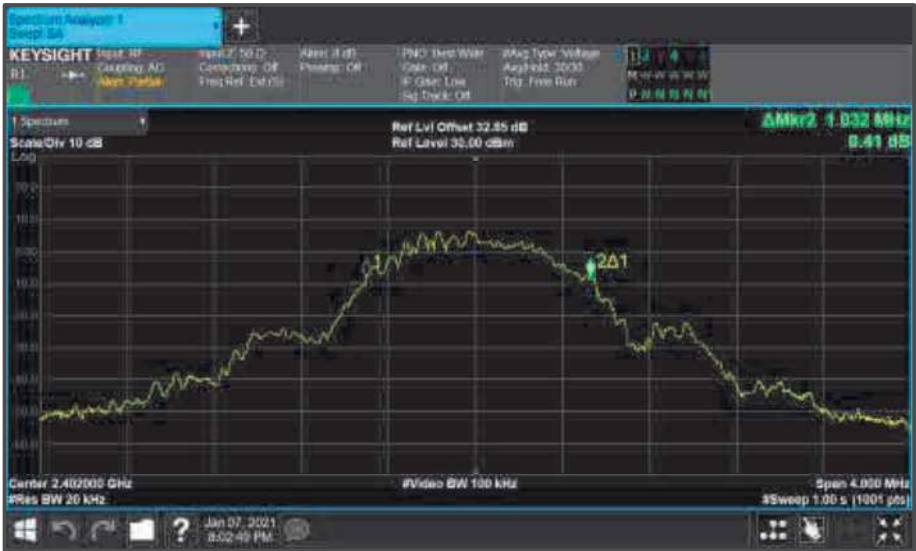
Figure 51 - Core0 (C) 2402 MHz (CH0) 99% Bandwidth
