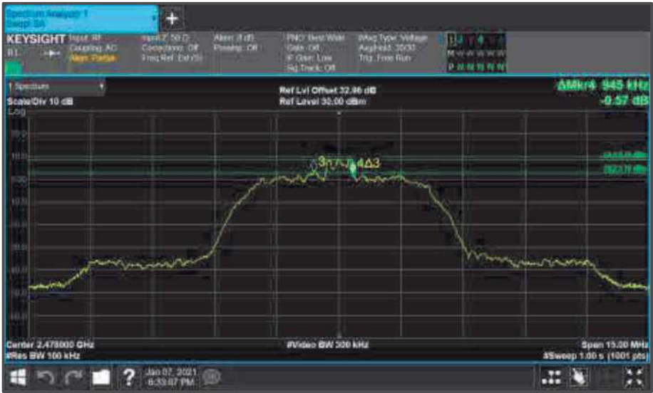
Figure 120 - Core0 (C) 2478 MHz (CH76) 6 dB Bandwidth
