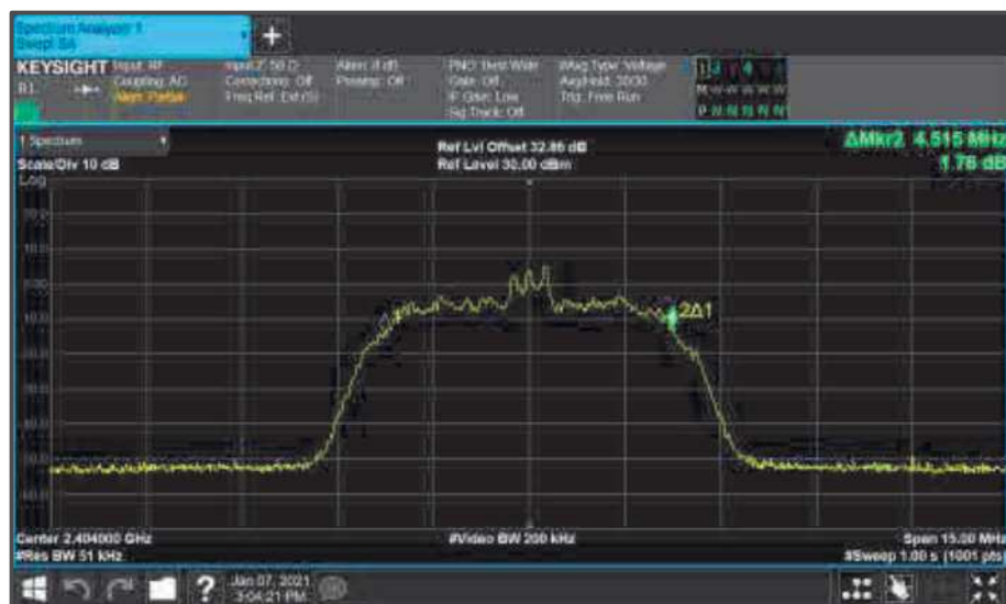
Figure 79 - Core2 (A) 2404 MHz (CH2) 99% Bandwidth
