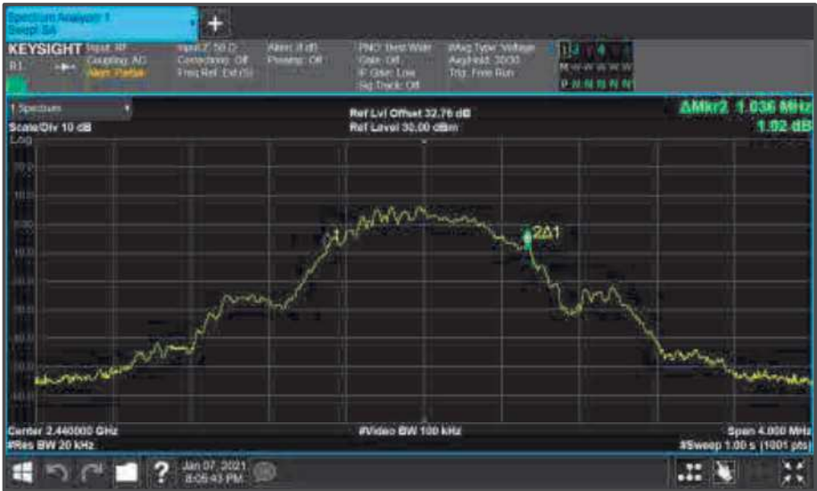
Figure 53 - Core1 (B) 2440 MHz (CH19) 99% Bandwidth
