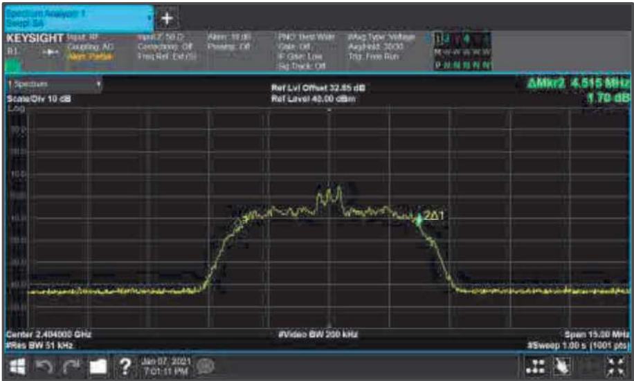
Figure 27 - Core0 (C) 2404 MHz (CH2) 99% Bandwidth
