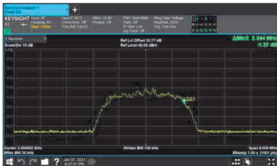
Figure 13 - Core1 (B) 2404 MHz (CH2) 99% Bandwidth
