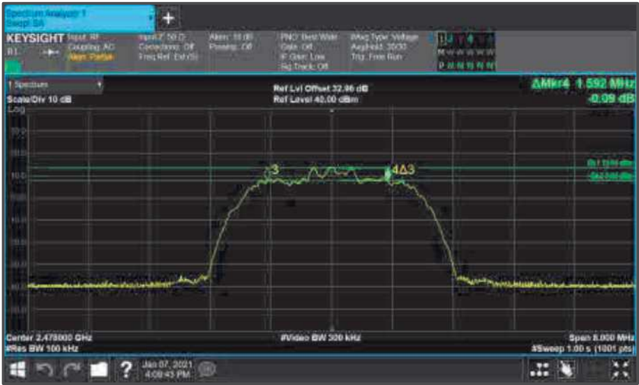
Figure 6 - Core0 (C) 2478 MHz (CH76) 6 dB Bandwidth
