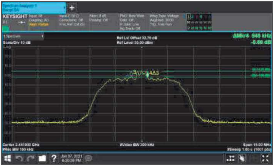
Figure 114 - Core1 (B) 2441 MHz (CH39) 6 dB Bandwidth
