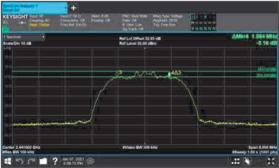
Figure 76 - Core2 (A) 2441 MHz (CH39) 6 dB Bandwidth
