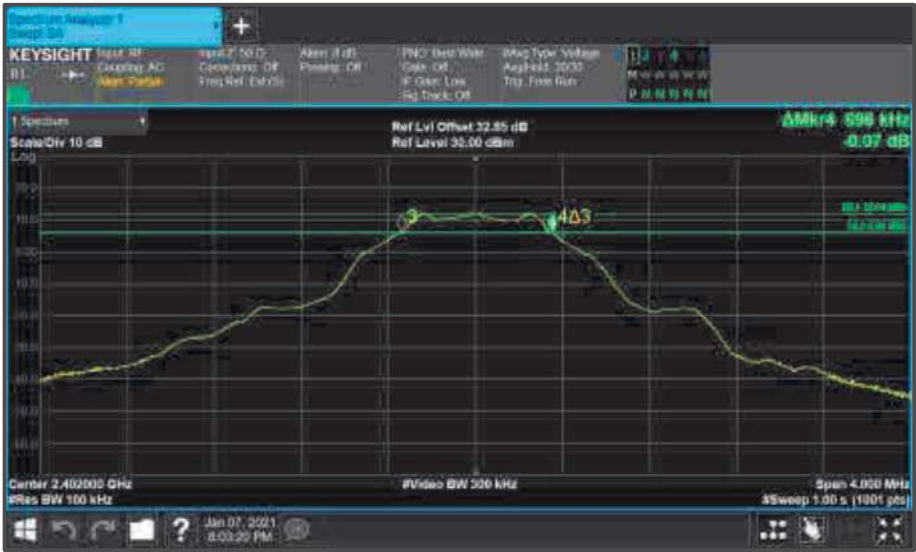
Figure 52 - Core0 (C) 2402 MHz (CH0) 6 dB Bandwidth
