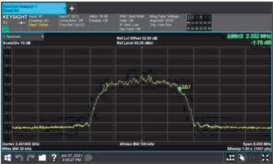
Figure 3 - Core0 (C) 2441 MHz (CH39) 99% Bandwidth
