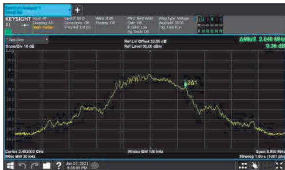
Figure 43 - Core0 (C) 2402 MHz (CH0) 99% Bandwidth
