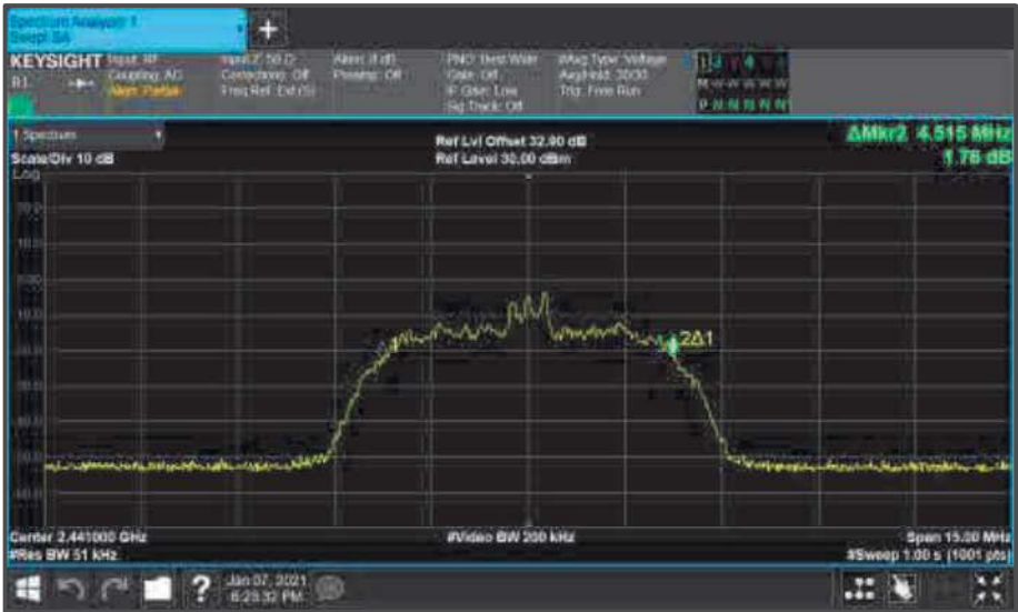
Figure 115 - Core0 (C) 2441 MHz (CH39) 99% Bandwidth
