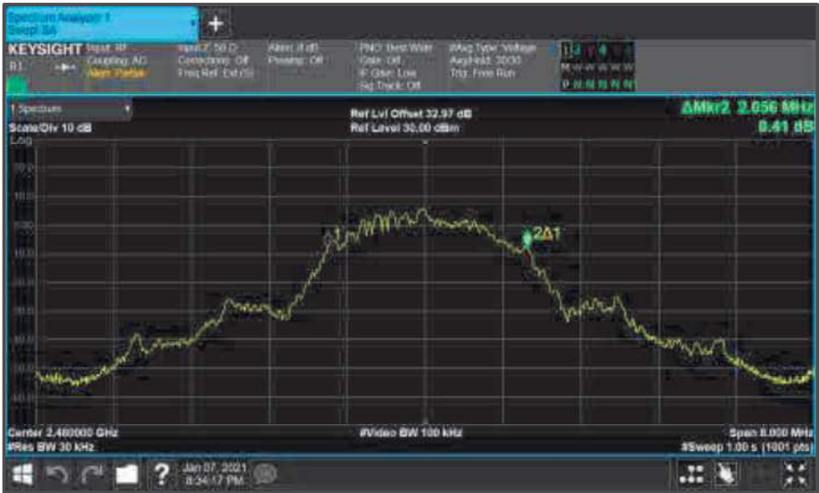
Figure 71 - Core0 (C) 2480 MHz (CH39) 99% Bandwidth
