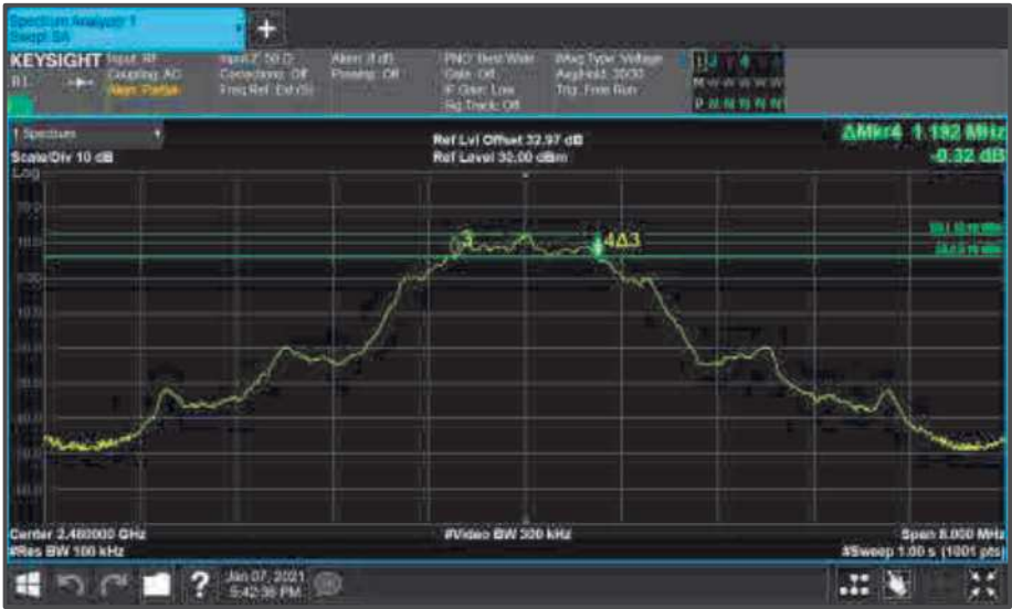
Figure 48 - Core0 (C) 2480 MHz (CH39) 6 dB Bandwidth
