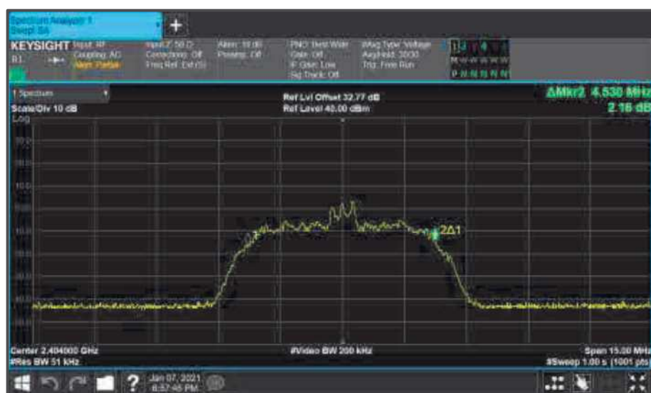
Figure 25 - Core1 (B) 2404 MHz (CH2) 99% Bandwidth
