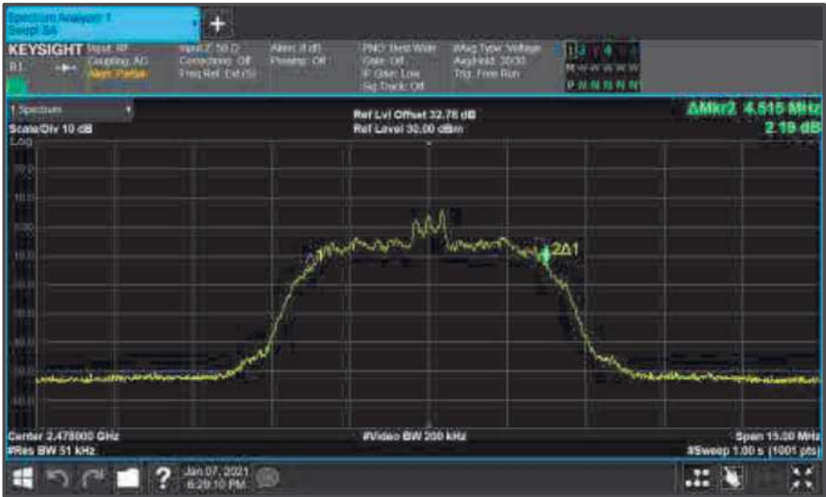
Figure 117 - Core1 (B) 2478 MHz (CH76) 99% Bandwidth
