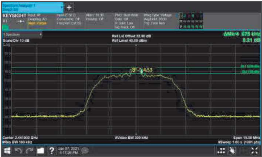
Figure 10 - Core0 (C) 2441 MHz (CH39) 6 dB Bandwidth
