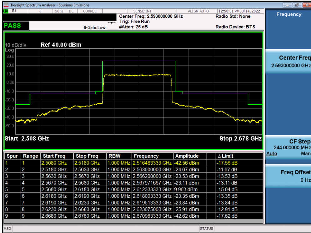
Plot 7-282. Middle ACP Plot (NR Band n41 - 50MHz DFT-s-OFDM \pi/2 BPSK - Full RB)
