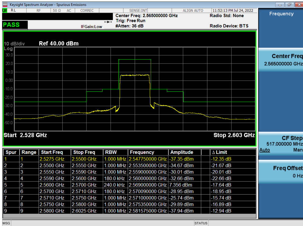
Plot 7-224. Upper ACP Plot (LTE Band 7 - 10MHz QPSK – Full RB)
