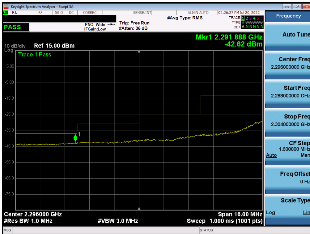
Plot 7-244. Extended Lower Band Edge Plot (NR Band n30 - 5MHz DFT-s-OFDM QPSK – Full RB)
