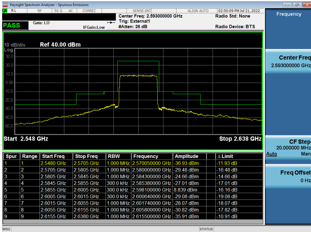
Plot 7-238. Middle ACP Plot (LTE Band 41 - 15MHz QPSK – Full RB)
