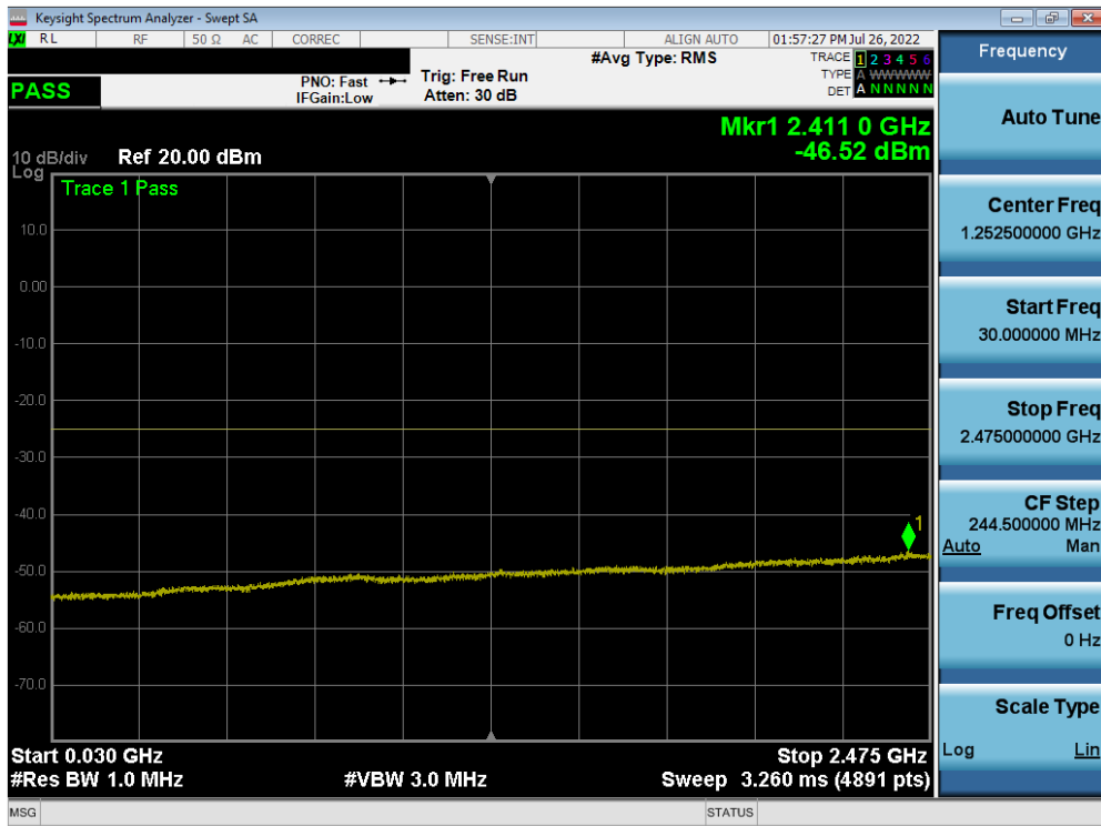
Plot 7-193. Conducted Spurious Plot (ULCA LTE B7 – (20+20)MHz QPSK - RB Size 1, RB Offset 0 - Low Channel)
