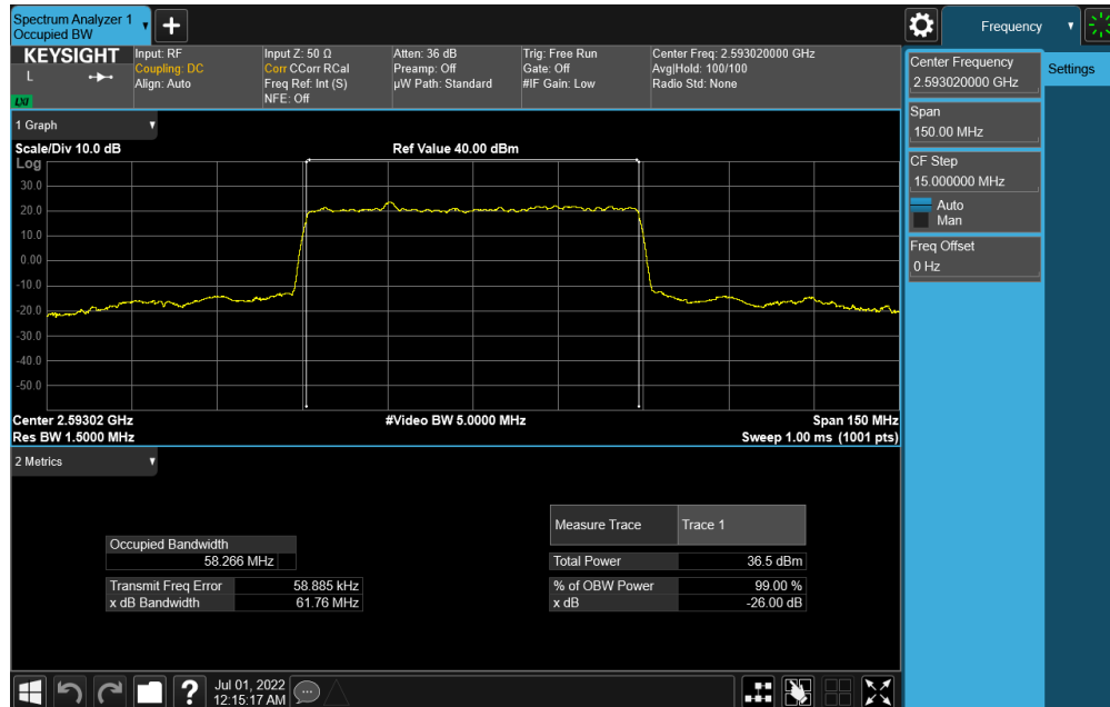
Plot 7-106. Occupied Bandwidth Plot (NR Band n41 - 60MHz DFT-s-OFDM \pi/2 BPSK - Full RB)
