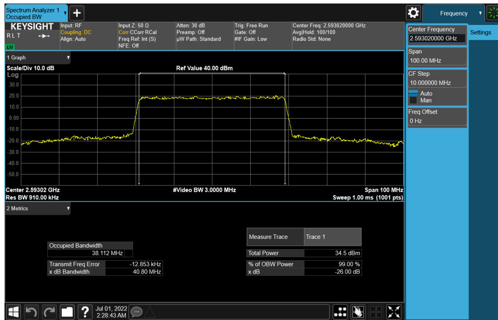
Plot 7-97. Occupied Bandwidth Plot (NR Band n41 - 40MHz CP-OFDM QPSK - Full RB)
