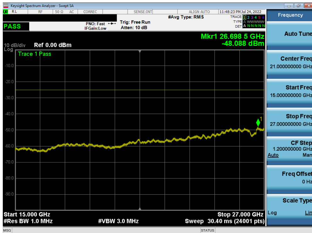
Plot 7-156. Conducted Spurious Plot (LTE Band 7 - 20MHz QPSK - RB Size 1, RB Offset 0 - High Channel)
