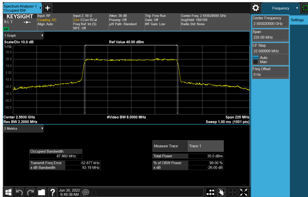
Plot 7-123. Occupied Bandwidth Plot (NR Band n41 - 90MHz CP-OFDM 16-QAM - Full RB)
