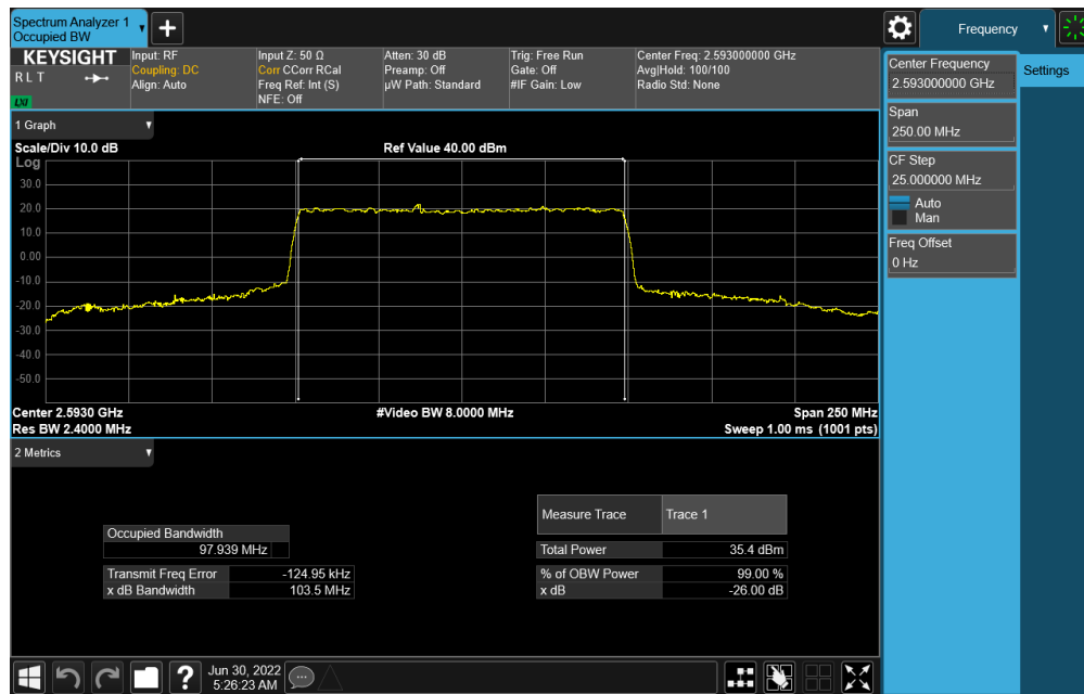
Plot 7-127. Occupied Bandwidth Plot (NR Band n41 - 100MHz CP-OFDM QPSK - Full RB)
