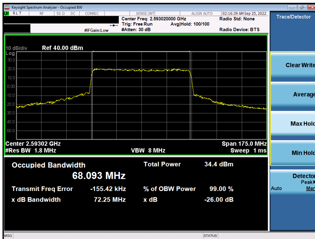
Plot 7-113. Occupied Bandwidth Plot (NR Band n41 - 70MHz DFT-s-OFDM 16-QAM - Full RB)
