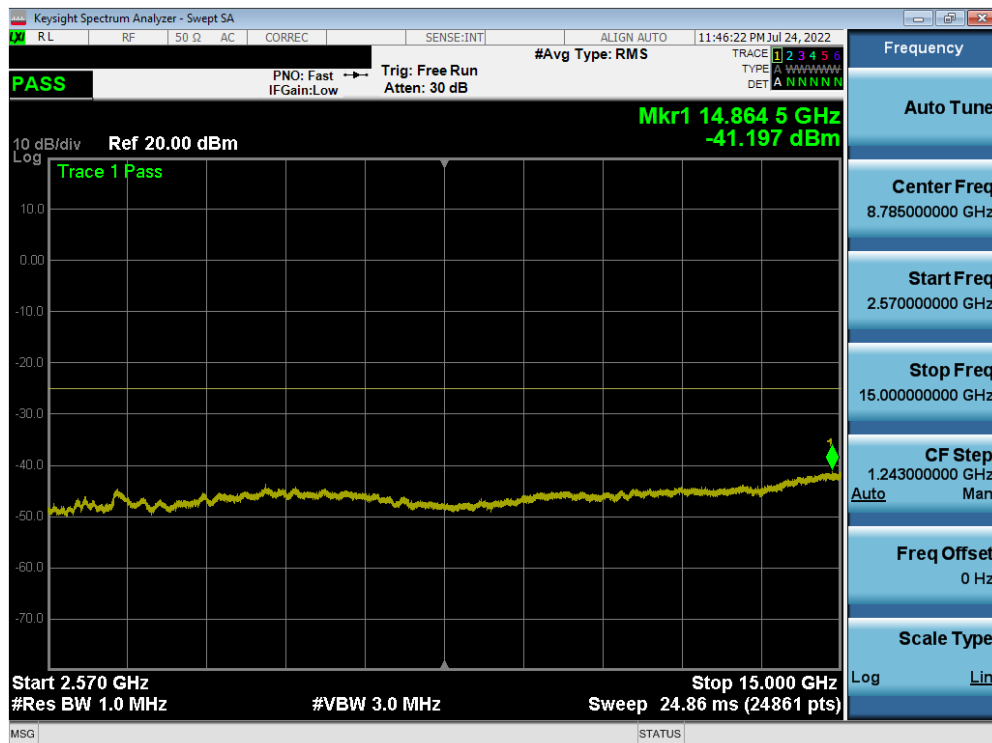
Plot 7-149. Conducted Spurious Plot (LTE Band 7 - 20MHz QPSK - RB Size 1, RB Offset 0 - Low Channel)
