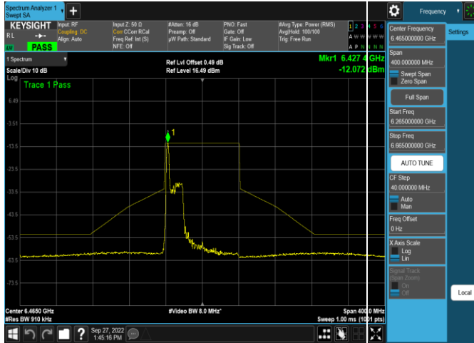
Plot 7-561. In-Band Emission Plot SDM Antenna 5b (80MHz 802.11ax RU26 (UNII Band 6) – Ch. 103)
