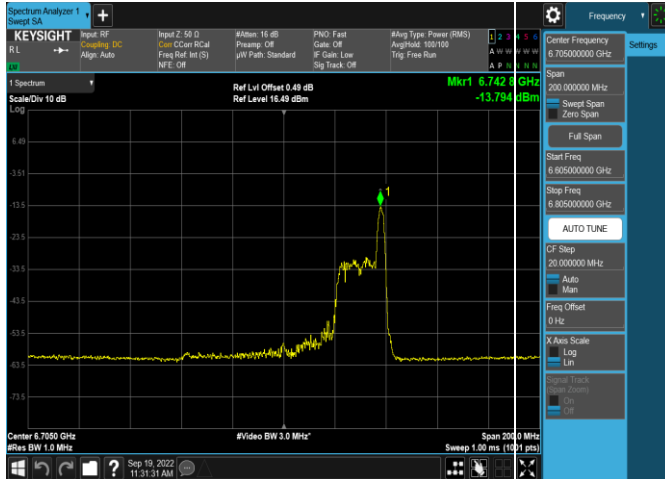
Plot 7-341. Power Spectral Density Plot SDM Antenna 5b (80MHz 802.11ax RU26 (UNII Band 7) – Ch. 151)
