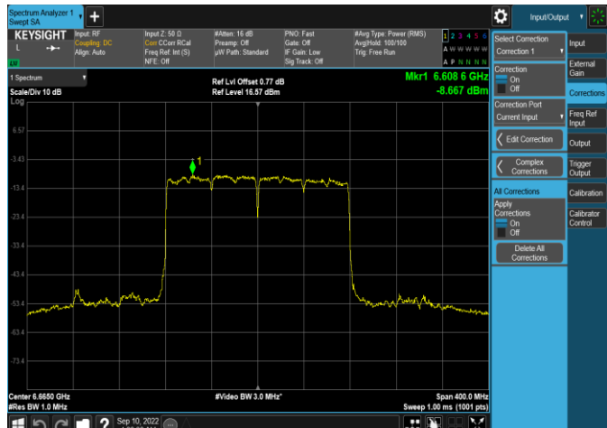
Plot 7-352. Power Spectral Density Plot SDM Antenna 4a (160MHz 802.11ax RU996x2 (UNII Band 7) – Ch. 143)
