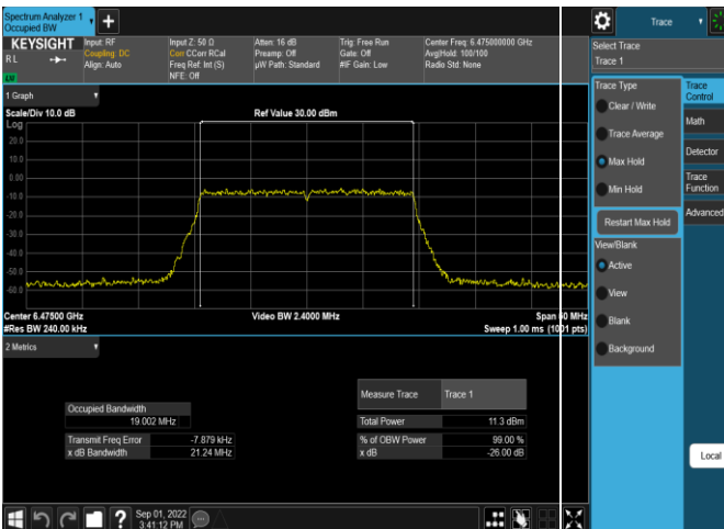
Plot 7-20. 26dB & 99% Bandwidth Plot Antenna 5b (20MHz 802.11ax RU242 (UNII Band 6) – Ch. 105)
