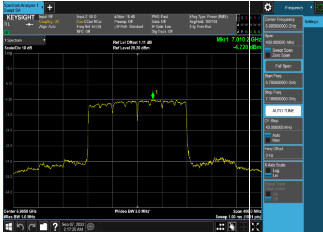
Plot 7-343. Power Spectral Density Plot SDM Antenna 5b (160MHz 802.11ax (UNII Band 8) – Ch. 207, MCS11)
