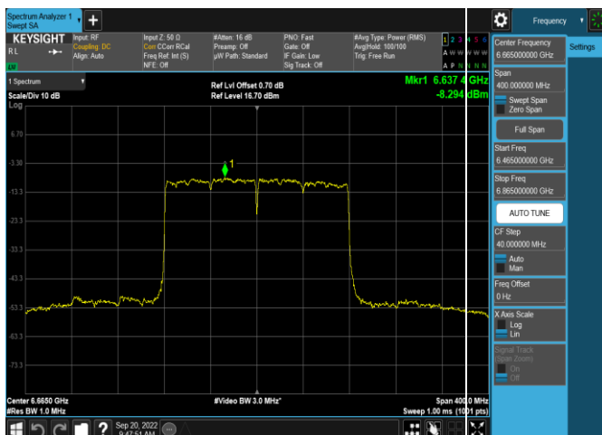
Plot 7-199. Power Spectral Density Plot Antenna 4a (160MHz 802.11ax (UNII Band 7) – Ch. 143, MCS2)
